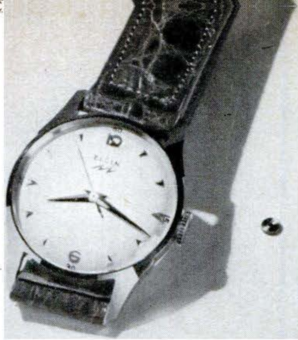
trated by experimental field coil for it (right), wound with 3,000 turns of insulated copper wire only 1/6 as thick as human hair.
