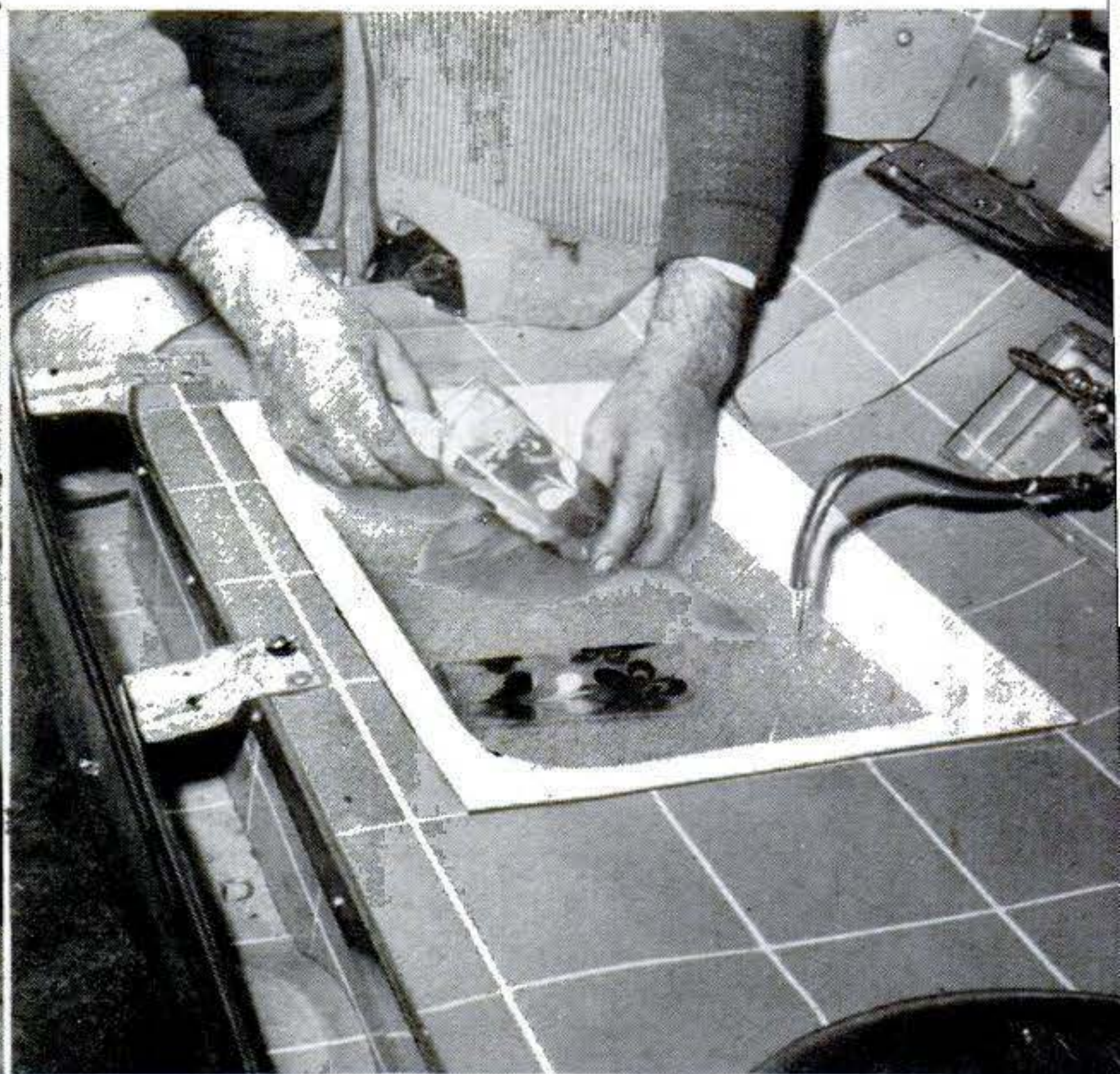
KITCHEN SINK big enough to do dinner dishes has running hot water and is surrounded by linoleum tile. It's hidden away beneath right-hand side of rear-seat cushion.
