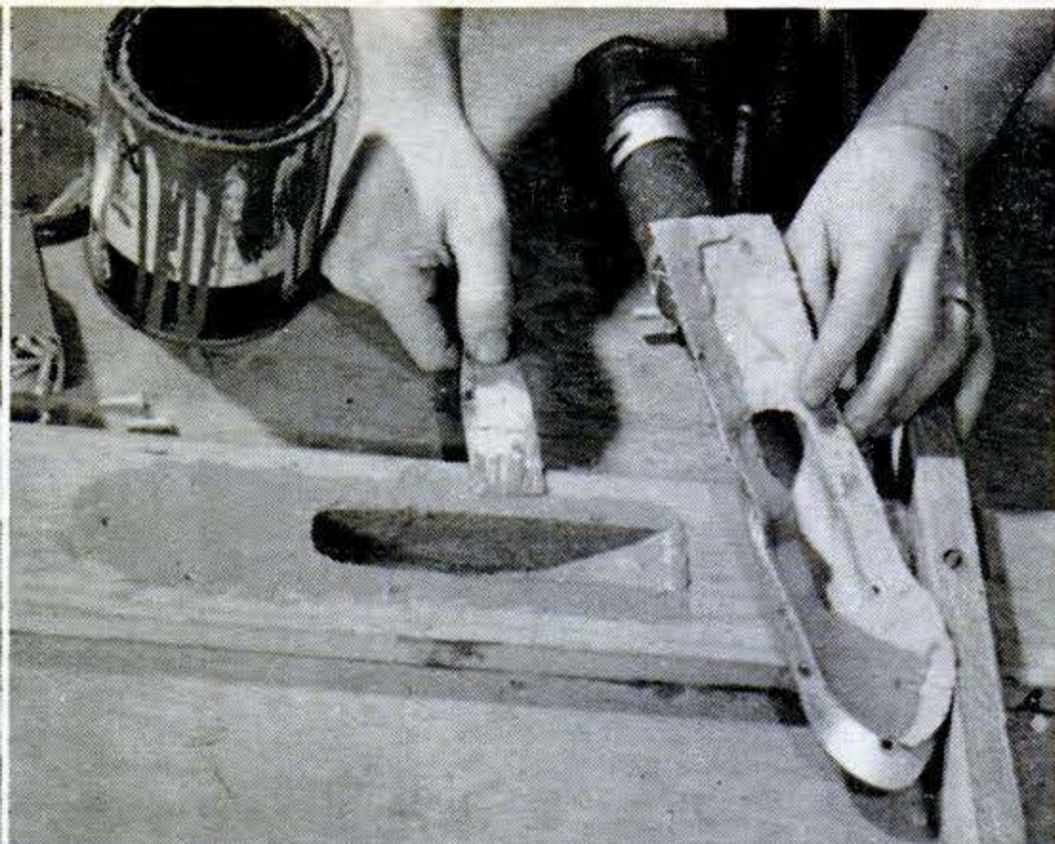
16 SHAFT-LOG SEAL. Cut canvas gasket for shaft log and soak gasket in paint. Smear thick marine paint around opening before screwing down log. Don't overtighten screws.
