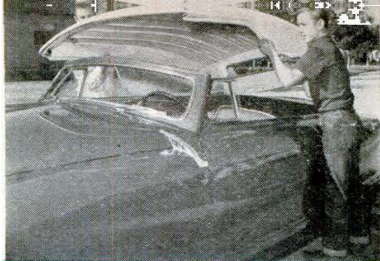
IN THREE MINUTES , hard top can be removed from remodeled Rambler. After unsnapping fasteners, the brothers lift off 200-pound top as above.
