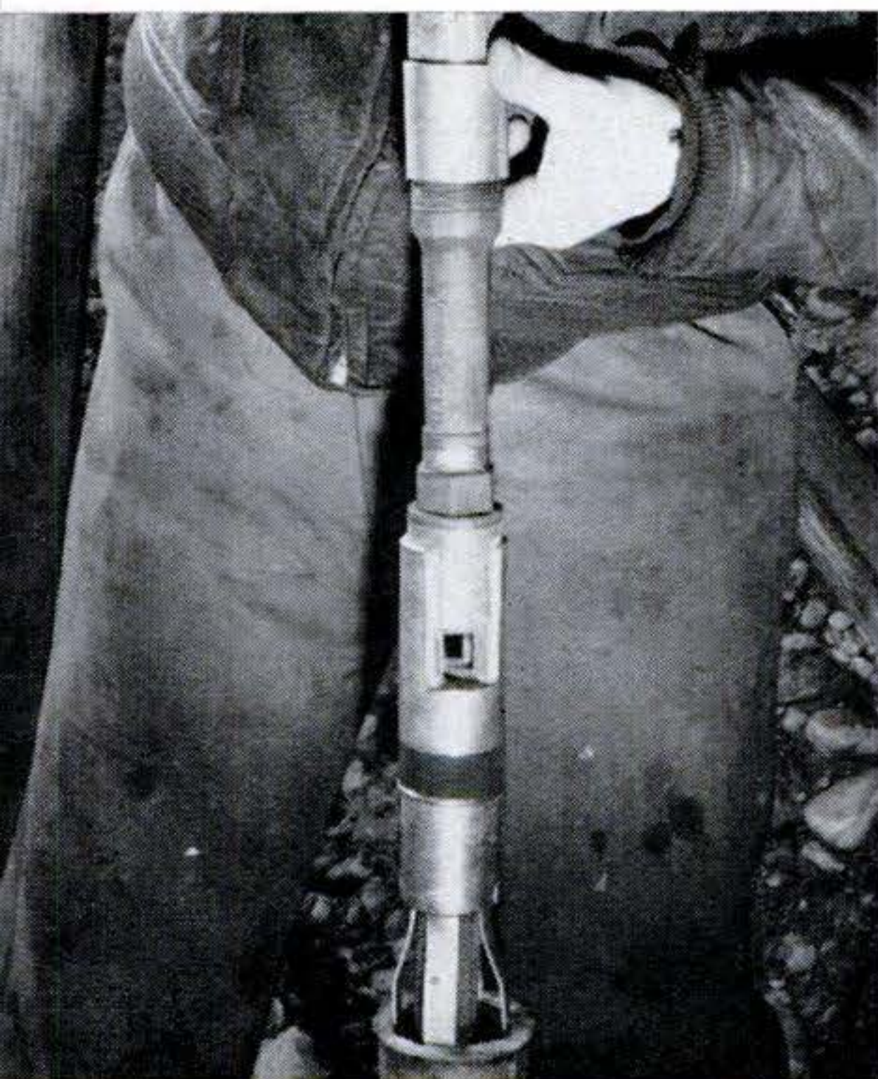
6. PACKER-TYPE JET and foot valve at bottom of suction pipe were also needed. If casing is larger than 2", a two-pipe jet can be used. Without room for two pipes, space between casing and suction pipe serves as a pressure pipe.
