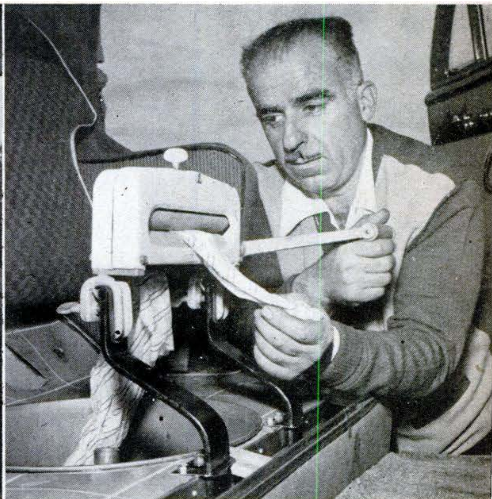
WASHING MACHINE , beneath left-hand side of rear-seat cushion, has tiny homemade wringer cut down from a standard model. Lid of "home laundry" contains electric power unit.
