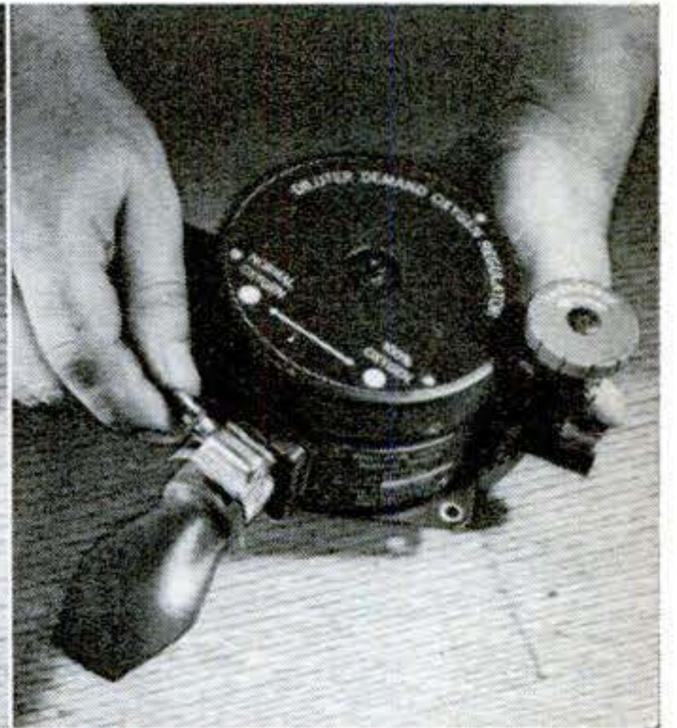
13 Slip flutter valve over heater fitting and clamp with screw-type hose clamp. Rubber noisemaker can be used as flutter valve.
