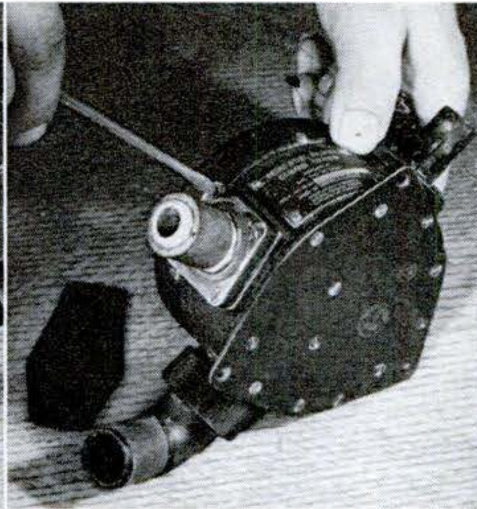
12 Screw flange back in original position and force short length of auto-heater hose over heater fitting. Grease all screws.
