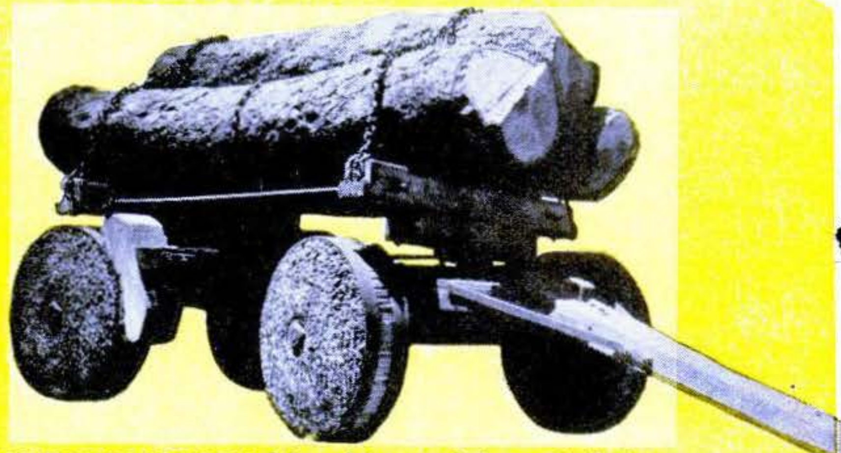
LOGGING WAGON like this model carried timber out of the thick forests of the Pacific Northwest in frontier days. Oak pegs were pounded into the wheels for strength.
