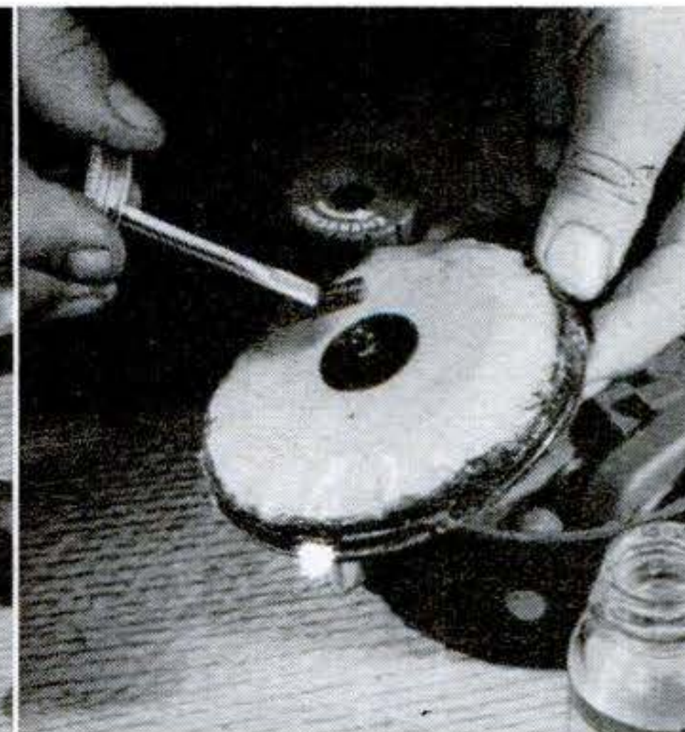
18 Waterproof diaphragm with several coats of rubber cement. Dust final coat with talcum to prevent it from sticking to cover.
