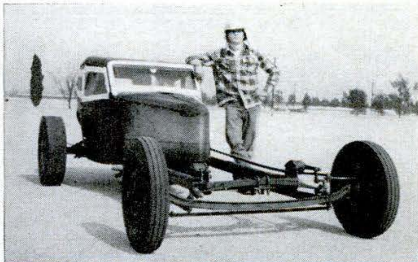
MODIFIED RAILSTER run by Bob Gorman has Austin body and G-string hood for safety if 1,565-lb. car capsizes or engine blows up. Car has hit 121 m.p.h.
