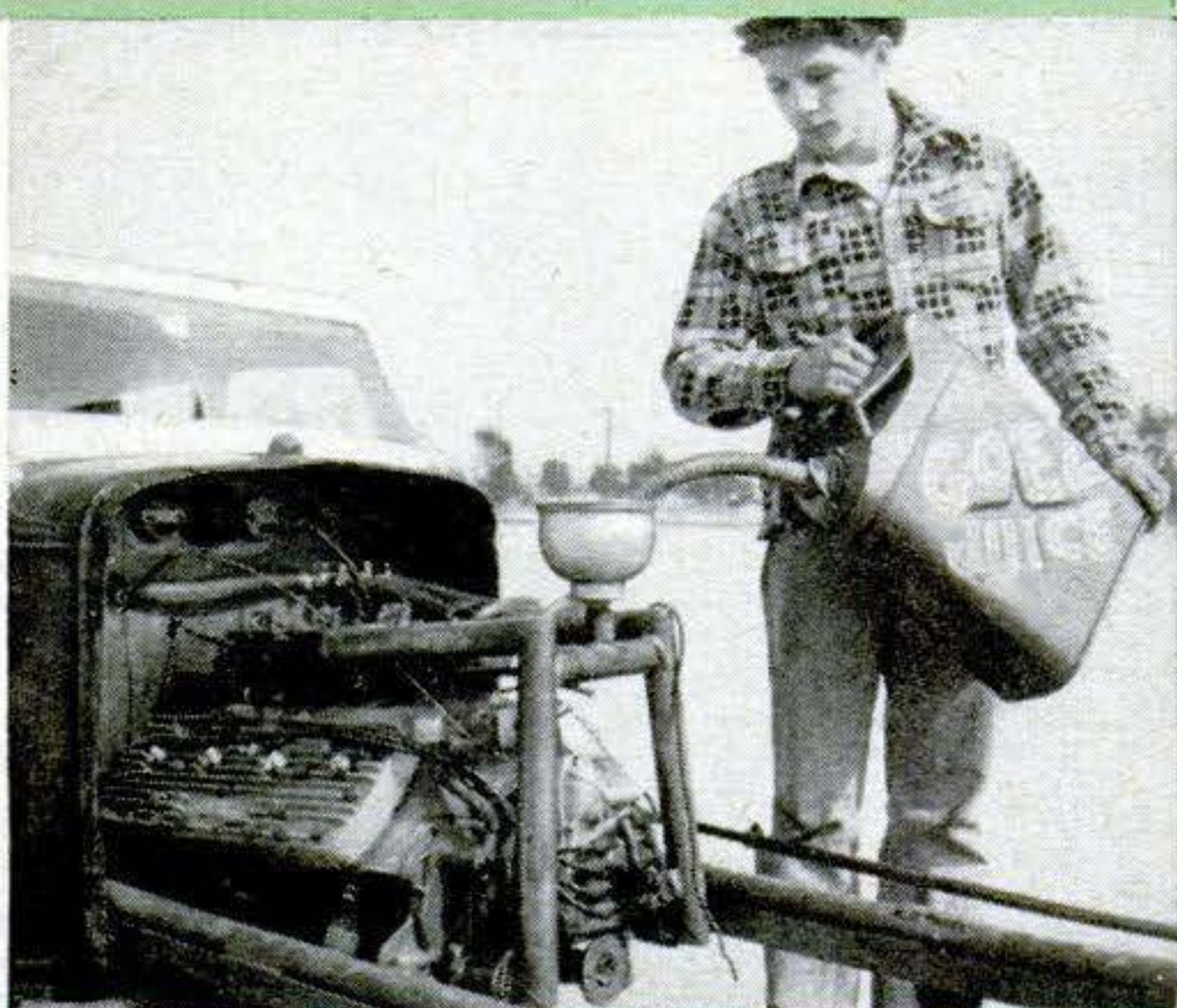
FOUR GALLONS of water are poured into tubes connecting two sides of engine block. Radiators are not used. Some engines slant toward rear for traction.
