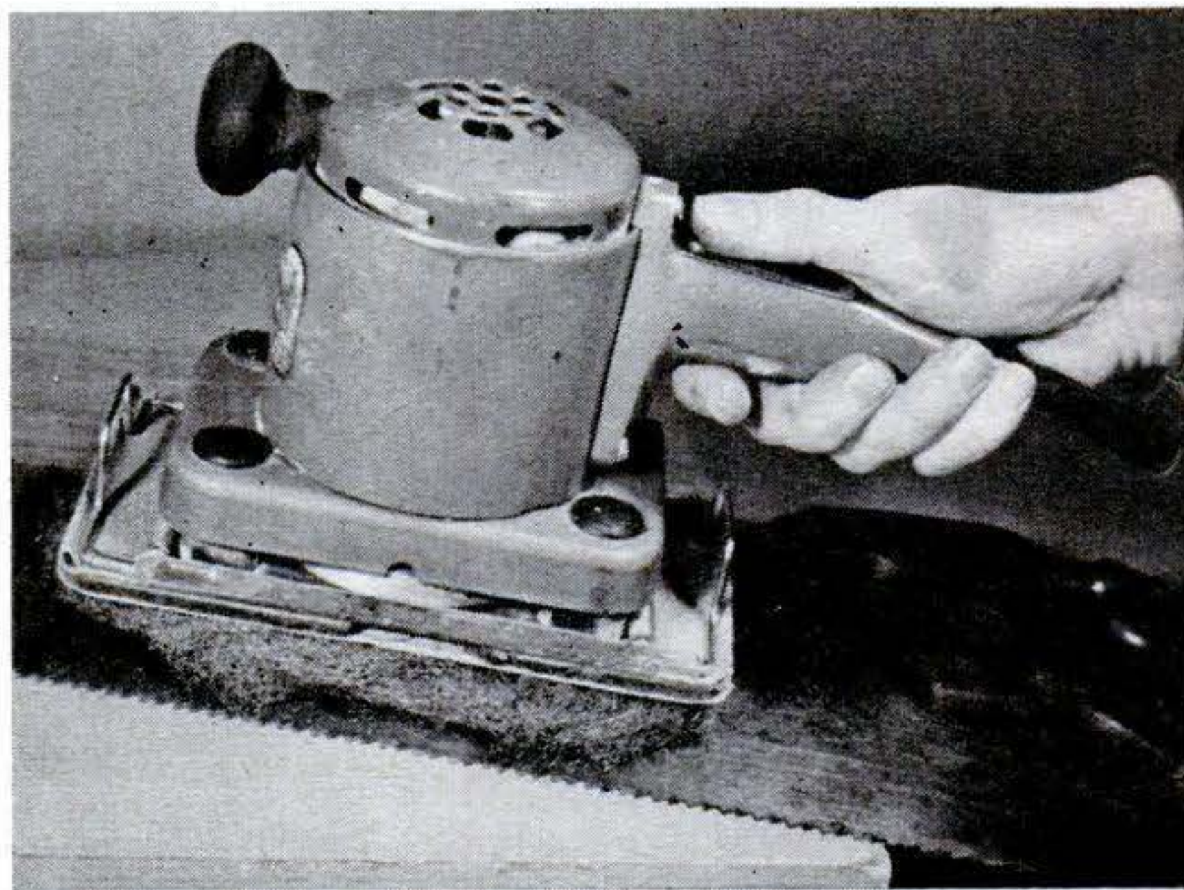
TO REMOVE RUST , apply satin finish to lacquered surfaces or smooth shellac between coats, drive steel-wool with coarse sandpaper.
