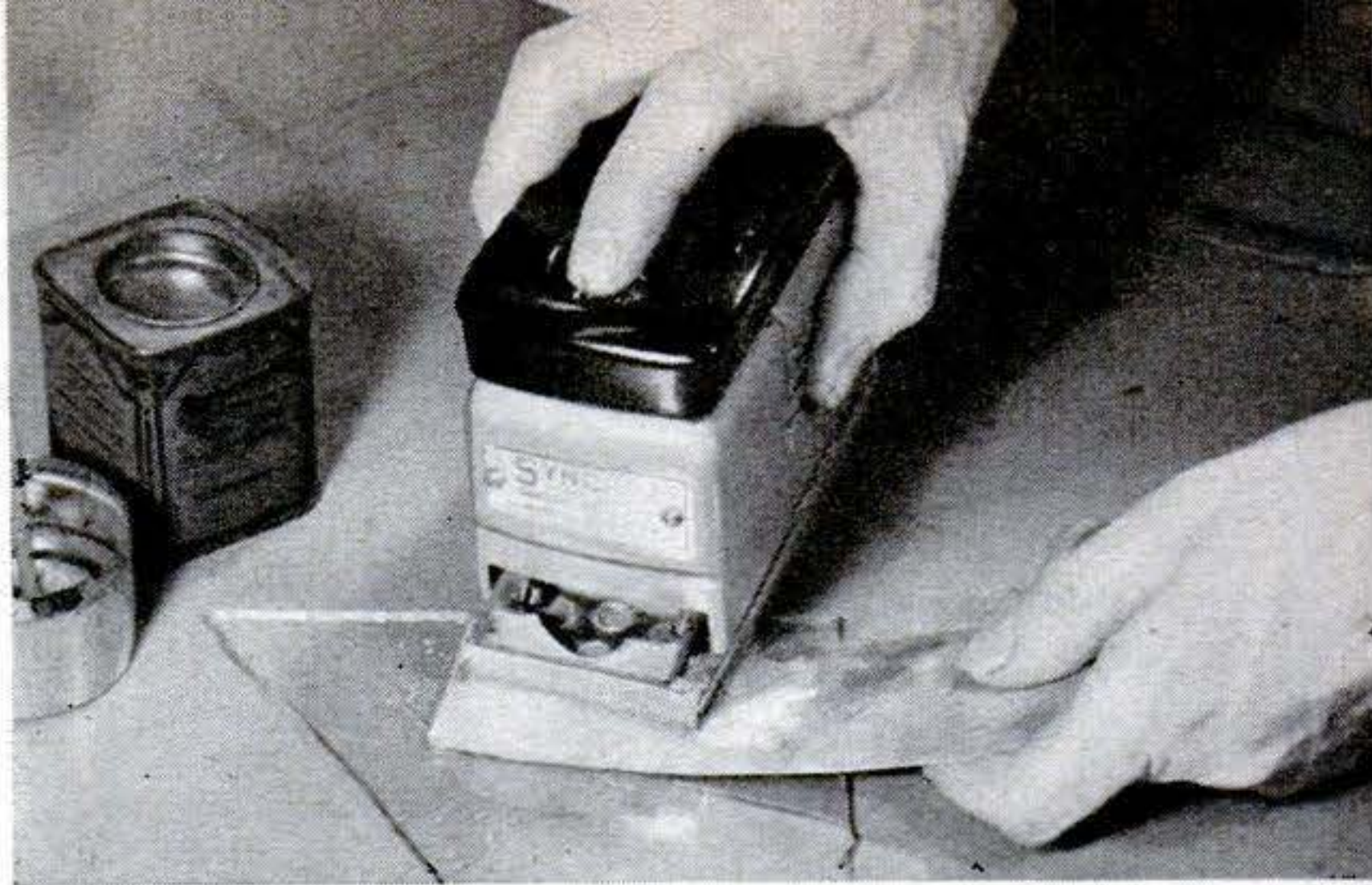
ETCHING GROUND GLASS for camera. Strip of sheet metal is agitated by sander over glass covered with oil-moistened valve-grinding compound or abrasive grit.
