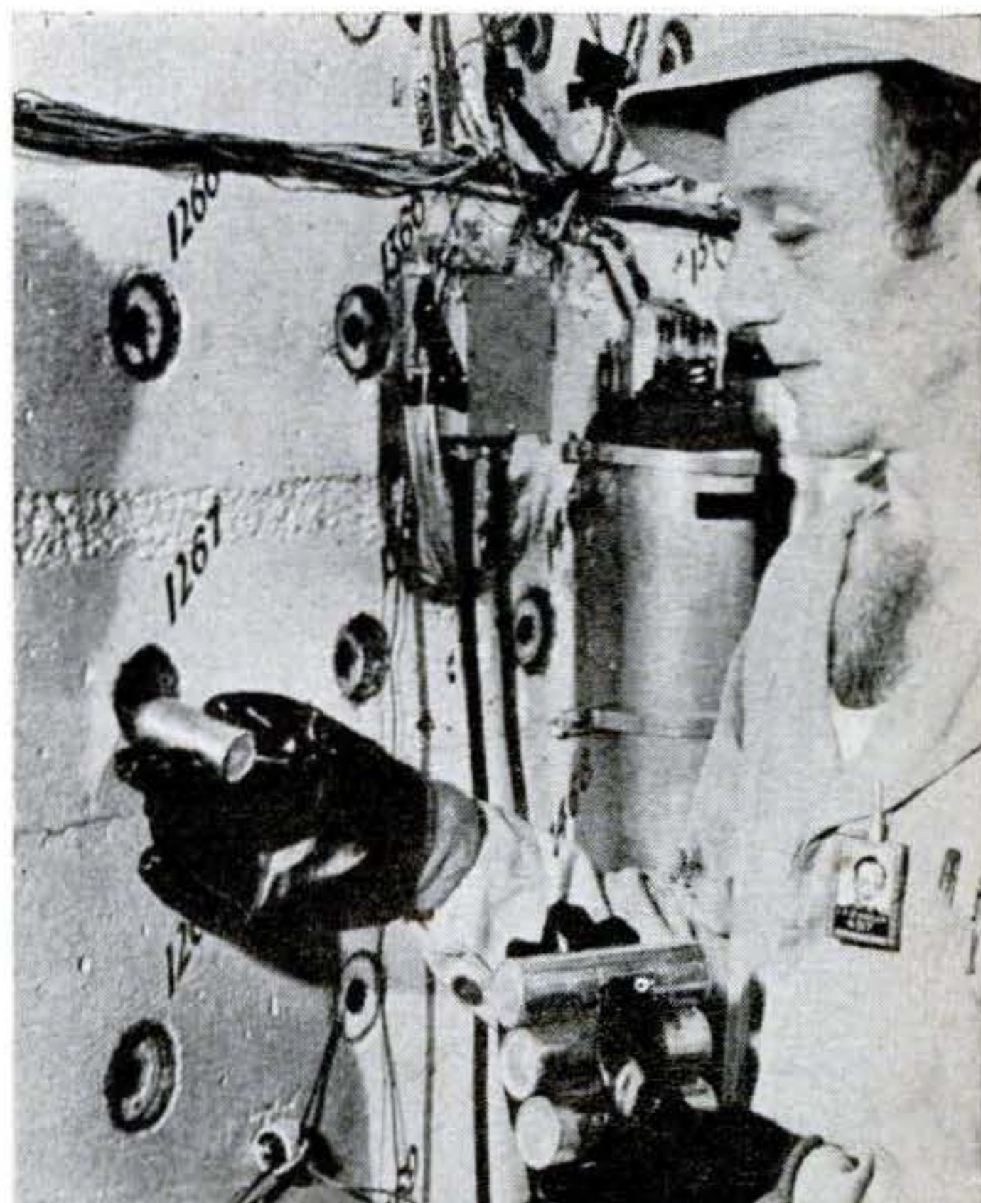
“SLUGS” OF URANIUM from mill, in aluminum cans, will fuel atomic piles as above.
