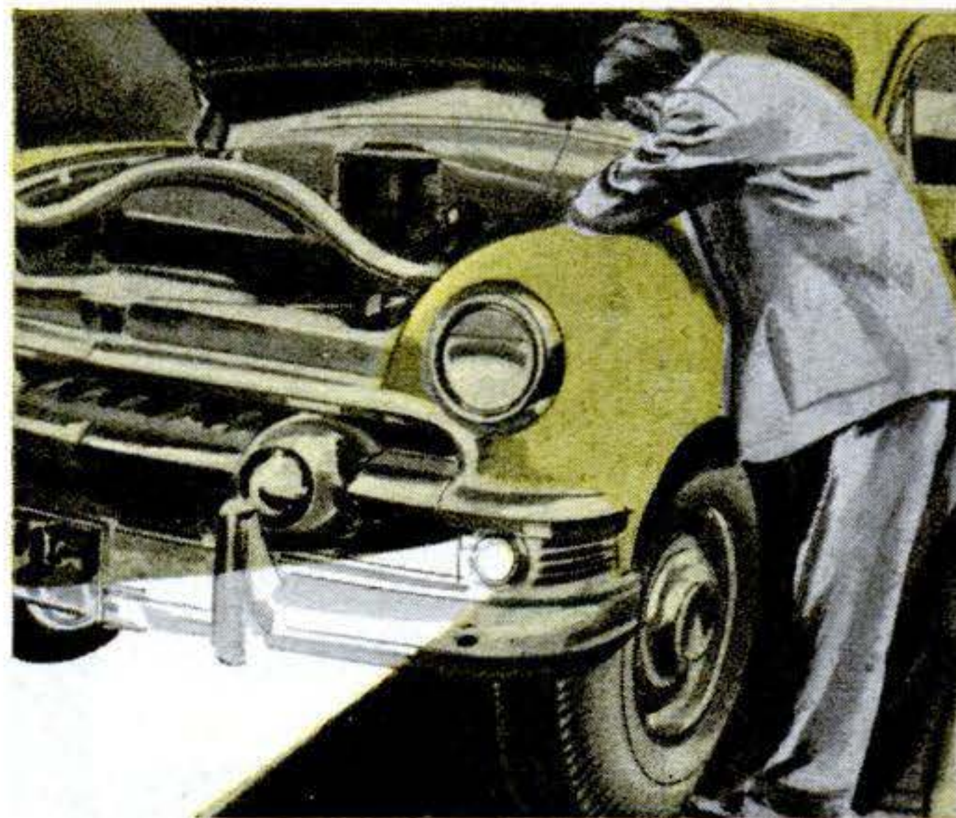
A LOW-WATT HEADLAMP wired across the fuse terminal of a car. It would give some light if a fuse blew during a night drive.— S. Ramya, Panadure, Ceylon.
