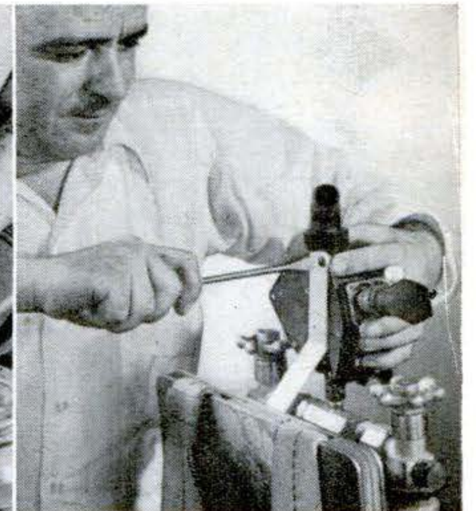
19 Mount regulator on tank connector and brace it with aluminum strip. Use 1/8" pipe nipple to join regulator to connector.
