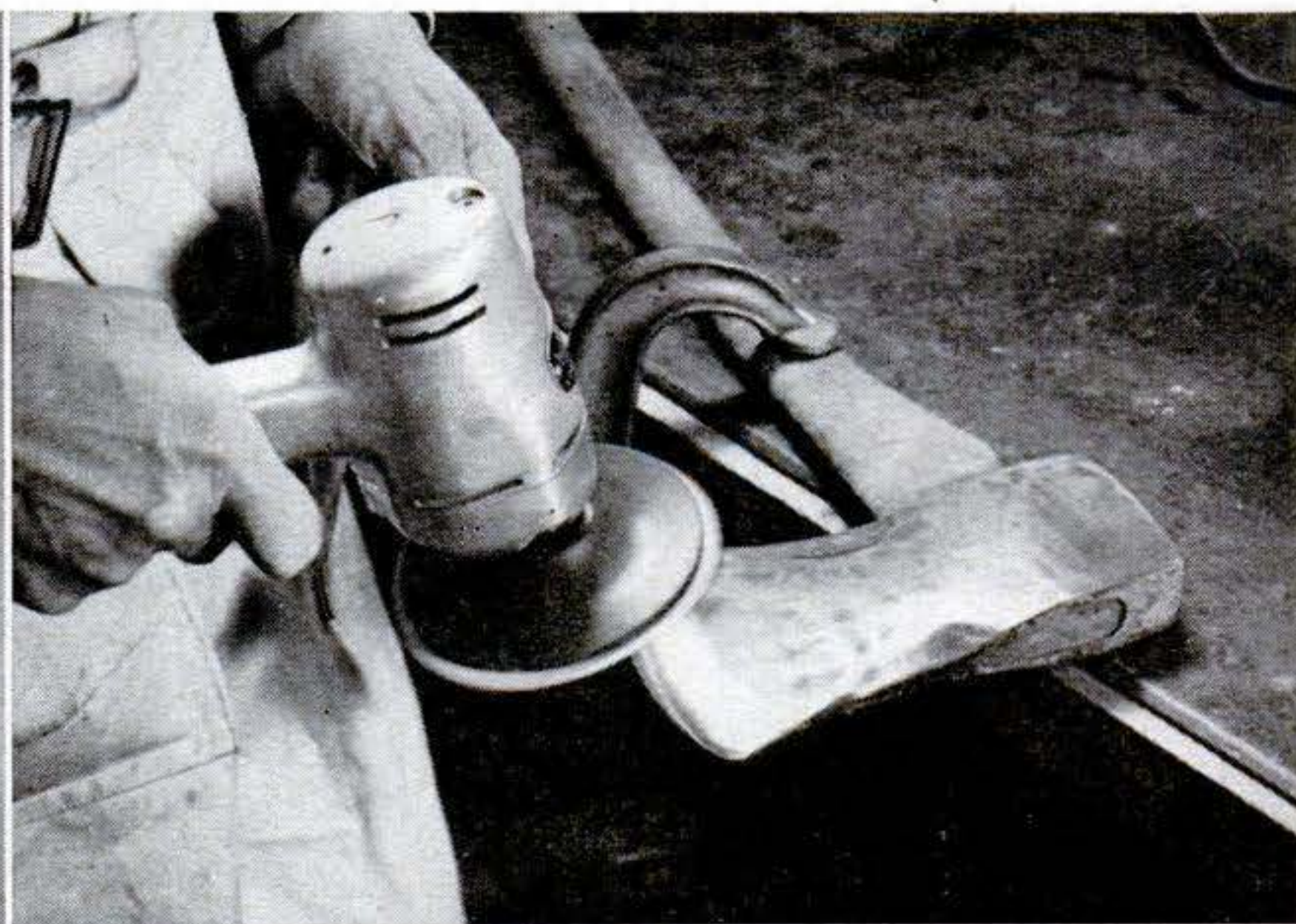
AX EDGE is restored with disk sander. Coarse abrasive disk is used to remove nicks, fine disk to produce sharp edge, extra fine disk to brighten ax head.
