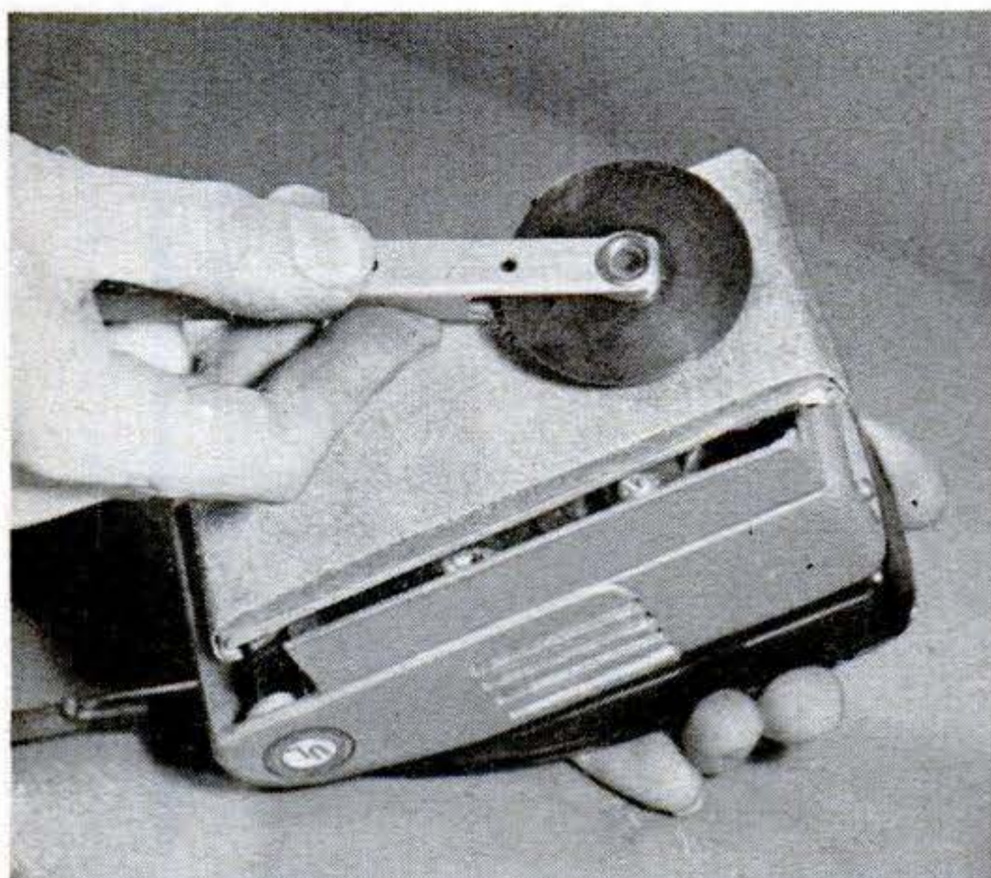
CIRCULAR KNIFE is quickly given new edge by holding it against sheet of metal-cutting abrasive mounted on sander shoe. Knife rotates as it is sharpened.
