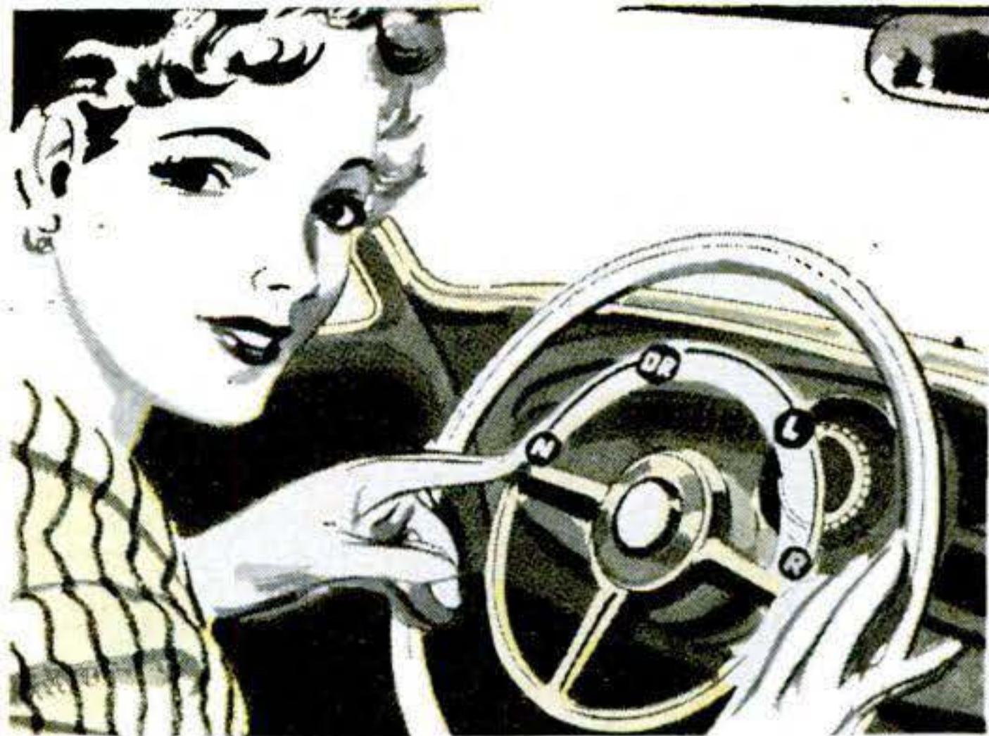
SELECTOR BUTTONS for drive, low, park and reverse mounted on a steering-column horn ring in cars with automatic transmissions.— D. W. Taber, Marietta, Ohio.
