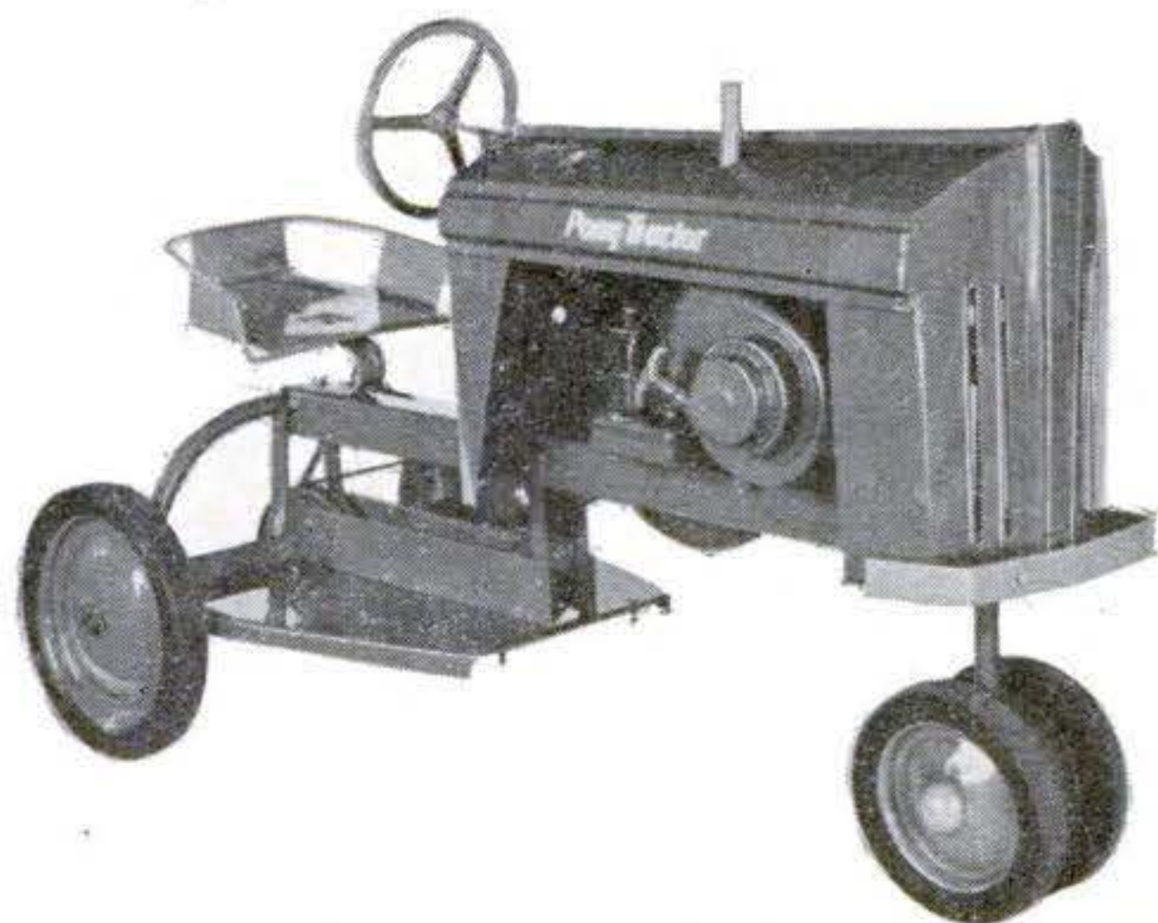
BABY TRACTOR is so simple a child can drive it, yet it will haul up to 500-lb. loads and hit 6 m.p.h. Available with a trailer cart to handle light earth-moving chores, the Norbel Pony Tractor can also be hooked up to a mower, a lawn roller or a wagon train full of kids.
