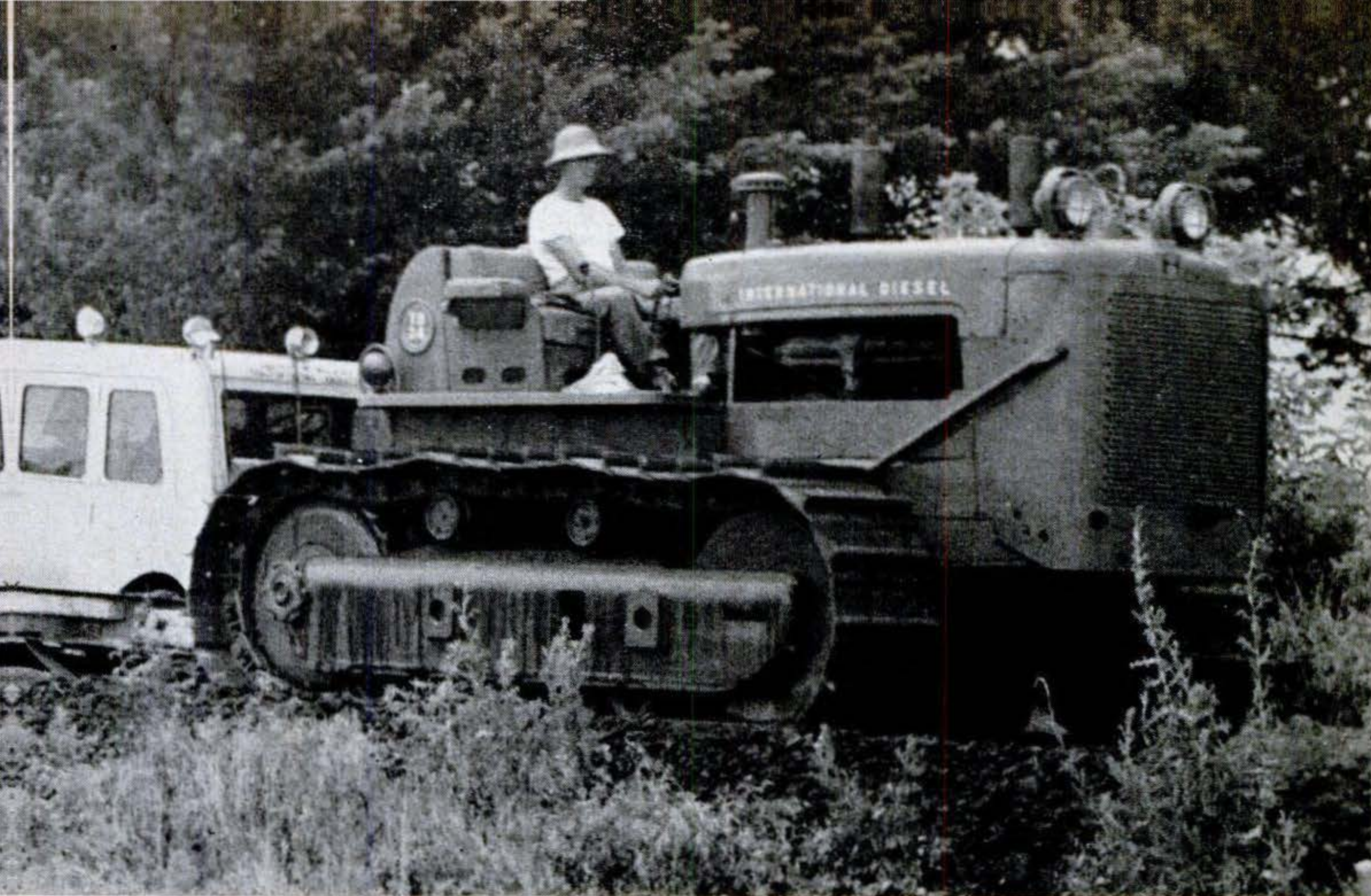
At 1½ m.p.h., the behemoth pulled 33,714 pounds, put out a drawbar horsepower of 148.43.
