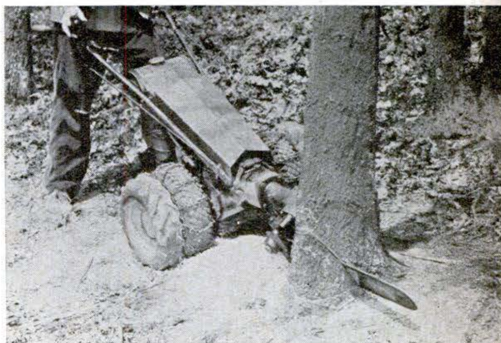
DUAL WHEELS , quickly mounted on this 5-hp. Gravely, let it bull right through rough terrain and up steep slopes. Nose drive can be fitted with more than 20 different attachments, including the chain saw above.
