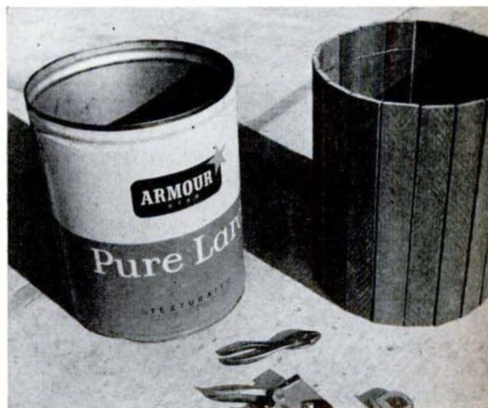
A LARD CAN is transformed into a plant tub by wiring together slats cut the same height as the can. Slip the assembly over the can.
