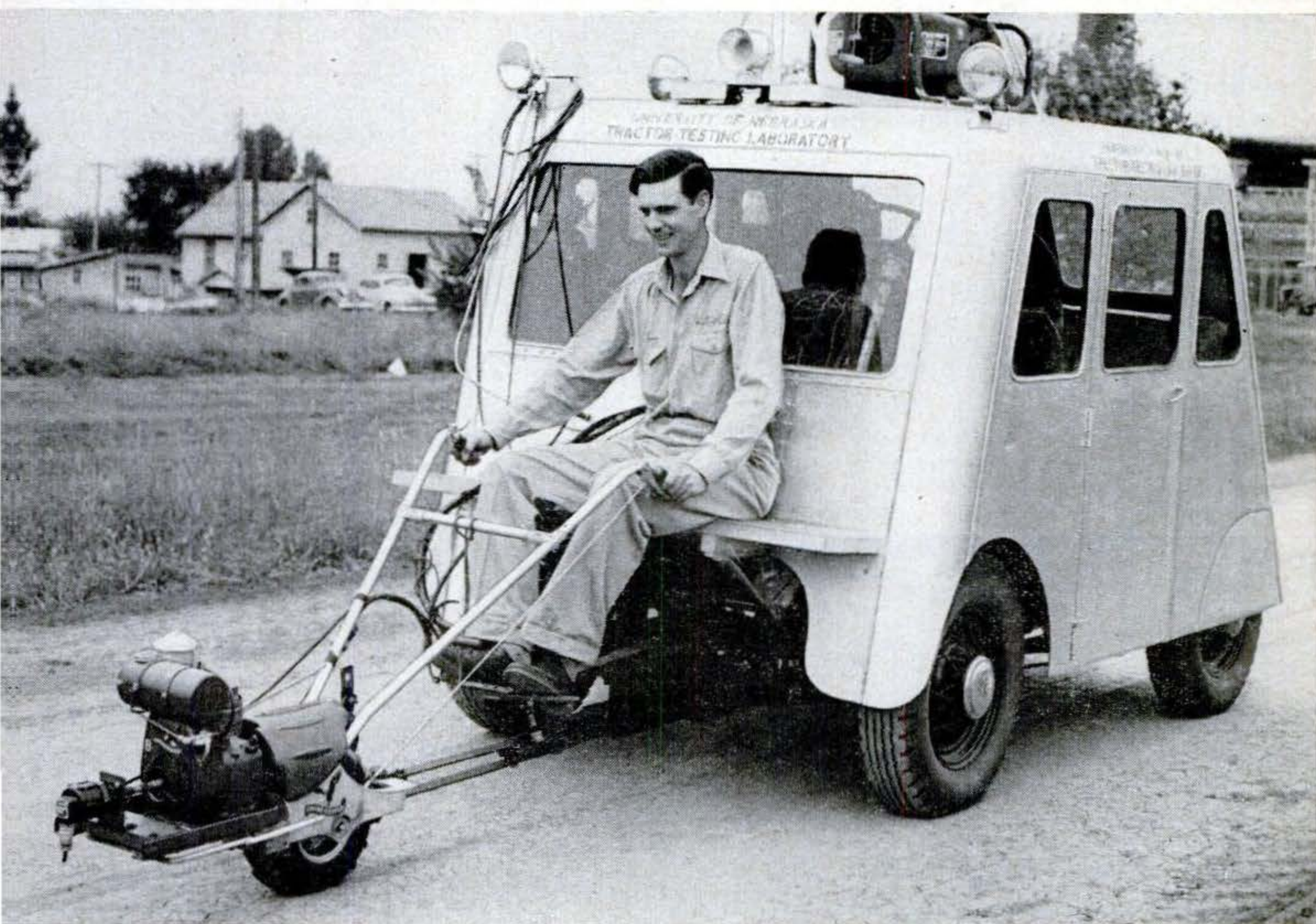
SMALLEST MODEL ever tested was this ½-hp. Choremaster, a walking tractor for garden
