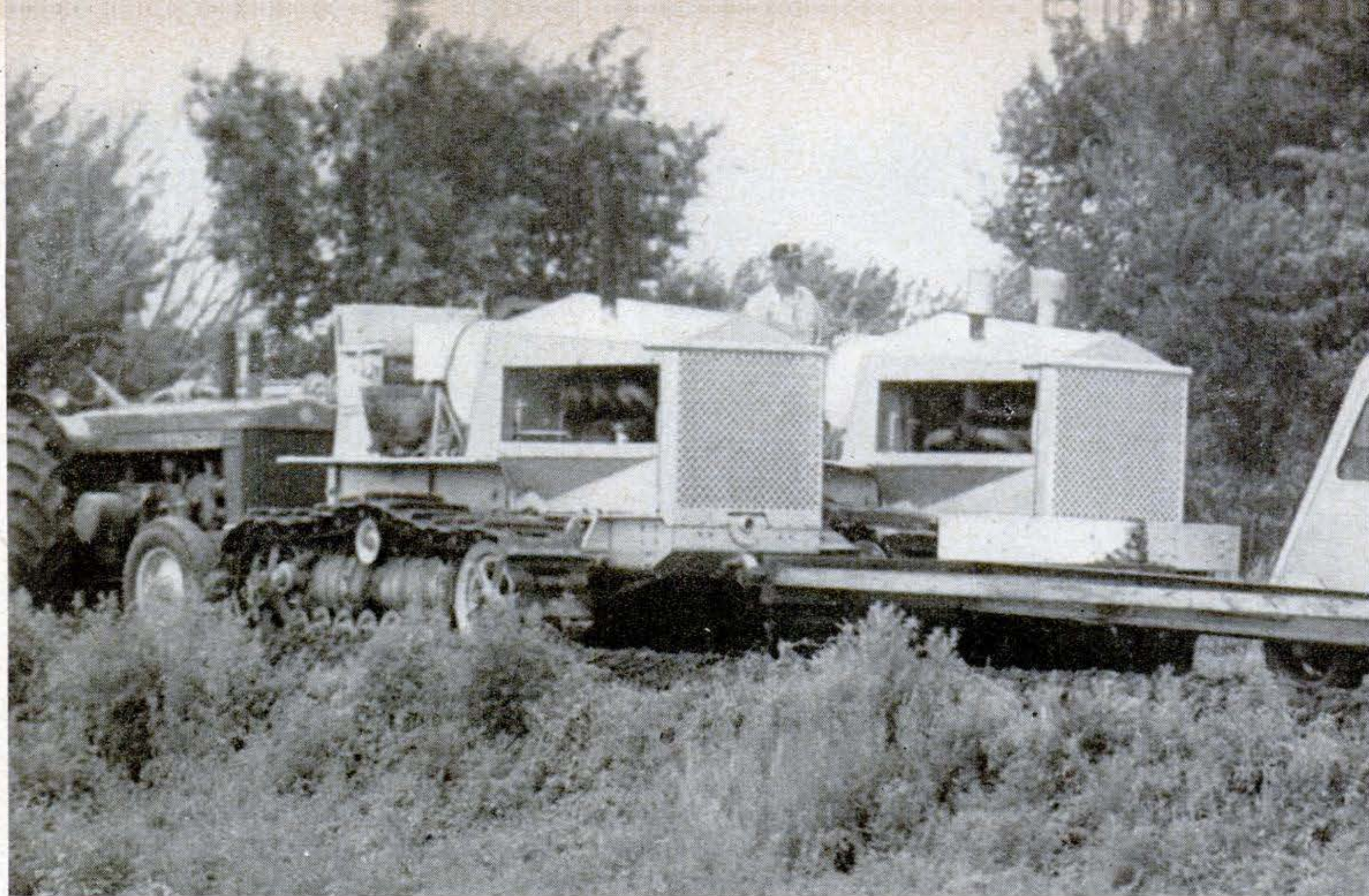
International Harvester TD 24 pulls Nebraska's test car plus a string of tractors in gear.
