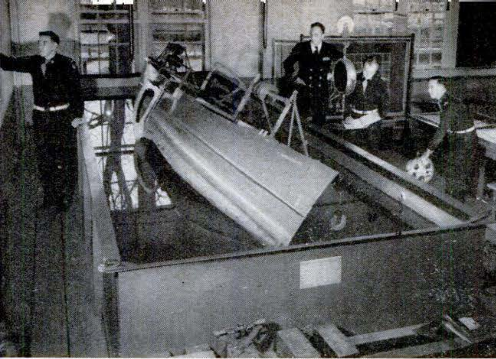
SHIP MODEL named Miss Calculation shows the students what can happen when a vessel is improperly loaded or the cargo shifts. Lead weights simulate any loading condition.
