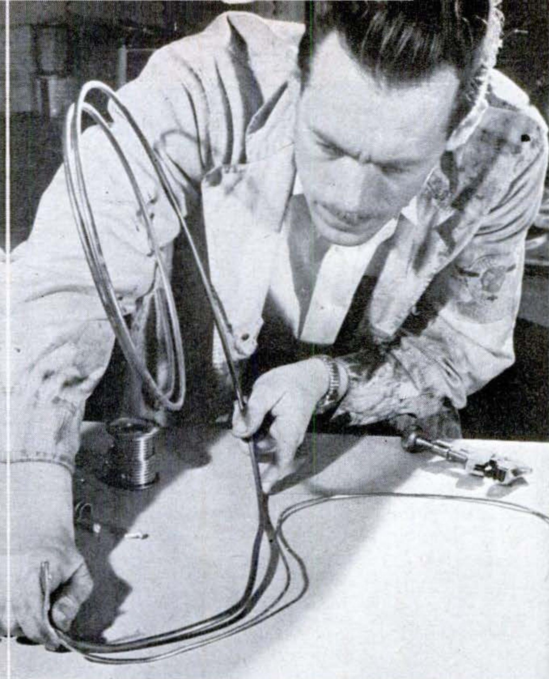
SHAPE AND LENGTH of hydraulic tubing for vacuum and hydraulic lines can be found by making templates with soft wire solder. Form copper tubing gently to match solder-wire contours, avoiding sharp bends and flats.
