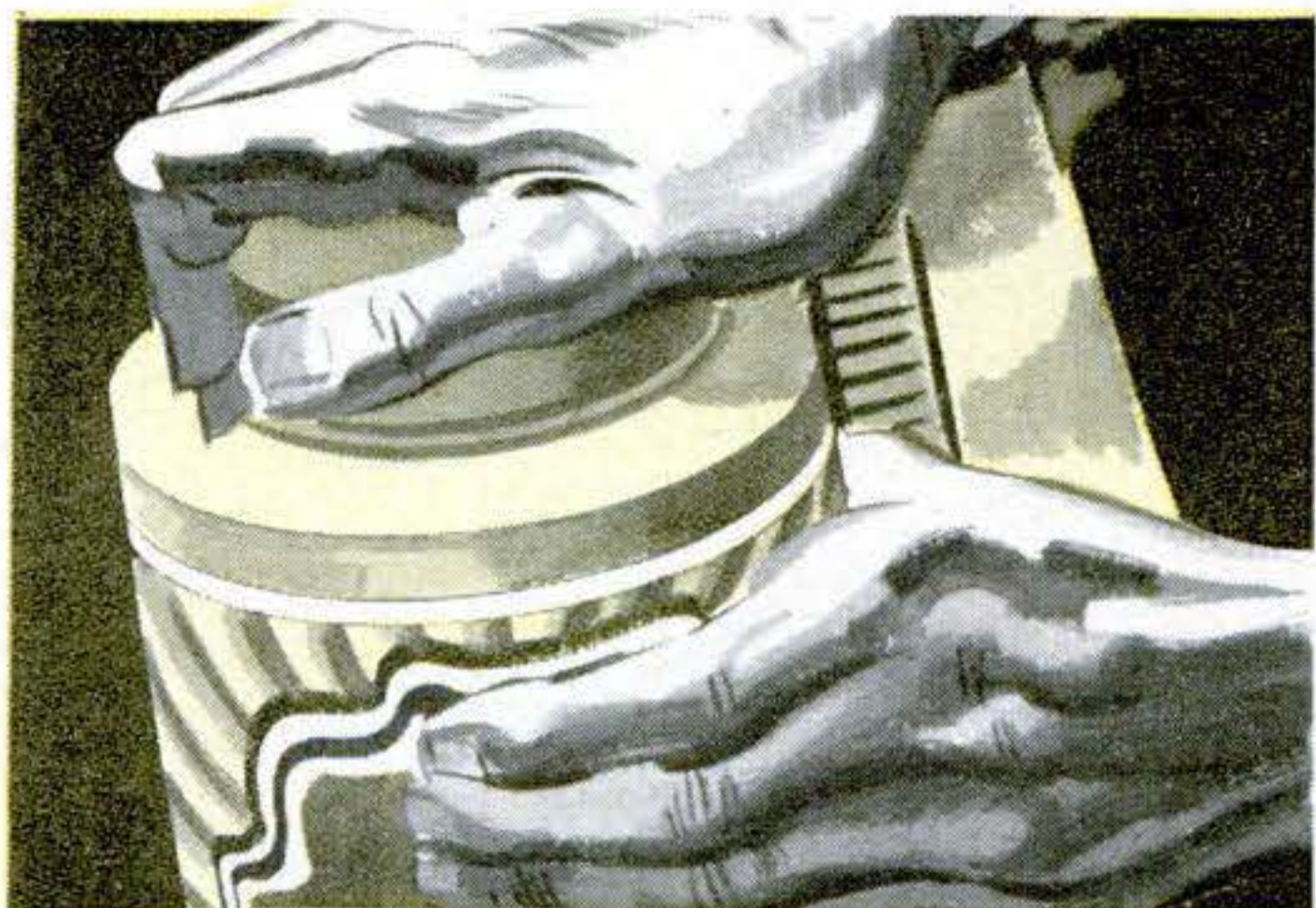
A PAINT SPRAY GUN that would screw directly onto a threaded paint can or onto a collar that would grip and puncture the can.— R. H. West, Rochelle Park, N. J.
