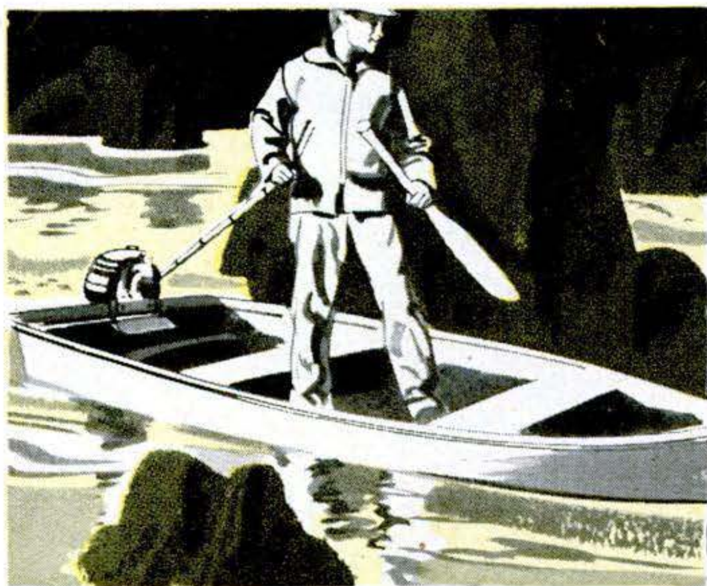
AN OUTBOARD MOTOR with a telescoping handle so a skipper could stand up to steer safely through rocky places and narrow channels.— R. Turley, Pointe aux Trembles, Quebec.
