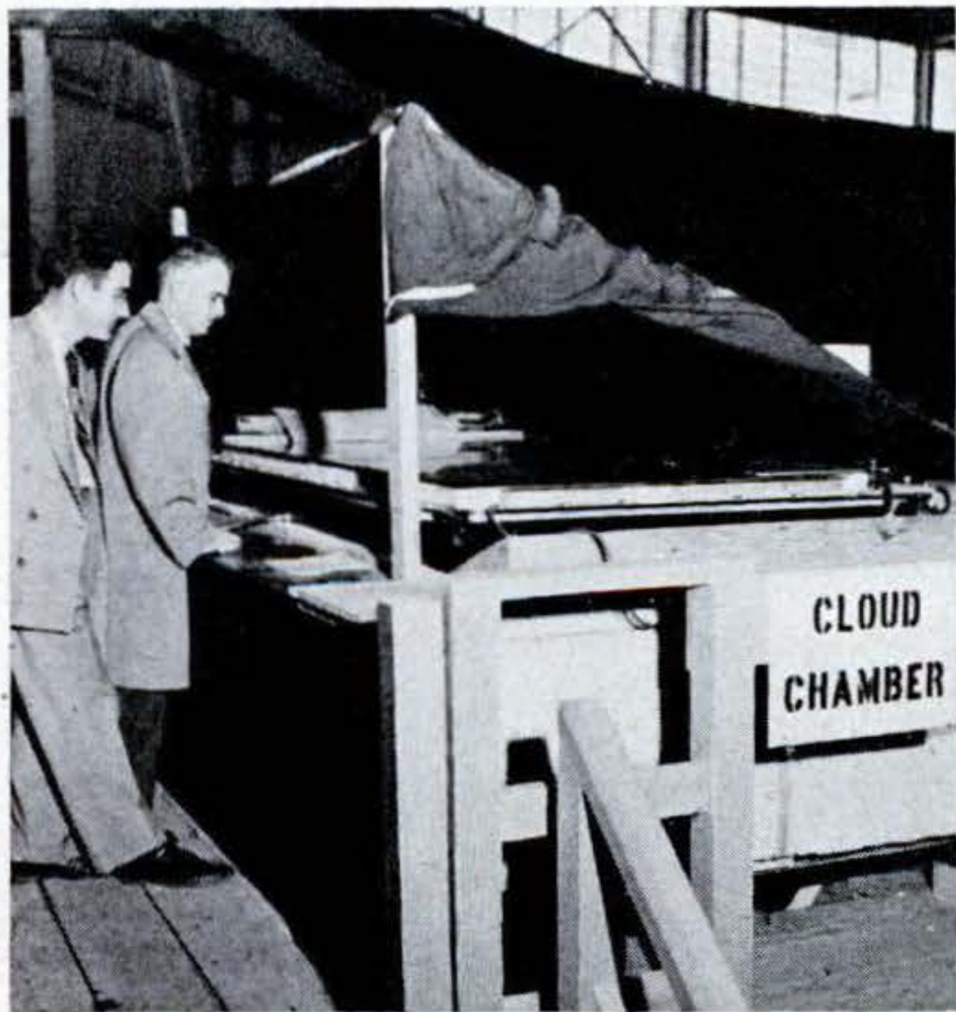
TO CATCH ATOMIC FRAGMENTS broken off in bevatron, world's biggest cloud chamber was built. It is a glass-enclosed box filled with alcohol vapor, which condenses to form a trail along the paths of atomic particles.
