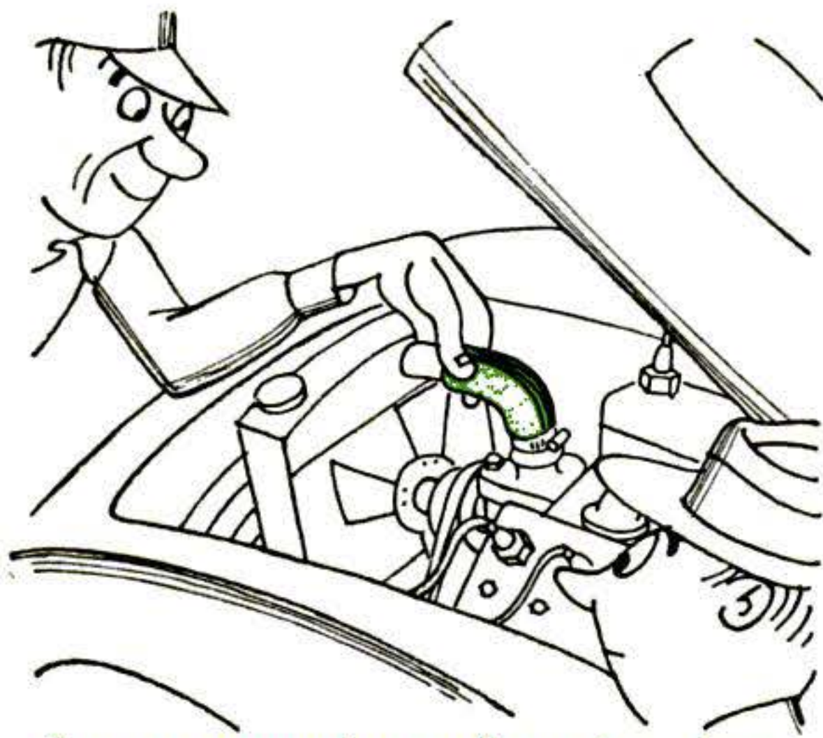
Spongy connections indicate hose decay
