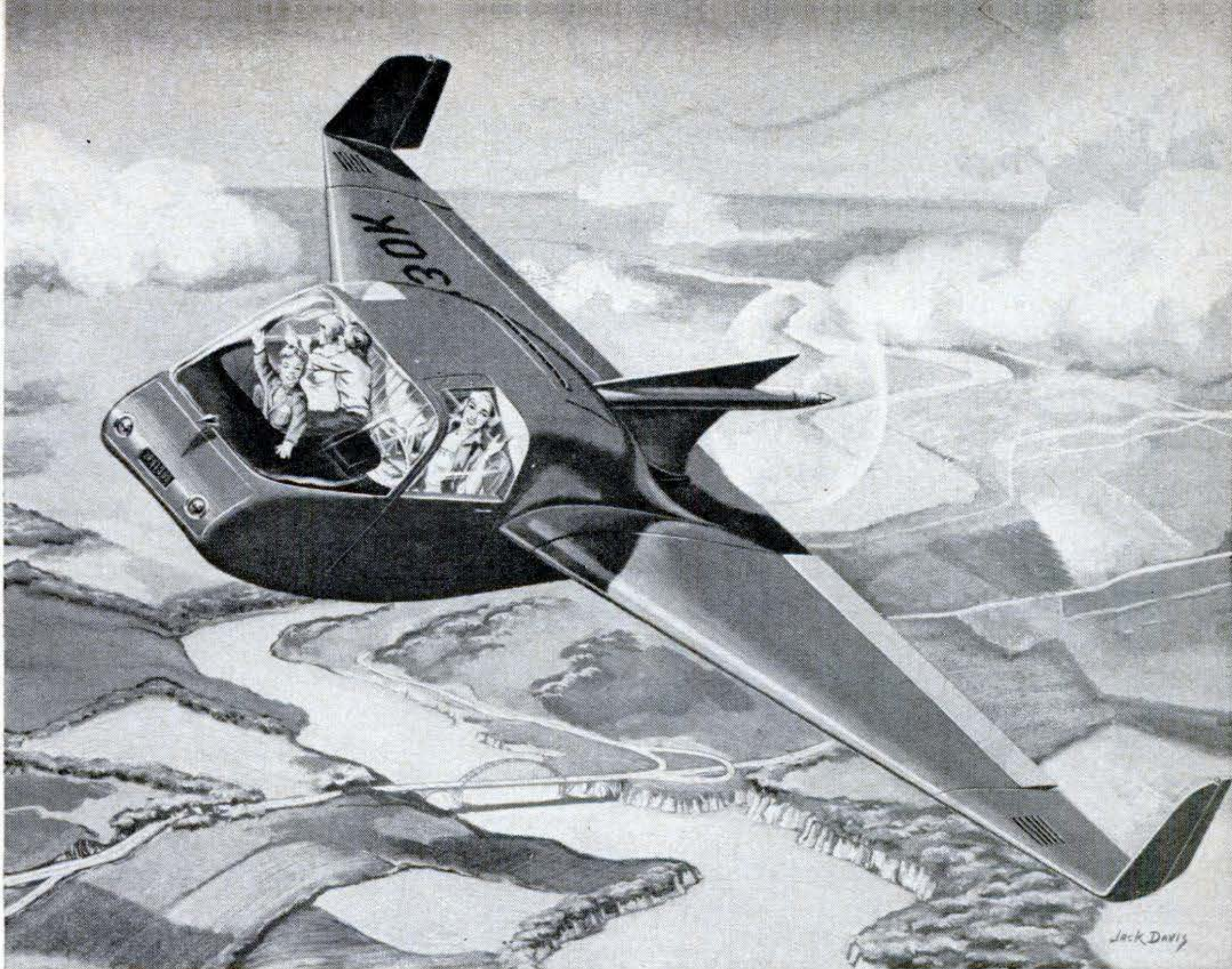
Four passengers are no squeeze in the roomy cabin of Coleman's delta-wing pusher plane.
