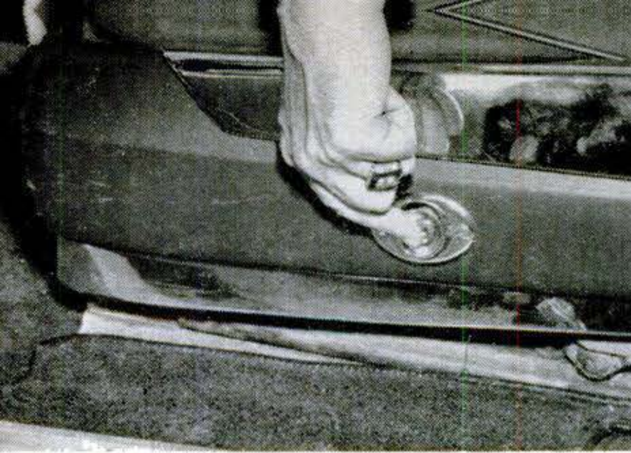
FOUR-WAY TOGGLE SWITCH replaces seat-control buttons. Just flip the lever the way you want the seat to go.
