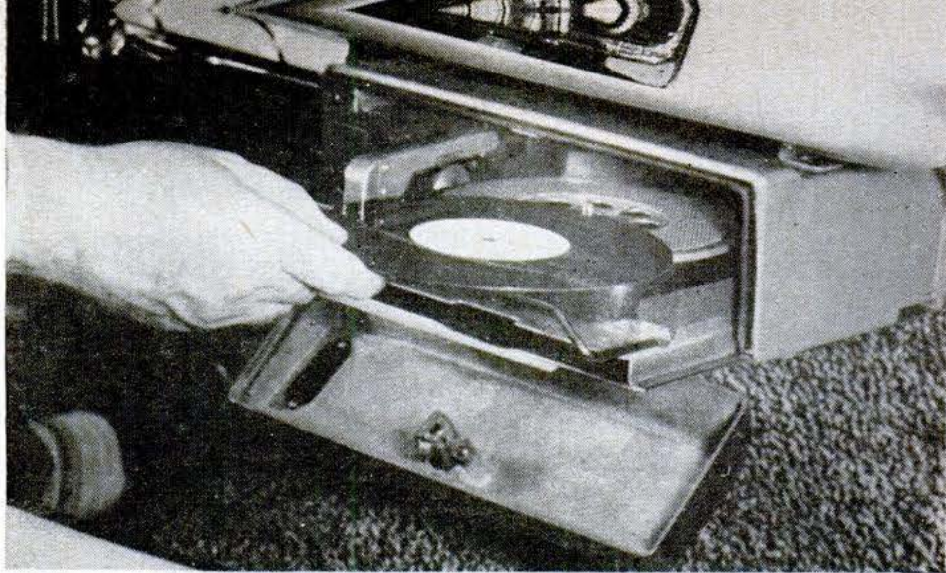
AS EASY TO WORK AS RADIO , auto phonograph has stops at back to guide record over spindle. You needn't look.
