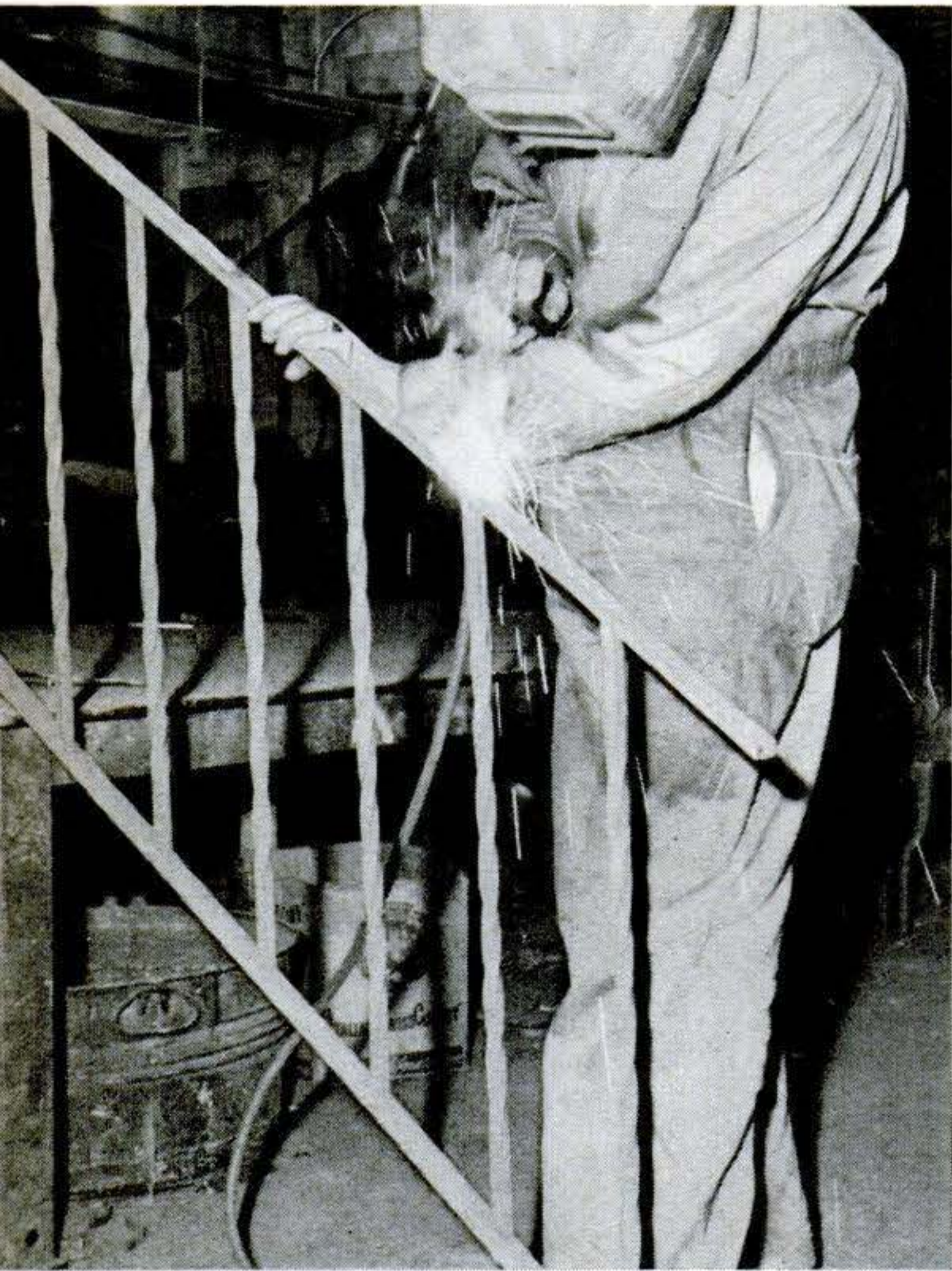
HOT-ROLLED MILD STEEL is too low in carbon content to harden when heated. Tough, it can be twisted or bent; welds easily. Use it for assemblies like this decorative stair rail.
