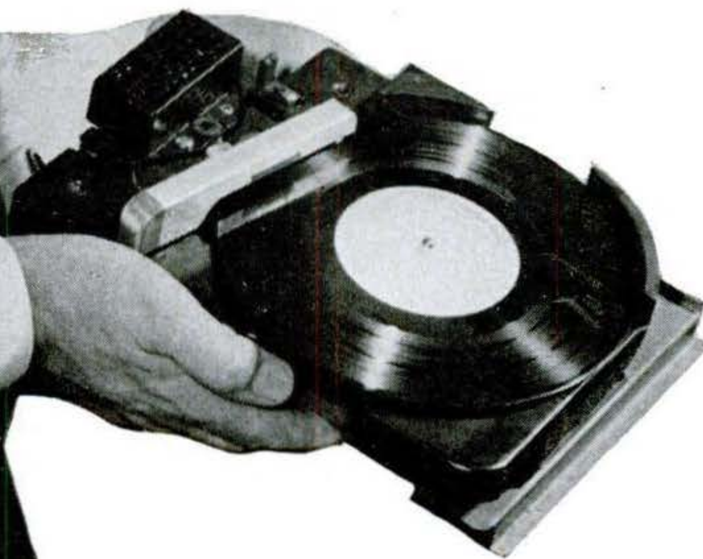
YOU'D HAVE TO DRIVE UP A WALL to make the needle skip a groove. The player was making good music when tilted for this photo by Dr. Peter Goldmark, Columbia Broadcasting System research chief. The new unit is an optional accessory for Dodge and other Chrysler cars.
