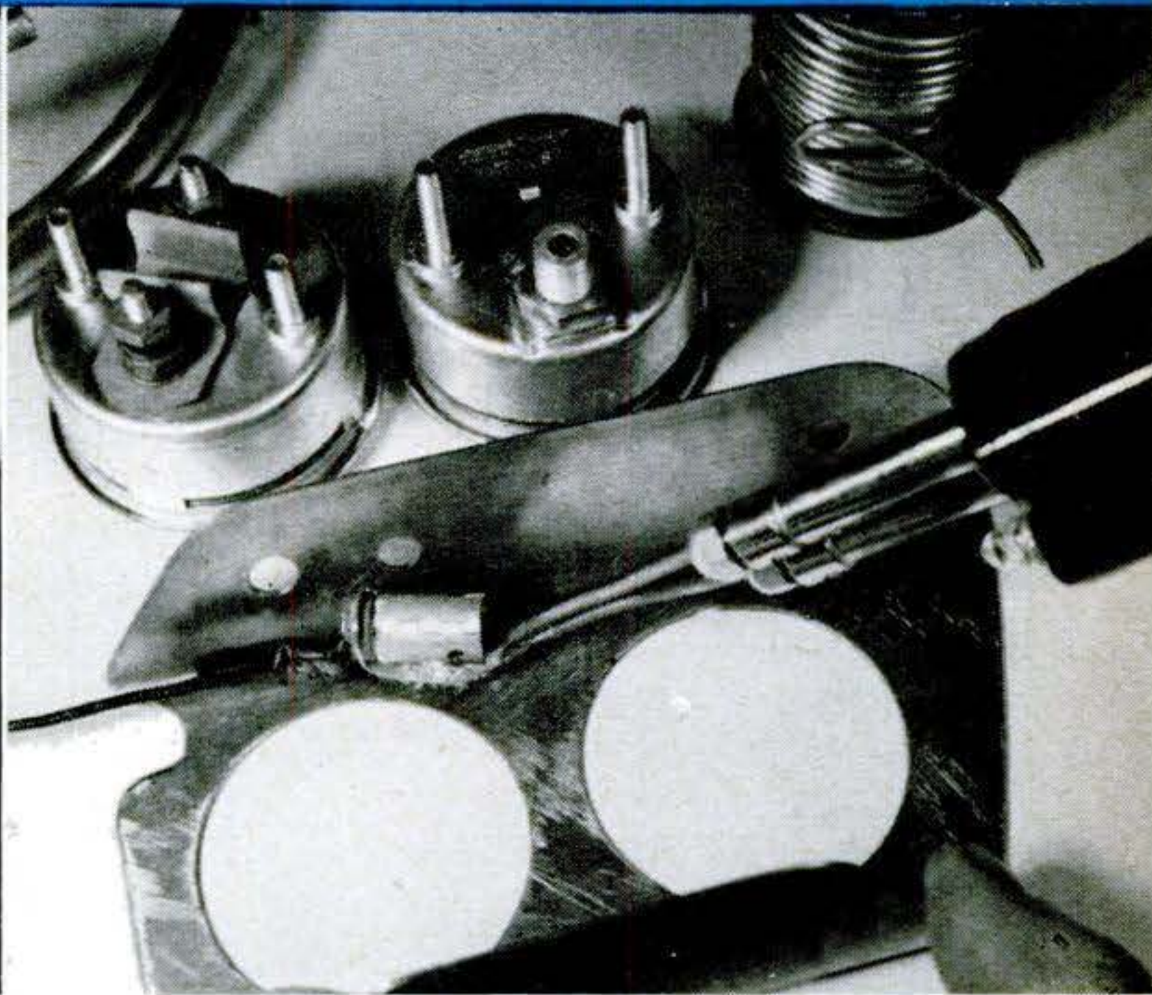
A BULB SOCKET soldered on back of the metal panel lights the gauges that the writer installed. Connected in parallel with dash light, the lamp shines through slots in the gauges.
