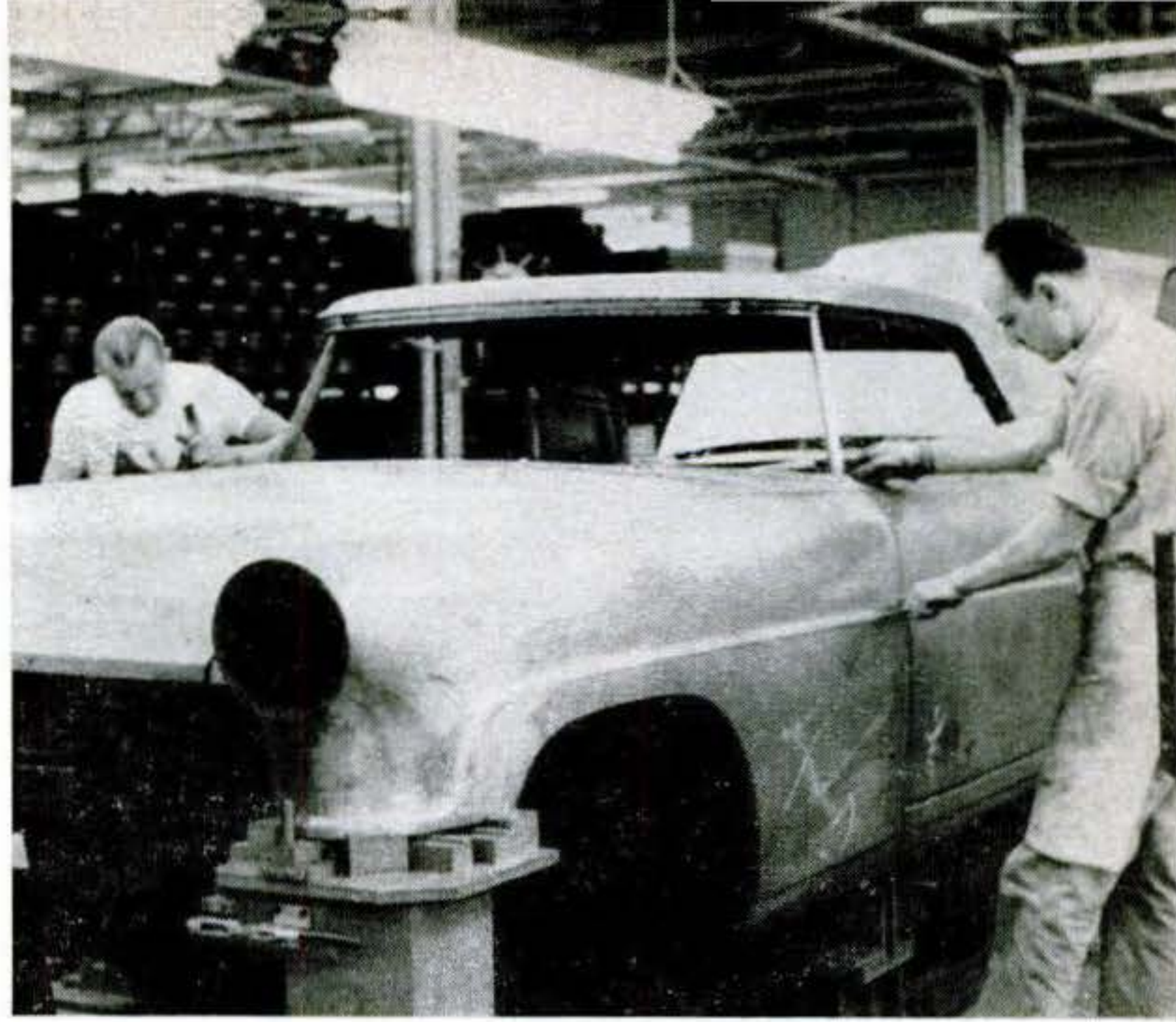
1 TRIAL MARRIAGE. Body parts are assembled "in the white"—unpainted—and fitted to a tolerance of .025 inch. When right they are keyed for later identical reassembly.
