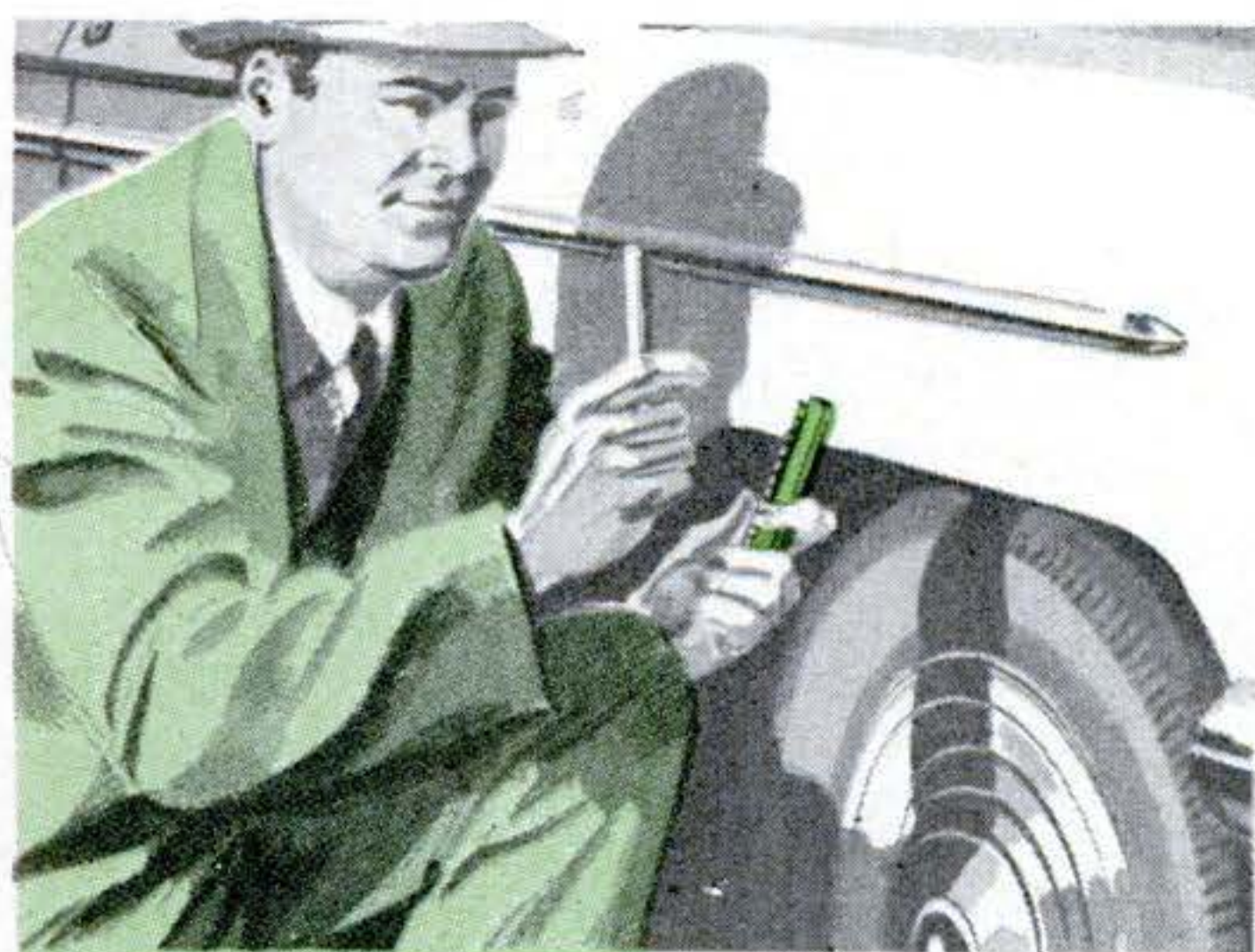
A TIRE-PRESSURE GAUGE that would give a temperature reading. Recommended pressures at various temperatures could be printed on case.— Ray Welder, Wittenberg, Wis.
