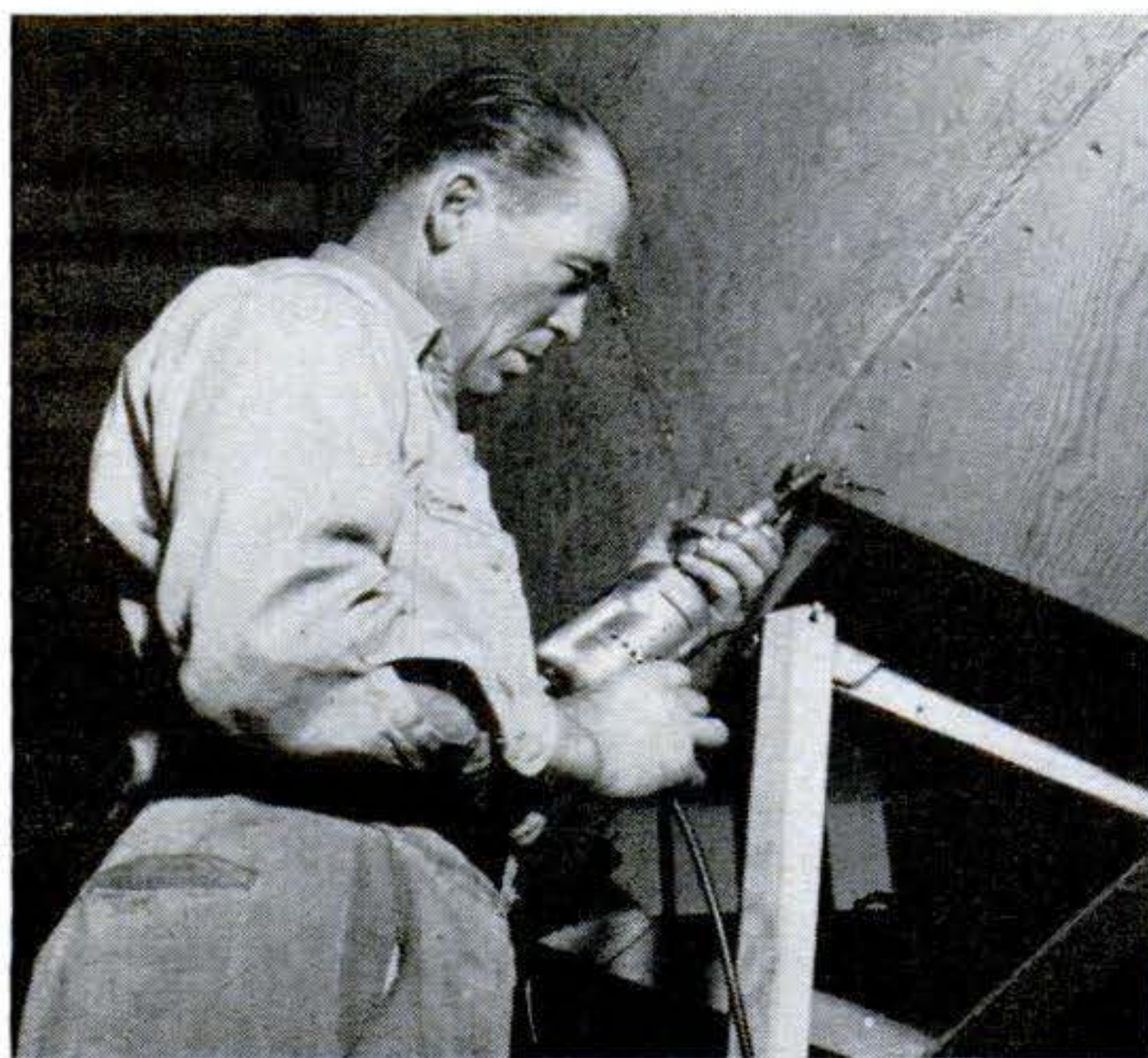
PUTTING IN SCREWS , a large part of boatbuilding, is speeded by power. Each customer gets electric drill with a screwdriving attachment.
