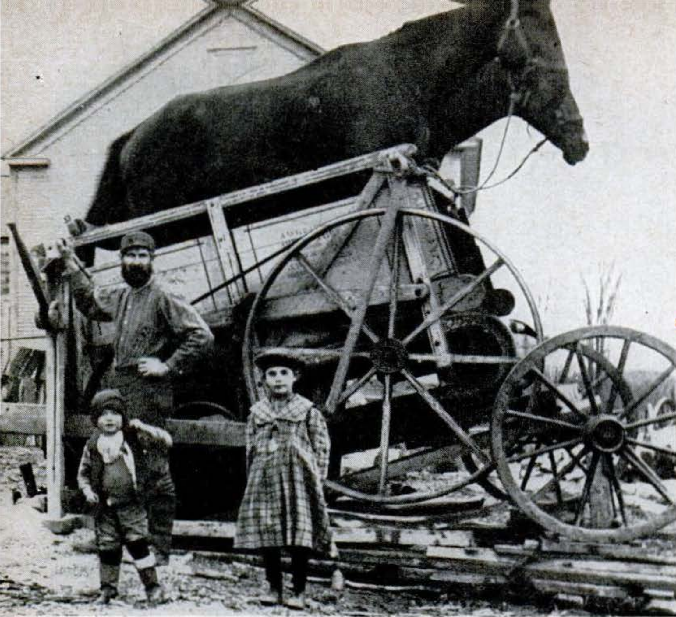
Two-horsepower engine running Vermont drag saw, around 1914.
