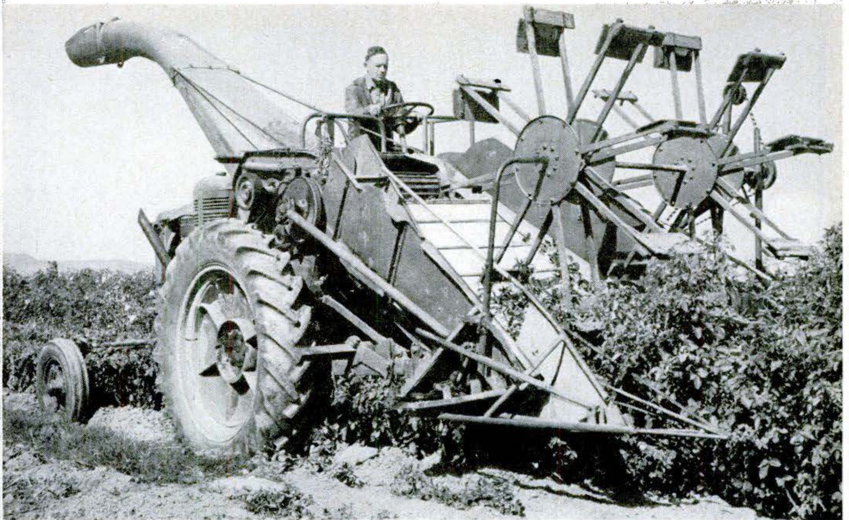
THRESHER HARVESTS SEED. Machine reaps two rows on each trip. Paddles force bushes against
