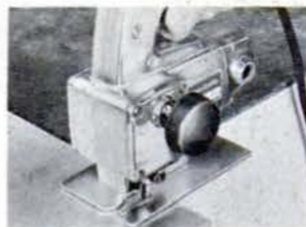
Metal cutting—sheet metal, pipe, bar stock, rods are quickly and accurately cut.
