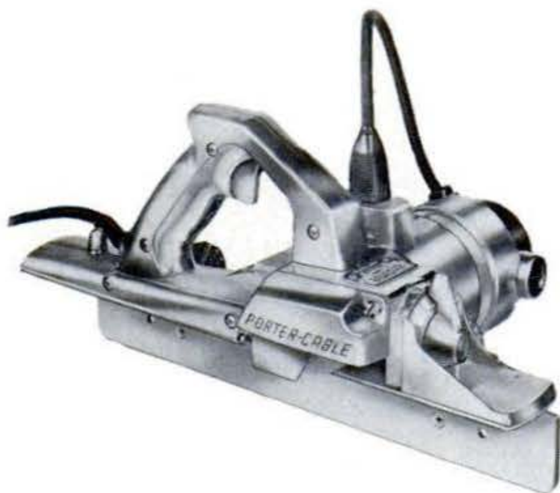
This 16" plane attachment features a long shoe base, patented chip disposal, fingertip depth adjustment up to 3/32" deep, bevel adjustment to 45°. High-speed router motor produces a glass-smooth edge even on glue-bonded plywood.
