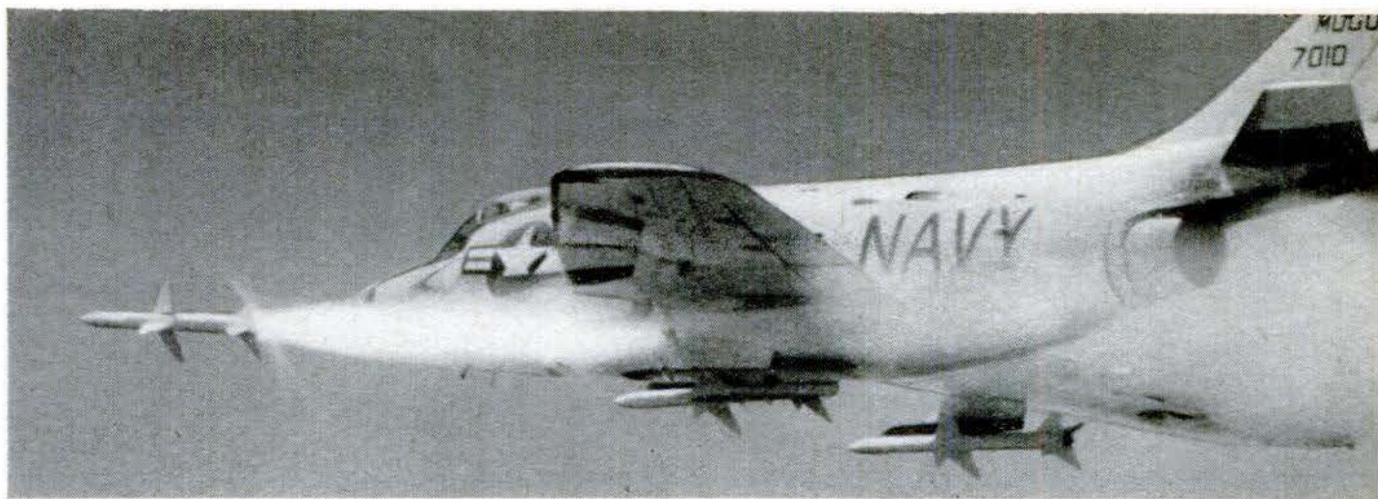
SPARROW WITH BIG STING. A split second after firing, a Sparrow III, newest Navy supersonic guided missile, streaks toward its target. Recently made operational with the Seventh Fleet in the Pacific, the deadly air-to-air weapon packs 50 percent more wallop than its predecessor.
