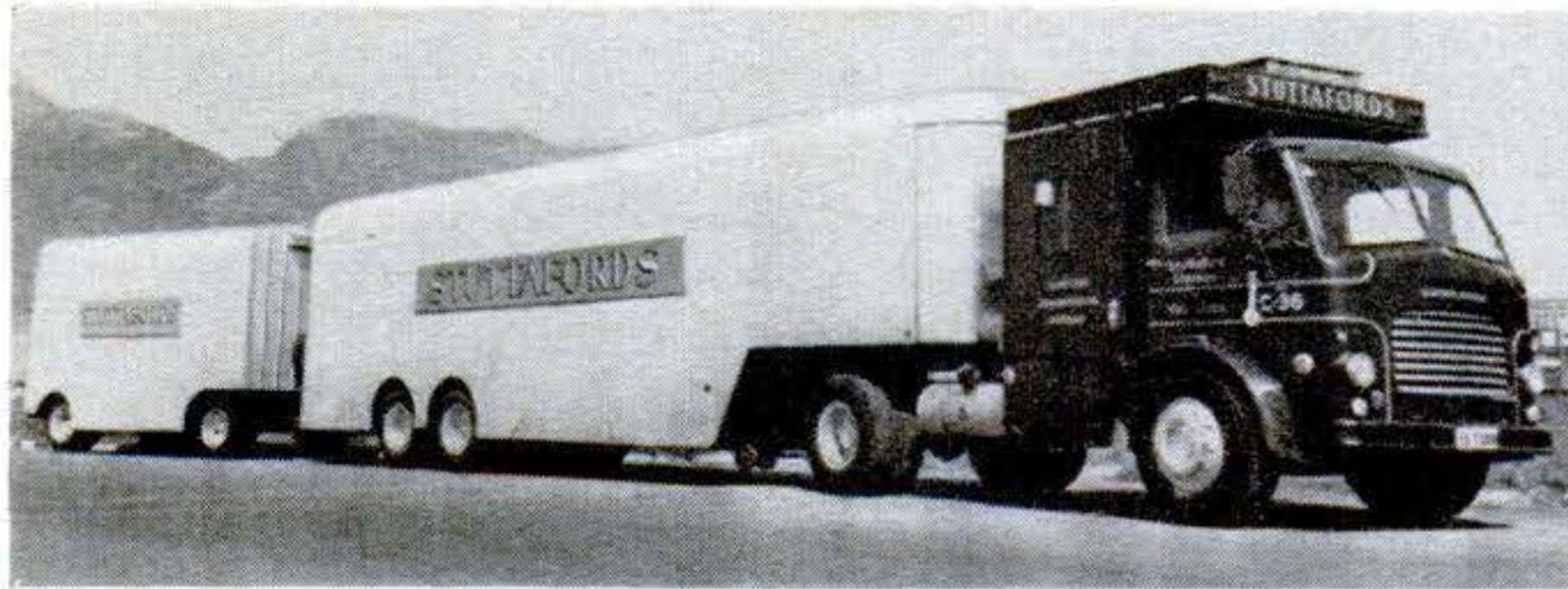
TANDEM TRAILERS. For long-distance moving in South Africa, a Cape Town hauler uses this giant road train. It carries 16-ton loads on trips of 1,500 miles or more. Tractor and two aluminum trailers make up a train over 60 feet long.
