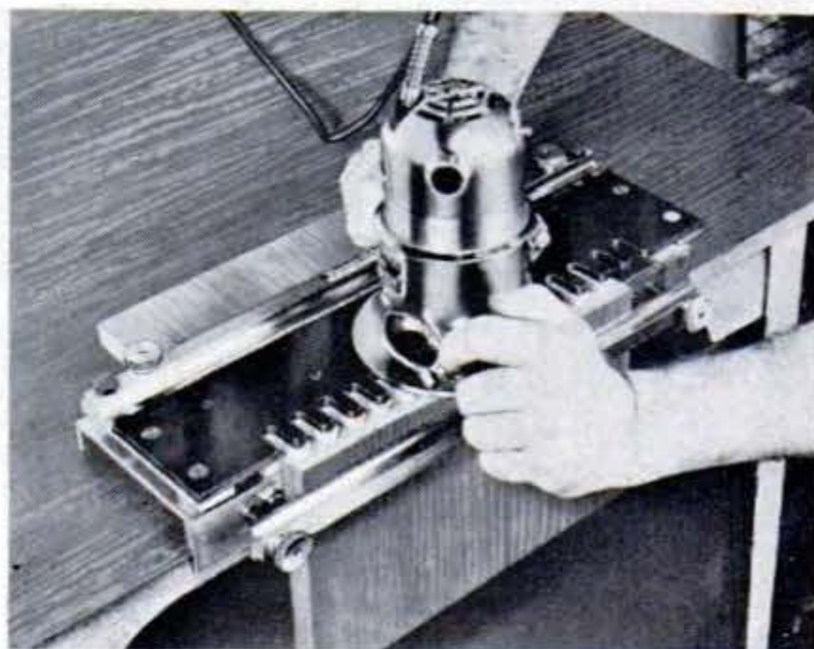
In using the dovetail templet, a perfect joint can be made in 12 seconds.
