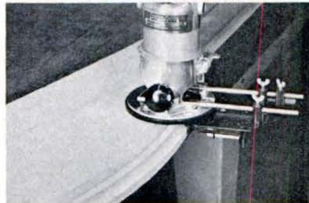
For inlay work on curved pieces, 5-in-1 attachment acts as a radius guide. A simple adjustment converts it to a straight edge guide.
