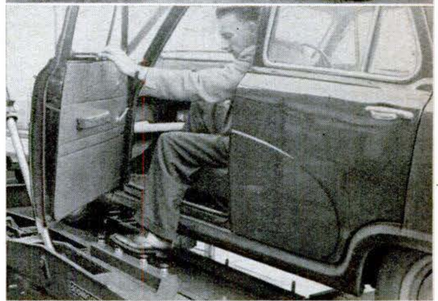
CAR LIFT. The drive-on ramp of this British four-car transporter is an elevator that rises to the upper deck. One man loads and unloads the cargo with the aid of foot controls (lower photo). The ramp then folds forward for highway travel.
