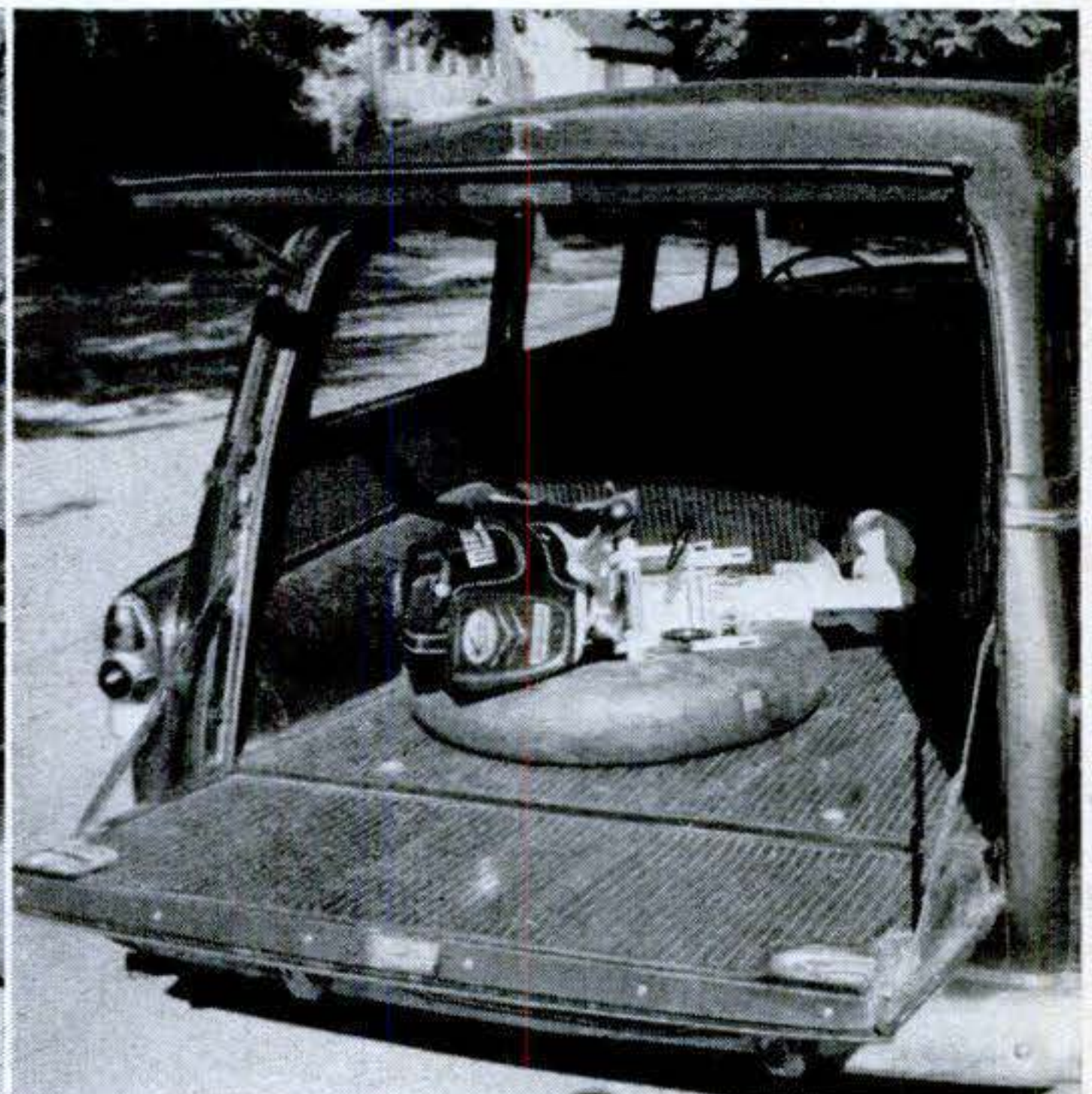
inner tube inflated to 10 pounds and it slides easily into a wagon. You'll save the outboard's muscles, too, during drives over backwoods roads. Place the motor with projecting controls facing up, to protect them and prevent puncturing the cushioning inner tube.
