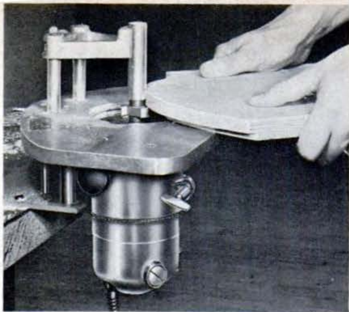
A rabbet or step cut being made with the shaper table. Router motors and cutters may be adjusted for varying depths of cut and hundreds of shapes.
