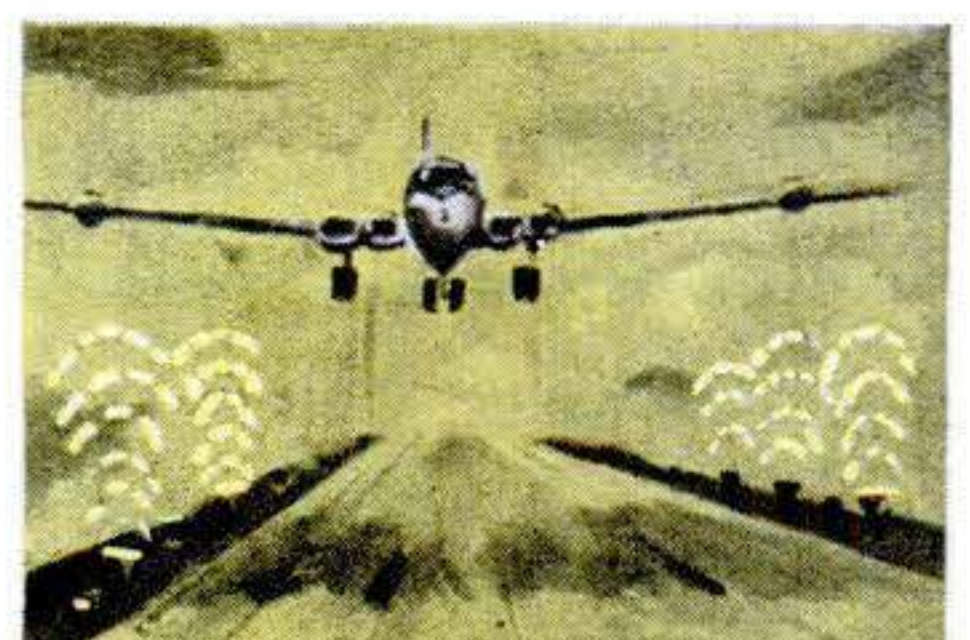
CLEARING FOG. Powerful sound from horns cuts chimney smoke, is now being tested as a landing aid for fog-bound airports.
