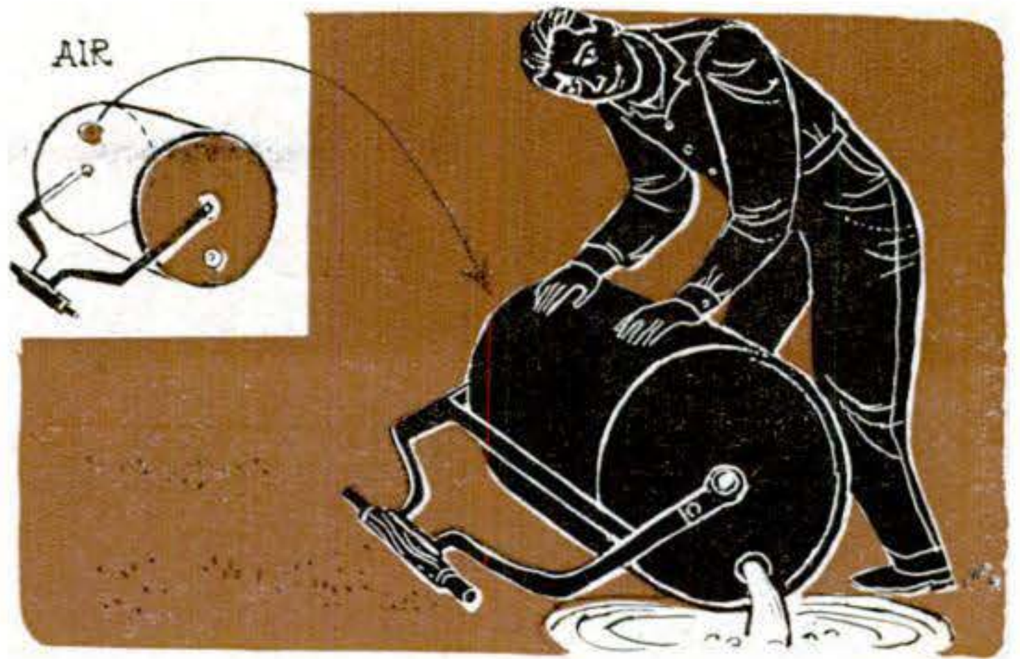
A LAWN ROLLER WITH TWO OPENINGS. A drain on one side and an air intake on the other, both with plugs, would make emptying a roller faster and easier.— Joseph P. Izzo, Providence.
