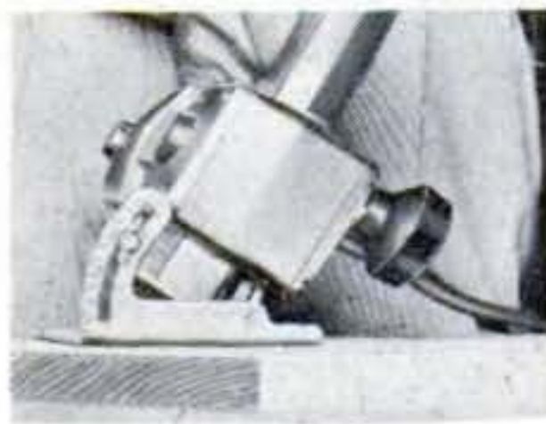
Angle cuts—equipped with the angle base, quickly and easily cuts accurate angles up to 45°.
