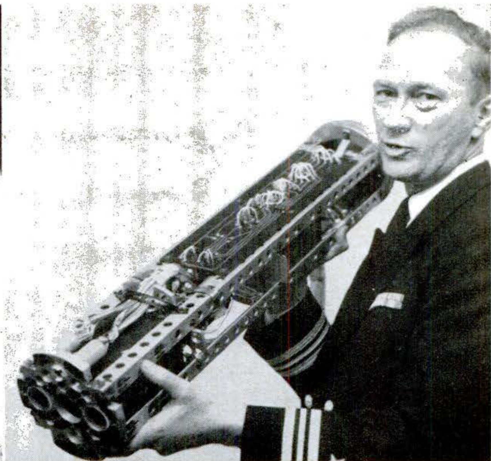
HURRICANE-SPOTTER. A movie-camera unit shot up 86 miles from Wallops Island, Va., in the rocket at left was recovered at sea after it had taken pictures of cloud formations from Florida to Maine. Navy and Weather Bureau expect the new technique to help give advance warning of tropical storms, such as the one shown at upper left in the photo-mosaic.
