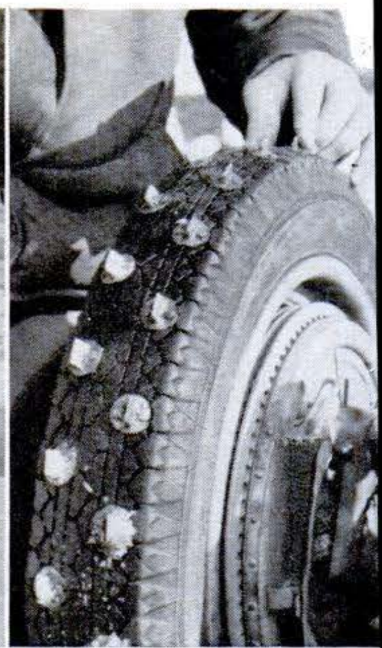
SPIKED TIRES. Special steel wedges sunk into the treads of racing-car tires (above, right) are one way to help tame skids even on a treacherous track. They were used by drivers in the first European Grand Prix on ice (left) run last winter over the course at Cortina d'Ampezzo, Italy.
