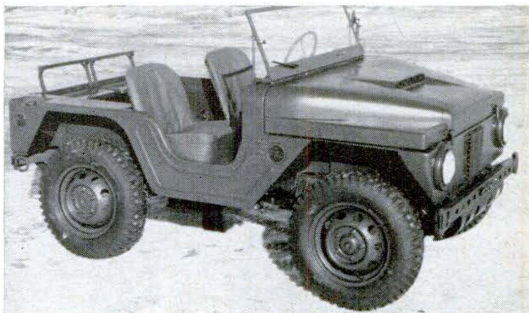
MIGHTY MITE. An air-cooled aluminum V-4 engine [PS, Feb.] powers this quarter-ton, four-wheel-drive vehicle being produced by American Motors for the Marines. The 1,700-pound car can be helicopter-lifted. It has a speed range from 2.5 to 62 m.p.h., can climb a 45-degree grade and ford water to a depth of 60 inches. The frame is of steel, the body of aluminum.
