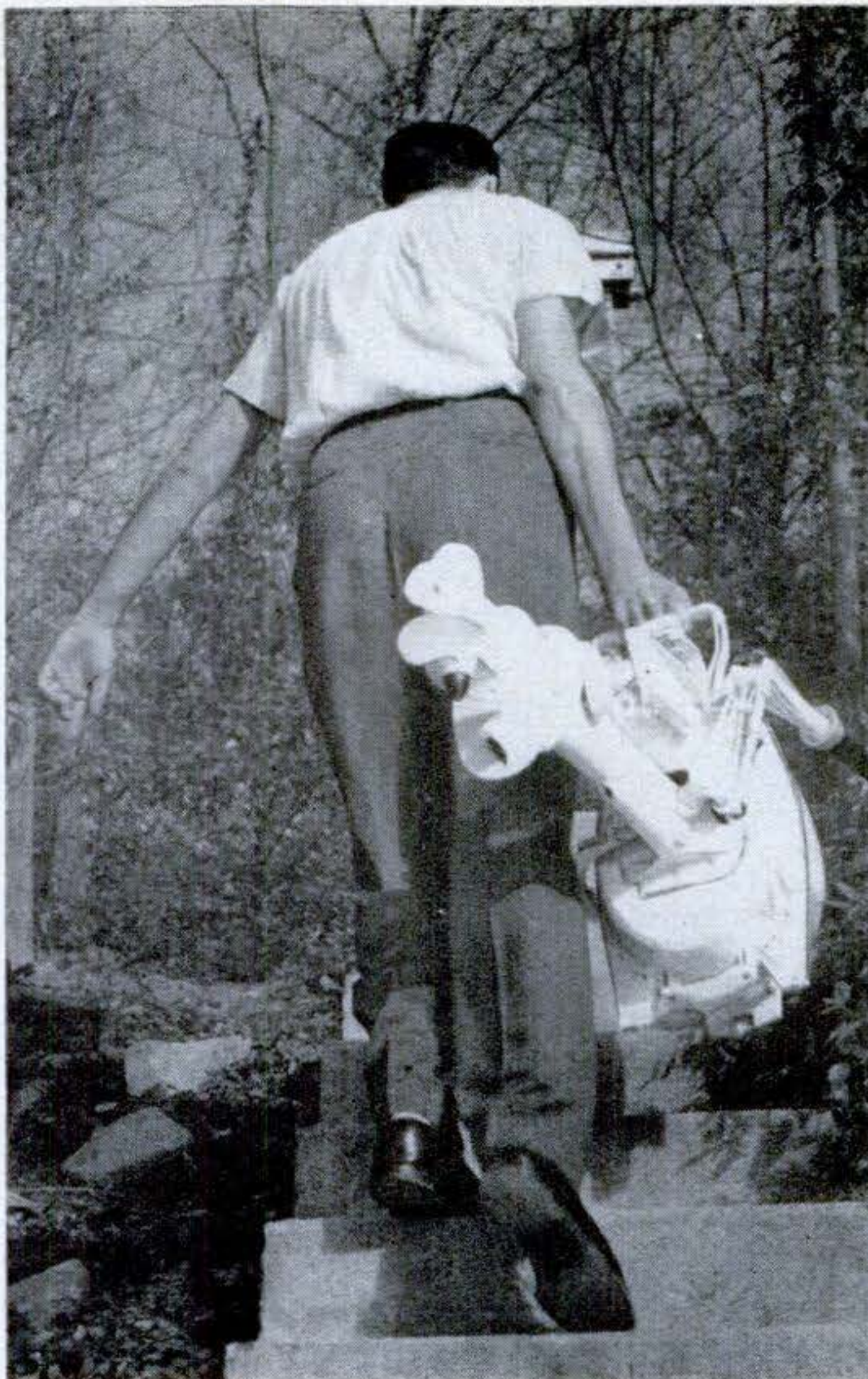
UPSTAIRS AND DOWNSTAIRS: In both cases, the right way is with the motor hood facing upstairs to keep from banging the underwater element
