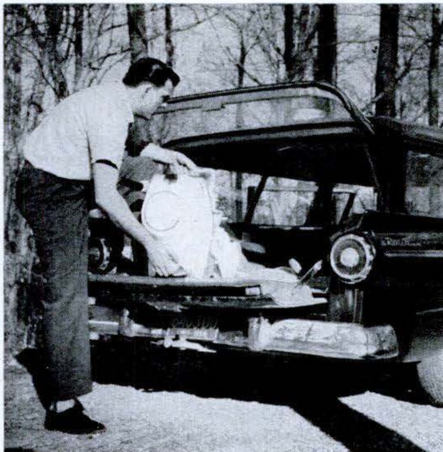
CAR LOADING: When you put a motor in a car or wagon, raise it to the trunk or tailgate edge and rest it there while you place one foot alongside. Then lift it the rest of the way up. Reverse the procedure when unloading, making sure the footing is firm behind you. Cradle a motor in an
