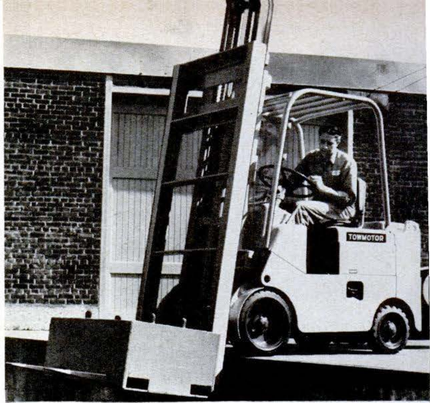
UNDER AND OVER. Here's a fork lift that lowers a three-ton load seven feet below the floor or raises it 12 feet above. This Towmotor model has a transparent heat shield, is used by a steel mill to dunk castings in a quench tank.
