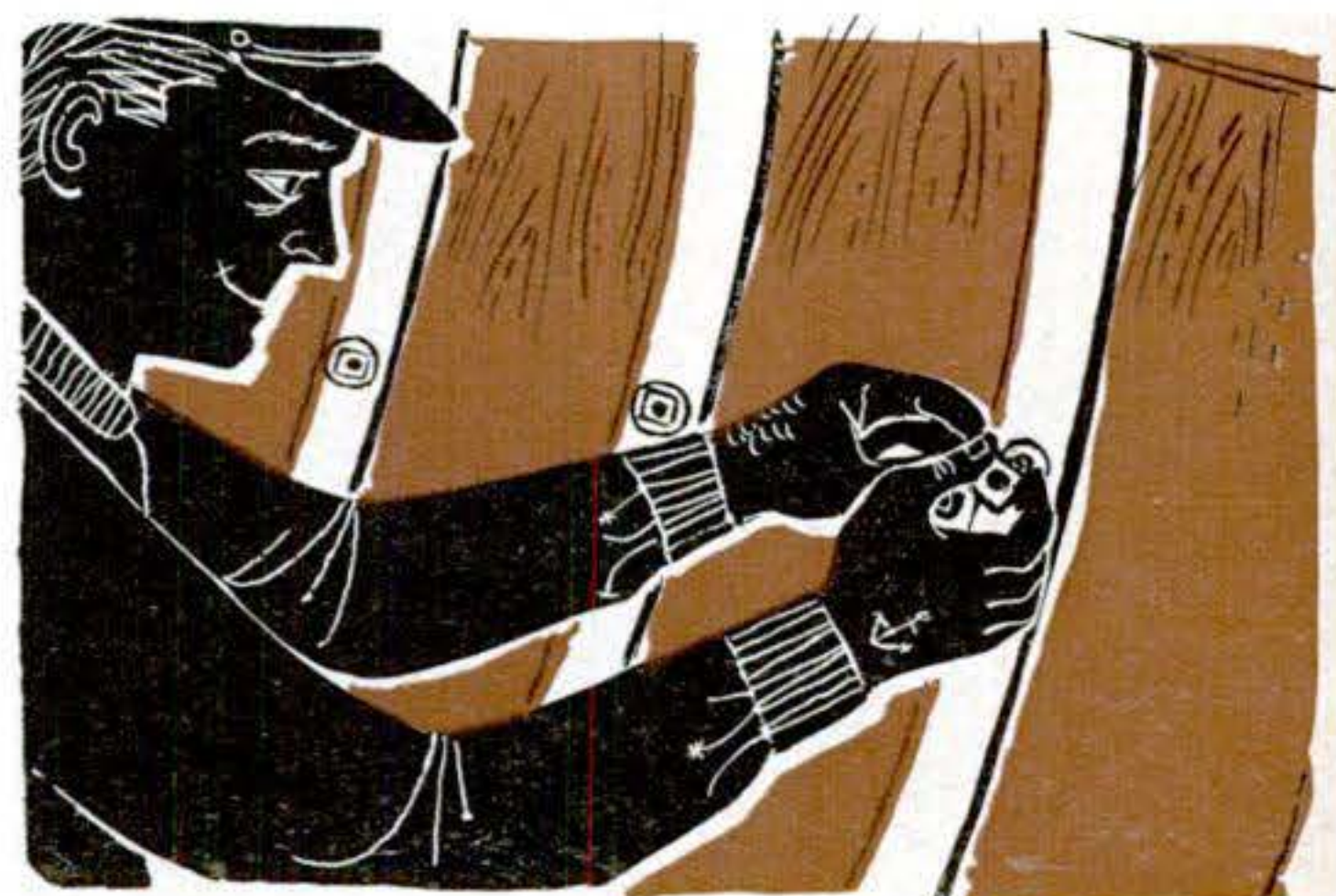
ALUMINUM-RIBBED BOATS IN KIT FORM. The metal ribs could be bolted to plywood, eliminating screws that so frequently pull out or break off.— K. N. Croshier, Poughkeepsie, N. Y.
