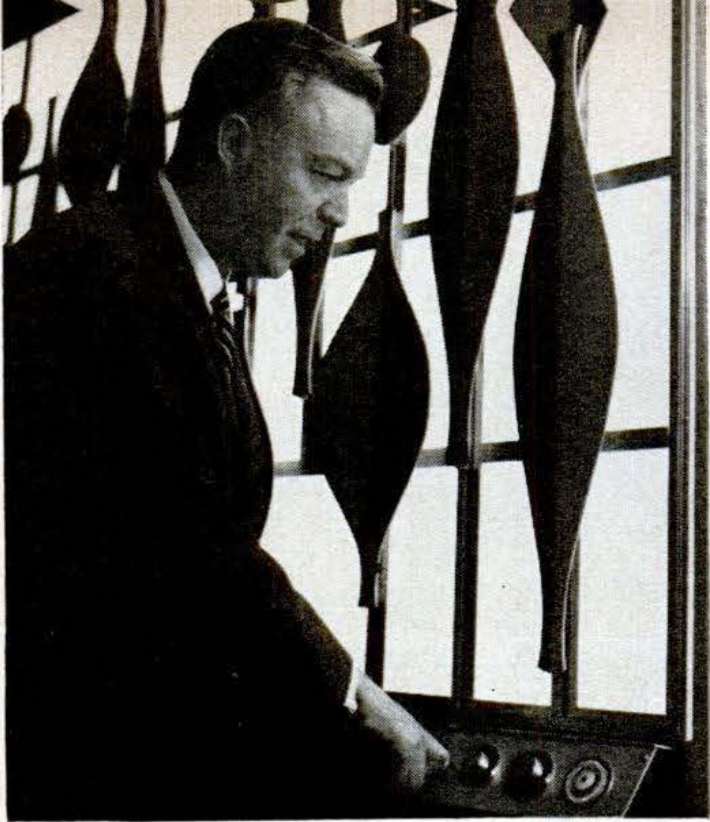
HOT-COLD LIGHT. This luminescent panel may not only light a room but heat and cool it, too. The aluminum cut-outs are part of a dial-controlled thermo-electric heating and cooling system under study by Westinghouse.
