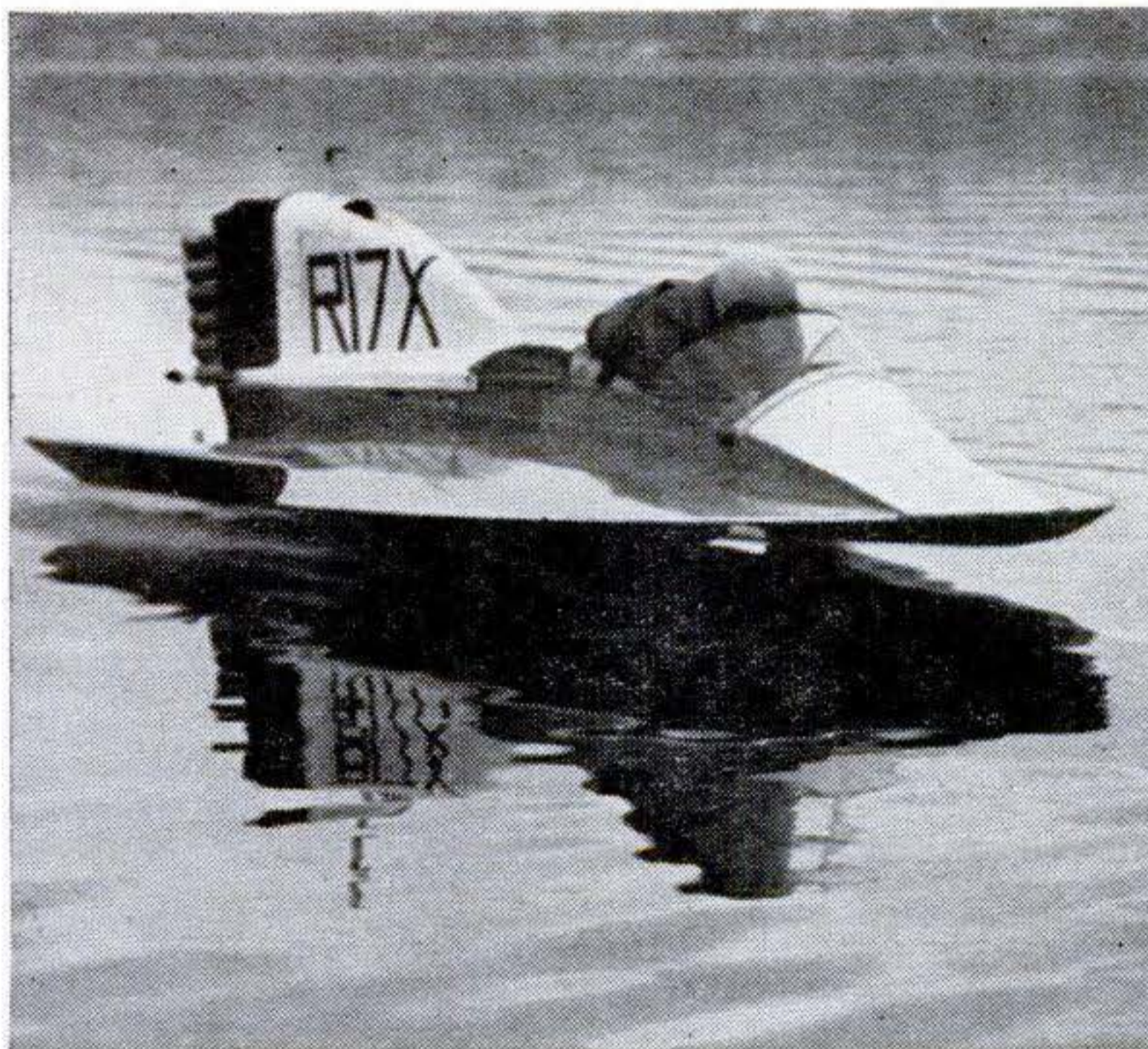
SET FOR RECORD , Ross moves to starting line. At top speed, entire hull rides out of water with lower half of propeller below water line.
