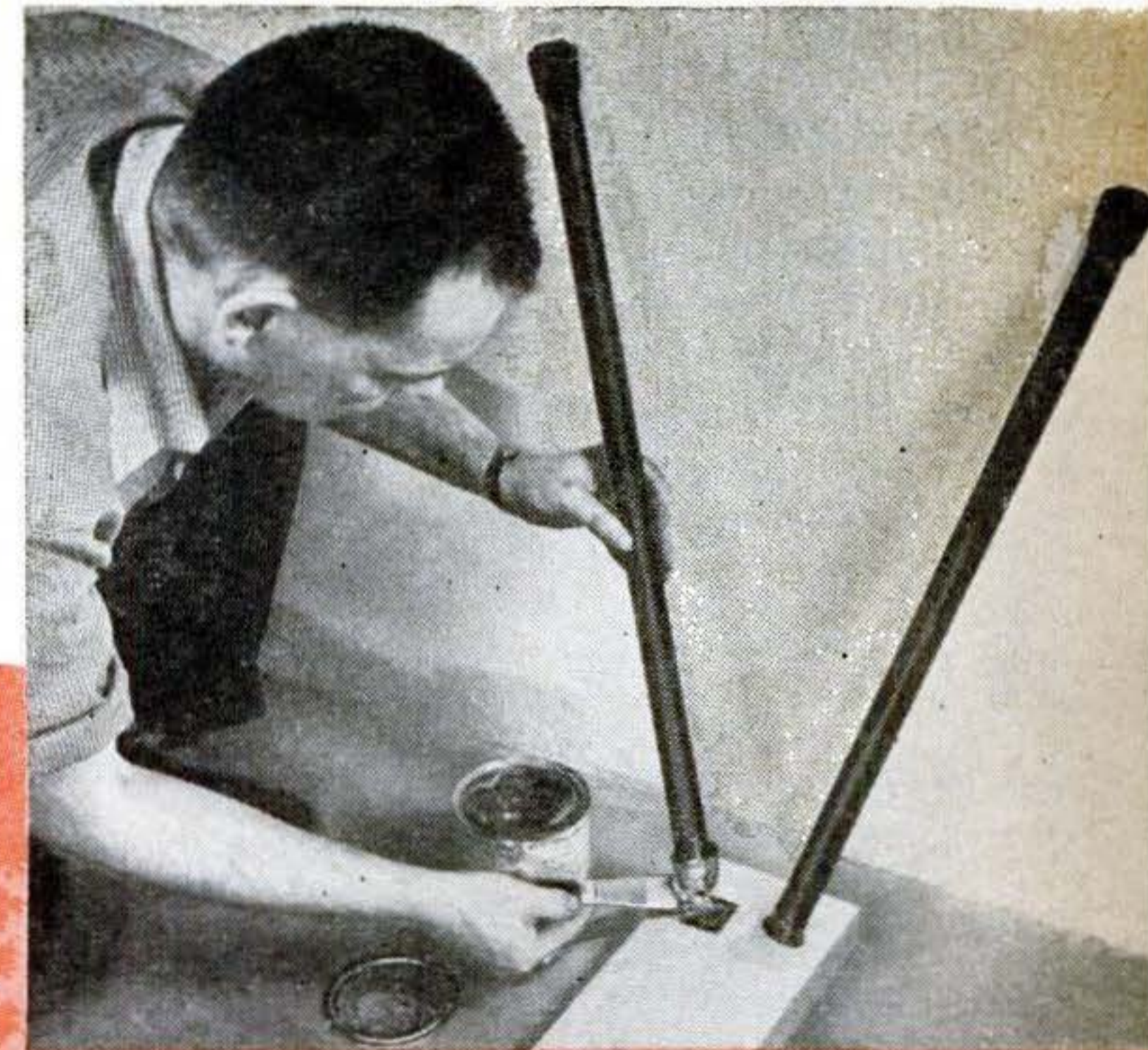
PIPE LEGS are easy to dismantle. Screw caps on 24" lengths of \frac{3}{4} " pipe and use metal-filled epoxy paste to bed the caps in recesses chiseled in the rail. Legs can then be unscrewed. Fit leg ends with rubber crutch tips to save floors.
