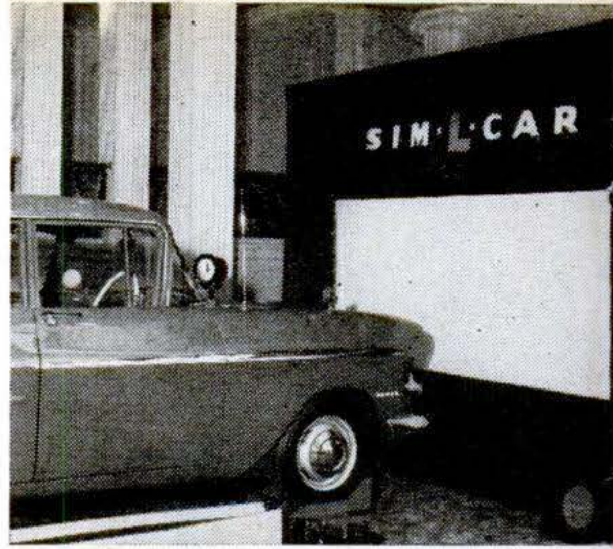
CAR ON RAMP has front wheels mounted on swivels so learner can practice making turns.
