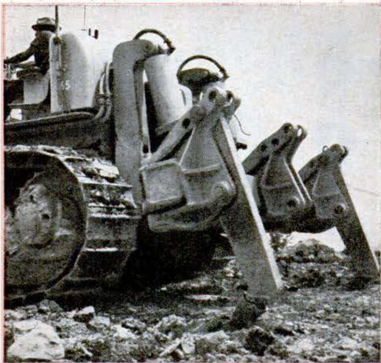
1 HYDRAULIC POWER lowers rippers until rear end of tractor is raised off ground.
