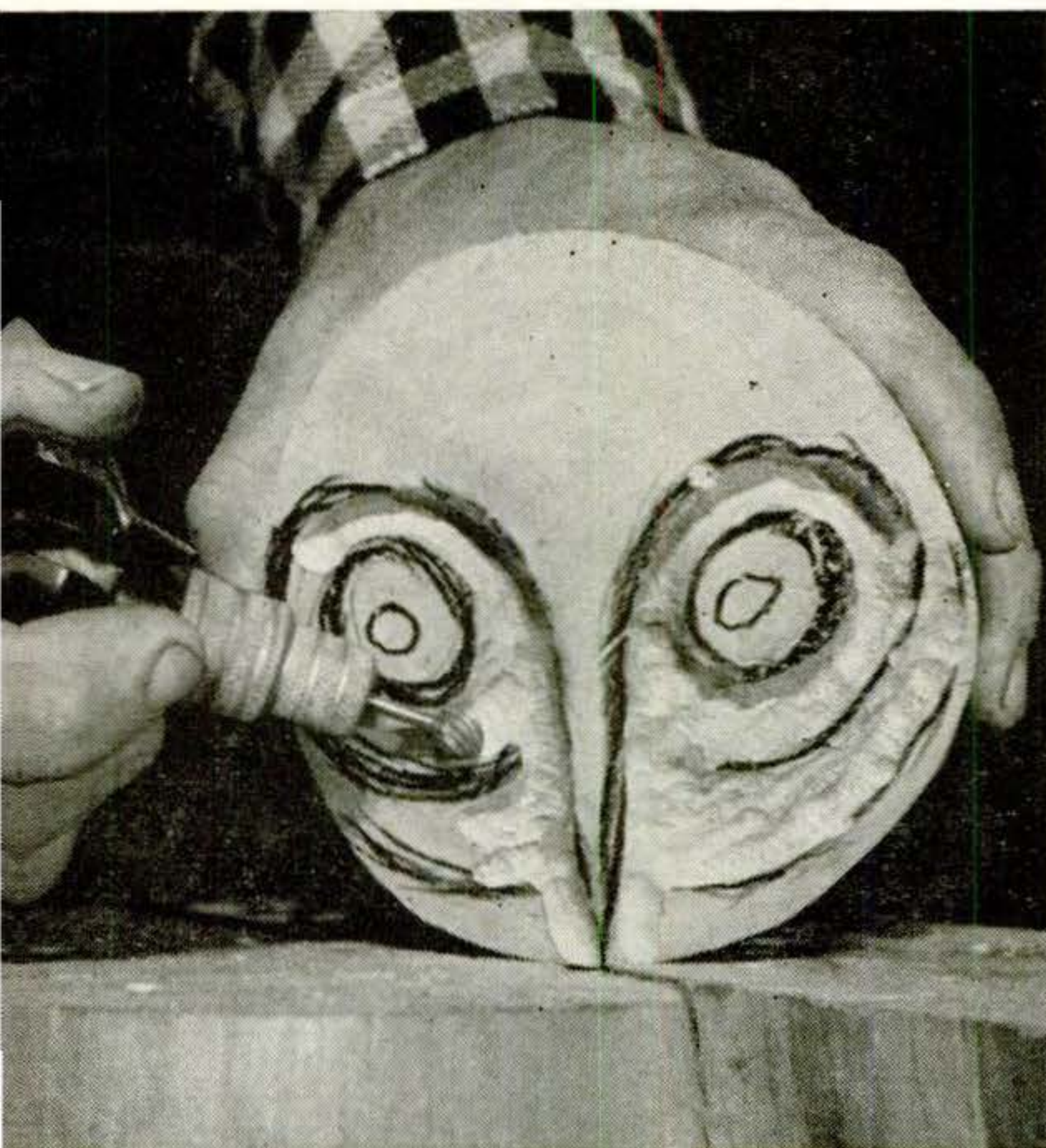
3 TINY ROTARY FILE quickly routs out wood between the lines, leaving high spots. Such files work best in a high-speed hand grinder, but can also be used in an electric drill.
