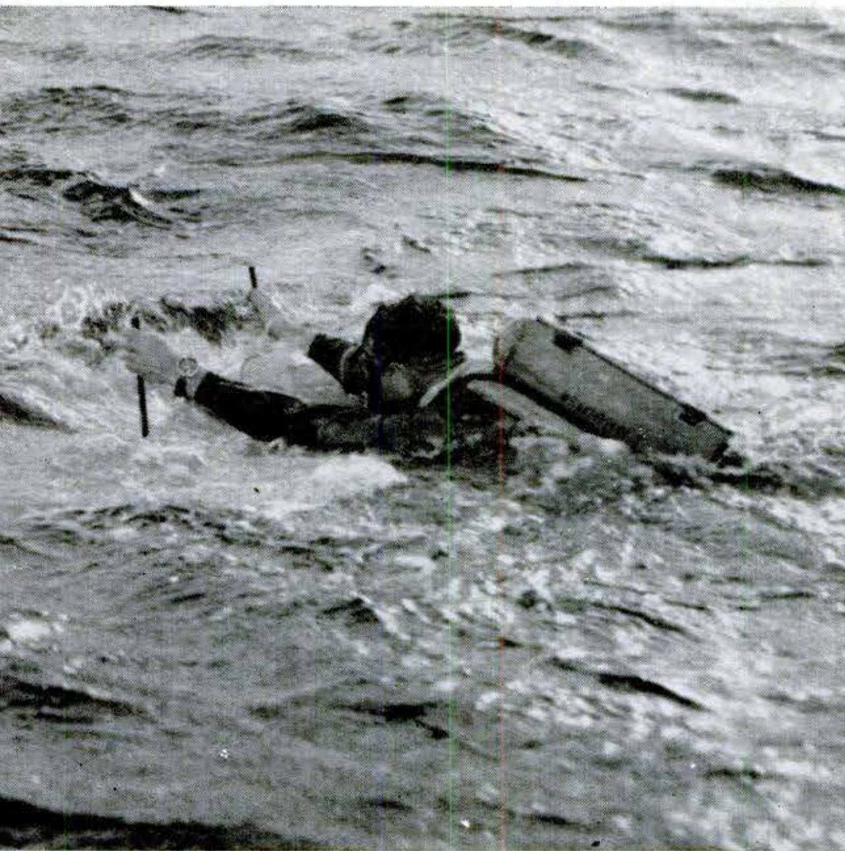
GOING DOWN: A push forward on hand levers tilts hydroplanes at the board's sides for a dive. Usual cruising depth is about 30 feet.
