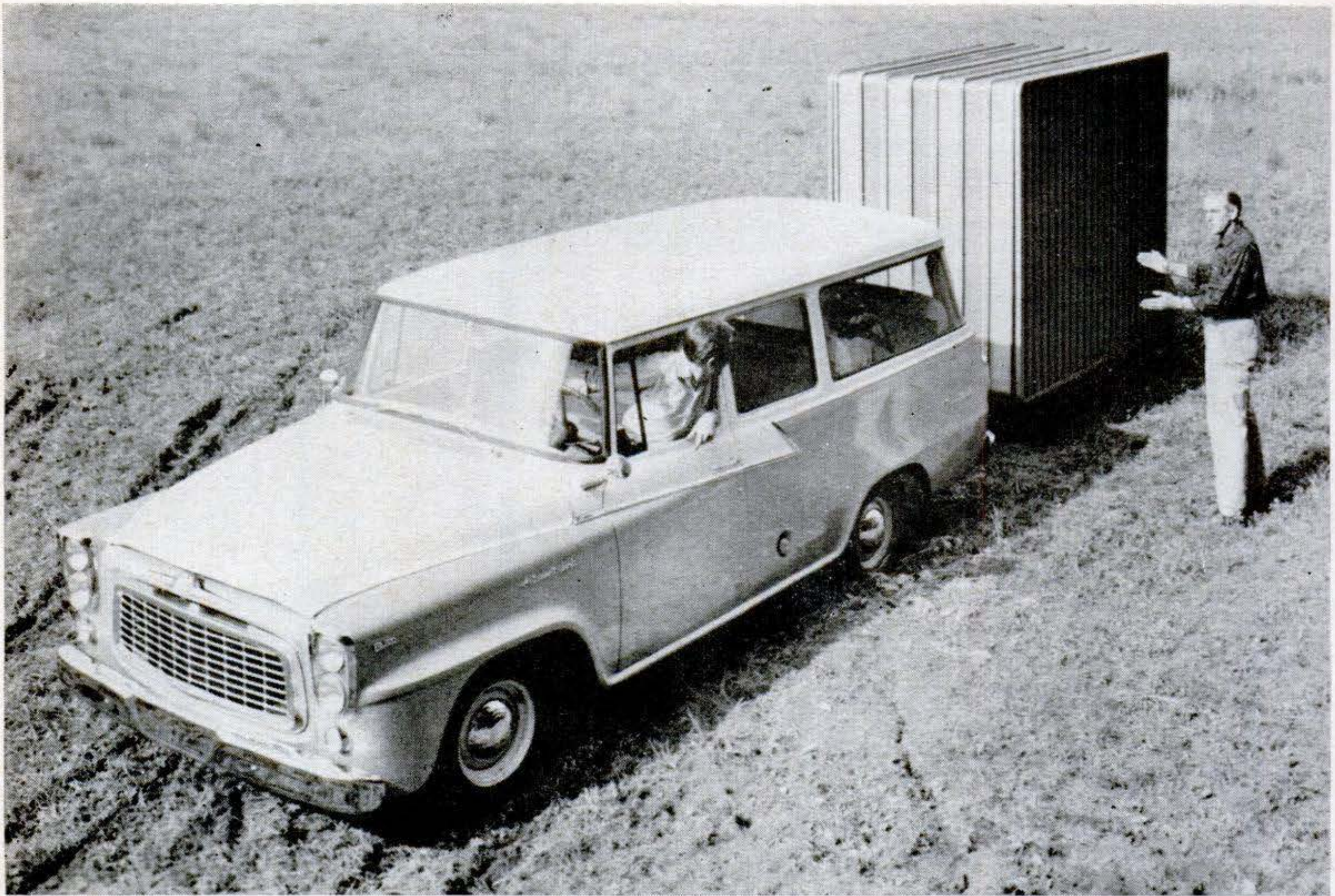
1. FOLDED INTO A COMPACT BOX , this trailer house rides easily on wheels behind a car for on-highway travel.
