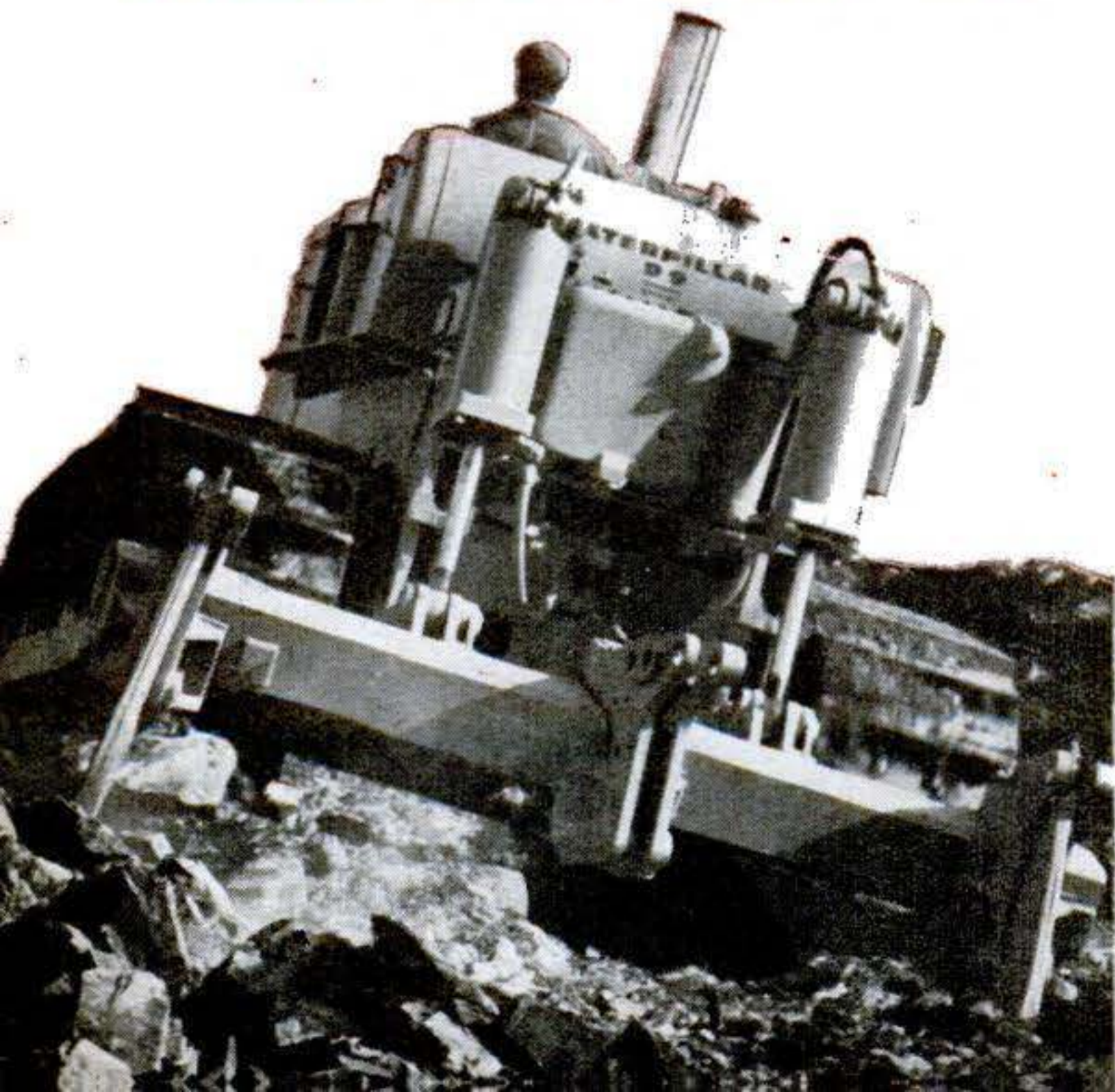
3 TWIN RIPPER TEETH leave broken fragments small enough for scraper loading.
