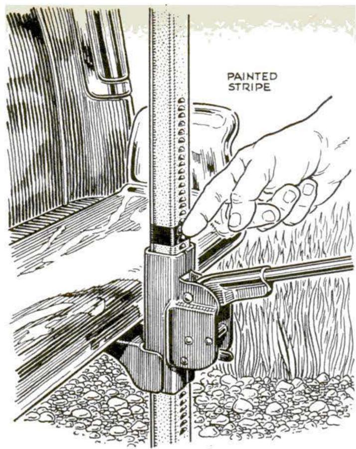
After taking off a flat tire, many motorists find they must jack up the car another inch or two in order to put on the spare. You can avoid this hazard by marking the proper height on the jack stand and raising the car to the mark.
