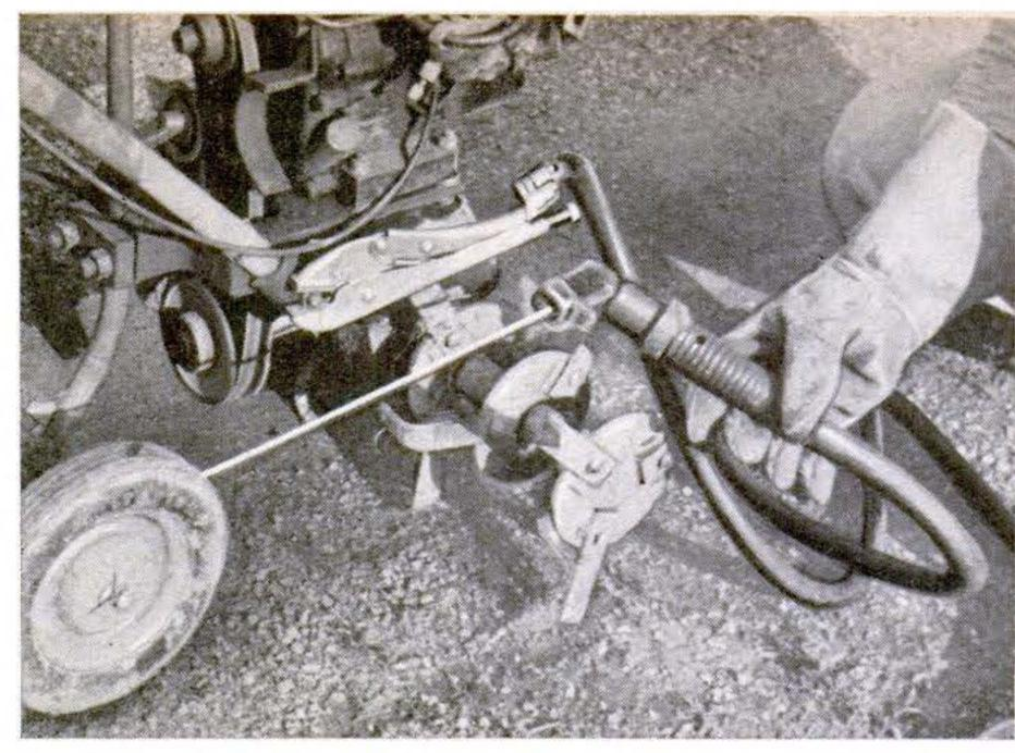
of the work to be welded and know I'll have a good ground until I release their grip.—John Krill, North Lima, Ohio.
