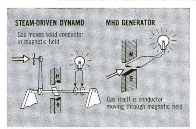
Then its atoms are shaken so hard that electrons come loose and can move around. In the MHD generator, this ionized gas passes between the poles of a magnet. The magnetic field pushes the freed electrons to one side, where they are collected by a contact and fed out to run motors, lights, and toasters. MHD electricity is direct current, and has to be changed to AC for the customers.
