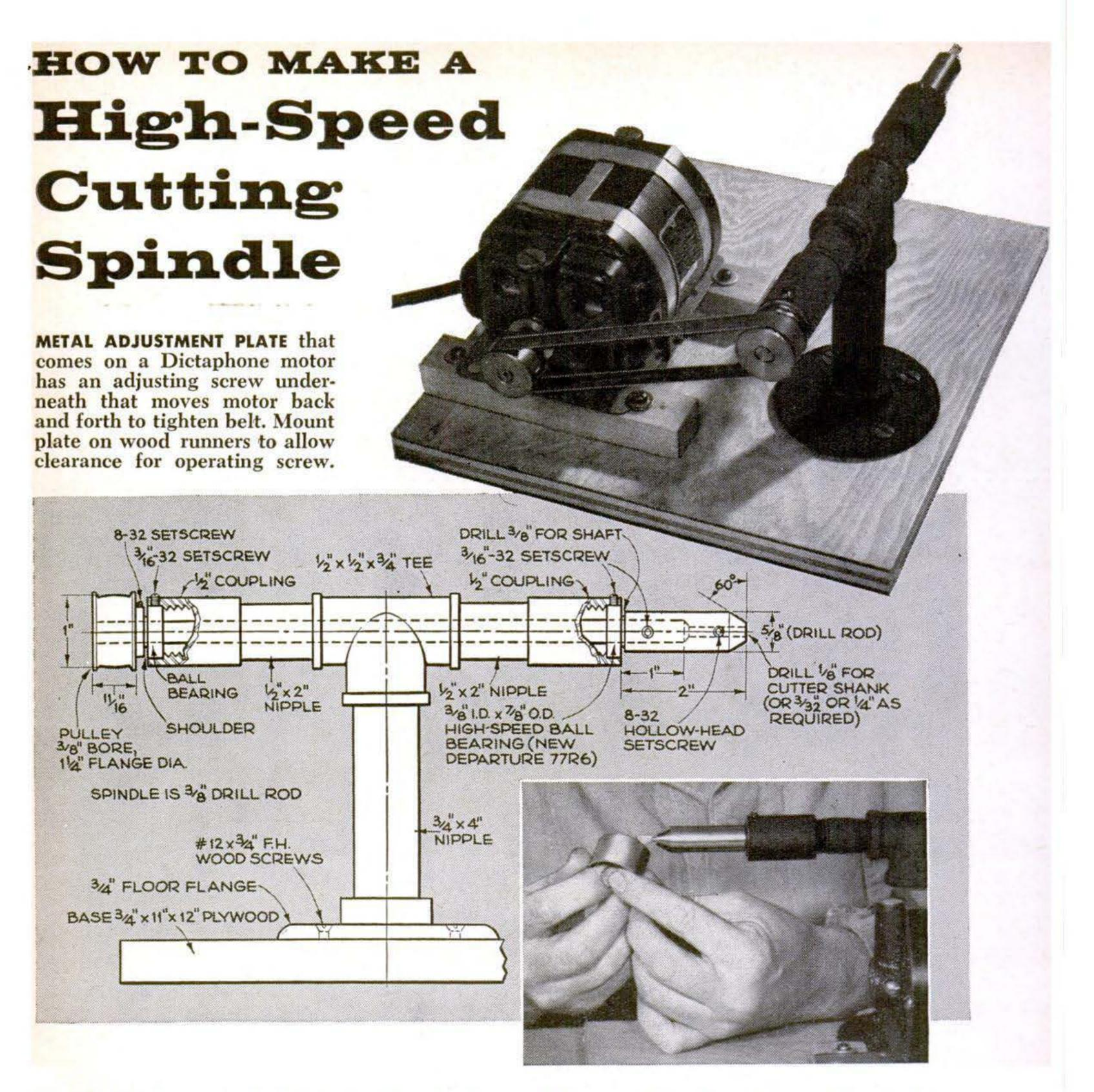
FIT this homemade high-speed spindle with an appropriate cutter and you can easily dispose of many tedious shop jobs. As a freehand milling machine or a fast-working wood-carving machine, it offers new scope to machine, wood-carving, and modelmaking projects.
