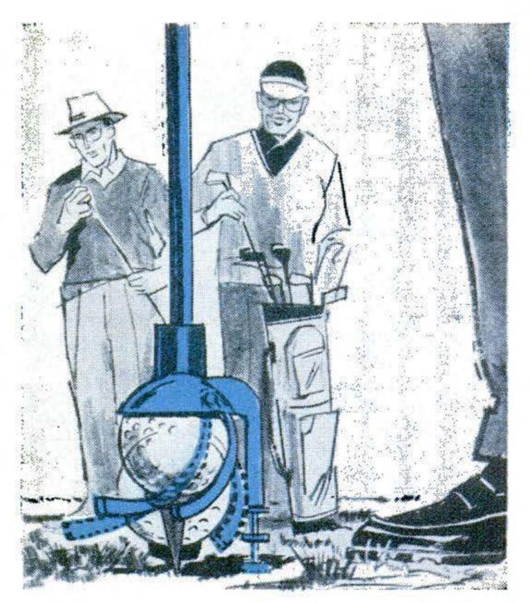
No-Stoop Gripper Tees Golf Ball. You could set up a tee and golf ball without bending if you put a gripper like this on your club handle. You'd place ball and tee between the claws and press the tee into the ground. A ground-contacting plunger would then open the claws.
