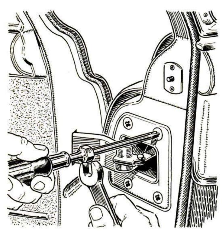
Extra leverage can be applied to a screw-driver with a nut welded on its shank. Press the screwdriver firmly into the screw slot and turn the nut with a wrench. The most stubborn screws can be removed this way without damaging them.
