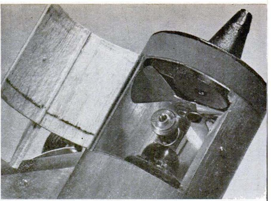
IT'S A TIGHT SQUEEZE for engine and prop inside the barrel fuselage, but you can reach them easily through this large hinged hatch. Prop is spun automatically by spring starter.
