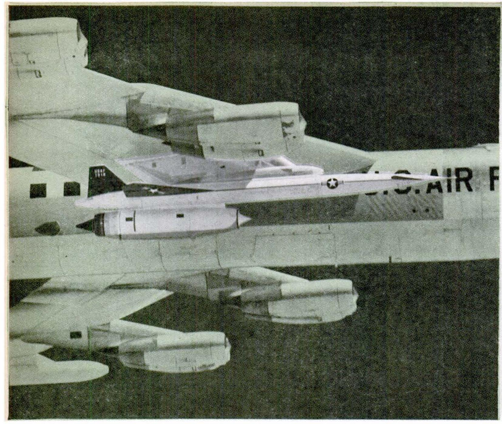
Hound Dog missile, snuggled under the wing of a B-52G, can be instructed on course and target
