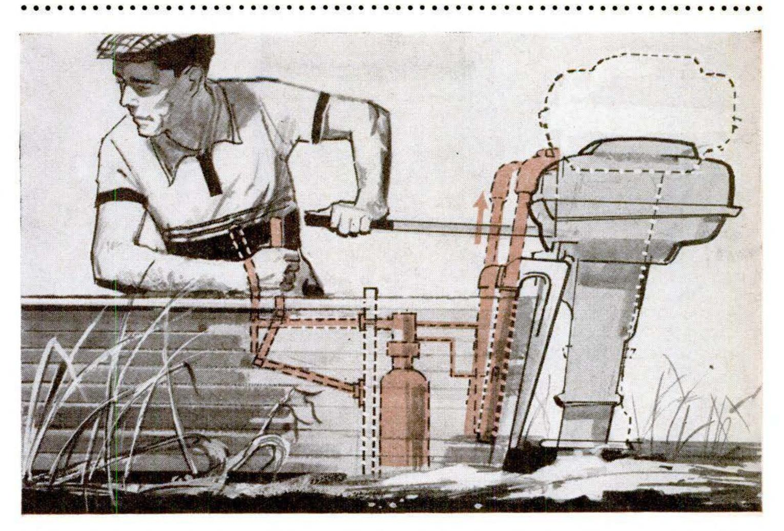
Piston Adjusts Outboard Depth. Instead of tilting or stopping an outboard to prevent prop fouling, you could just pump it upward on this recently patented bracket
