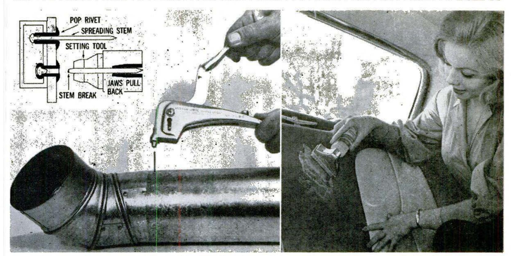
when you can't get behind to back up a rivet. It uses a special rivet, pulling a headed stem through to spread the underside and popping the stem off on the inside. Setting tool and assortment of rivets, \$19.95. United Shoe Machinery Corp., 101 River Rd., Shelton, Conn.
