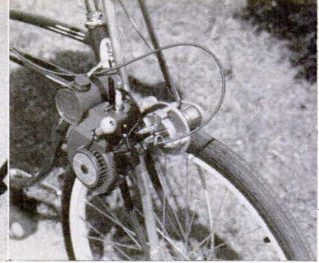
TEN-MINUTE motorbike conversion: Engine mounted on handlebar powers a drive wheel that turns the tire. Savidge Co., Venice, Calif., makes the kit.
