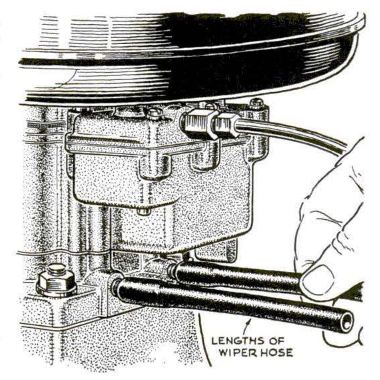
A good idle-mixture adjustment sometimes changes when the air cleaner is put on. A more precise adjustment can be made with the cleaner on the carb by slipping hose over the adjusting screws. Twisting the hose turns the screws.
