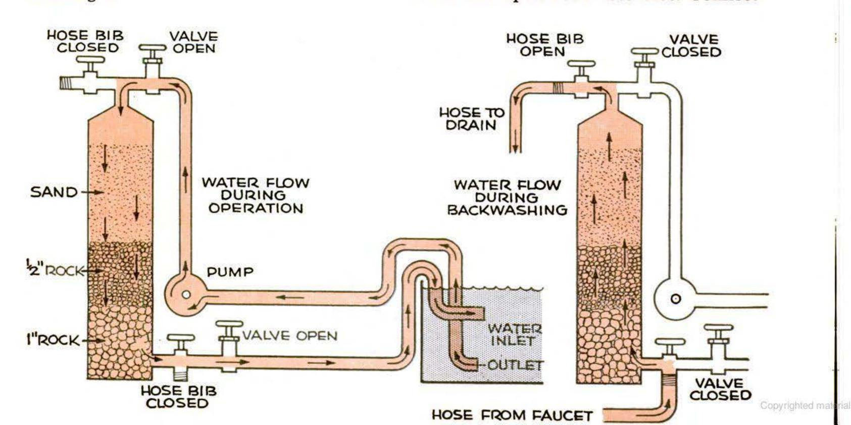
a hose from a faucet to the lower hose bib, and run a second hose from the top hose bib to the nearest drain or sewer.
