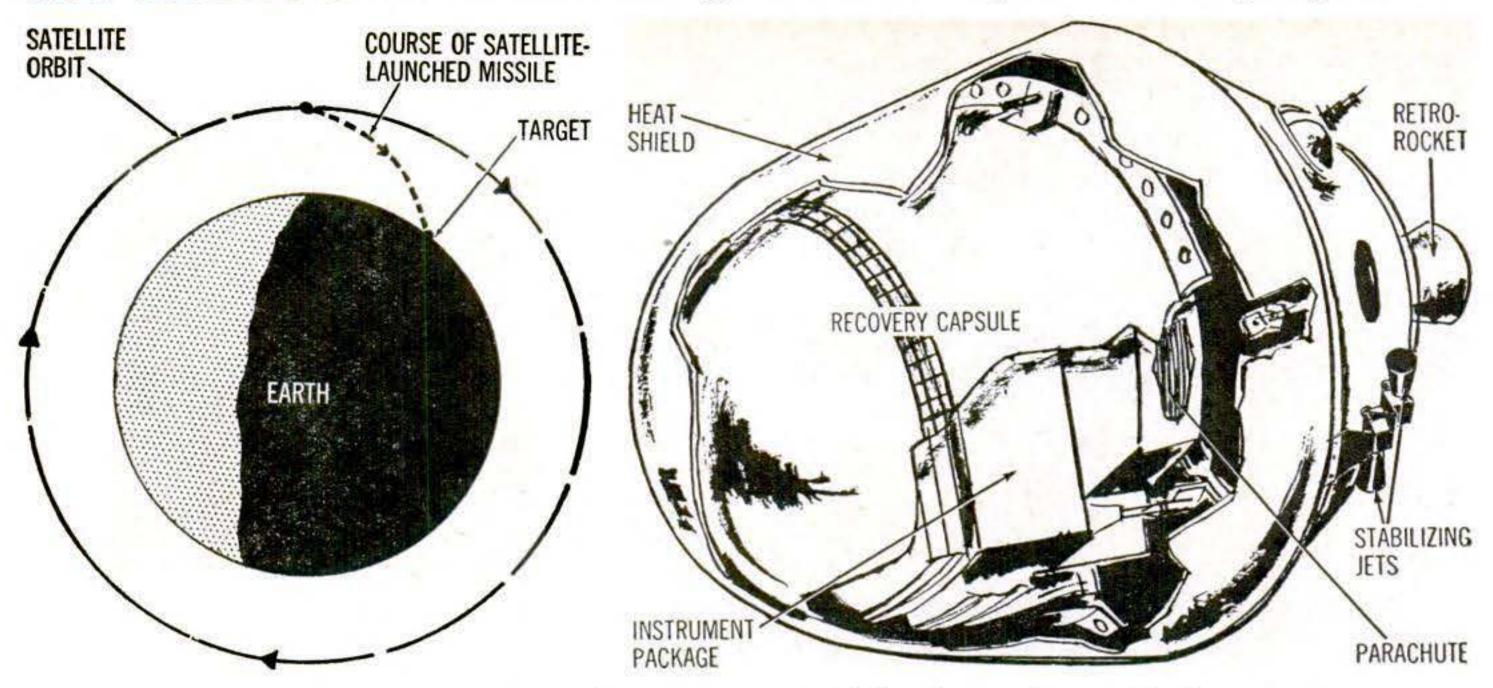
satellite-launched H-bomb missile, firing retro-rocket, would drop from orbit to target on earth. Diagram of trajectory, above, is based on official one in a recent report warning of
