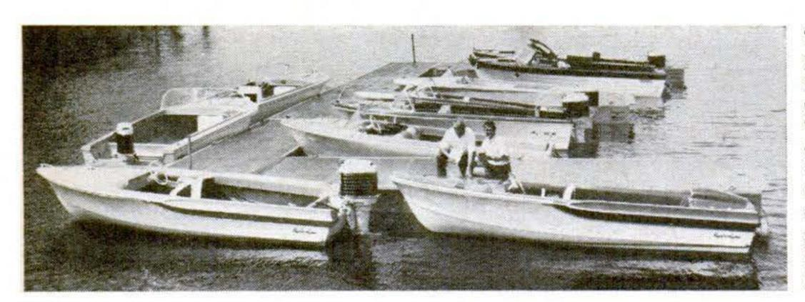
rest boats, five matched pairs of them, were used by author. One of each pair is equipped with an outboard; the other has an inboard-outboard. For most tests, boats were operated side by side. At right, a pair of Glass Magic hulls moves out for fuel and speed tests.
