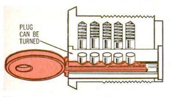
shear points aligned, the key can turn the plug. A notch too low will leave a driver to bar the plug. One too high will raise a pin to do so. Thus a key having but one slightly wrong notch will not free the plug.
