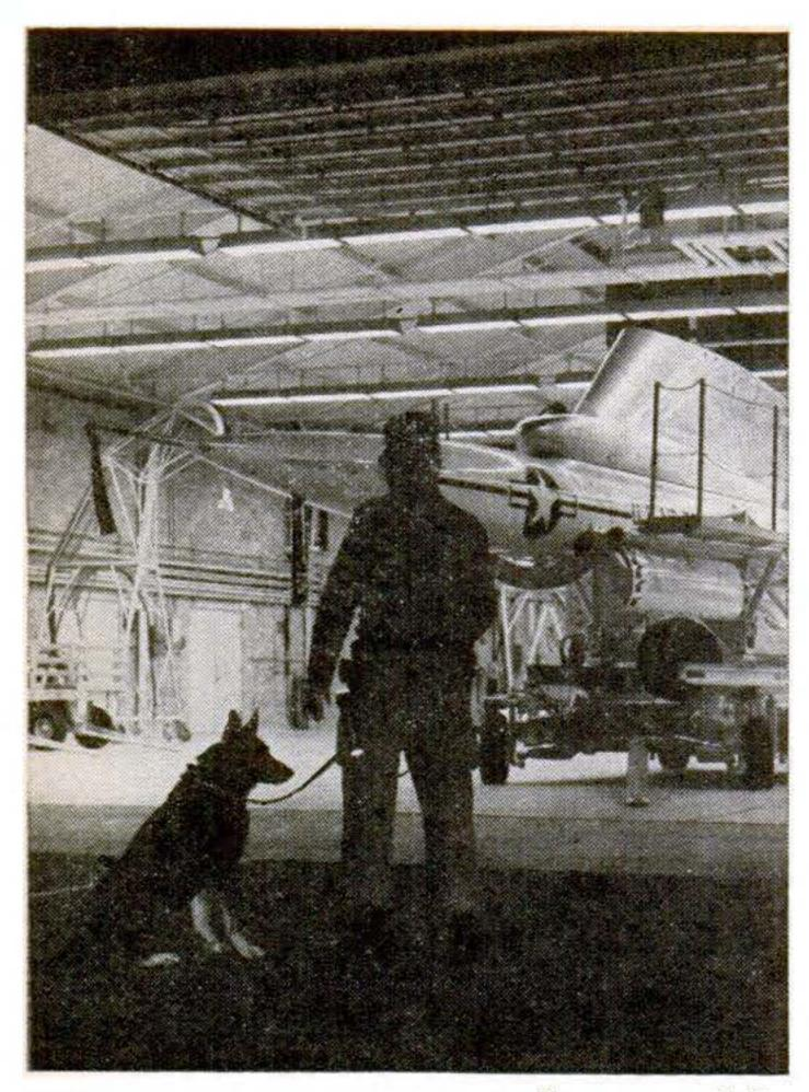
GAM-77 AND ITS PYLON are shown on dolly for inspection and maintenance. The pylon is an integral part of the system, and is used by the missile until the instant of launch.
