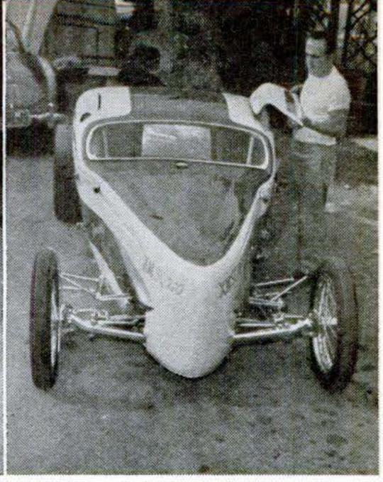
CADILLAC ENGINE is in the rear, just as in a VW—but no VW's innards ever looked like this! Treadless rear tires give maximum traction.
