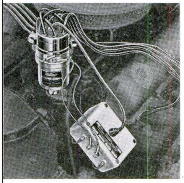
MAGNETO replaces coil and distributor to step up spark. Mini-Mag normally runs as a magneto, but an associated power pack converts it to battery ignition for starting. For car, truck, marine engines, \$125. Mallory Electric Corp., 12416 Cloverdale Ave., Detroit.
