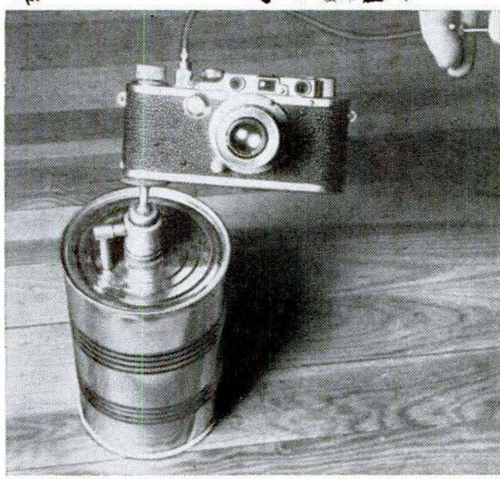
TRY THIS "CAN POD" for those difficult lowangle or table-top shots that can't be made with a tripod. Bolt a small swivel head to a large fruit-juice can, and you'll be able to set the camera at any angle. Cover the lower rim of the can with tape to provide a nonslip edge.
