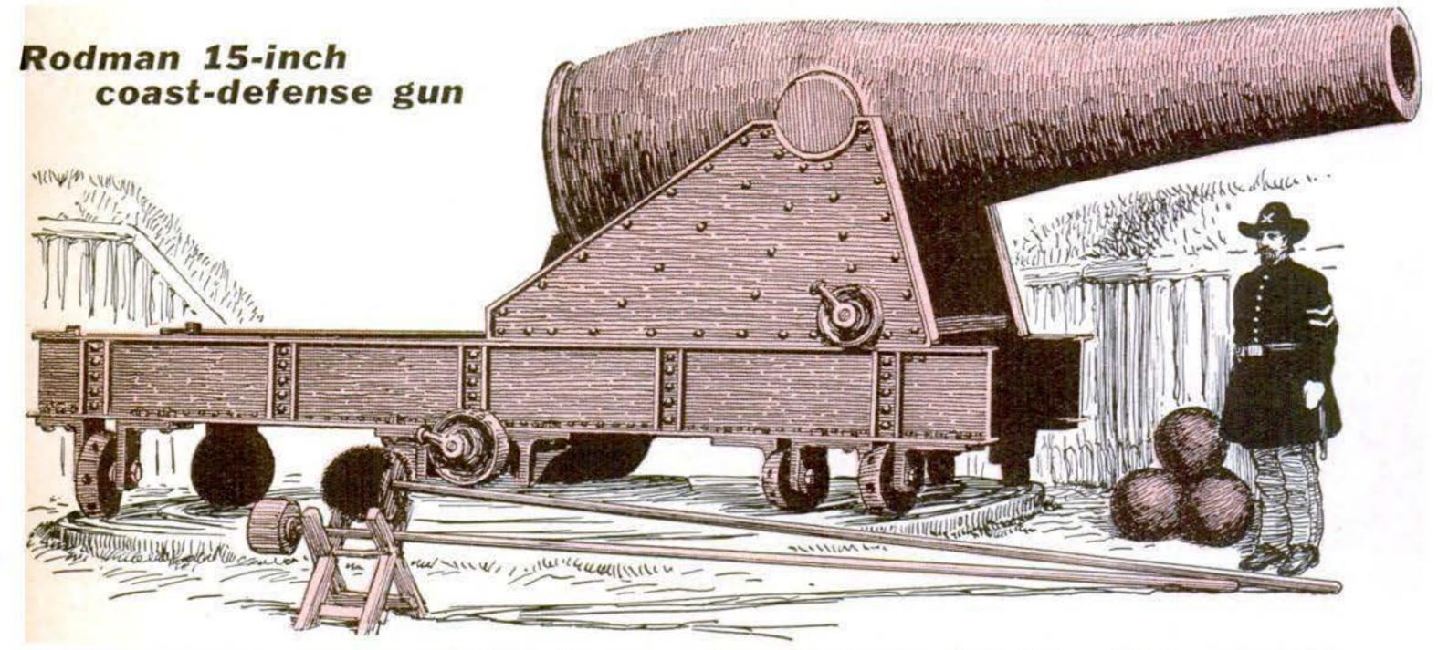
WHEN CAST-IRON GUNS COOLED from the outside, the outer surface was harder than the wall of the bore, and the stresses set up in the metal added nothing to strength. Captain Rodman cast guns around a water-cooled core; the outer metal then tended to shrink and compress the bore. His guns proved stronger than
