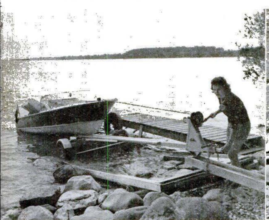
TO HAUL OUT THE BOAT, roll the trailer to end of ramp and use winch to pull the boat onto the trailer. Snap trailer's safety chain in bow eye to keep the boat from rolling back, then slack off the winch and disconnect the line.
