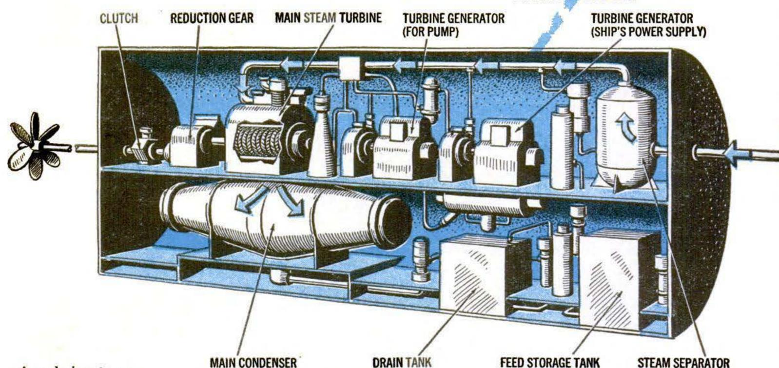
A-sub is steampropelled, adding complications that diesel-electrics avoid. Steam turbine turns propeller through reduction gear. Seagoing Nautilus has twin turbines and screws (one shown above).
