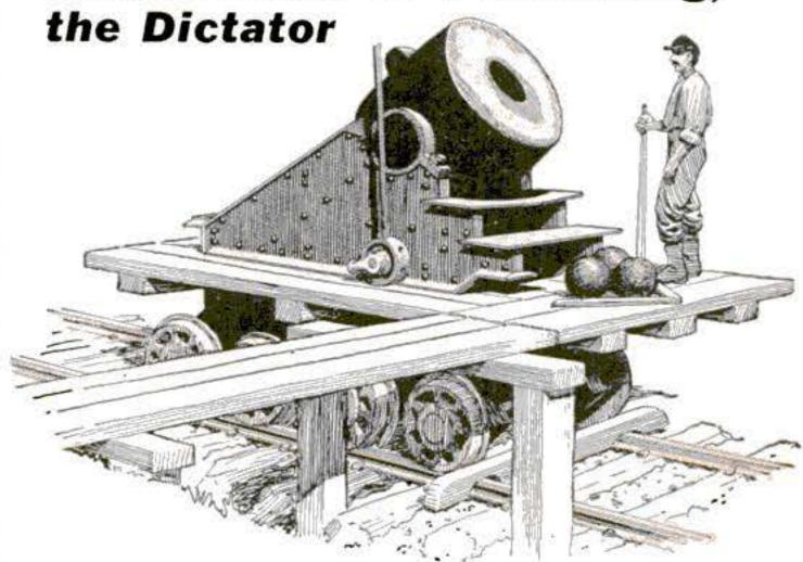
THICKER (45 inches across) than long, it fired a 13-inch shell. Its first flatcar collapsed under the recoil.
