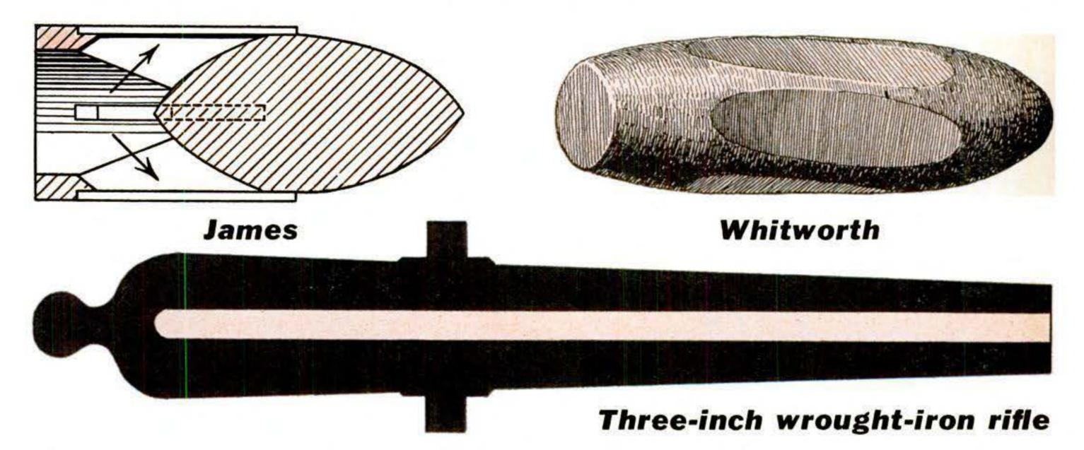
CHARLES T. JAMES' PROJECTILE (above, left) served the big converted siege rifles and the three-inch wrought-iron rifle. A deep depression in the base of his shell was slotted to allow gas to press outward against the sheet-lead sleeve that surrounded the base of the projectile, forcing it into the rifling.
