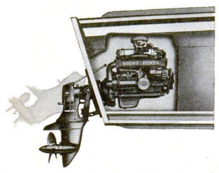
**VOLVO AQUAMATIC DRIVE** is transom-mounted with vibration-damping rubber supports. Engine power is transmitted from the crankshaft through a Rzeppa universal joint that allows the outdrive unit to pivot or tilt in relation to the drive shaft. The tiller telescopes into a tube when the unit is tilted. The lower drive head is similar to that of an outboard.
