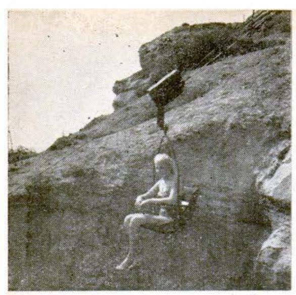
abrupt 85-foot drop below is a thrilling experience. Chair and trolley are supported by 7/16-inch high-strengthalloy messenger cable; a 1/4-inch aircraft cable pulls the trolley.
