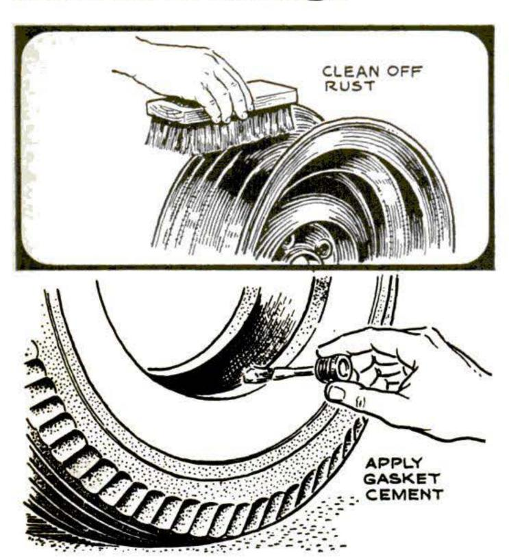
Tubeless tires that leak at the bead can be made airtight by cleaning the wheel rim and applying gasket cement to the rim and the tire bead. Overinflate the tire about 10 pounds to insure a good seal, then reduce pressure to normal.
