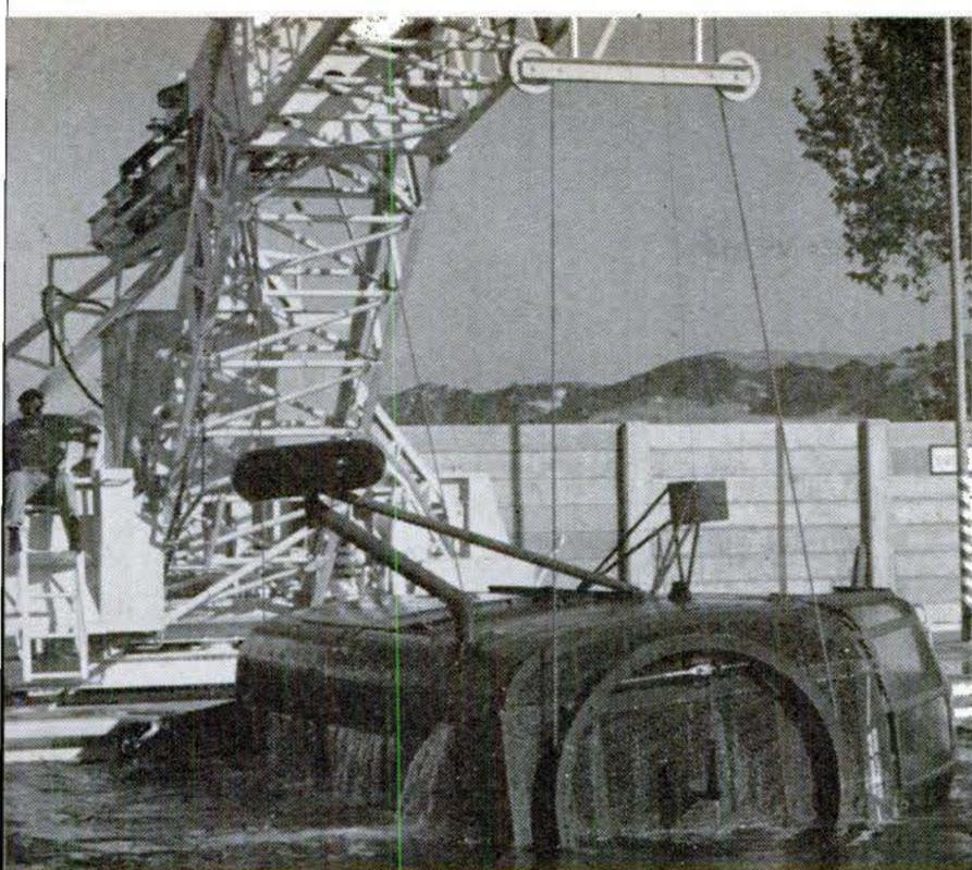
2. OVER AND UNDER: Mechanism is capable of ditching at various angles. Here the fuselage strikes surface on one side and submerges.
