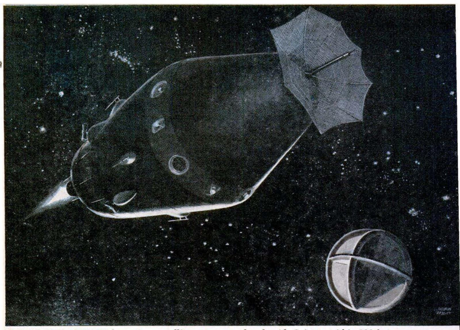
"SAINT" ANTI-SATELLITE inspects a satellite, as in coming trials. In likely design pictured, retro-rocket and umbrellalike radar antenna
