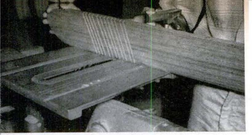
closely spaced saw cuts permit tip of ski to be curved easily after soaking. Slots are 3/8" deep and 1/2" apart. They can be made with a handsaw if blade is carefully kept level.
