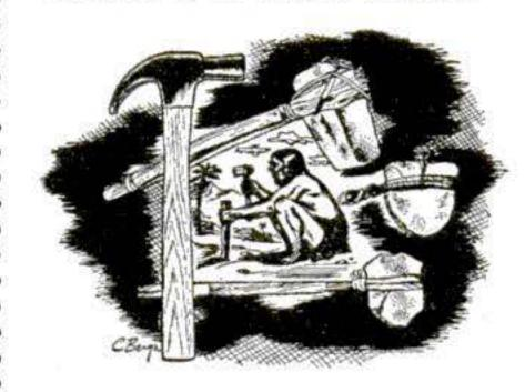
HAMMER: nearest rock was man's first striking tool. Later, Stone Age man used a rounded stone to flake other stones into a hammer shape, and tied on a handle. The handle was made more secure when Neolithic man learned to make shaft holes. The first metal hammers of modern form appeared about 1500 B.C. By early Roman times, the familiar claw hammer was in the carpenter's kit.
