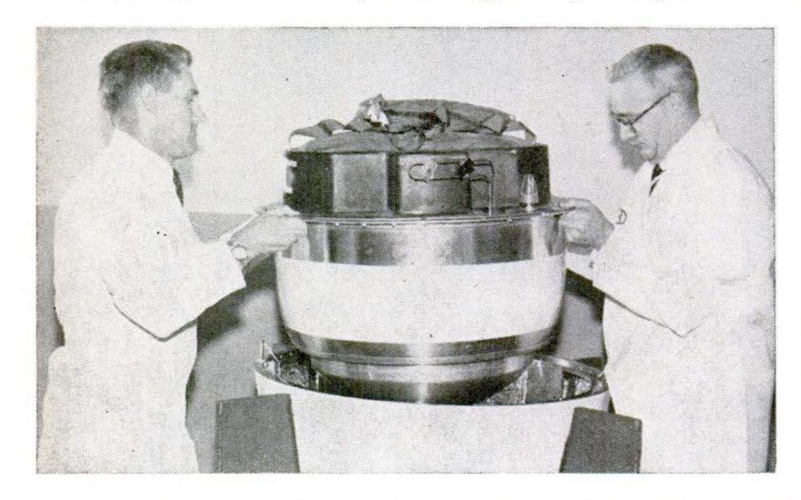
FIRST OBJECT ever brought to earth from orbit was Discoverer capsule. Photo at left shows it being lowered into heat shield that protects it from high temperature and shock of passage through atmosphere. Then parachute opens and lifts it free, for final approach to earth. Discoverer capsules range up to 350-pound size. A version not much larger (600 pounds or more) could hold an H-bomb.
