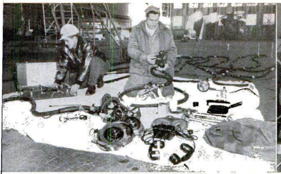
DIVING GEAR is laid out for inspection by divers before they enter a gas-filled bag. Each man usually gets 250 feet of air hose.
