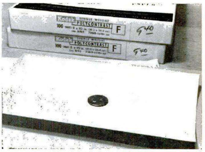
IS YOUR SAFELIGHT SAFE? Here's how to tell. Place a coin on a sheet of photographic paper for two or three minutes, then develop the paper. If the coin's outline shows up, it means the light is too bright. Dim it with a lower-wattage bulb or move it farther away.
