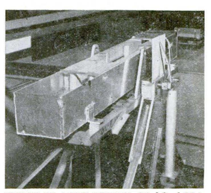
coming up: DIRTY WEATHER. Model of Matsonia's tank is bench-tested at Stevens Institute of Technology. Under controlled rocking, the behavior of water is measured electronically.
