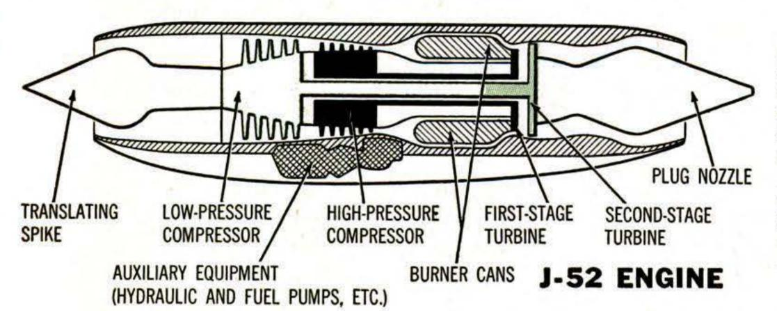
has a "translating" inlet spike that moves out automatically as speed increases, keeping sonic shock wave from entering inlet and choking off airflow. This movement also adapts inlet area to varying speed and altitude.
