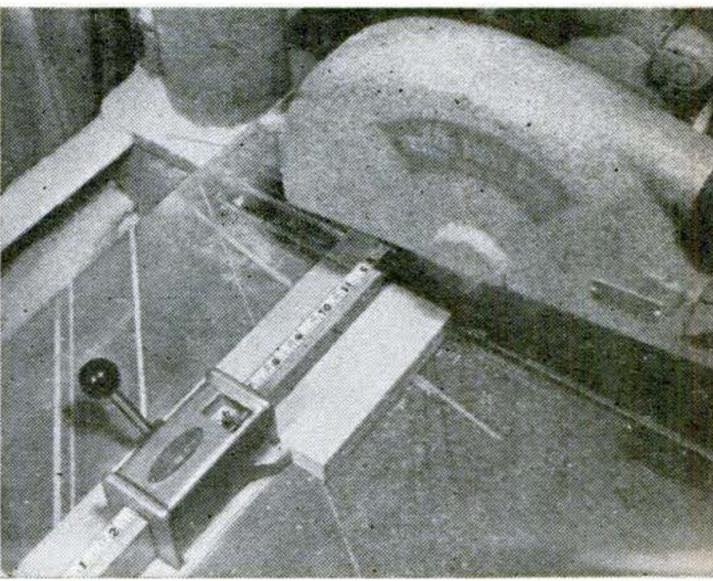
SAW STOP lets you cut duplicate parts to precise length with one setting. The aluminum casting fits over a tape recessed into top edge of any hardwood backstop 25/32 to 13/15 inch thick. Numbers are read through window with help of a pointer. Right- and left-hand versions for radial, swing, band, and table saws with miter-gauge groove. \$7.50. Rex Mfg., Box 253, Fontana, Calif.
