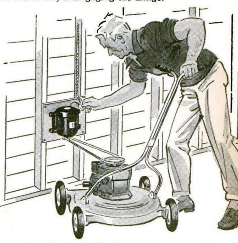
WHAT COULD BE SIMPLER? A. W. Aiken mounted a motor upside down on a garage wall to spin his rotary-mower engine until it starts. Moving mower toward the motor releases the V belt.
