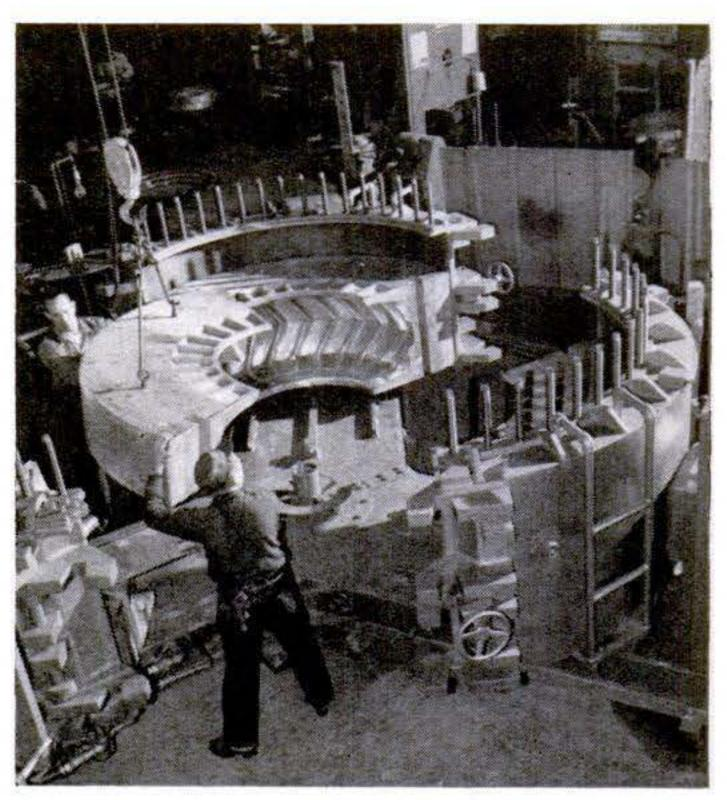
TIRE RETREADER. This machine will be put into operation at Firestone's plant in Portland, Ore., to retread giant truck tires. It can handle 1,100 pounds of rubber, vulcanizing it on a carcass in 16 hours under 150 tons of pressure.
