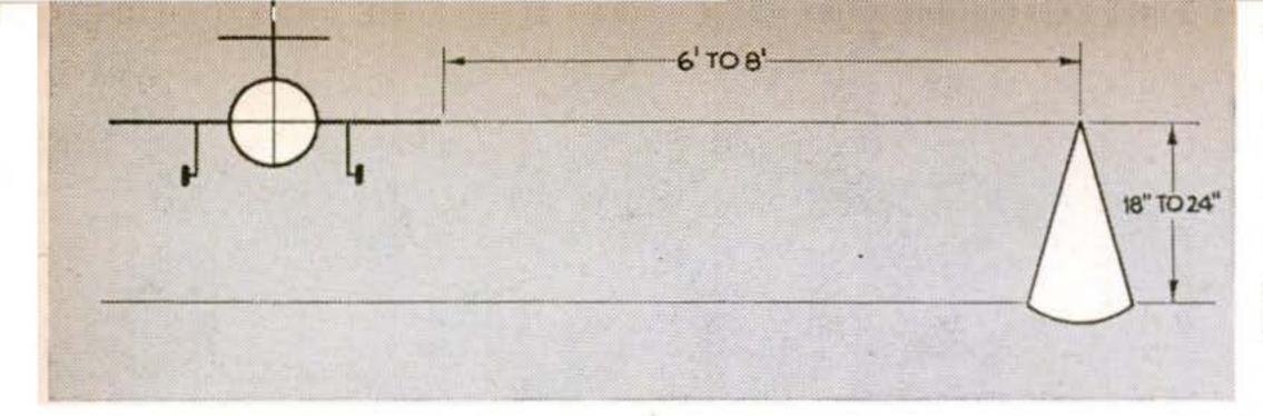
the ducted fan flies best close to earth with the tether level. Use a low pylon and a short line, and adjust the ship so it flies at a fixed altitude of about 2'.
