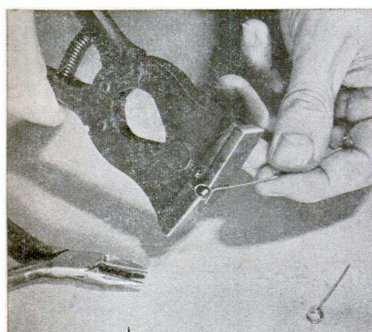
NEAT, ROUND LOOPS can be made by bending the wire a full turn, then a half turn, and snipping off the overlapping end. Special cutters with hardened steel jaws should be used.
