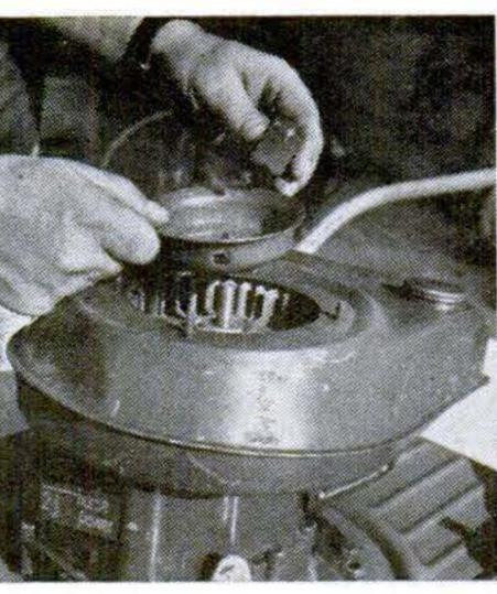
move rope-starting attachment (sometimes a pulley).
