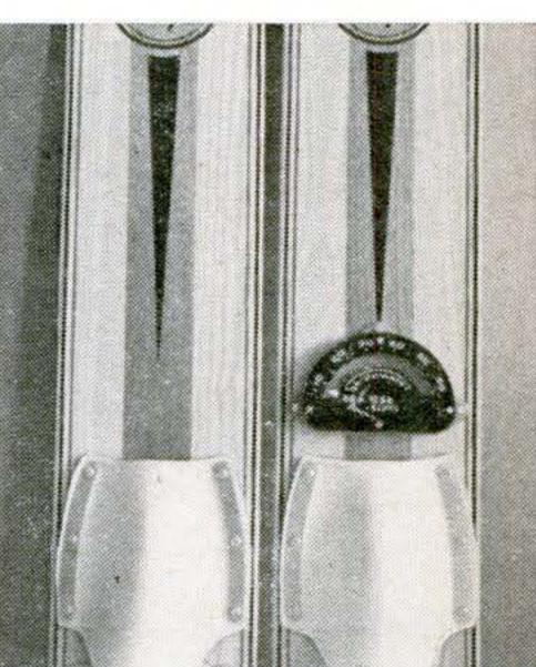
SPEEDOMETER is designed for water skis to record your speed on sharp turns and cuts that often double the rate of your towboat. Drill hole for its Pitot tube and fasten plastic case to one ski. Price, \$7.95. Nash Mfg. Co., 312 West Ripy, Fort Worth.
