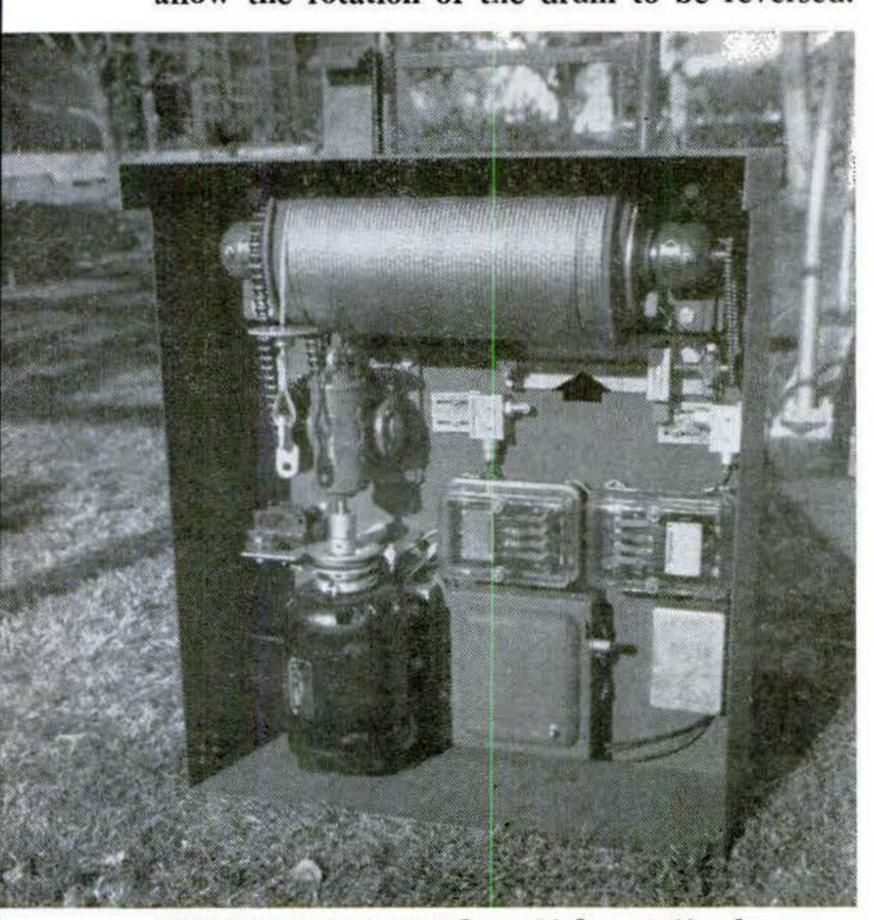
A threaded rod (arrow) is connected by a roller chain to the cable drum and turns with it. When the cable is fully wound or fully unwound, a threaded block screwed along rod opens a limit switch and shuts off the motor.
