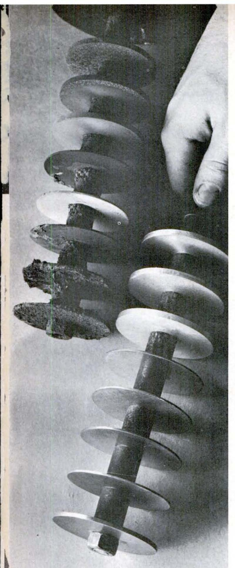
In a six-week test, discs of these cooling system metals were inserted in DOWGARD Coolant and also in a solution of a good antifreeze and water. The difference between the two sets of discs was remarkable. Those taken out of the antifreeze-water solution showed definite signs of rust and corrosion. On the discs which had been in DOW-GARD—not a speck!
