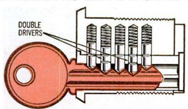
INDIVIDUAL KEYS for the two locks above both raise the two-part drivers only to their first shear points (see above). Below is a master key inserted in the first lock. Three of its bittings are the same as corresponding ones on the individual key. The two that lift the two-part drivers, however, are higher and raise them to the second shear points so the lock can be opened.
