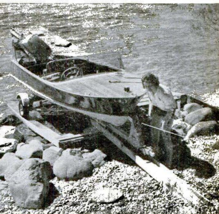
TIE WINCH LINE to a tree or stake driven into the ground ahead of the ramp, and crank the winch to pull trailer and boat up to top of the ramp. A little grease on the tongue runner will make the trailer tongue slide easier.
