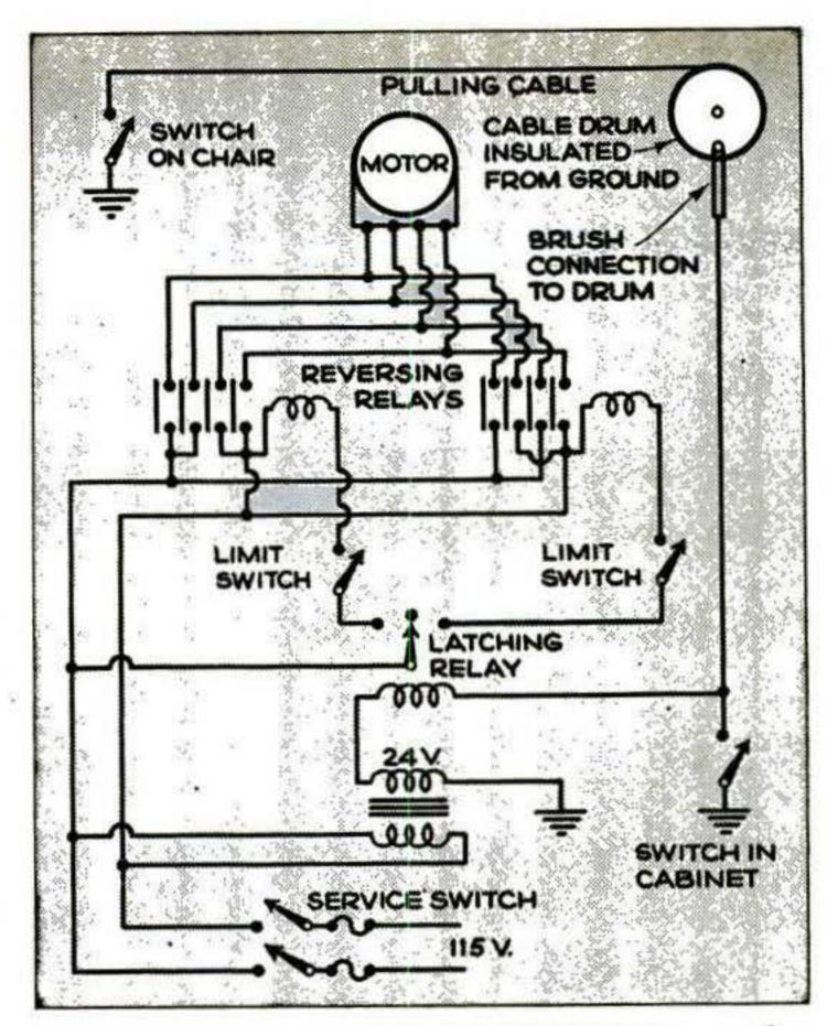
LOW-VOLTAGE STEPPING-RELAY SYSTEM uses the pulling cable as the control wire (this is safe, since the wire carries only 24 volts) and the load-carrying cable as the ground line, to keep the wiring simple. Relays leading to the motor allow the rotation of the drum to be reversed.
