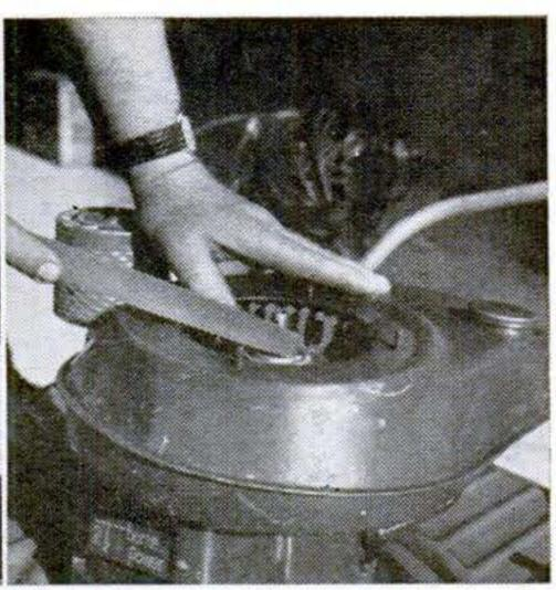
FILE A FLAT, approximately 3/16" wide, on one side of the threaded engine shaft.
