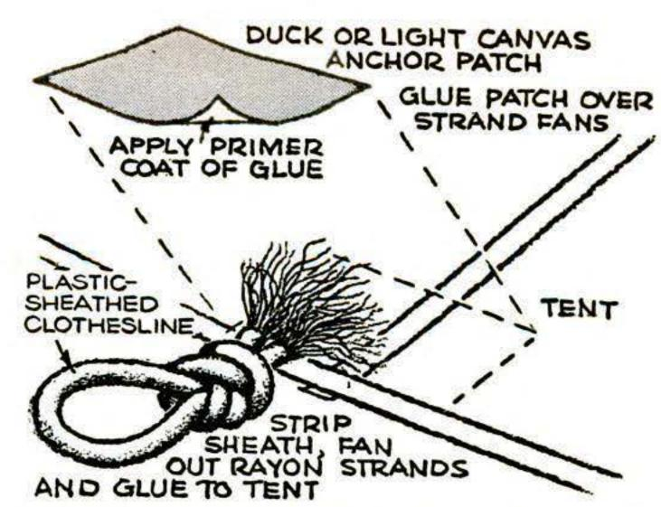
FOR RUGGED TRAIL USE, tents can have separately applied stake loops, instead of extensions of the tapes. Let the primer coat set before gluing the patch over the strands.
