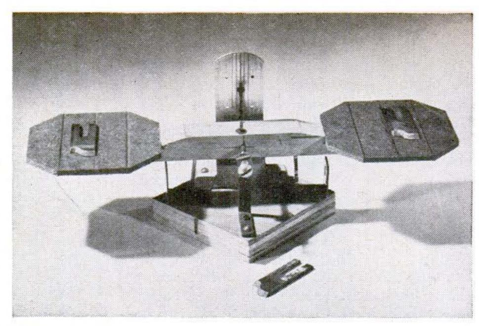
on the scale to check the weight of each against the others. If one knife outweighs the others, grind off a bit more until it balances just right.—Andrew J. Poggi, South Norwalk, Conn.
