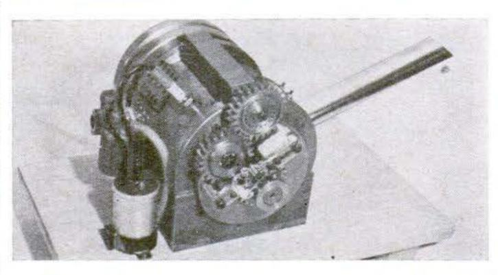
The picture shows, on the left, the carburetor and ignition coil; at right, the exhaust stack. The gears at center turn the bypass shaft.
