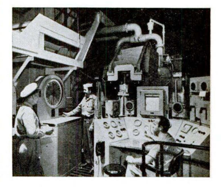
With no place to go, landlocked sub engine lacks prop. Drive shaft ends in water brake—big paddle wheel in tank (background), which absorbs power, indicates output on scale (left).
