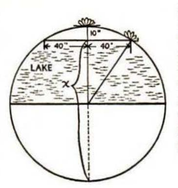
Water lily. Think of the lily stem as the radius of a circle. The water's surface is a chord perpendicular to the radius. The product of the segments of a chord equals the product of the segments of the diameter perpendicular to it:
