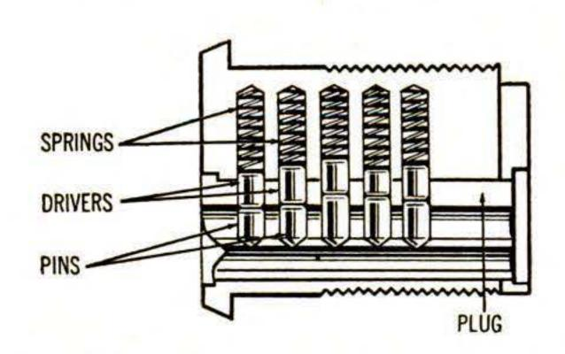
with key out, all pins are pushed against the lower keyway ridge. Partly in cylinder, partly in plug, the drivers keep plug from being turned, have greater shear strength than anything that can be inserted to force it.
