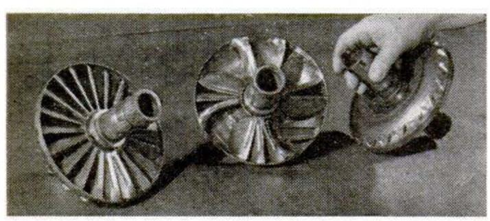
A CUTE TRICK that helps explain the success of good rebuilding is shown above. Usable sections of two damaged fluid couplings at right are salvaged to make one good coupling, shown at left, for a Jetaway transmission.
