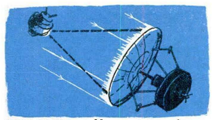
solar mirror would concentrate sun's rays to "cook" a satellite, putting its heat-sensitive electronic gear out of commission.
