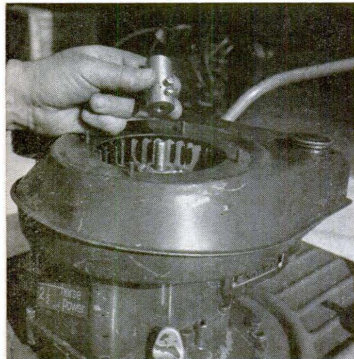
FASTEN SHORT EXTENSION—a motor-shaft arbor, or rod bored to fit—on the end of the shaft.
