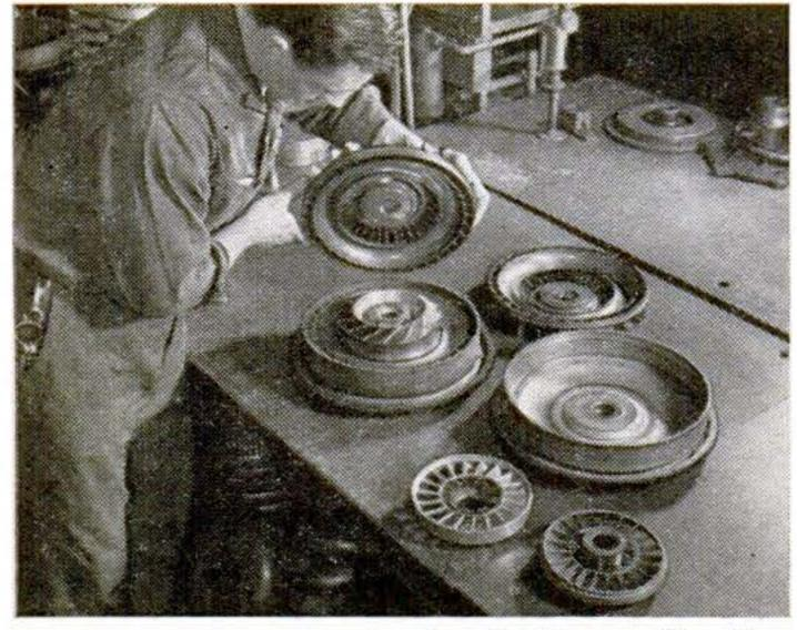
tween engine and transmission. Some, like these Chrysler converters, are factory-sealed. The rebuilder cuts them open, restores their innards, and then welds them back together.
