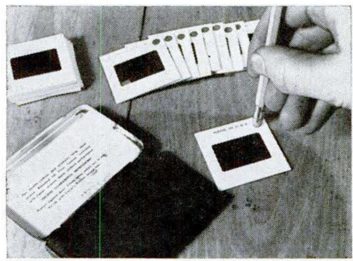
YOU CAN MARK SLIDES QUICKLY for correct projection with an ordinary pencil eraser and an ink pad. Arrange the slides in the proper upsidedown and left-right order, then stamp a dot in each upper right-hand corner. You'll be able to spot the dots even in dim light.
