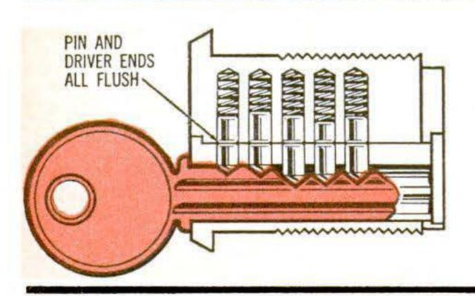
rounded pin ends ride over key bittings until each settles into its own notch, whose depth brings shear point between driver and pin exactly to surface of the plug. The right key aligns all five.
