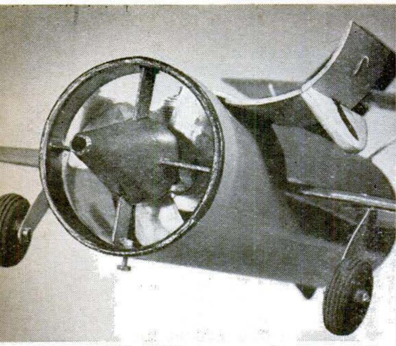
**SPIKE-SHAPED NOSE** squeezes air ahead of the prop, speeding it up and adding thrust. Note obstruction-free fuselage and wide-set wheels—nothing to foul up a fast, safe landing.
