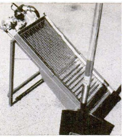
DRY CONCENTRATOR separates gold from dirt. Engine-operated bellows under rippled lower end blows up sand and leaves the heavier gold particles.
