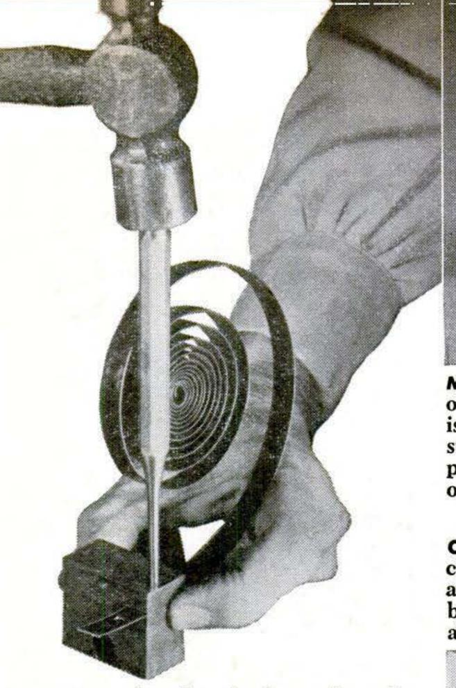
A CLOCK SPRING that has broken off at its anchor point can be reset if you know how to make new holes for the screws. A steel block, slotted and drilled through for a pin punch, will help you make neat holes in a flat spring.
