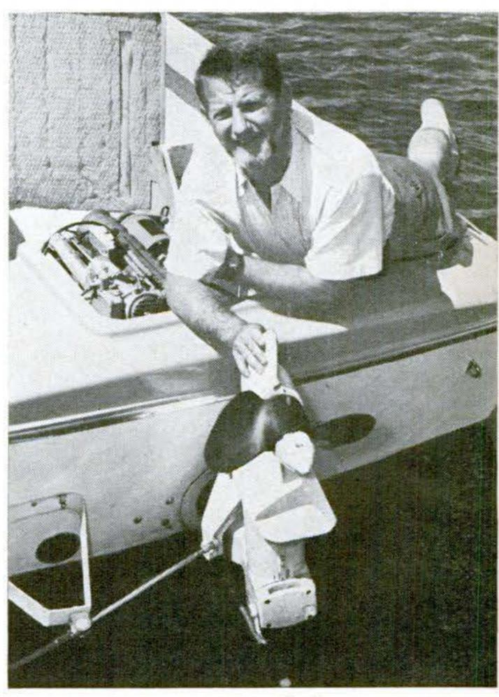
FULL-PIVOTING FEATURE of the Eaton Powernaut allows lower drive unit to swing up through 180 degrees. It takes plenty of muscle to swing it, but this feature could prove handy for a deep-water prop change or inspection.
