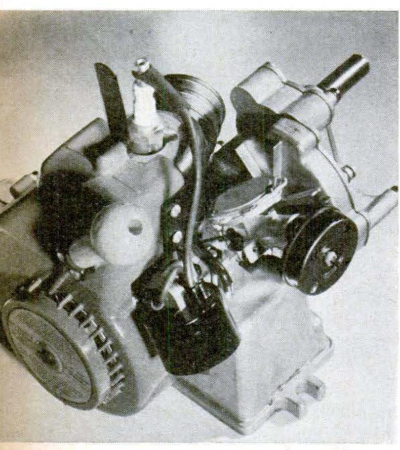
DIAPHRAGM-TYPE CARBURETOR lets Ohlsson & Rice engine run in any attitude, even inverted. Sensitive air-vane governor cuts in and out with eye-blinking quickness. Recoil starter and choke control provide easy starting.
