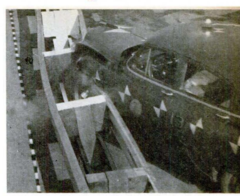
TRAVELING AT 60, a radio-controlled car piles into a divider in tests run by California highway engineers. Car received \$900 damage; dummy inside took a peak 18-G deceleration.
