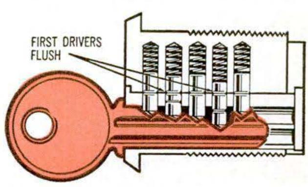
THE SAME MASTER KEY inserted in the second lock lifts its two-part drivers also to the second shear point, which is the same in both locks. A key that lifts one driver to its first shear point and the other to its second could be made for one lock, but would not open the other. Further master-keying possibilities might be achieved by doubling more than two of the drivers.
