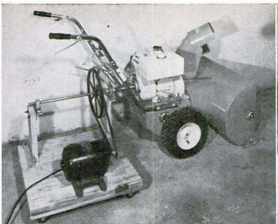
COLD-STIFFENED 41/2-HP. ENGINE on this snow blower starts easily in spite of freezing temperatures when Herbert Phillips cranks it with notched flange driven by a 1/2-hp. motor. Close-
