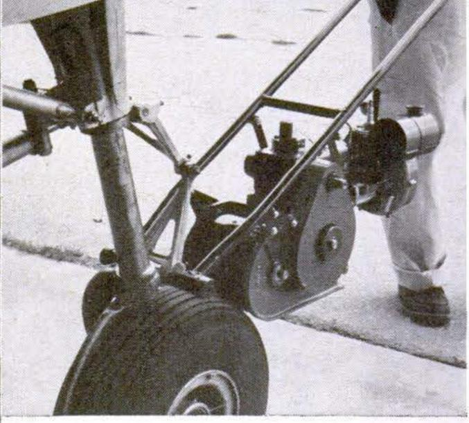
O & R engine is attached to landing gear. Pressure on the handle forces the drive wheel against tire to move the plane.
