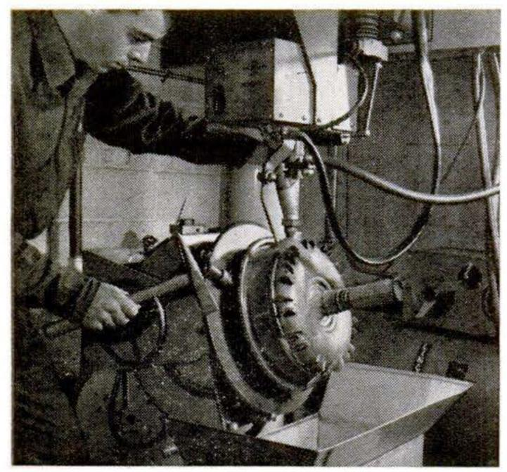
AUTOMATIC WELDER is resealing this converter. Hand welding could do the job, but a jig built onto the machine rotates the housing while flux and rod are fed in measured quantities to produce a perfect bead in one minute.
