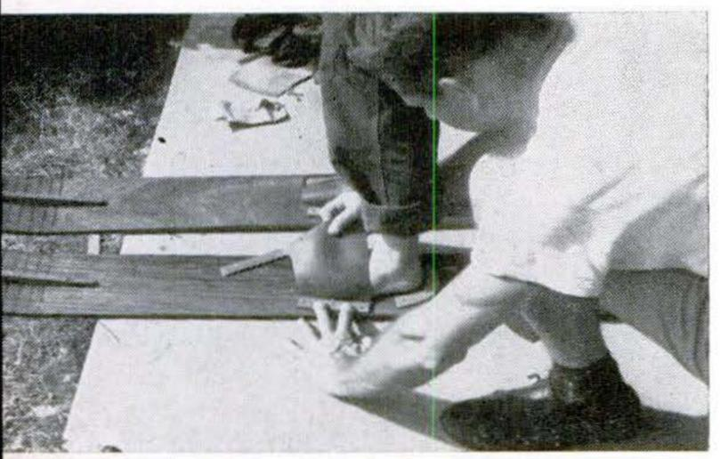
clamp one side of harness, then pull rubber across foot and mark it for second cleat. Toe and heel pockets should grip foot snugly but be loose enough to get in and out of easily.
