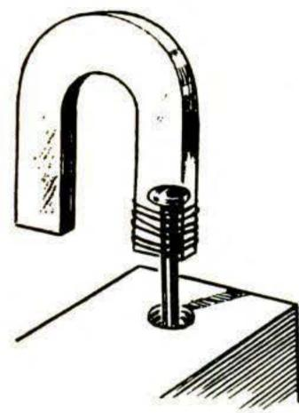
SMALL chips of metal that refuse to be dislodged from drill holes can often be withdrawn by attaching a horseshoe magnet to a nail or other narrow piece of metal to extend the magnetic pull into the hole.—Charles Carroll, Marion, Ohio.
