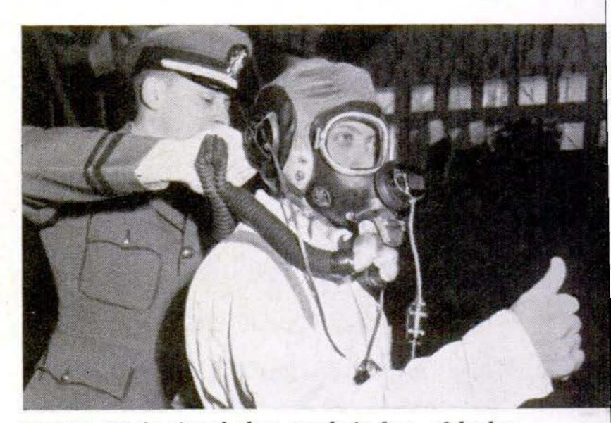
THUMB UP is signal that mask is free of leaks. Navy officer has closed off hose to determine if air is seeping around mask's edges.
