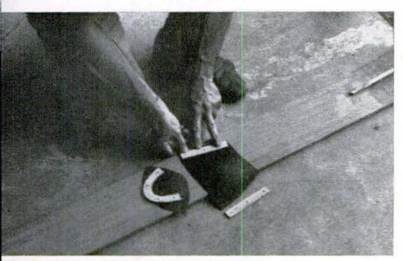
HOMEMADE HARNESSES consist of pieces of inner tube clamped to the skis with thin plywood cleats. Cut the rubber oversize and fit it with the foot in place. Trim off the excess.
