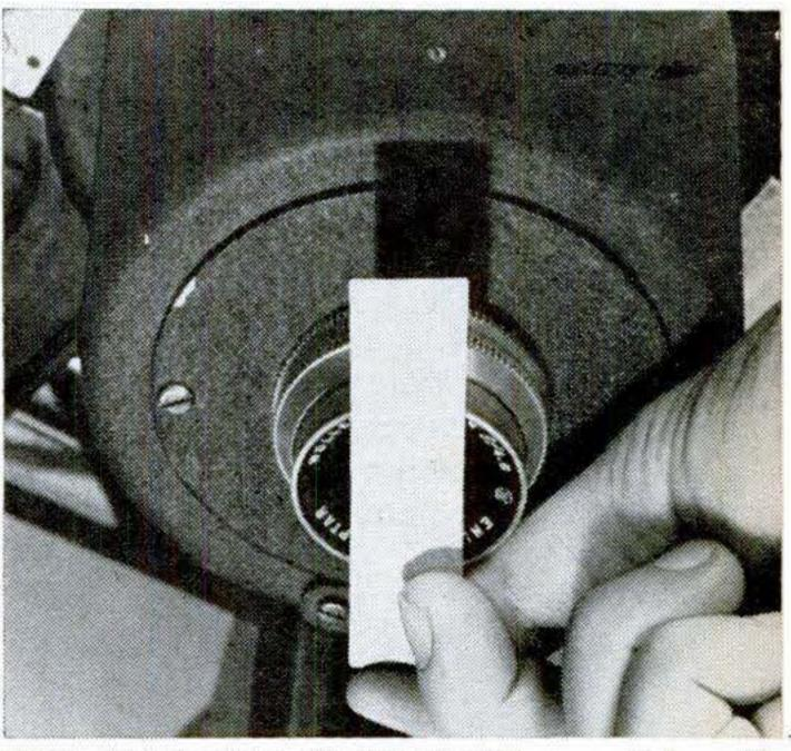
YOU CAN FOCUS AN ENLARGER accurately with this split-beam trick. Hold a strip of cardboard across the center of the lens. When the enlarger is out of focus, you will see a double image on the easel. As the focus becomes sharp, the images will blend into one.
