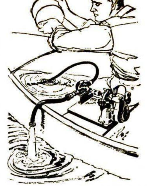
PORTABLE AIR COMPRESSOR for skin diving delivers 11/2 c.f.m. of oil-free air at 50 p.s.i. It's manufactured by Westec-Sweetland, Los Angeles.
