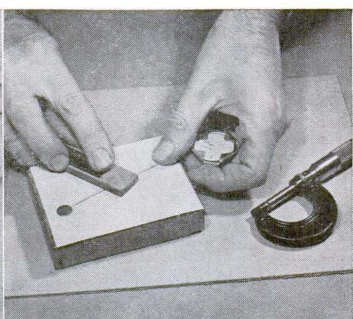
TO LIGHTEN THE ACTION of a spring, reduce its diameter by rubbing it as above with a fine-grit abrasive stone moistened in oil. Check its stiffness frequently as you slim it down.
