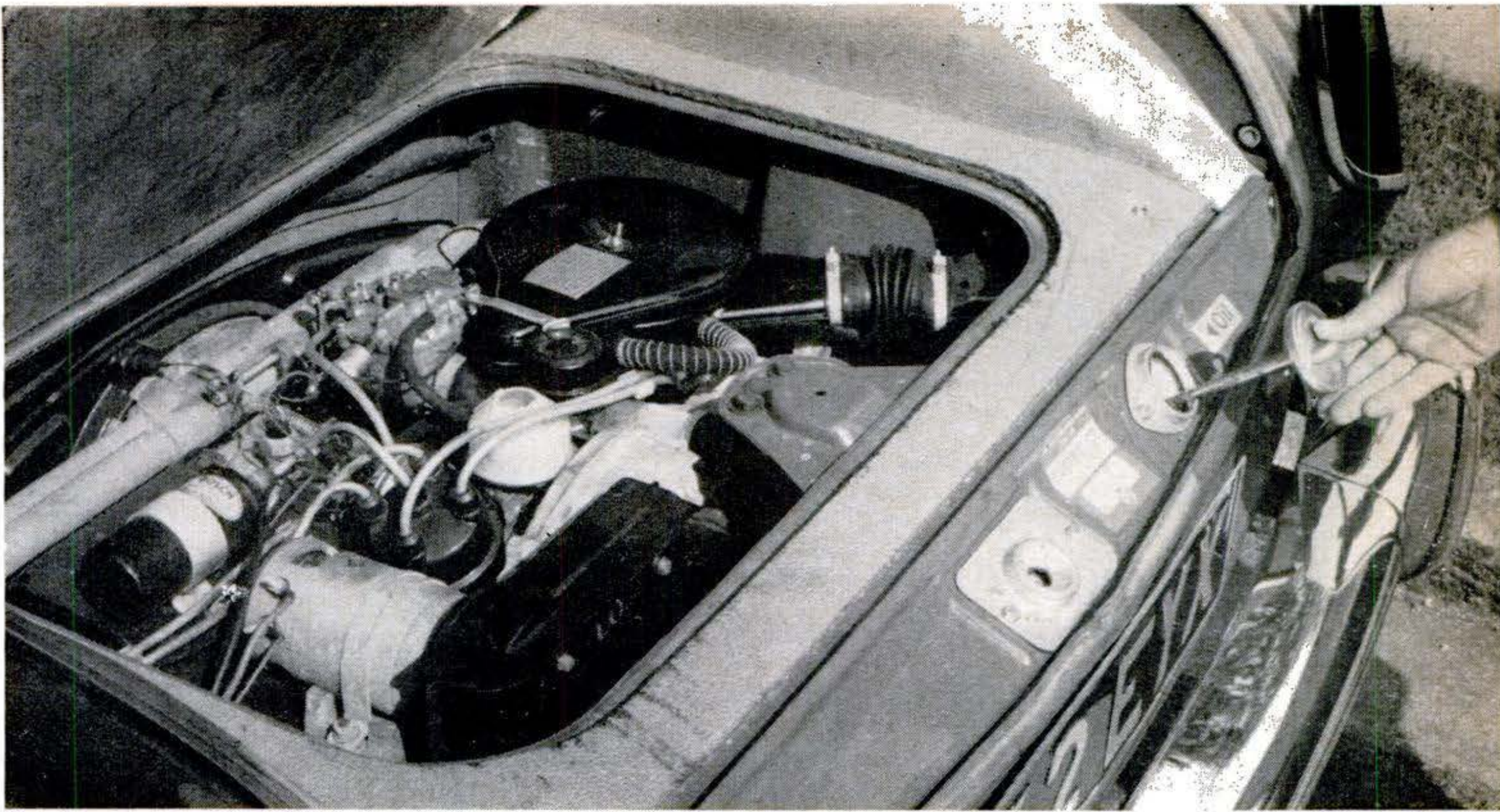
Foil-lined trapdoor in rear trunk gives easy access to top layer of flat four. Combined oil filler-dipstick is outside the engine compartment, just inside the trunk sill, where it won't be covered by luggage.
