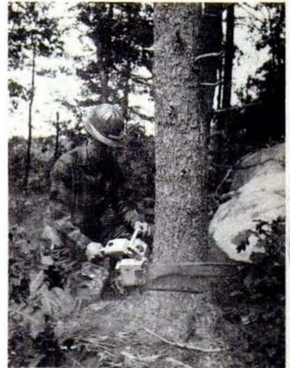
First, the Notch. Two quick cuts and it's done. The notch predetermines the direction in which the tree will fall.
