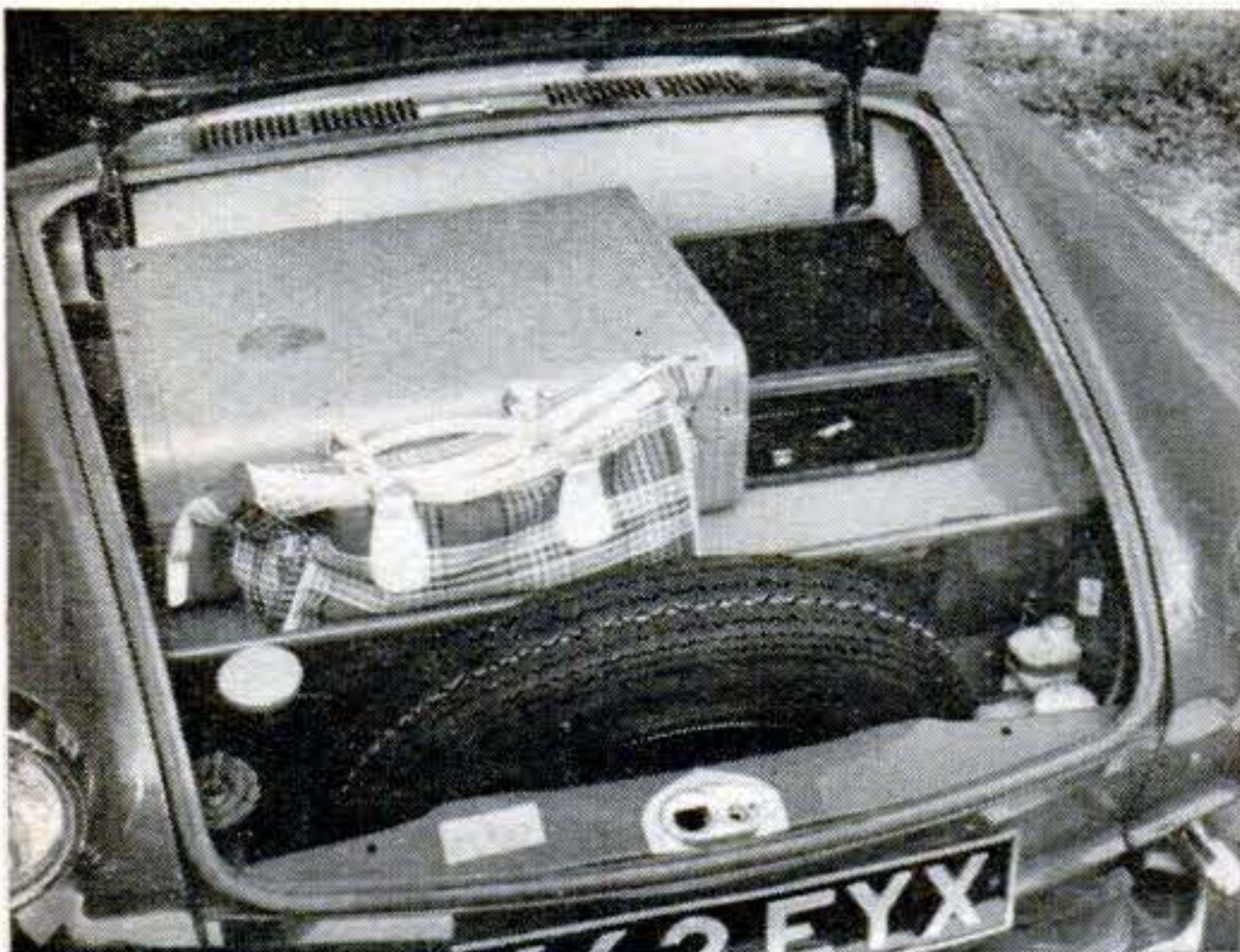
Spare-tire compartment also houses jack, windshield-wiper water bottle, brake fluid. Gas tank is under the trunk floor.
