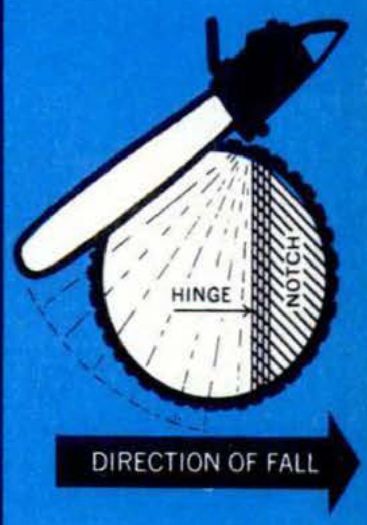
Figure 3 — Felling cut is made by placing bumper against the tree trunk, then cutting in an arc, pivoting on the bumper and keeping the cut parallel to the notch. As you cut, watch both cut and top of tree for signs of movement. The moment tree starts to tip, release throttle and get 20-25' back from the trunk. Keep alert.
