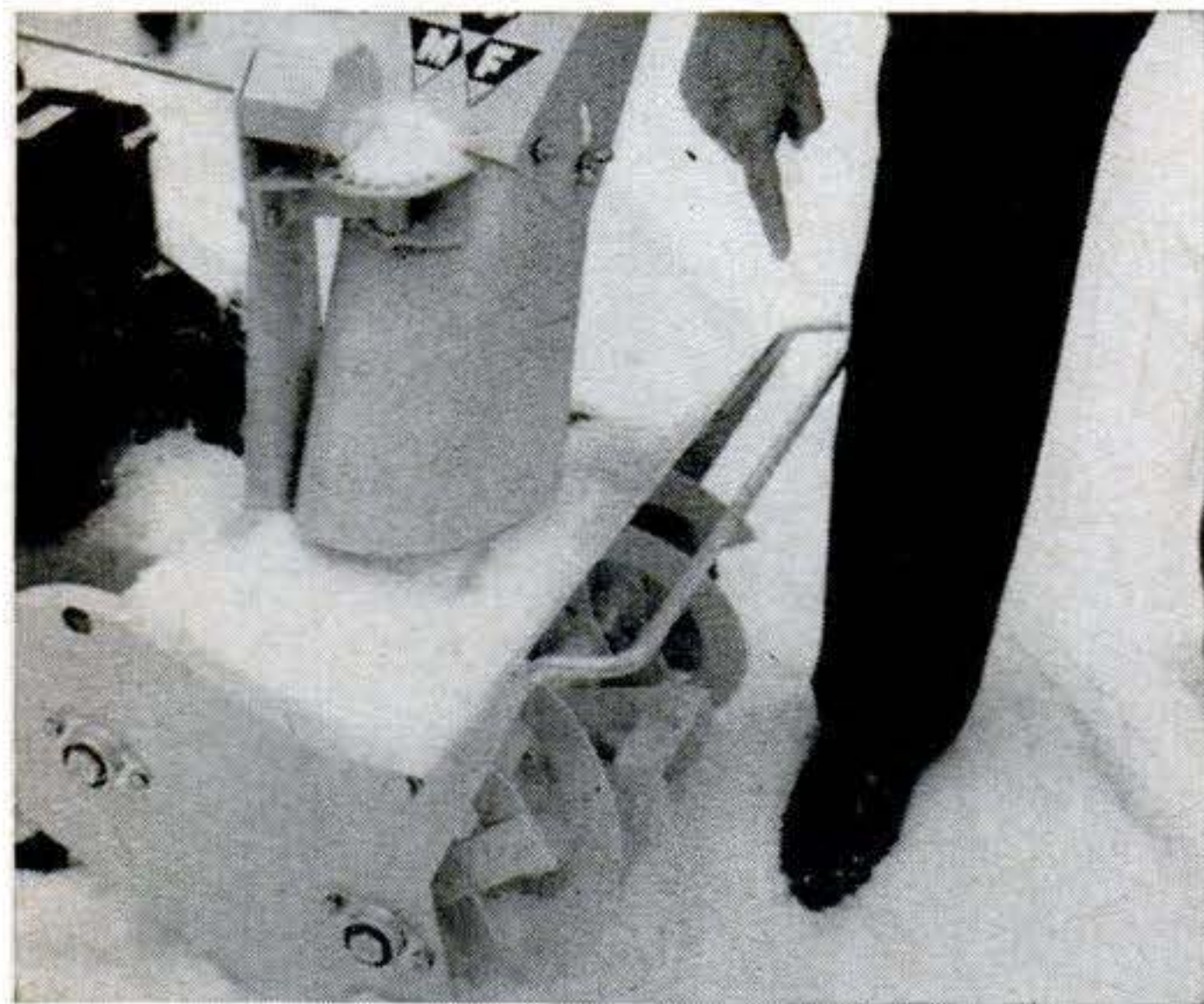
Massey Ferguson's guard keeps toes safe.
