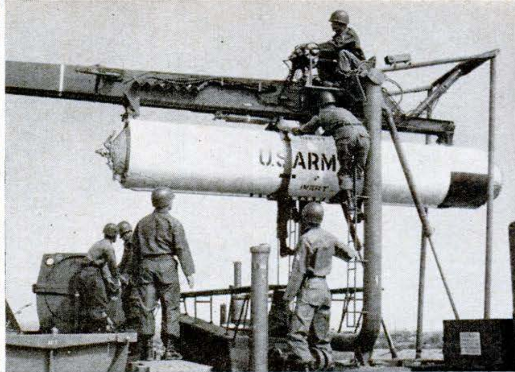
2 Rocket section is lifted out of its container by an electrohydraulic hoist, hung and locked to boom's underside by three hooks.
