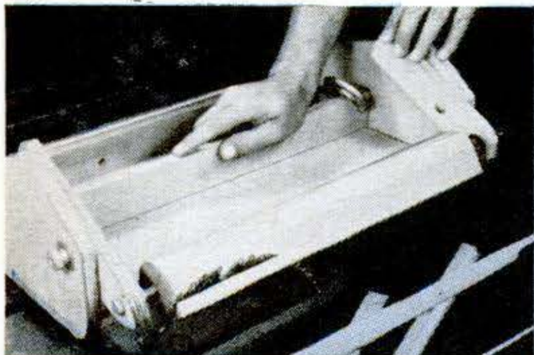
Fluting and reeding on a table saw? Easy as pie with this jig. Page 138.
