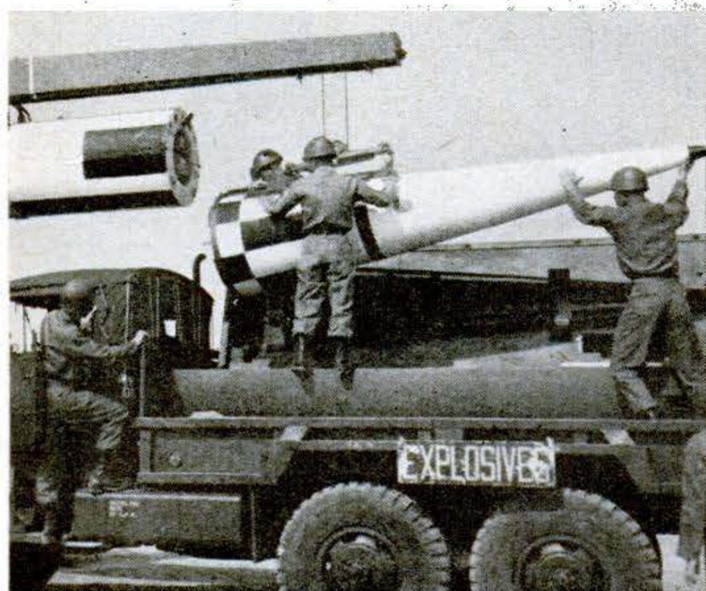
4 Warhead—which can be nuclear, biological, or chemical—is mated. Detonation circuit will obey preset electronic-brain signals.
