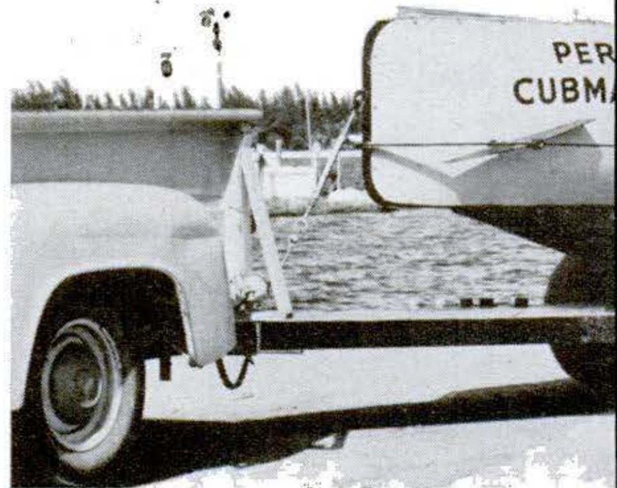
Special trailer makes 4,000-pound Cubmarine easy to tow on land. Flappers on each side of bow are
