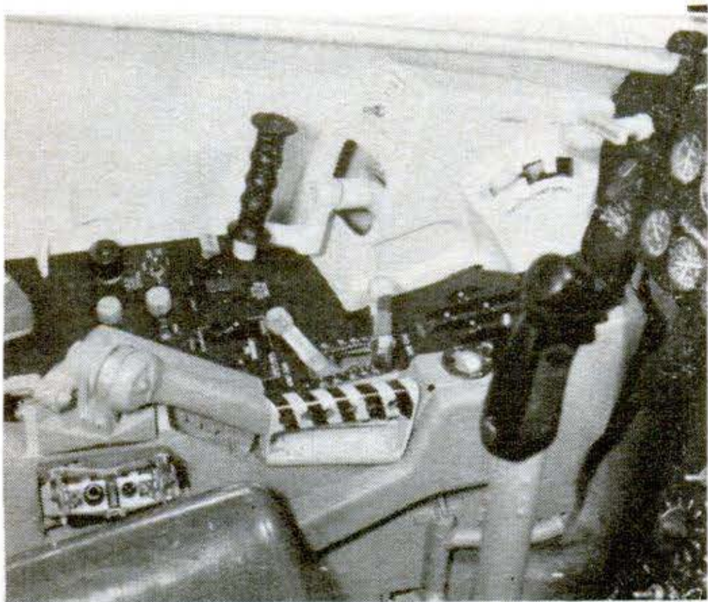
In the thin air of subspace, where aerodynamic control is lost, pilot uses steam jets, controlled by stick at his left (top center of photo). Striped handle is for emergency ejection seat.
