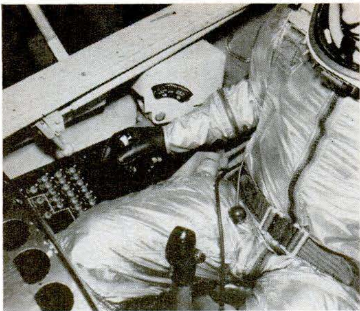
Pilot gets a choice of conventional center stick or one at his right in atmospheric flight. Both wiggle tail and wing surfaces. Side stick is used when G-forces won't let him reach center stick.
