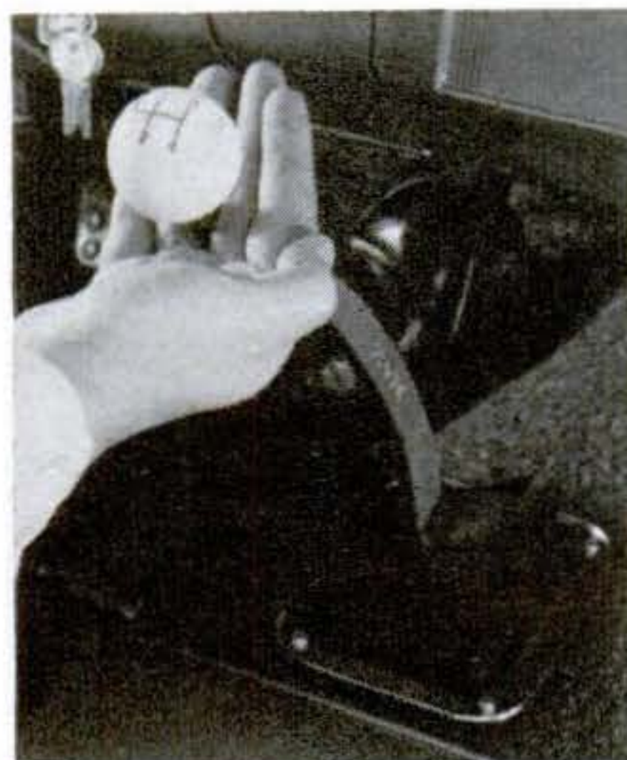
Dodge and Plymouth offer four-speed manual shift with various engines. Ratios with Dodge's 383-inch engine are 2.2, 1.66, 1.31, 1. Optional axle ratios are 3.23 and 3.55.
