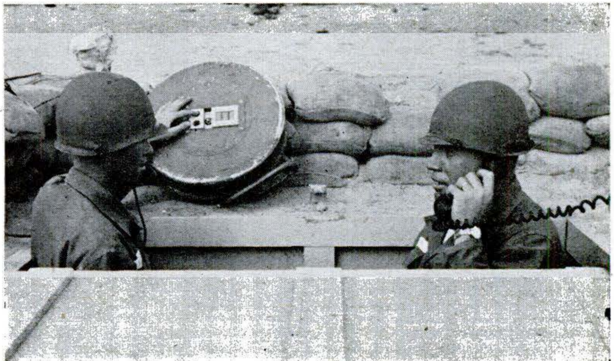
8 Last few minutes of Sergeant countdown is monitored from a remote-control firing pit about 250 yards away from the launcher. Manual override can stop countdown up to the last split second if the missile self-testing circuits indicate a malfunction, or on radiophone orders from a higher command.
