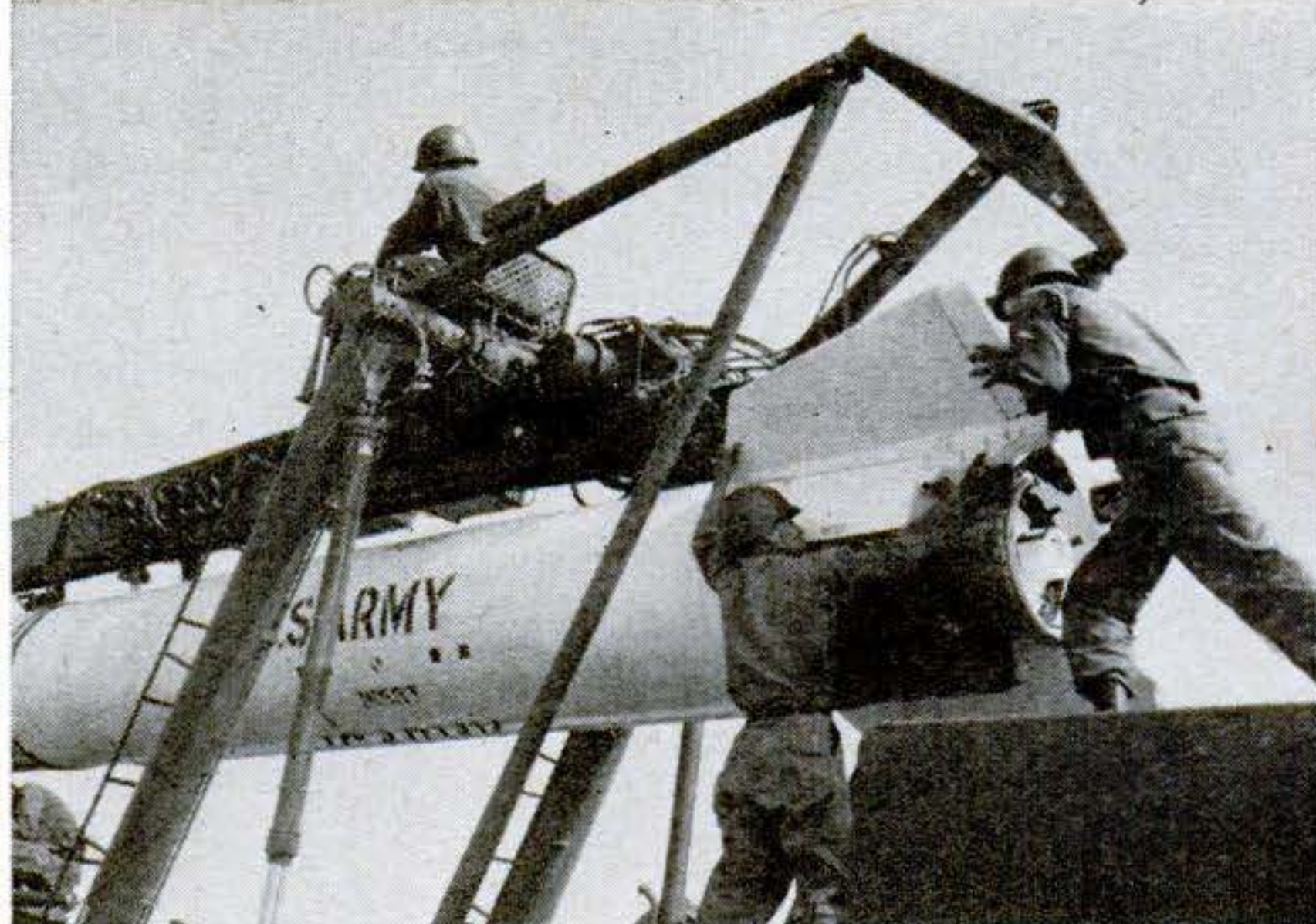
5 Control fins are attached to rear of the rocket. They provide aerodynamic stability, attitude control, and some maneuverability.
