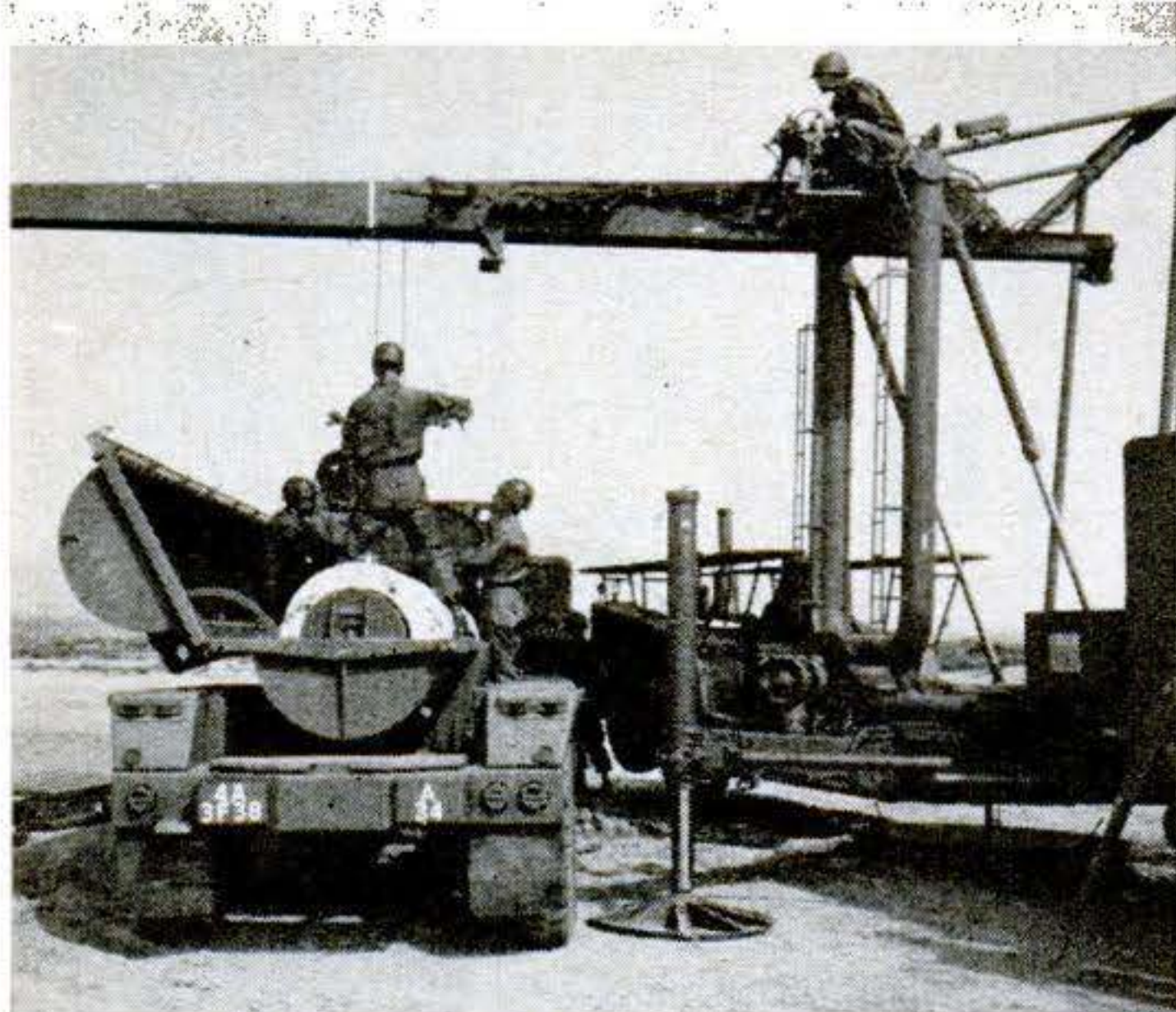
1 Assembly begins: Launcher boom is swung out as truck carrying rocket-engine and guidance-section containers pulls alongside.
