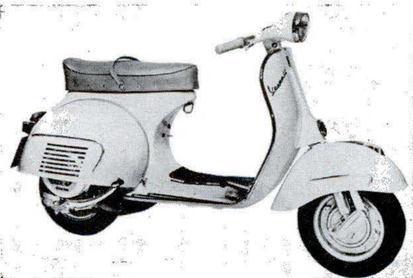
Power egg is hinged to ride up and down with wheel. Trailing link and coil spring carry the front wheel.
