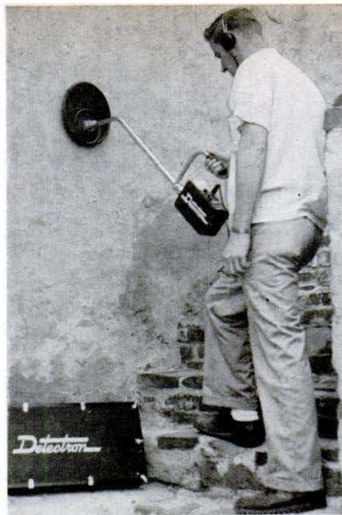
Scanning walls and ceilings is done the same way as floors: Detector head is held parallel, a few inches away.
