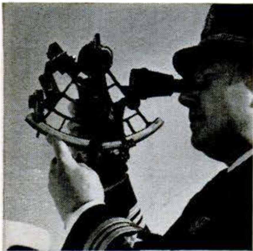
Ocean vessels, navigating by stars and sun, still use time-honored sextant—as on the S.S. United States, above.
