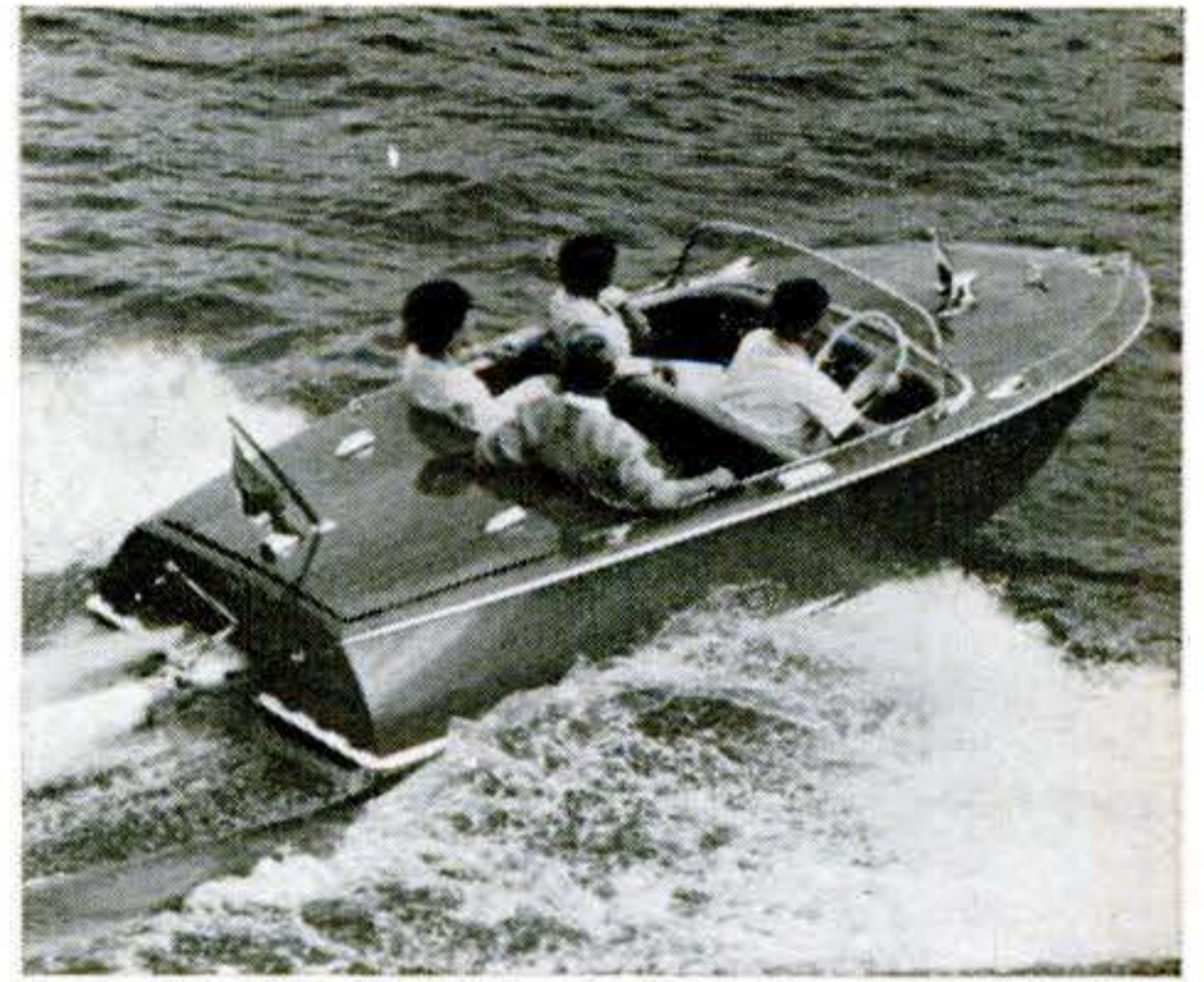
Water jet swivels to steer no-prop, no-rudder, shallow-draft experimental boat.
