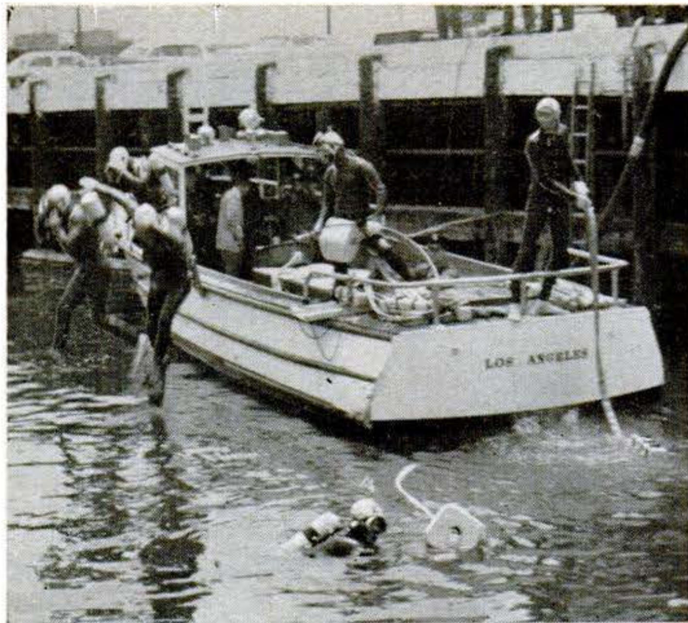
"Into the water" is signal for firemen to dive in with equipment. Buoyant balsa blocks are strapped on hose, form collar behind nozzle.
