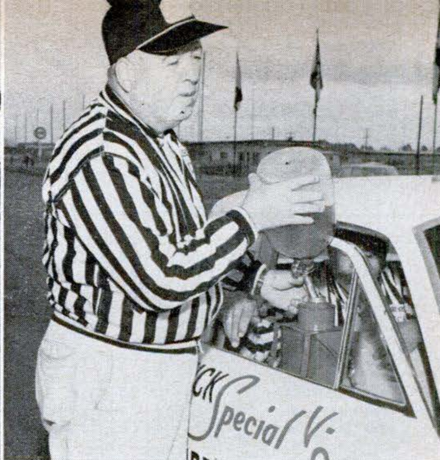
Special one-gallon tank on front door is connected by tubing to fuel pump, and premeasured fuel is poured in immediately before start.
