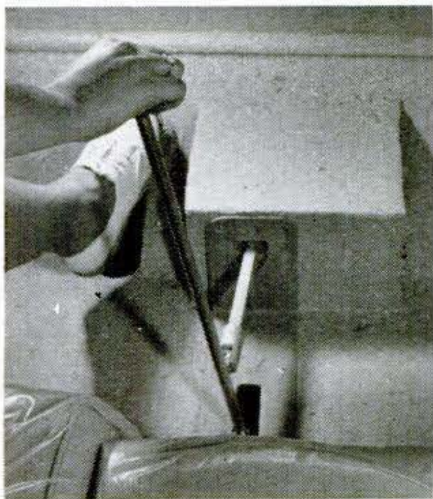
Shift lever controls bow jets when moved sideways; and forward, neutral, and reverse position of control gate when moved fore and aft.
