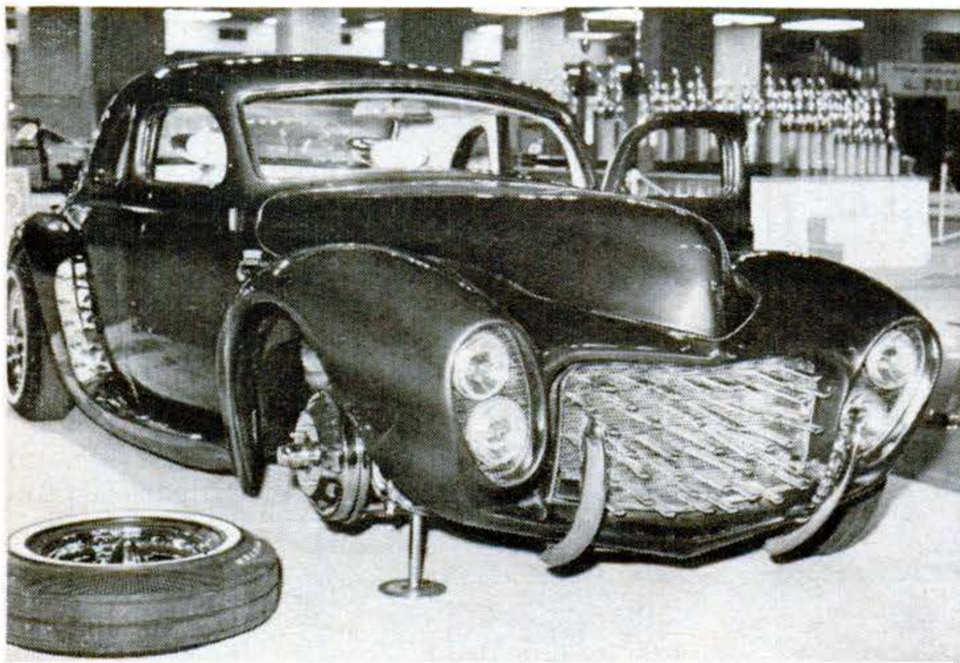
The hood is the only hint that this is a 1940 Ford. A strip was cut from the body at the center line and the two halves welded back together for sleeker appearance. The top was cut down. Right front wheel is off to show chromed brake drum. Quad lights and custom grille are new. An Oldsmobile engine powers the car.
