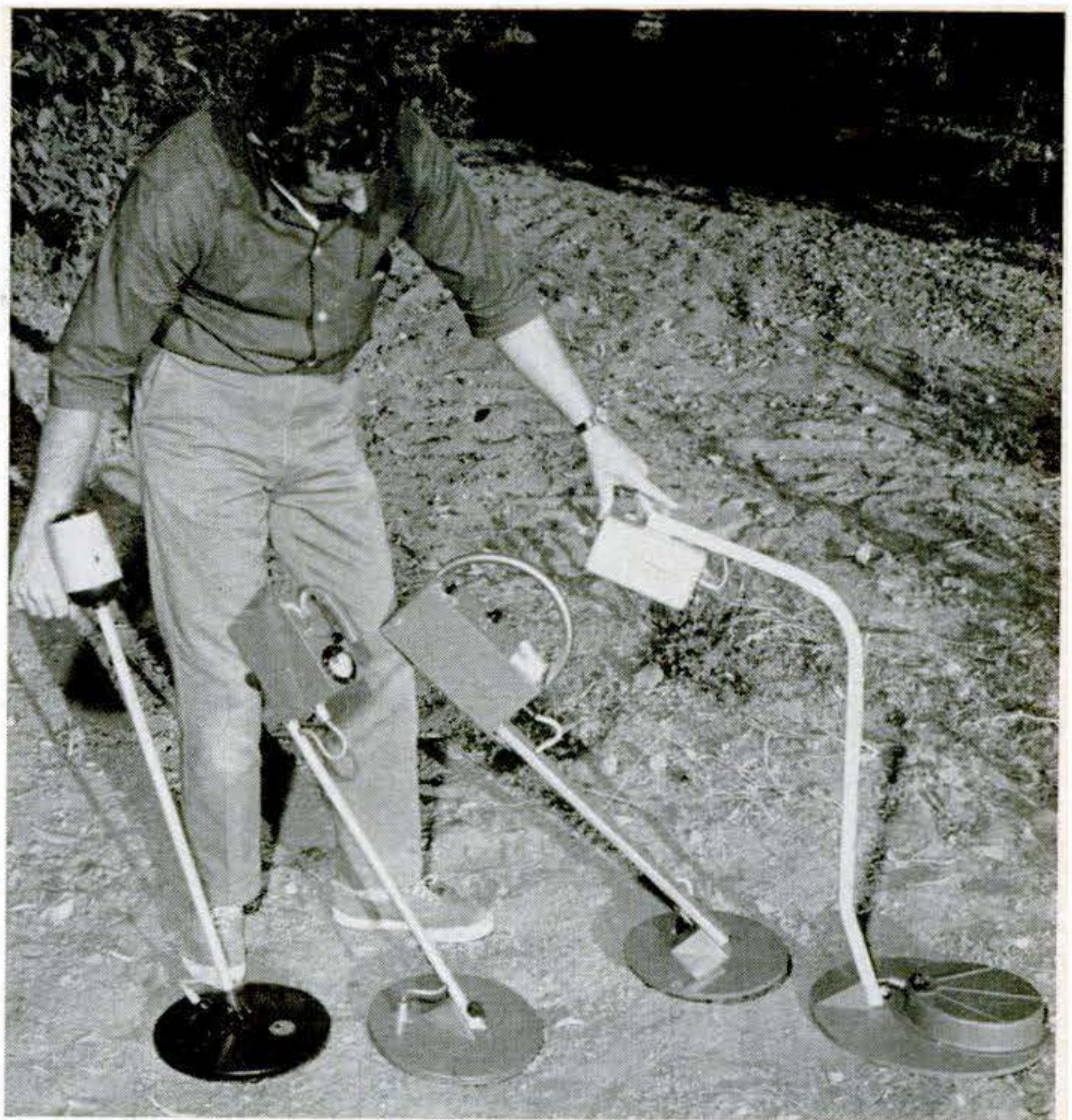
Most detectors have about the same depth range, but sensitivity varies greatly from brand to brand. Shown from left to right are Metrotech, Geo-Finder, Detectron, and Goldak.
