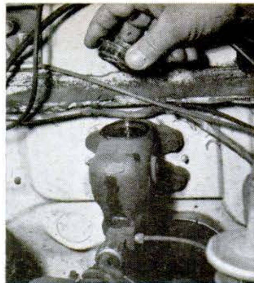
Check brake fluid in the master cylinder. It should be about \frac{1}{4} " from the top.
