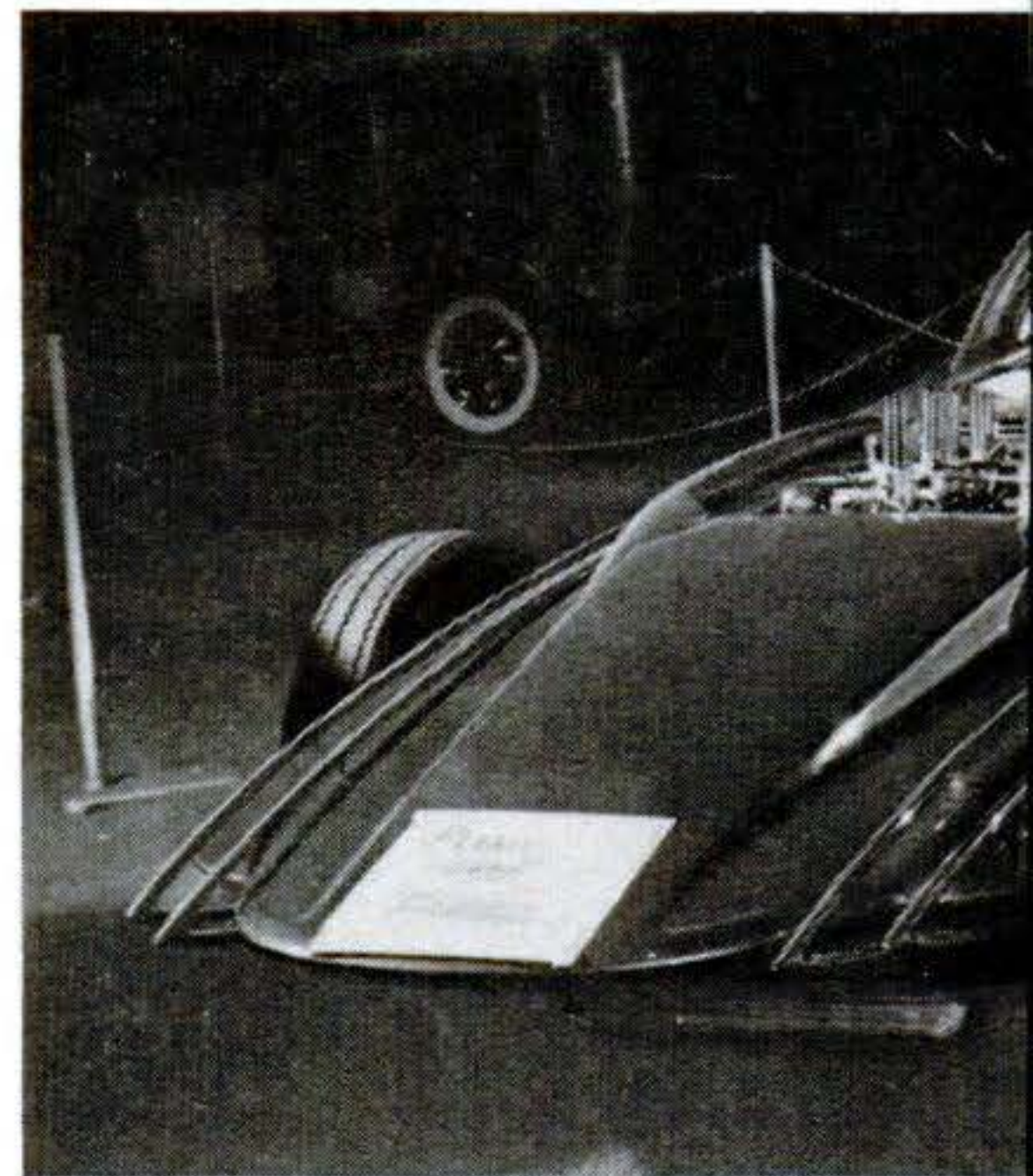
Latest of bubble tops is this dream car with hand-formed metal body over Buick chassis. Engine is modified and fuel-injected Buick V-8. Canopy can
