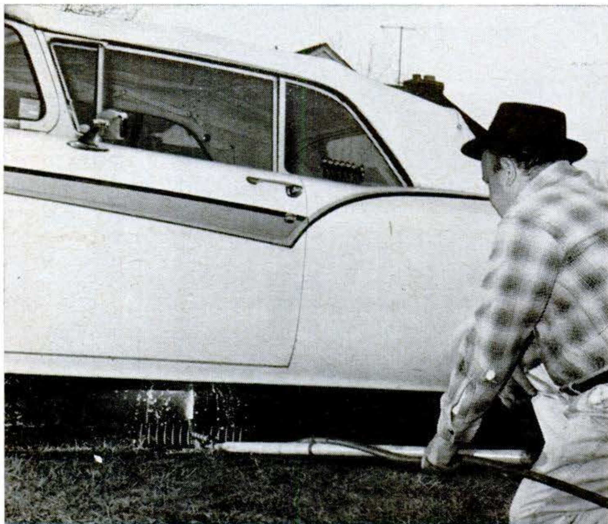
Check brake fluid in the master cylinder. It should be about \frac{1}{4} " from the top.
