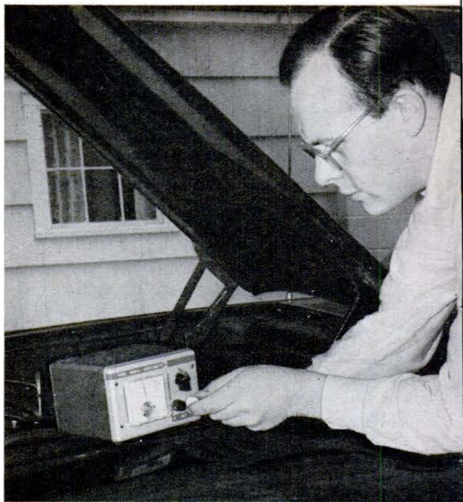
Engine r.p.m. and point dwell are measured with instrument connected to the distributor primary. A switch selects meter function.
