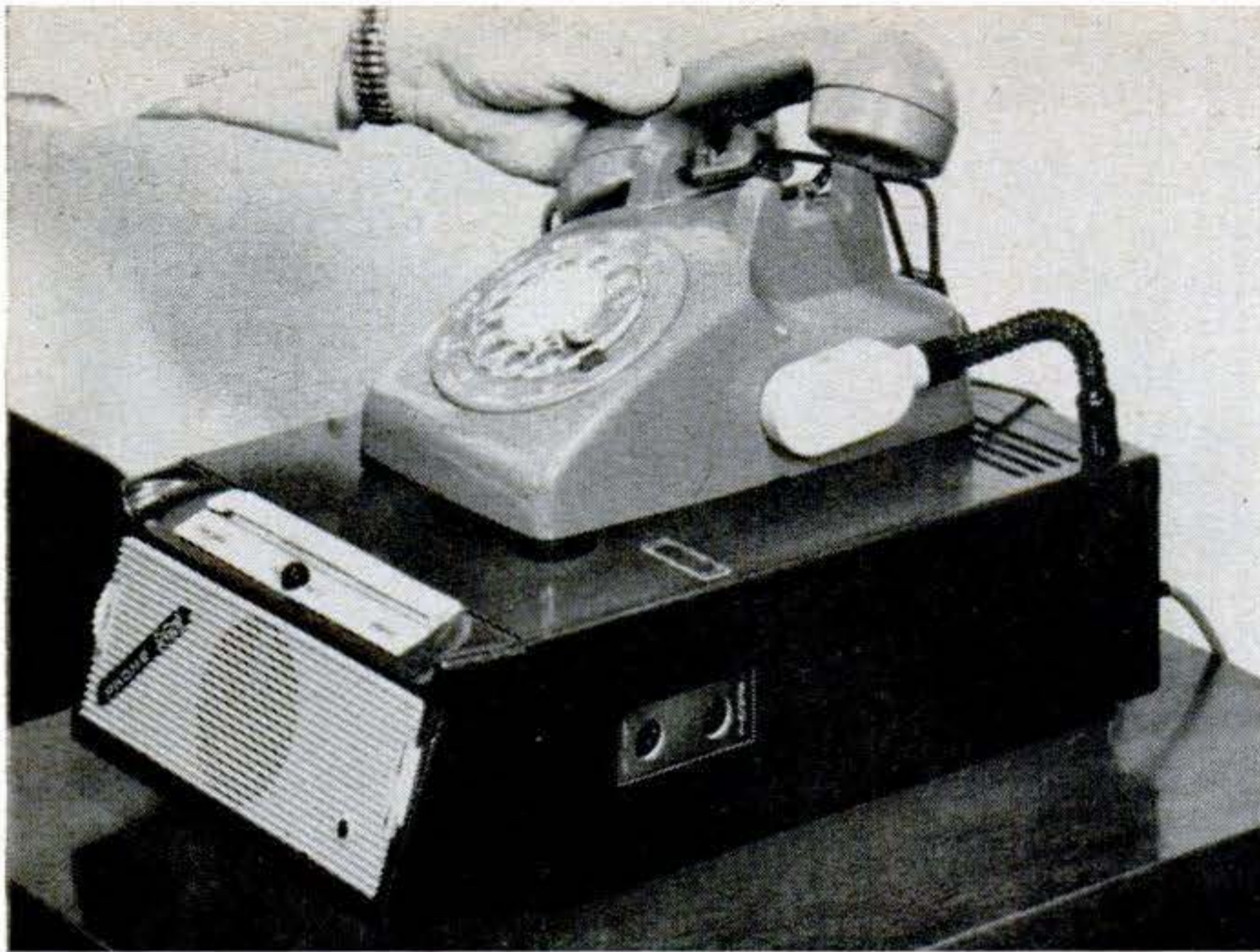
Handpiece rests on arms. Ring of bell opens circuit. Pickup is at side. Case contains controls and head-set jacks.
