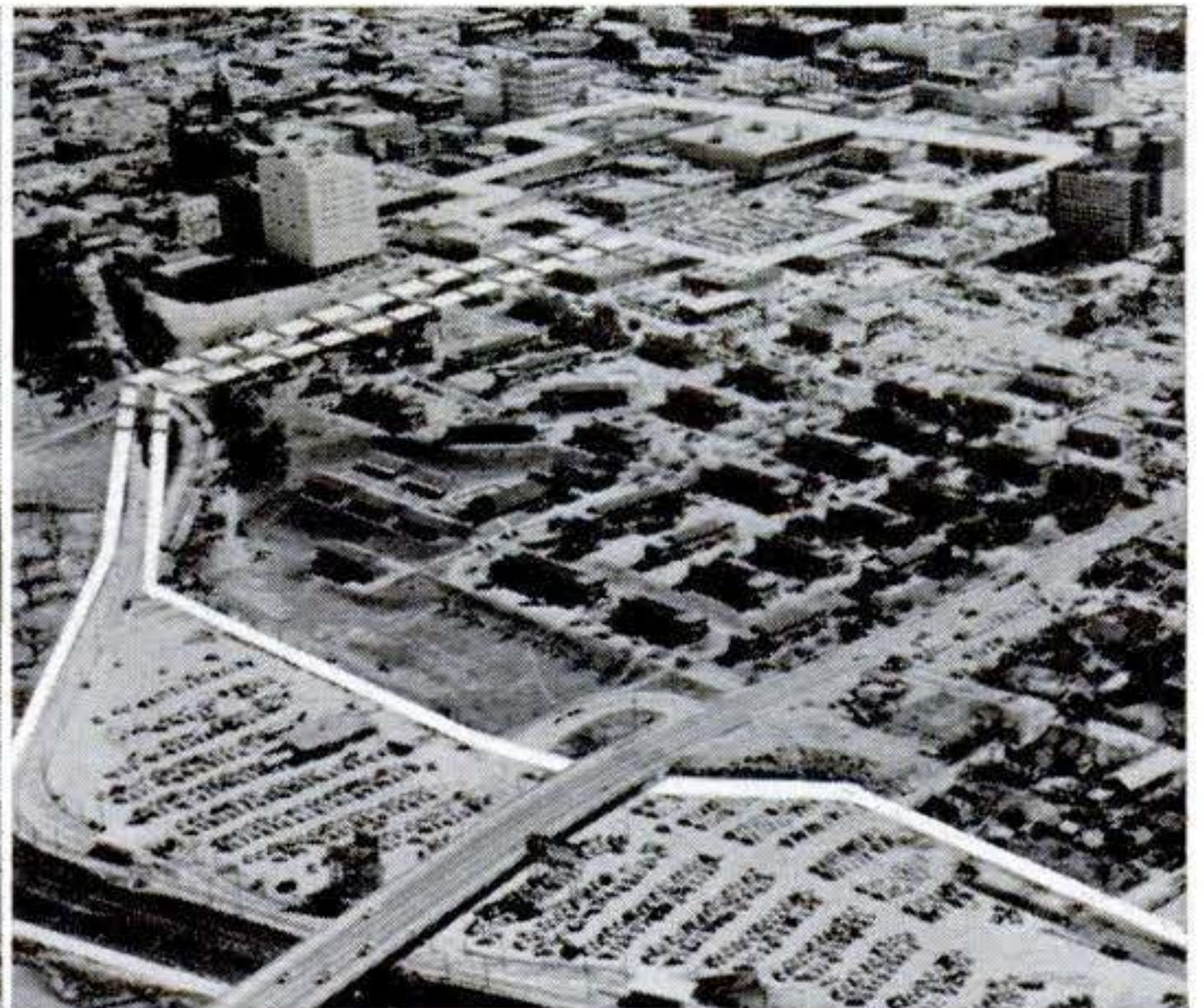
Railway runs from parking lot to store. Surface track is solid, subway is dotted line.
