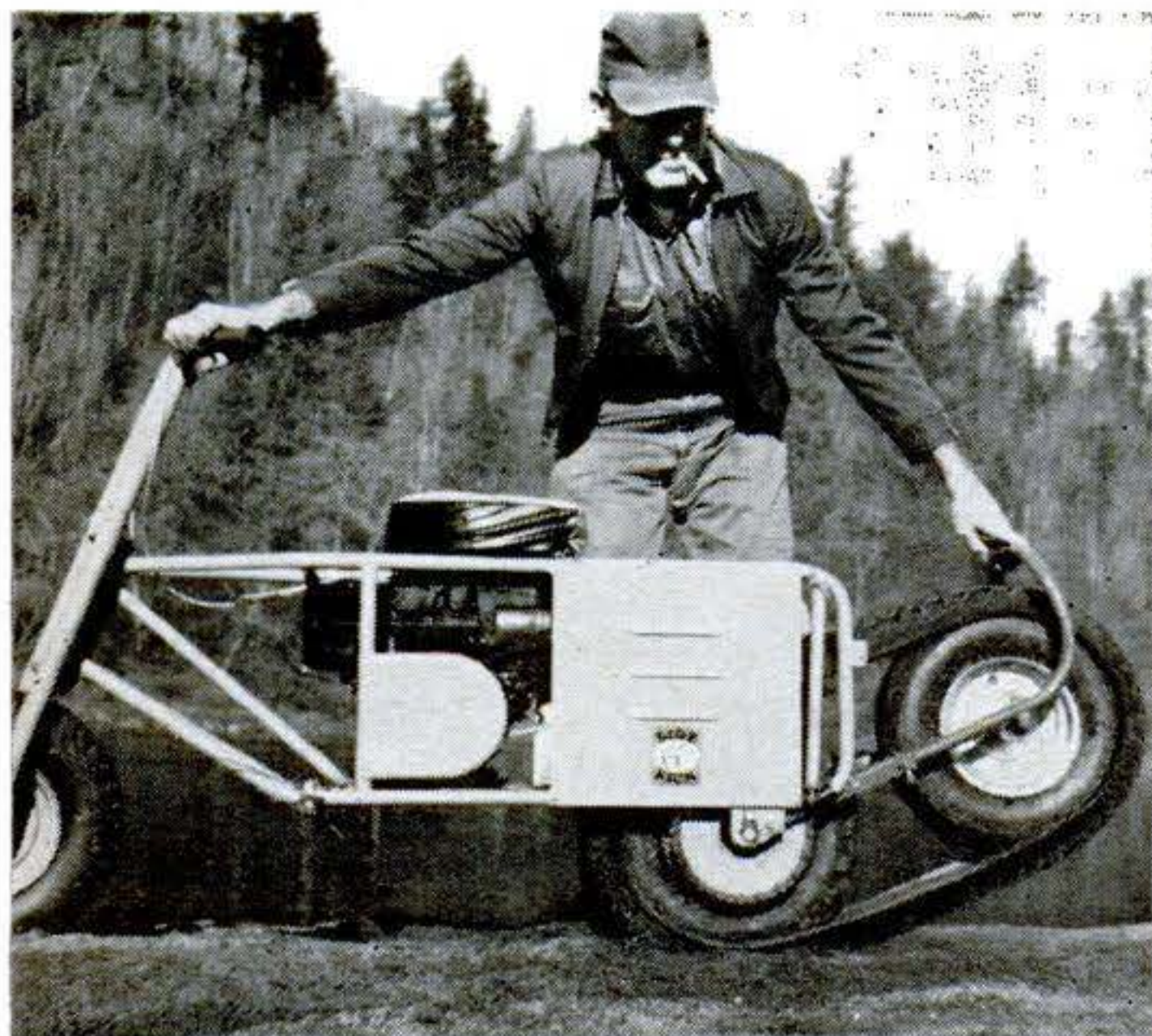
1. Katagote swivels up and down freely, adds little more than 20 pounds to scooter's weight.
