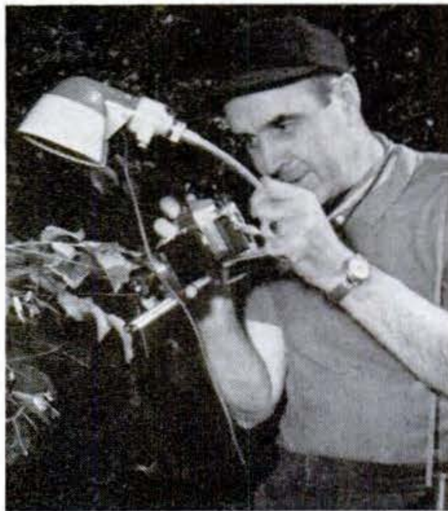
Brevoort's favorite for nature shots is the 35mm single-lens reflex. His electronic flash head, mounted on an inexpensive gooseneck arrangement, permits moving flash in any direction.
