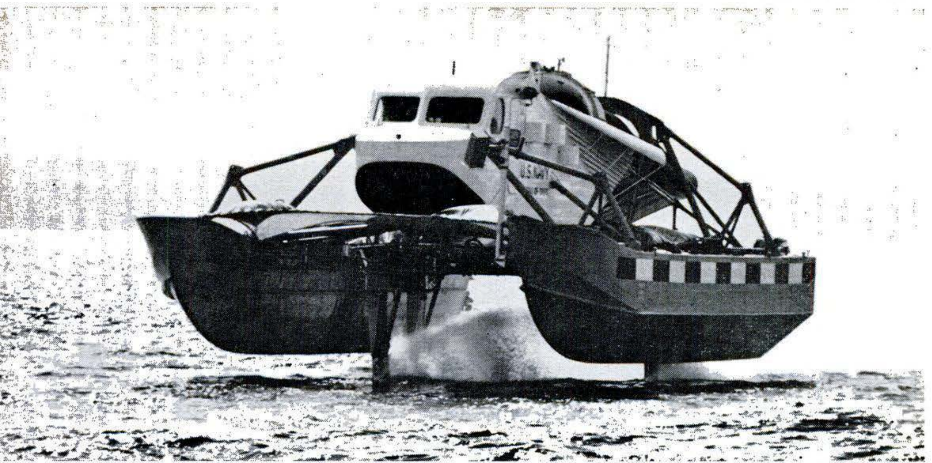
Rising above waves, hydrofoil catamaran hits 60 m.p.h. Navy is using it for research on foils.
