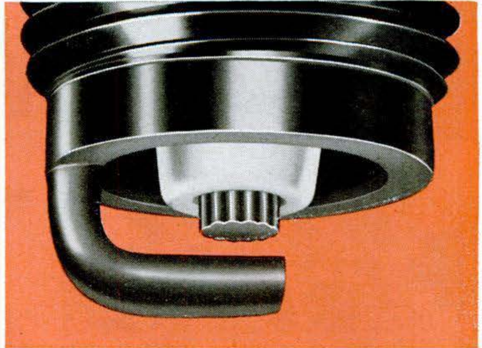
Electrodes of Isovolt alloy resist wear. Center electrode is knurled for better sparking longer.
