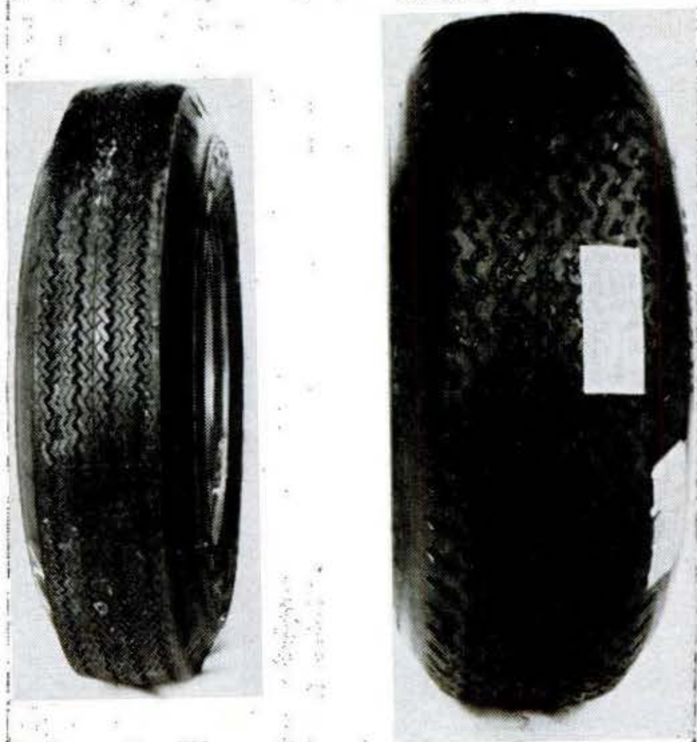
Stock-racing tire dwarfs passenger tire at left. Racing tire has wider tread, shallower grooves; pressures run about 40 to 60 p.s.i.
