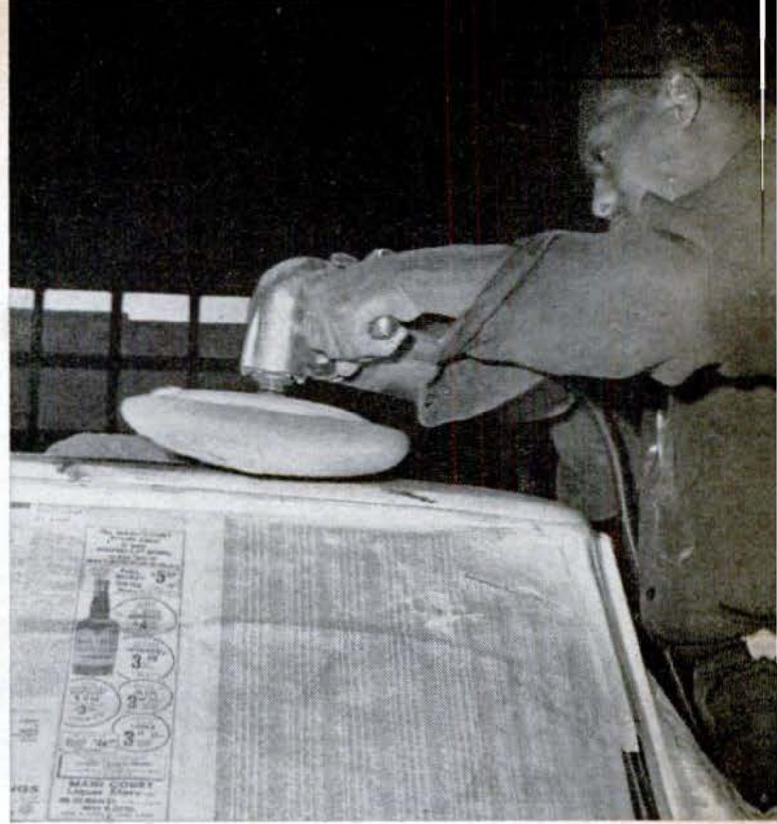
Compounding is a job that's often slighted. This man is buffing a new paint job to "rub out" the finish and put sparkle in it. This also removes tiny and unsightly "orange-peel" wrinkles.
