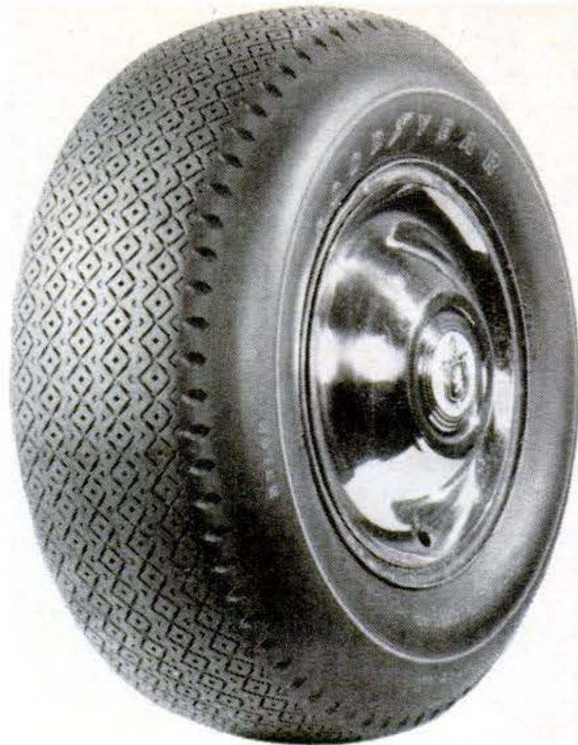
Asphalt-racing tire has tie bars \frac{1}{32} inch below surface to make tread almost solid as it wears down. Otherwise, tread would tend to feather in one direction as it wore, losing traction.
