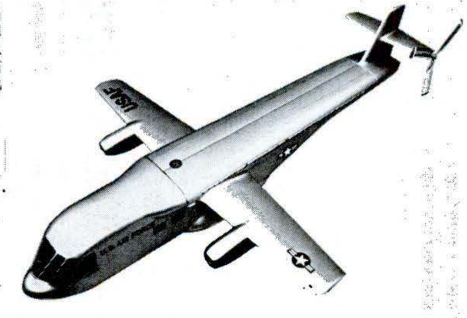
Lid on fuselage reclosed, fixed-wing aircraft powered by wing jets flies on mission at speeds up to 500 m.p.h.
