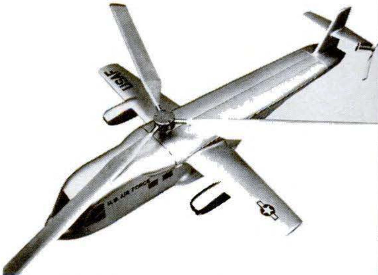
Working model of new VTOL whirls rotor blades to take off and land like a conventional helicopter.
