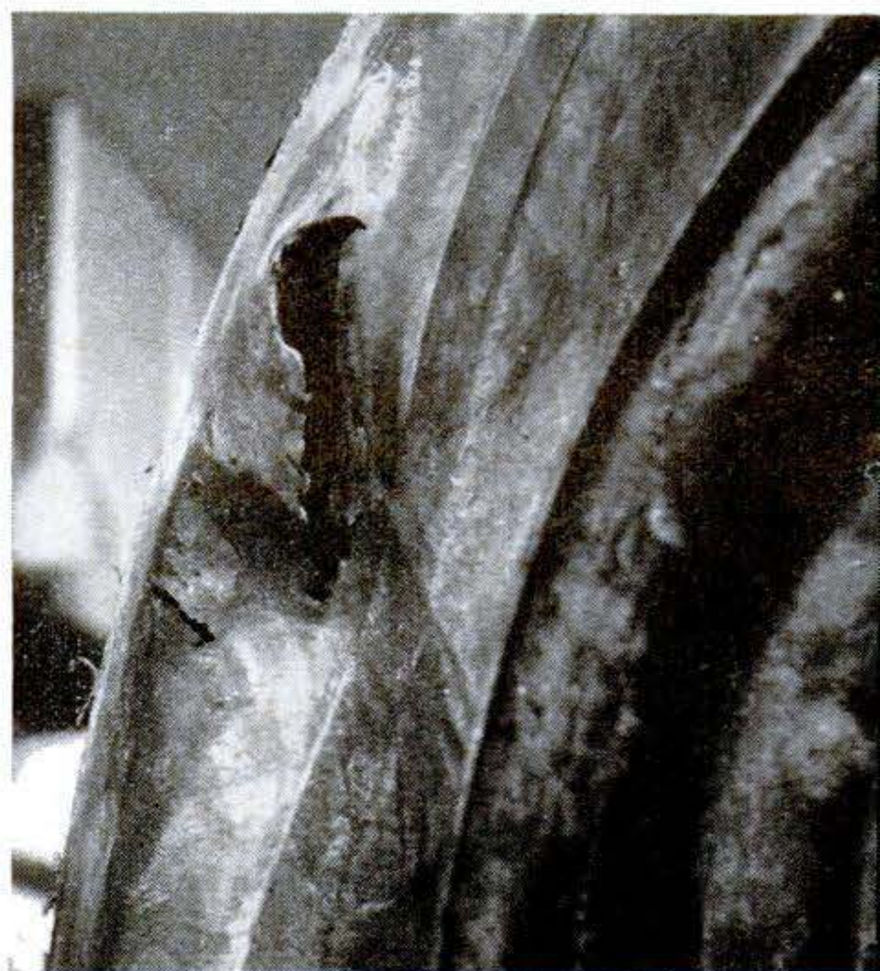
This two-ply tire failed after running at reduced pressure for 75 miles. A four-ply, running under identical conditions on same car, went 125 miles without an outright failure.
