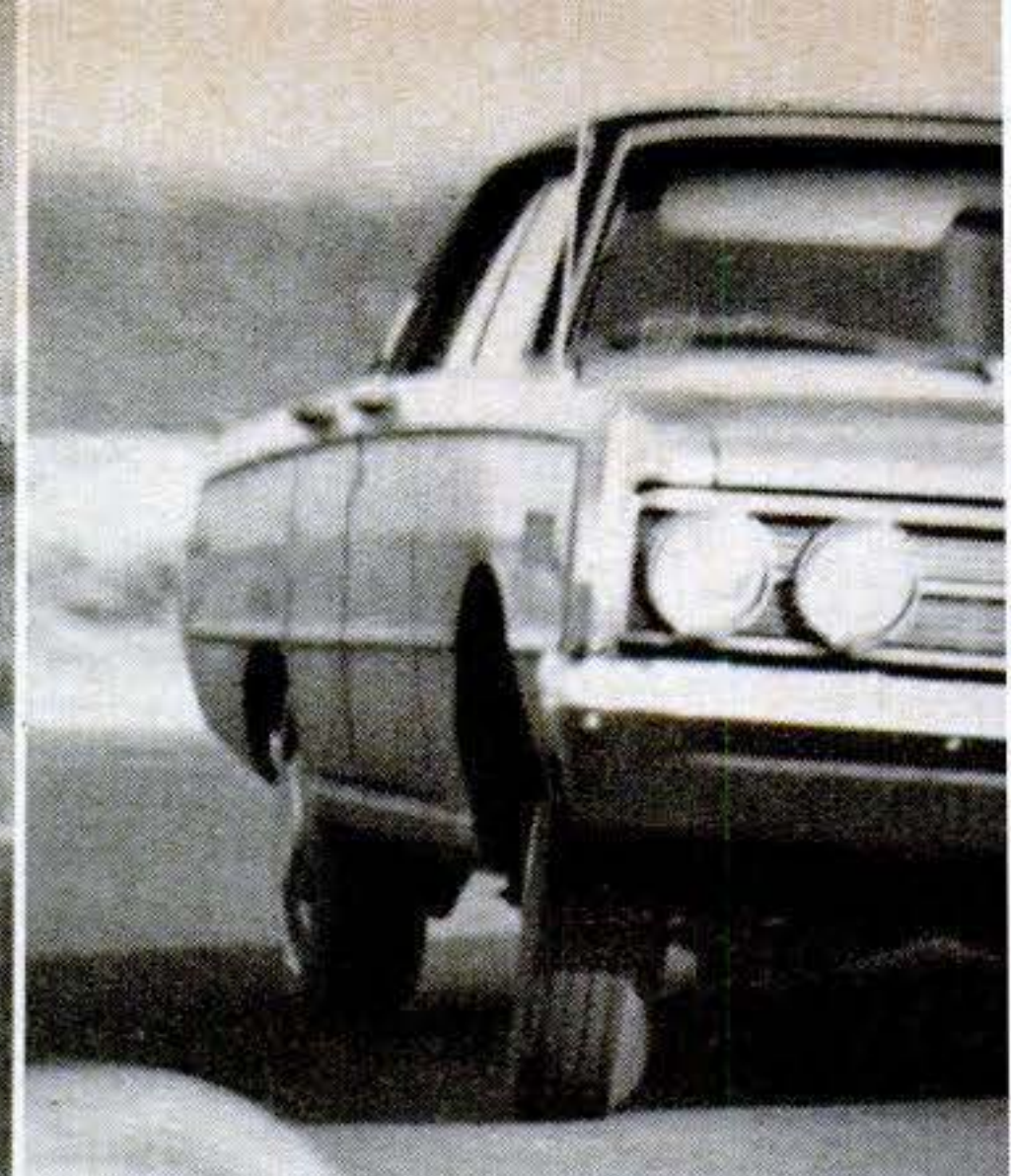
MERCURY shows excess understeer at 60 m.p.h. on the
