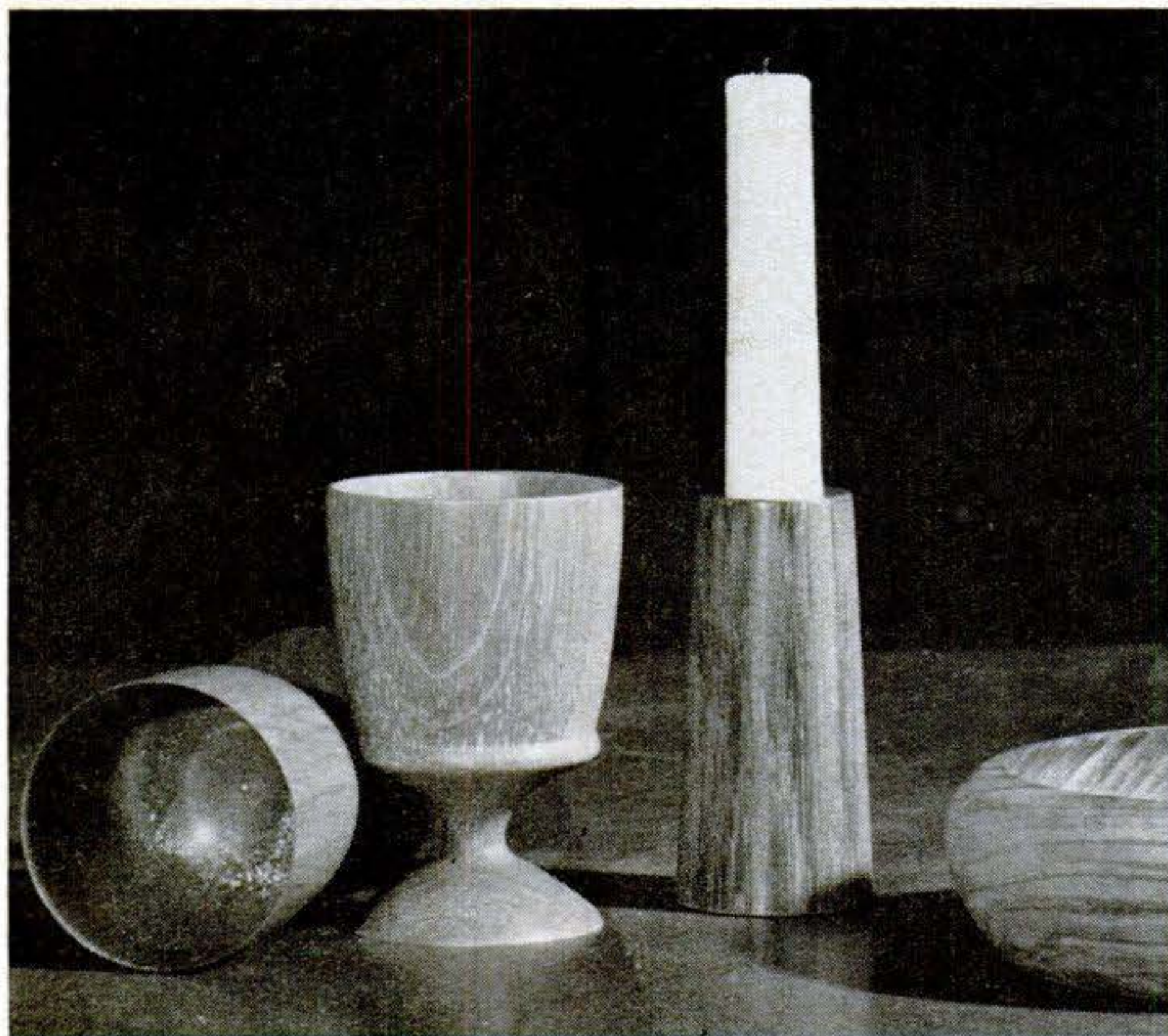
Craftsmen's pieces are turned from vinyl-impregnated wood. Goblets have fine, thin edges. Dye added to vinyl tints through to center.
