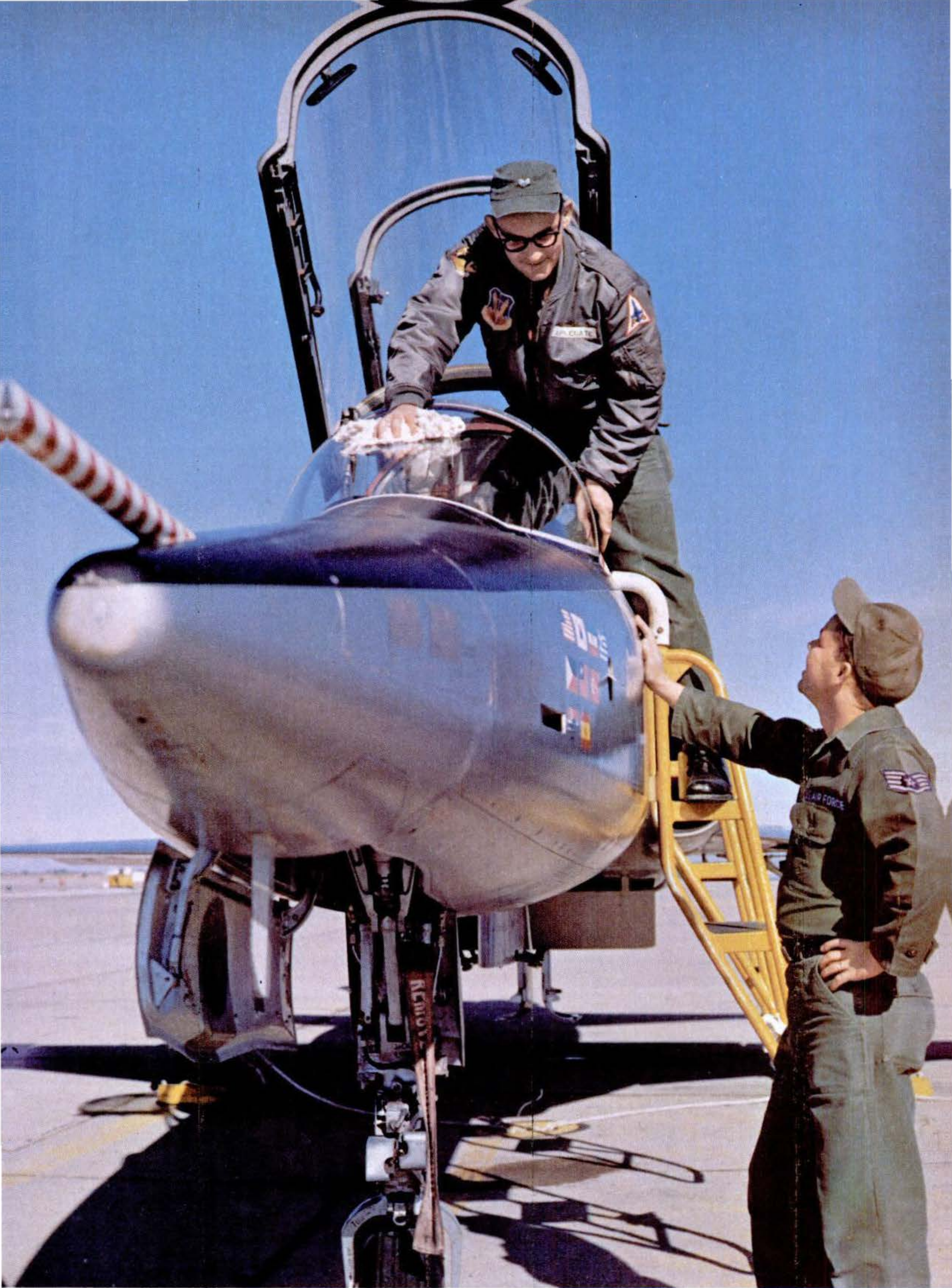
Built low to the ground, F-5 is easy for mechanics to maintain. Even engine change is simple.
