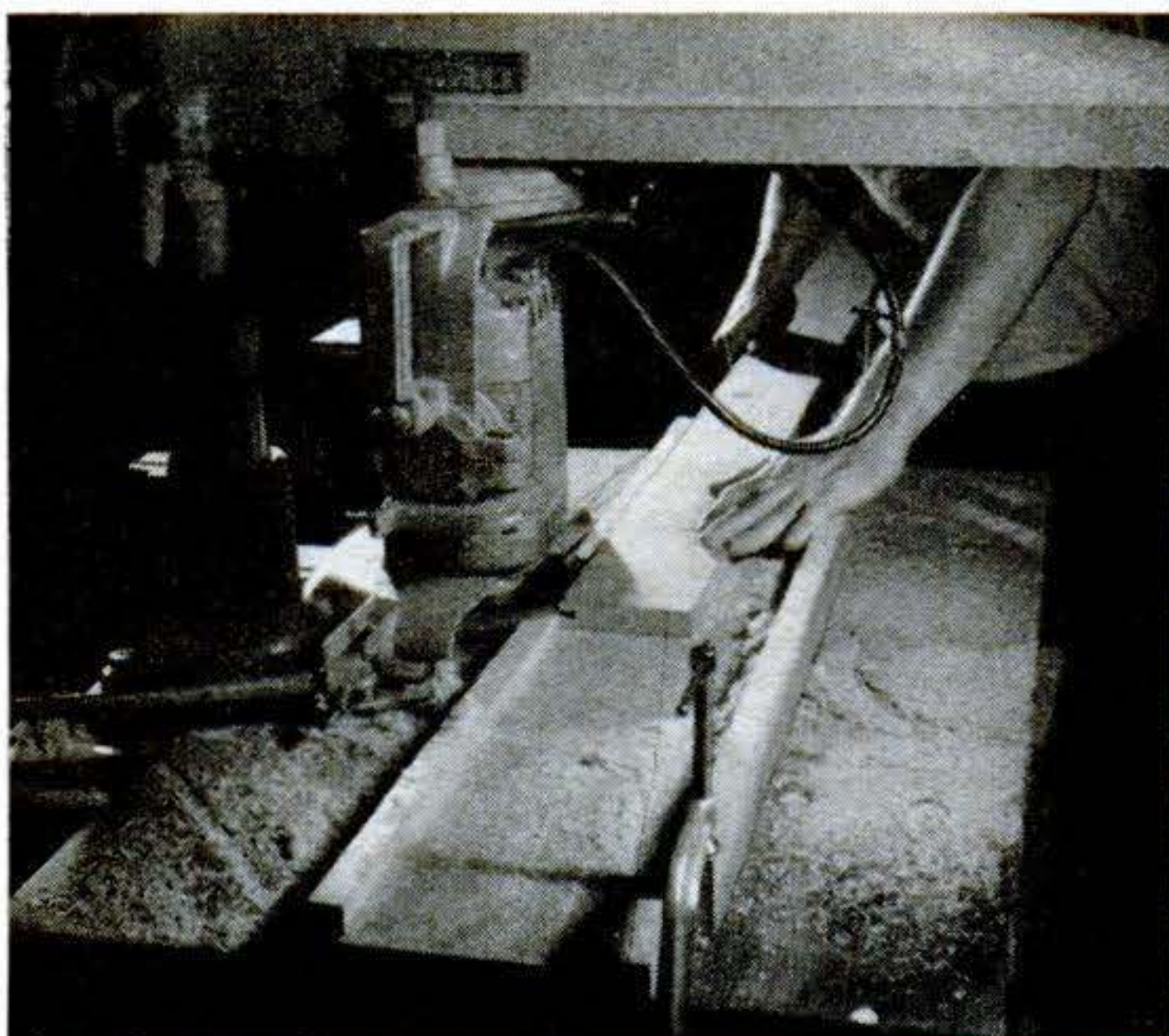
Cut grooves in the center of one edge with a dado. You'll have to change the setup for a table saw.
