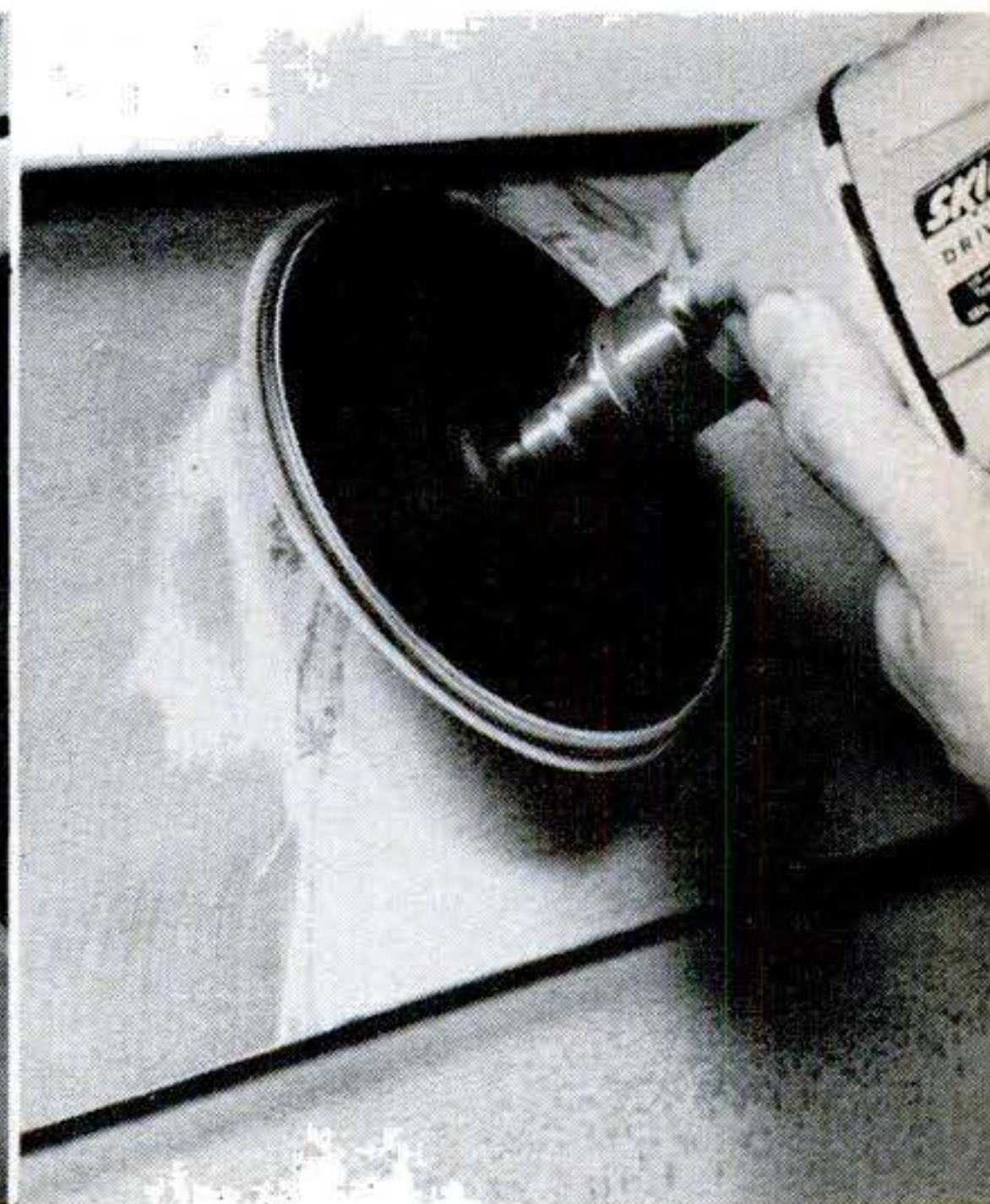
Removing paint: A slow speed helps keep heat from softening the paint and clogging the disk.
