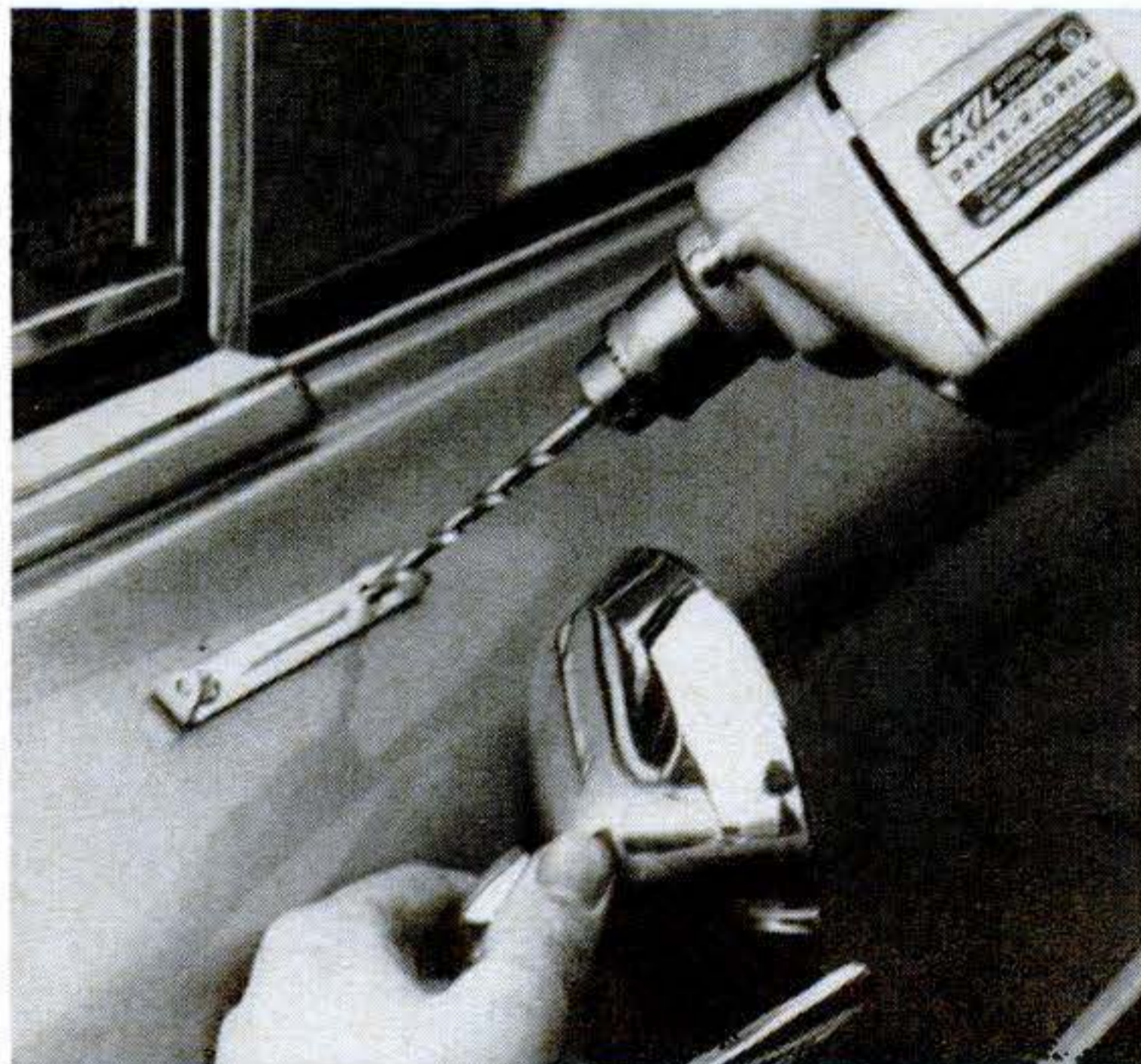
Drilling ordinary steel: Turn slowly, start without a punch mark. Stop trigger at about midrange.
