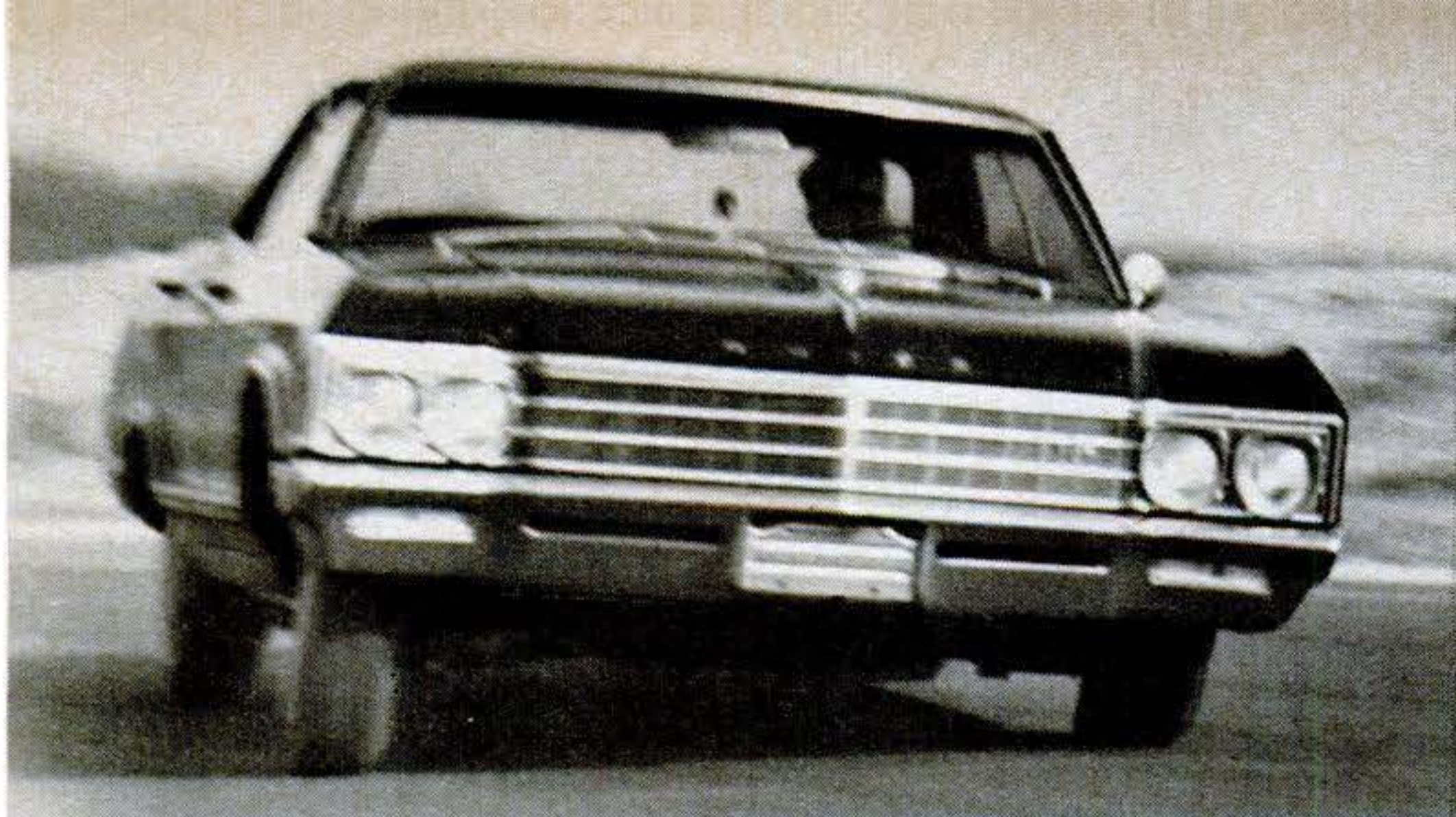
BUICK corners at 60 m.p.h. with some body roll but fine steering precision. It proves that soft springing is not incompatible with good handling.
