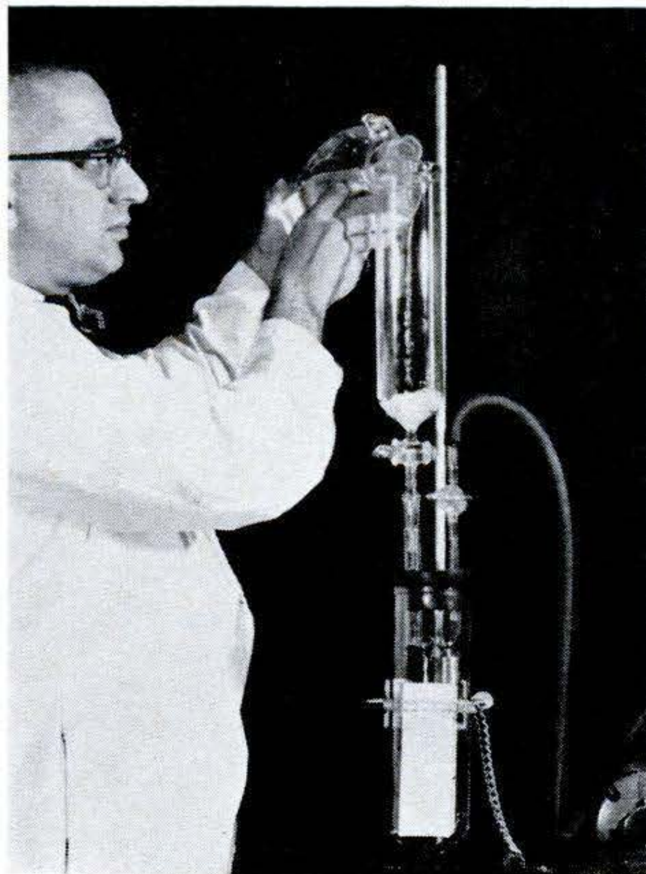
Vinyl is poured into chamber, and wood soaked in it for 15 to 20 minutes.
