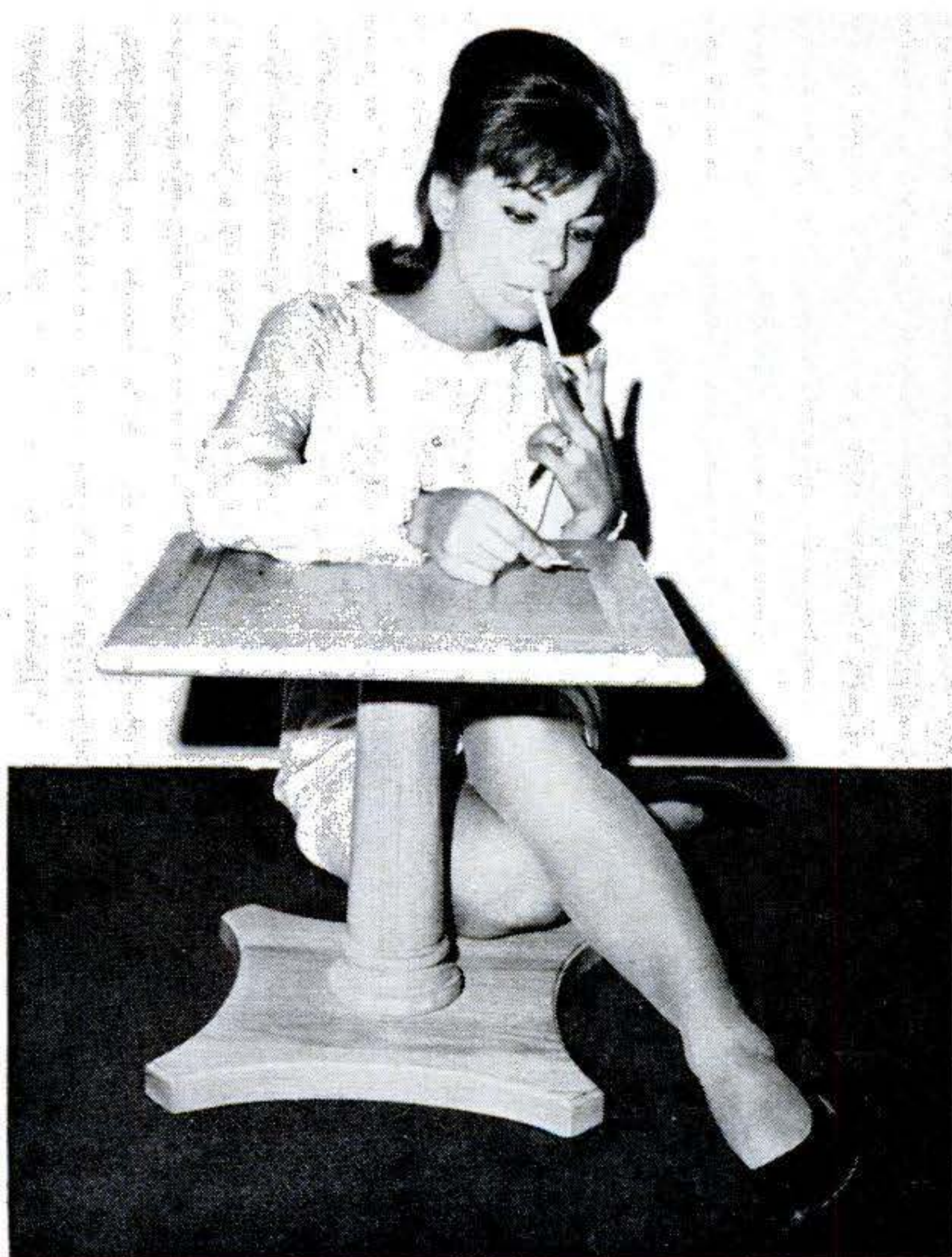
Coffee table made in Kroehler plant withstands burn from match. Scorch can be sanded without refinish.
