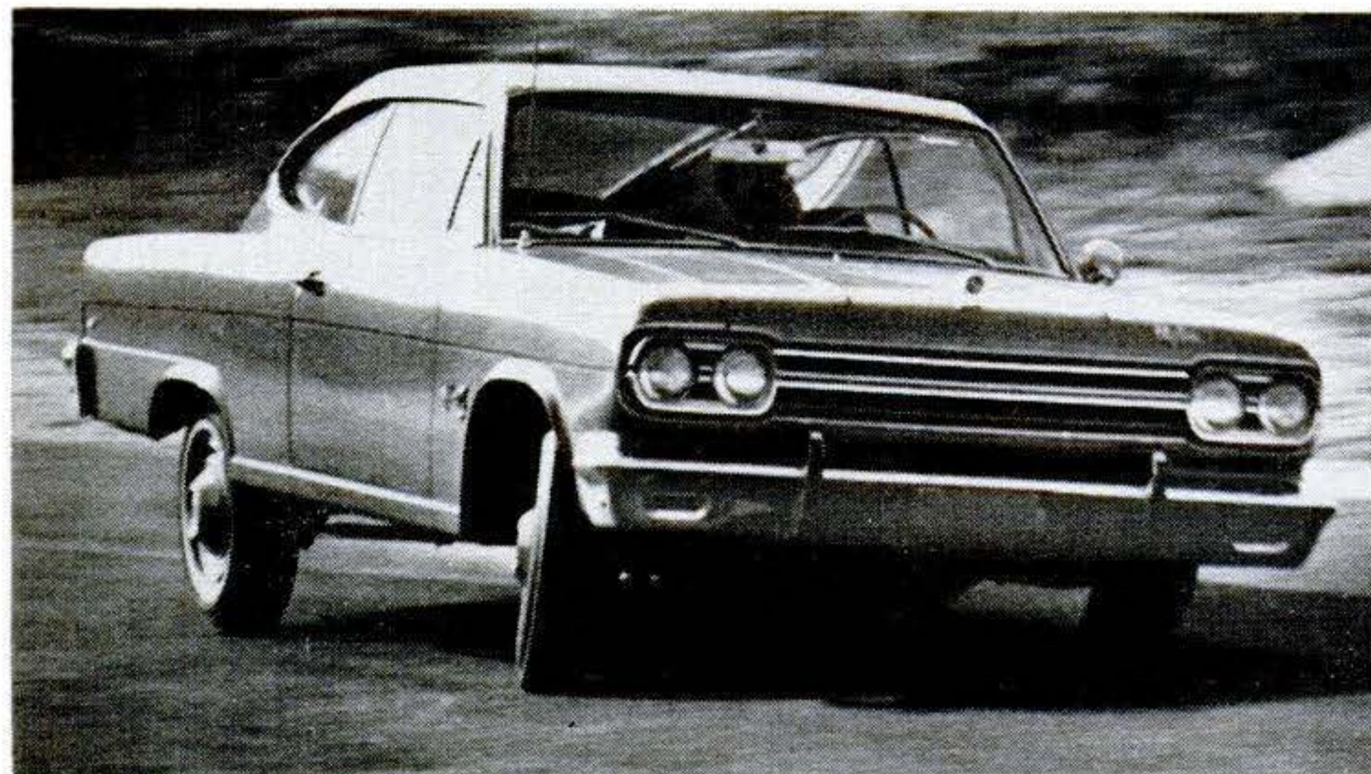
MARLIN has best ride comfort. Hefty stabilizer bar restricts body roll, but car understeers to excess—following its nose, not its front wheels.
