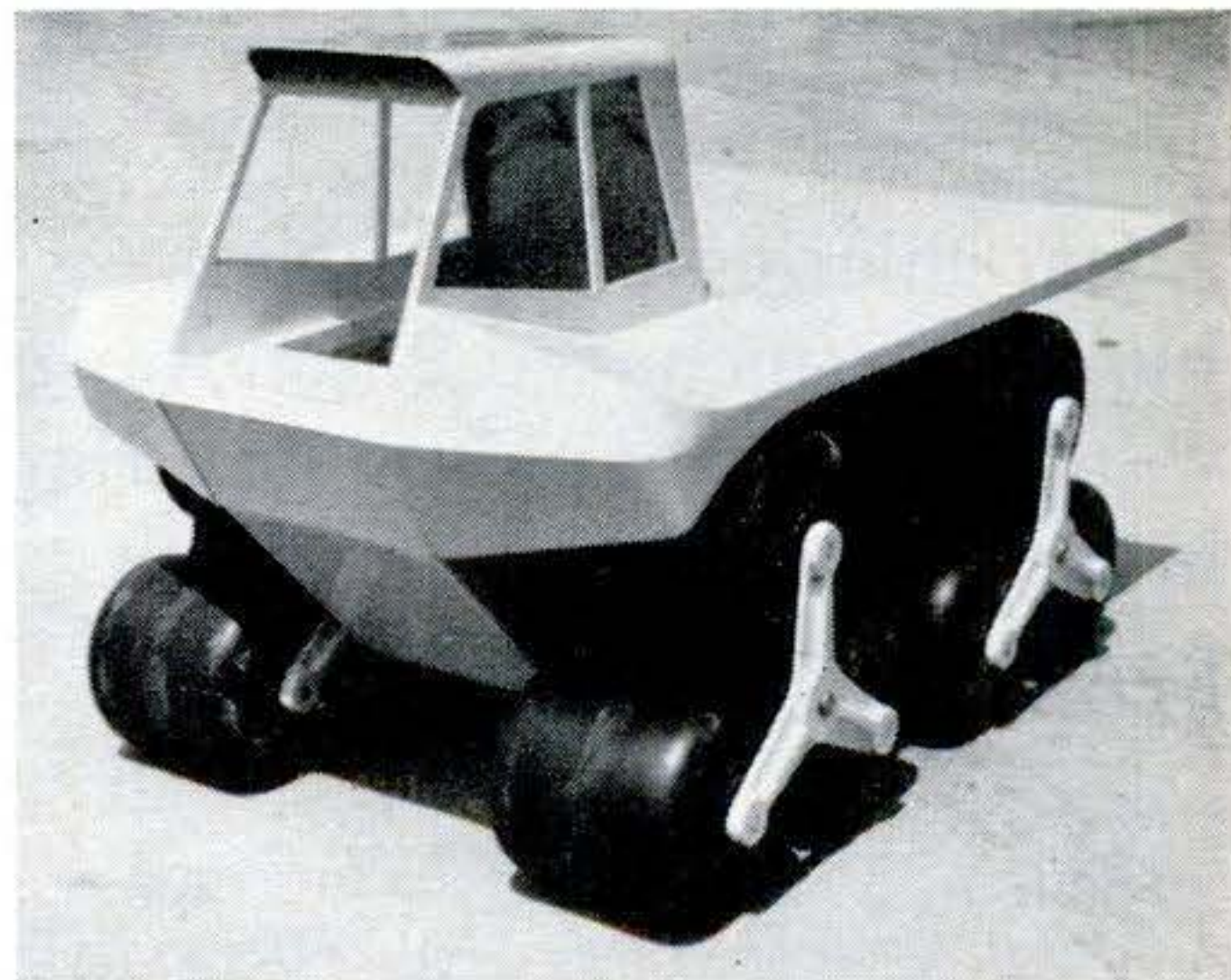
Lower wheels remain level on hard roads.
