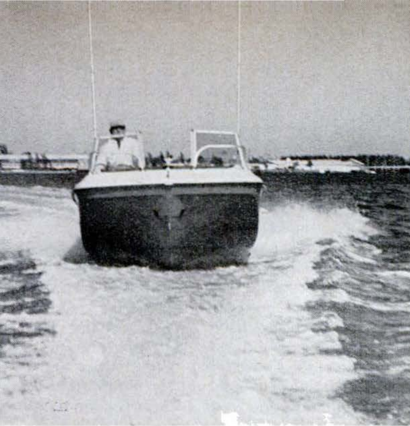
She holds course like a train on tracks, even when astride a bigger boat's wake. The tri-keel hull form is the secret of her directional stability.
