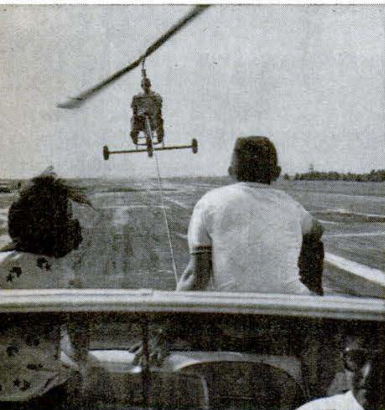
A Gyroglider (without engine) looks like this from the ground at the end of a tow rope tied to a car.
