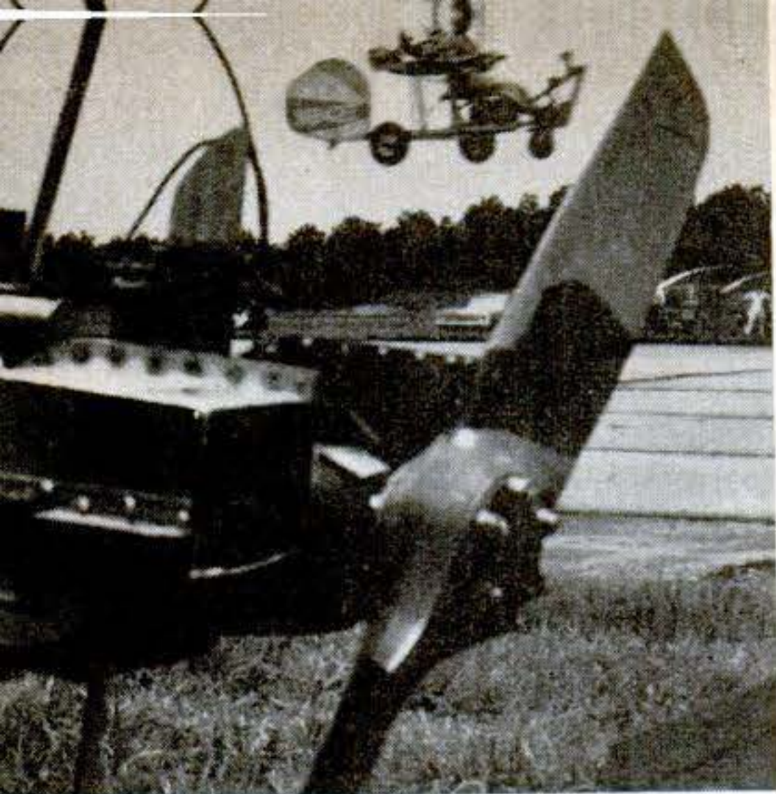
Engine frequently is a surplus four-banger built for the Air Force to power a radio-controlled target. Price: as little as $149.
