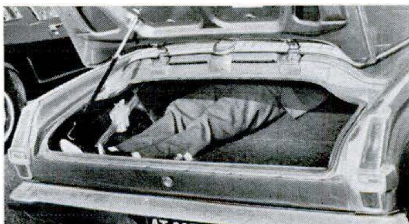
BARRACUDA carries spare below trunk floor. The tank filler neck sticks through the left fender. Rear seats fold away to create station-wagon-like area.
