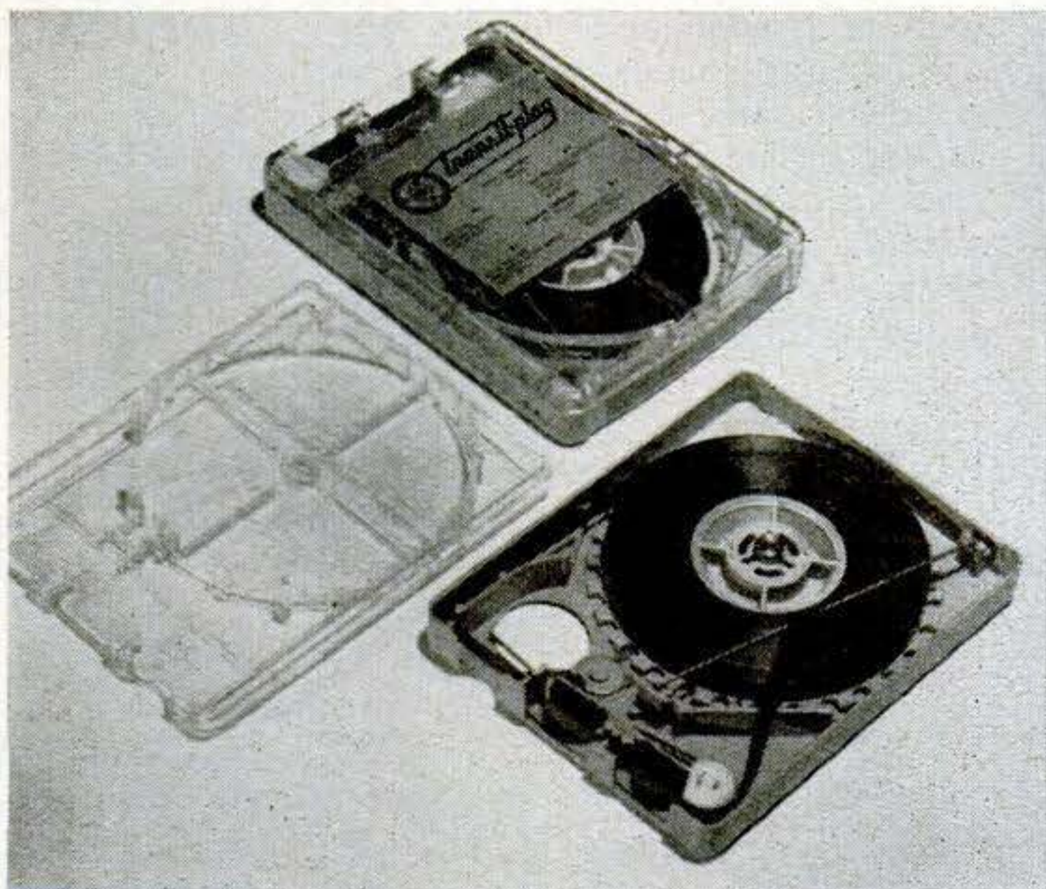
The "300" cartridge is loaded with 394' of lubricated tape, spliced to form a continuous loop. Monaurally recorded cartridges contain four adjacent music tracks, and play for a total of one hour.
