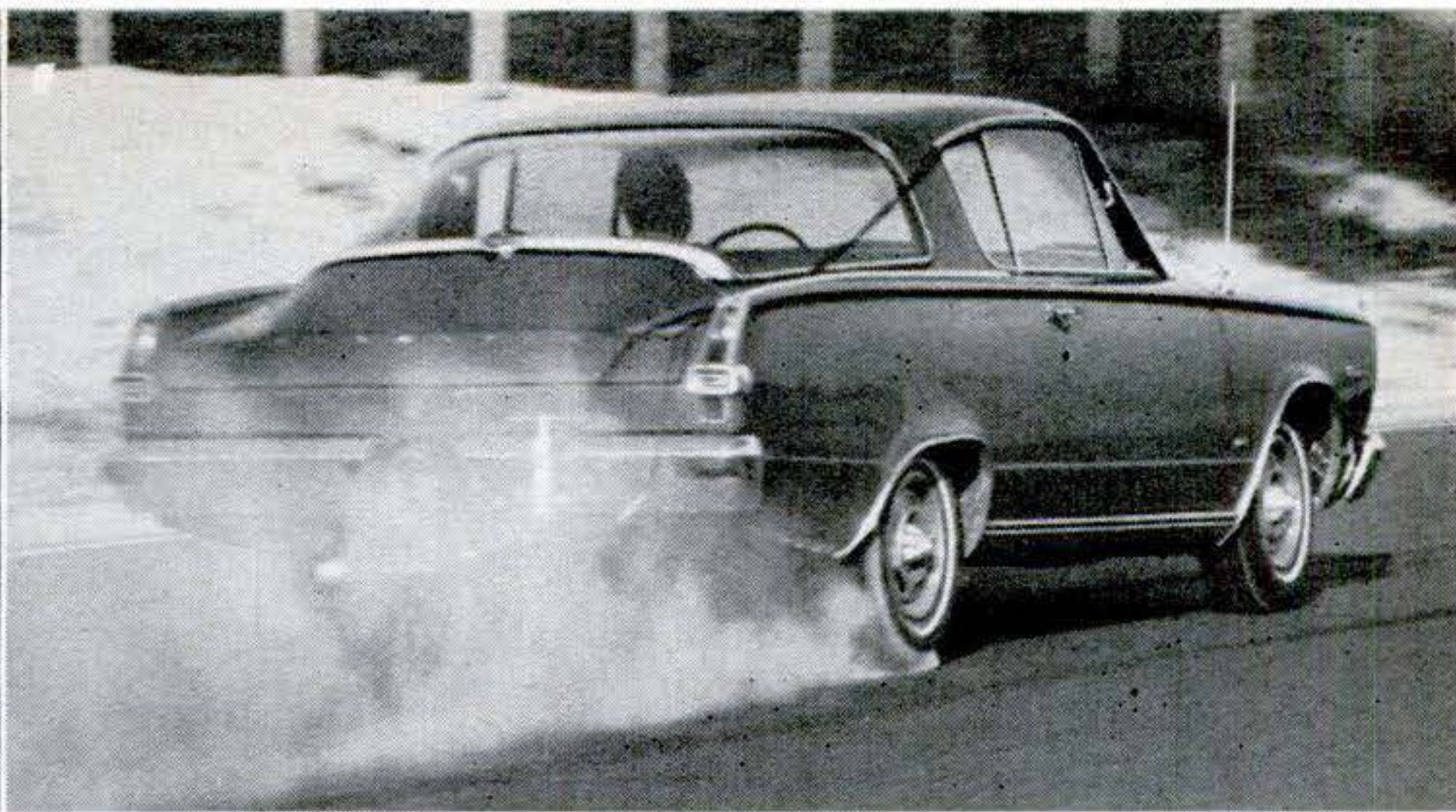
BARRACUDA brakes were poor. Front-brake fade set in early, and locking-up the rear wheels failed to shorten braking distances significantly.
