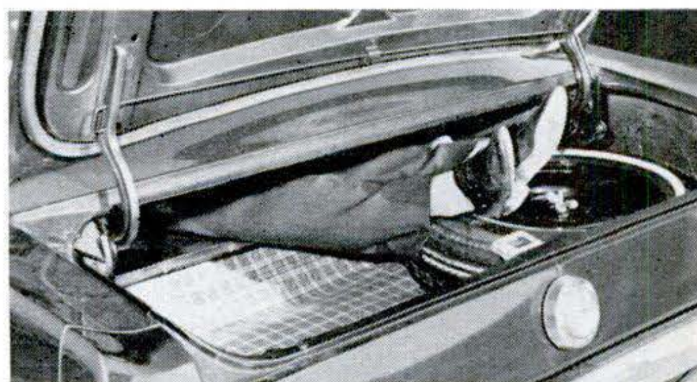
MUSTANG has low and wide trunk. Spare wheel hogs space. The rear seat folds away to carry odd-shaped loads. Fuel-tank cap is below the trunk-lid lock.
