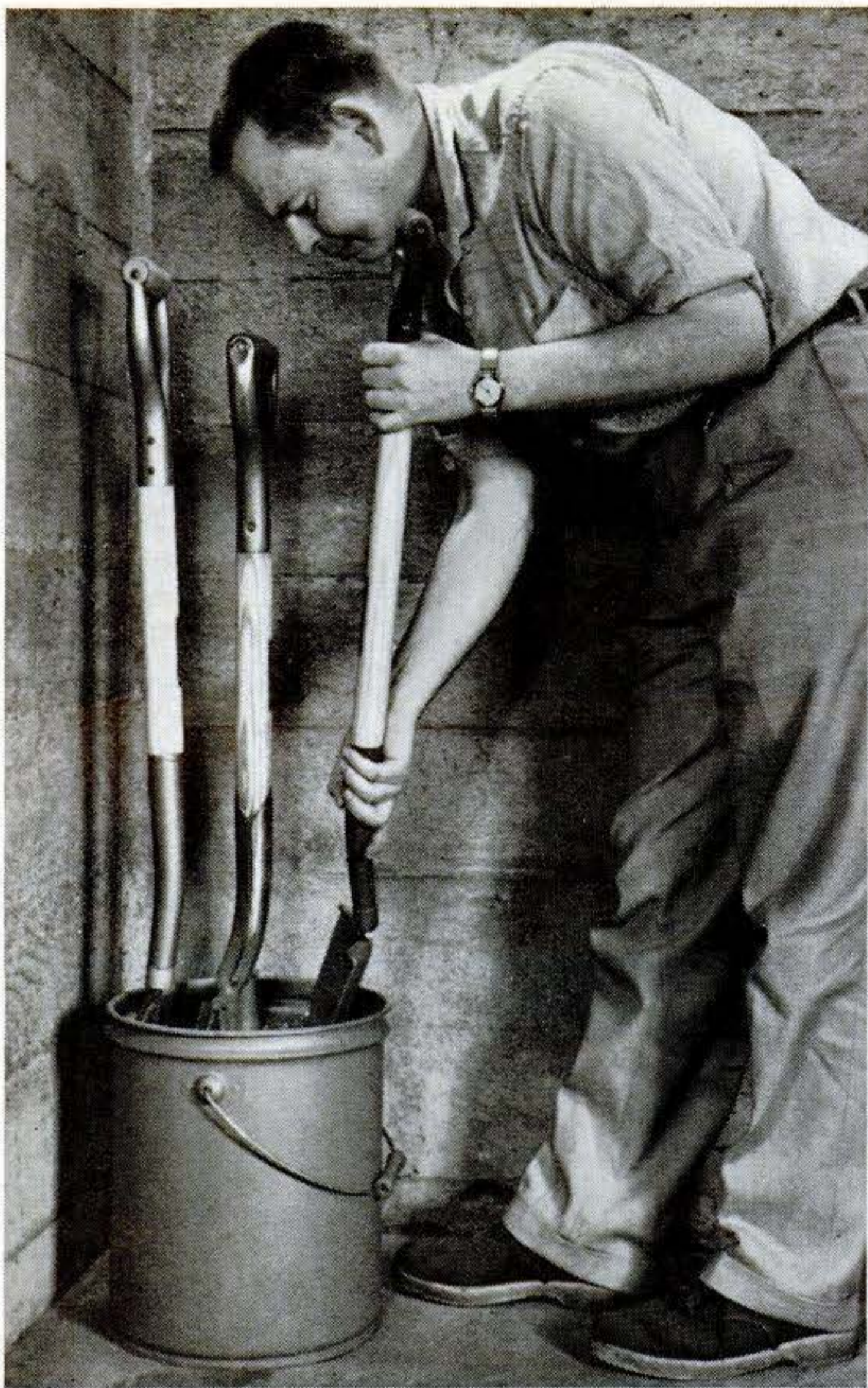
Garden spades and shovels can be cleaned, oiled, and stored in a container of oily sand. Mix about a pint of motor oil thoroughly into dry sand. Work shovel up and down to clean it and coat it with oil.
