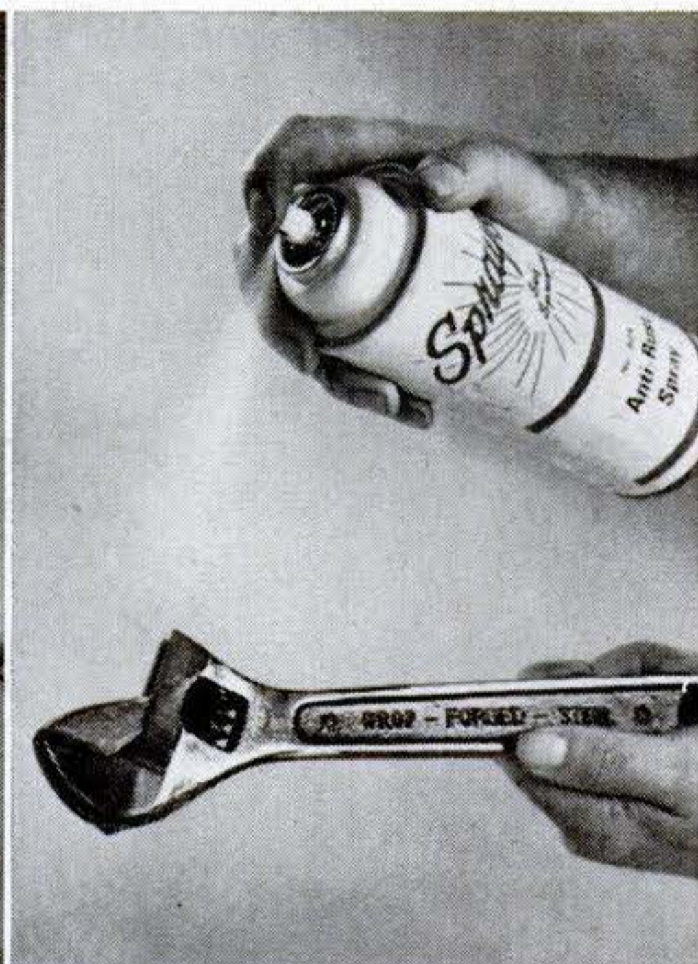
Steel tools used only occasionally should be coated with rust inhibitor. Anti-rust spray you buy at the hardware store displaces moisture and dries to a protective film. Solvent removes the coating. PS
