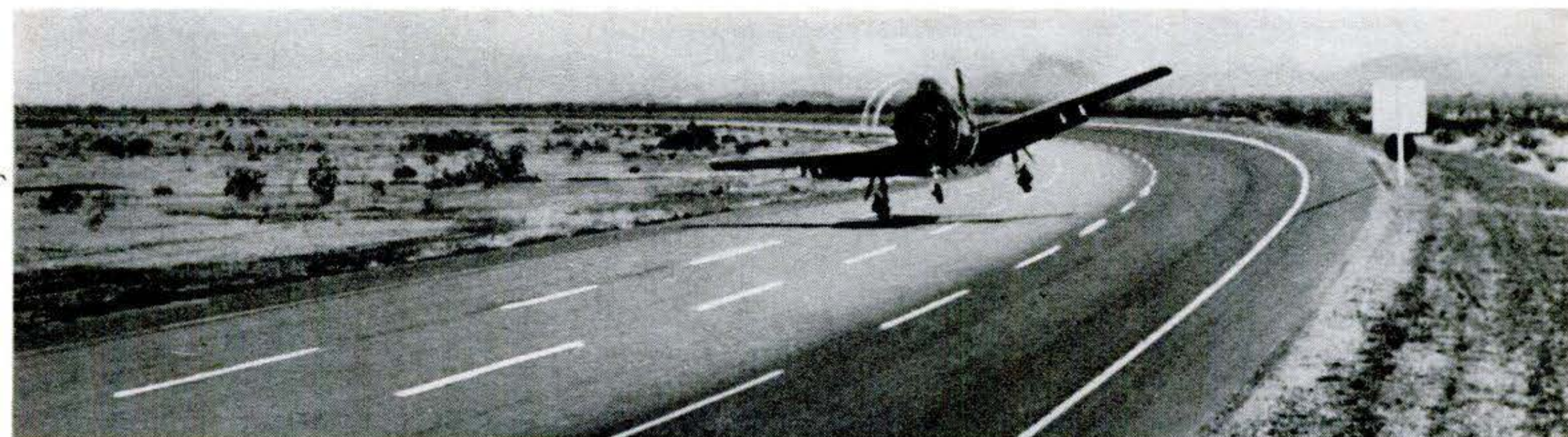
Navy plane touches down on banked circular track in Arizona, in one of many successful trials with
