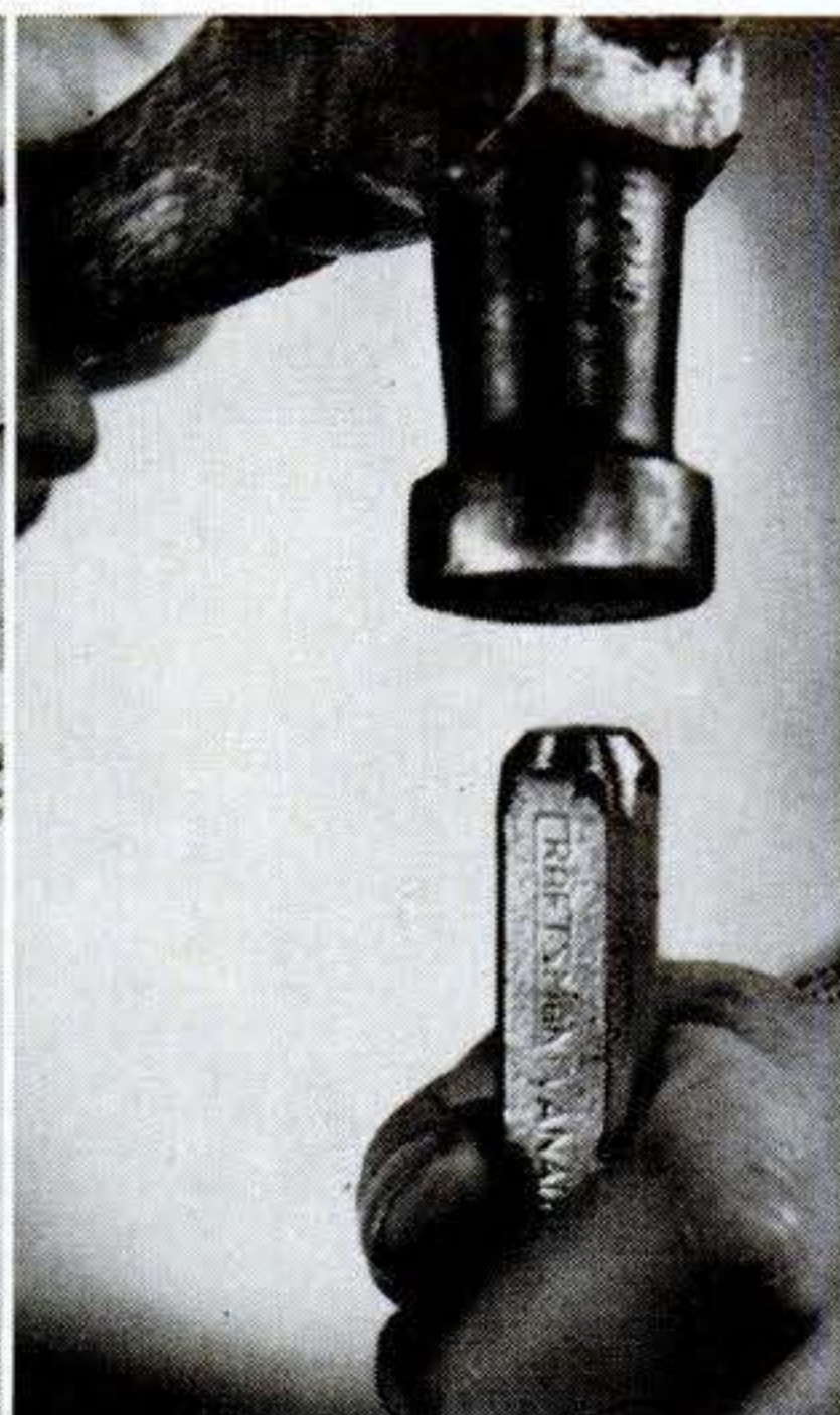
Tools you whang with a hammer—cold chisels, punches, star drills—gradually mushroom over on the striking end. To keep bits of steel from flying off, chamfer the heads.
