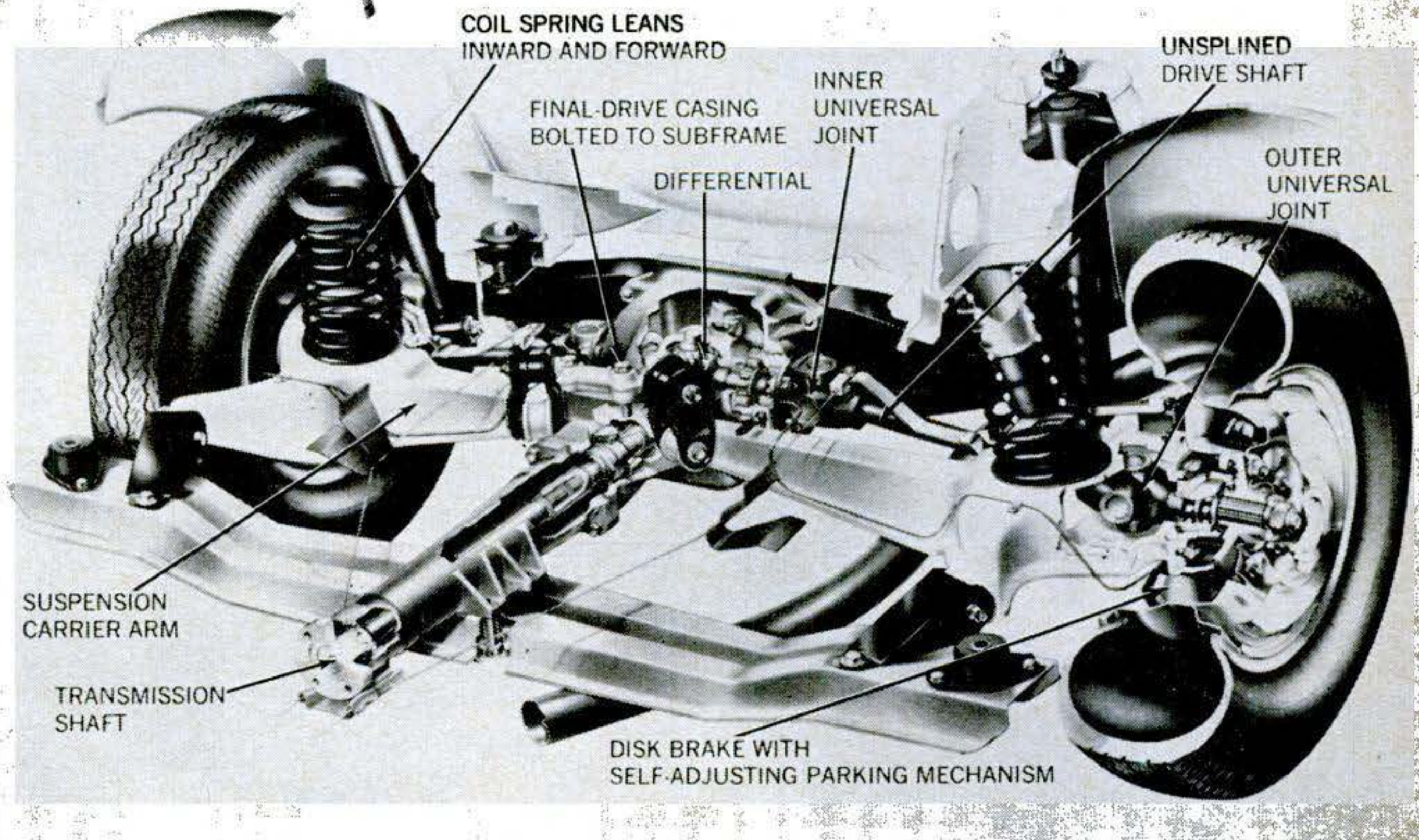
Unsplined half-shafts and semitrailing arms are combined in Ford Zodiac's unusual rear suspension.
