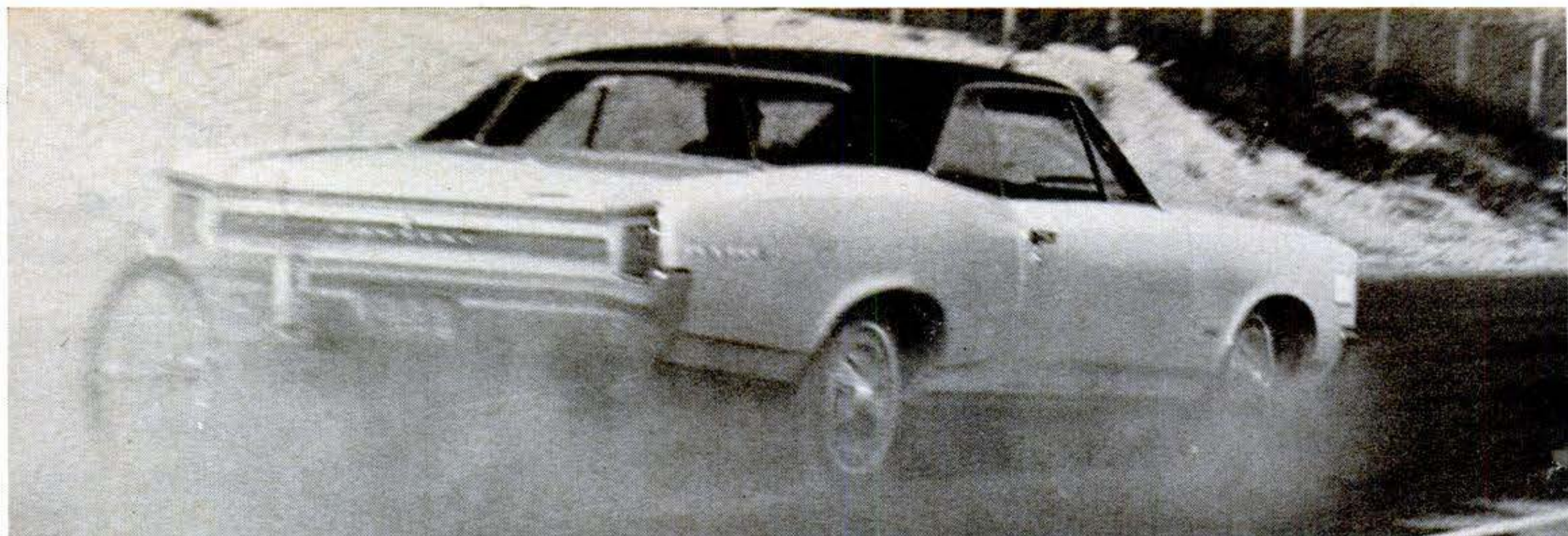
Le Mans stopped from 65 m.p.h. with severe nose dive and slight pull to right.
