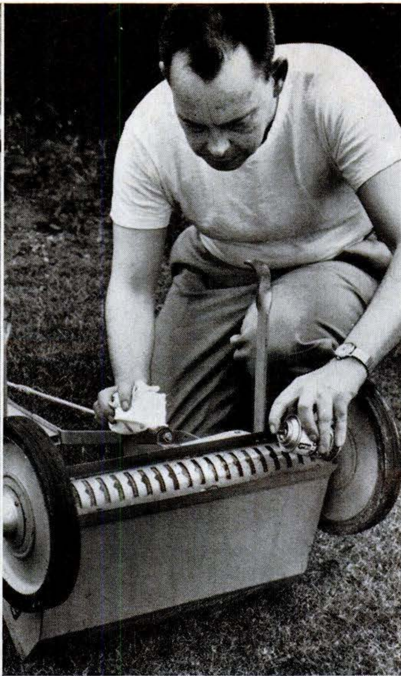
Don't wash a fertilizer spreader with water. Most fertilizers are chemical salts that, when dissolved, are quite corrosive. Wipe down the spreader with a dry rag, then spray the shutter mechanism with oil.
