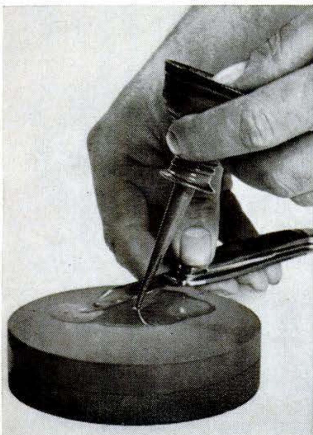
Oilstones last almost forever if cleaned regularly. Use a shallow pan of lacquer thinner. Clean off the gummed oil with a rag. Use lots of oil when whetting; it keeps cuttings from loading the grit.
