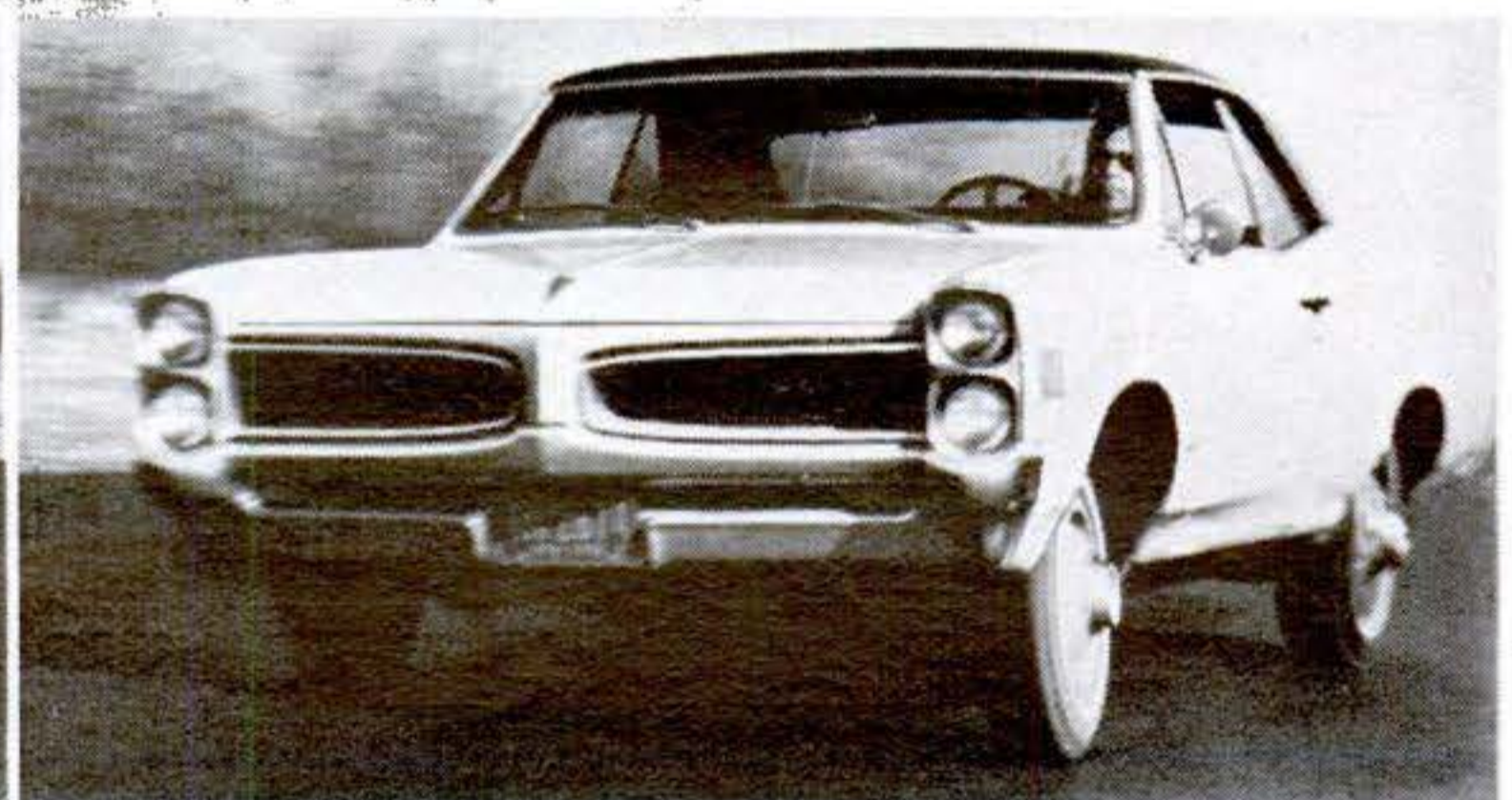
Le Mans enters curve with slight understeer . . . . . remains neutral throughout curve until . . .
