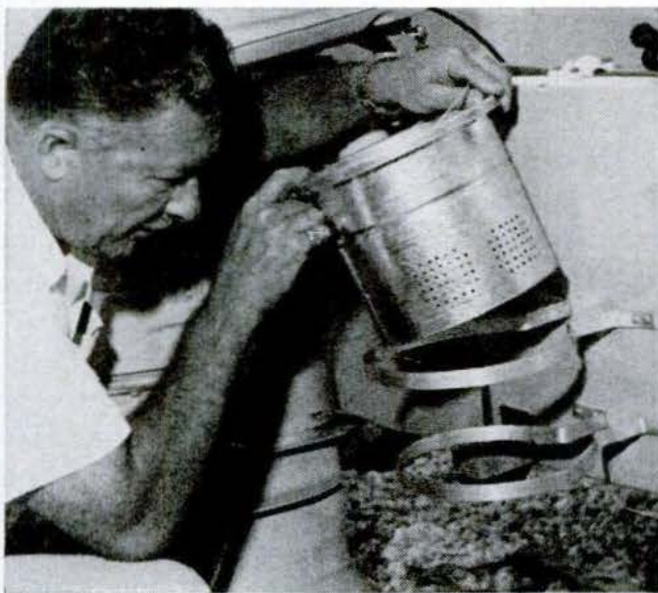
Aluminum straps hold bait bucket to transom. Fasten the straps with aluminum screws to prevent corrosion from dissimilar metals.
