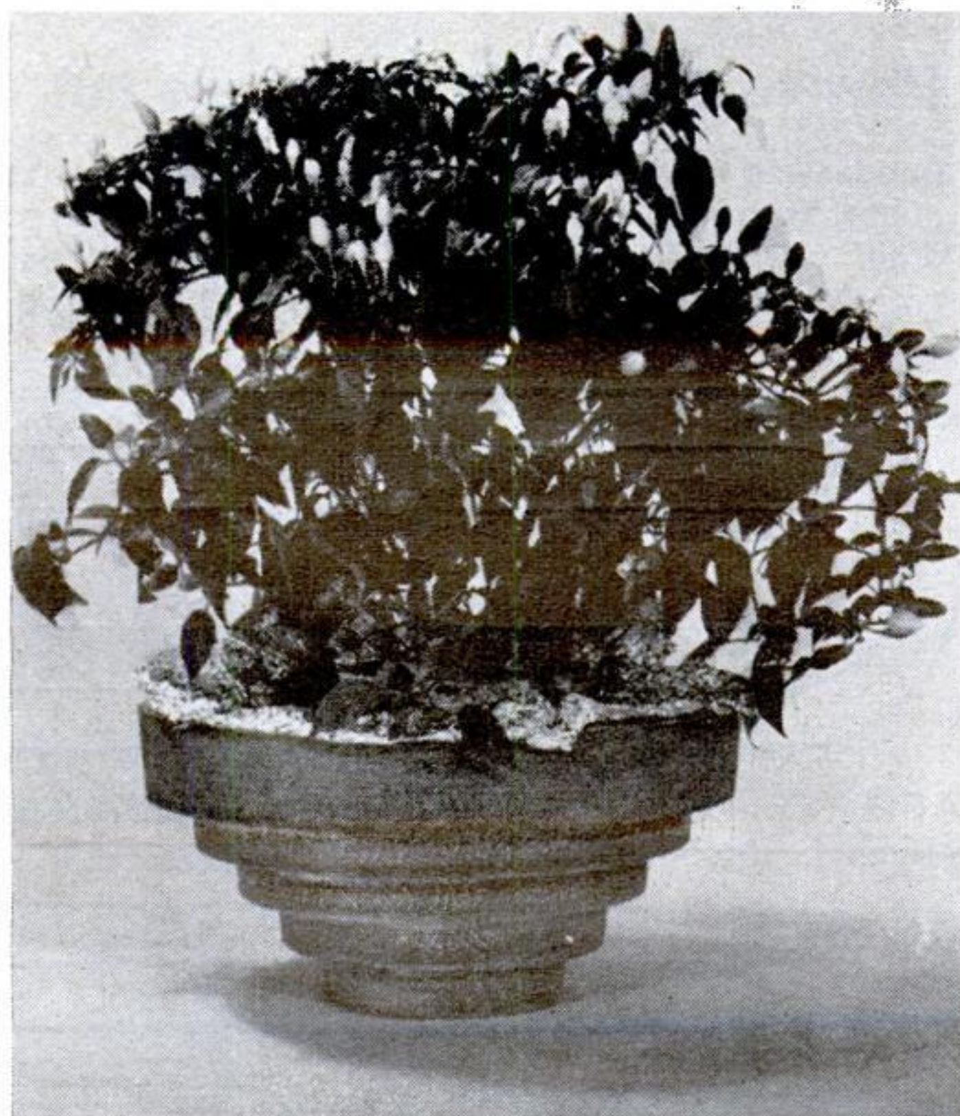
Planter , 6" deep and 10" in diameter, was cut from a piece of stock 1 \frac{5}{8} " thick by 10" square. The edge of each piece was coated with glue; it was then forced tightly into the piece it was cut from.
