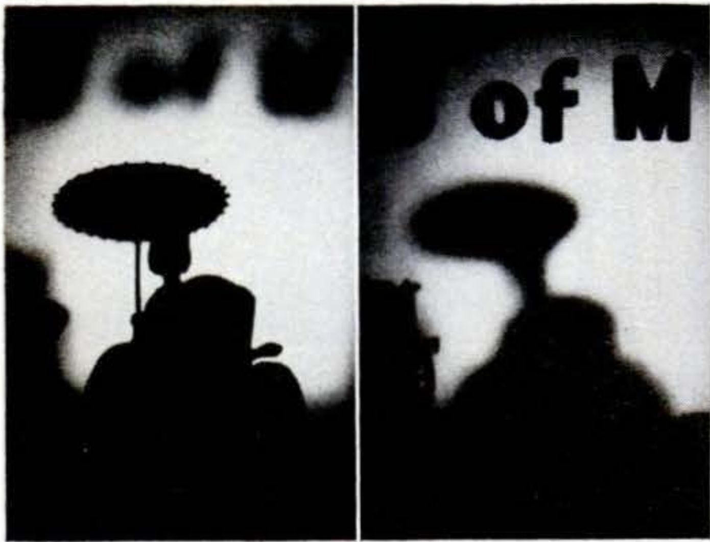
Two conventional photos of a single reconstructed hologram show its true 3D nature. Focusing on the figurine of a girl in a rickshaw throws top of sign out of focus; focusing on sign defocuses rickshaw.
