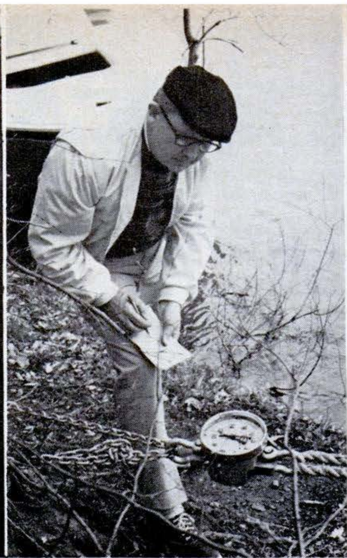
Scale interposed between tree and line to boat tells the story of the maximum thrust exerted by jet discharge. At 4,200 r.p.m., it was 1,350 pounds.
