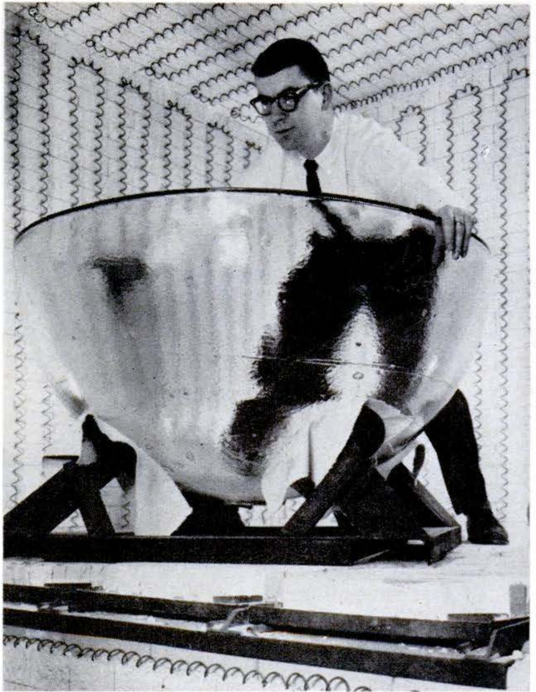
First of the big glass bubbles: Corning 44-inch hemisphere (slightly smaller than the 56-inch units now being cast) is placed in an asbestos-lined annealing oven. Annealing eliminates internal strains.
