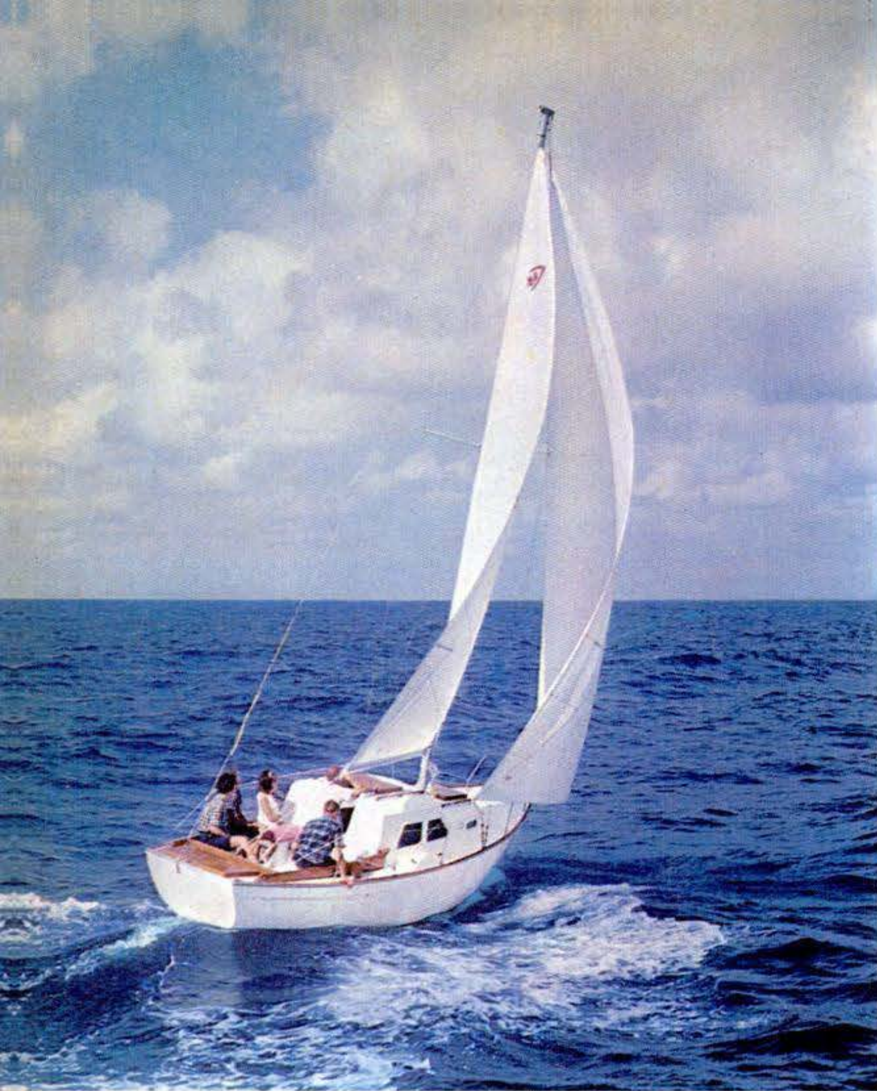
Chris-Craft Capri is 26-foot fiberglass Sparkman-and-Stephens-designed sloop. Four berths, 301 square-foot sail, 4,800-pound displacement.
