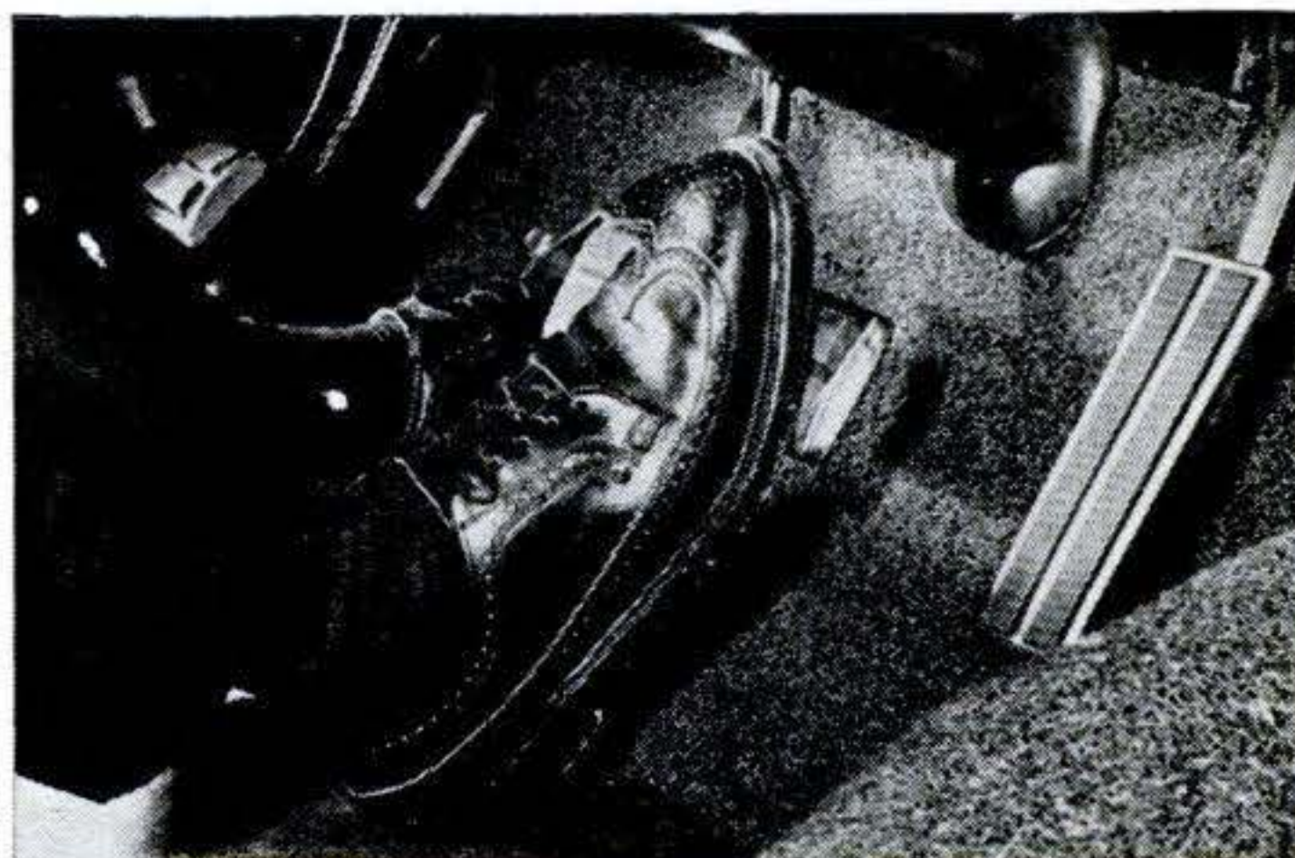
Power-brake pedal with little travel on the Mercury was inconveniently high (five inches) off the floor.
