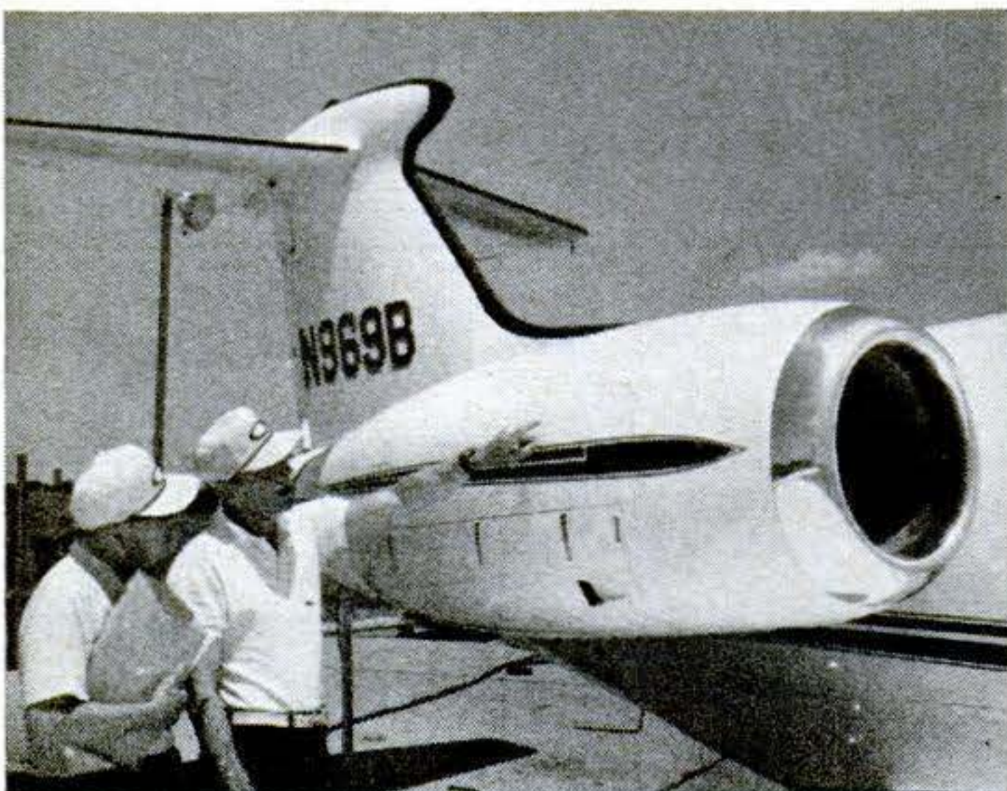
Kaye shows PS writer Francis one of two engines, each producing 2,850 pounds of takeoff thrust.
