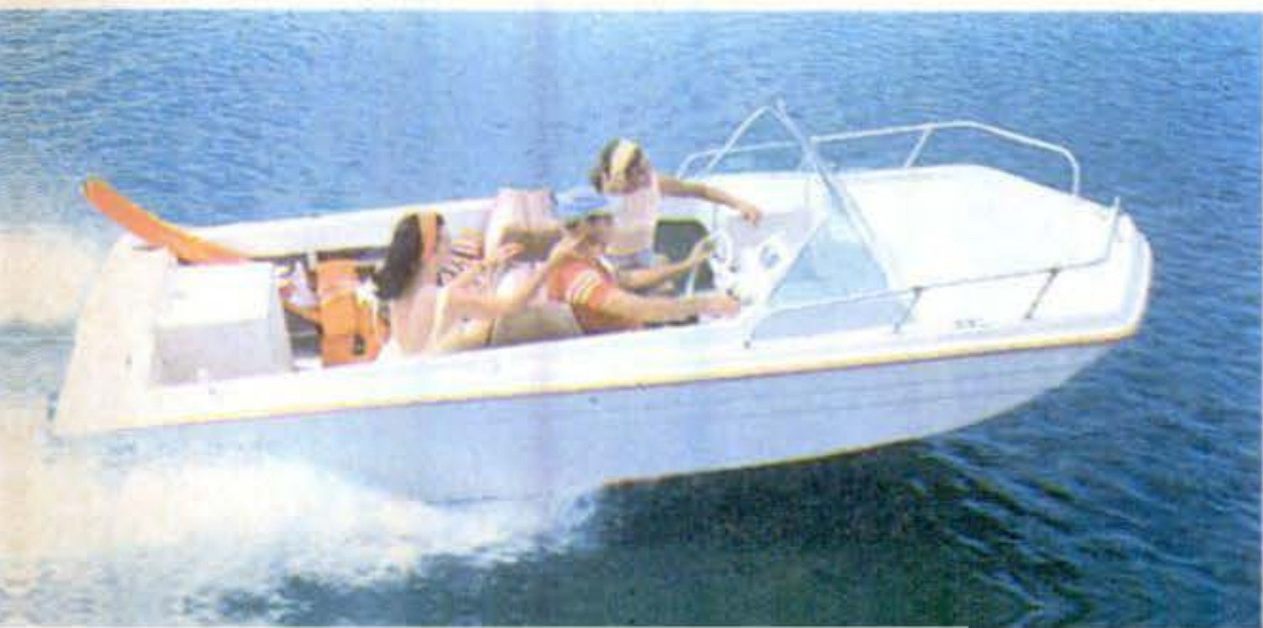
Thunderbird has a stable-riding cathedral hull. Boat above is powered with MerCruiser 120-hp. stern drive. Models are available from 15 to 22 feet.
