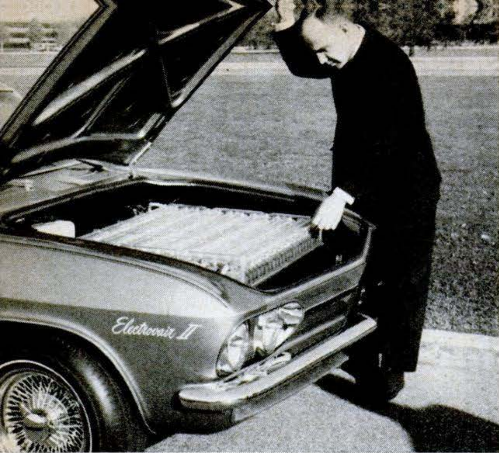
PS Detroit Editor Dunne looks over car's forward batteries. Tires are oversize to carry added weight.
