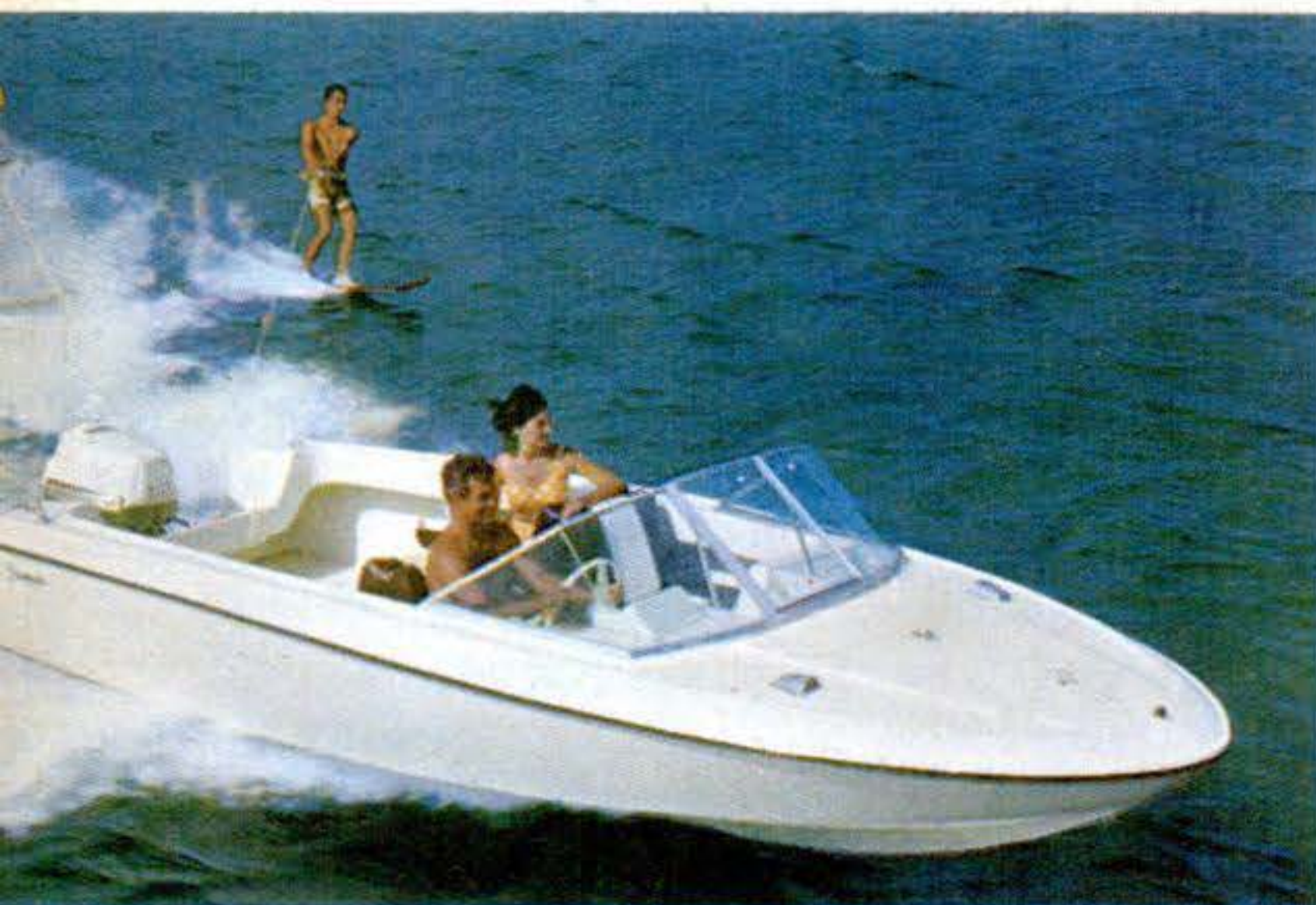
Formula 190 and Johnson outboard team up as top ski combination. Fiberglass 19-footer has tangent chine for stability at rest and moving.
