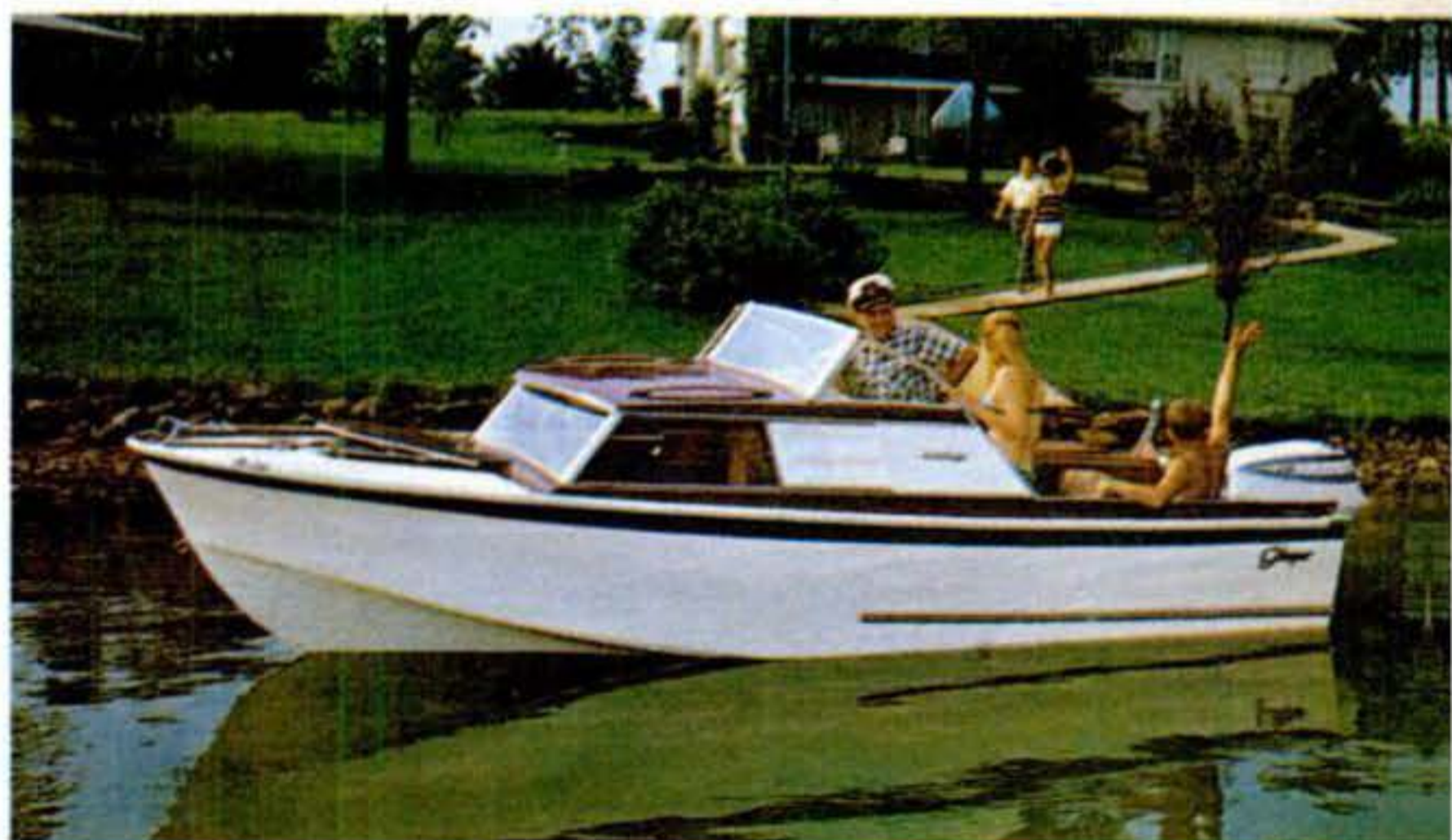
Evinrude-powered Glasspar Seafair Sedan is 17 feet long. Has twin bunks. Fiberglass, with modified-V hard-chine hull. Two 12-gallon gas tanks.
