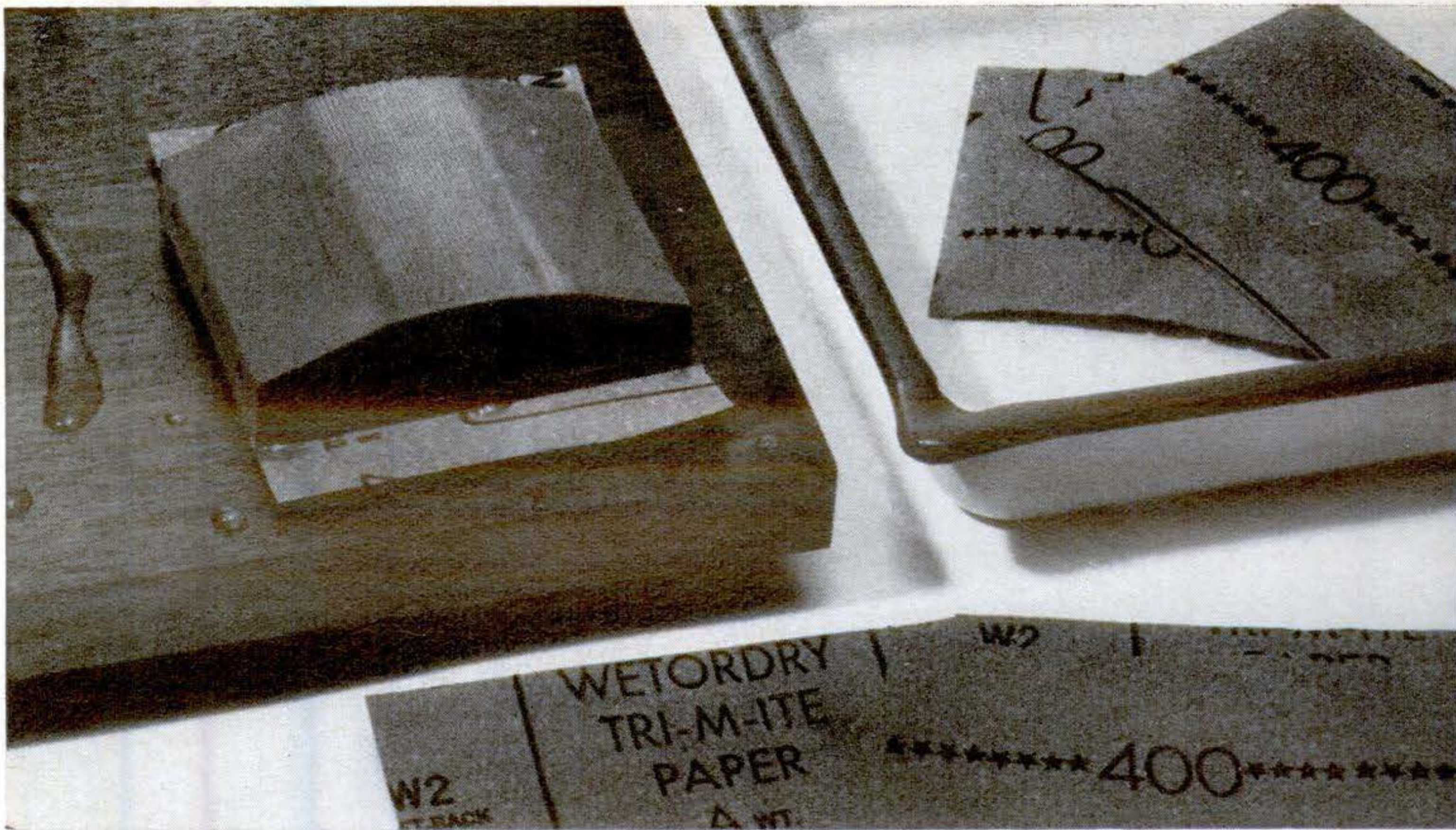
Water and waterproof sandpaper used with a rubber block is the fastest, smoothest way to a rubbed finish. Use 400-grit paper or finer. Keep a few pieces soaking as you work so the backing is soft before you use it.
