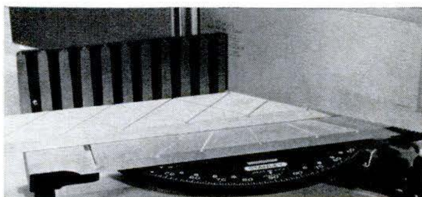
Decorative surface cuts like this diamond pattern are feasible in unlimited variations by changing saw angle, attitude of work, and depth of cut.
