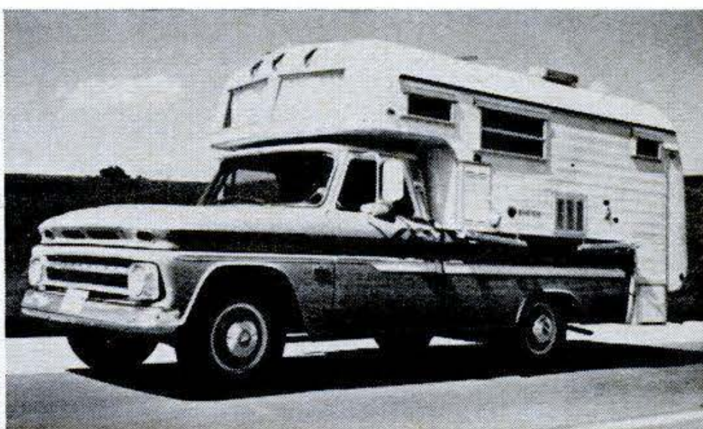
Ready to roll: Photo shows the Interstater with back retracted flat for highway use.
