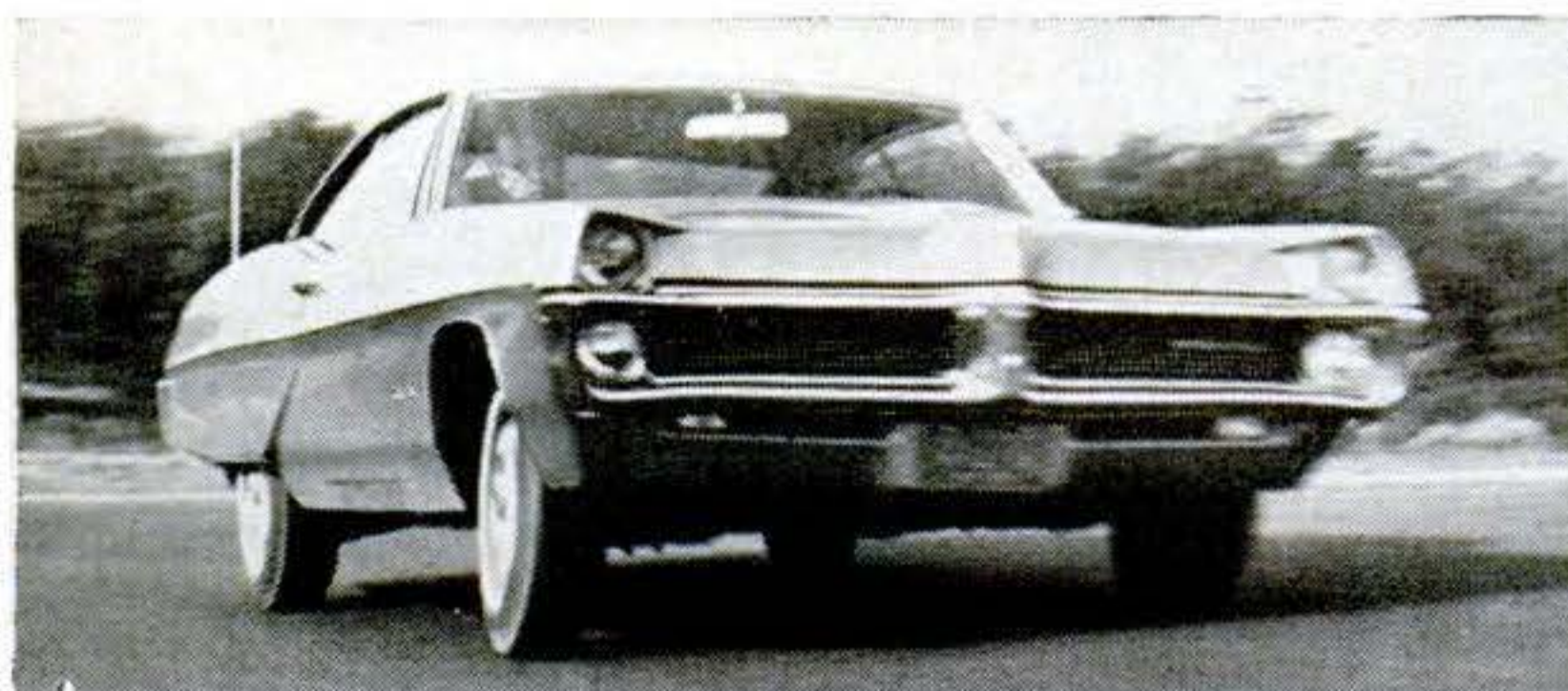
Pontiac's tail began to drift out when side force reached 0.84 g on a 255-foot-radius turn.
