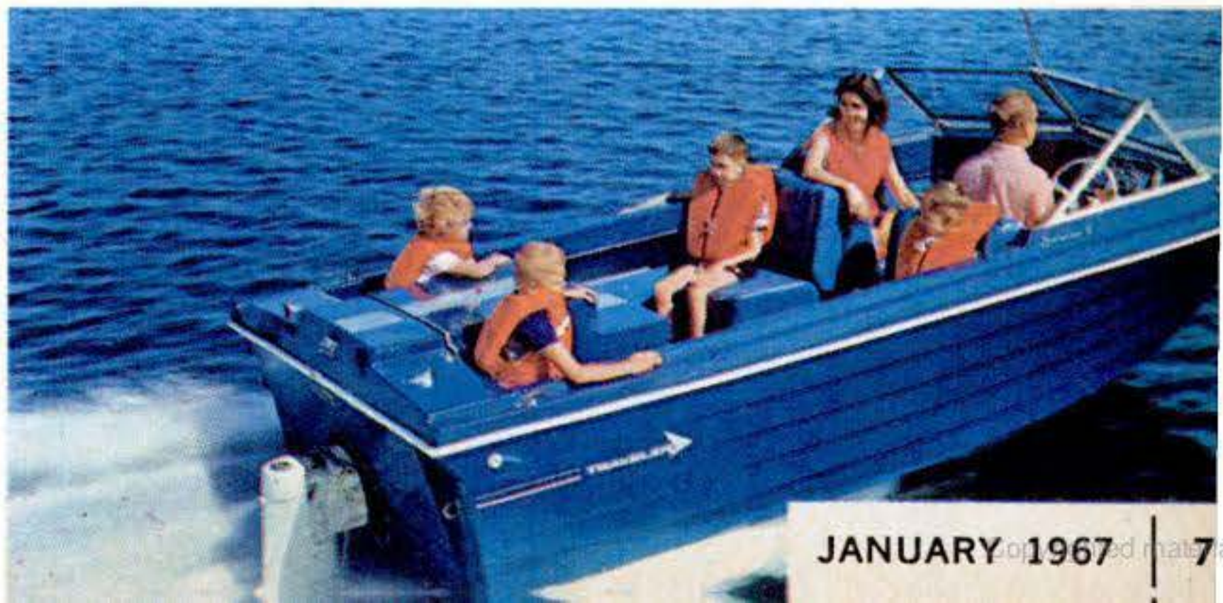
Traveler Saturn is a husky 17-foot multipurpose runabout. Power comes from OMC stern-drive unit. It handles up to 160 hp., has deep-V keel.
