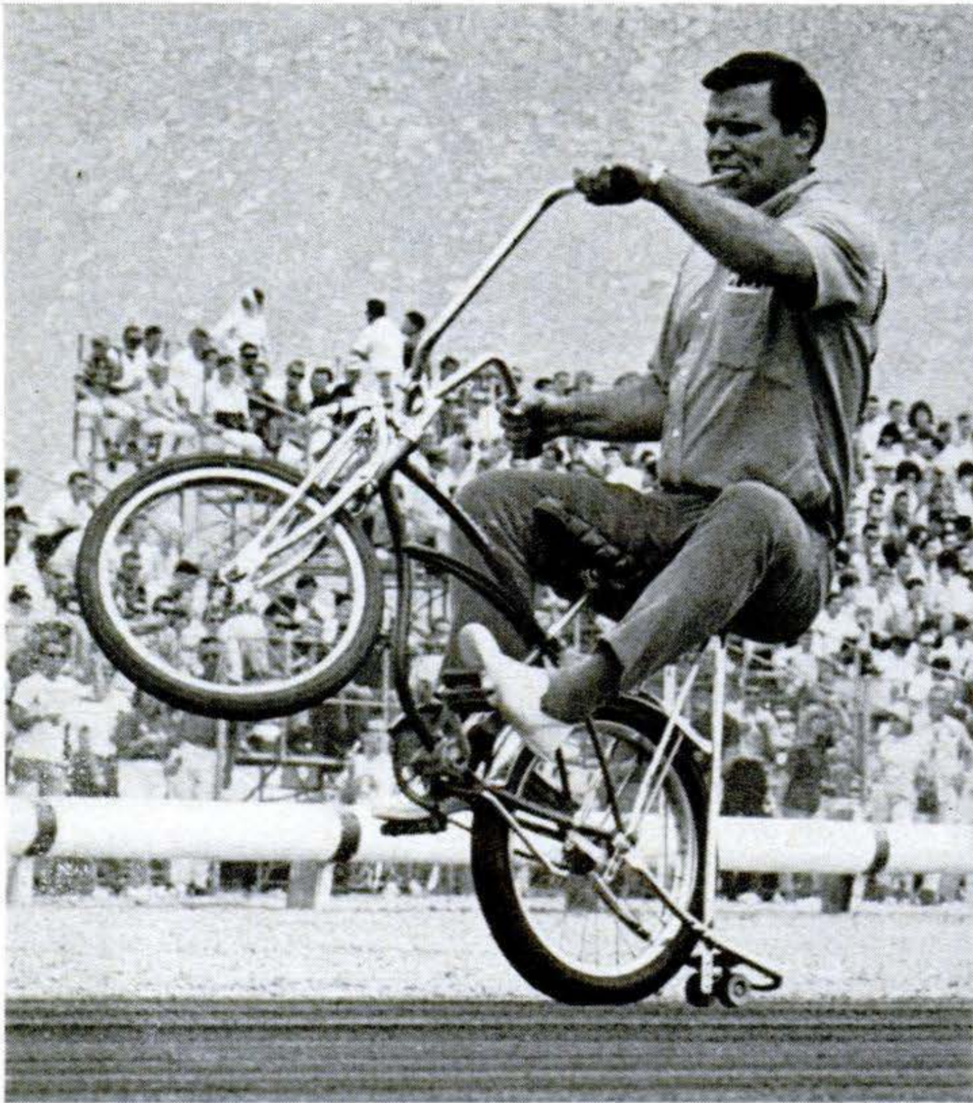
Wheelie-Bar attachment is made of steel tubing and skate wheels.
