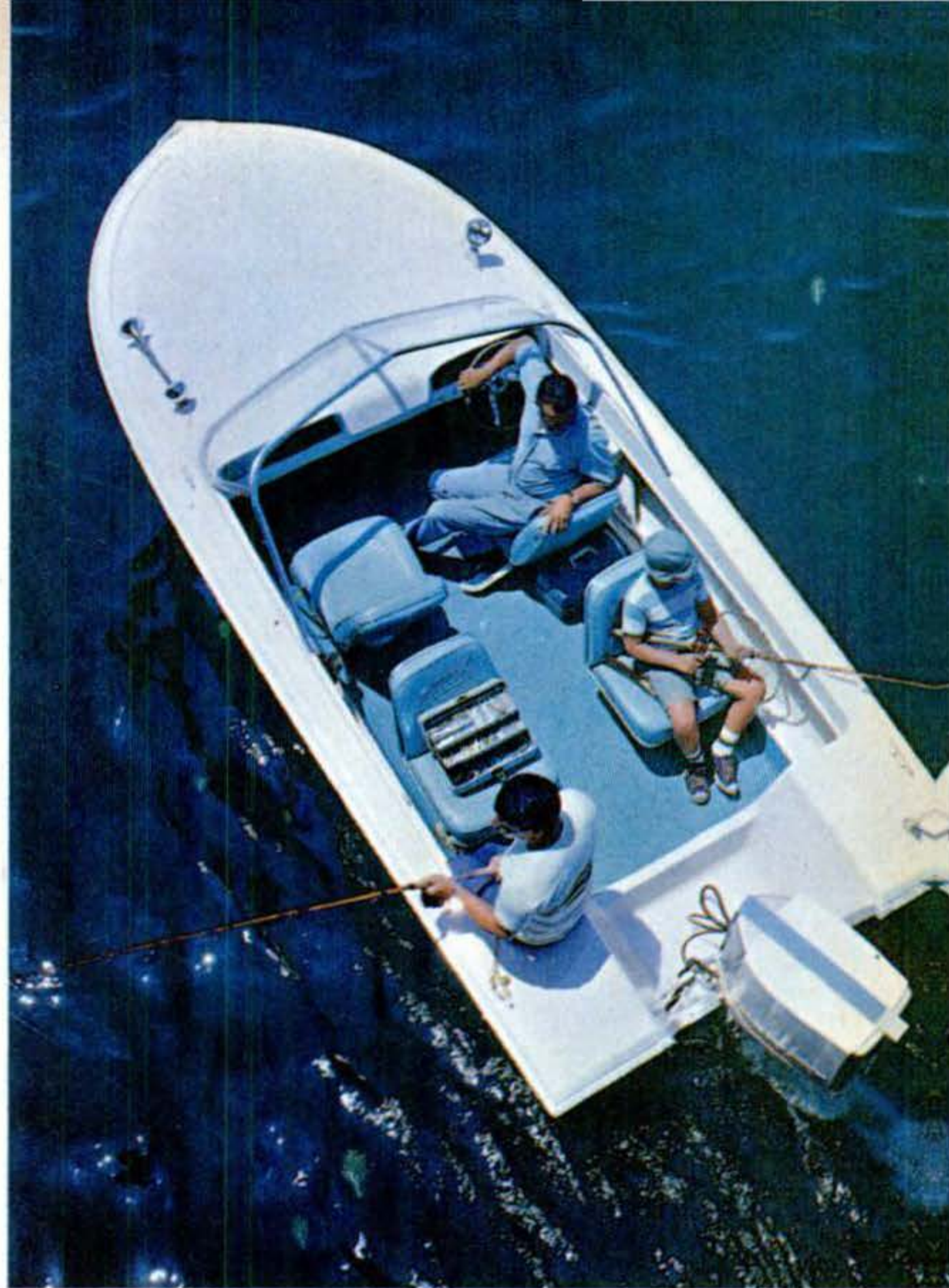
Starcraft's 16-foot Upstart claims a new feature: the ability to right herself from a swamped position without help from crew or centerboard.
