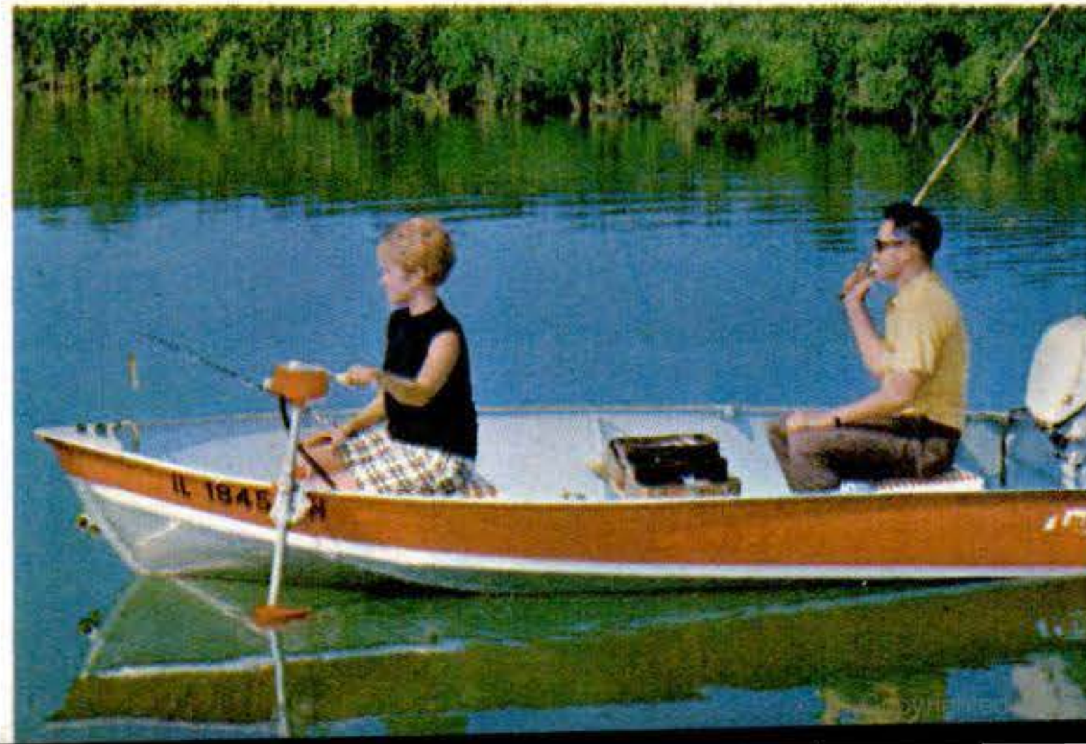
Lund aluminum Fisherman has Johnson outboard on the stern, new Tempo-Troll electric trolling motor at the bow. Rheostat controls trolling speed.
