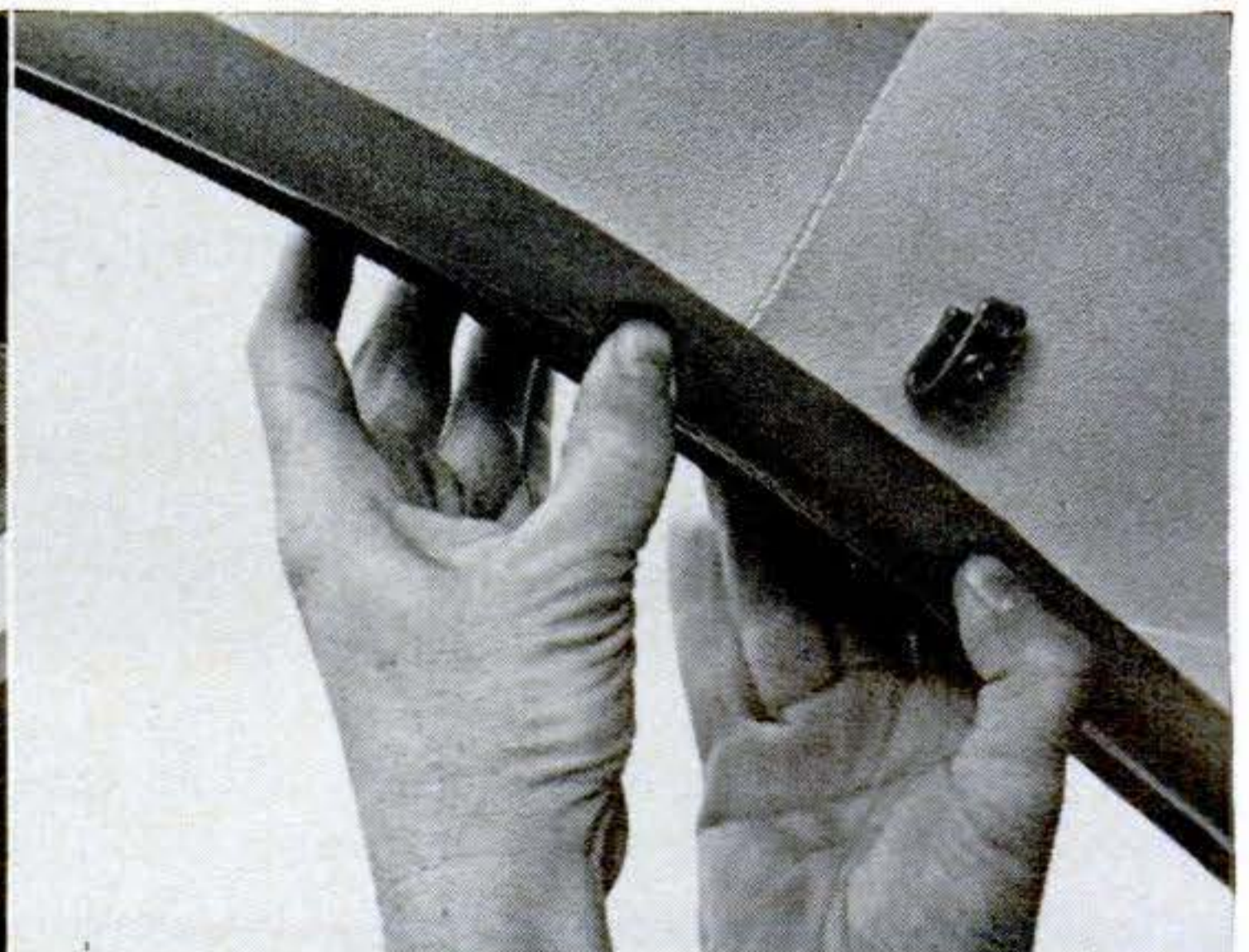
Soft-padded molding surrounded the roof girders on the Mercury—a small but good safety item.
