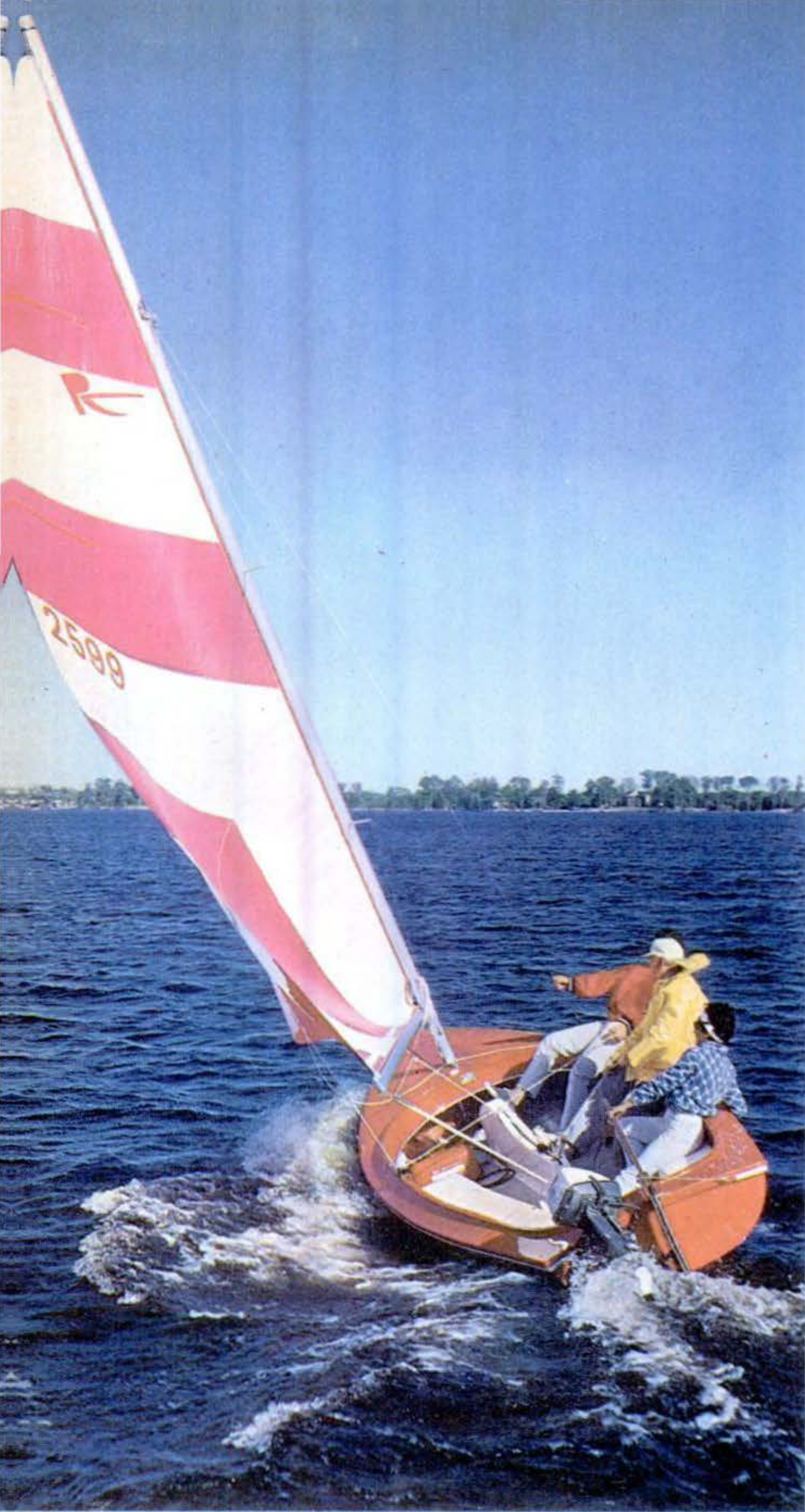
Sleek Rebel is one of a fleet of fine sailing craft made by Ray Greene & Co., Toledo, Ohio. A 16-footer, the Rebel has a fiberglass hull and is sloop rigged.
