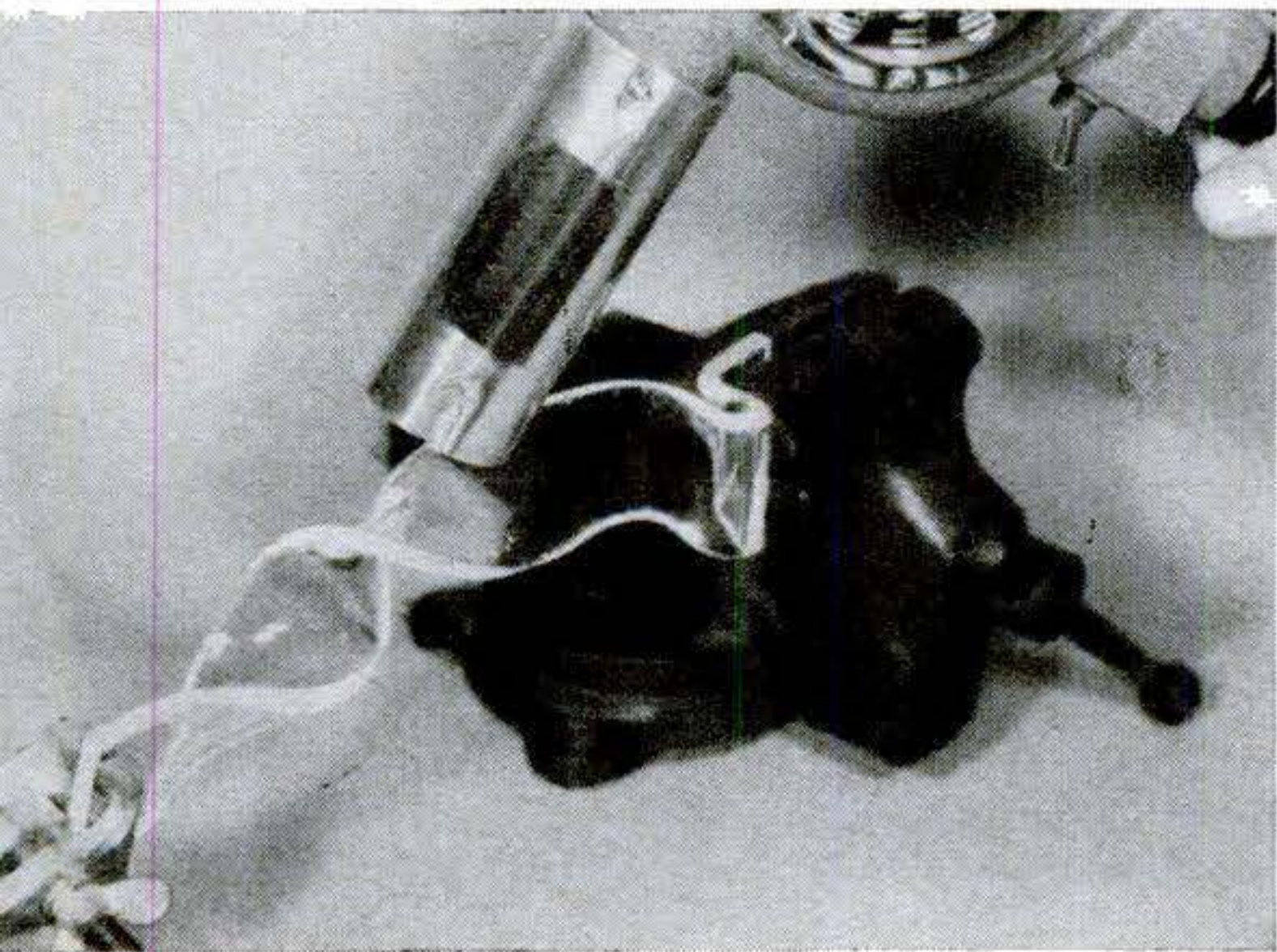
Gun readily heats plastics for forming and repairing. Most plastics soften at around 325 degrees.
