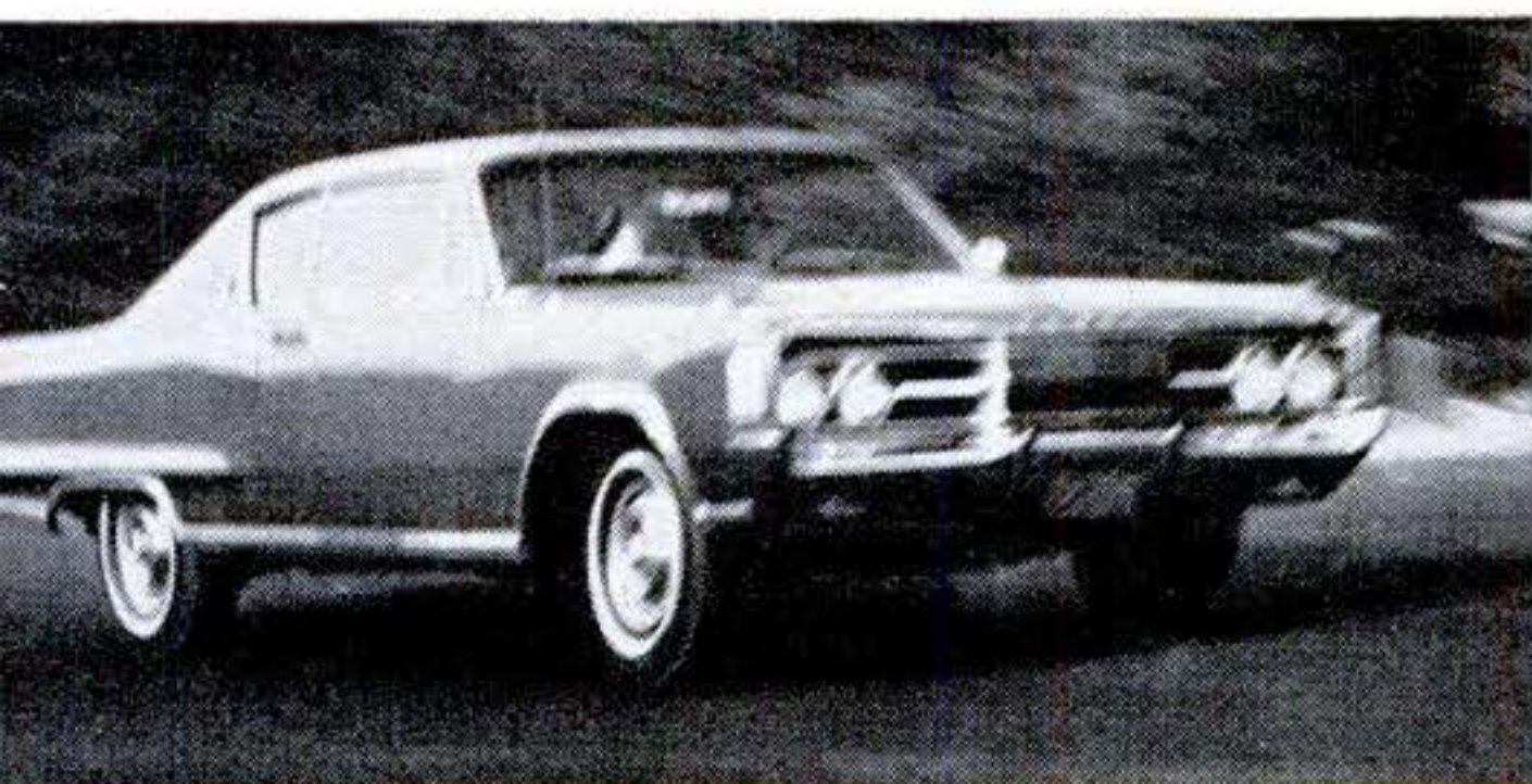
Dodge threatened early tail-end drift but the car maintained stability up to 0.82-g side force.
