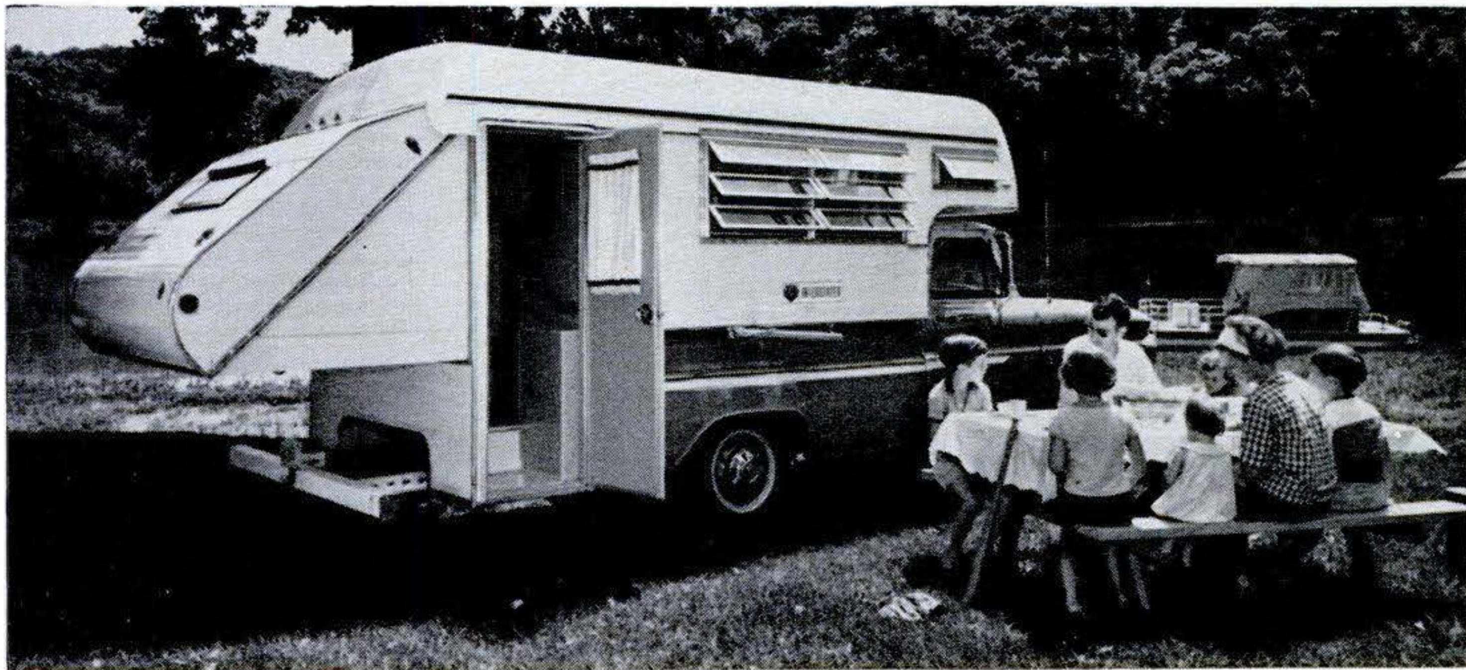
Camper's back pops out when you're stopped and increases the interior living area by about a third.
