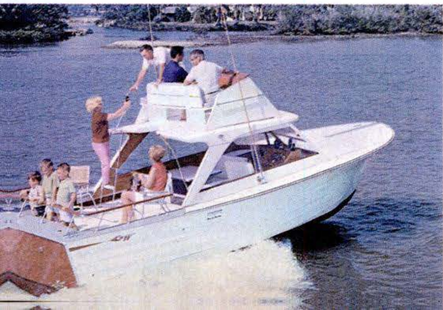
Grady-White Catalina hardtop is 27 feet long. Of lapstrake design, wood construction. Has 220-hp. engine, or can be fitted with twin 157-hp. engines.
