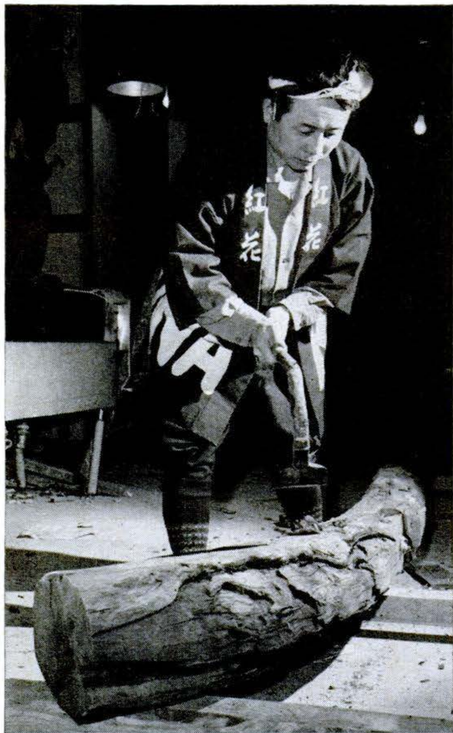
Using curved-handled adze, Shoji fashions a beam out of a rough piece of timber. The rough marks of the adze on the surface are not smoothed out but are left there to make an interesting textural pattern. Japanese name for this tool is chona.
