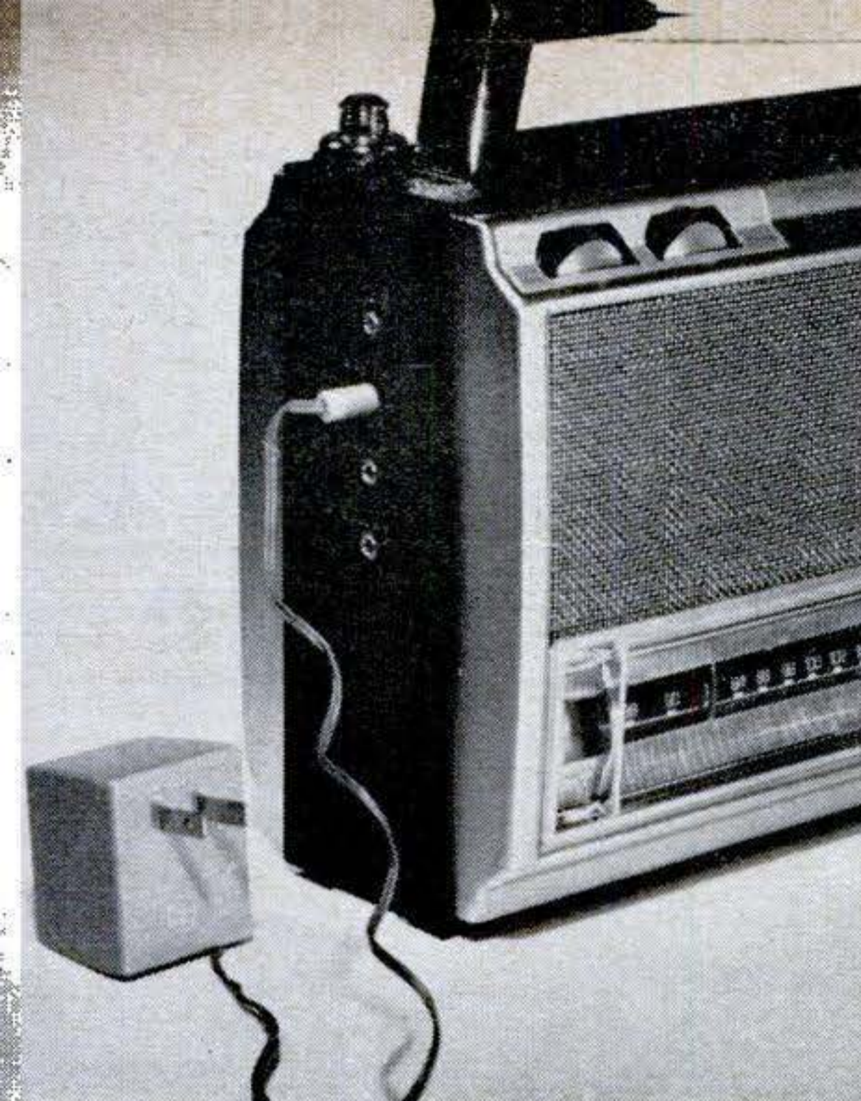
Lafayette Globepacer uses an outboard AC adapter that plugs into a side-mounted power jack. The adapter's output plug is a special shape so that it won't fit into an earphone jack by mistake.
