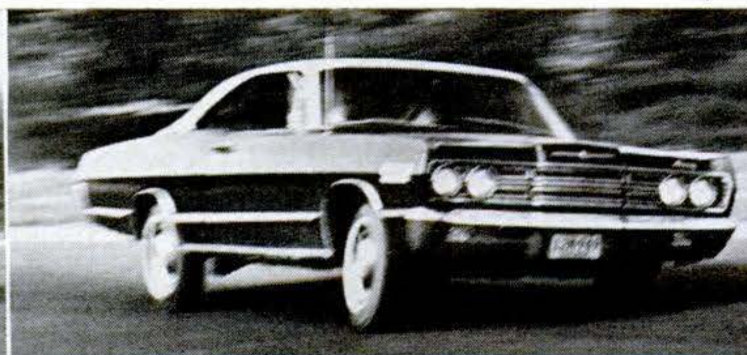
Mercury's understeer built up steadily on same turn. The maximum side force was 0.77 g.
