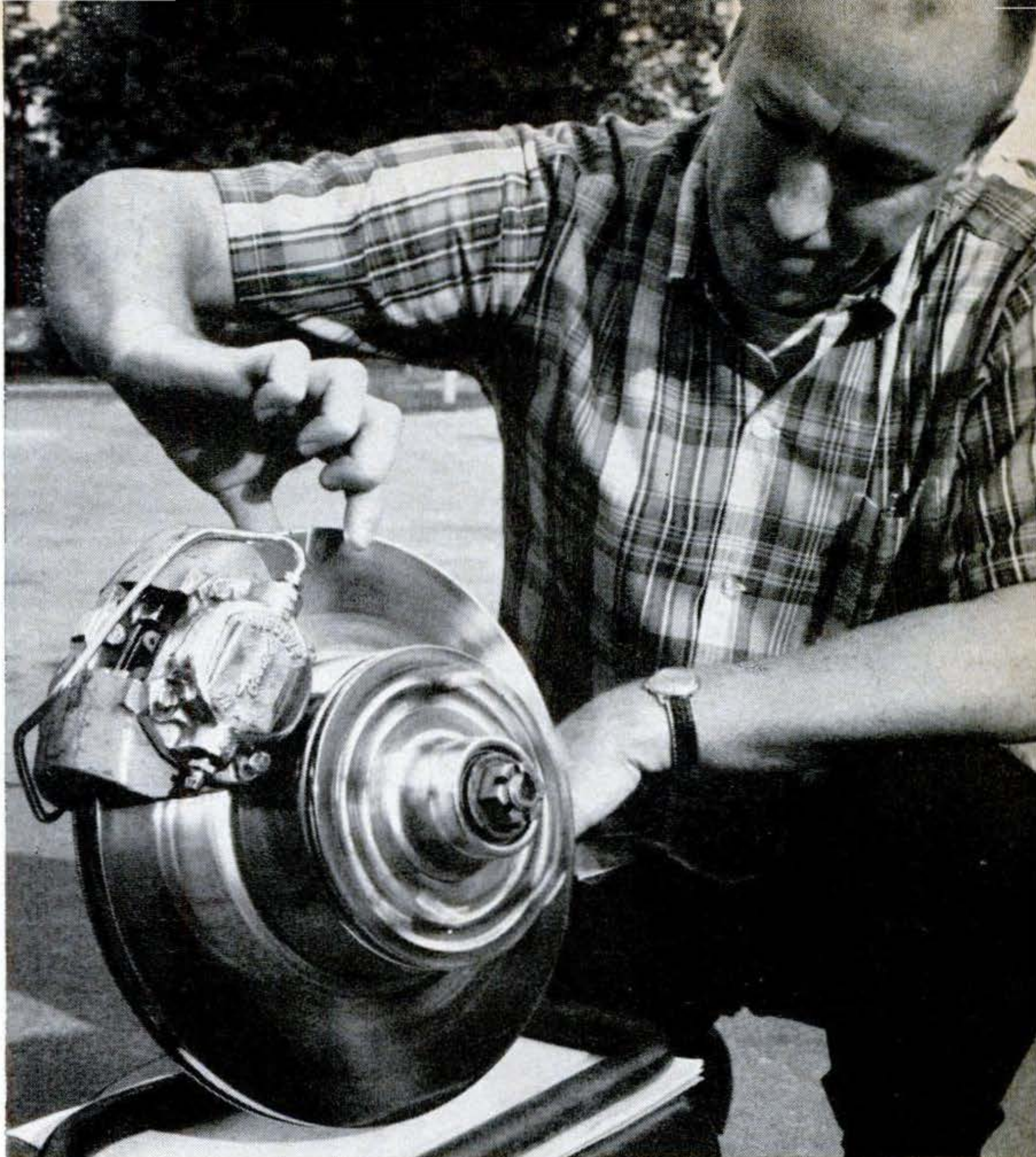
Disk-brake calipers act like a pair of powerful fingers squeezing the disk from both sides to stop it—and the car—when pedal pressure is applied.
