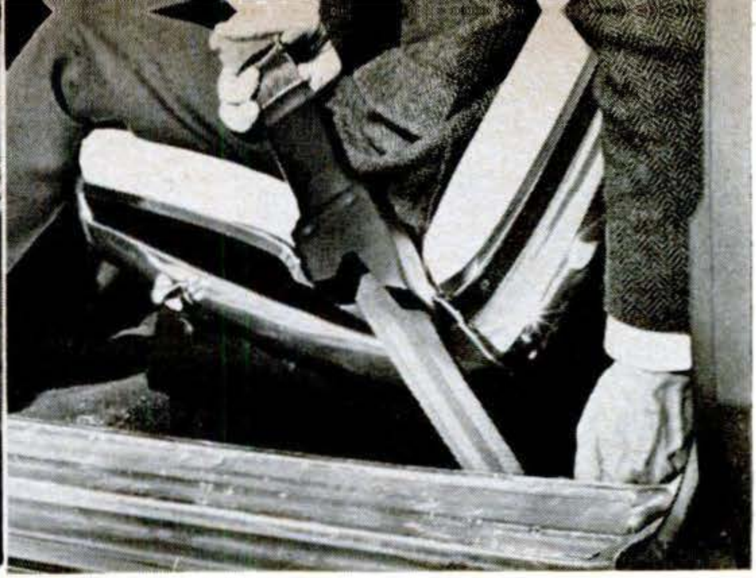
Floor-mounted sheath for seat belt on the Dodge was loose. Irritating—and it slowed buckling-up.
