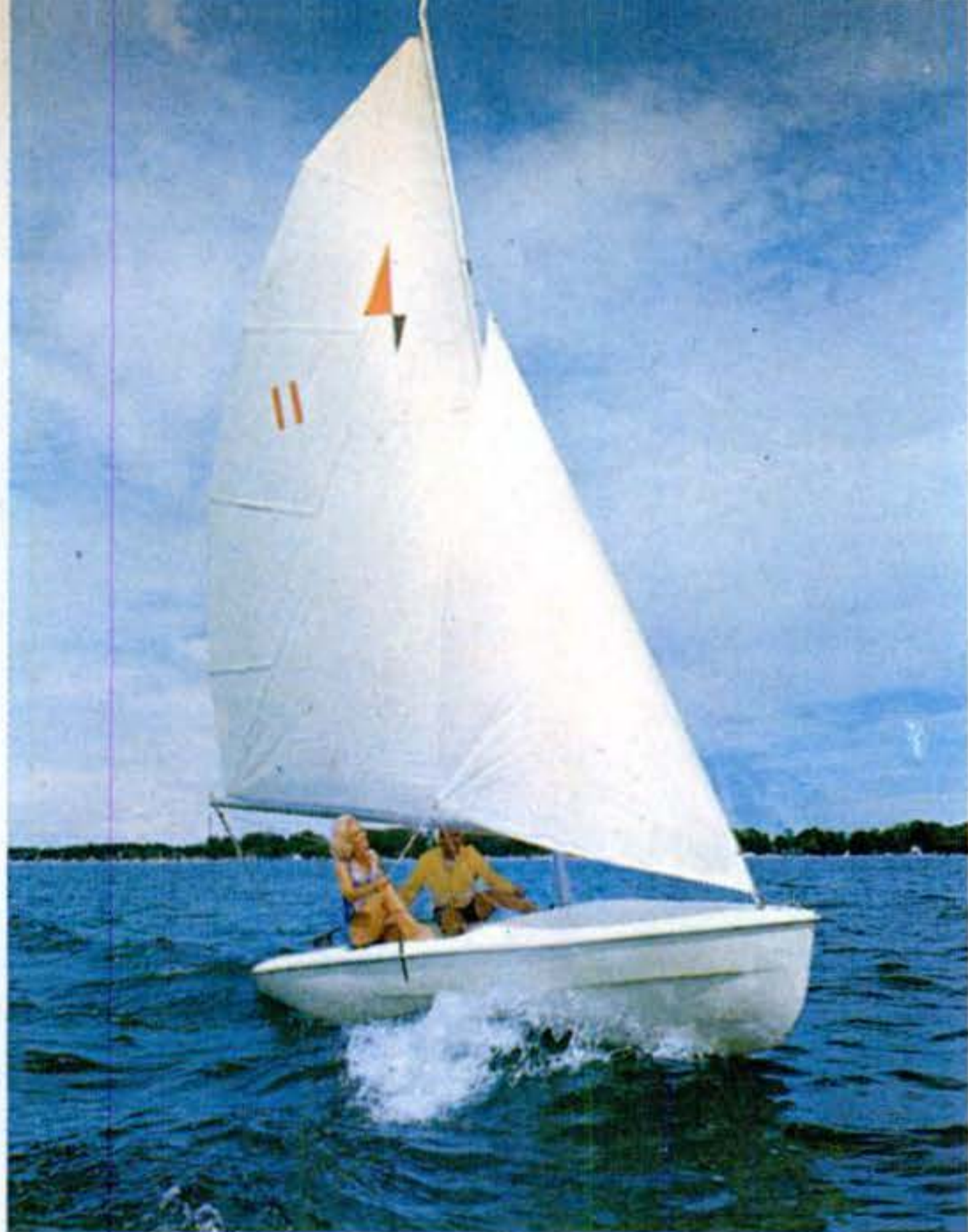
Starcraft's 16-foot Upstart claims a new feature: the ability to right herself from a swamped position without help from crew or centerboard.
