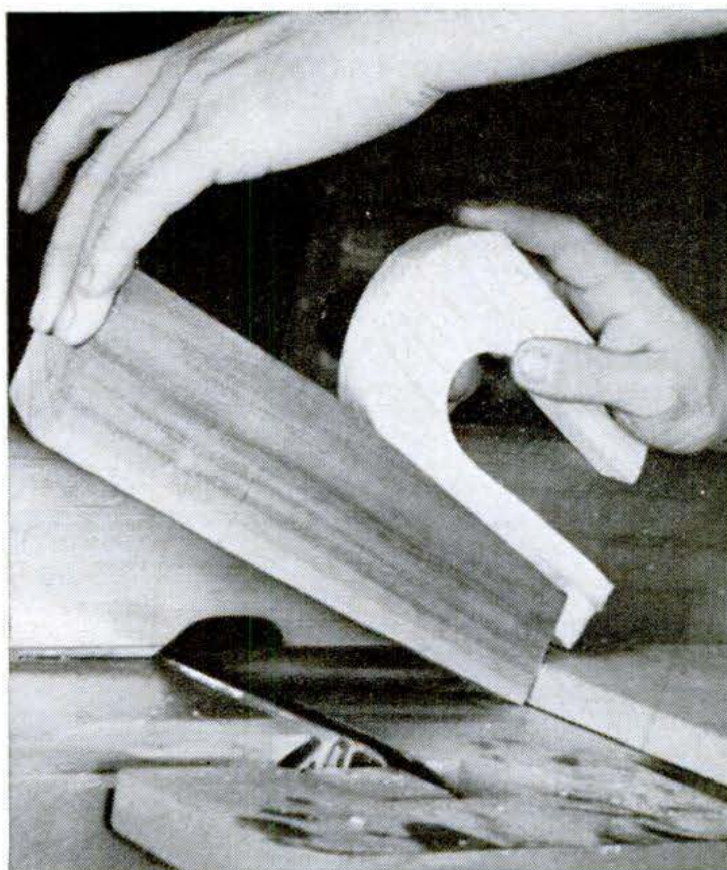
Clamp stop block to table to keep jointer from throwing the hull block back at you. Hold block as shown, lowering it on cutter and pushing with push stick. (Note: Jointer guard should be in place.)
