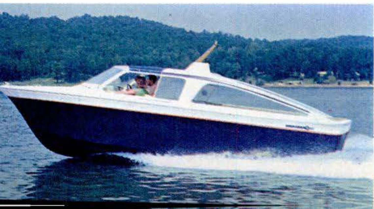
Jet-drive Bar Harbor by Buehler Turbocraft is 24 feet long. Fold-up top adds ventilation. Hull is a deep V. Three-stage jet drive, 290 to 325 hp.
