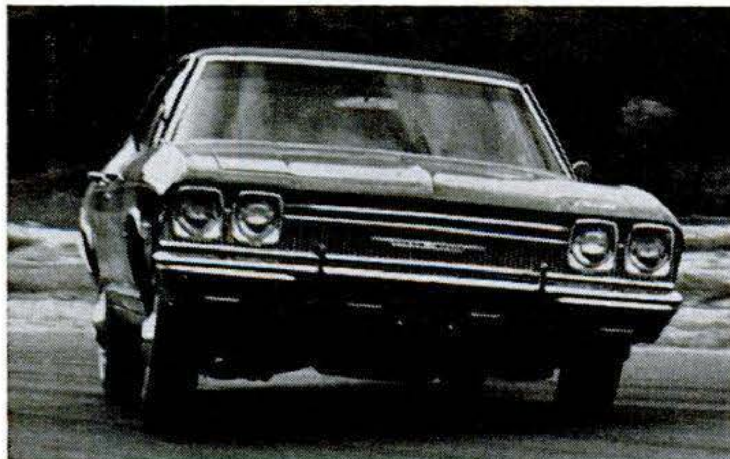
If you accelerate hard in the turn, rear-wheel slip angles will build up, and the car heads nicely for the next straightaway in complete balance.
