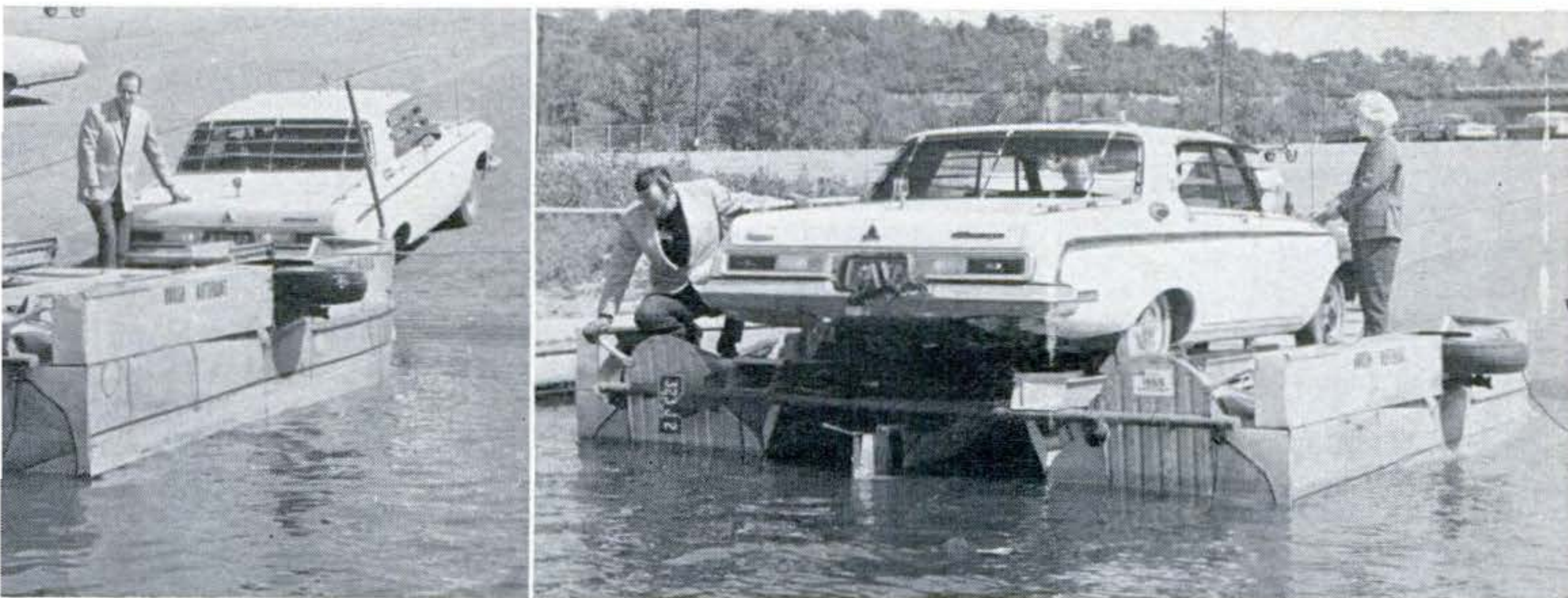
Then the boat is backed into water. A ramp permits the car to be backed onto deck over twin hulls.
