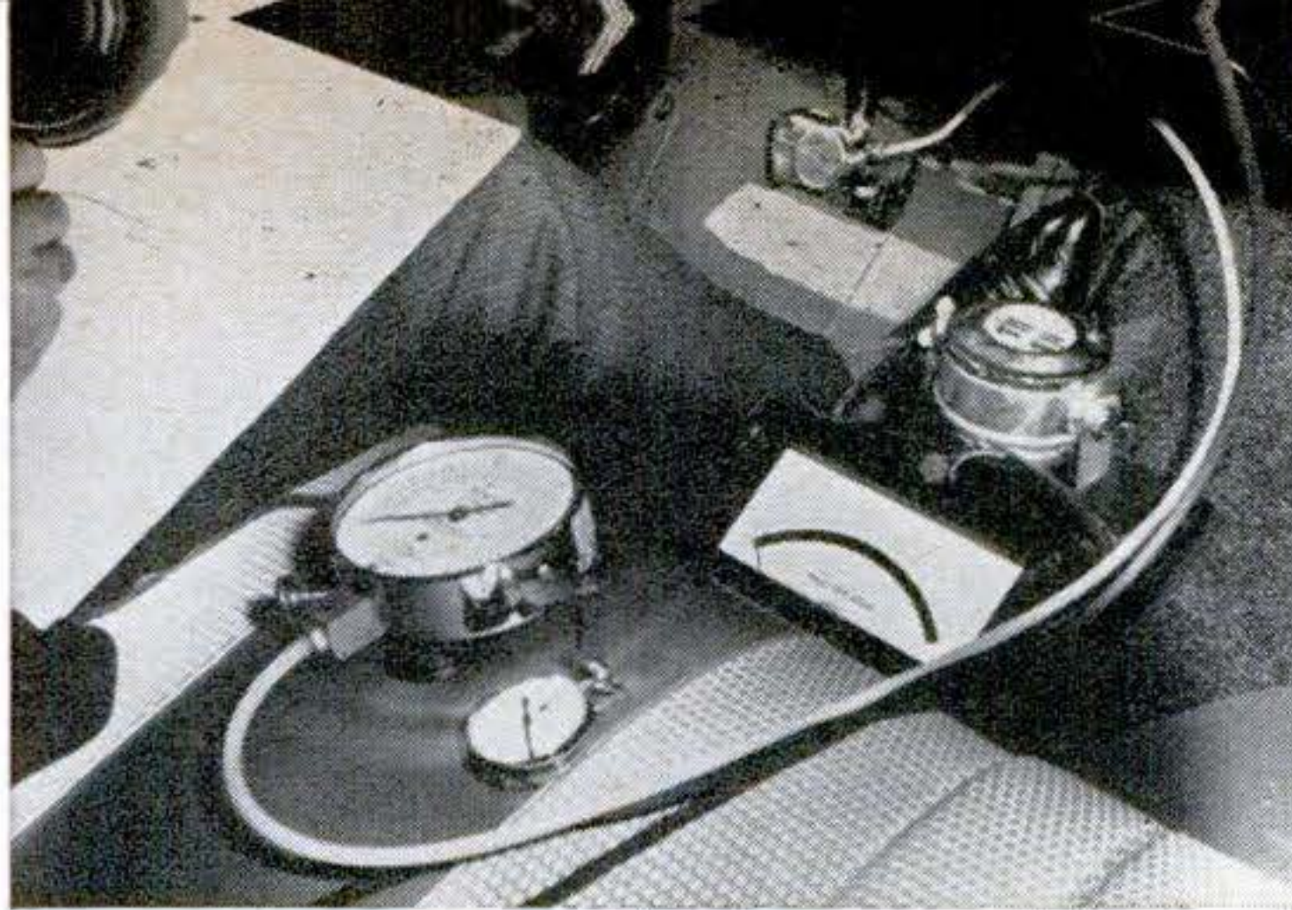
PS test equipment includes (from left): pressometer, stopwatch, fifth-wheel speedometer, Tapley meter, and pressometer sending unit (on brake pedal).
