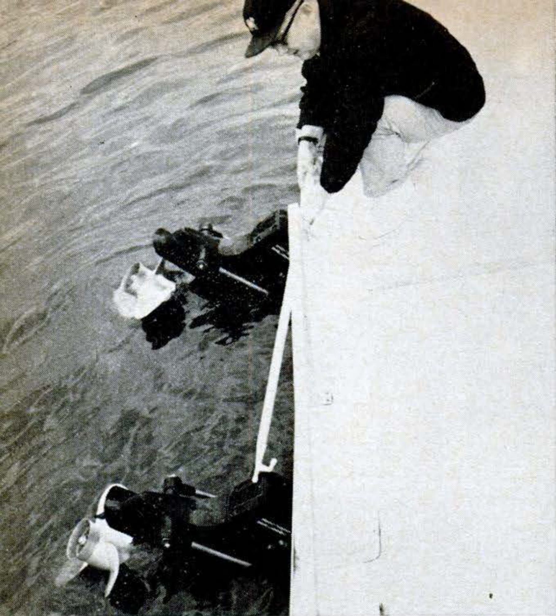
Twin stern-drive units are spaced far enough apart to give inboard maneuverability with one operating in forward, one in reverse. Power steering gives them fingertip control for "outboard" maneuverability.
