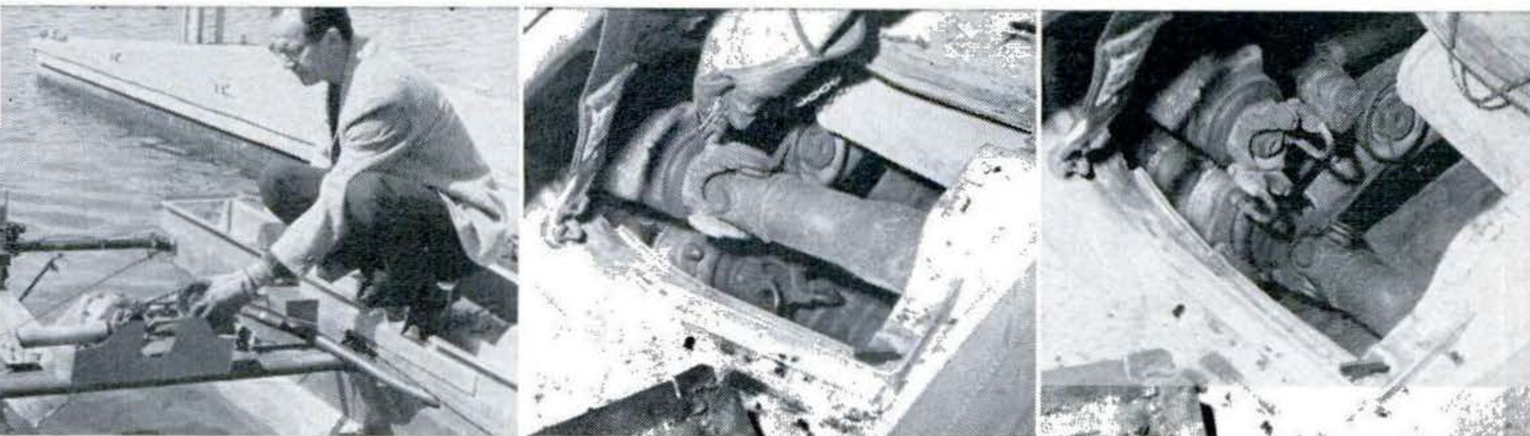
Brush checks the drive-shaft coupler (left), then loosens nuts holding
