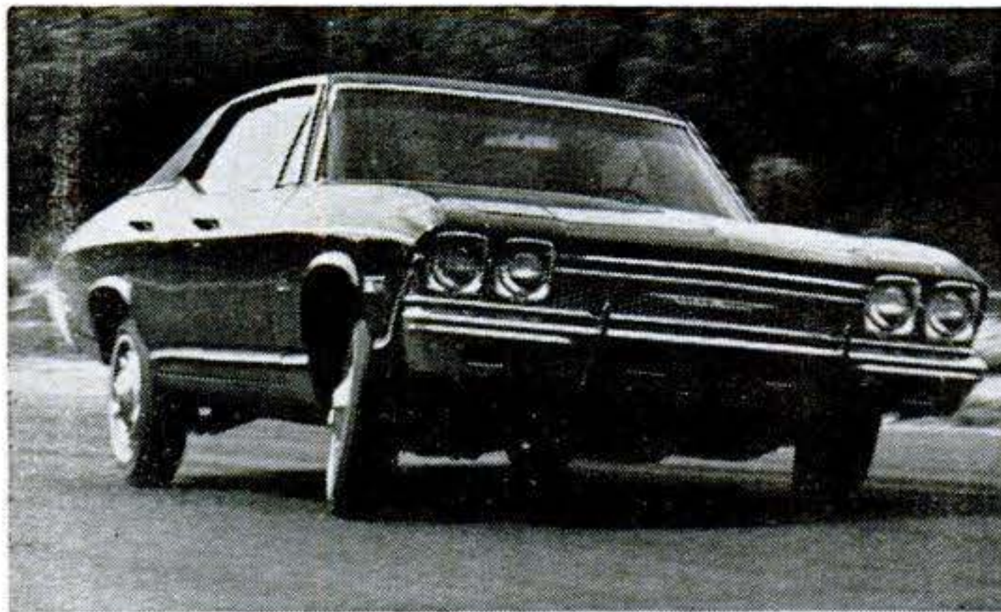
On a long, constant-radius turn the Chevelle is ideal. The car is stable and fully under control, with a marked initial understeer and some body roll.
