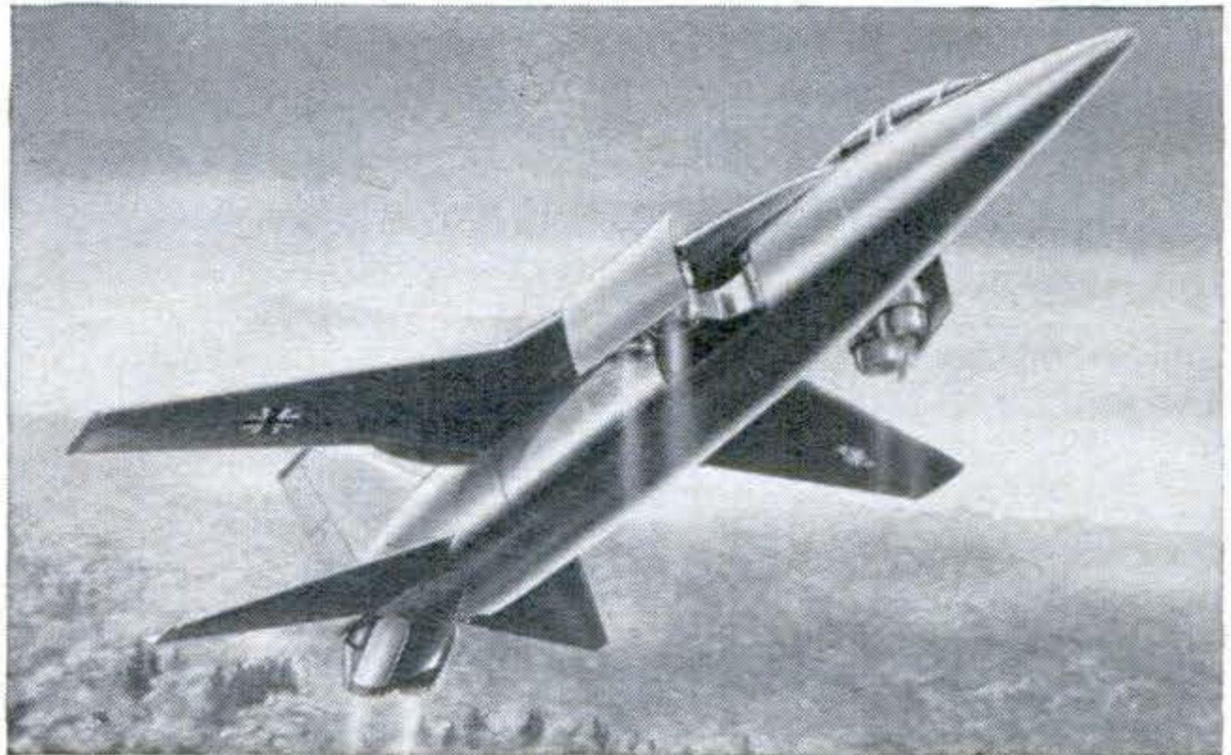
Extra engines disappear into fuselage when wings are swept back for high-speed flight.
