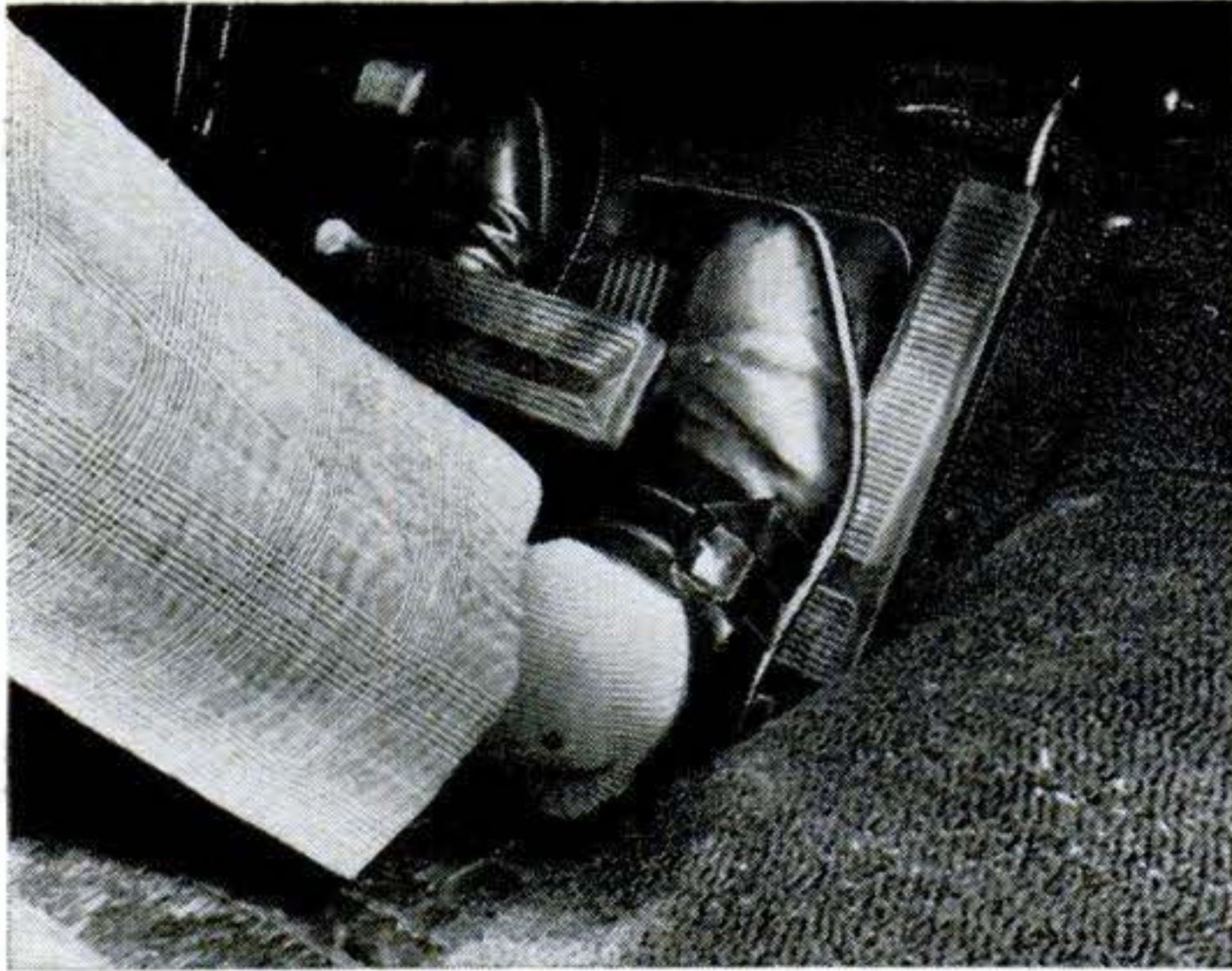
Brake pedal is mounted high off the floor. Toes can get caught when your foot swings over—or do all Rambler drivers use their left foot on the brake?
