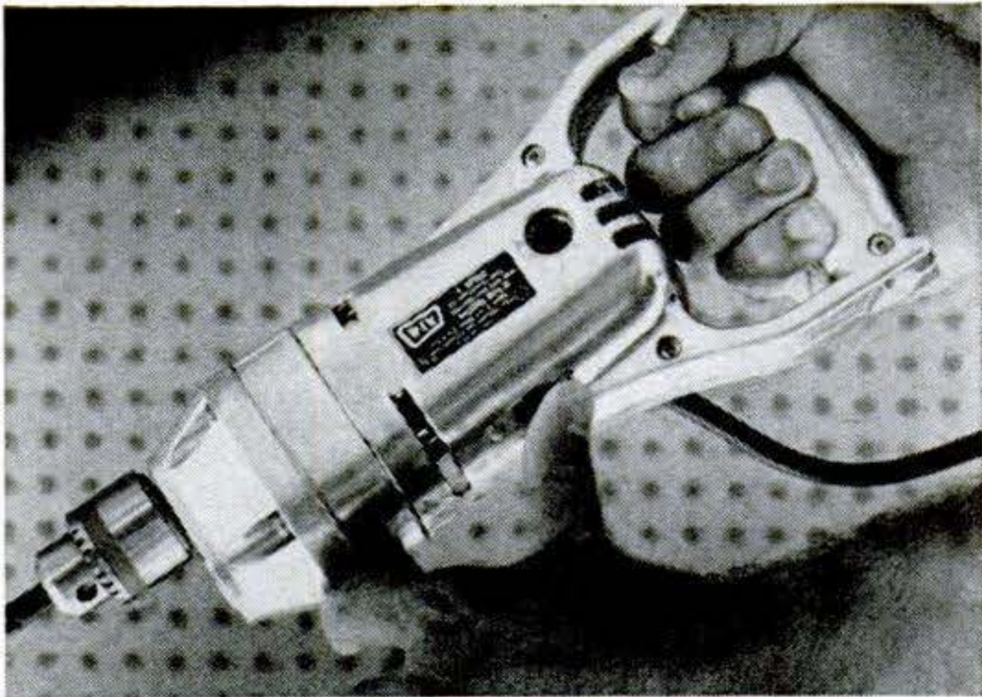
To change speed on Wen's model 808D, the chuck is inserted in one of two speed spindles. The side-mounted switch gives two speeds to each spindle.
