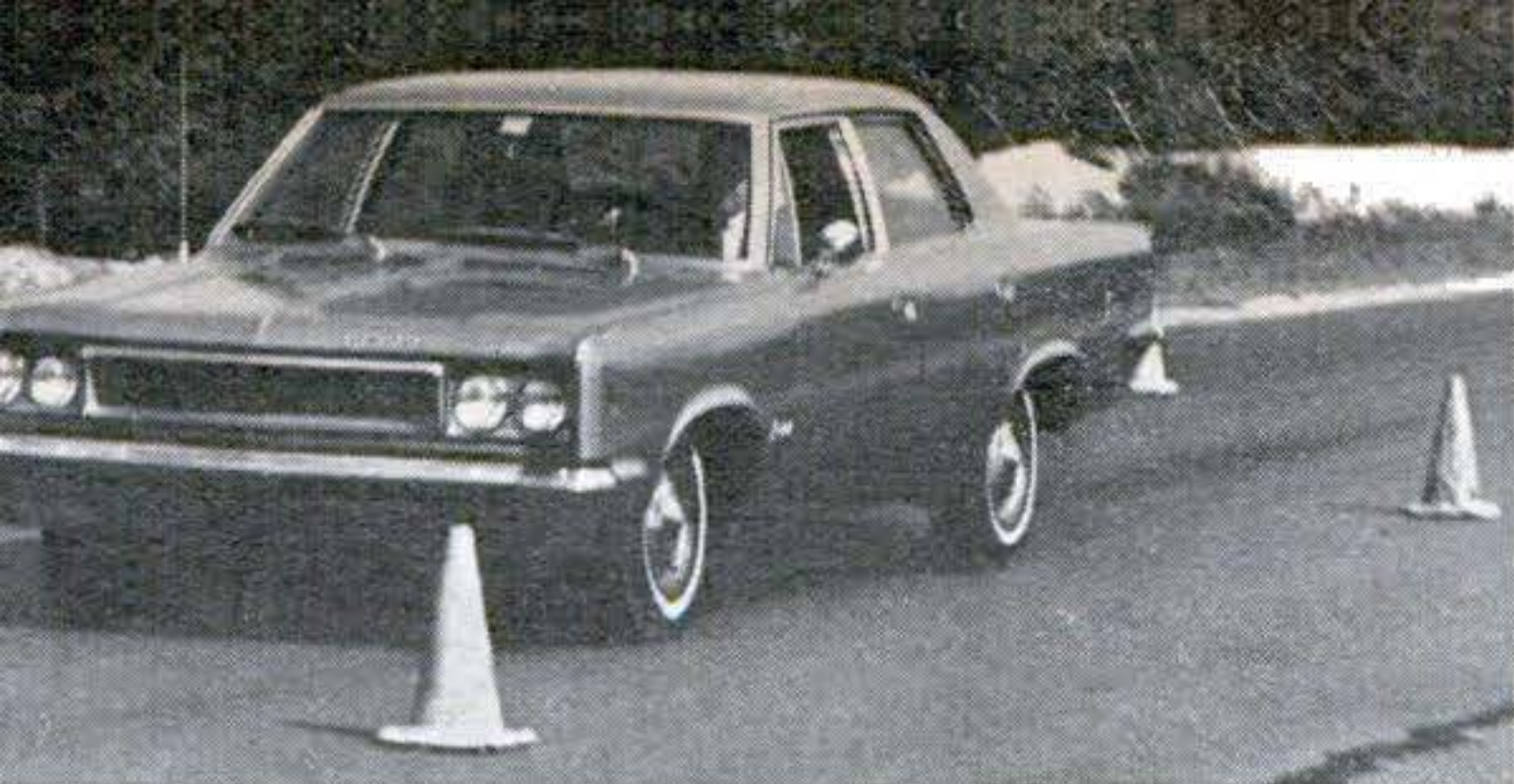
Ten half-g warm-up stops from 60 m.p.h. produced no fade, no increase in pedal pressure. With hot brakes, Rebel stopped in 144 feet from 60 m.p.h.
