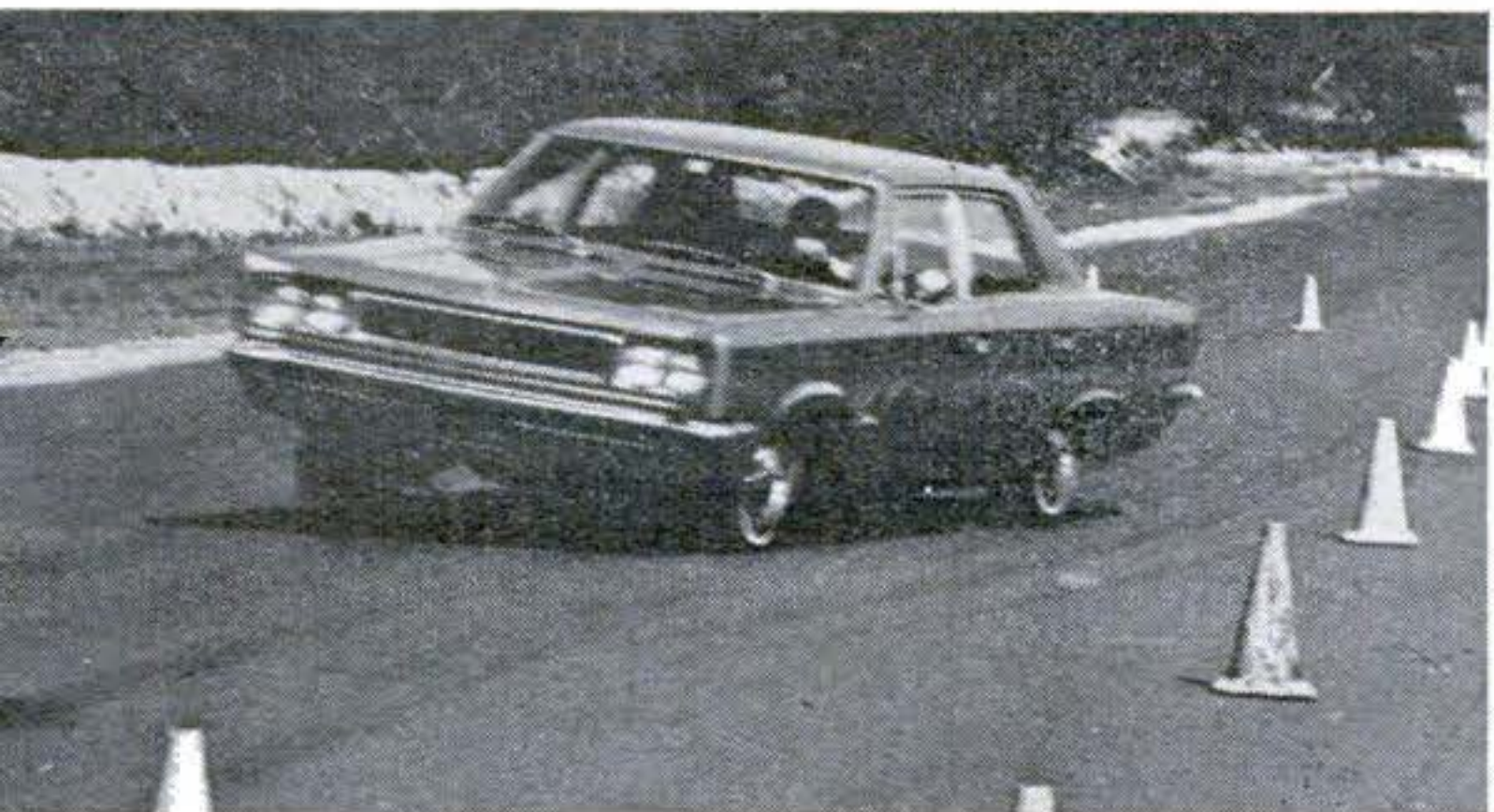
Two sudden lane changes within 180 feet at 60 m.p.h. were tried on Rambler several times. It didn't knock down a single marker of lanes and barriers.
