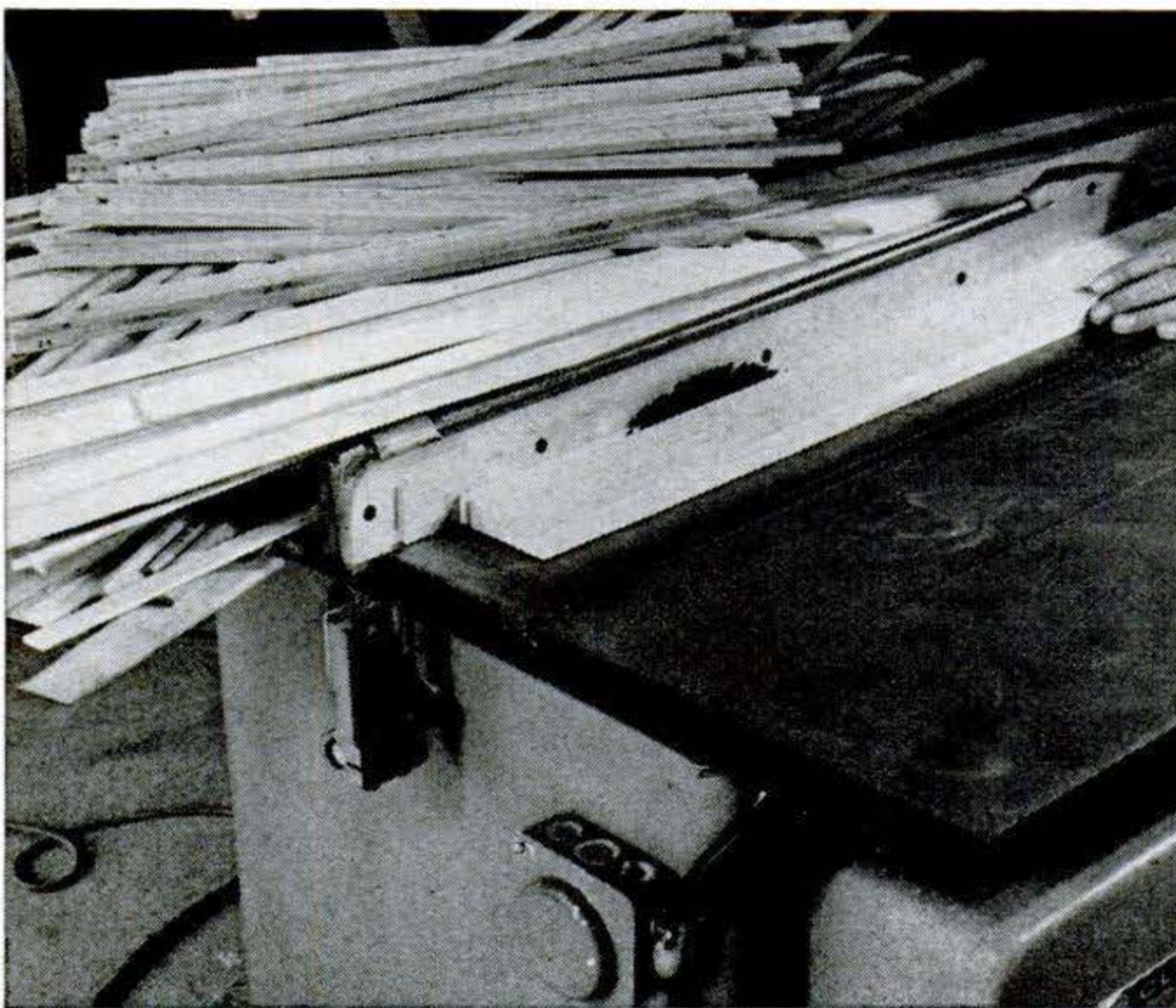
These tests involved ripping through about 1,100' of 2" construction-grade fir, \frac{3}{4} " hardboard-surfaced particle board, \frac{3}{4} " DF plywood, and redwood. Final
