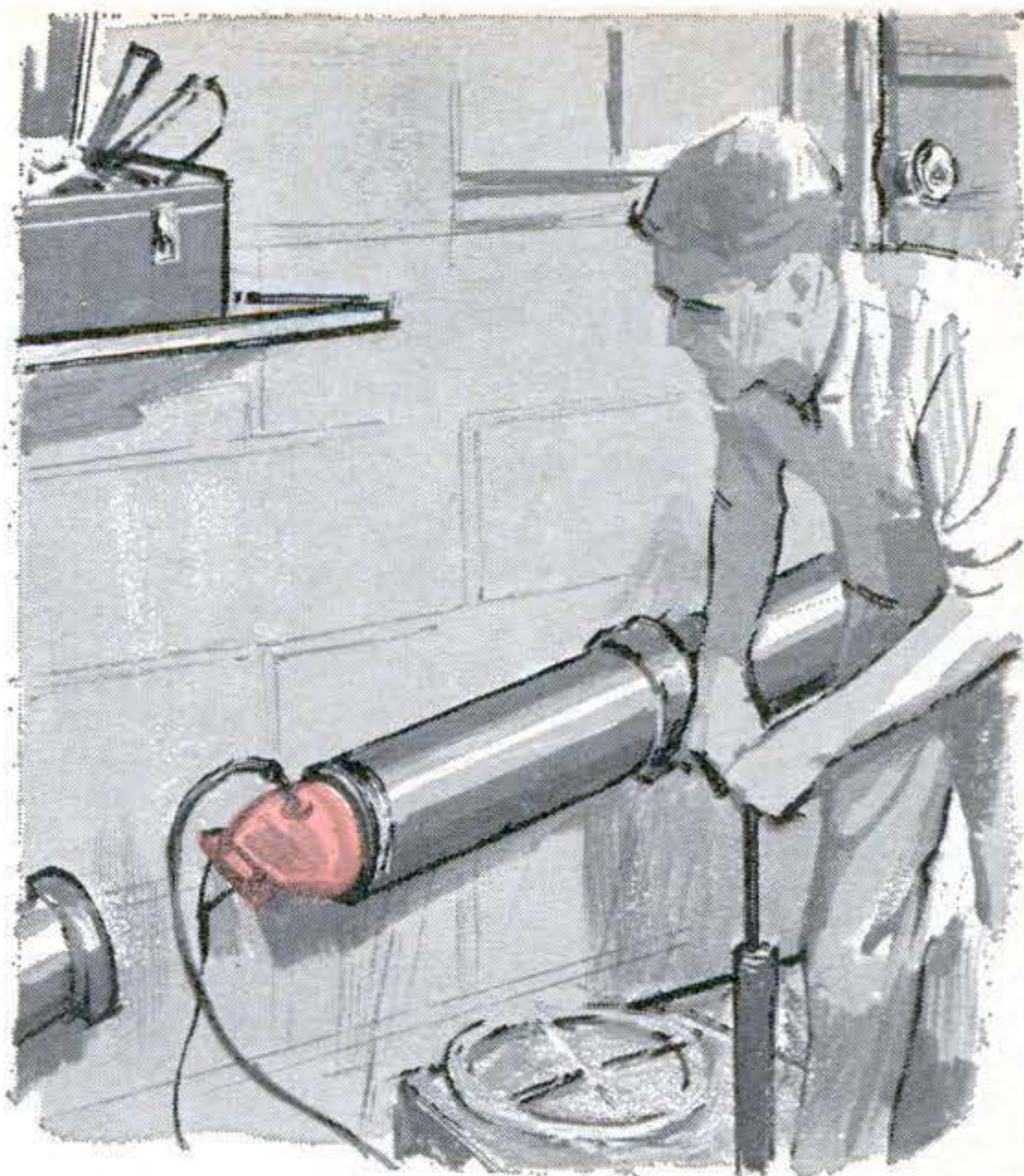
Pumped stopper seals pipe. This inflatable plug might make it easier to make repairs or check the flow in pipe lines. Instead of hammering in a wedge, you'd insert a plastic bladder and inflate it with a bicycle pump until the flow stopped. The plug would accommodate to roughness or irregularity in the pipe and, deflated, would slip out.
