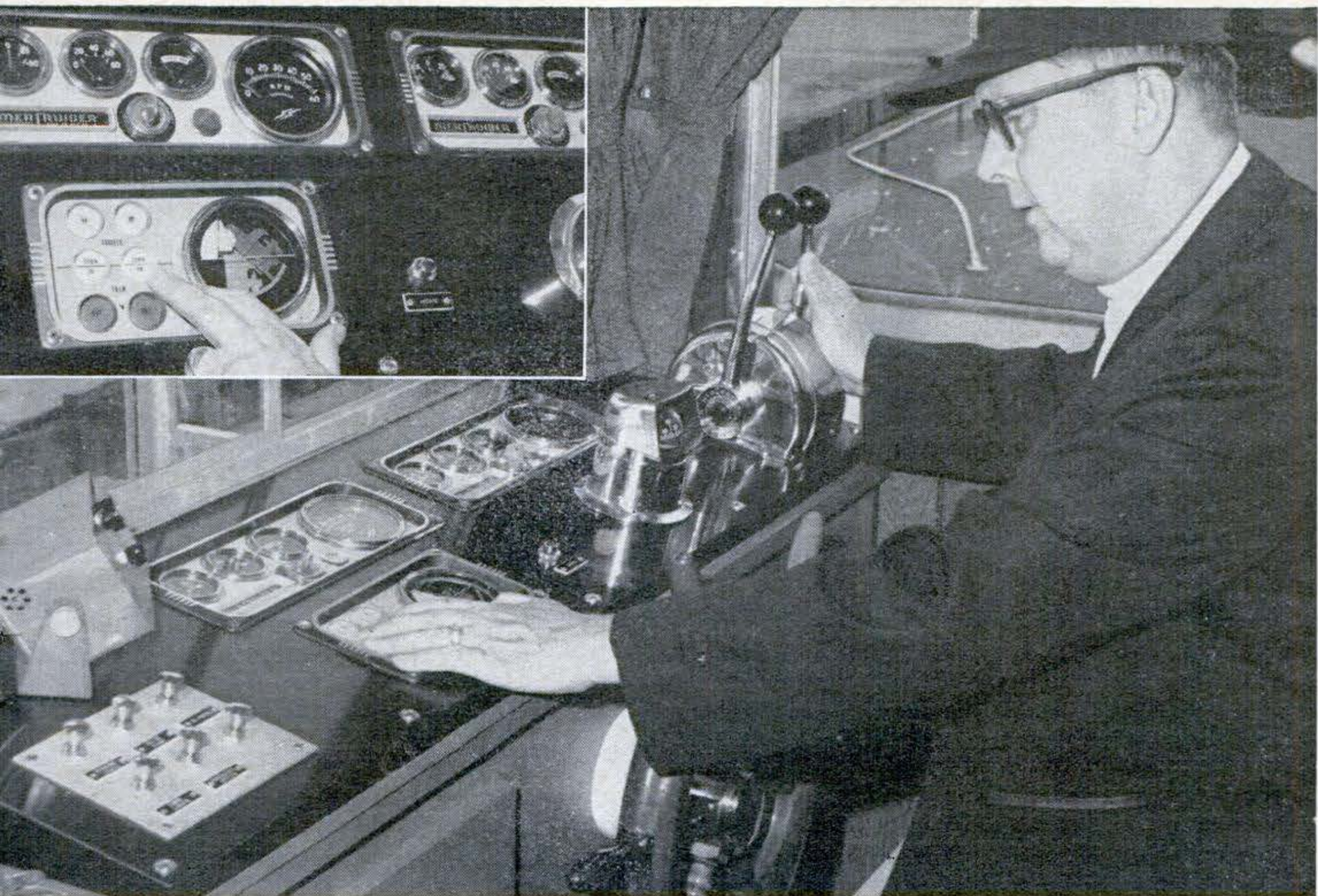
Morse single-lever controls actuate hydraulic marine transmissions, make shifting each 250-hp.
