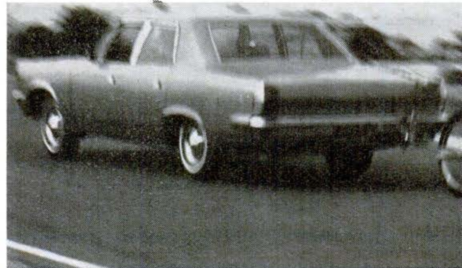
Rebel reached 60 in 11.2 seconds, 80 in 21 seconds. Speeding up from 25 to 70 took 11.2 seconds. At an indicated 60 m.p.h., true speed was 59 m.p.h.
