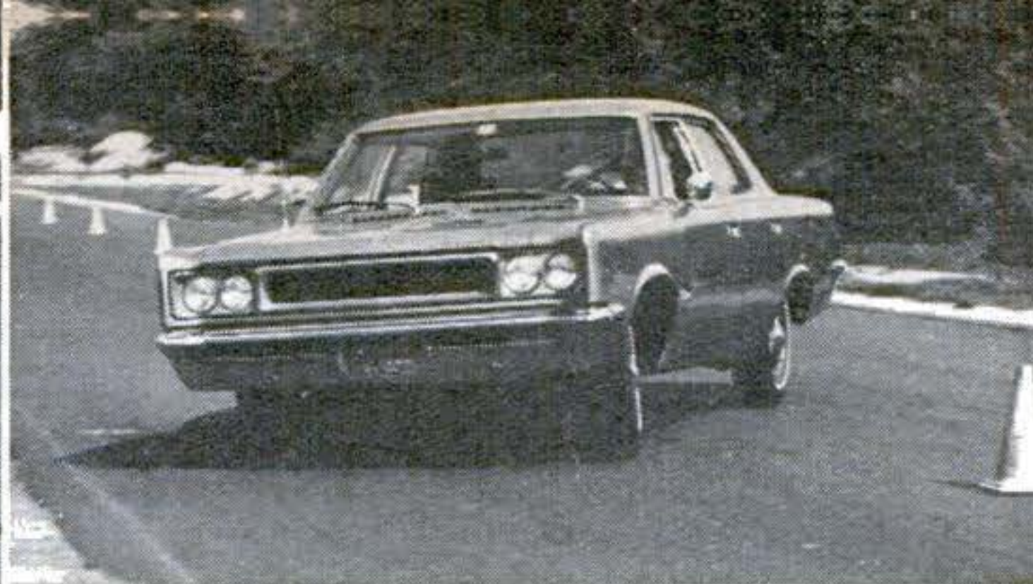
Slalom test between cones spaced at 40 feet gave 20-m.p.h. maximum speed. Faults: slow steering and beginning pump catch in the power assist.
