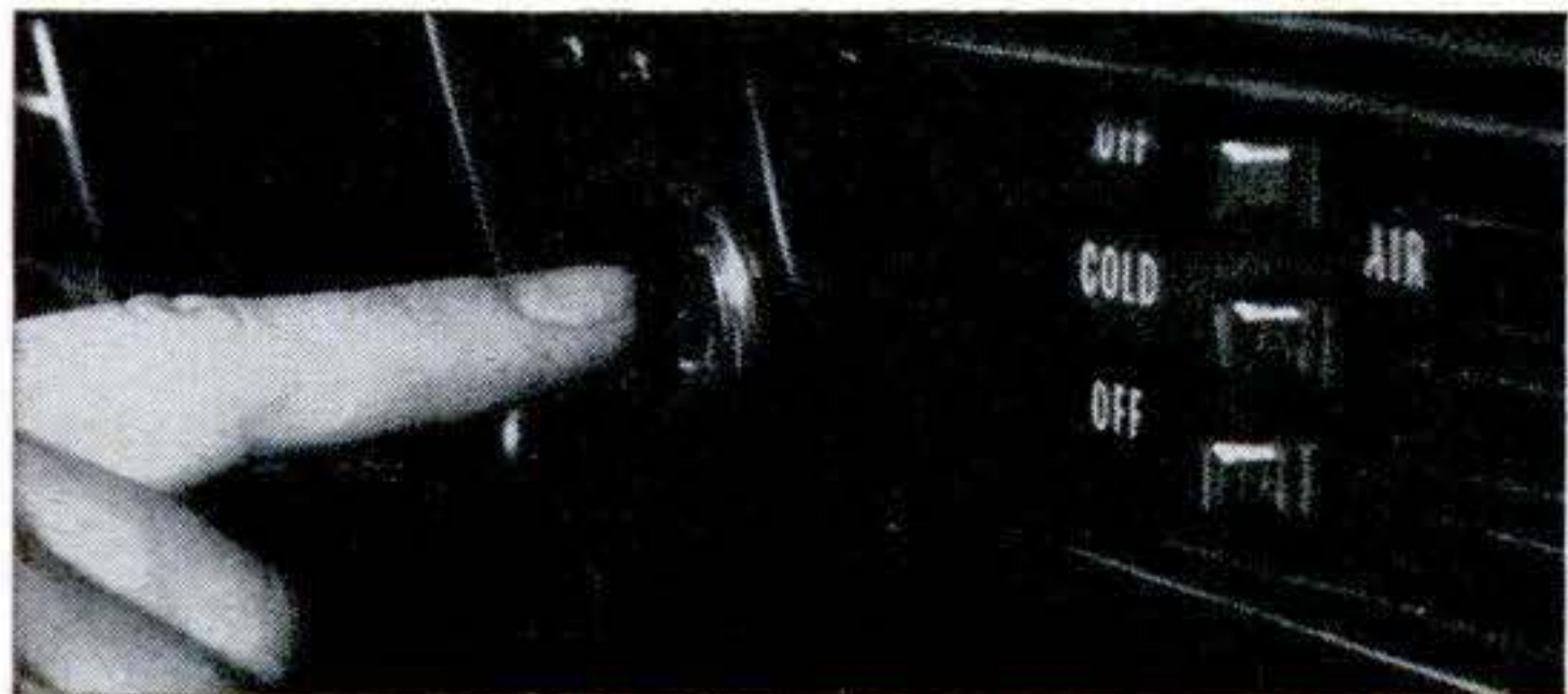
Recessed ignition lock is fine for safety but inconvenient for men with big fingers. The recess should be big enough to allow a good grip on the key.
