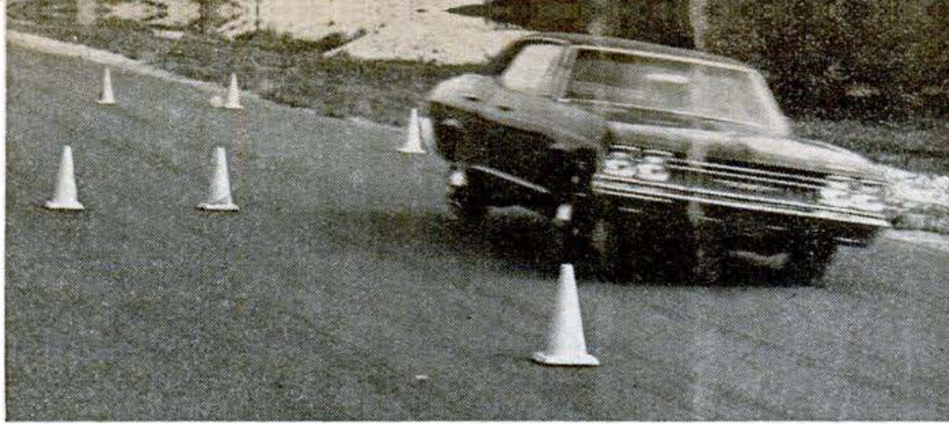
Sudden high-speed lane change is Chevelle's weak point. Up to 55 m.p.h. it's okay. At higher speeds, the steering response is slow.
