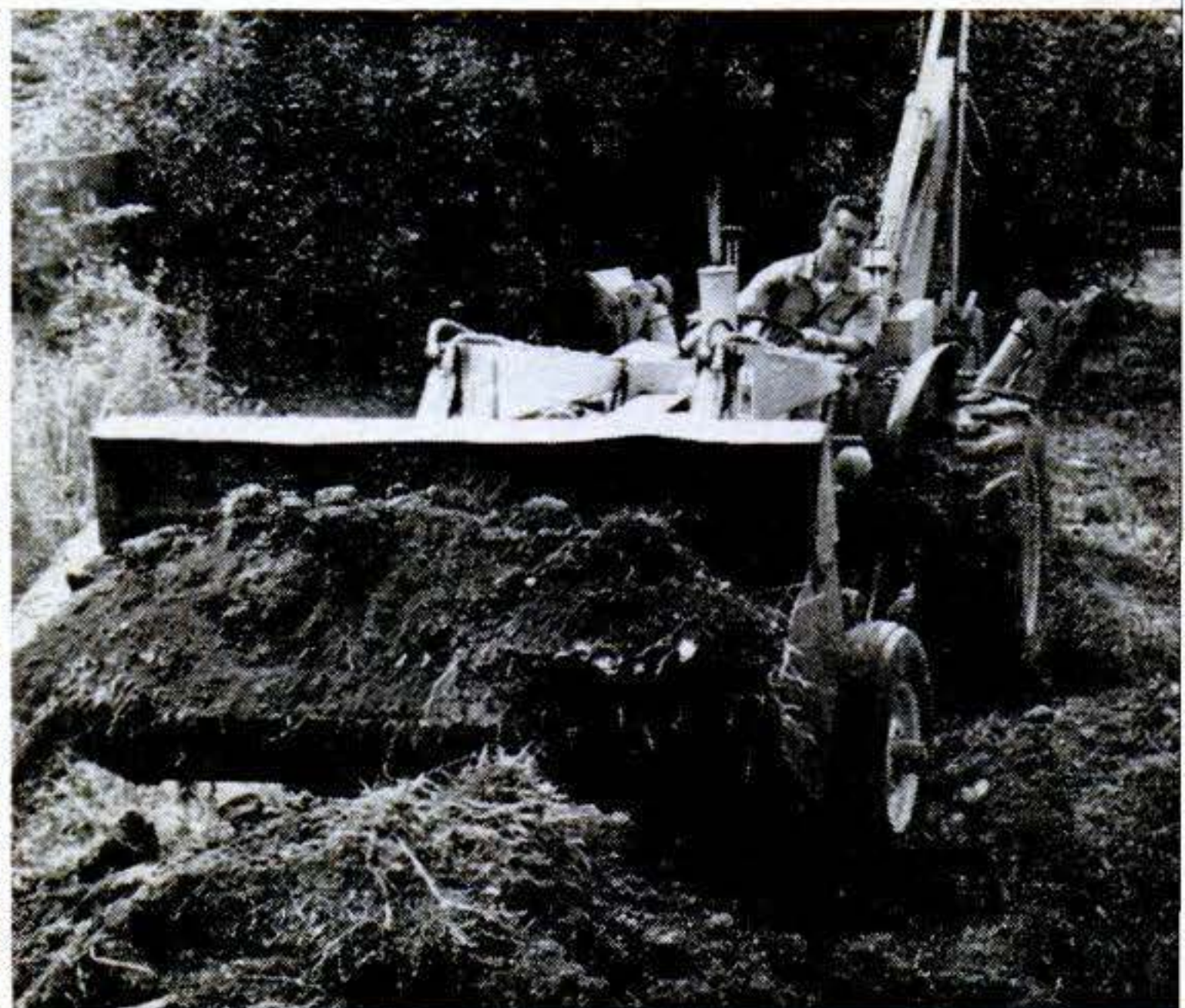
Backfilling and bulldozing are done with the boom bucket. You control the bucket with two levers while you drive the tractor. Power steering eases driving.
