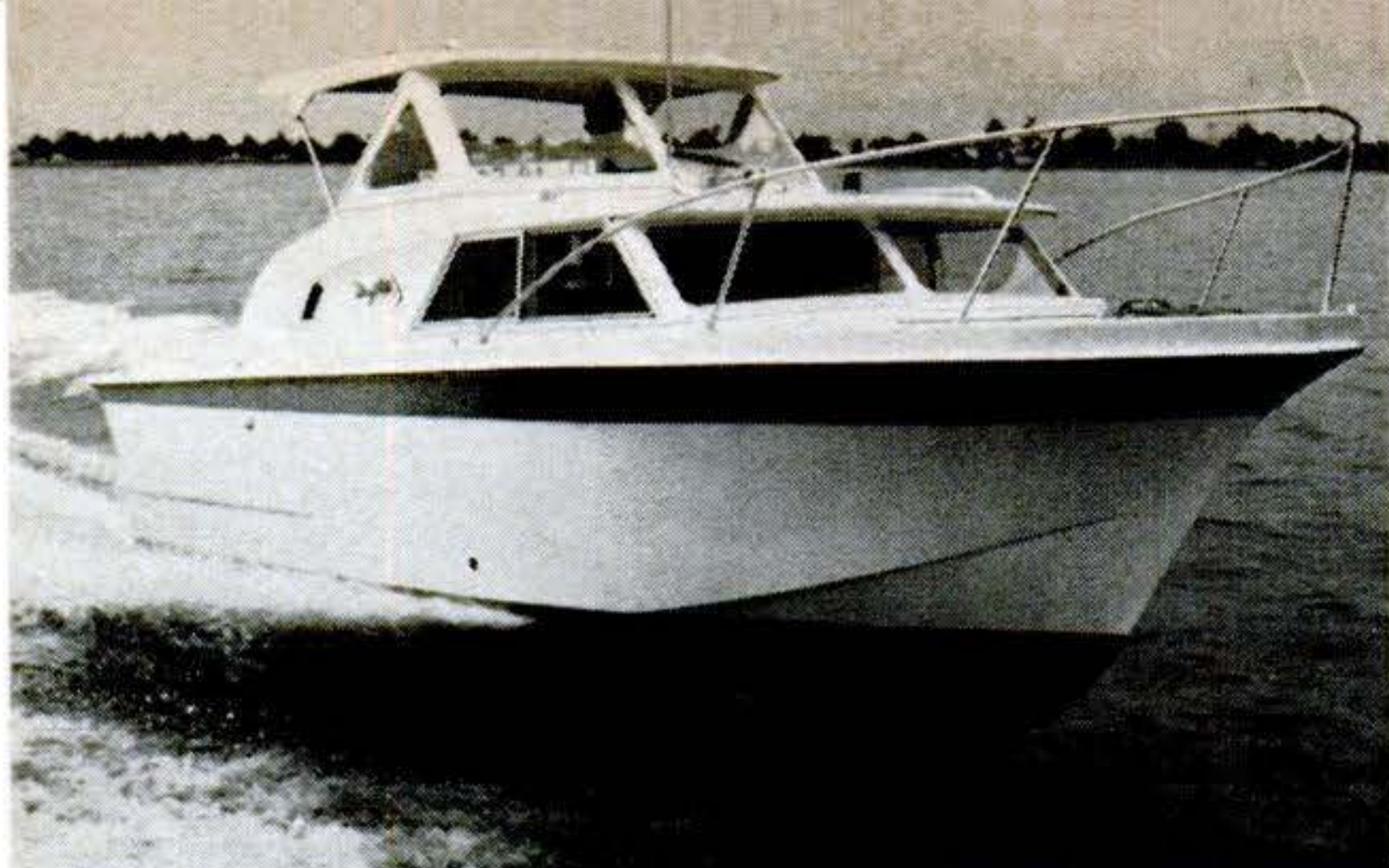
Uniflite fiberglass cruiser is a 23-footer. It's a heavy boat, but the 210-hp. inboard engine gave it plenty of acceleration and a high top speed. Power during the test proved smooth at all points, from low idle through maximum r.p.m.
