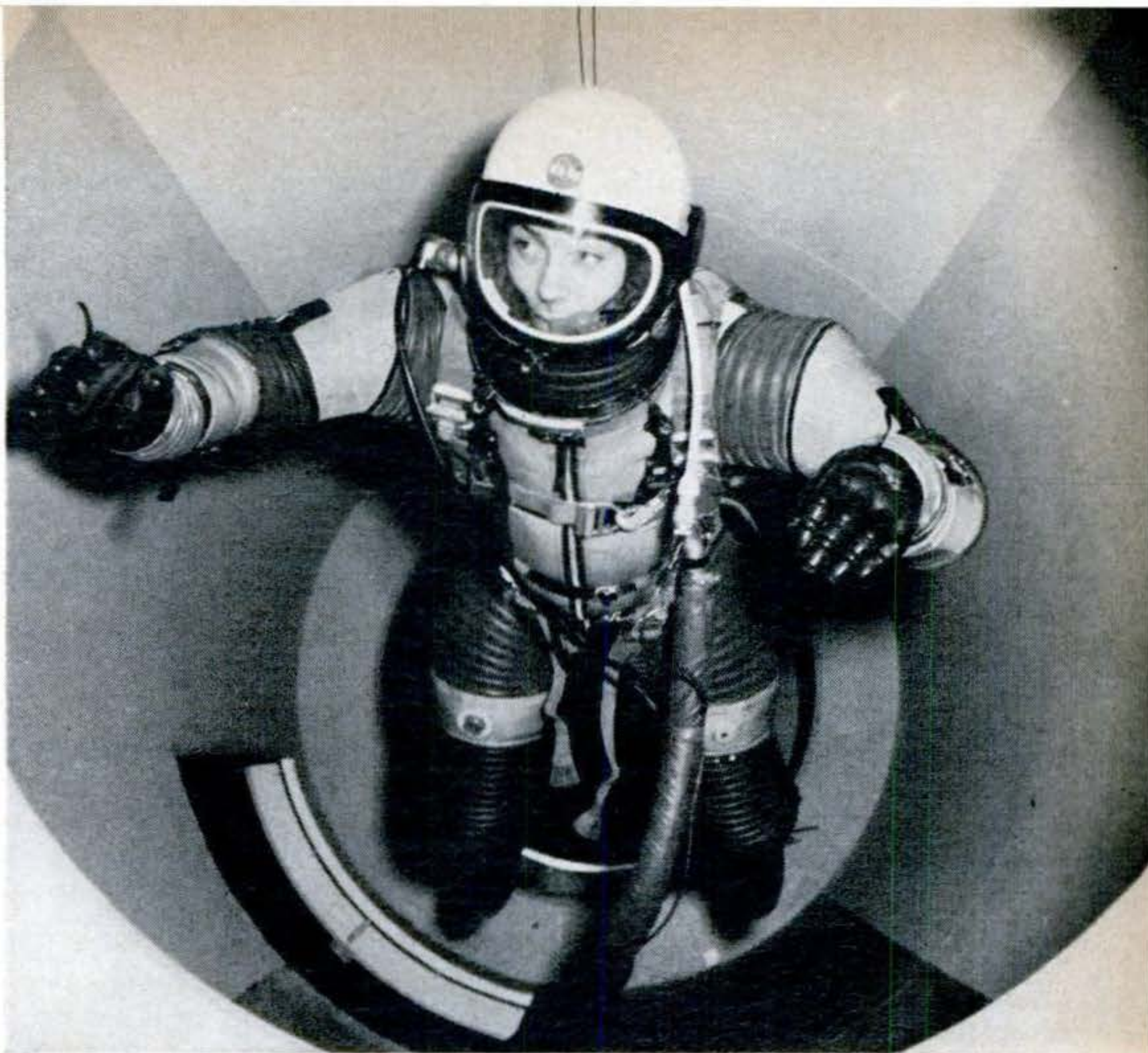
Engineer in spacesuit tries out mock-up of airlock for NASA's coming Orbital Workshop in a spent Saturn IV-B stage—one of our first spacecraft that will have a "two-gas" atmosphere. Astronauts on 30-day missions in the two-story laboratory will breathe a mixture of nitrogen and oxygen. But it will not eliminate fire hazard—since it will be under only one-third the pressure of natural air, and so must contain a much higher concentration of oxygen than air does.
