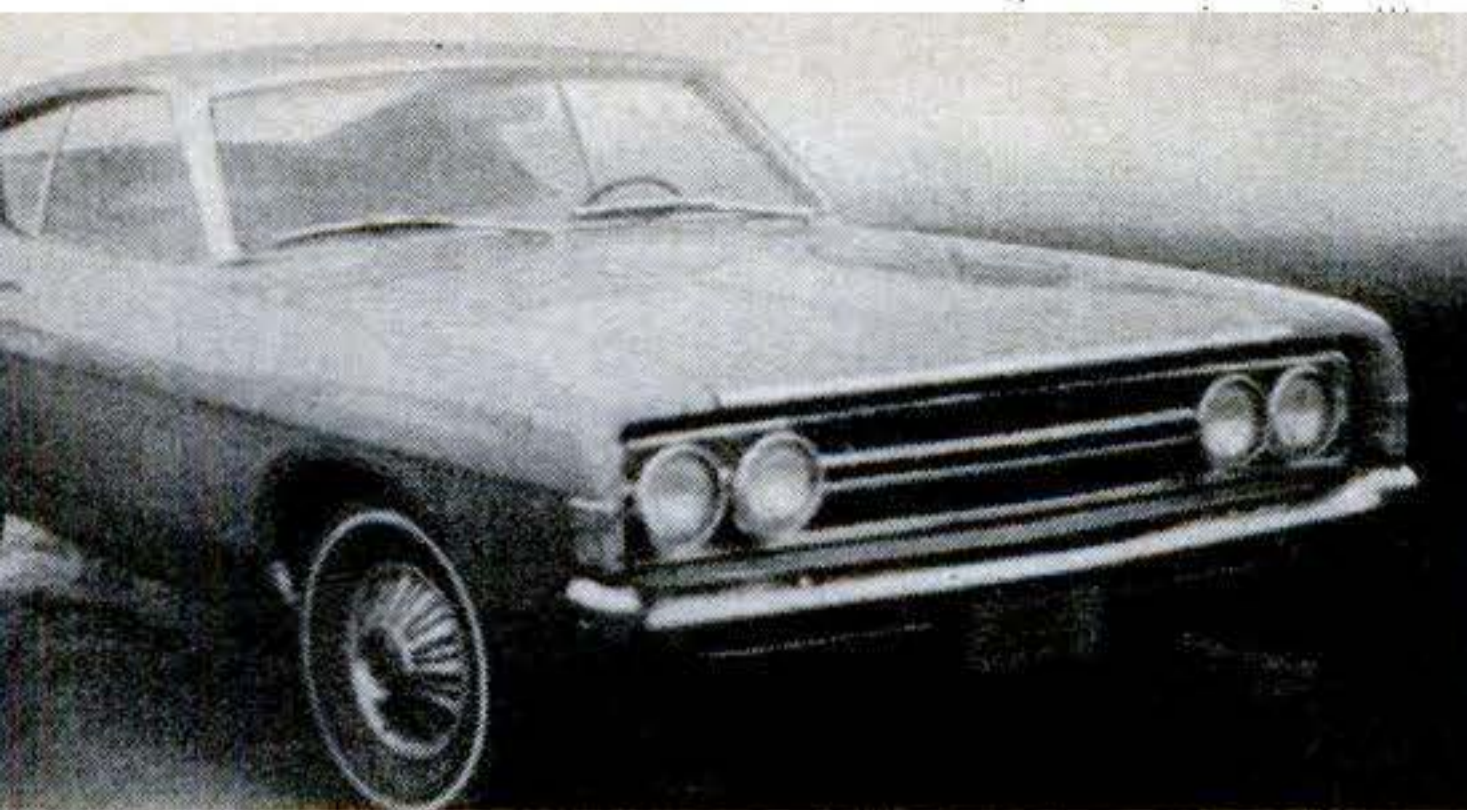
Fairlane front end has side-by-side headlights. Body structure is unit-construction again as in 1967.
