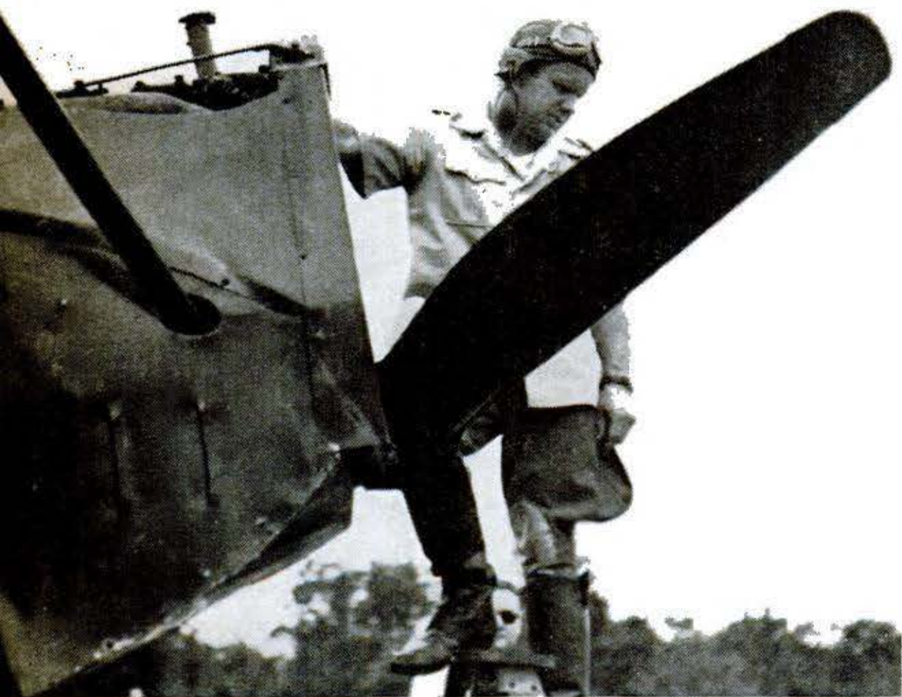
Pilot adjusts valve clearance and oils valve stems of 180-hp. Mercedes engine that powers this antique Fokker D-7. The engine is original. Simple and reliable, it can be kept in condition with no more than a screwdriver and an adjustable wrench.
