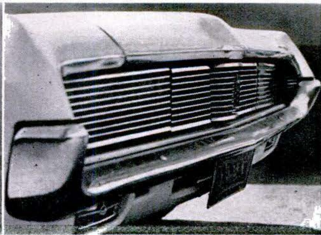
Cougar grille acquires big-car appearance with concealed dual headlights nearest the outer edges.
