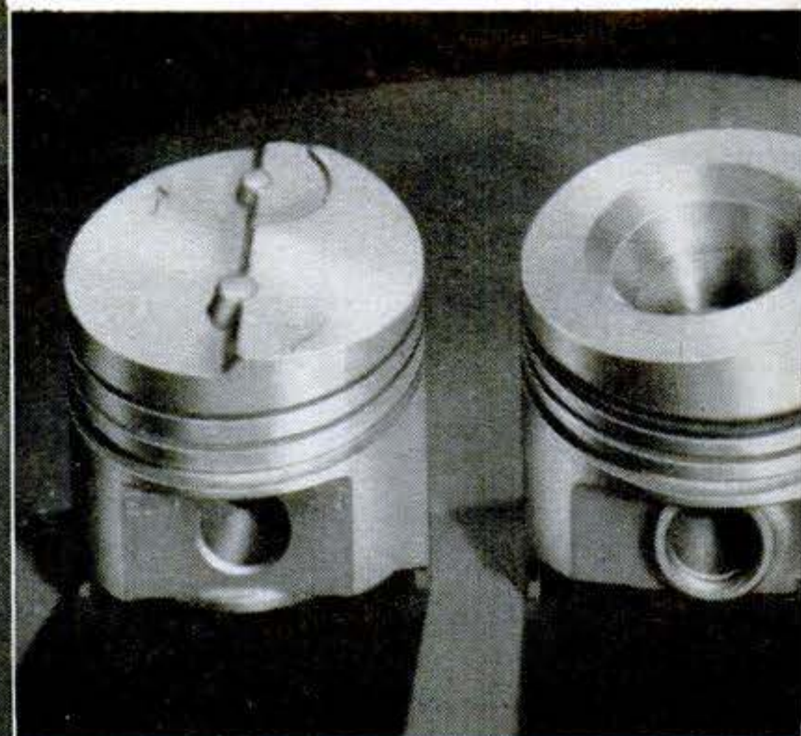
Piston at left is standard on pre-'66 430-cu-in. Lincoln engine with combustion chamber recessed in cylinder head. FCP-engine piston (right) contains combustion chamber, and allows a flush head.
