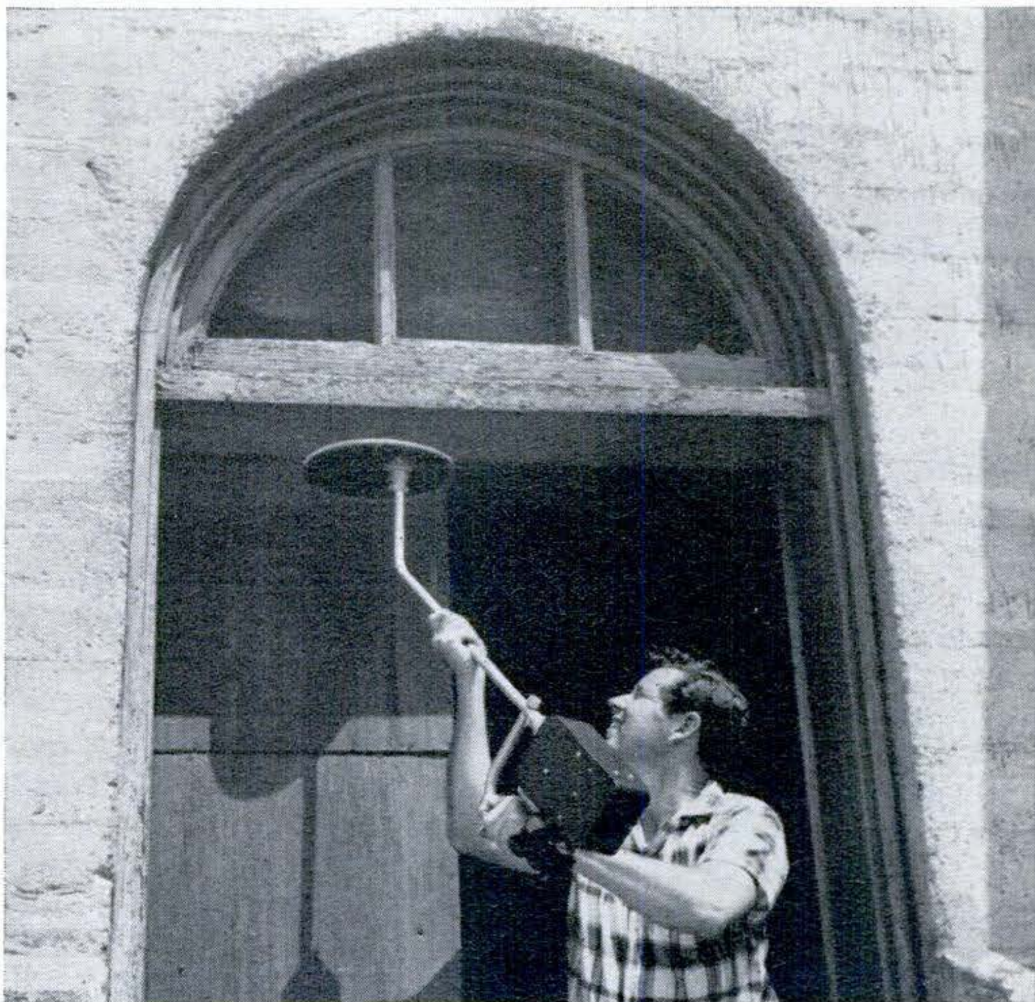
Old beams sometimes are hollow—so don't pass them up without a test. Look in particular for places that look as though the wood has been drilled out and a plug tapped back in and painted. That was a popular trick.
