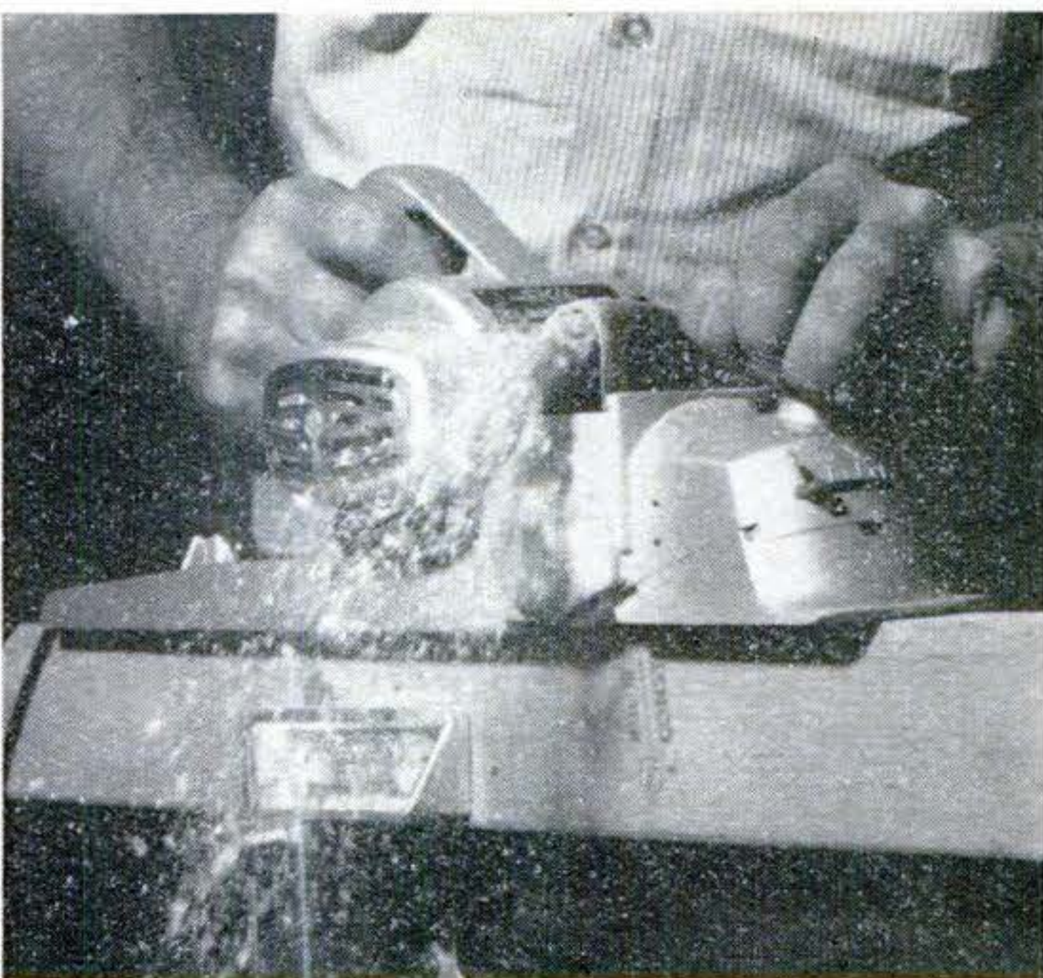
One of the big ones chews its way down a length of two-by-four—removing \frac{1}{8} " of stock as it goes. Adjustable chute directs sawdust away from operator.
