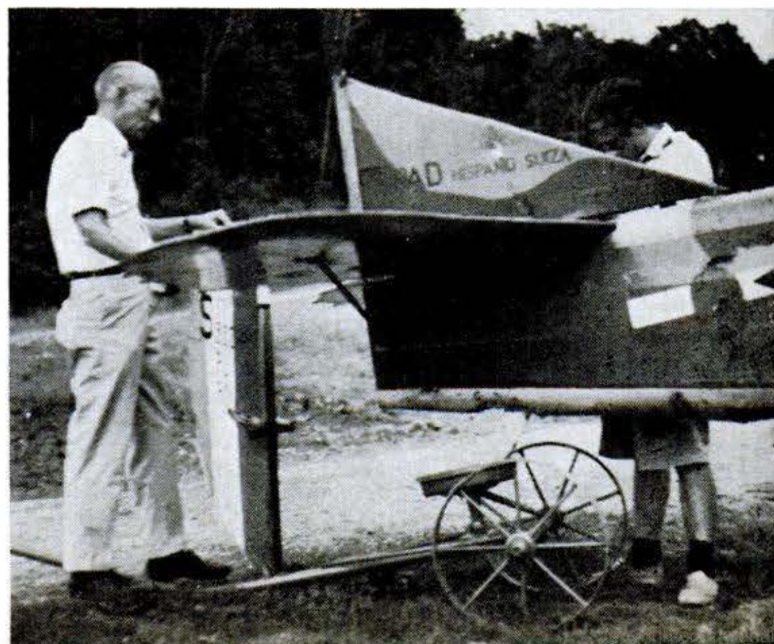
1910 Bleriot shows the state of the art prior to World War I. Although Louis Bleriot flew one like it across the English Channel in 1909, the antique shown seldom flies higher than 20 feet, or more than a mile or two. It's powered by a 25-hp. engine.
