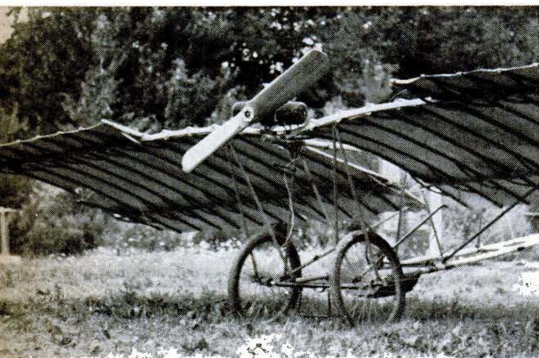
1910 Bleriot shows the state of the art prior to World War I. Although Louis Bleriot flew one like it across the English Channel in 1909, the antique shown seldom flies higher than 20 feet, or more than a mile or two. It's powered by a 25-hp. engine.
