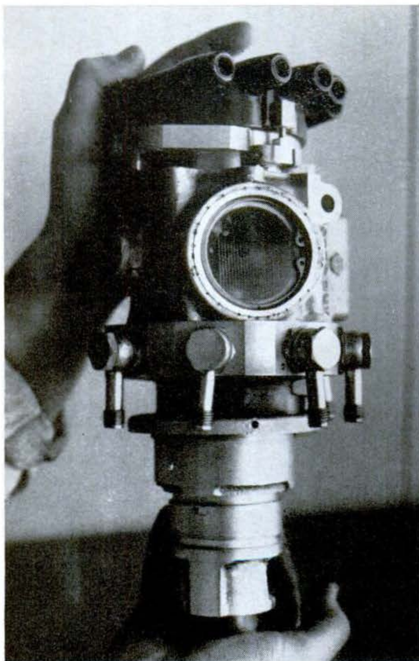
Injection pump is of relatively simple design with a separate plunger for each injector—operated by a swashplate—and a central metering shaft.
