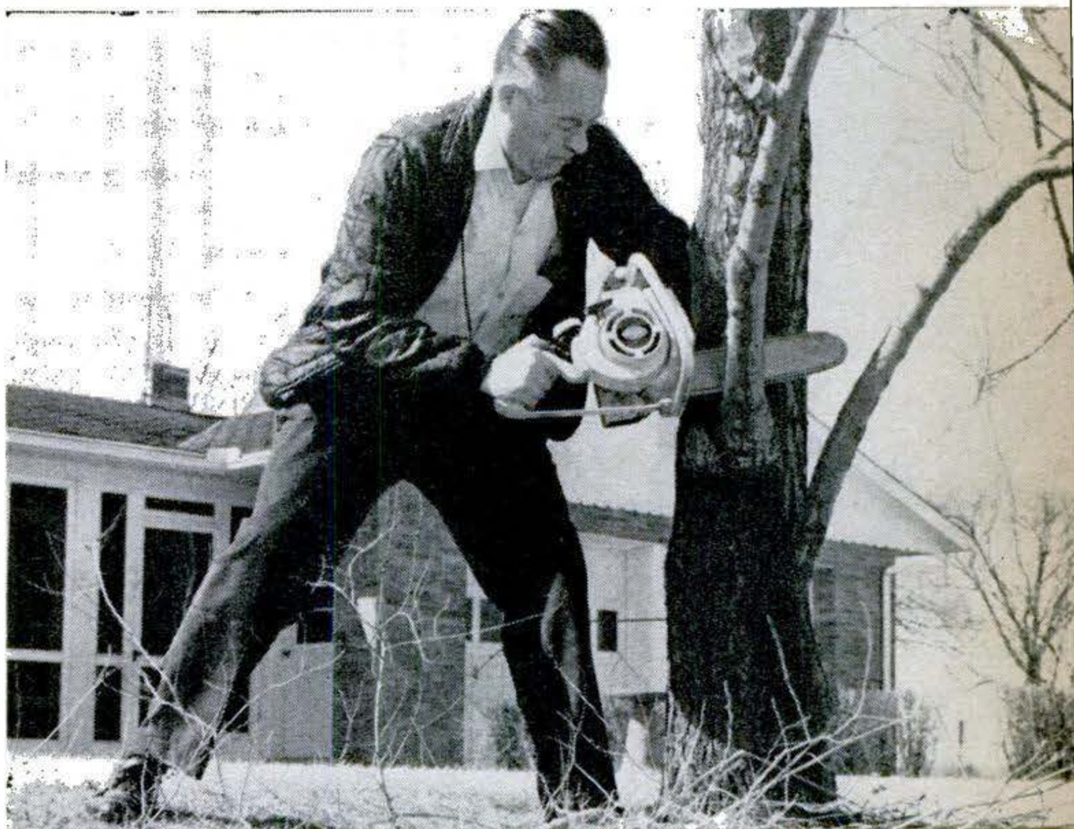
In typical trimming operation, lightweight chain saw cuts cleanly with little vibration. Chain oiling is automatic.
