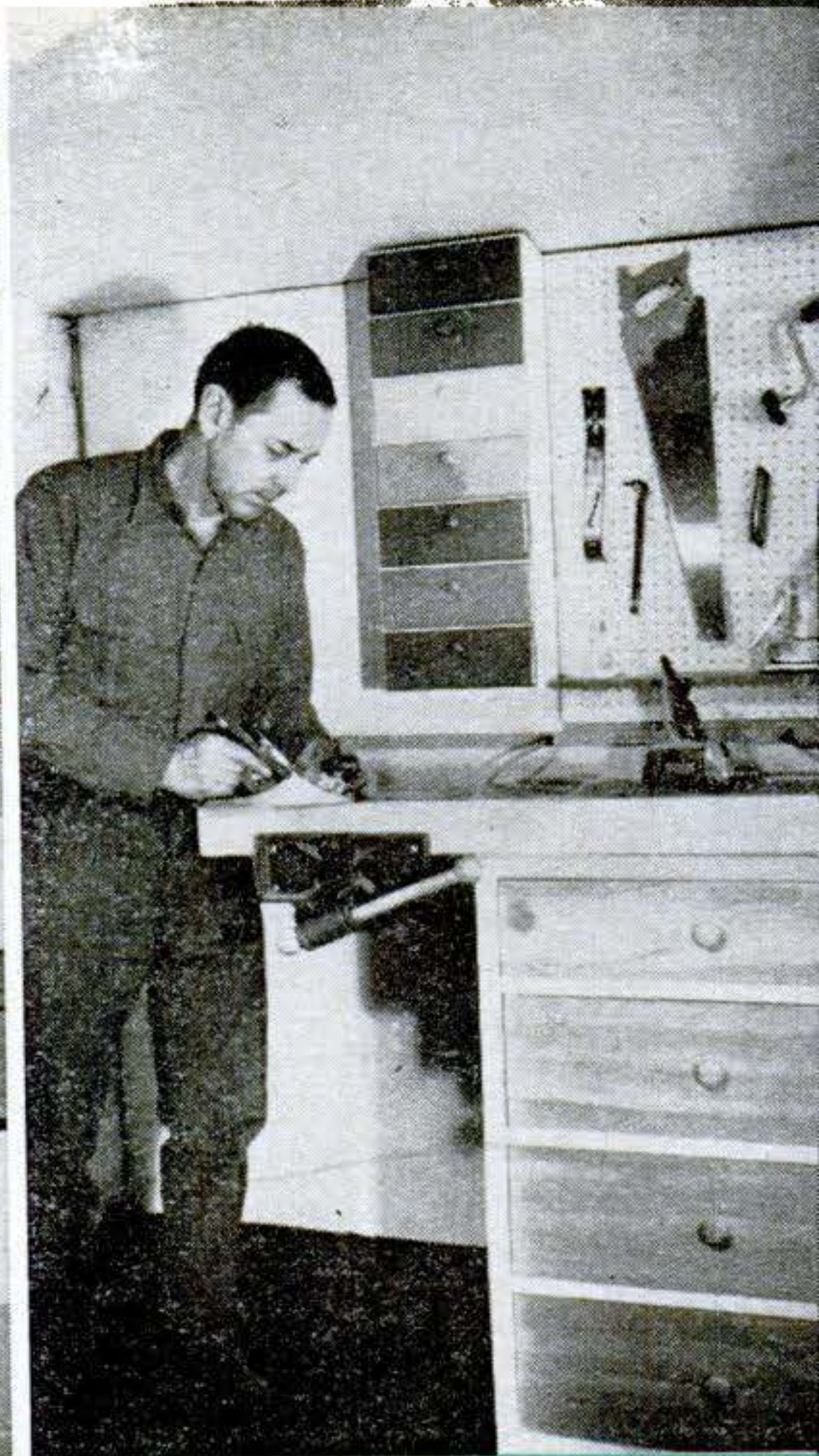
Narrow shop at left has plenty of worktop, ample storage. Drawers in cabinet (above) are built half-depth (see sketch at right) to limit their projection into walkway. Storage shelves are accessible from the side to utilize space behind the drawers.
