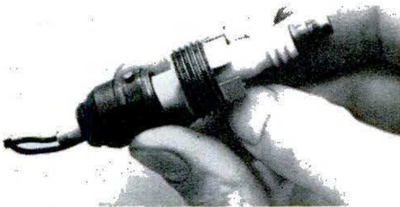
Spark gap has remarkably large surface area and requires plugs of special metals: Iconel base with a gold-palladium tip. Gap erosion is negligible and any tiny surface cracks are considered harmless.
