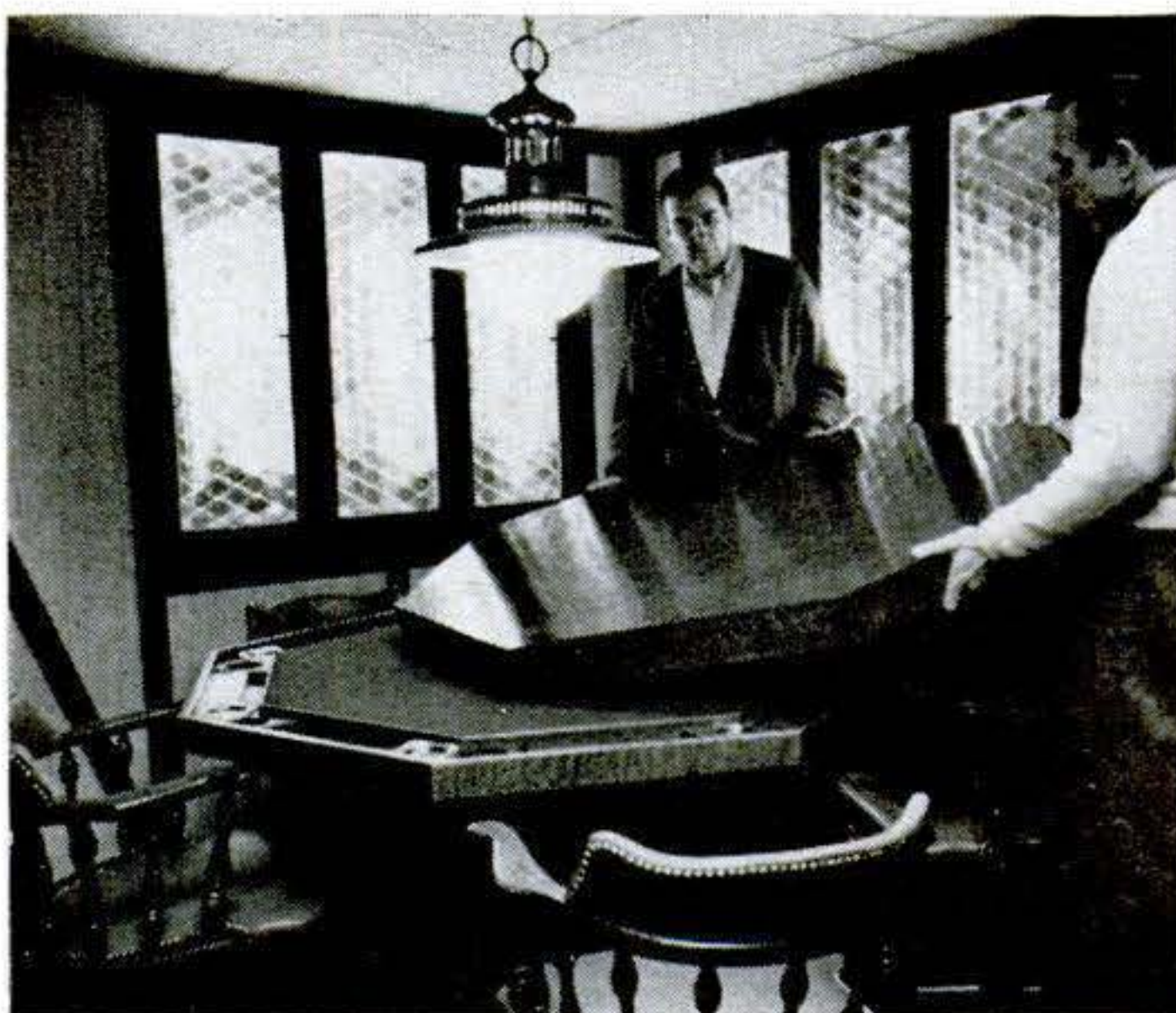
Social corner features octagonal poker table with custom-fitted top that lets it double for refreshments. Top is walnut hardboard with one-by-four pine lip stained to match. Note corner "window."
