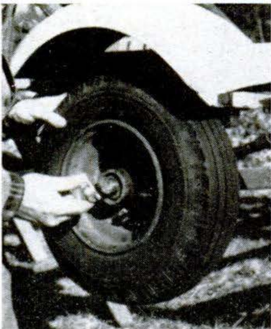
If you run a dry trailer, it will soon break down. Check wheel bearings before and after each season's use. They should also be inspected from time to time during an extended trip. Submersion or heat expansion may make grease leak.
