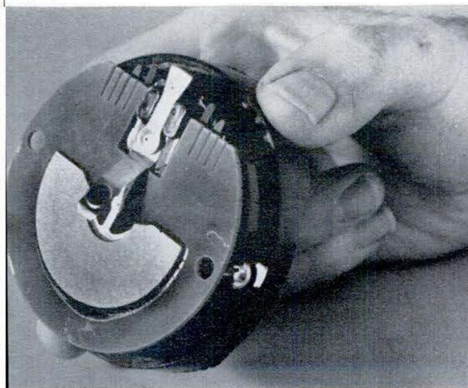
Solar Volt all-electronic supercharger shown above fits in place of the standard distributor rotor. It proved disappointing in gasoline economy but gave some slight improvement in car performance.
