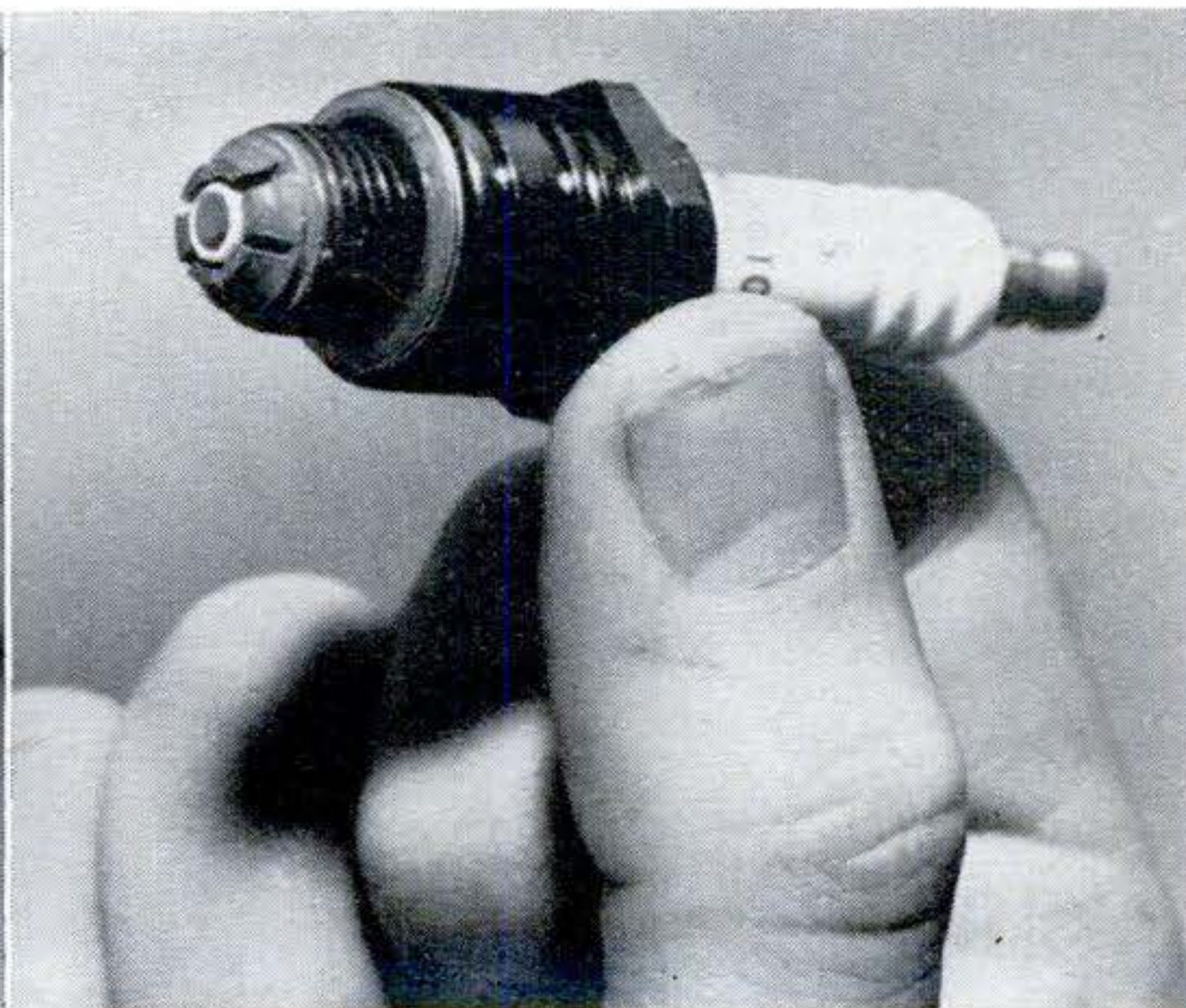
Fire injectors take the place of normal spark plugs and do the same job. PS tests showed insignificant differences compared with standard plugs—but there was certainly no improvement.
