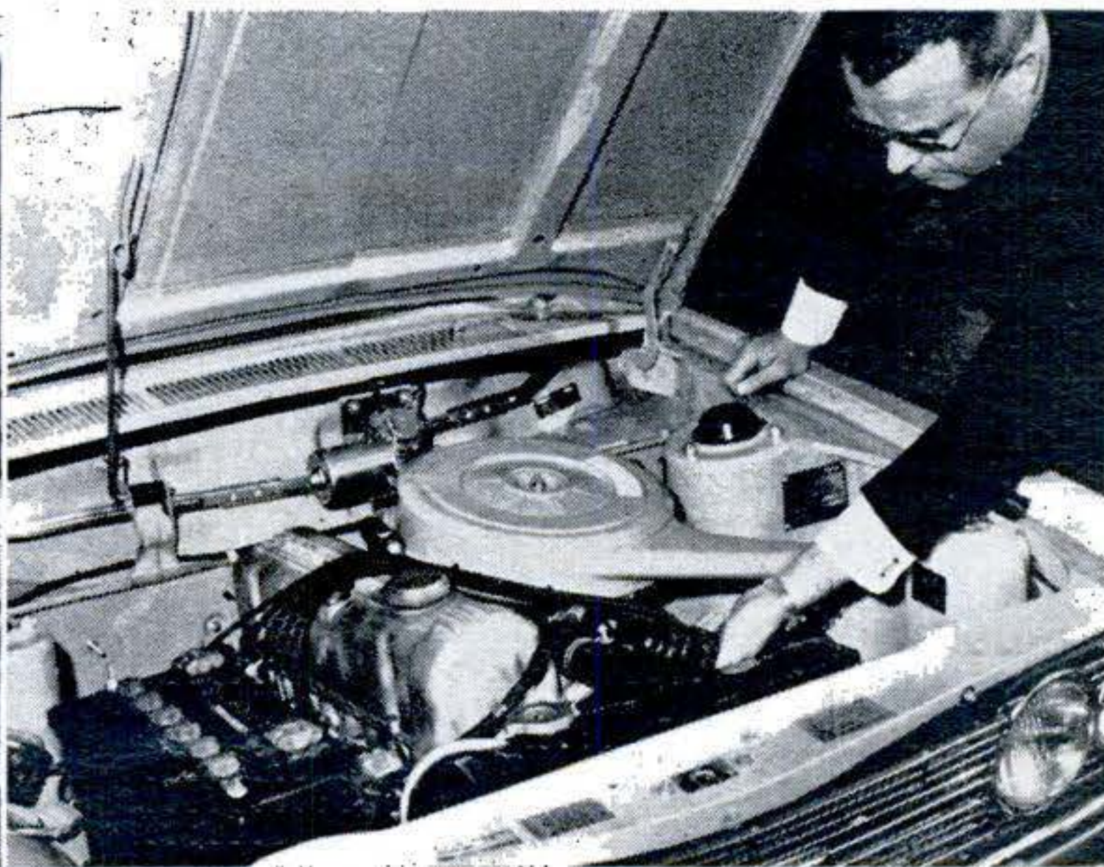
Single-overhead-camshaft engine is the first thing you notice when you open the Datsun's hood. Service accessibility was good but not outstanding. Norbye's left hand holds the distributor cap.
