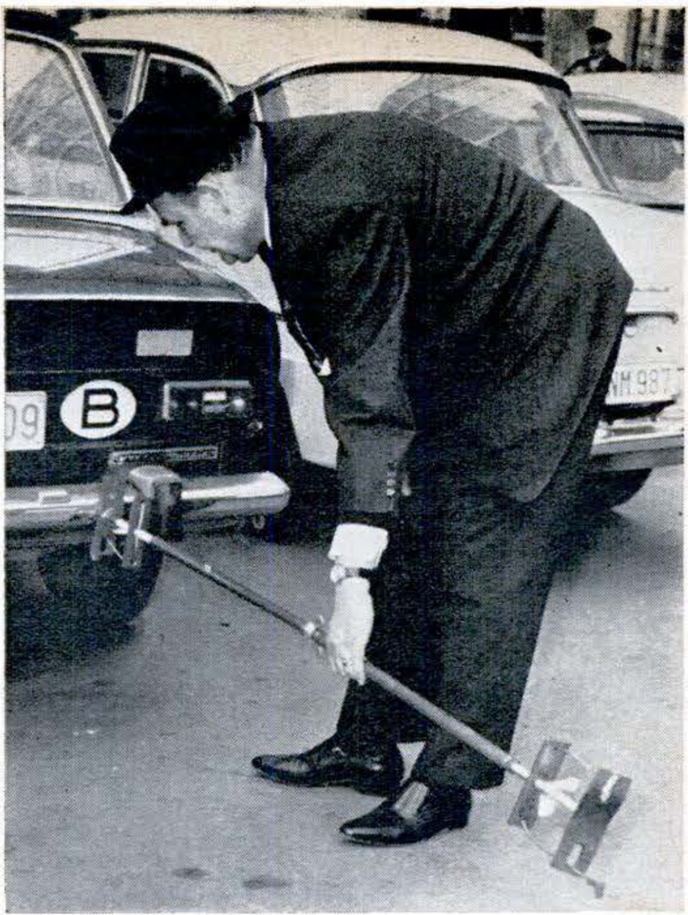
Clamp-on towbar keeps the tow at a fixed distance, eliminates jerking on starting and over-run on braking. Clips at each end hook onto bumper, are tensioned by a wingnut. Ball joints seating against the contact plate permit movement in all directions.—A. Classen, 437 Marl i. W., Bergstr. 10, Germany.
