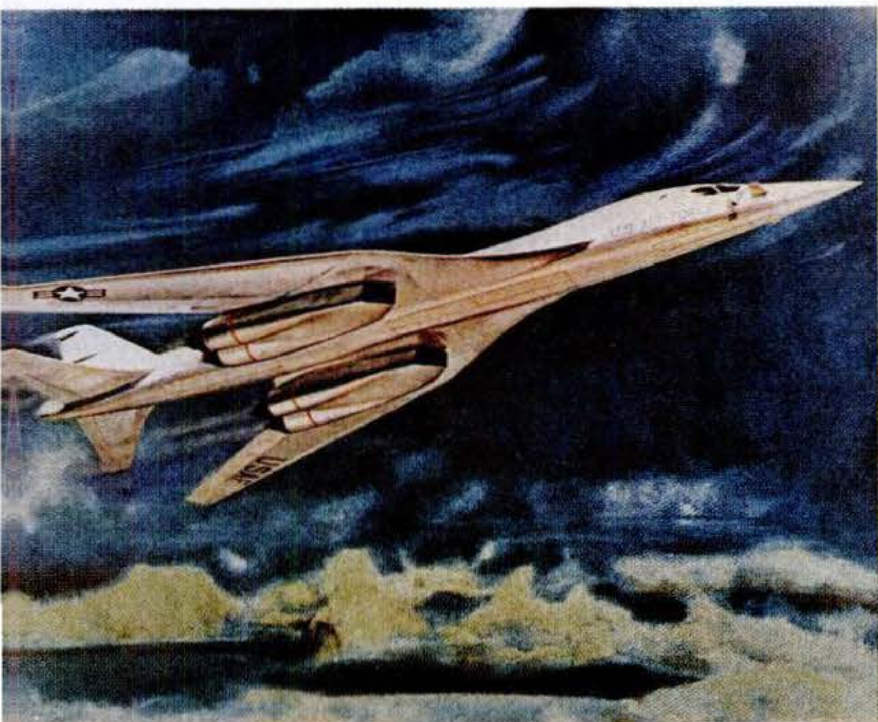
Underbelly view of B-1 shows position of four engines in two separate pods under fixed inner portion of variable sweep-wing. Bumps on rudder house sensors for electronic countermeasures.
