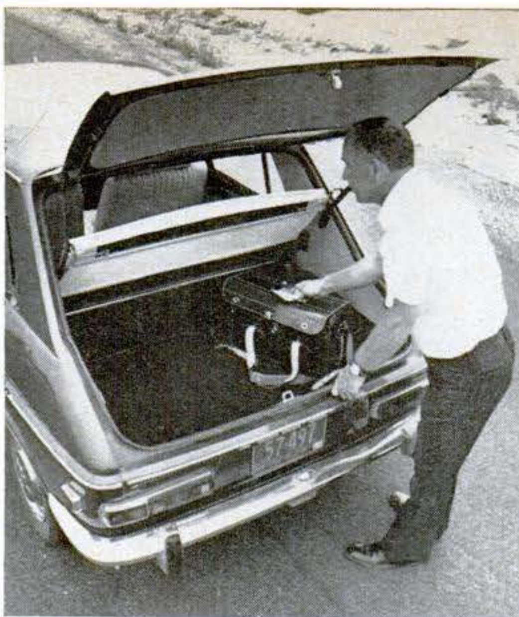
Extremely versatile back seat and trunk give the Simca the carrying capacity of a station wagon. The trunk lid is hinged at roof level, and the rear seat folds down to make a flat loading platform.
