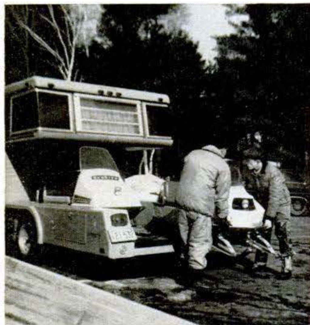
Ramps slide out for handy loading on the Trans-Por-Teer. Fitting this Evinrude Skeeter and Polaris Playmate snugly into the parking port proved to be relatively easy.
