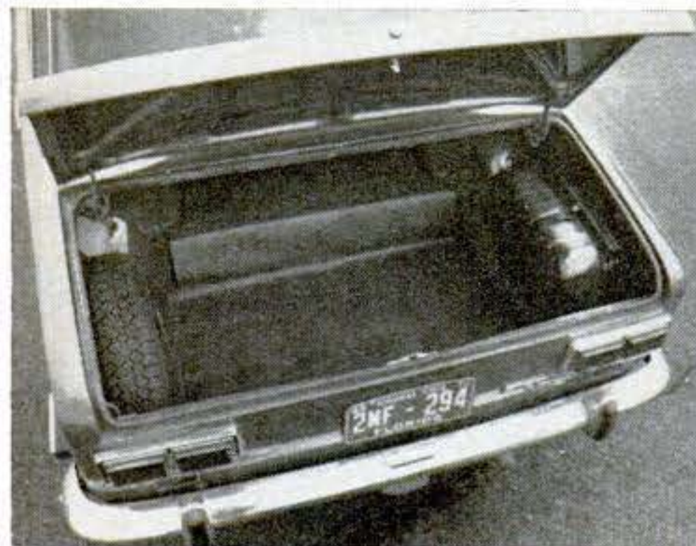
Fiat trunk is long and deep, holds 14 cubic feet of useful space, with 31-inch liftover height. Fuel tank is in right fender.
