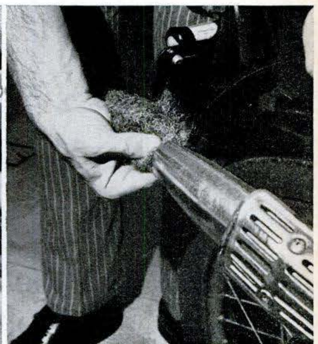
If baffles blow out of your muffler , you're likely to get a ticket. As a substitute, insert a large piece of coarse steel wool inside muffler to cut down noise level.
