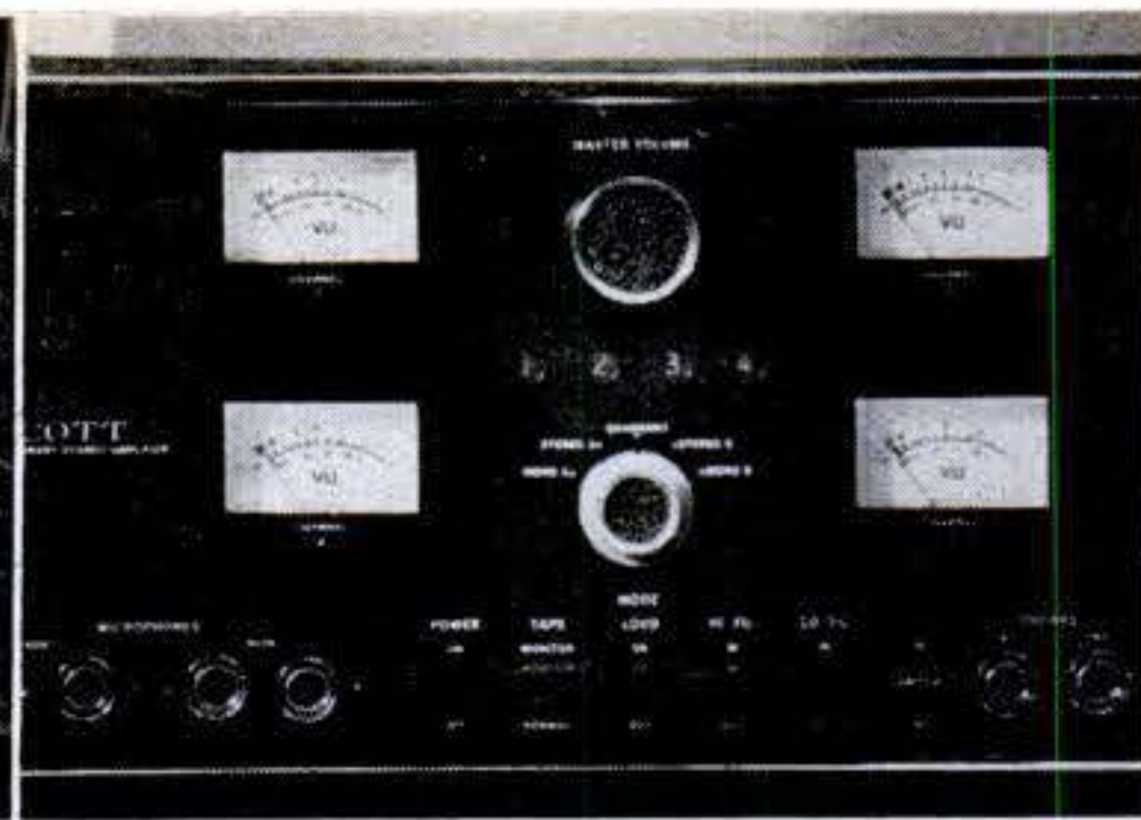
All the controls you need to balance four speakers are on Scott's new 499 amplifier.
