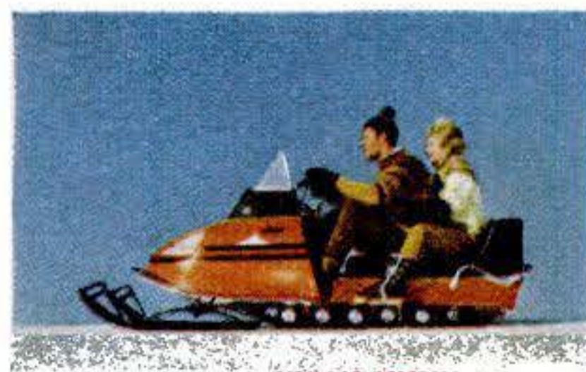
Ariens Arrow 400L snowmobile with 19" wide track and 399cc, twin cylinder Kohler engine.
