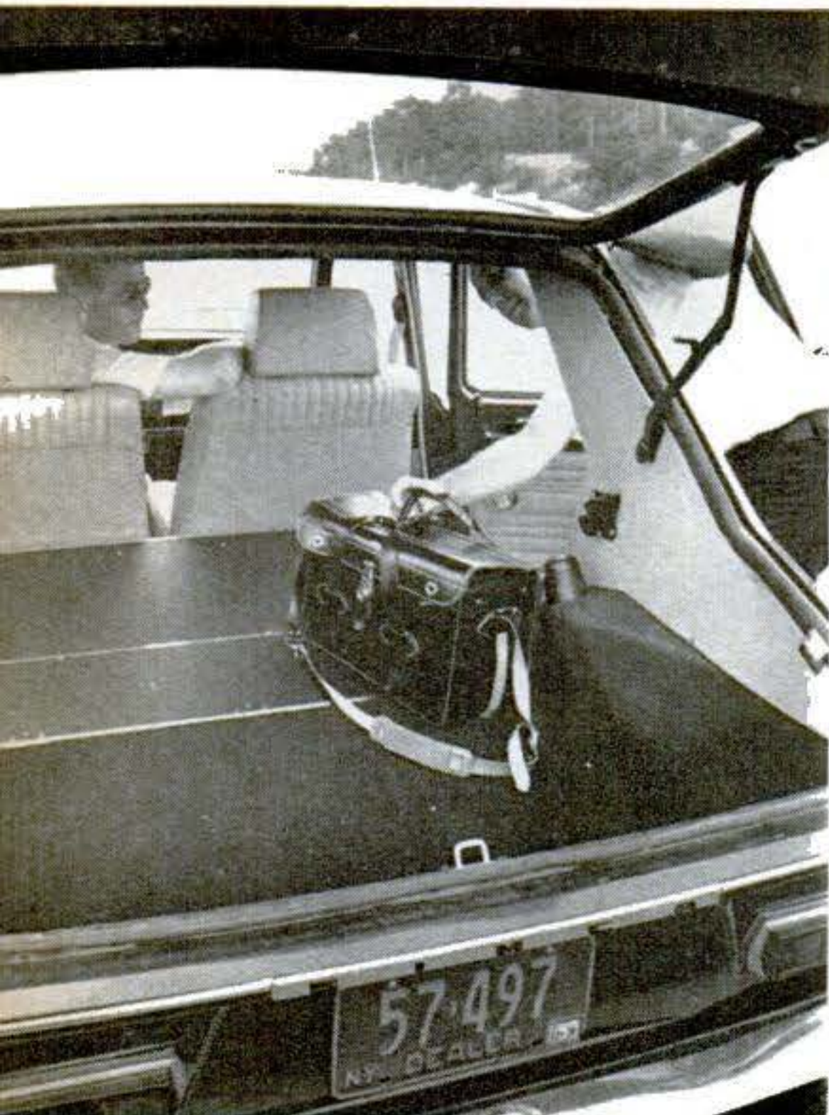
Extremely versatile back seat and trunk give the Simca the carrying capacity of a station wagon. The trunk lid is hinged at roof level, and the rear seat folds down to make a flat loading platform.
