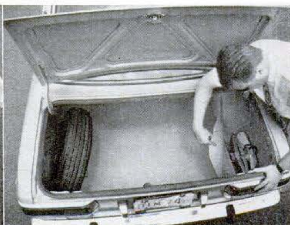
Toyota trunk holds 10.9 cubic feet, with 32.5-inch liftover. Tools store at right, spare wheel in slanting position at left.
