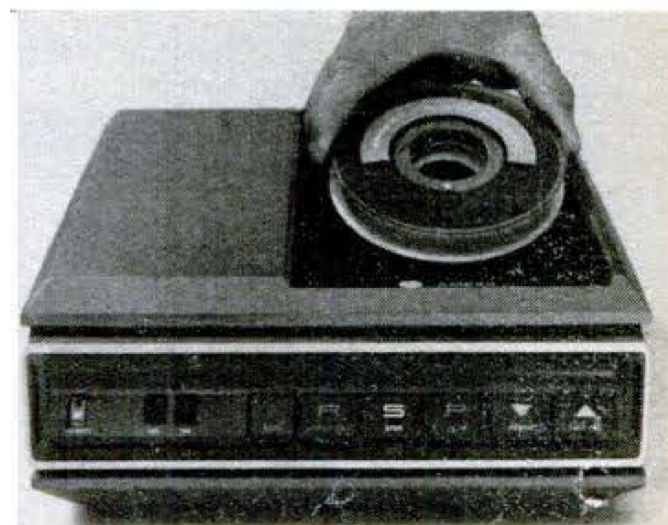
Plastic cartridge for Instavision uses standard video tape of half-inch width.
