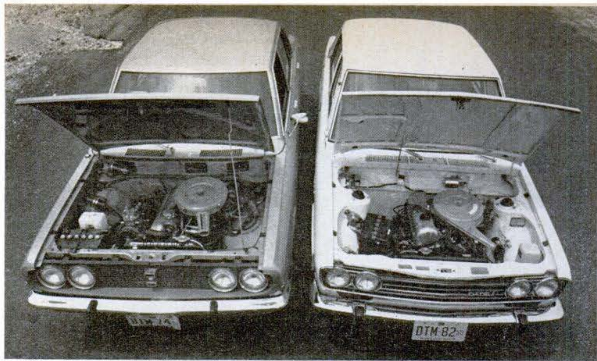
Toyota and Datsun (right) have overhead-cam engines. Both can claim first-class ser-
