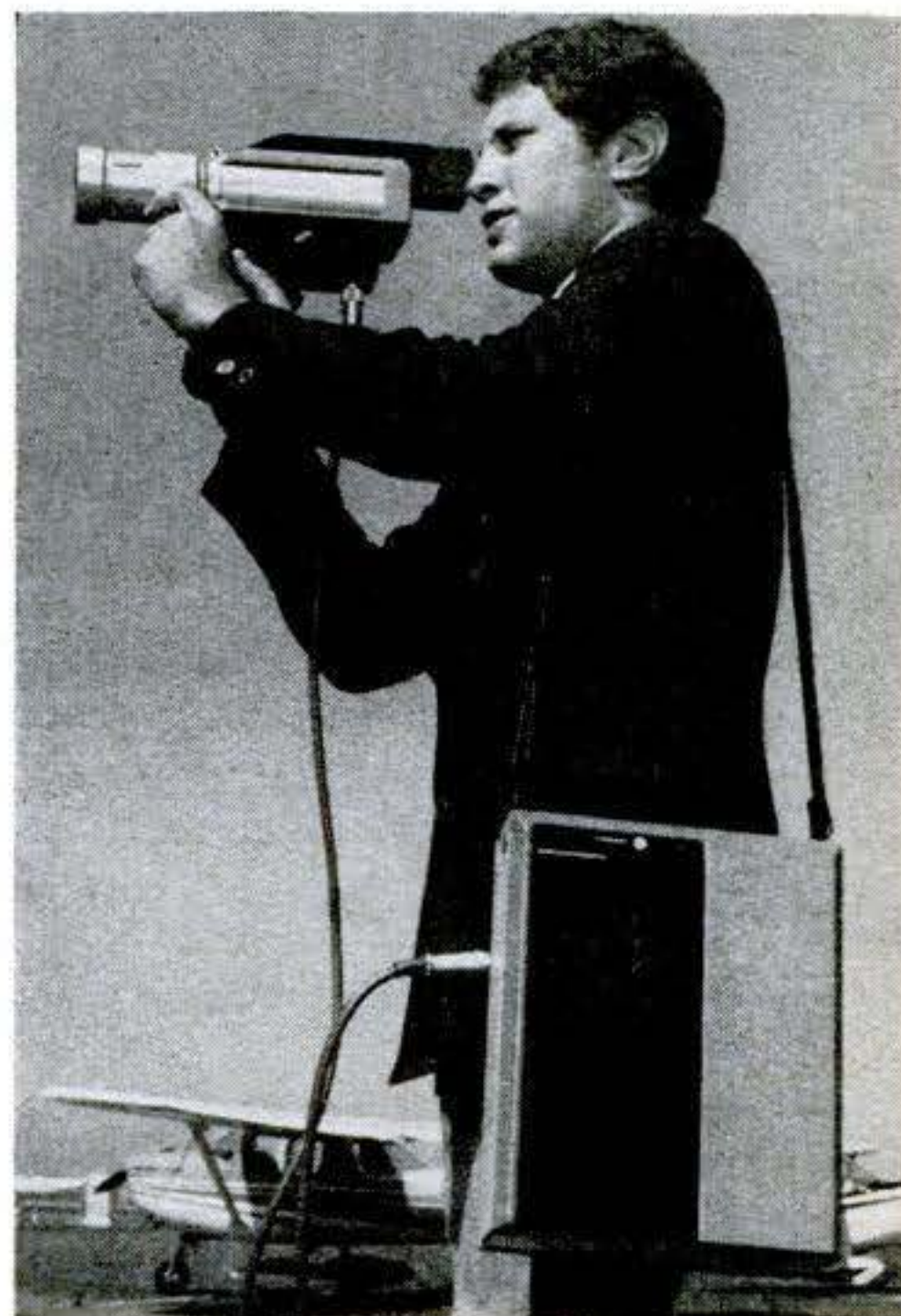
Late entry in cartridge-TV sweepstakes is Instavision. The Ampex portable records off a matching camera or from color or B&W TV set; works on AC and batteries.
