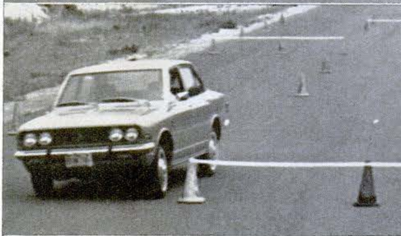
Lane change: Simca (top) proved remarkably surefooted—it has front-wheel drive—and stayed level at all times. Toyota was slowest, due to body roll and tire slip.
