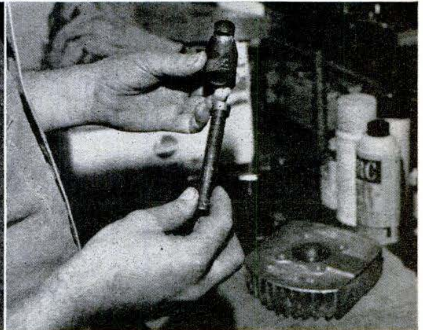
4 Heli-Coil is slipped on the insertion shaft, as shown. It is then screwed into the base of the tool. Be sure that all parts are clean and lightly lubricated.
