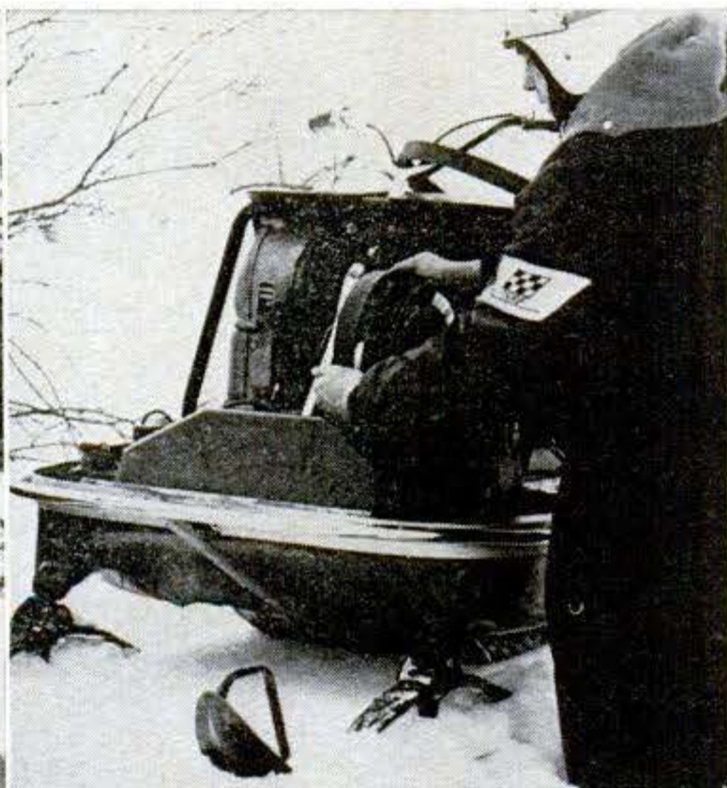
A glazed drive belt gets replaced before starting out on a trip to the lighthouse. A shot of winter grease in the squeeze pulley bearing put quick end to the glazing.
