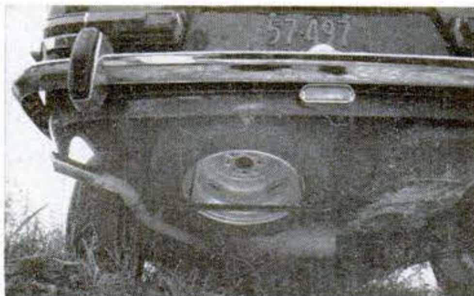
Simca spare wheel is stored out of the way, and removal requires tools. Job is difficult and tends to get clothes dirty.
