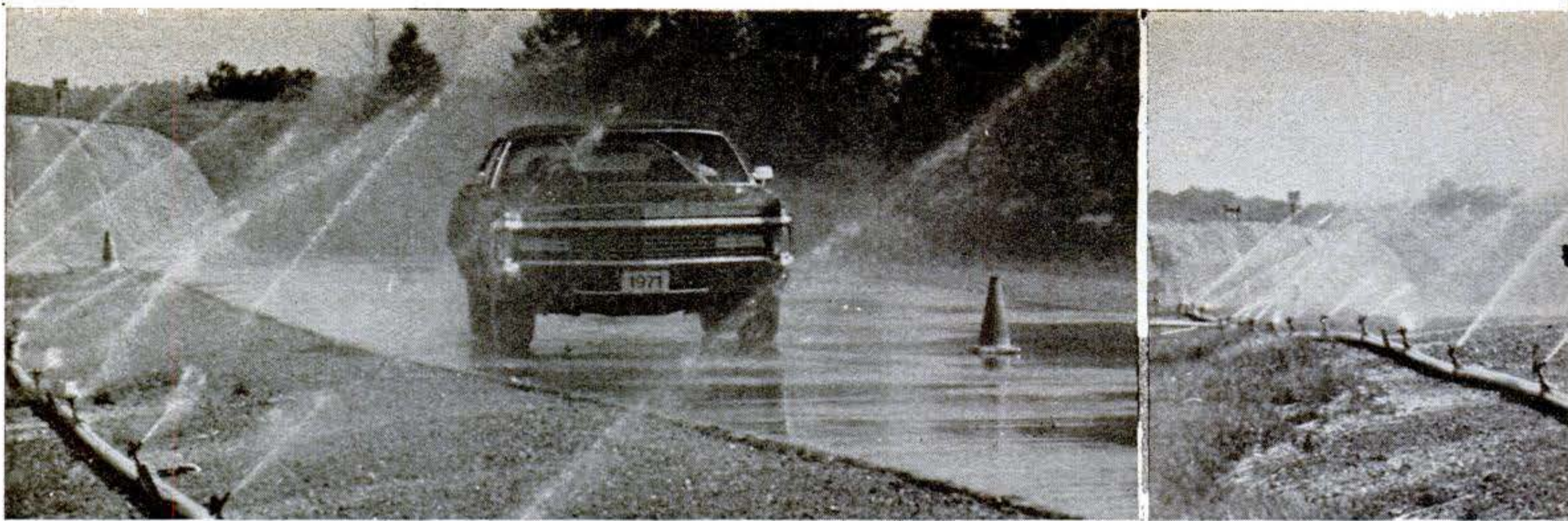
Imperial with Sure-Brake stops in straight line (left), 40 percent shorter than Imperial without Sure-Brake (right), which slowed
