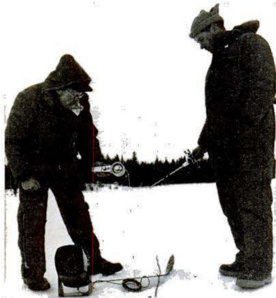
Electronic helpers are boon: Fish flasher—such as Vexilar Sound Off Sonar on ice, left—helps locate schools. Zonar electronic thermometer (held) helps choose depth.
