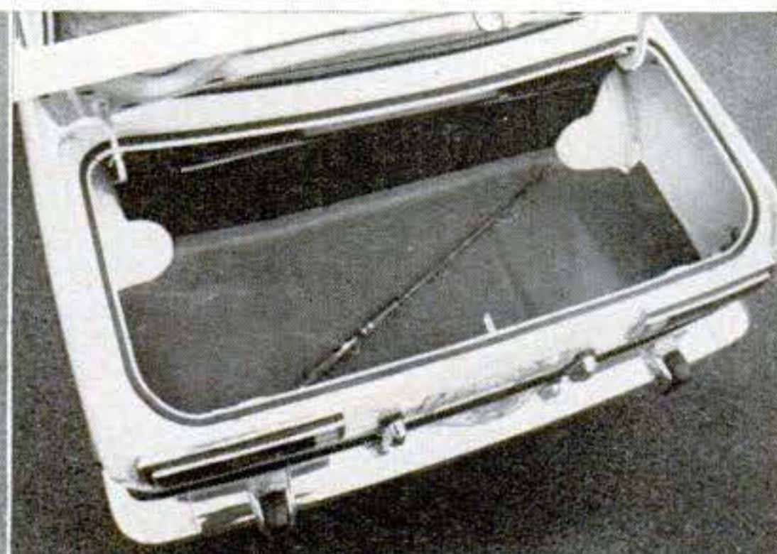
Datsun trunk has wide flat floor, holds 12.5 cubic feet, with 33-inch liftover. Tank and spare wheel are under trunk floor.
