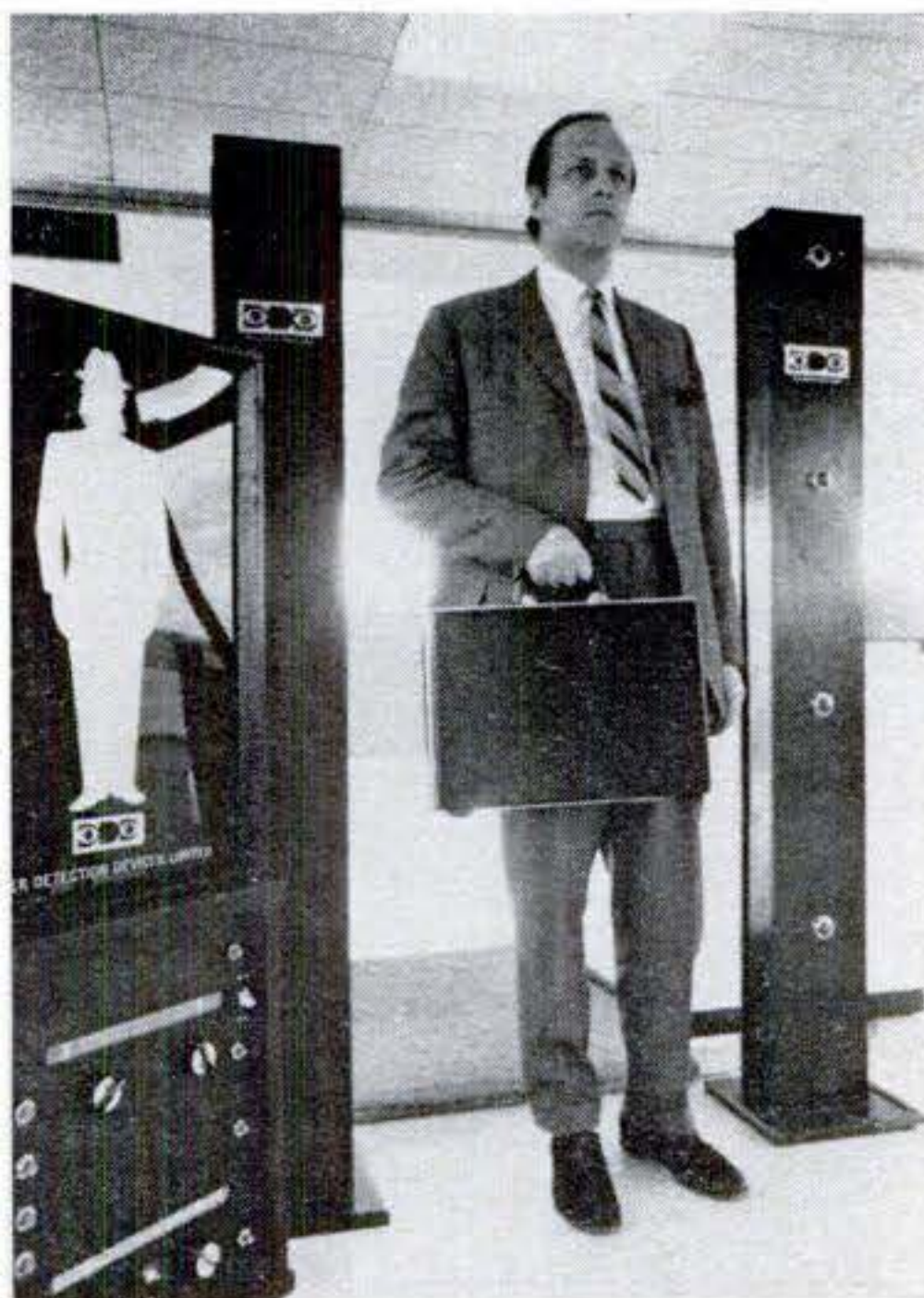
When a gun-toter walks through this British anti-hijacking device, made by Diver, it alerts three ways: A red light flashes, an alarm goes off, and a human figure on an adjacent screen lights up to indicate the weapon's location in clothing or baggage.
