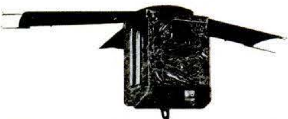
ITOS satellite of 1970 is a prototype of ESSA's new fleet of Improved TIROS Operational Satellites for weather watching.
