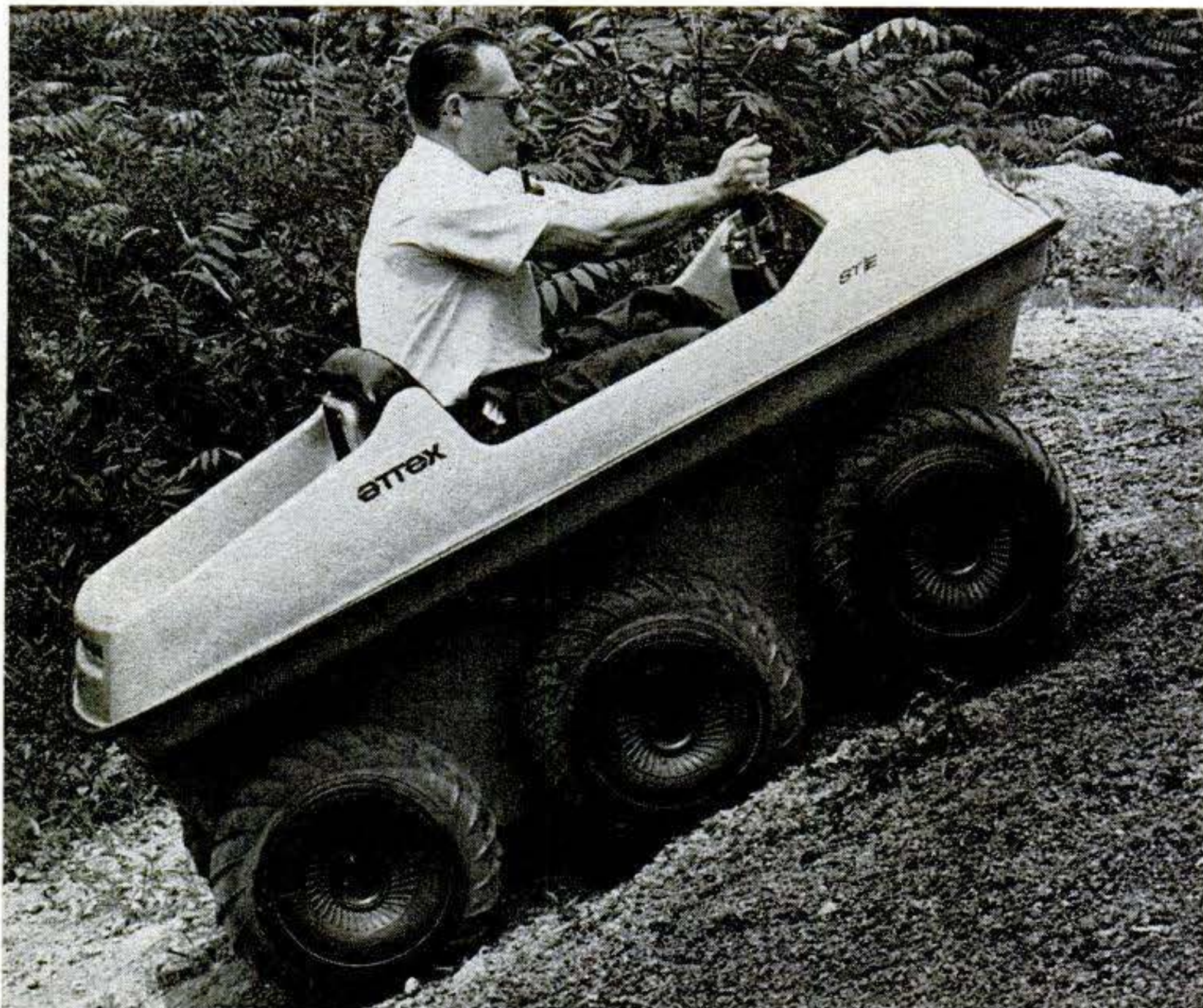
High torque from electric motor takes the Attex and author up a steep slope with ease.
