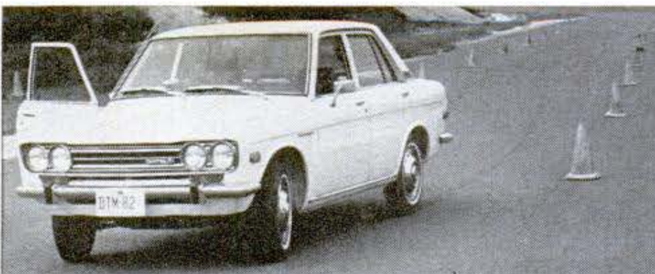
Datsun slewed to a stop from 60, fade-free but bothered by rear wheel locking, side pull. Distance: over 225 feet.
