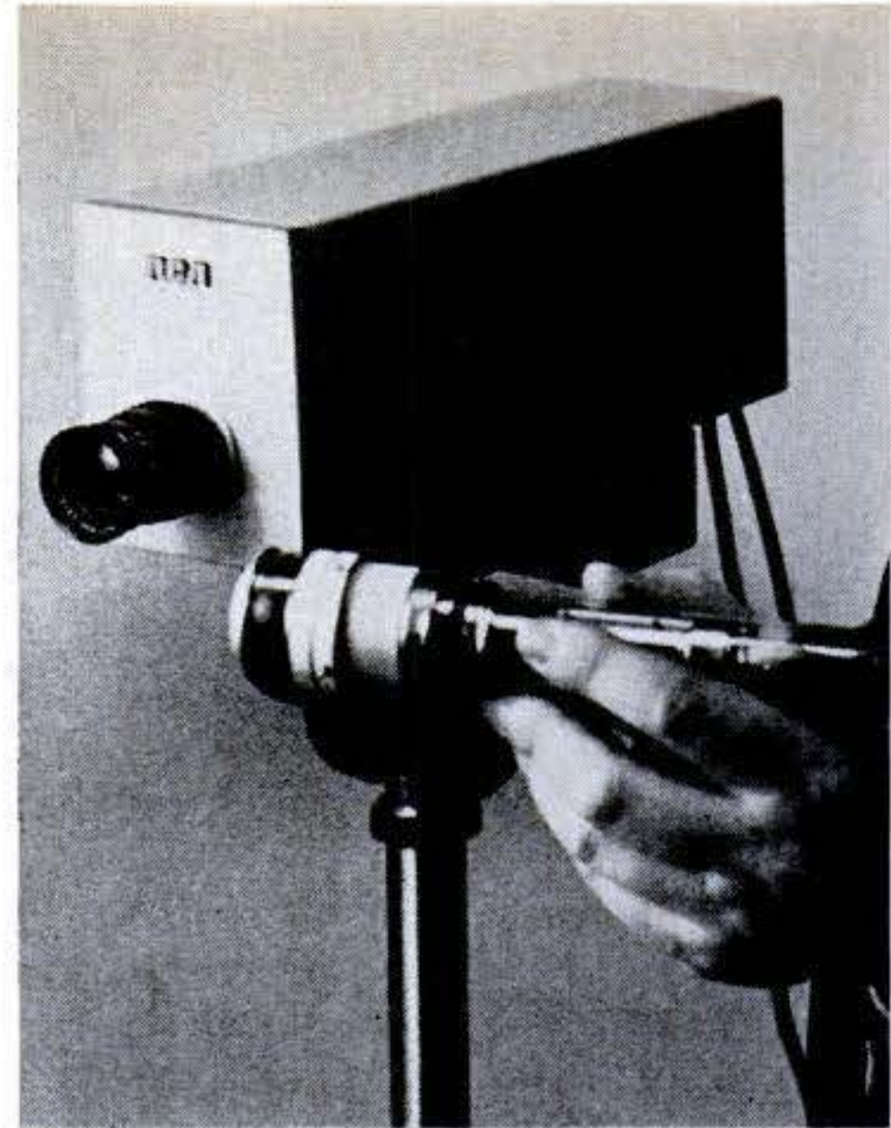
A prototype low-light-level TV camera is shown with the silicon intensifier tube that amplifies incoming light. The tube is similar in size to conventional vidicons.
