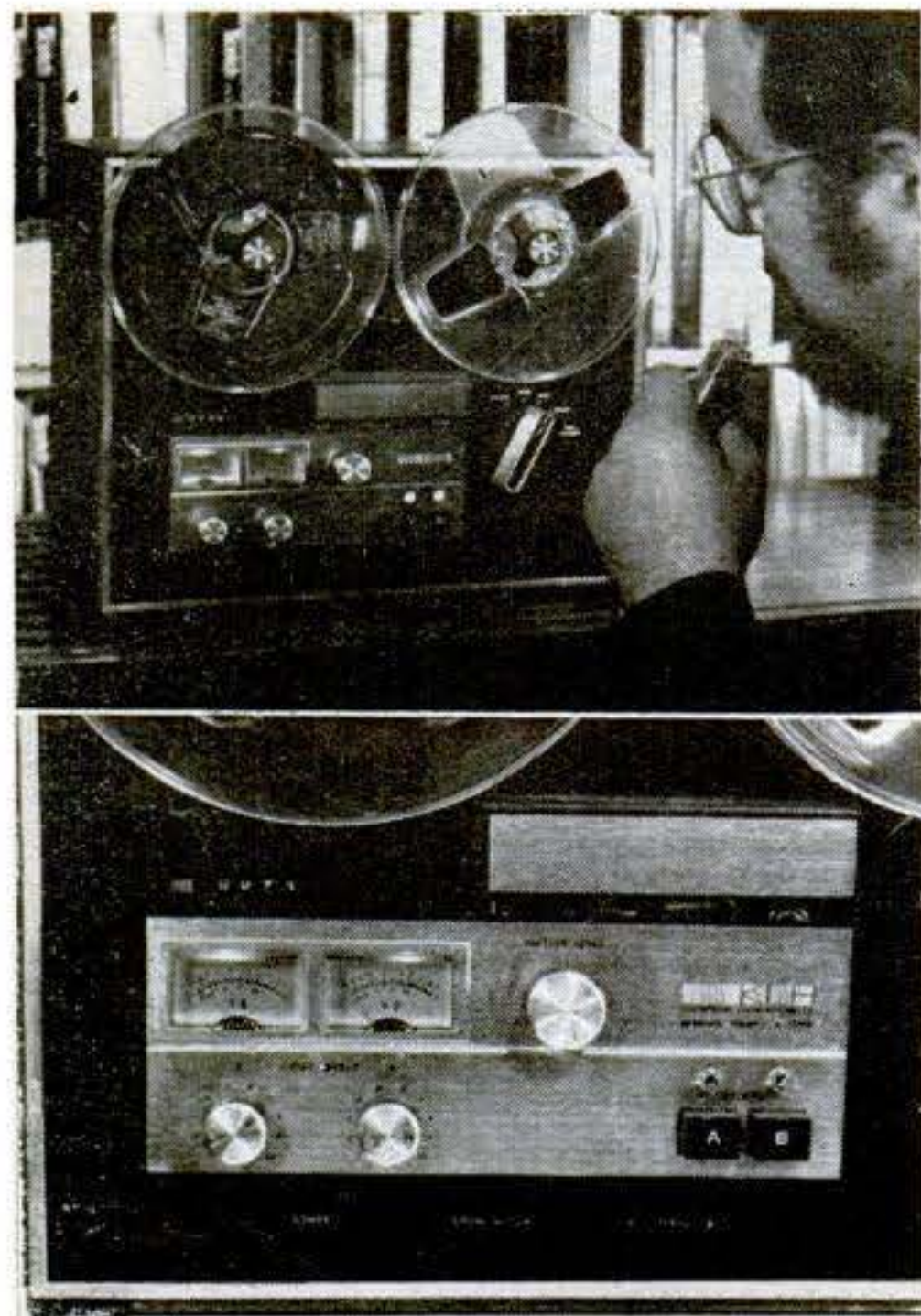
Using part of a professional noise-reducer circuit, the KLH 41 sharply lowers tape hiss.
