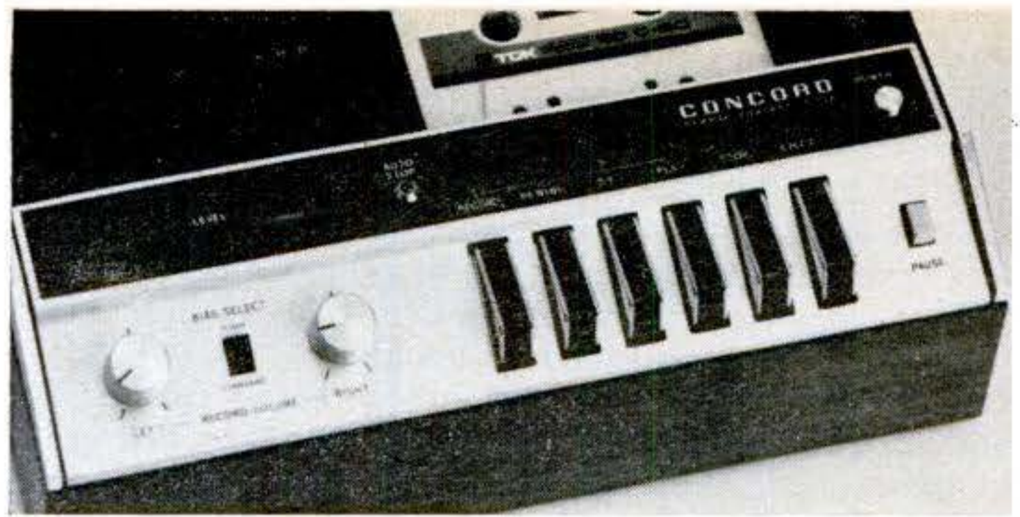
A bias select switch included on the Concord F-106 lets you increase the tape bias level for the new high-density tapes.
