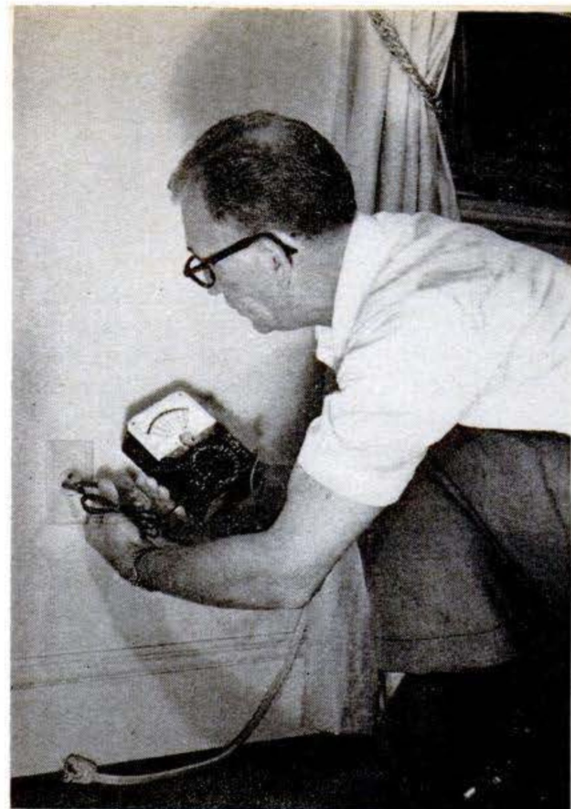
First place to check is outlet where major appliance—such as this window air conditioner—plugs in. Blown fuse? A house call by service technician to replace it would cost price of a good VOM.
