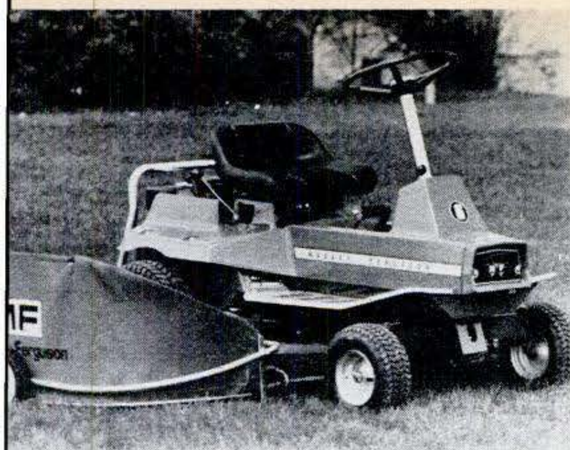
Massey-Ferguson six-horse rider has neat controls, fiberglass upper deck. Side car holds five bushels of grass or leaves.
