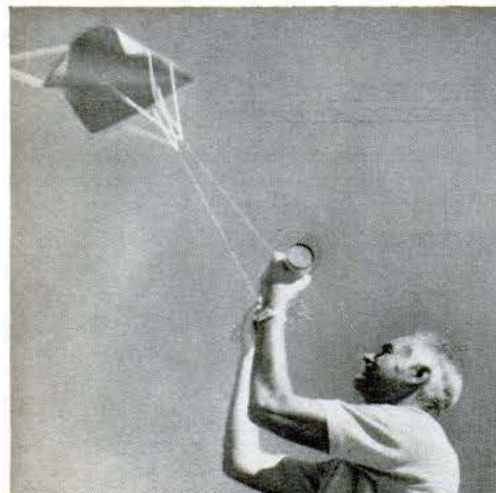
Inventor of the parawing , Francis Rogallo, launches small one at Kitty Hawk. Big versions of his design carry men aloft.
