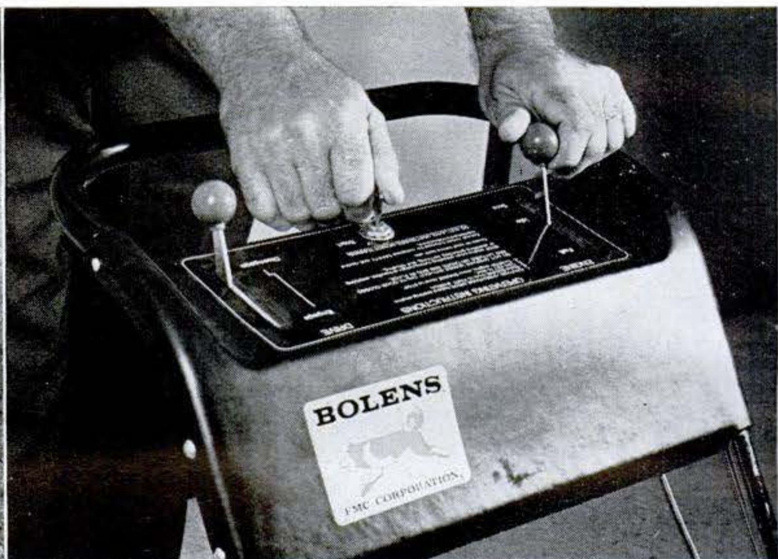
Bolens control panel on walk-behind lets you operate throttle and clutch while you keep your eyes on the ground ahead.
