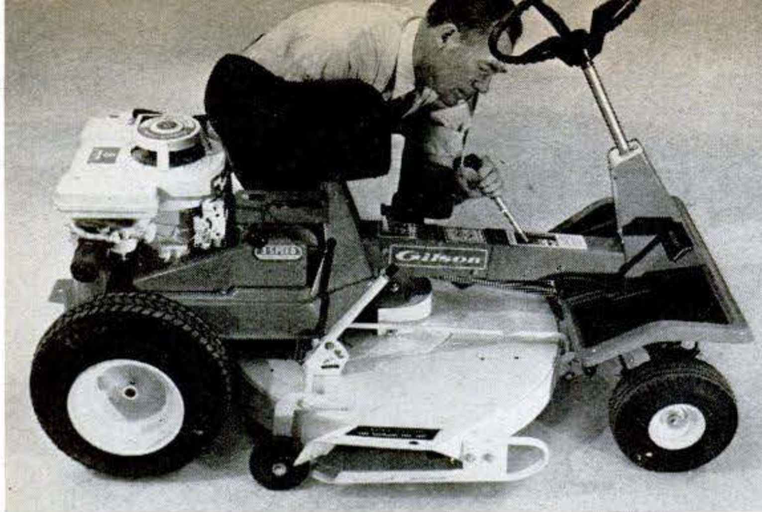
Gilson rider gate-shifts for no-error control, lets you shift without clutch or blockout. It cuts 30-inch swath with eight hp.
