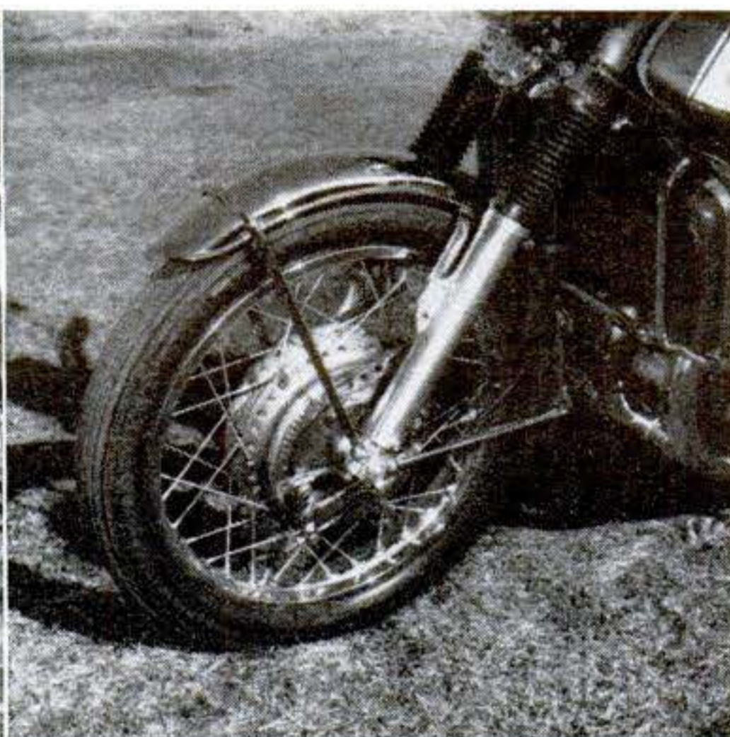
Good brakes? You bet. Instead of using disks up front, the GT-750 features an effective quadruple-leading-shoe setup.
