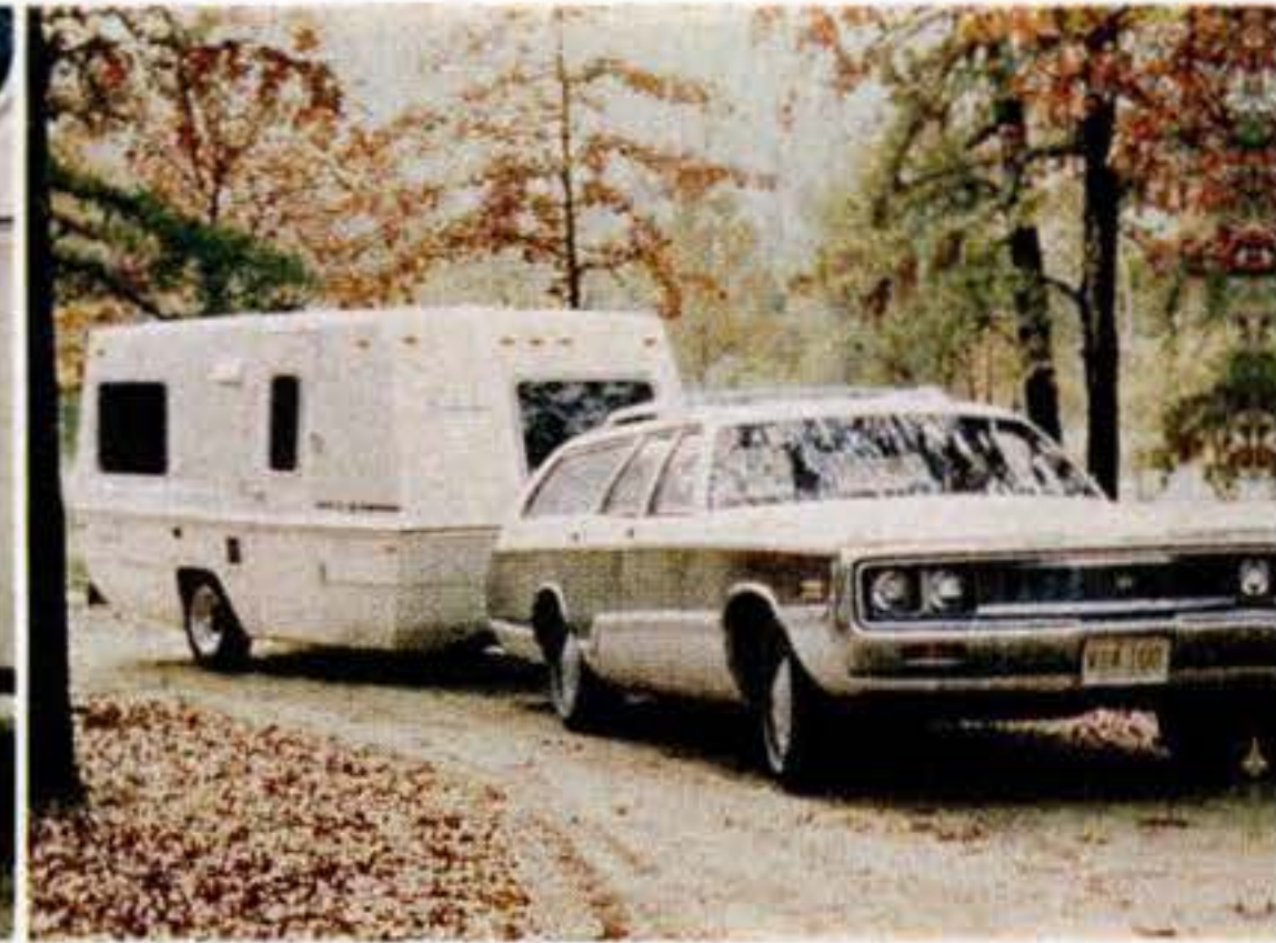
Low seven-foot height makes Amerigo easier to tow with standard car in head winds.
