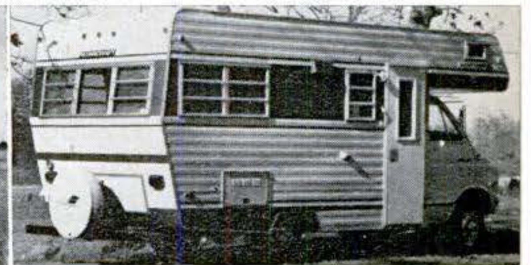
Aristocrat 19-foot Miniliner is built on Chevy cutaway van with 125-inch wheelbase. It sleeps six, is fully self-contained.
