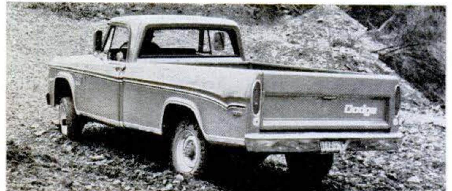
Dodge pickup truck above is equipped with the new manually operated Chrysler 4WD system with positive front/rear locking.
