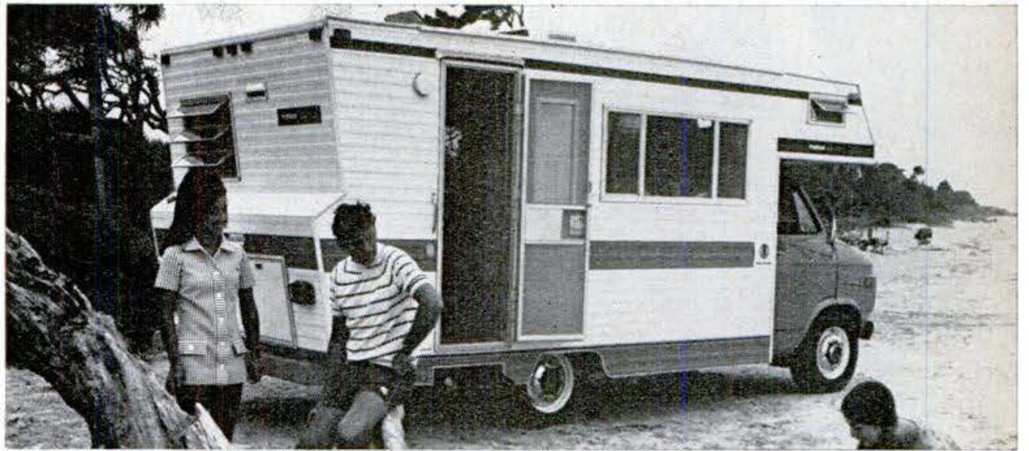
Starcraft 19-foot motor home is built on cutaway Dodge chassis with a 127-inch wheelbase. It's powered by a 360-cu.-in. V8, is available with rear or side galley.
