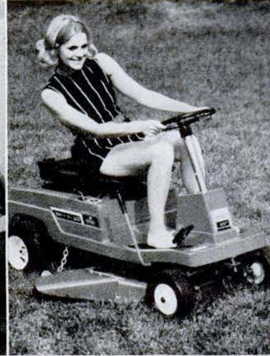
Sears rear-engine rider is an all-new model with seven hp, 26-inch cut, safety discharge chute, single-pedal foot control of both clutch and brake.
