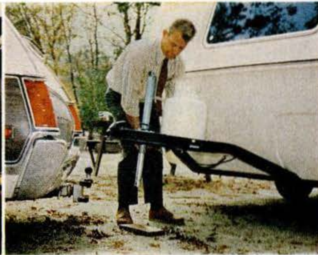
Tongue weight is light enough for one man to lift it and latch onto ball hitch.
