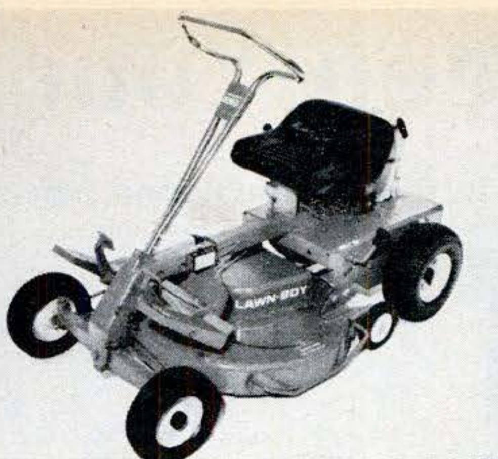
Lawn Boy 26-inch compact is a nimble and sturdy rider for small lawns. It has five-horse engine, two speeds forward, reverse.
