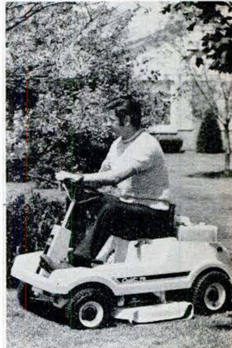
International Cadet 75 has side or rear discharge, two blades in floating deck that adjust on the go. Body is lightweight, rustproof fiberglass.
