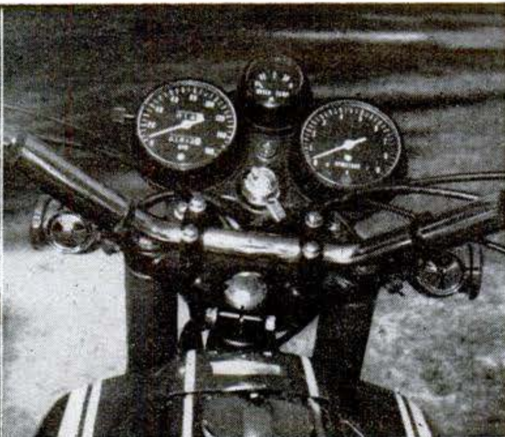
Instruments are shock-mounted. The temperature gauge is in the center. Ignition key is conveniently in the center, too.
