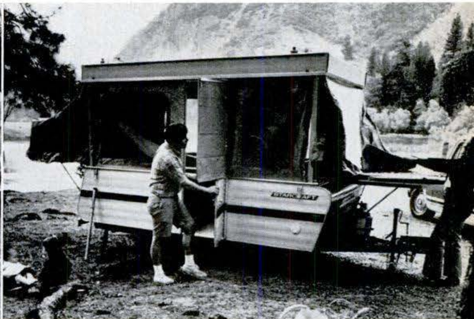
Starcraft Starmaster 6 is medium-size camper with lots of interior space, big swing-up galley, and 12v converter for interior lighting. Starcraft has rugged steel frame, sandwich walls.
