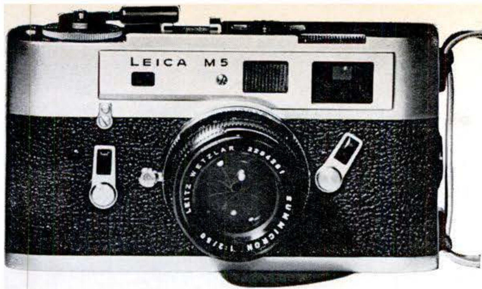
Front-mounted controls are almost identical to those on the M4 (M5's predecessor). Lever to right of lens selects viewing frames. Film-rewind crank? It's recessed into camera bottom.
