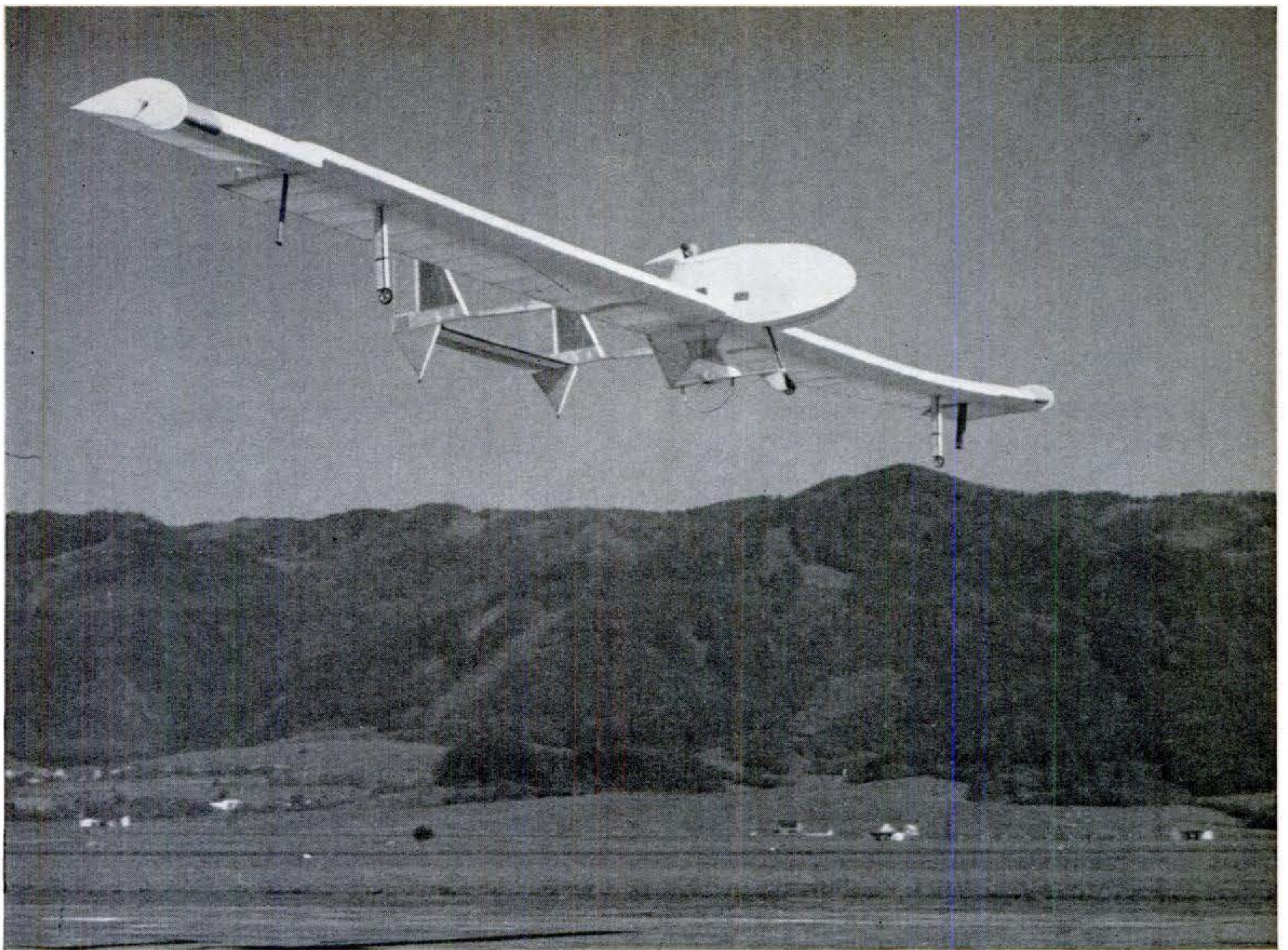
Tow-launched to 10 meters altitude, Josef Malliga's skycycle is pedaled 400 meters through the blue. It takes off man-powered, too.
