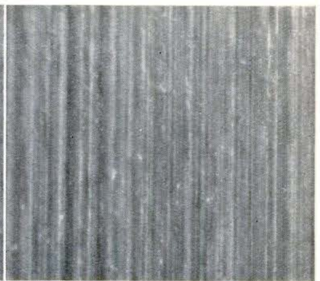
Garnet belt in the sander gives much smoother surface than aluminum oxide. Surface is easy to fine-sand before finishing.
