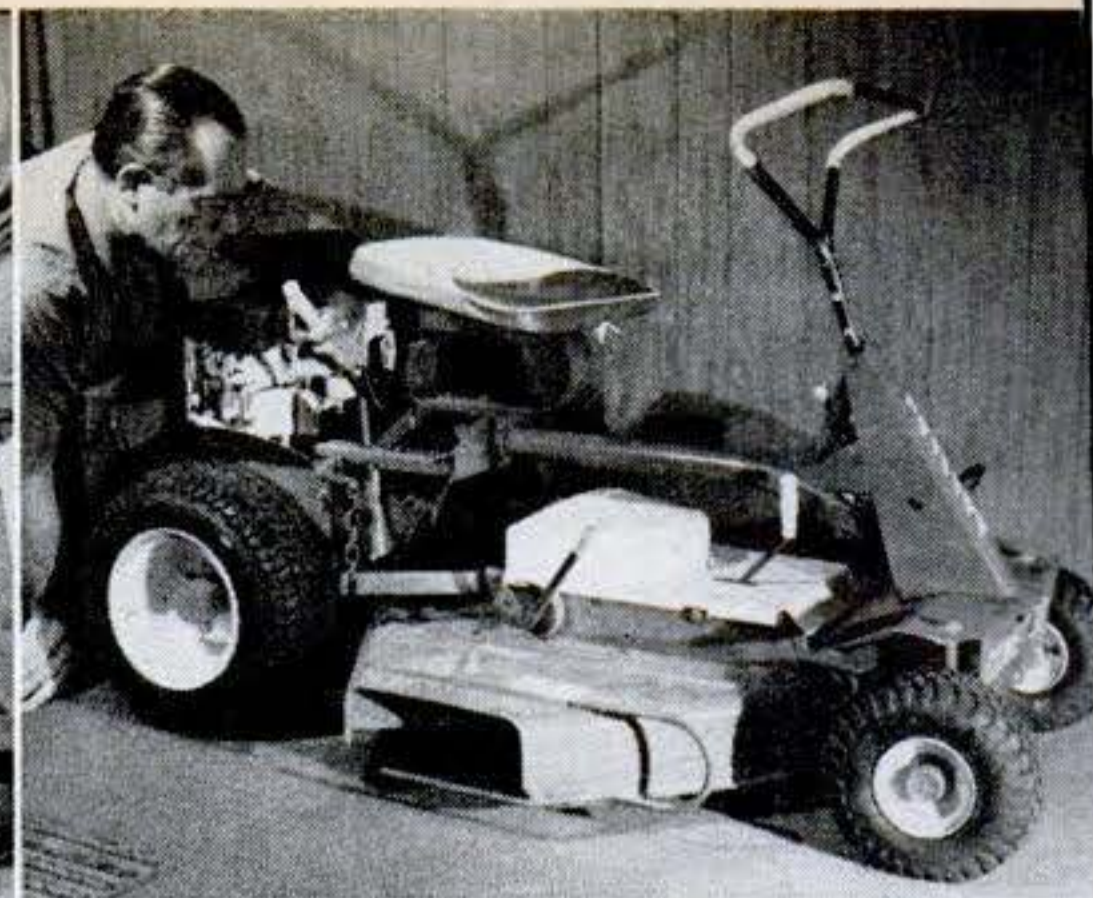
Snapper Comet has excellent deck mount, positive controls, and solid construction details including a tubular-type frame.
