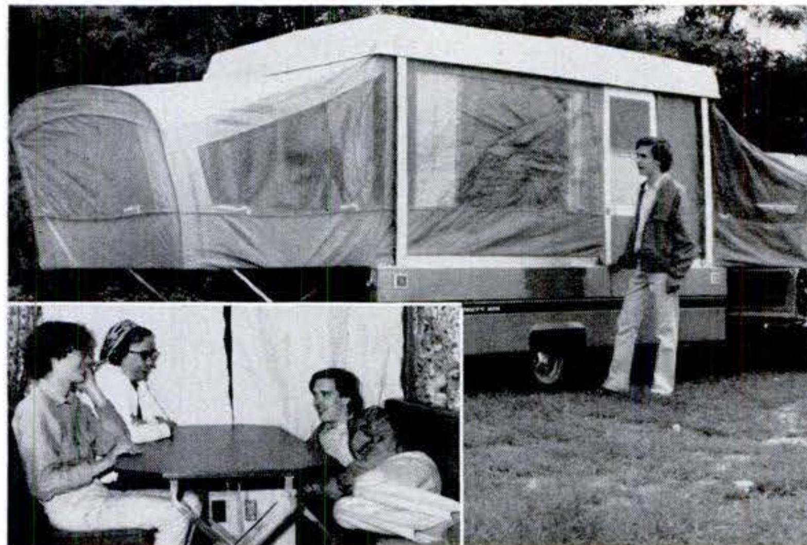
Coleman camper expands into a surprisingly large interior with Mylar picture windows. Bunks are big and comfortable, and the large dinette (inset) makes a good place to sit around and talk.
