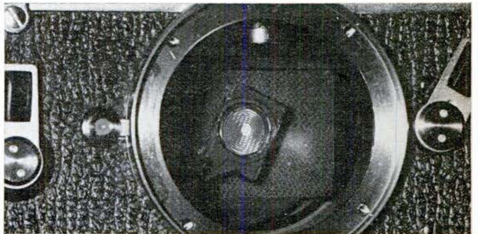
Meter cell sits on pivoting arm directly in front of focal-plane shutter. It swings down and to the side for exposure.
