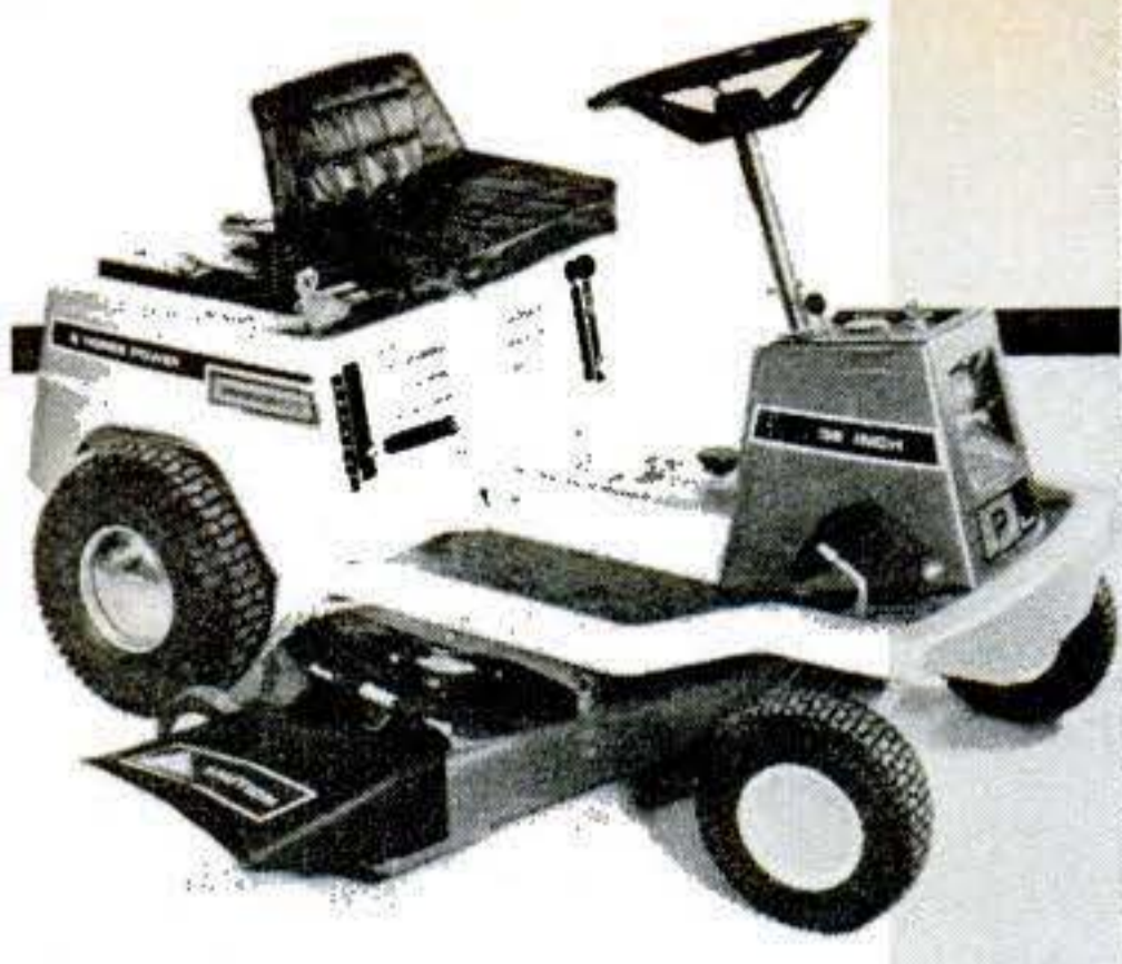
Penncraft mowers from J. C. Penny feature large, easy-to-reach controls and a safety interlock that prevents in-gear starting.
