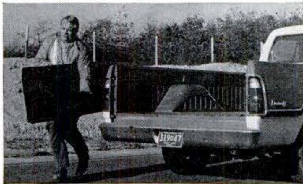
Dodge tailgate can be removed in half a minute without use of tools. Refitting it is equally simple and easy.
