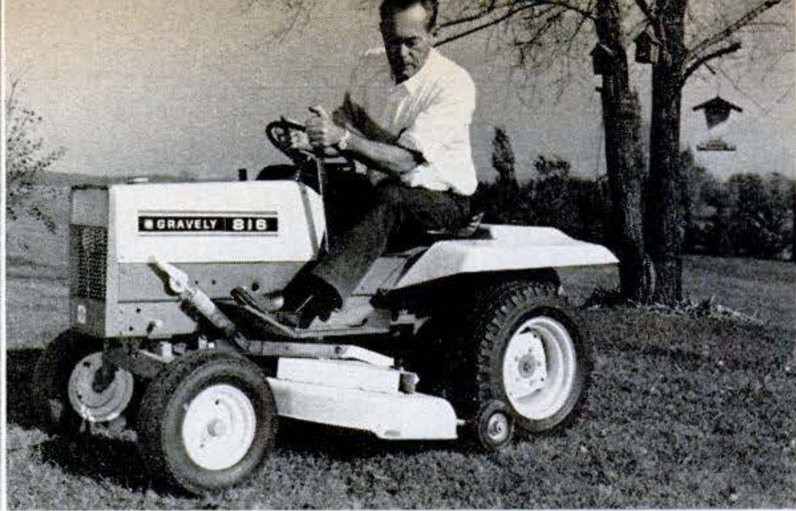
Gravely's new workhorse mower has an eight-speed, all-gear transmission, instant reverse, and high deck clearance.
