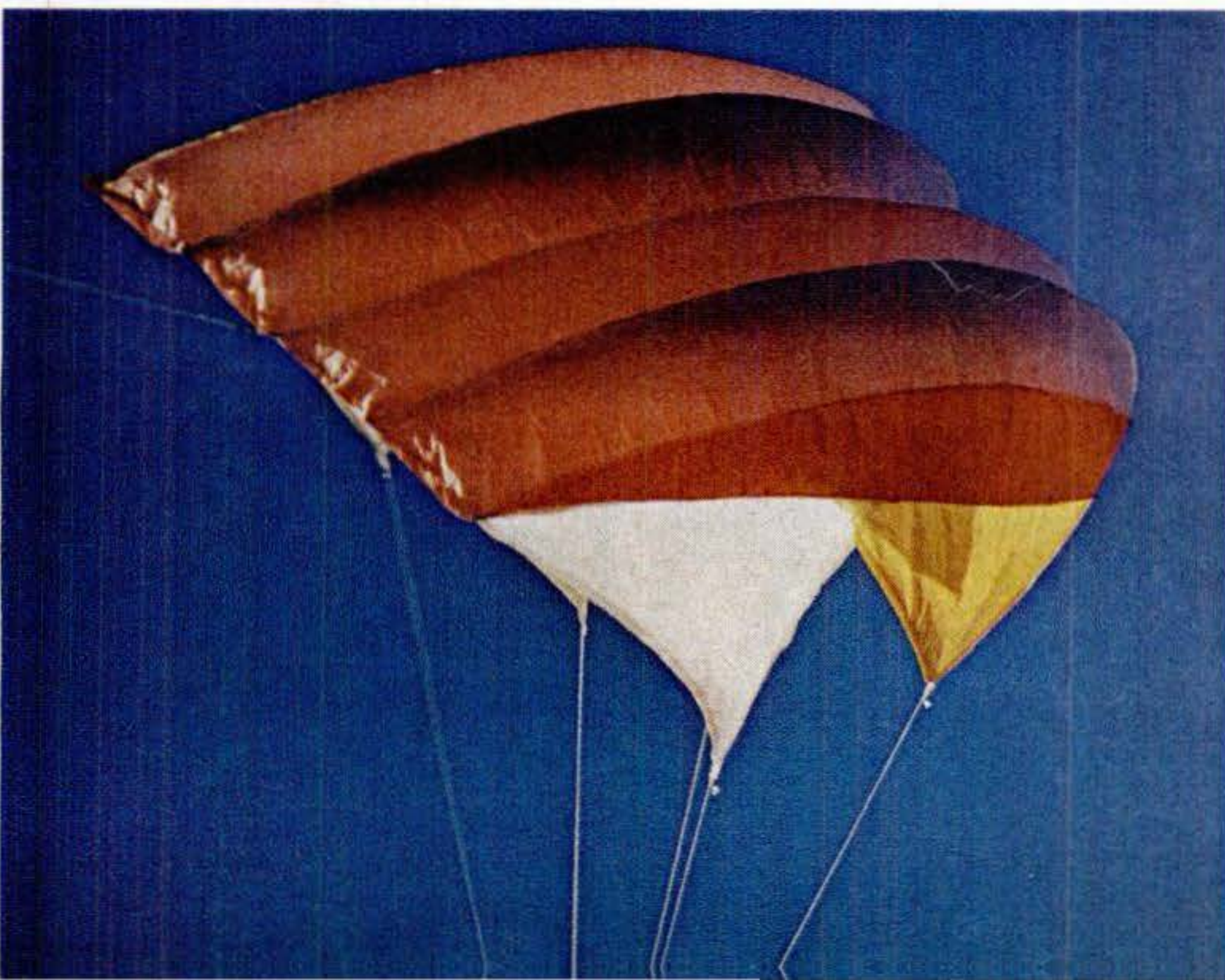
Domina Jalbert's Kytfoil is three-foot version of his famous big Airfoils used for atmospheric research and gliding parachutes. Open slots let ram air fill out sections to airfoil shape. Wind-sock tail cone (below) helps stabilize kite in strong gusts.
