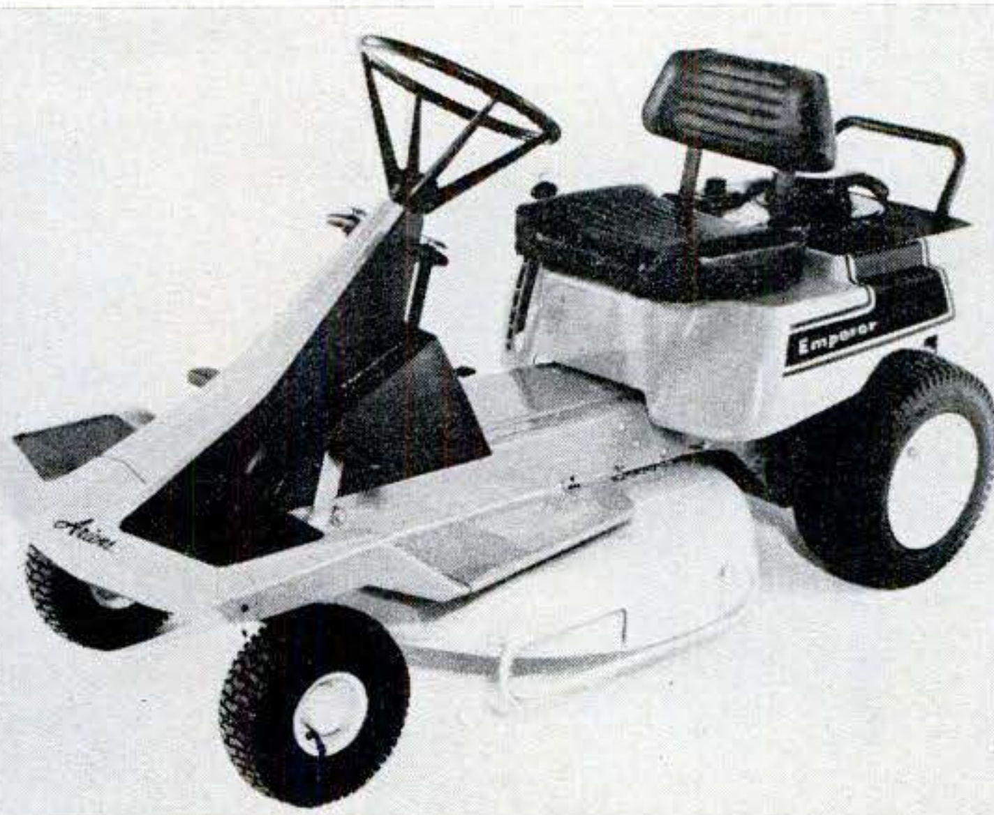
Sleekly styled Ariens encloses all mechanisms for looks and safety. Eight horses driving through six forward speeds cuts large lawns down to size. Controls, including separate clutch and brake, are easy to see and use. The Emperor II shown here has a built-in rear stand for easier servicing.
