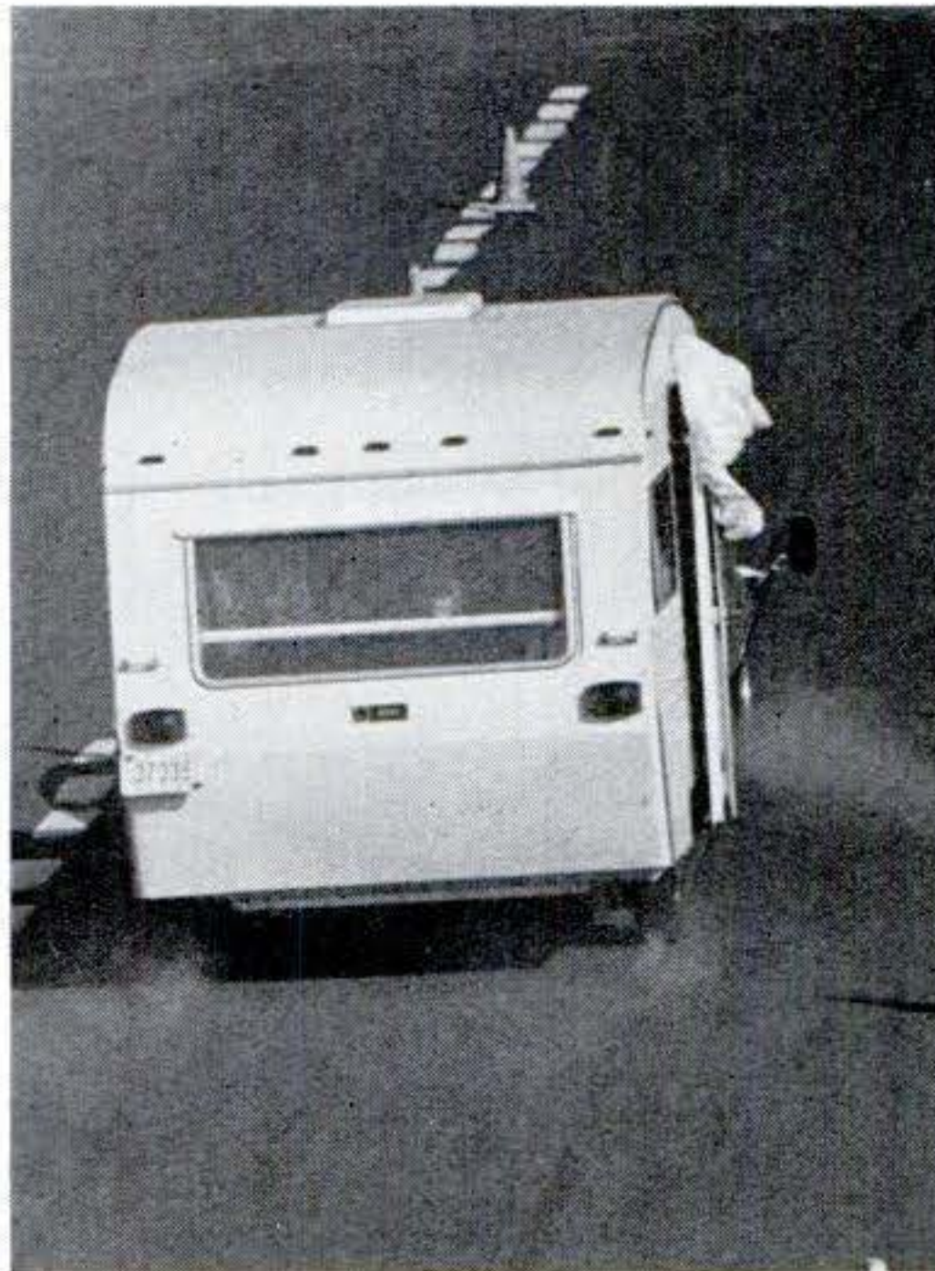
Vega/Sprite combination comes to a stop in brake test in 136 feet 10 inches, shortest stop of all rigs tested. Probable reason was the trailer's helping brakes.
