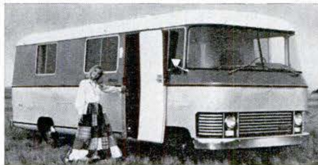
Revcon unit has a Toronado chassis with front-wheel drive. All-aluminum monocoque body of 25-foot RV lowers weight.
