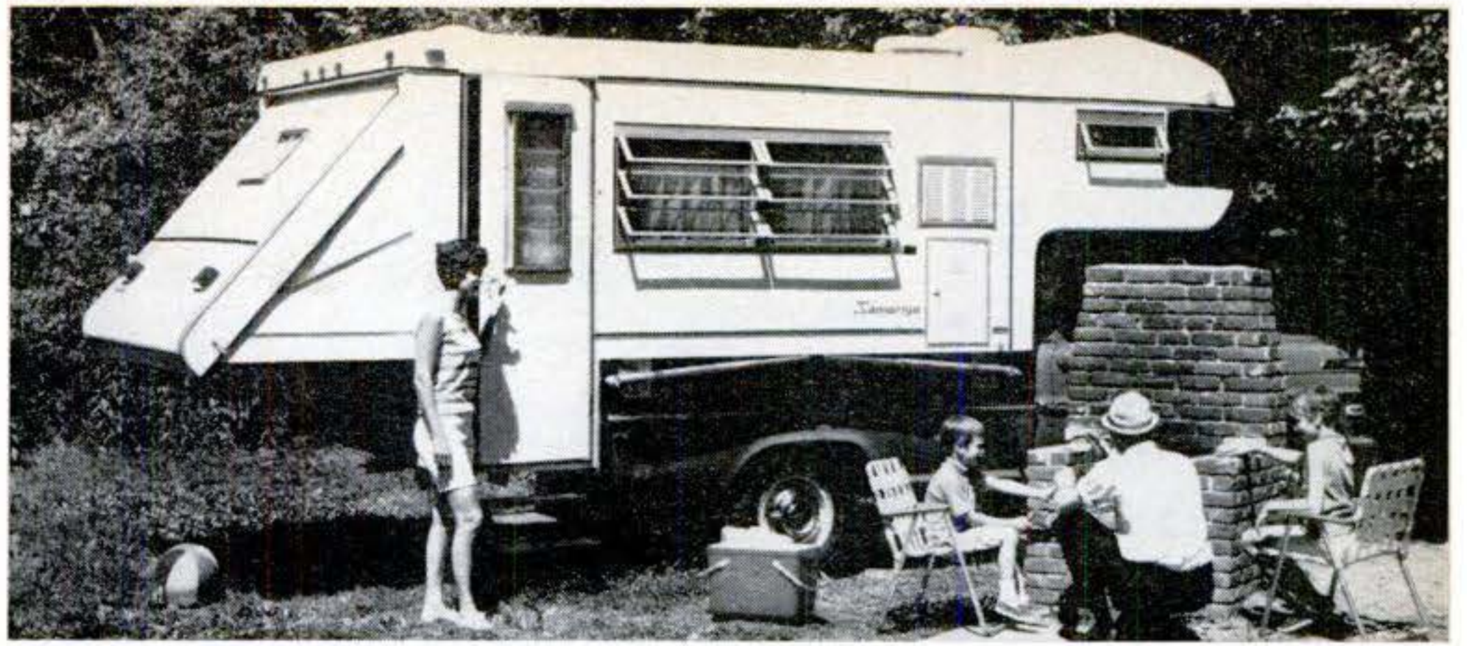
Amerigo camper uses camping-trailer design for extra sleep space: Bunk pops out
