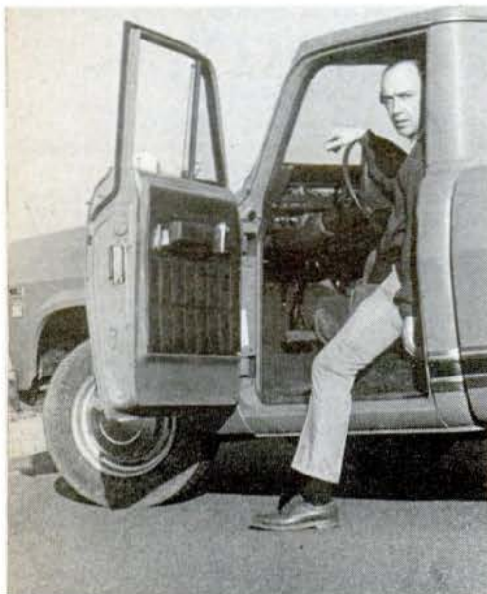
International has lowest step height with 16.5 inches (Dodge 18; Ford 19.25; and Chevrolet 20.5 inches).
