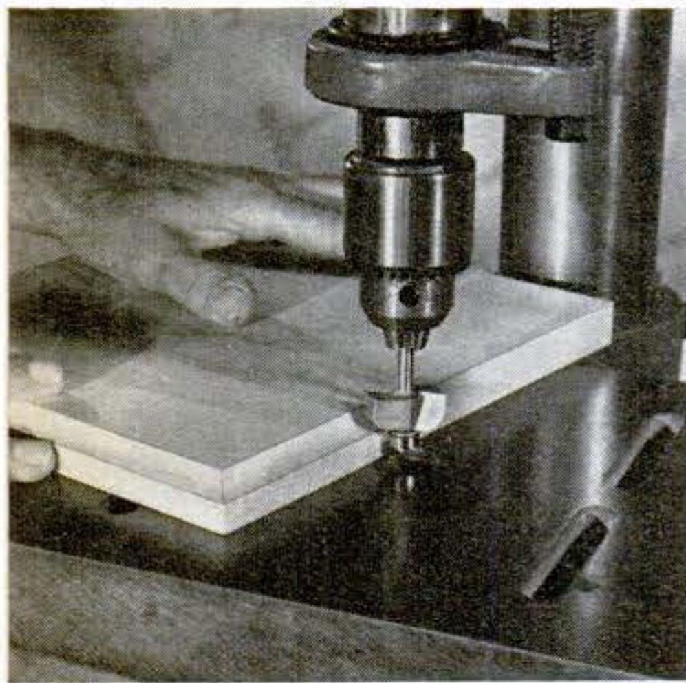
In a drill press, with slow rpm, super bits still do an impressive job. Ball-bearing pilot makes possible a slow feed rate.
