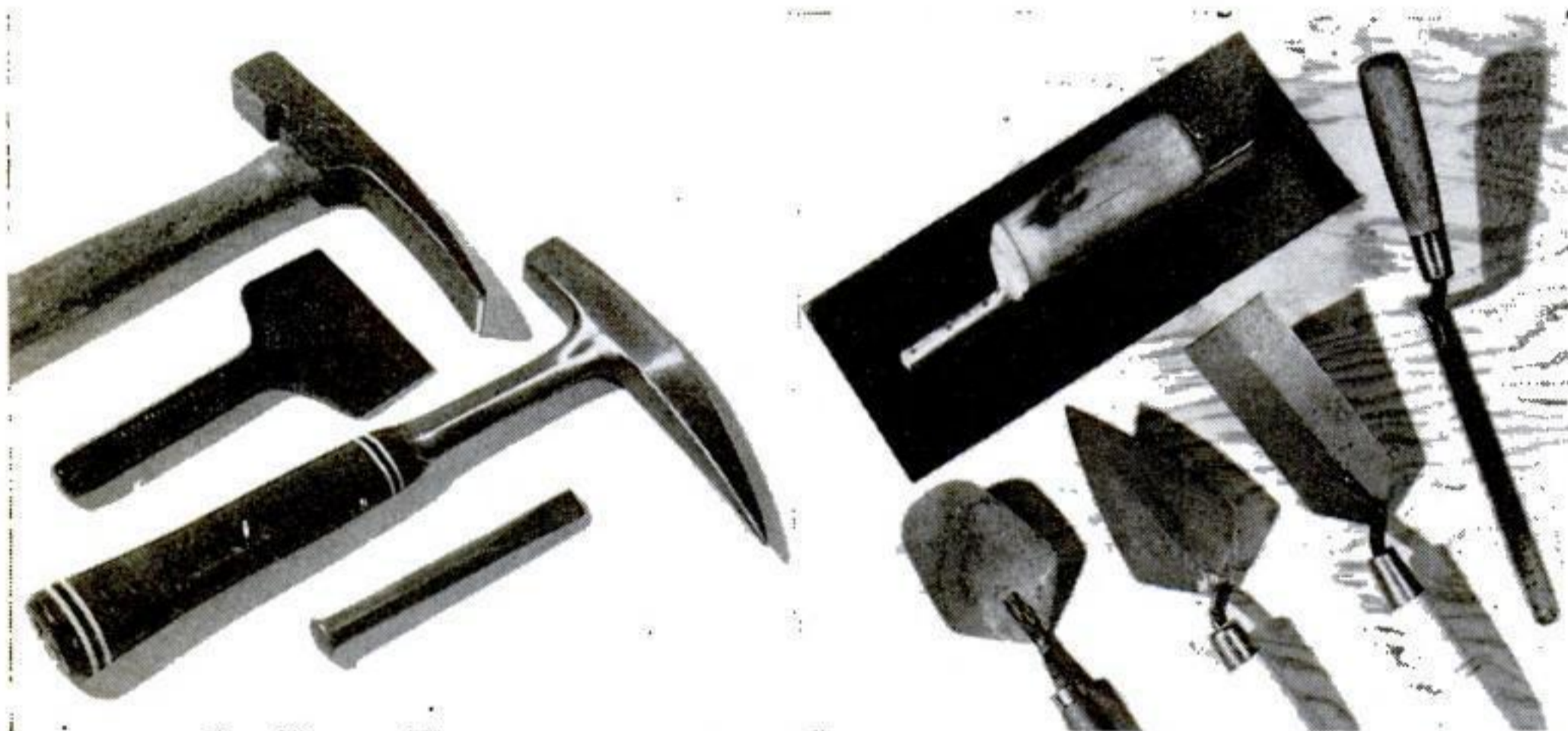
The tools: At left are mason's hammer, chipping chisel, prospector's pick, cold chisel. Above at right, plaster, round-end, small mason's, square-end, and tuck-pointing trowels.
