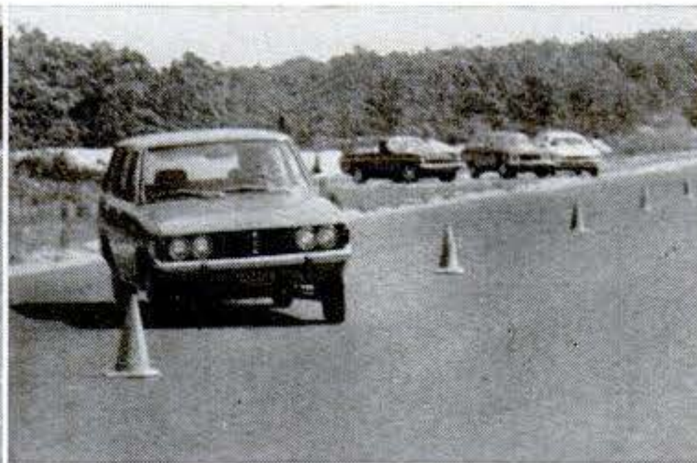
Colt in the slalom had the benefit of very light steering and ultra-rapid response, but handling accuracy was poor.
