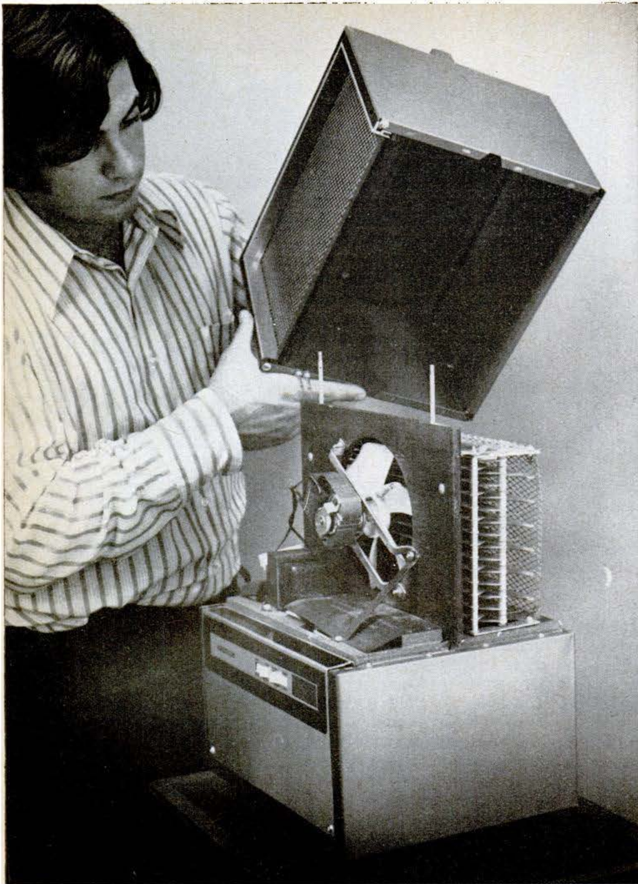
Cover lifts off Nautilus 777 portable to reveal electronic cell (right), detachable for
