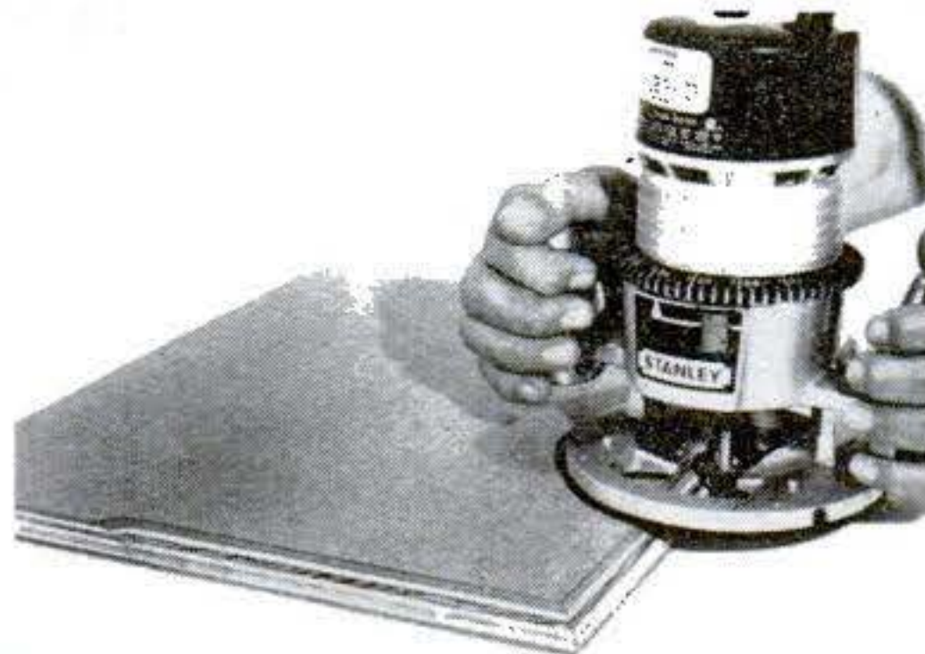
On hardboard-surfaced plywood, super bit produced this smooth, chipfree cut, ready for finishing without sandpaper touch-up.
