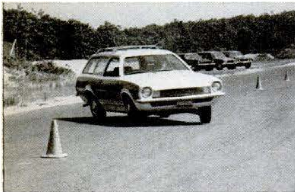
Pinto was fast in the low-speed slalom , but strong roll oversteer showed up, exaggerating the severity of the maneuver.
