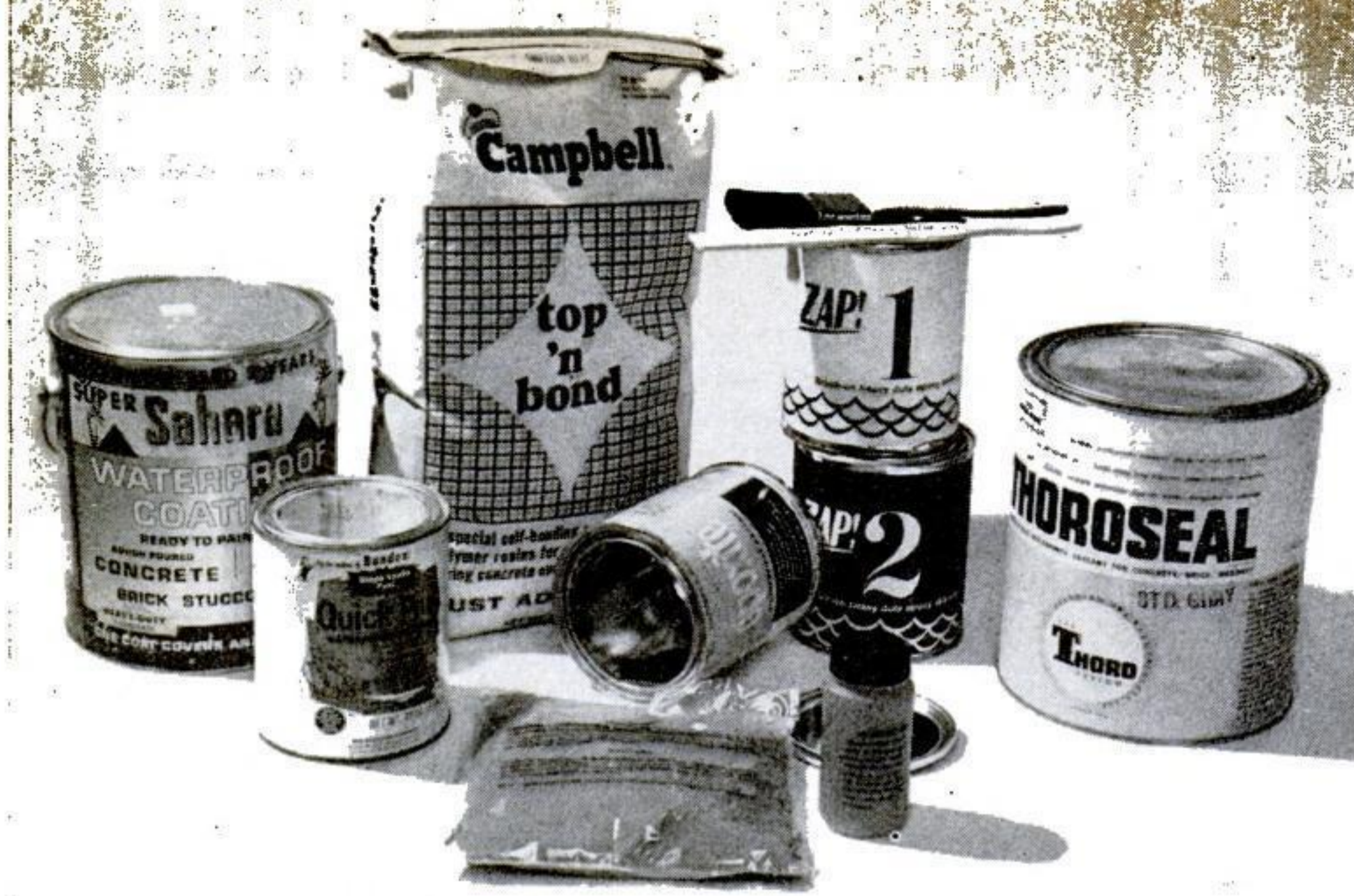
The materials (left to right): paint containing aggregates, hydraulic cement, cement formulated for small-volume setting, two epoxy coatings, cementitious paint.
