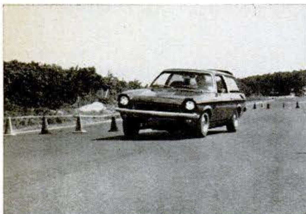
Vega in the lane-change test (top) matched Pinto (above) for speed, but was hampered by the progressivity of its variable-ratio steering, plus strong initial understeer. The Pinto went through with large slip angles on all four wheels. Steering effort was high.
