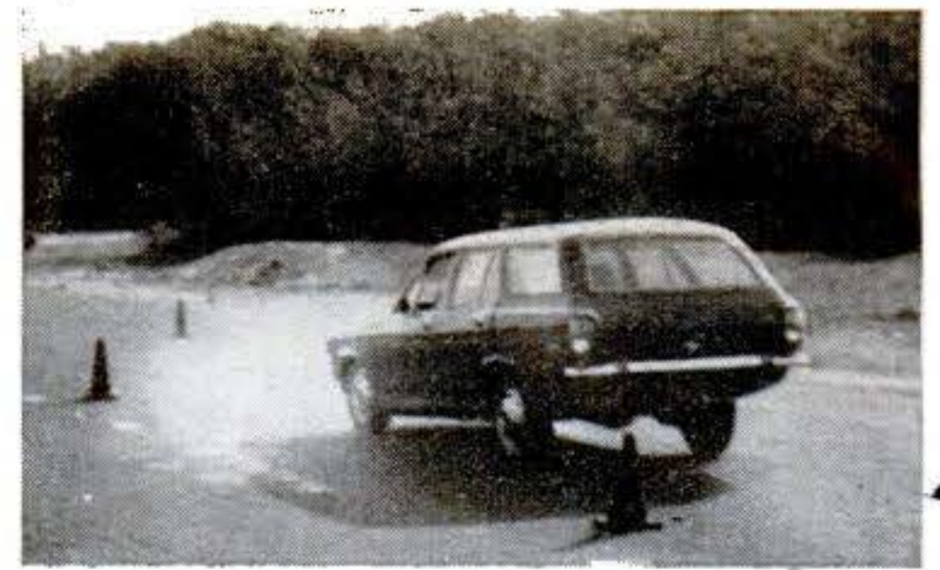
Cricket's brakes worked fine , but its narrow tires stretched stopping distances. Fade resistance was very strong.
