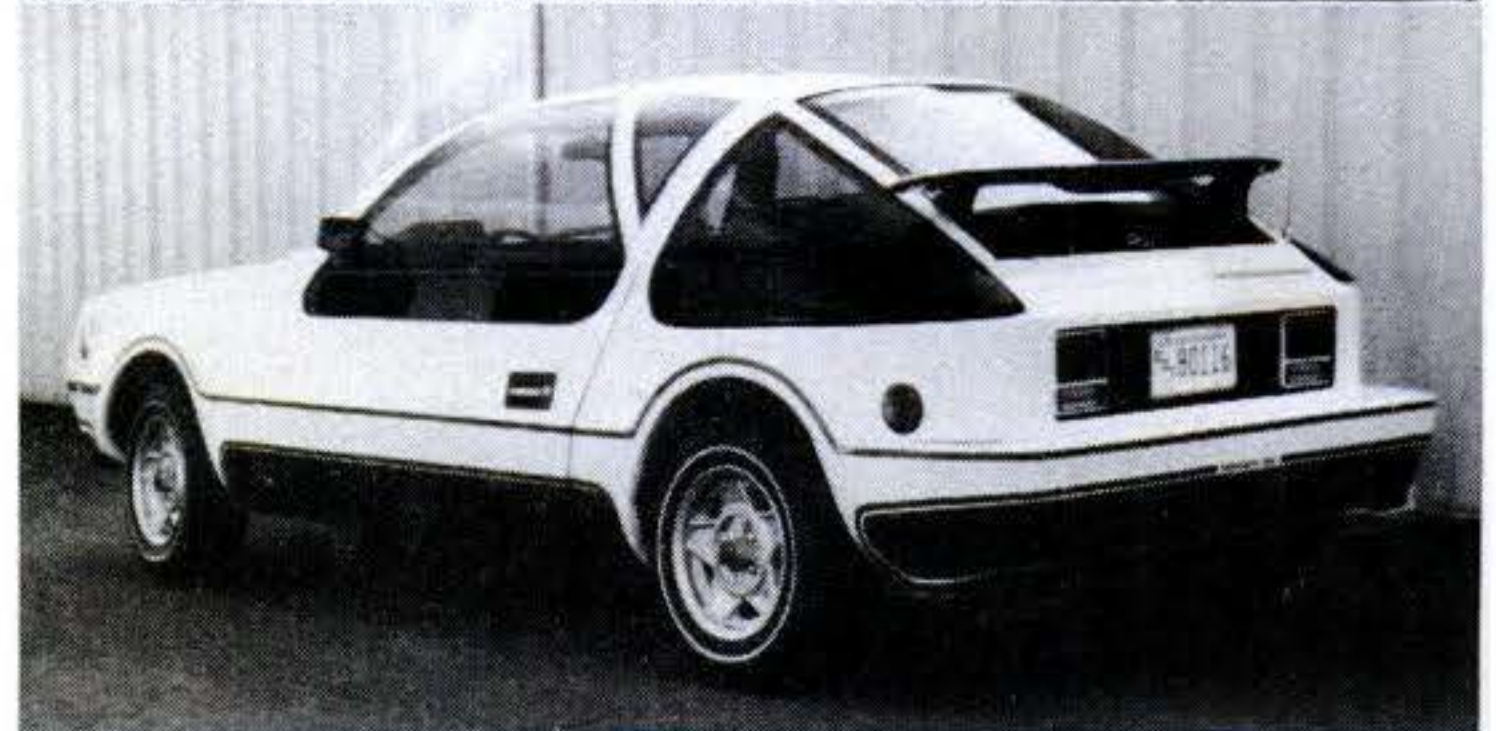
High-technology Minicars RSV has modified rear end in this version. Spoiler has been added to improve aerodynamics. It's a rear-engine, rear-drive car, and weighs about 2500 pounds.
