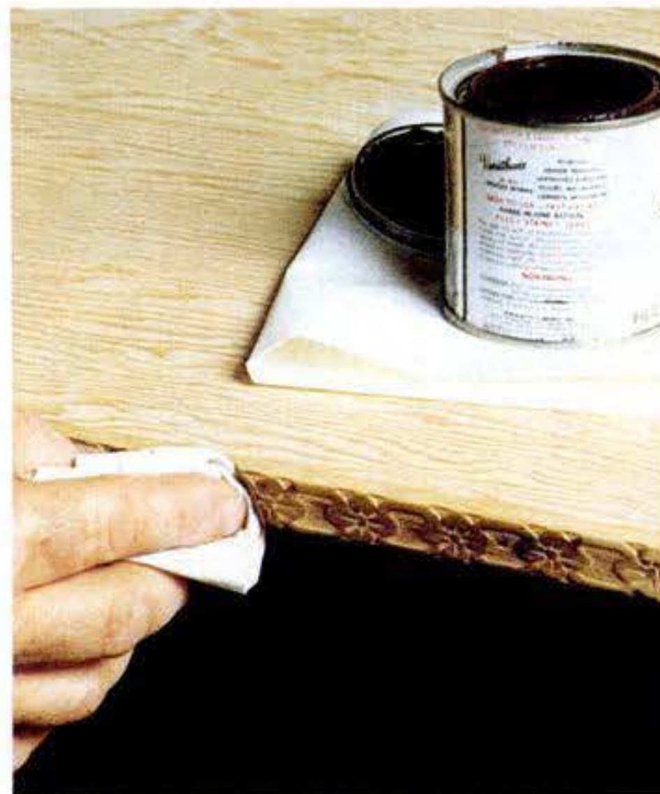
Decorative molding can be stained to match the surface, for a carved effect.
