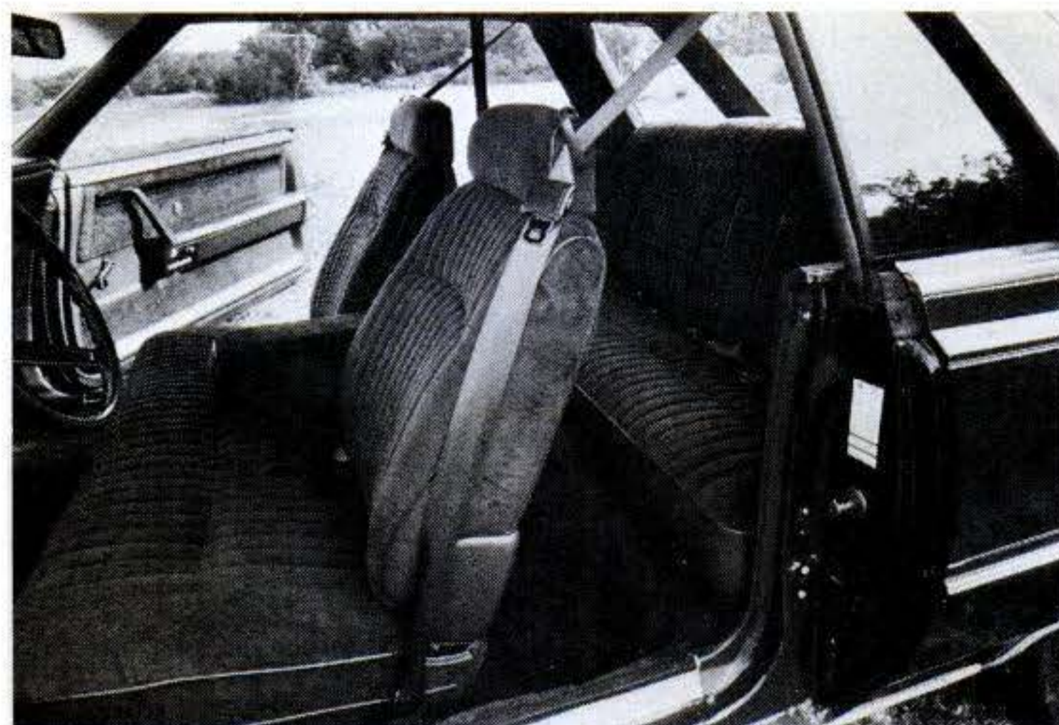
Unusual stagger of inside, outside door edges narrows rear-seat access on Cordoba (shown) and Mirada.
