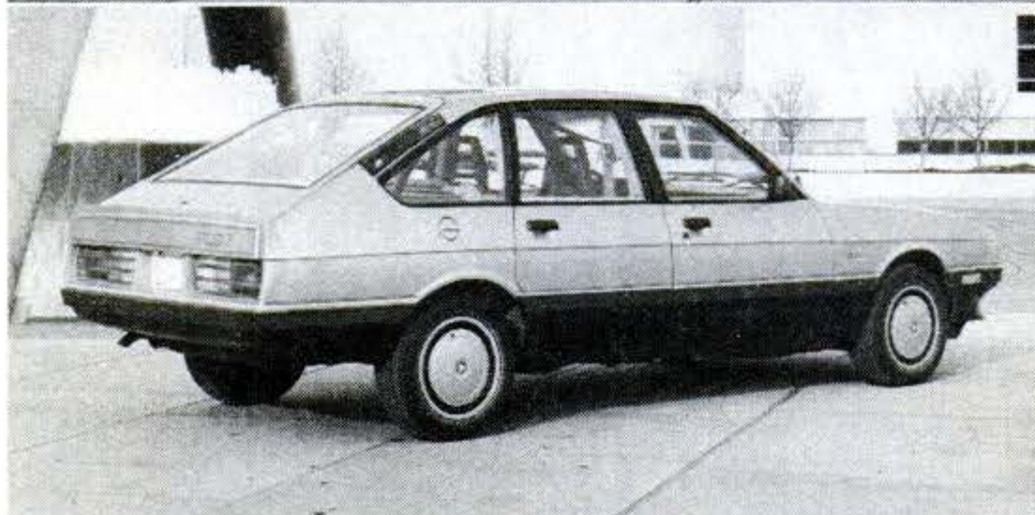
Calspan RSV doesn't look any different than most cars on the road now. It's actually a modified Simca 1308 with Omni/Horizon engine and drive trains. This RSV weighs 2675 pounds.
