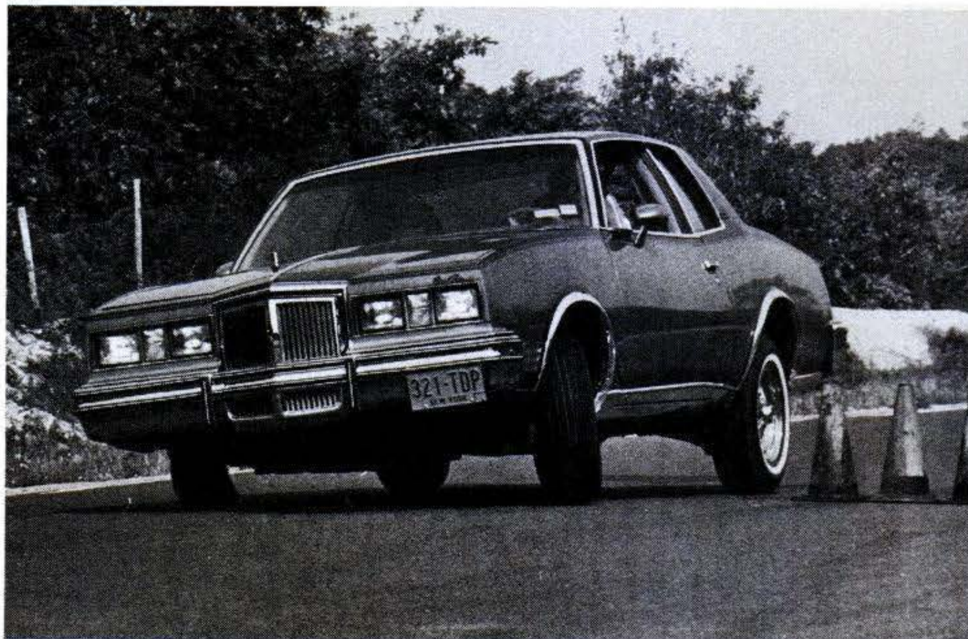
Grand Prix negotiates slalom course. With smallest front antisway bar, and none in the rear, its handling and maneuverability weren't quite up to others'.
