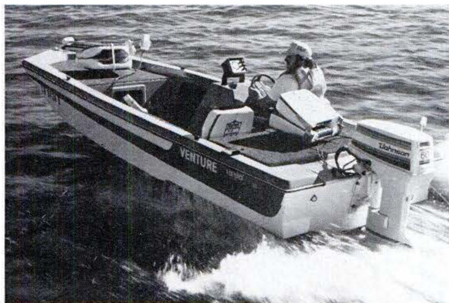
Johnson 60-hp model has same displacement (44.99 cu. in.) as last year's 55-hp model. The new design, with closer piston fit and better shaping of ports, boosts horsepower.
