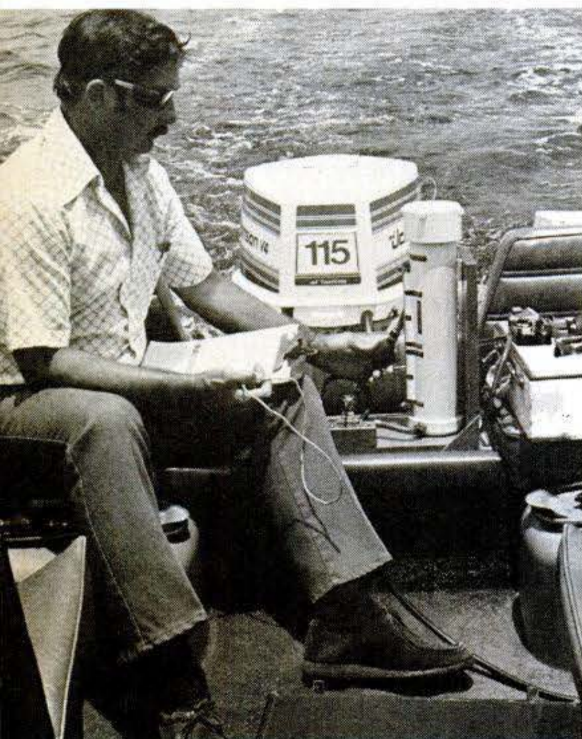
Testing Johnson's new 115-hp model, author Bob Stearns runs a fuel-economy check. New primer system allows easy rope starting in \frac{1}{3} flywheel revolution.
