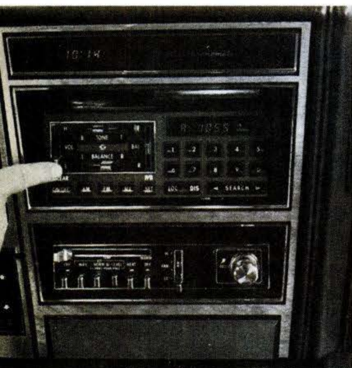
Mirada's electronically tuned radio proved easy to use, but speakers made dash vibrate, ruining sound quality.
