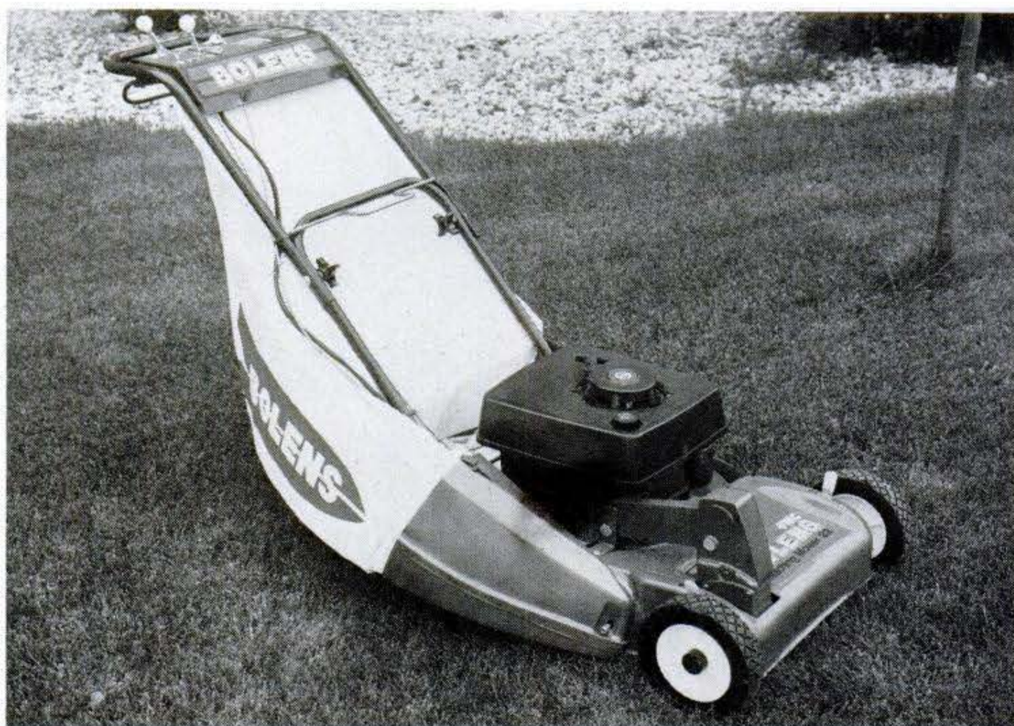
Attachments for conversion to side- or rear-baggers are offered on some mulchers.
