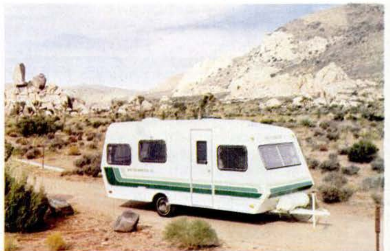
Most radical weight-shrinking effort was accomplished by Fleetwood Enterprises for this Wilderness II 19-foot travel trailer. It weighs just 1650 pounds—half the weight of standard units.
