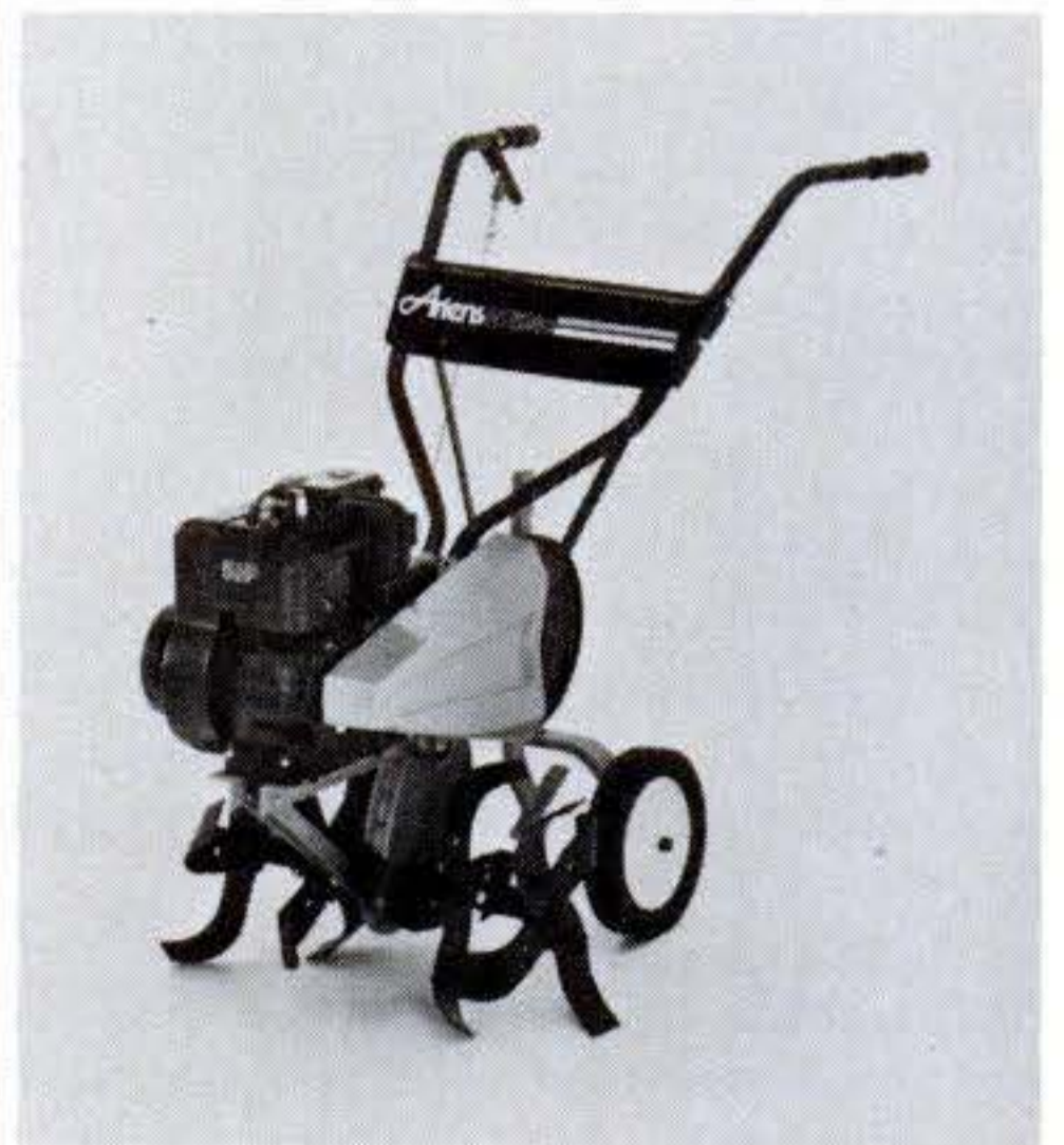
Ariens front-tine tiller has 14-in.-dia. tines and a seven-in. tilling depth.
