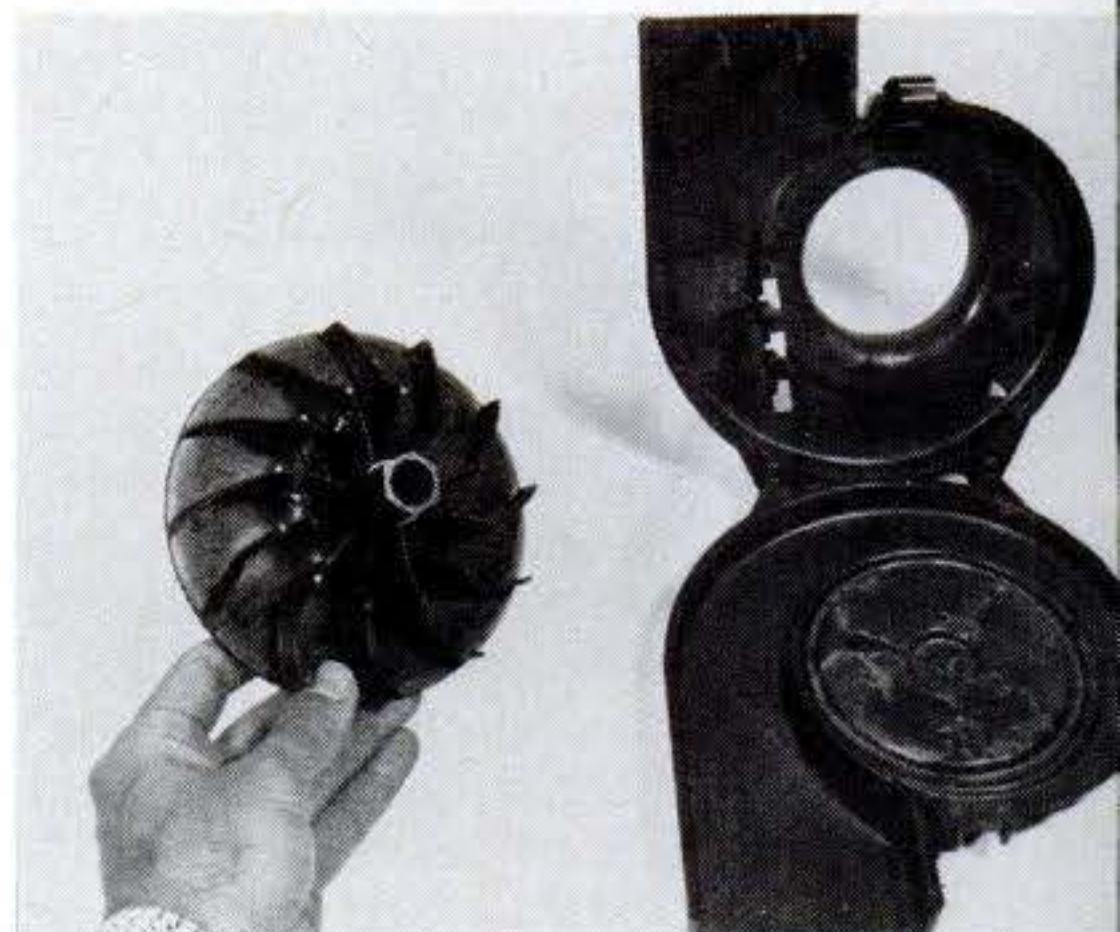
Axial fan-type blower (above) slips onto Homelite ST-100 cutter (top), producing a 100-mph airstream that whisks away clippings, leaves, and even light snow. The blower is a $20 option.
