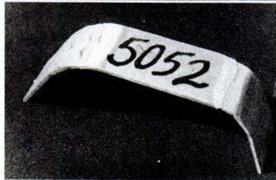
Not the prettiest joints , but the 5052 butt and V-joints stand up to a 90-degree bend—as strong as the parent metal.
