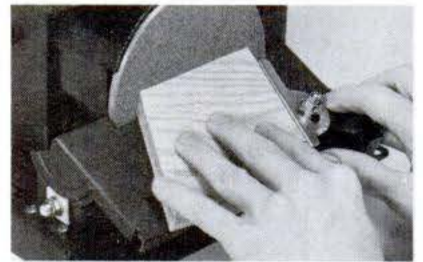
Large tilting table, adjustable miter gauge for sanding accurate angles.
