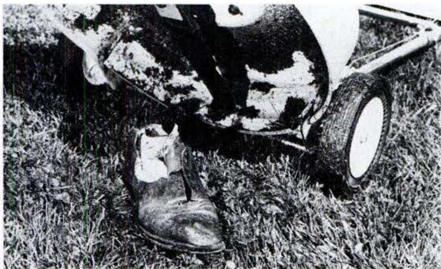
Running over this shoe several times with rubber blade did not produce slashing and shredding typical of damage caused by a metal blade. You can see a dent in the toe.
