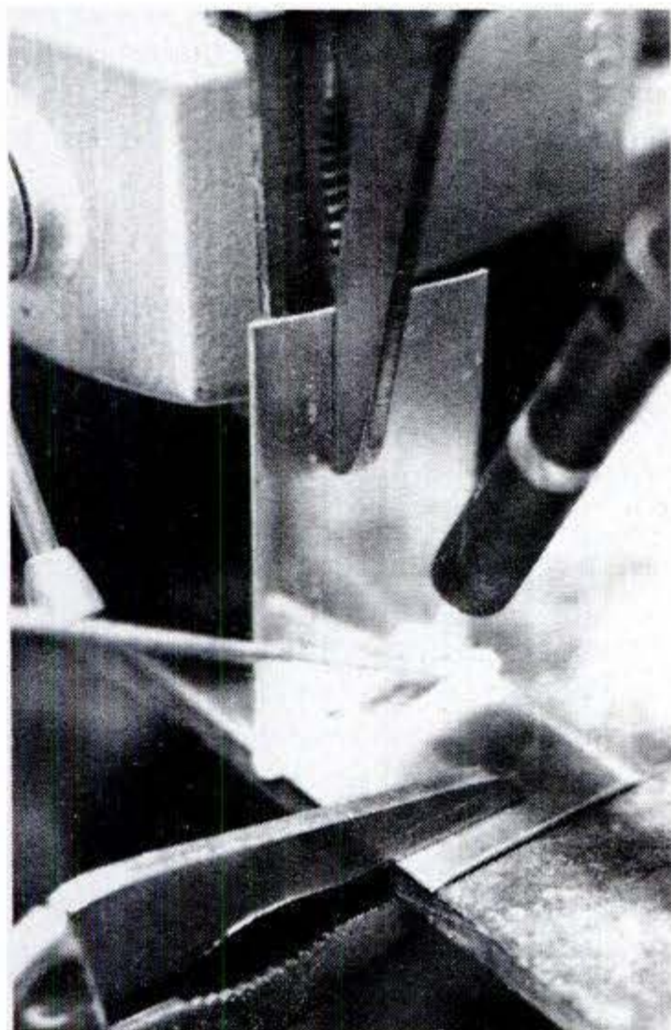
2024 aluminum can't be welded with conventional methods; Lumiweld can do it.
