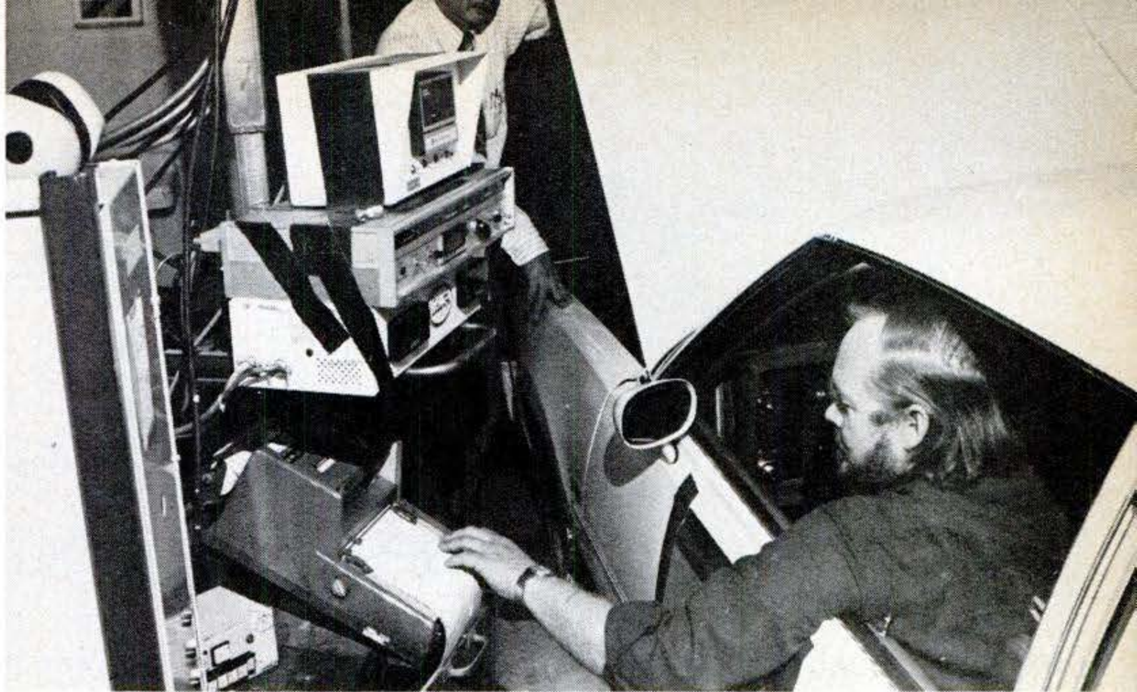
EPA's Peter Hutchins (rear) watches as technician runs car fitted with gas-saving device through standard EPA fuel-economy and emissions cycle on dynamometer.
