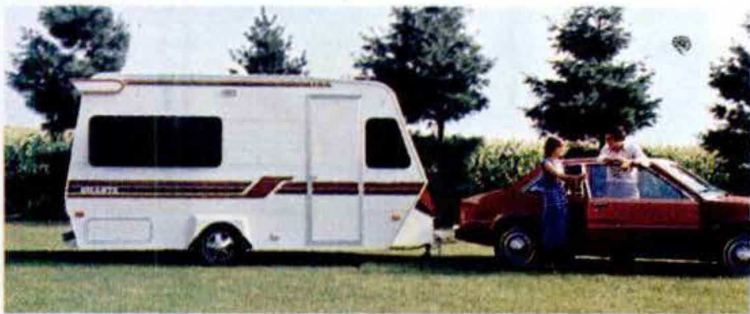
New lightweight 16-footer is Shasta's Ultra. A lighter, high-strength frame and new materials help keep its weight to 1395 pounds. Base price ranges from $3525 to $3695.
