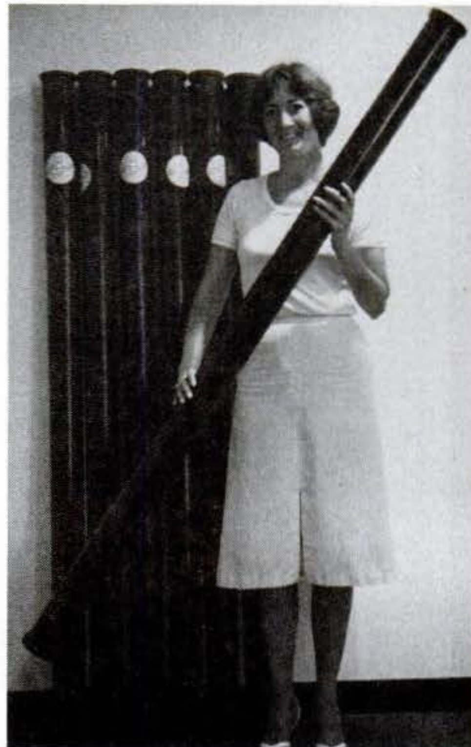
Phase-change salt is sealed inside PSI's 6'-long, 3½"-dia. polyethylene tubes (photo). Drawing (right) shows typical storage container for an average home. Drawings below show how tubes could be used in passive/active solar applications.
