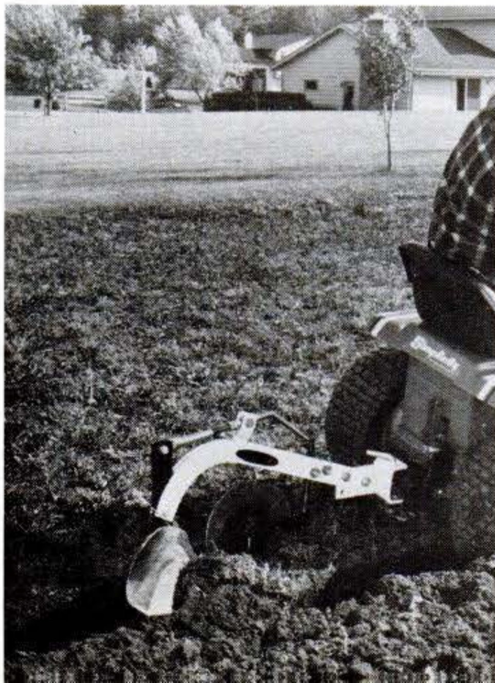
Ariens front-tine tiller has 14-in.-dia. tines and a seven-in. tilling depth.
