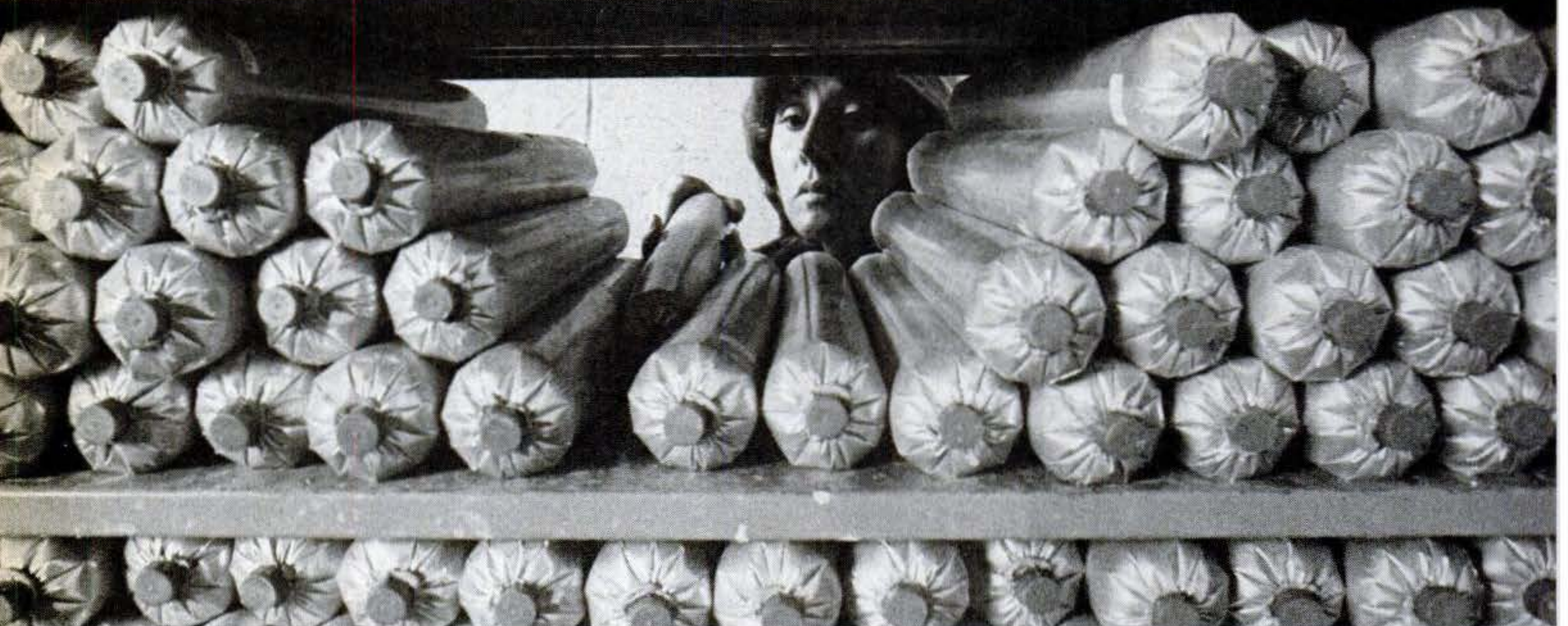
Salt sausages: University of Delaware borrowed technology from food-processing industry to develop low-cost polyester package.
