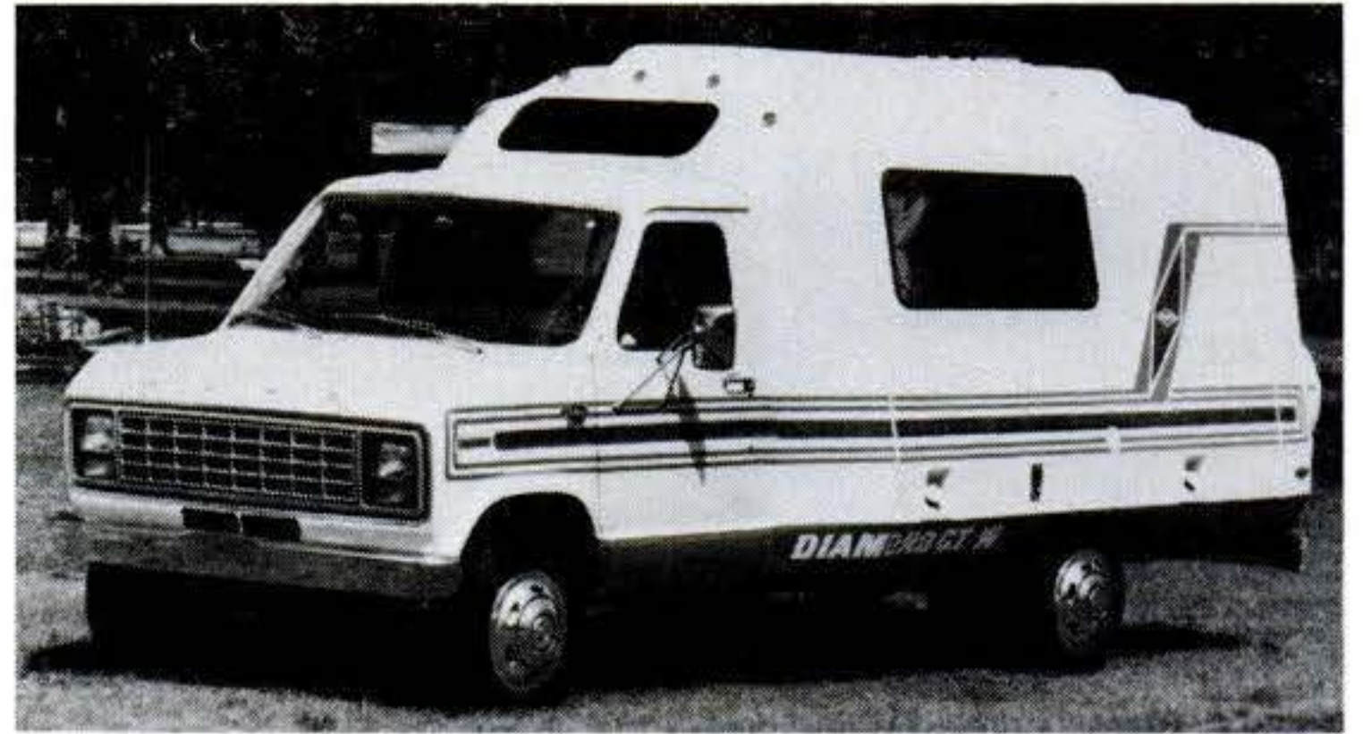
Honeycomb construction in Diamond's 20-foot GT Mini Home shell cuts weight by about 20 percent. Base price: $14,500.
