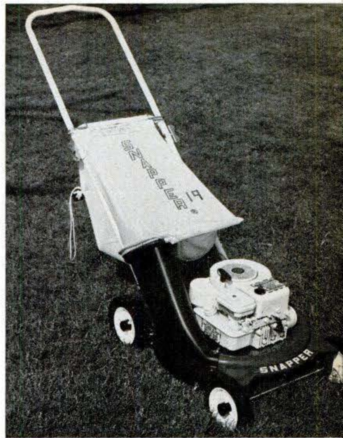
Options on Snapper's 19-in. mowers include two- or four-stroke engine, mulching adapter, and "Snapperizer," a converter to vacuum and shred leaves.
