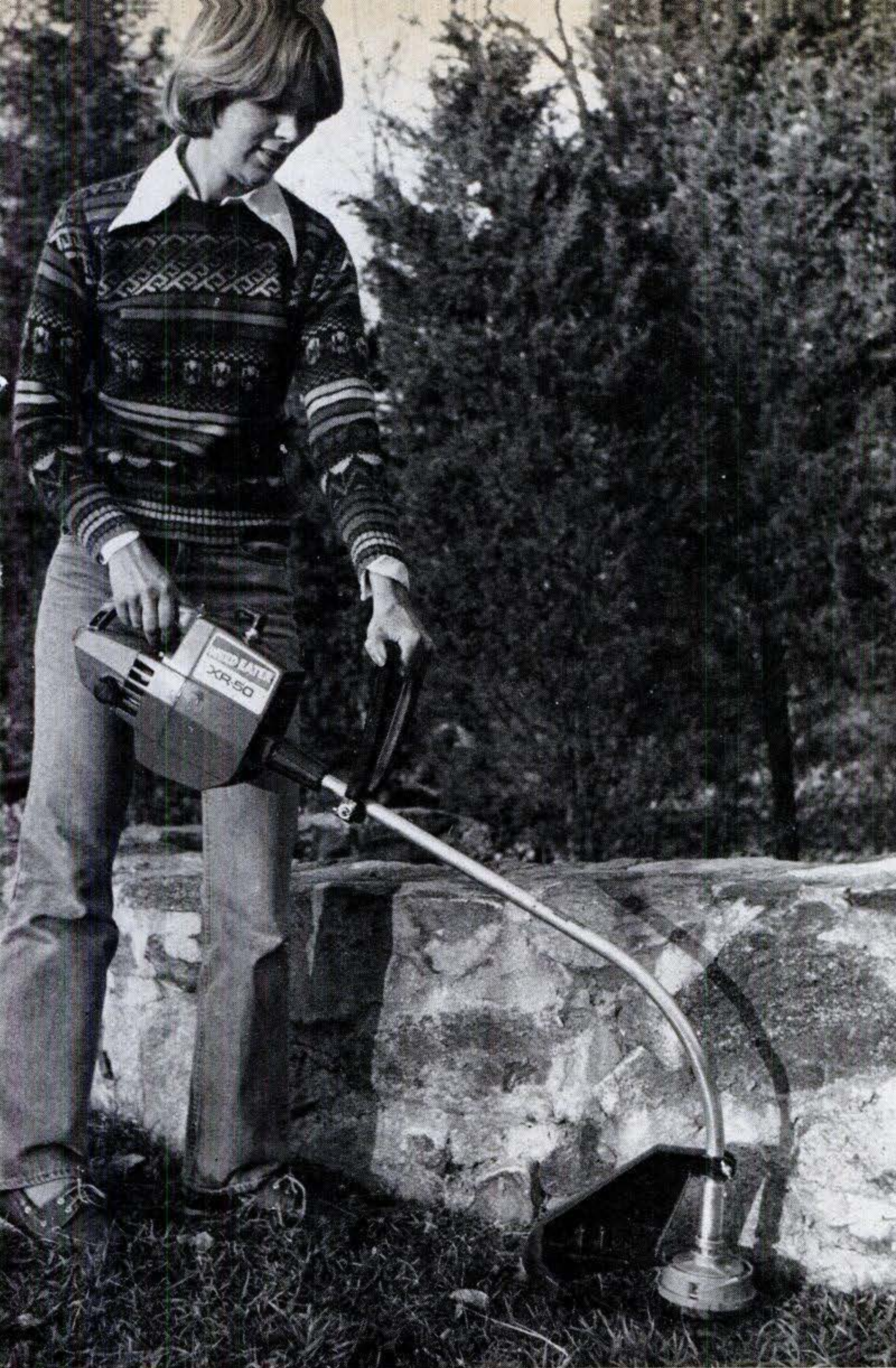
Toro 14-cc trimmer (above) has a smooth-running Kioritz engine designed especially for trimmers. The machine cuts a 12-inch swath with dual-line cutting head. One of five new gas-powered trimmers from Toro, it sells for $180. This is Toro's first year in the gas-trimmer market.
