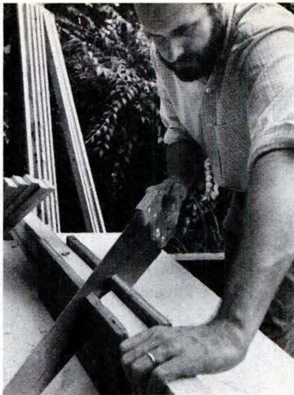
A sawing jig or miter box allows uniform cutting of four or five stacked slats. Here, eight-ft. furring is cut to six-ft. lengths, leaving two-footers for slatting of bin.
