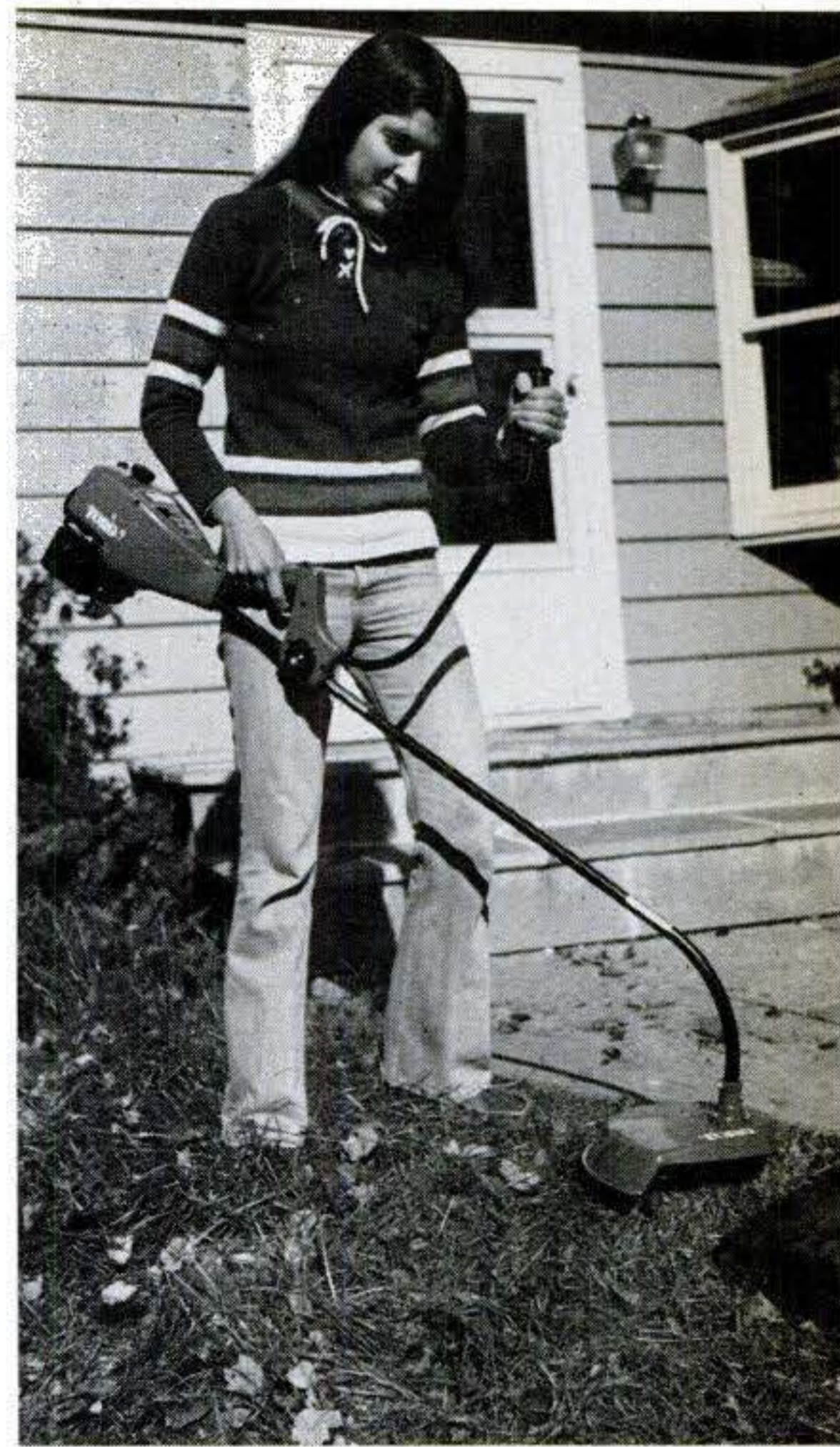
Toro 14-cc trimmer (above) has a smooth-running Kioritz engine designed especially for trimmers. The machine cuts a 12-inch swath with dual-line cutting head. One of five new gas-powered trimmers from Toro, it sells for $180. This is Toro's first year in the gas-trimmer market.
