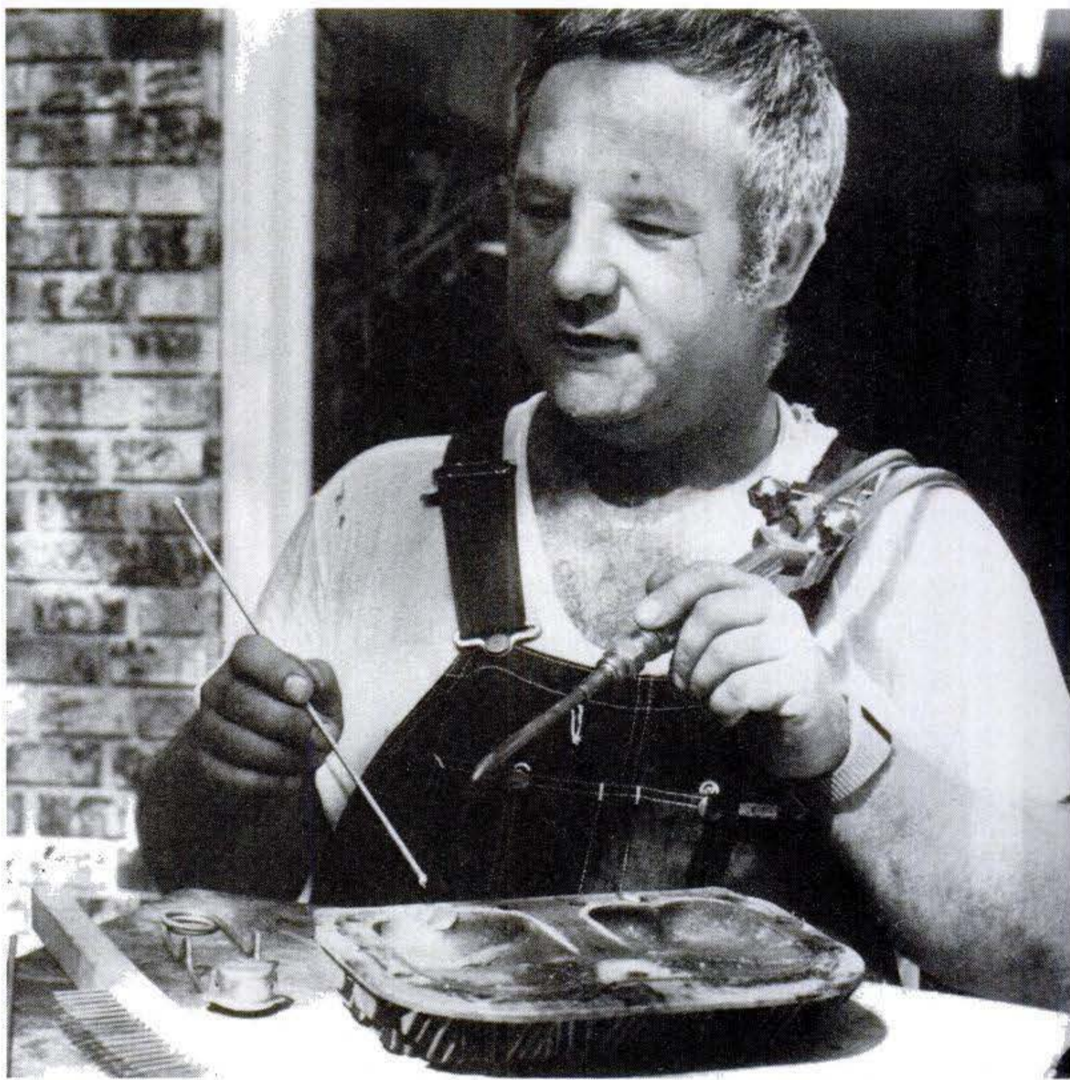
Jim Hille demonstrates his Lumiweld process on casting using oxygen-aided torch.
