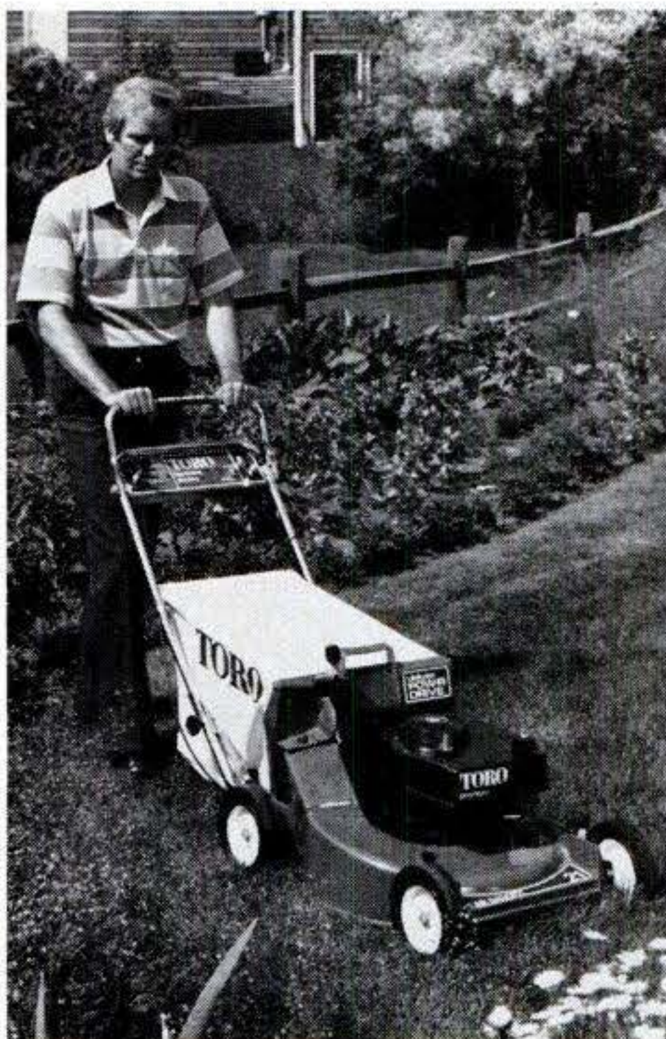
Electric start on Toro rear-bagger is safe and convenient, which should make users more willing to stop engine for blade checks without fearing restart hitches.
