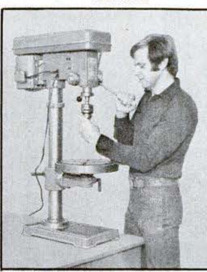
Precision ground quill has milled rear rack
