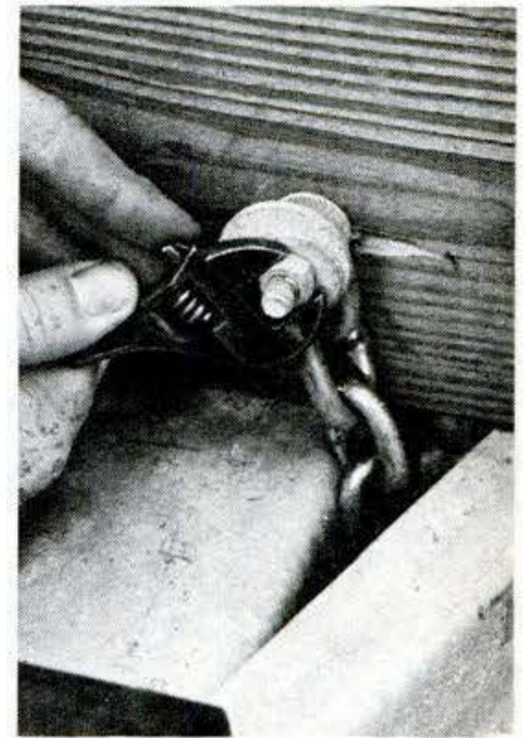
Strong safety chain is looped around the trailer tongue and bolted to the frame.
