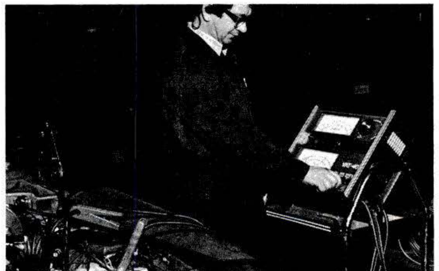
Inductive ammeter with a variable-control carbon pile, such as Sun's VAT 40 shown here, tests charging system.
