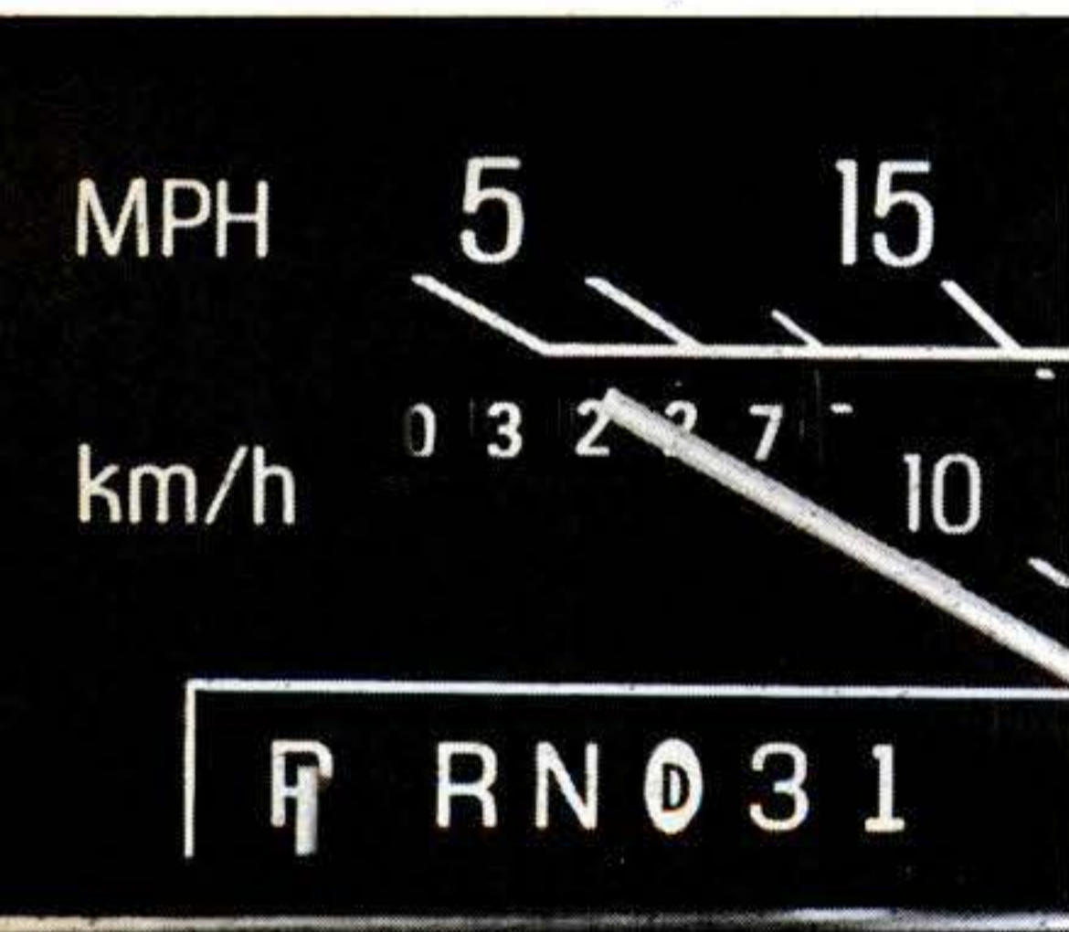
LTD's unusual shift quadrant markings: Overdrive range is available in the "OD" position, but it's locked out in "3" for hill climbing and around-town driving.
