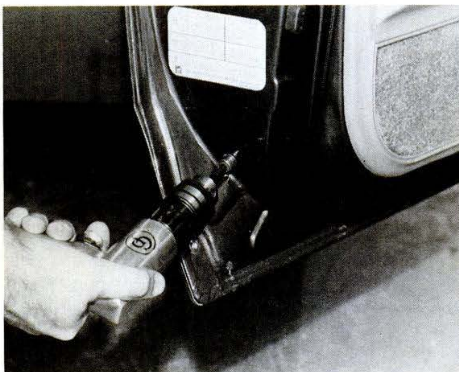
Drilling holes in a car door (above), then shooting in the rust-proofing compound (right), allows the thick gunk to creep into
