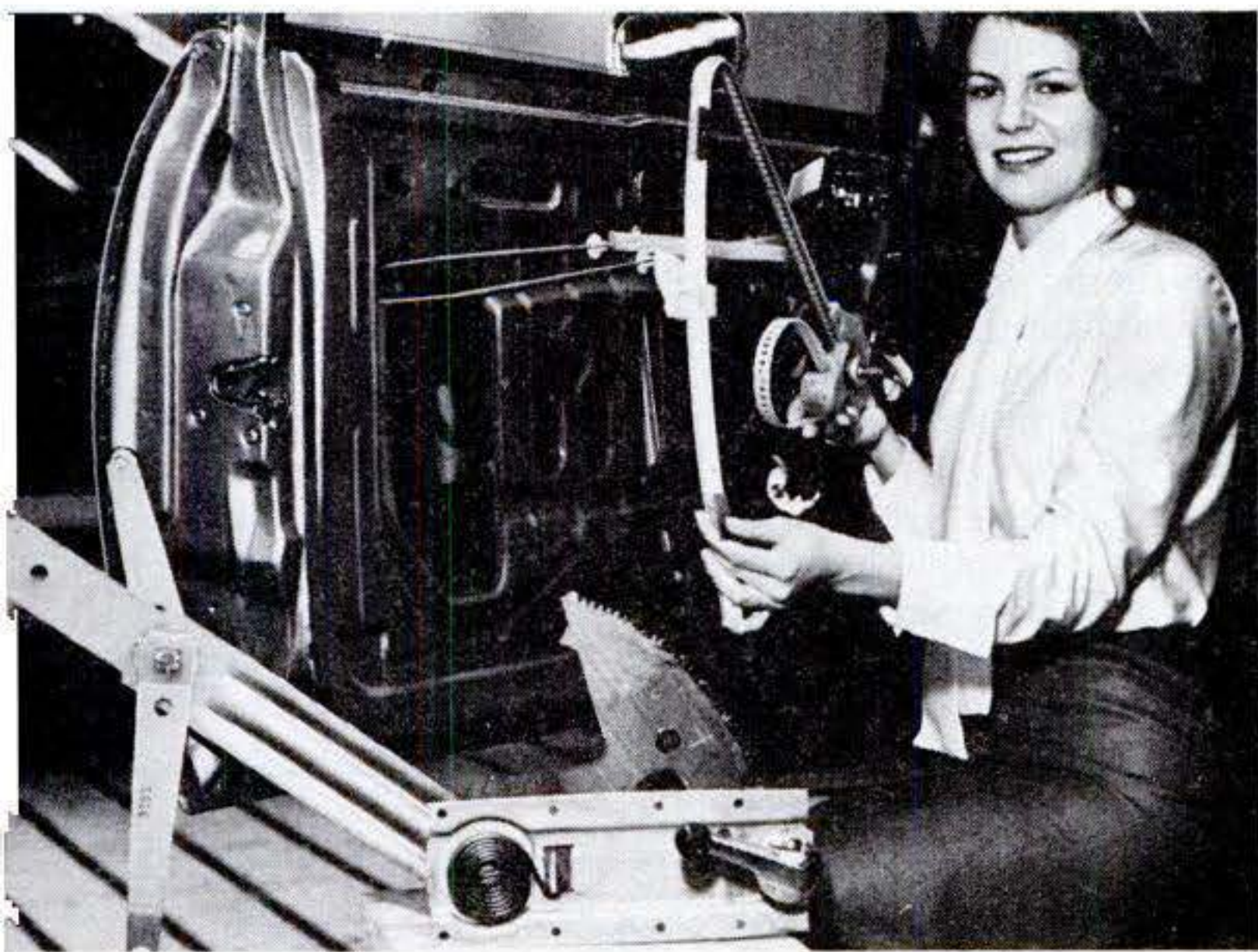
Complicate the rustproofing job. Door panels must now be removed on many cars, and the window-crank systems must be protected.
