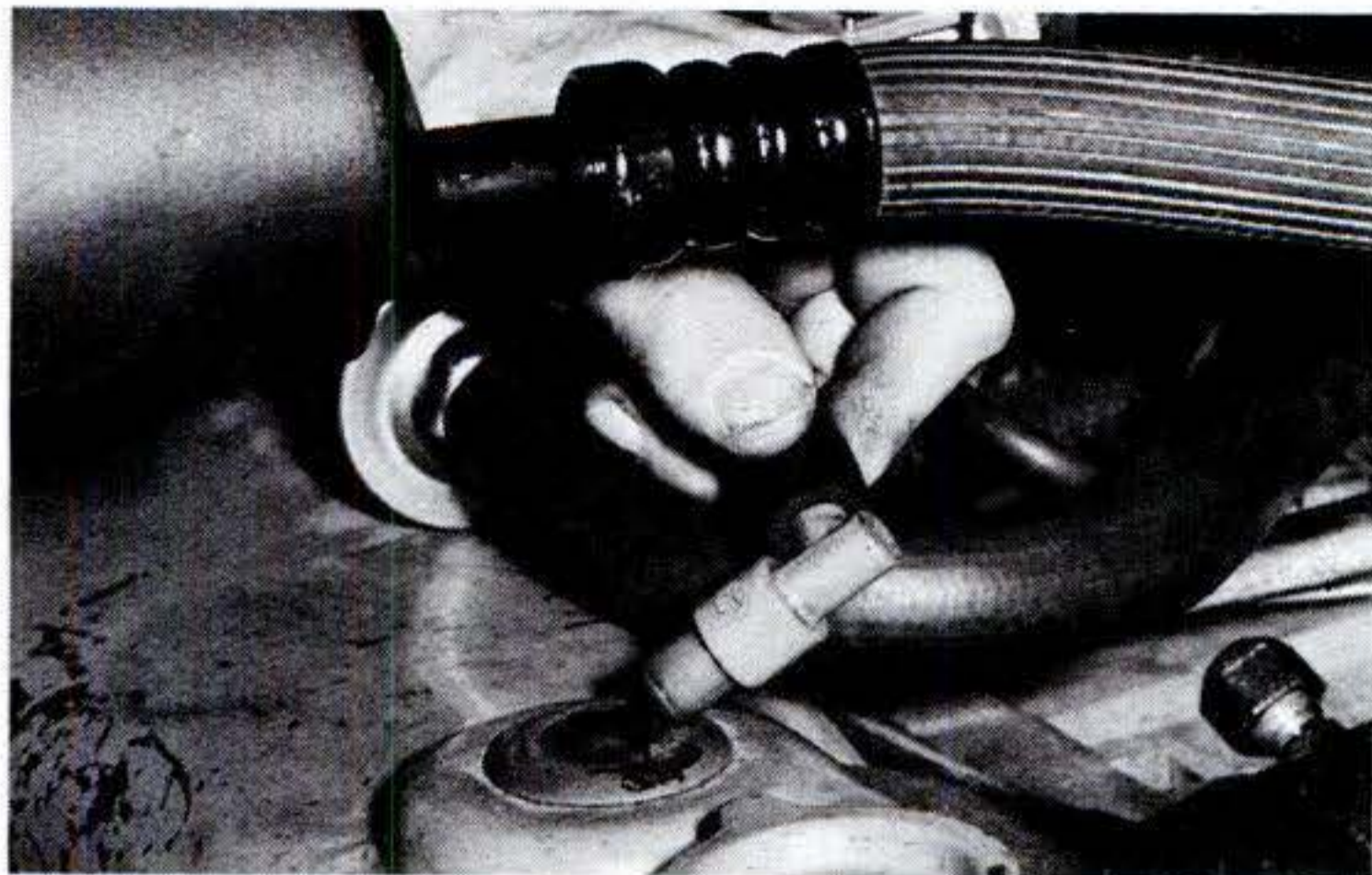
PCV valve is in the valve cover. It should fit tightly, both at its hose connection and in the valve-cover grommet.
