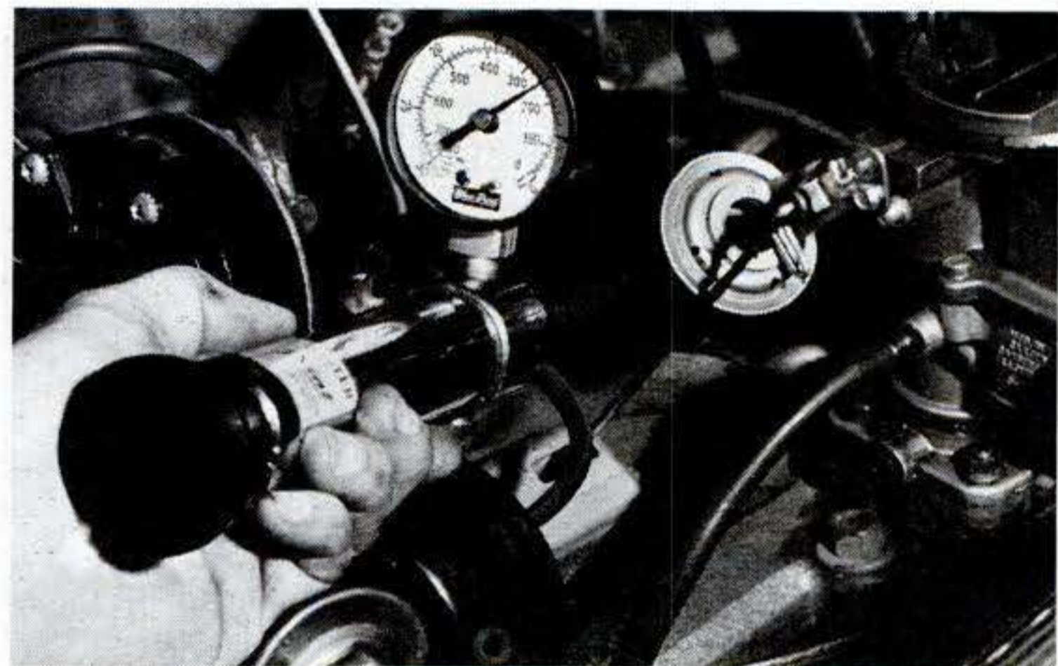
Vacuum pump is used to check the choke pull-off. A leaking choke pull-off must be replaced. It can't be repaired.
