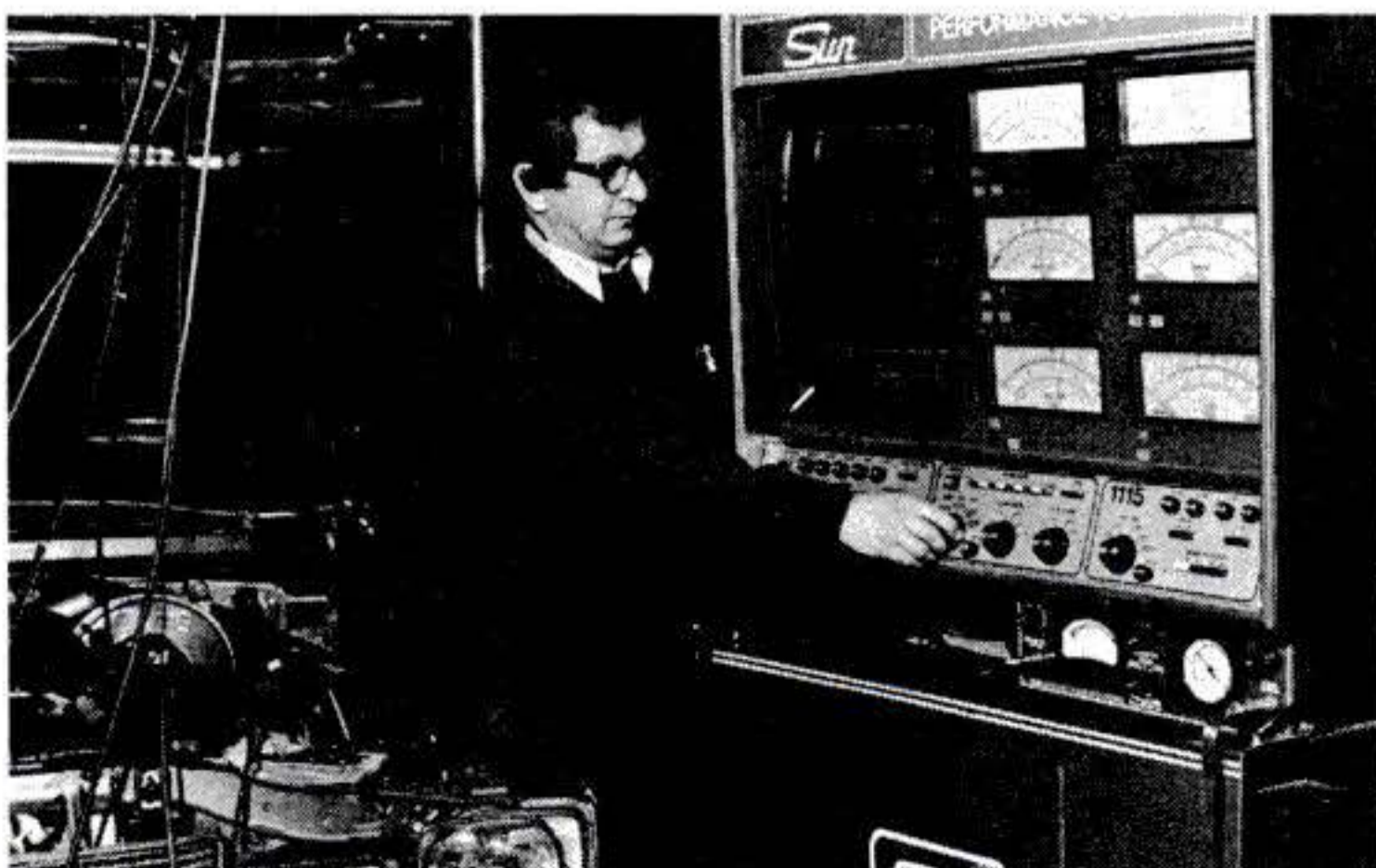
Professional mechanic Steve Mercaldo at the controls of what a pro might use to tune your car—Sun's 1115 analyzer.
