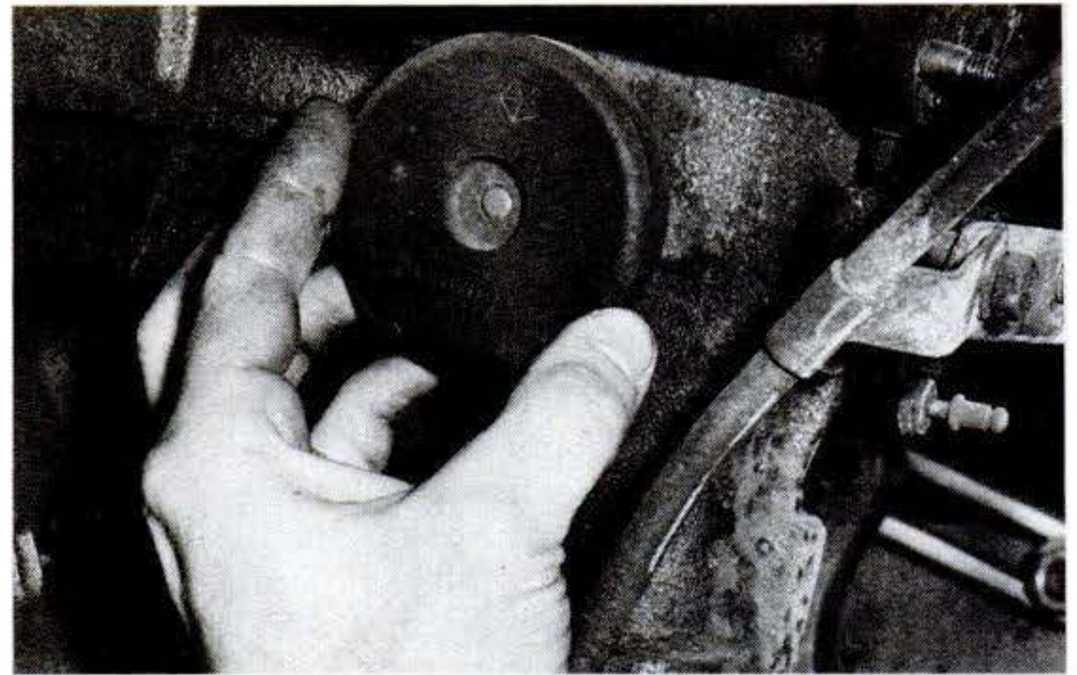
Manifold heat-control valve should move freely when you try to rotate it by hand. Don't touch it when it's hot.
