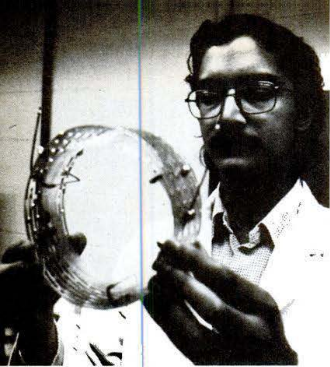
Coiled tube is the heart of apparatus used to detect amino acids in Antarctic meteorites (see text). Gas-liquid chromatography tube is operated inside an oven to maintain a precise temperature.
