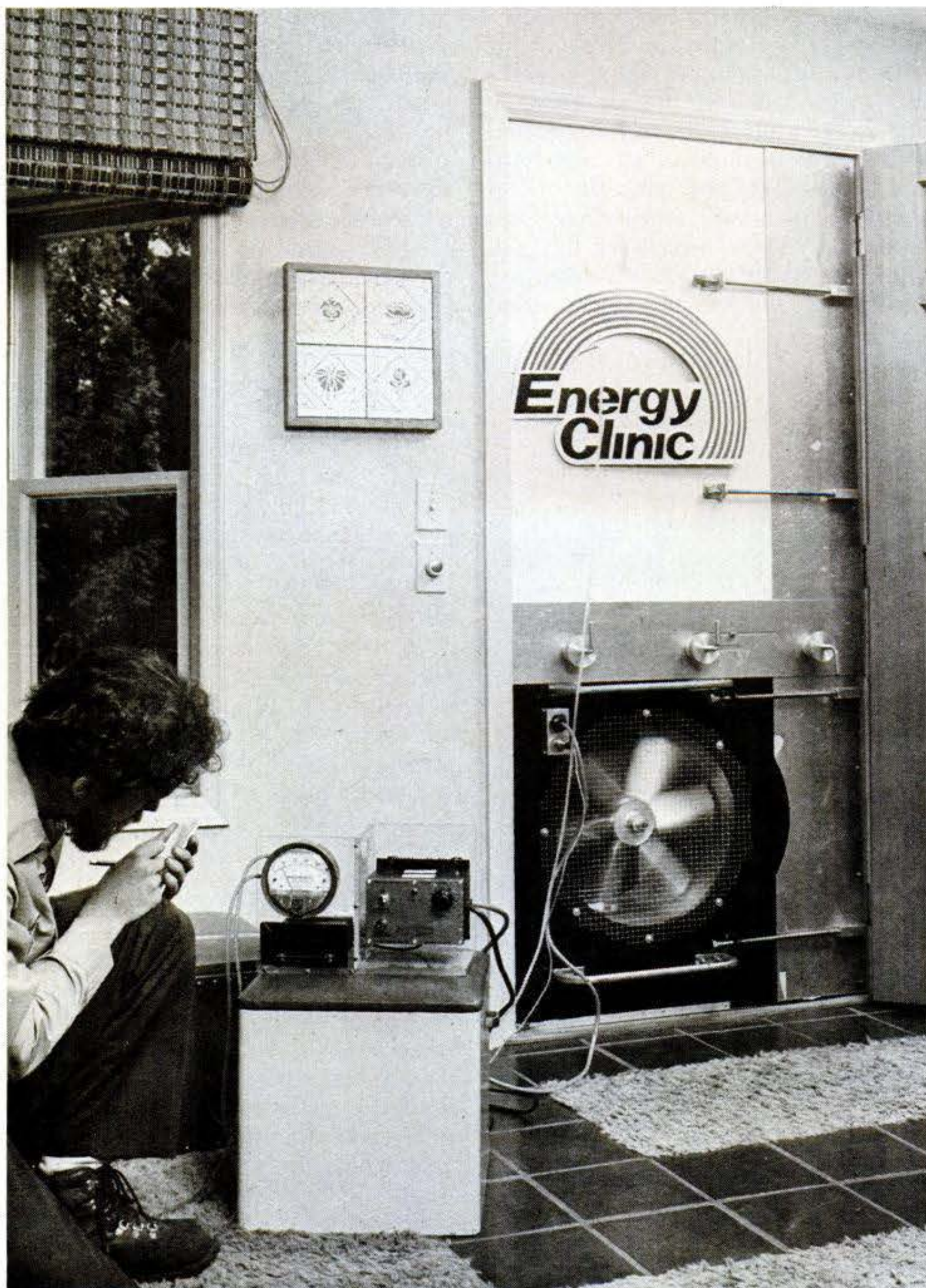
Blower door mounts in any exterior door to depressurize the home and “amplify” infiltration. Here, Energy Clinic’s Bill Mun-
