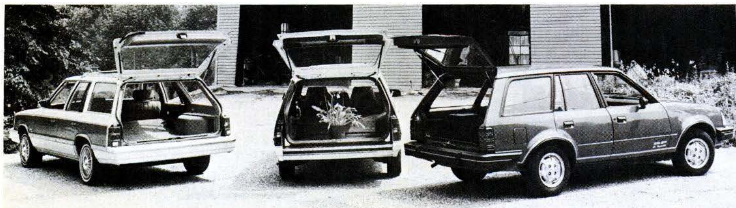
Top-pivoted tailgates are designed to offer unrestricted cargo loading, as well as some shelter from poor weather.
