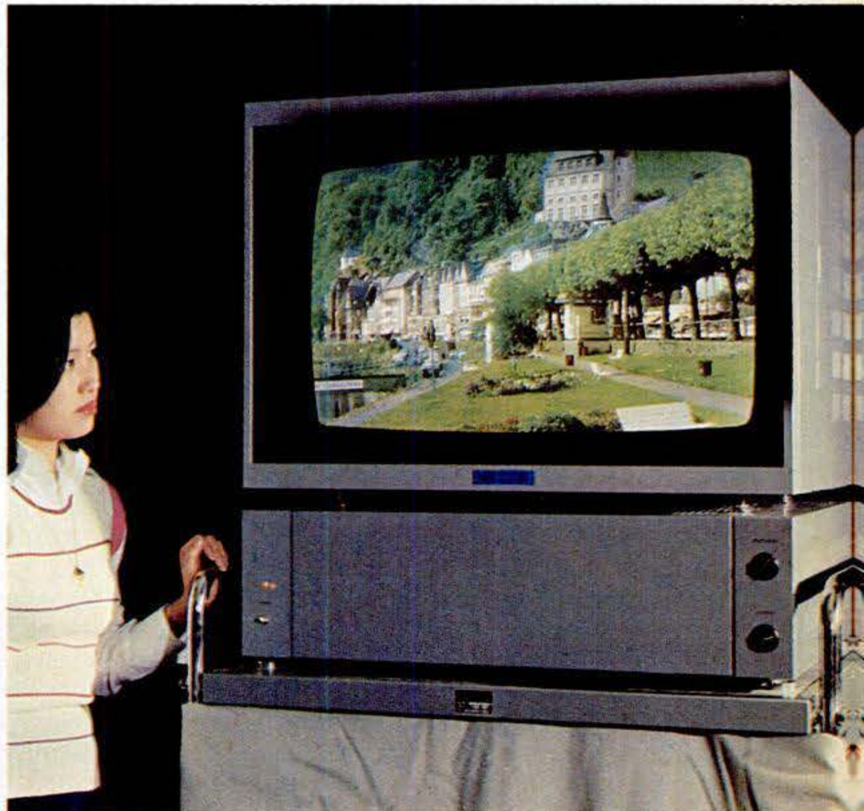
Wide-screen high-resolution monitor developed by NHK and Matsushita has 30-inch-diagonal screen, 5:3 aspect ratio. Phosphor dots are much smaller than on conventional shadow-mask tubes, and NHK uses a digital beam-convergence system.
