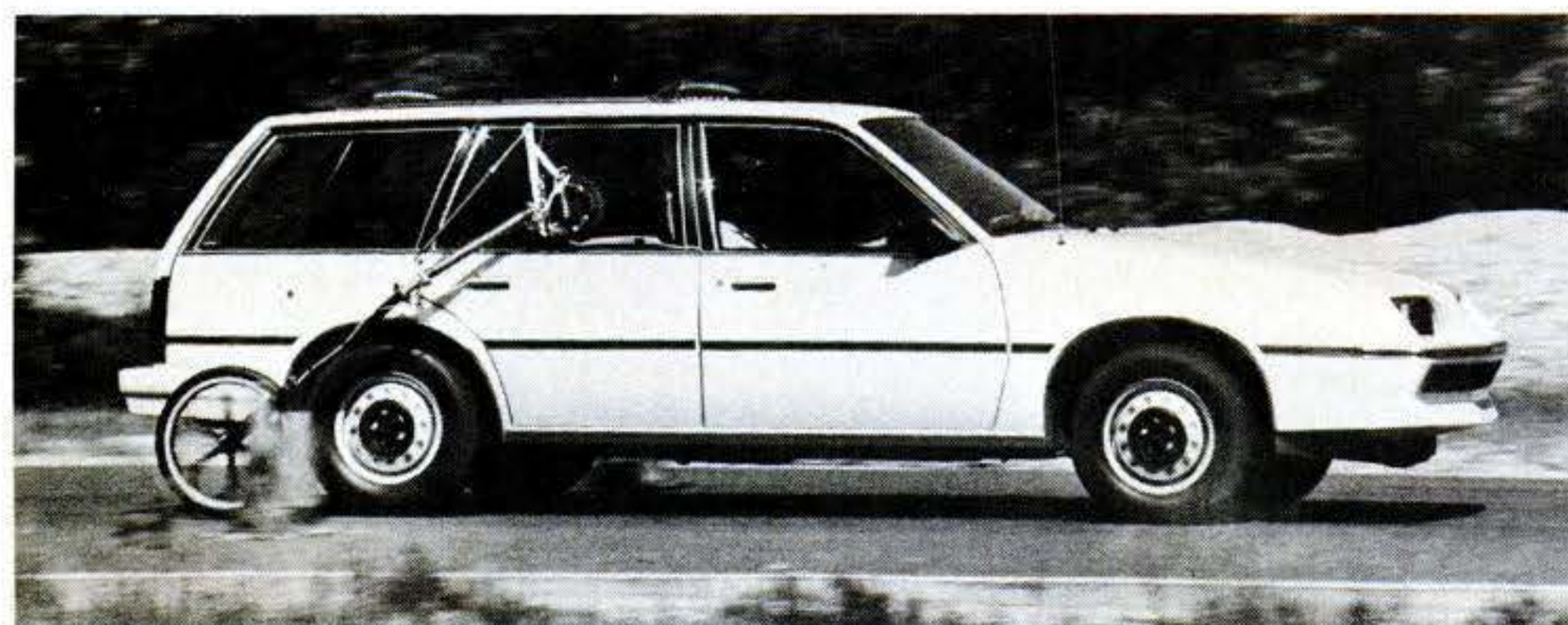
J2000 enters the test grid for a check of its 60-mph panic-stop characteristics.
