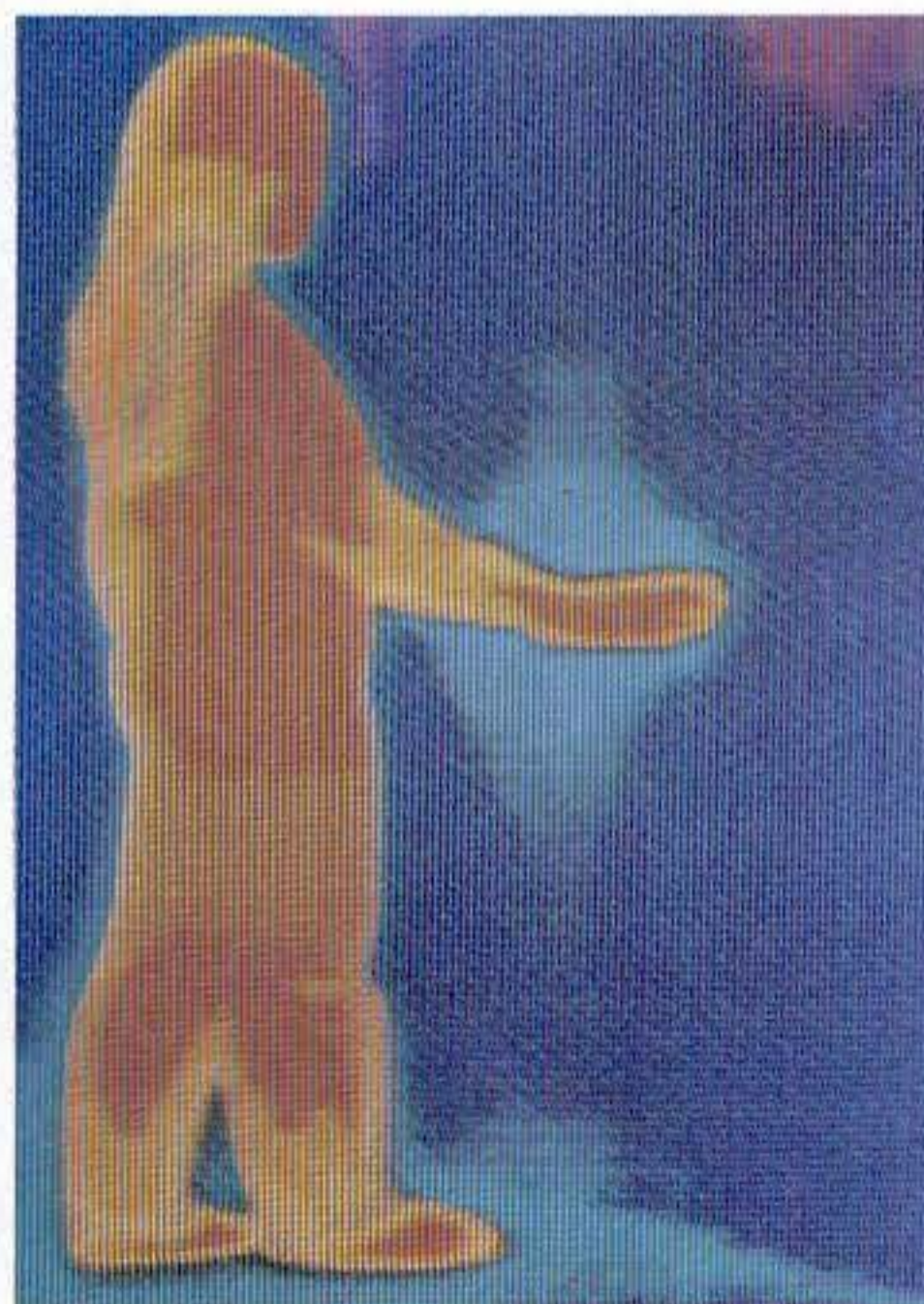
infrared camera, which shows that it reflects the body's infrared radiation back
