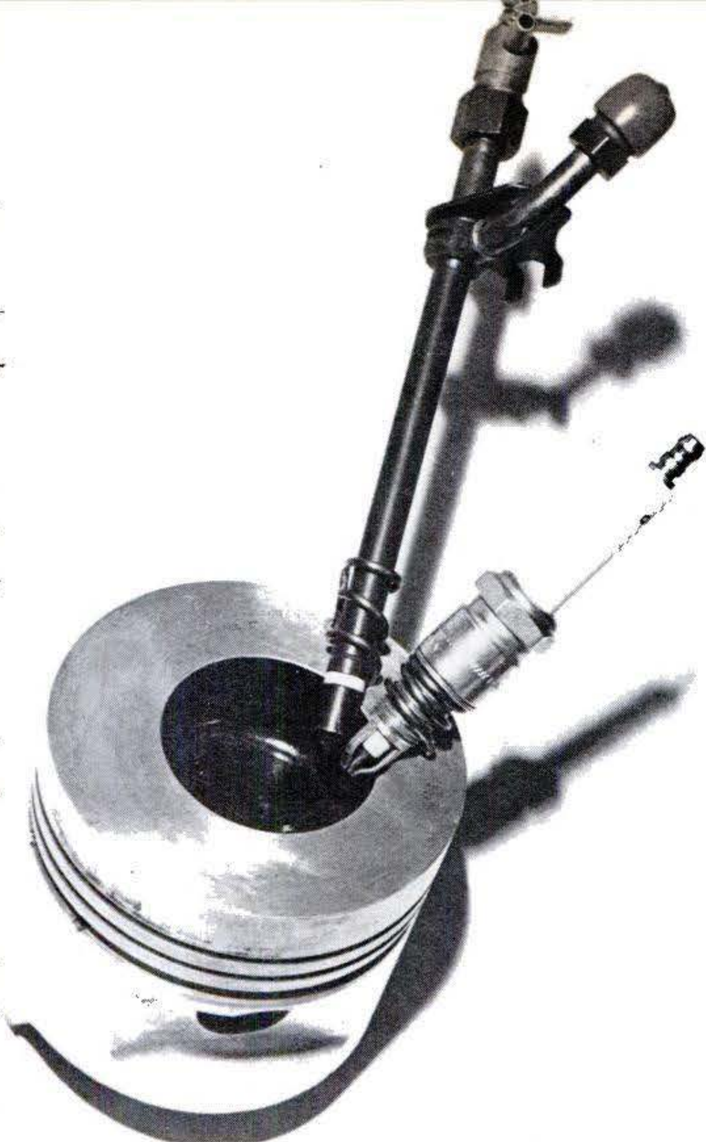
Closely spaced injector and spark plug create a flame front in the piston's dished area (above). Swirling air and continued fuel injection after spark termination feed the stationary flame front
