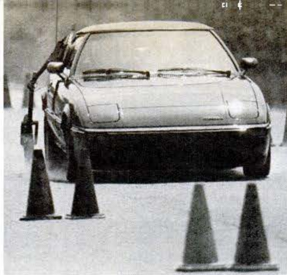
Mazda RX-7 stopped straight and with little brake lockup, but stopping distances were second-longest cold, longest hot.
