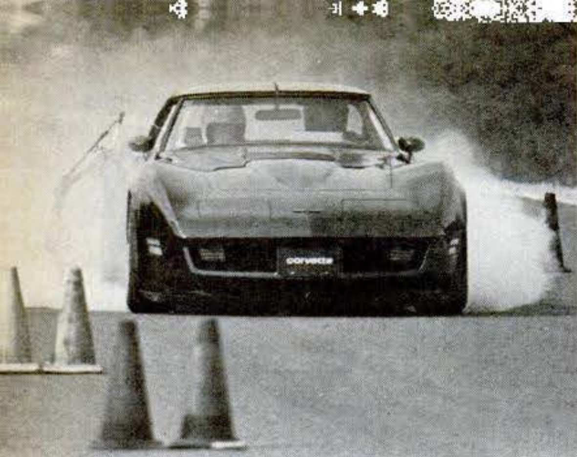
Corvette's smoky 60-mph panic stops were straight, but longest of all with cold brakes and second-longest hot.
