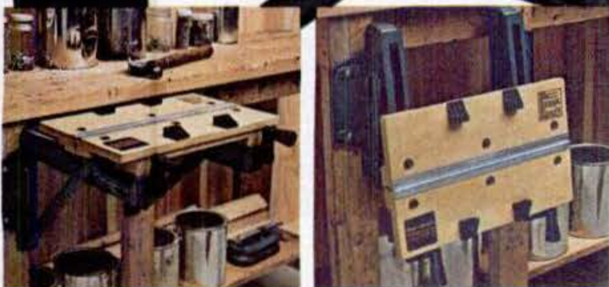
Mounts permanently to workbench or wall studs.
