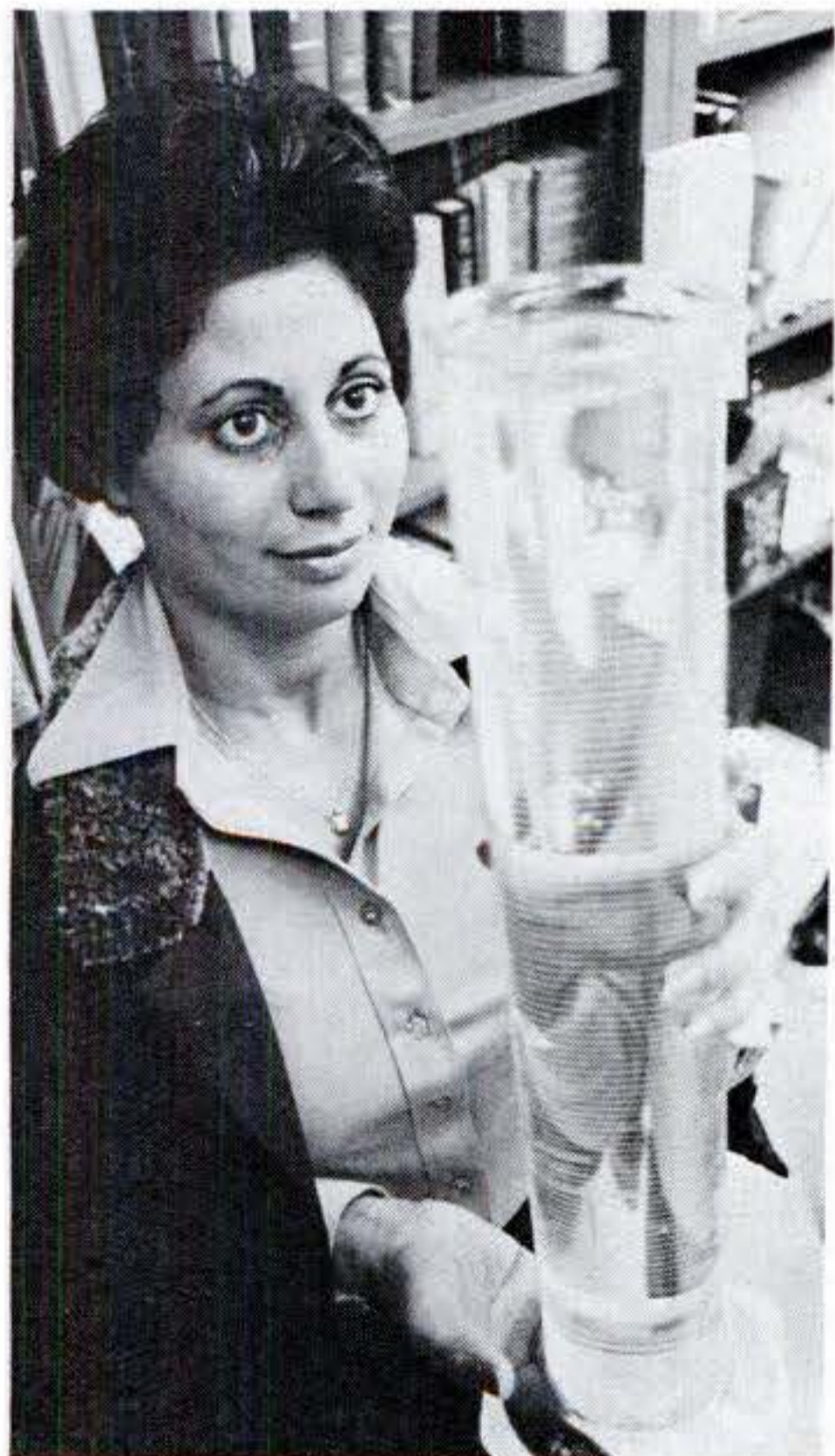
Clarity of her pond's polymer gel (top half in the cylinder) is demonstrated by Dr. Wilkins. Gels are still being tested for durability in ultraviolet light.
