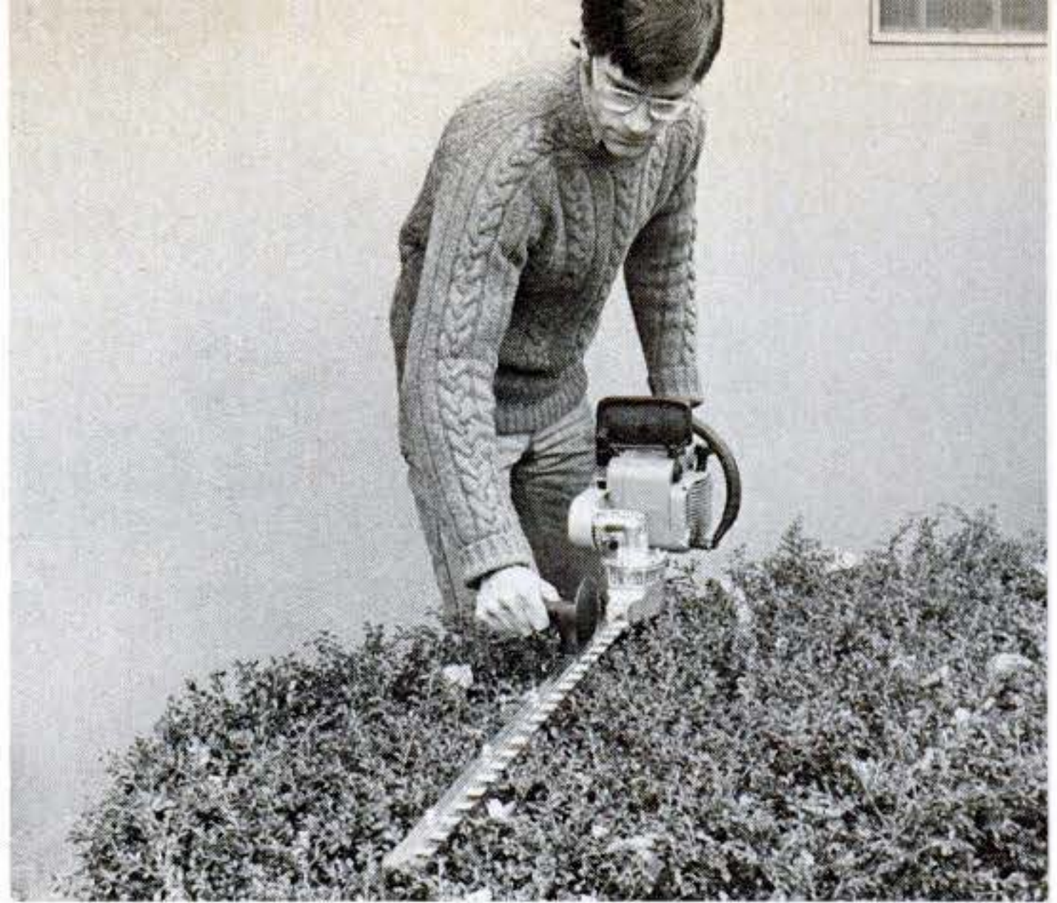
Hedge trimmer has extra-long, 30-inch chrome-steel blades. Chain-saw engine has ample power to handle dense hedges.
