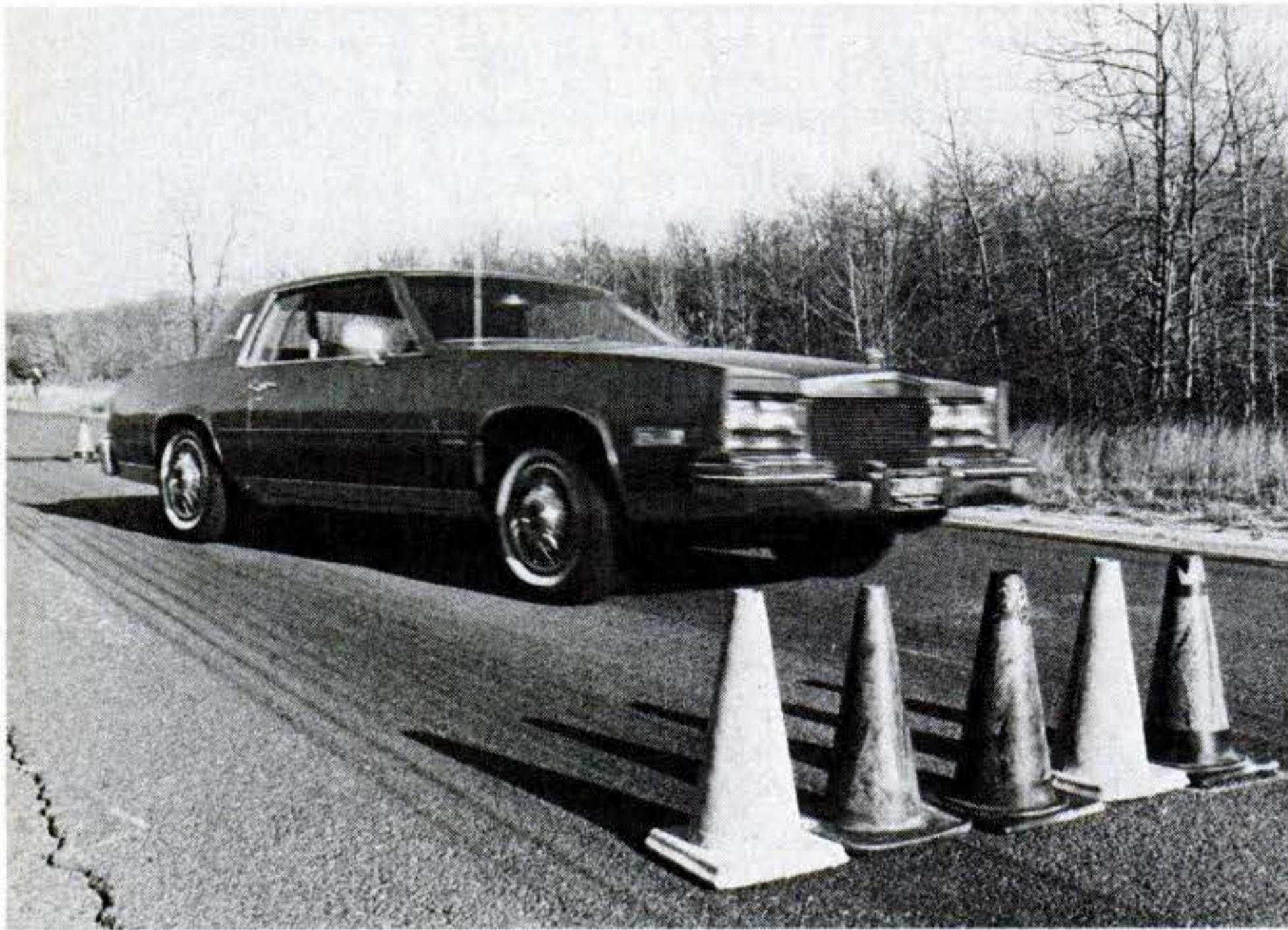
Eldorado's optional Touring Suspension produced handling and maneuverability far superior to that of the other cars. Here, it easily gets a top rating in the slalom.
