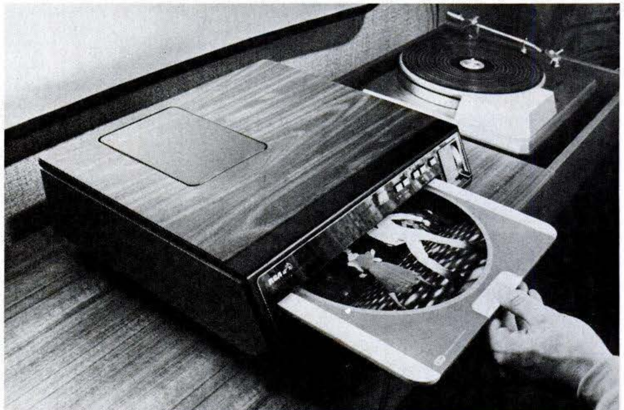
Disc and jacket are inserted into player. Jacket comes out, but the disc stays in.
