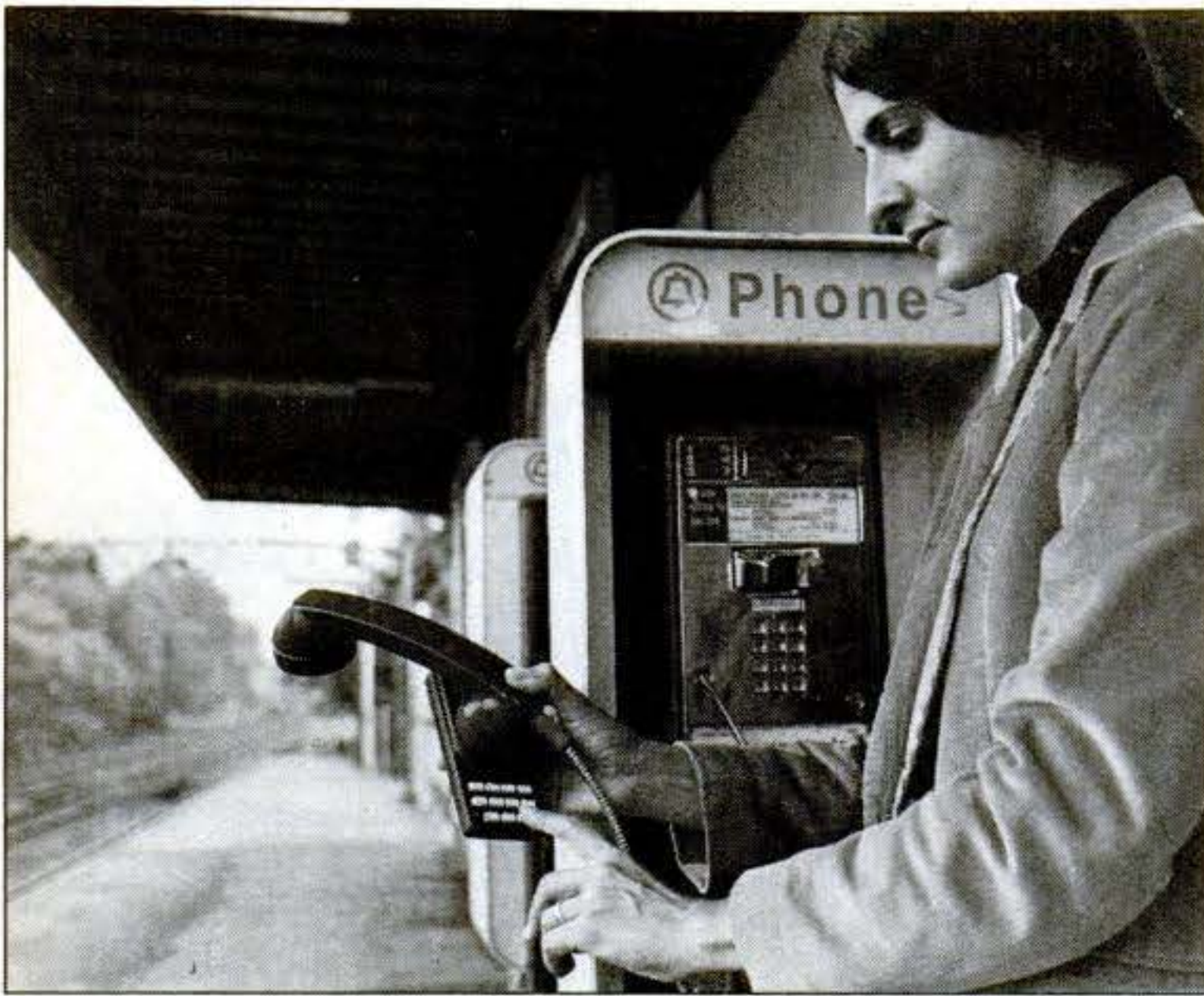
BSR's remote transmitter lets you send orders through phone lines. You call home and punch out commands on the keyboard. A telephone responder conveys them to the target switch.
