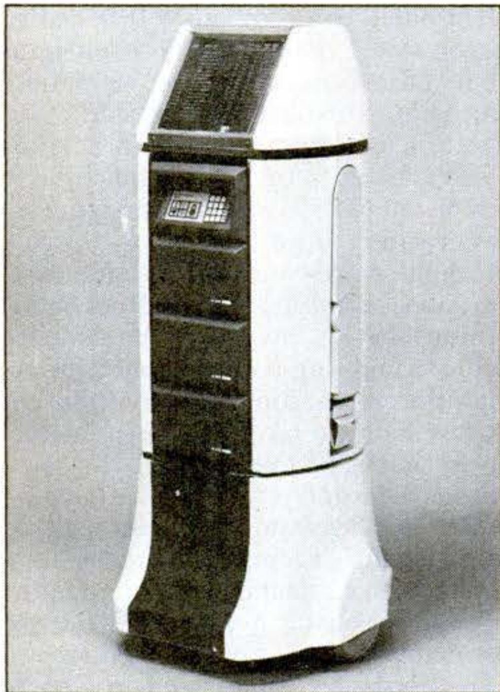
Mock-up of Genus robot includes optional on-board computer and triple-jointed arm. Base model would include top and bottom sections only.
