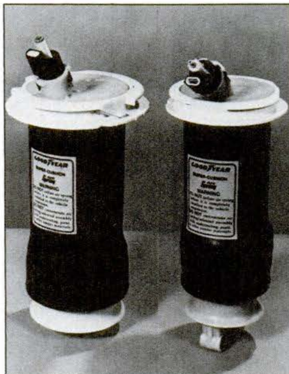
Air-ride components (top) are shown in their chassis locations on the new unit-body Lincoln. There are no complicated mechanical linkages. Two sensors at the front and one at the rear signal the microprocessor when adjustments are needed in vehicle ride height. The illustration (far left) reveals the simplicity and scant number of parts in the spring. Front (left) and rear springs are shown in the photo above. Internal pressures range from 65 to 100 psi.
