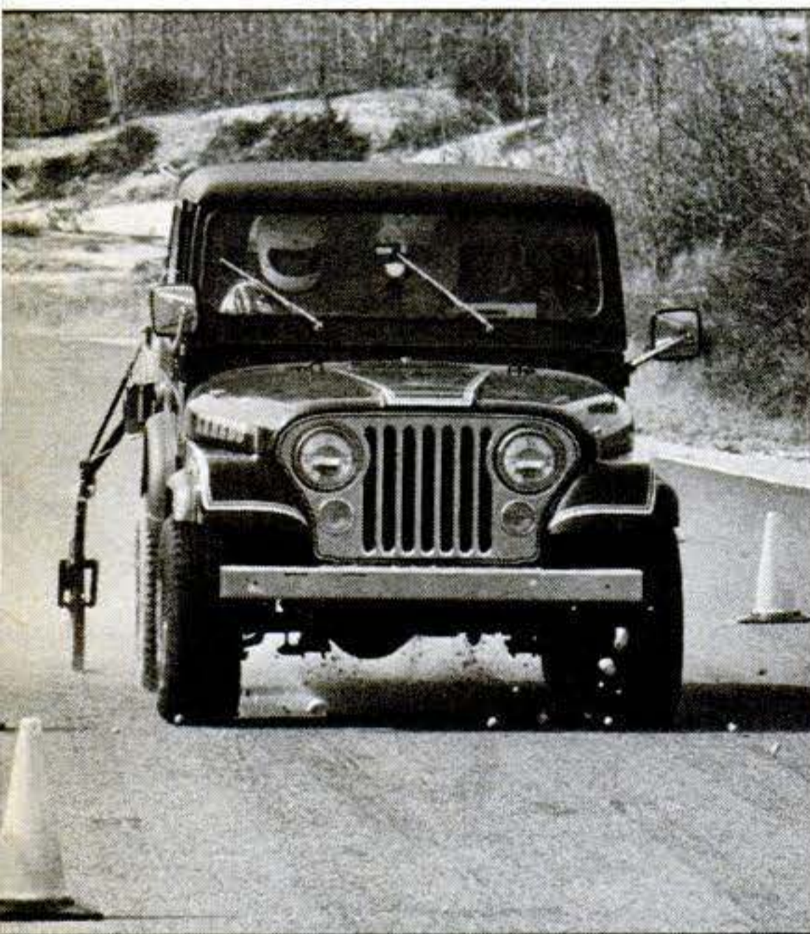
Jeep CJ-7's lower weight should have given it a great stopping advantage, but the lightly loaded rear tires had no bite.
