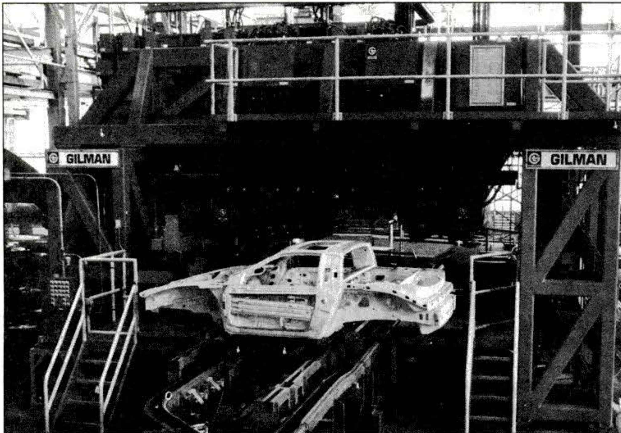
P-car frame goes into Gilman machine in demonstration. If a frame is out of toler-
