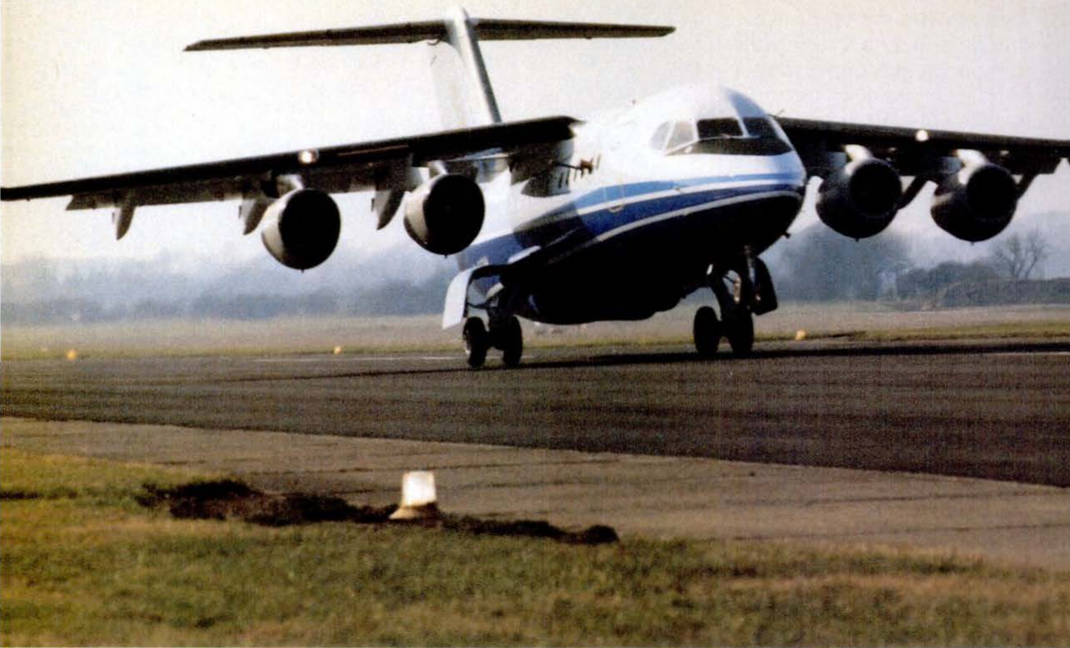
Four turbofans power British Aerospace BAe 146, a new 100-passenger commuter jet designed for flights as short as 150 miles.
