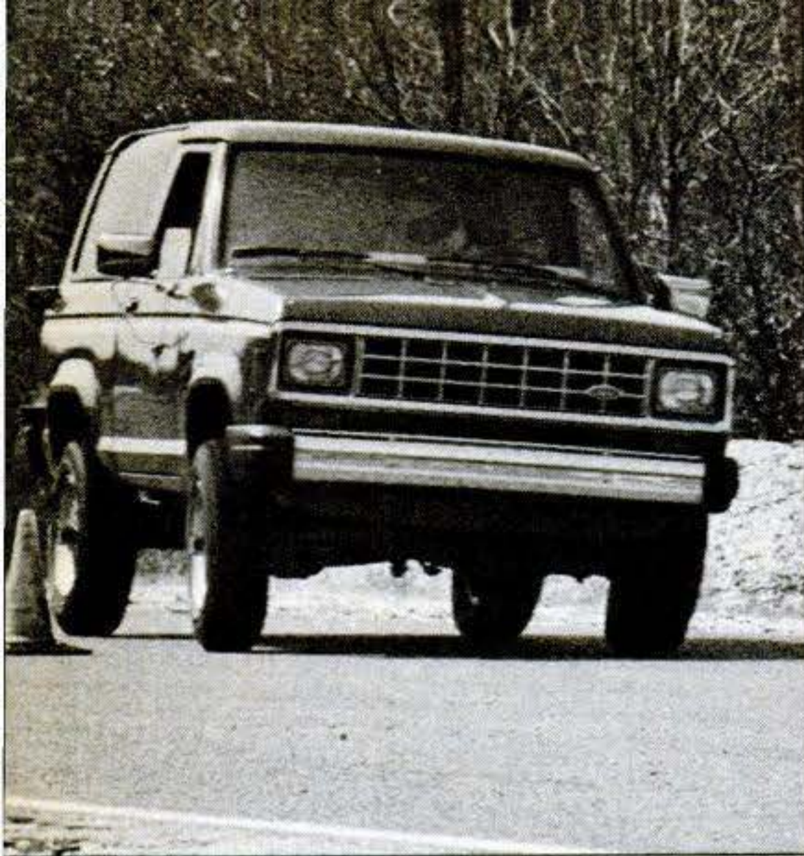
Bronco II revealed a strong tendency to under-steer when pushed hard through both high- and low-speed-handling tests.
