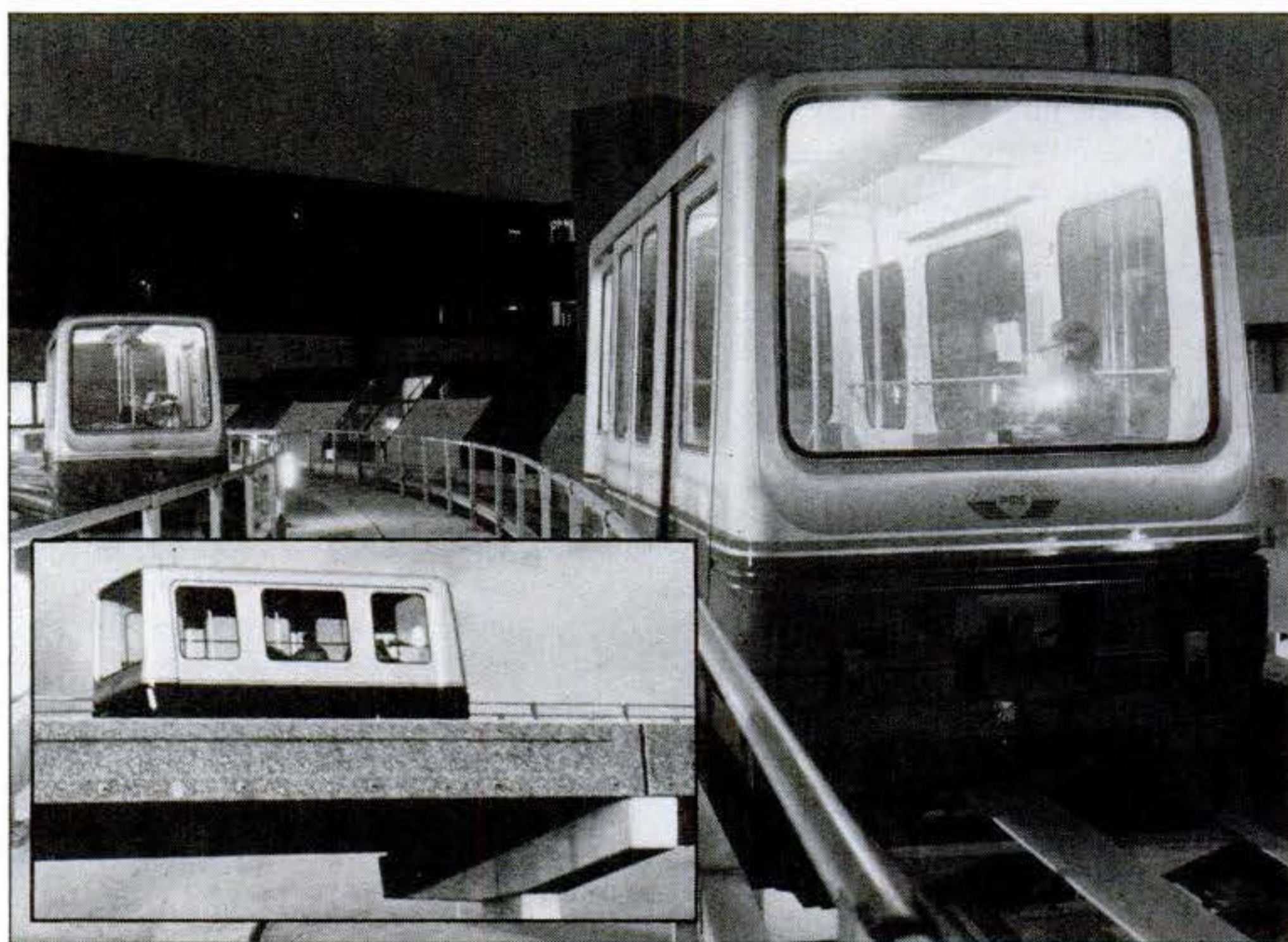
World's first commercial maglev service links Birmingham airport and a nearby rail station. Two cars, with fiber-
