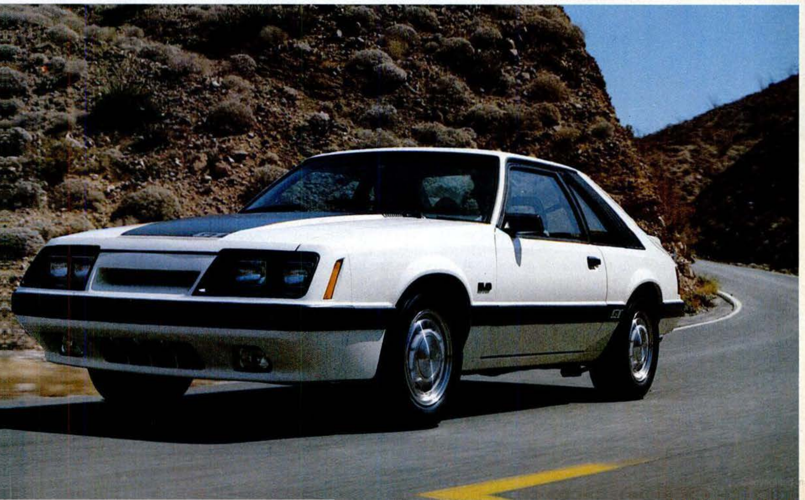
Merkur XR4Ti, sold by Lincoln-Mercury and built in Cologne, West Germany, will soon zig and zag down American roads. Ford Mustang GT sports a 210-hp V8 engine, 60-series unidirectional tires, and a short-throw five-speed manual transmission.
