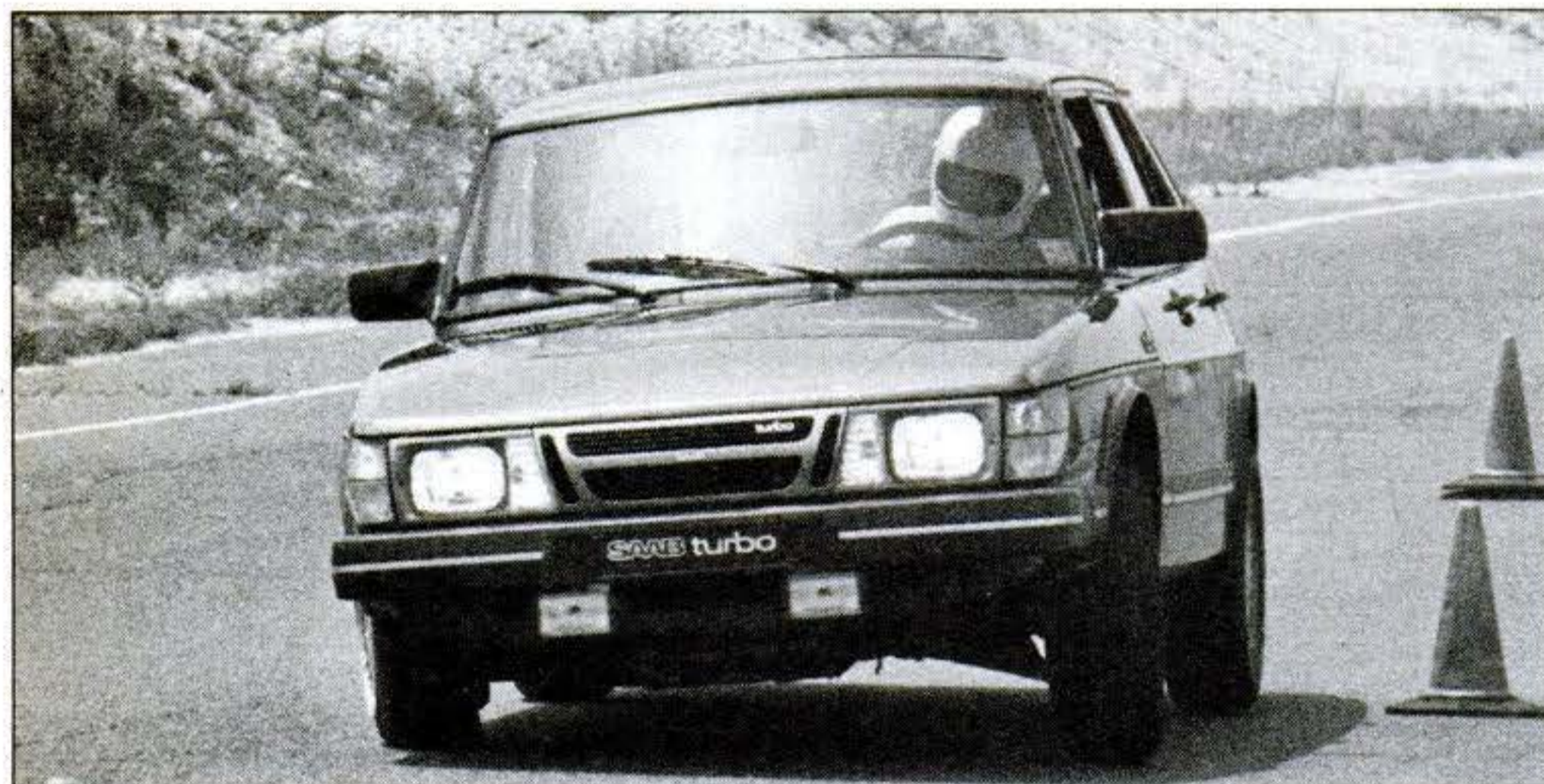
Saab 900 rolls slightly as it makes a pass through the low-speed maneuverability grid. The steering unit's quick response is important in this test.
