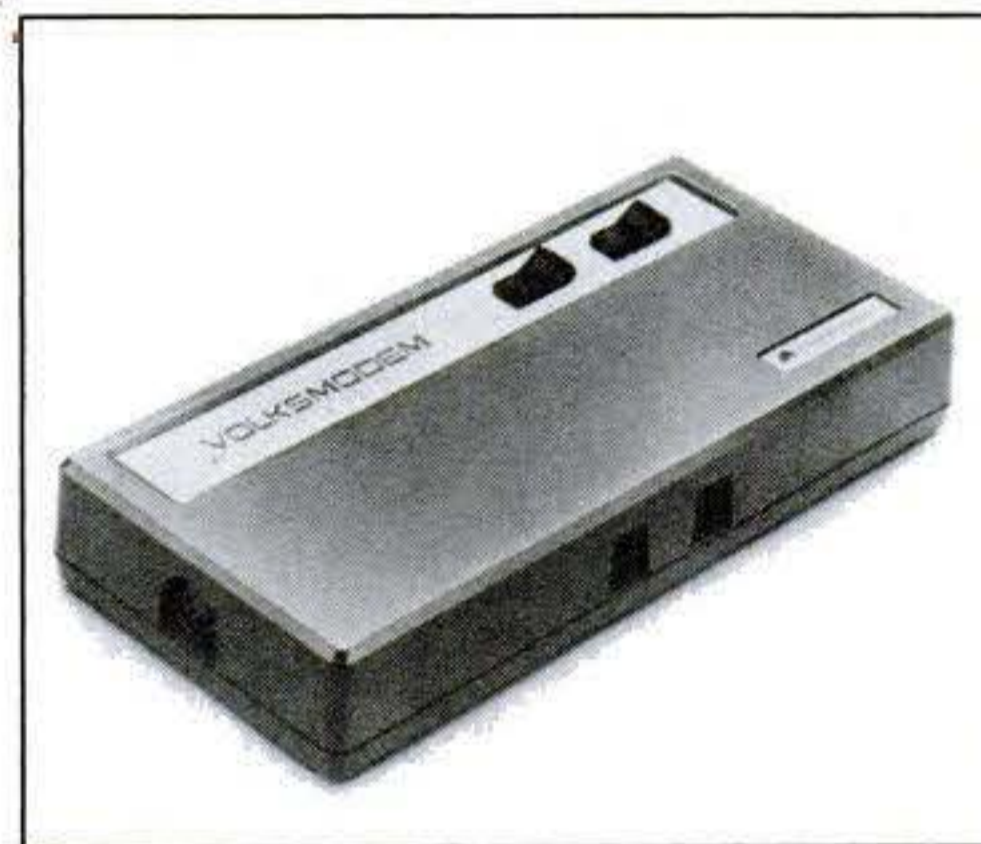
For portable use, this Anchor Automation's Volksmodem is powered by a nine-V battery. It lasts for about a year.
