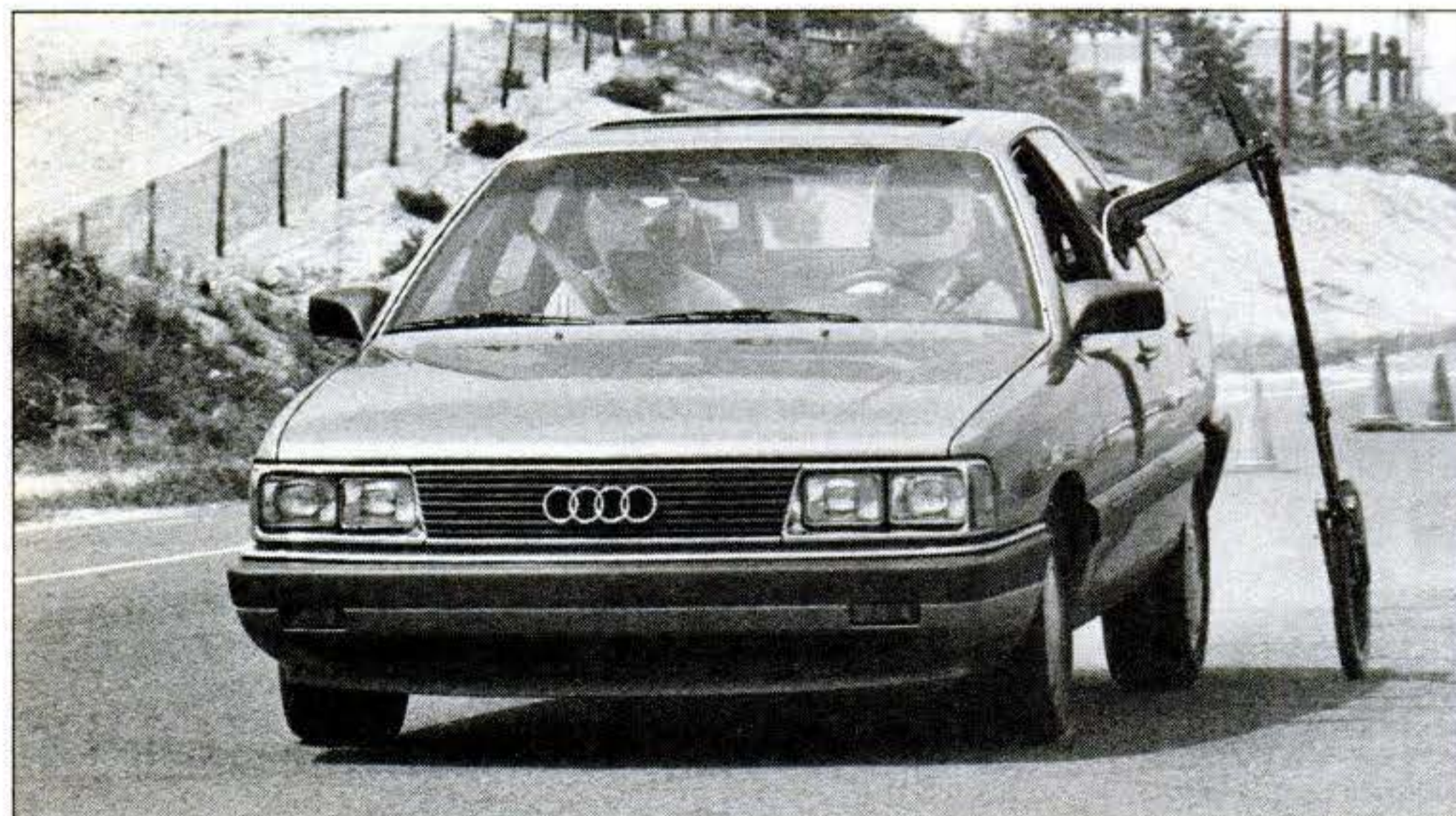
Audi 5000S squats on its front coils as it slides to a 175-ft. cold stop from 60 mph. A second stop with the brakes warm netted the same distance.
