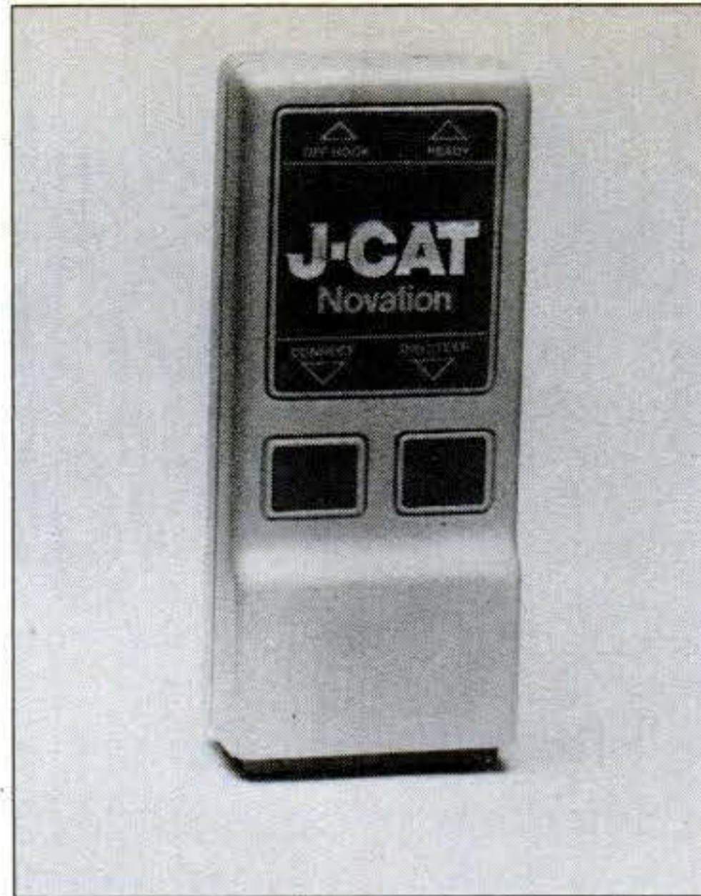
Buttons on Novation J-Cat smart modem allow manual connect and unit test. Status is given by LEDs.
