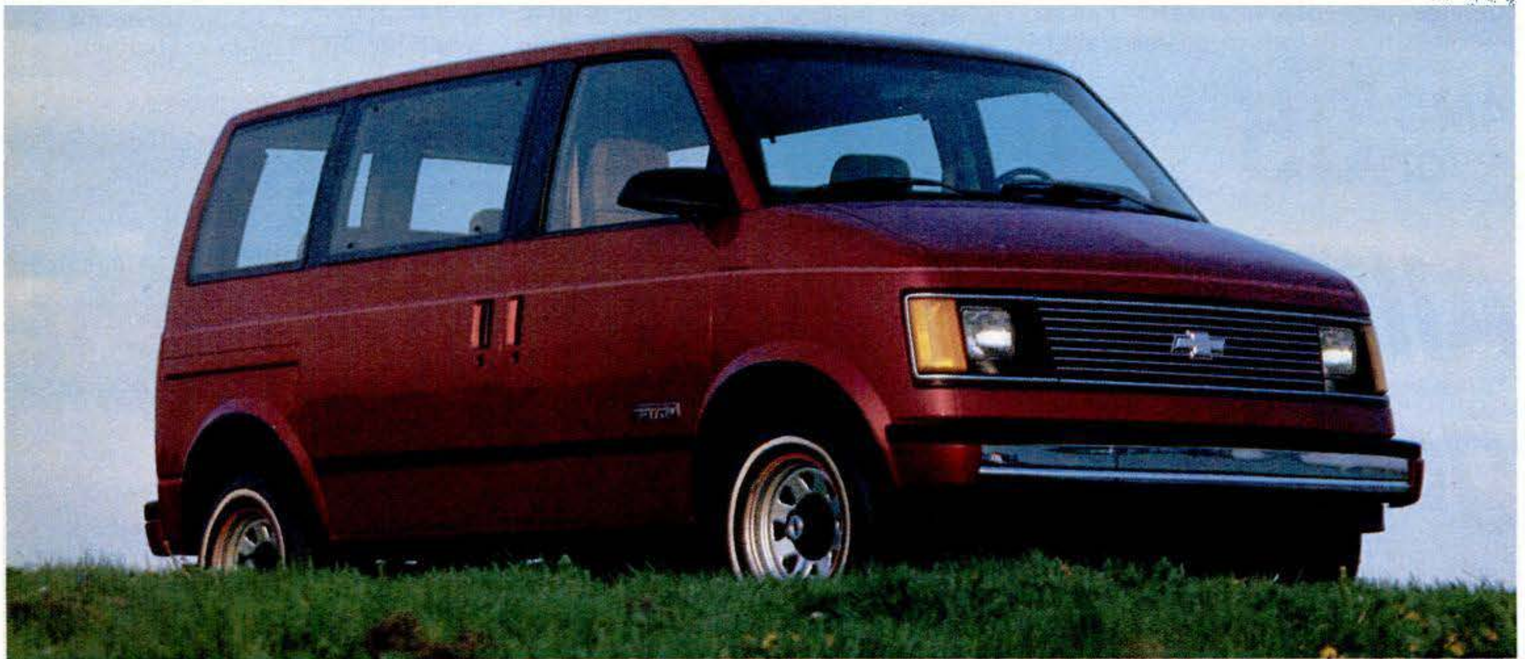
Aerodynamic details include near-flush door handles, a bonded windshield, flush side glass, and sleek side-view mirrors.
