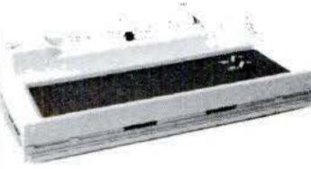
Receive only. Non-impact, thermal paper. 5 x 7 matrix-80 characters per line. Printing Rate: selectable, 10/30 char. per sec. Full/Half Duplex. Interface: Serial type/ RS232/C & Current loop. 300 baud rate. Dim: 14.6" x 15.25" x 4.25"
