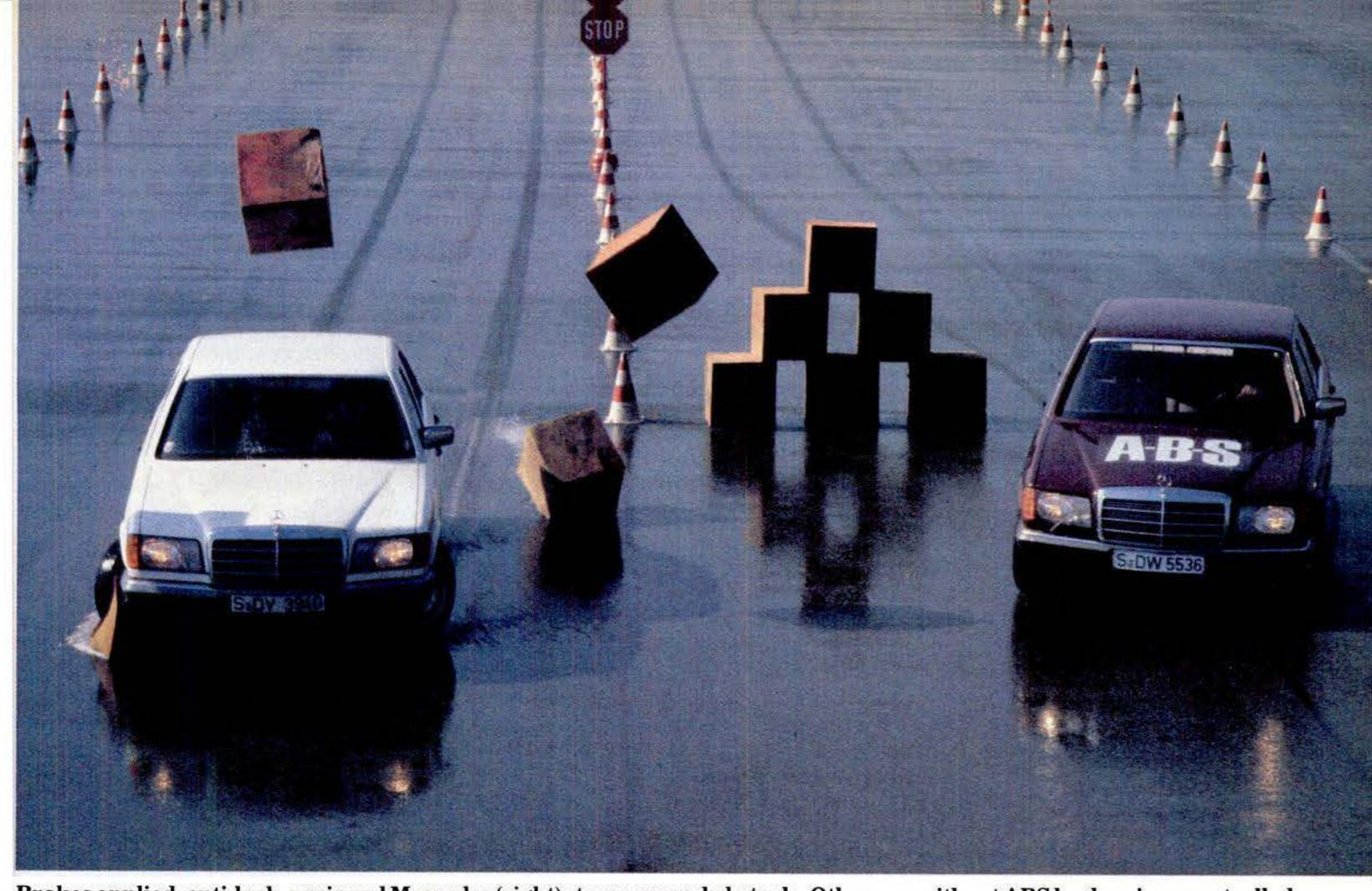
Brakes applied, anti-lock-equipped Mercedes (right) steers around obstacle. Other car, without ABS brakes, is uncontrolled.
