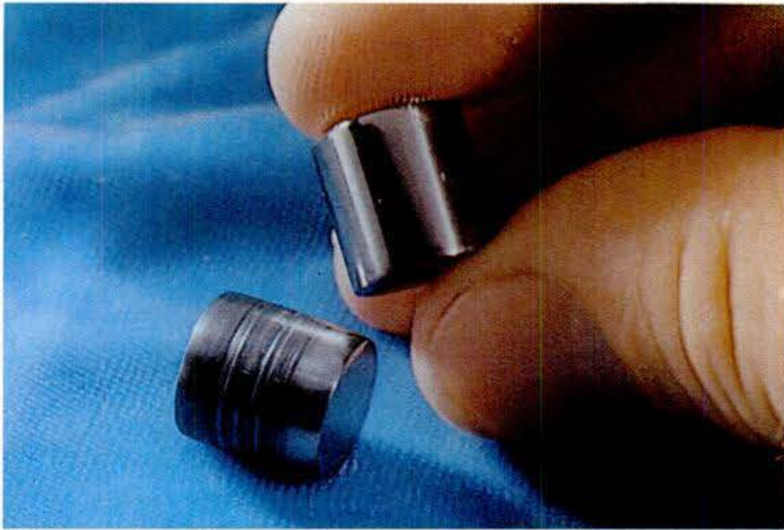
Nitrogen ions beamed into surface of titanium-aluminum alloy used for artificial hip joints transform the metal, making it exceptionally resistant to corrosion. Untreated sample, left, degrades in solution simulating body fluids.
