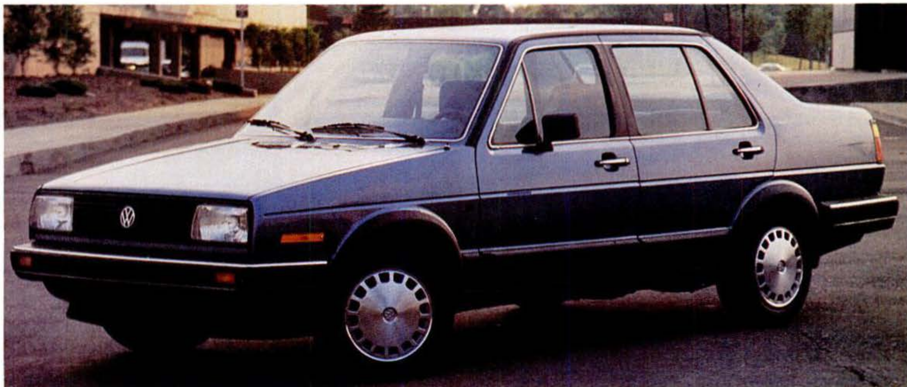
VW Golf (above) clips the corner during track testing. Below: Note Jetta's flush headlights and lack of rain channels.
