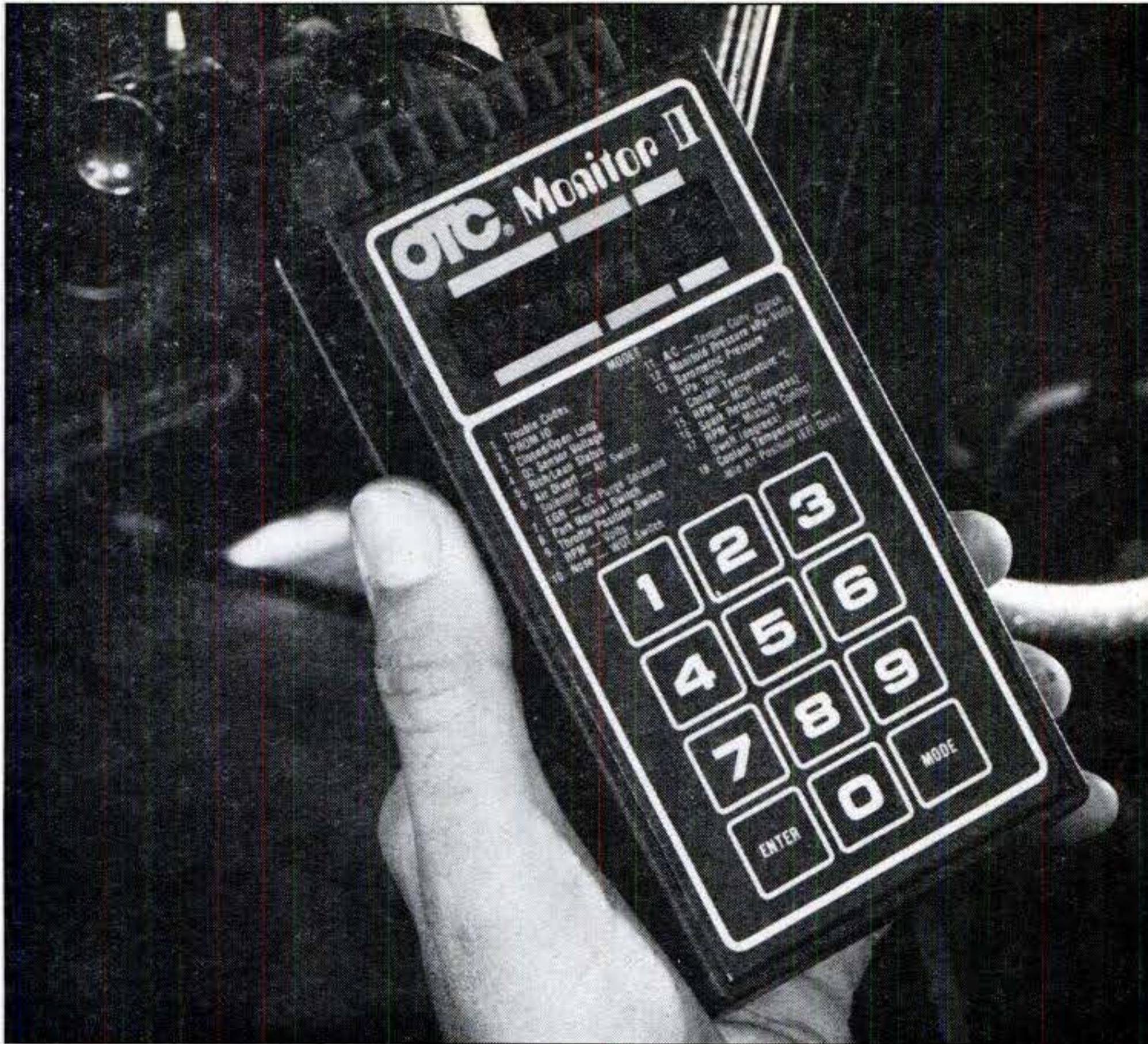
The hand-held OTC Monitor II uses a touch-pad keyboard to enter data and
