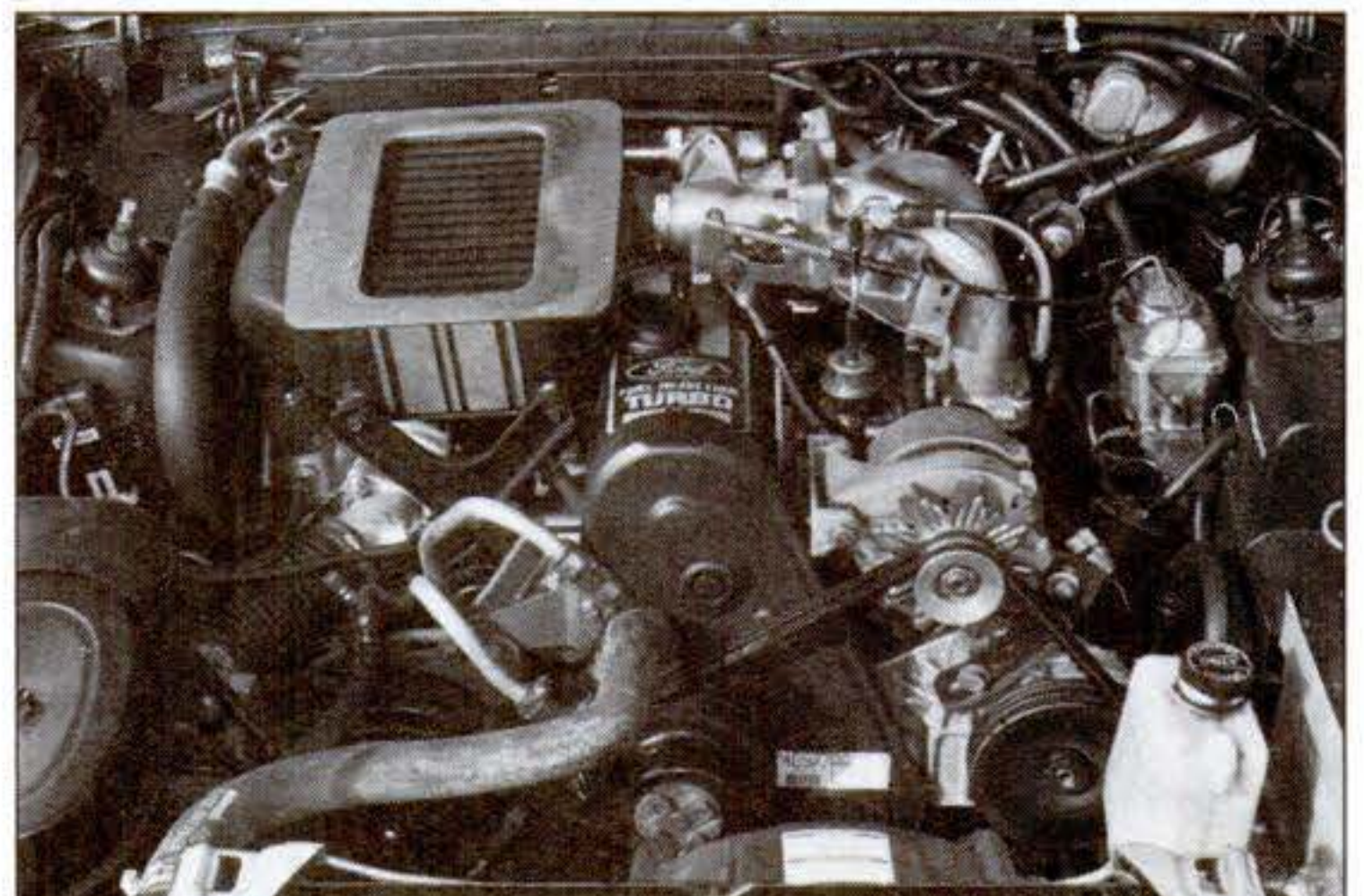
tang's striped intercooler, which cools the intake charge, is visible in the left-hand corner of the photo above.
