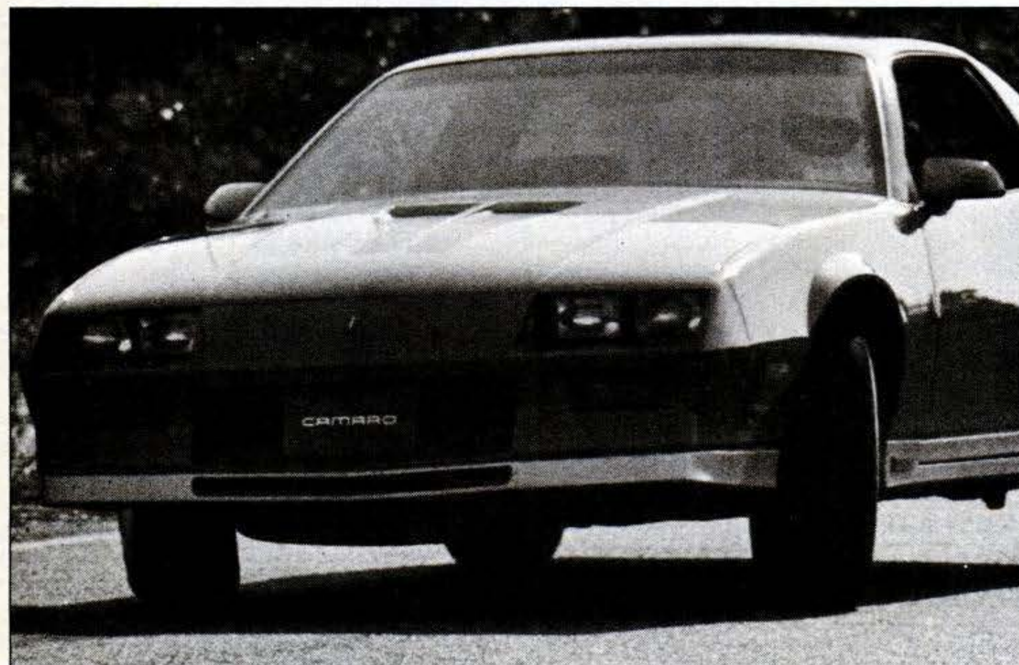
Camaro Z28's high spring rates, sticky rubber, and trigger-quick engine response all combined to make it the maneuverability champion of the test trio.
