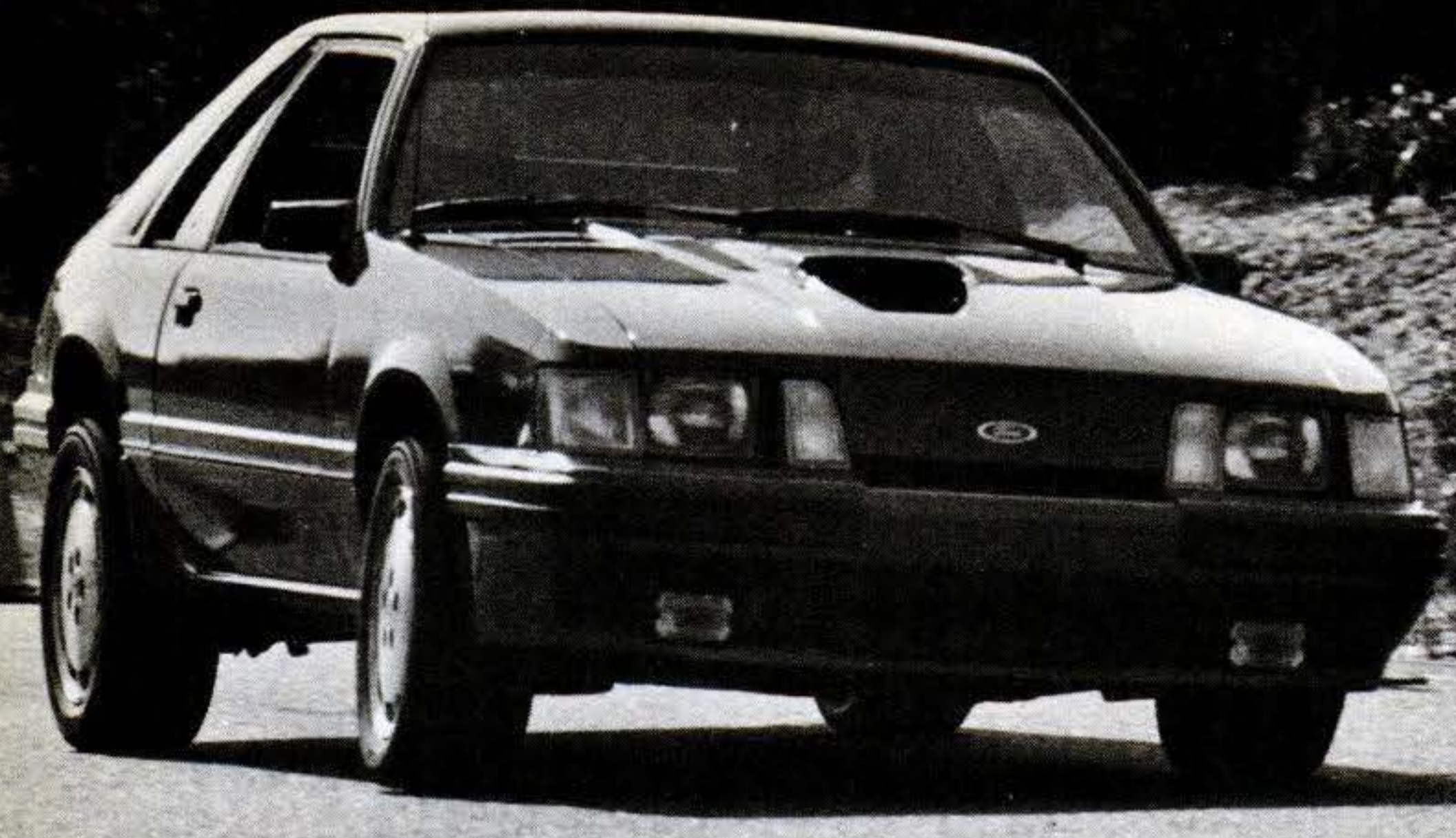
SVO Mustang's wide Goodyear Eagle GT P225/50VR16 tires and suspension tuning put the modified model within 8/10 mph of the top-handling Camaro Z28.
