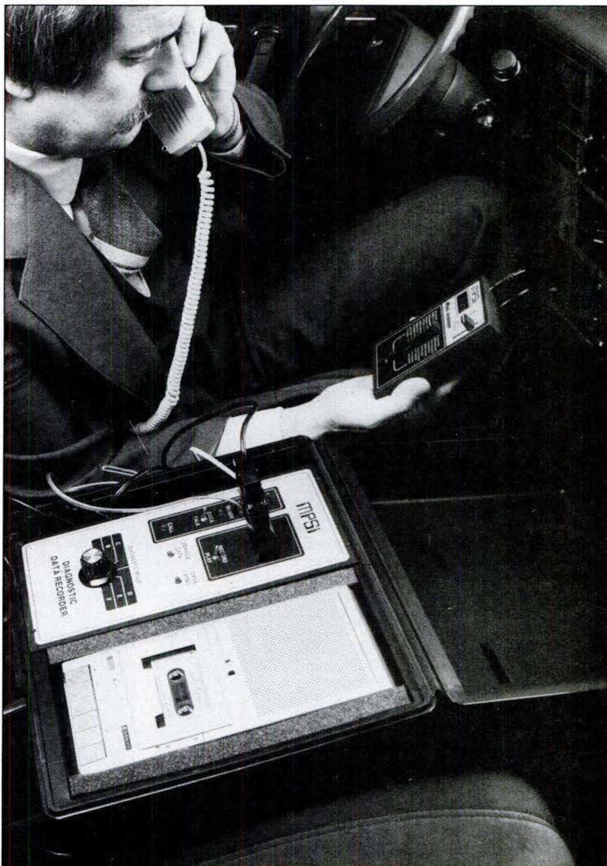
Car's diagnostic connector plugs into portable data recorder, which links to remote computer over phone line. Tape allows delayed data transmission.
