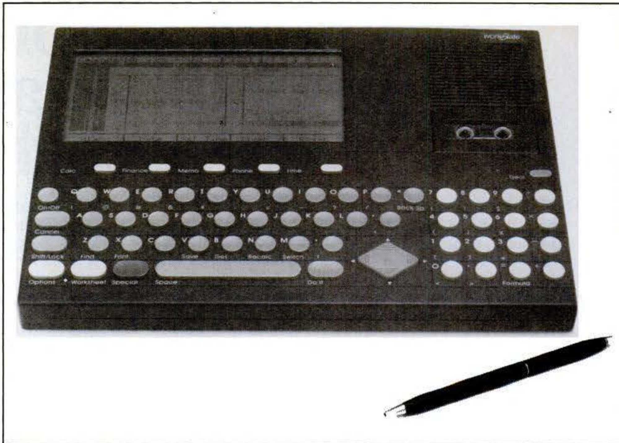
Small but versatile Workslate computer has 60 keys and LC display. It's powered by four AA batteries. A variety of business software is available.
