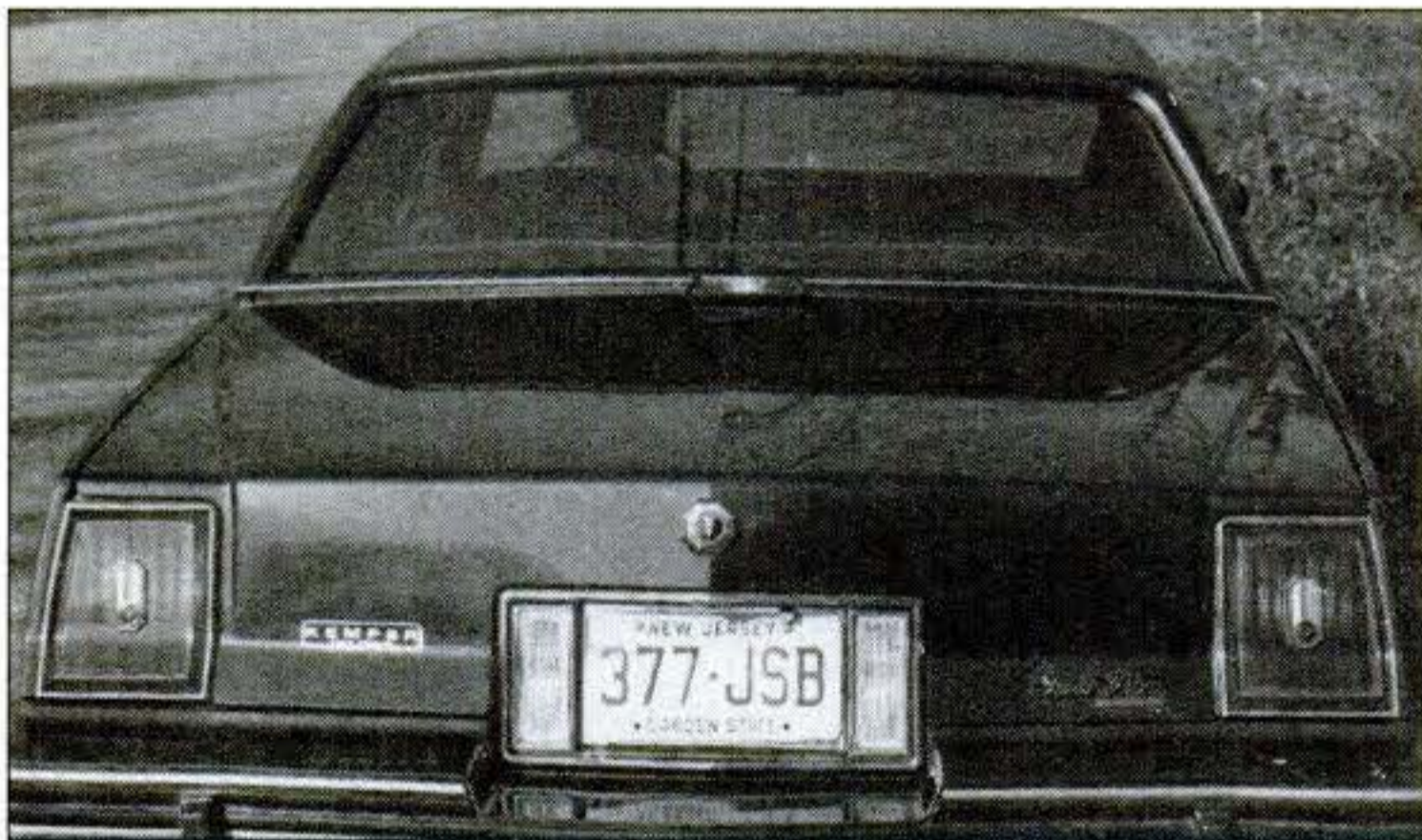
The third brake light on the author's car took 45 minutes to install. It flashes simultaneously with the hazard lights.
