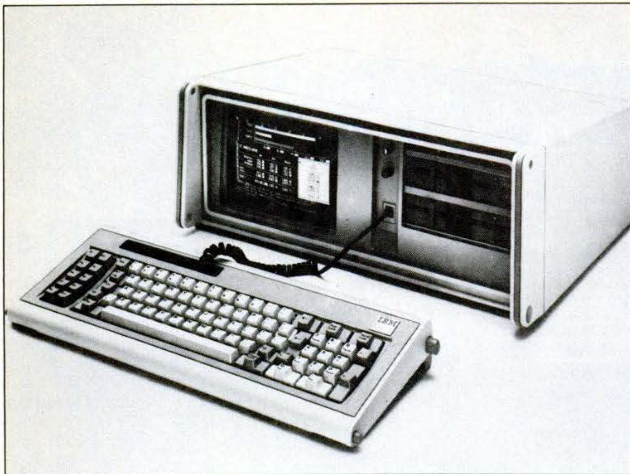
Keyboard of IBM's portable PC snaps out for work, snaps in to cover the nine-in. amber CRT display and disk drive when computer is transported.
