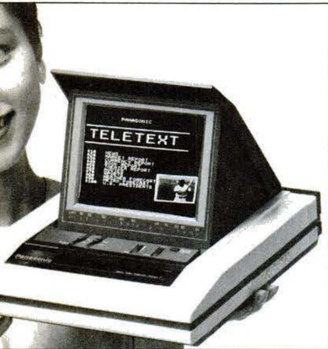
Collapsible rear-projection screen in Matsushita's prototype folds into a carrying case. Miniature optics (above) are arranged as in much larger sets.
