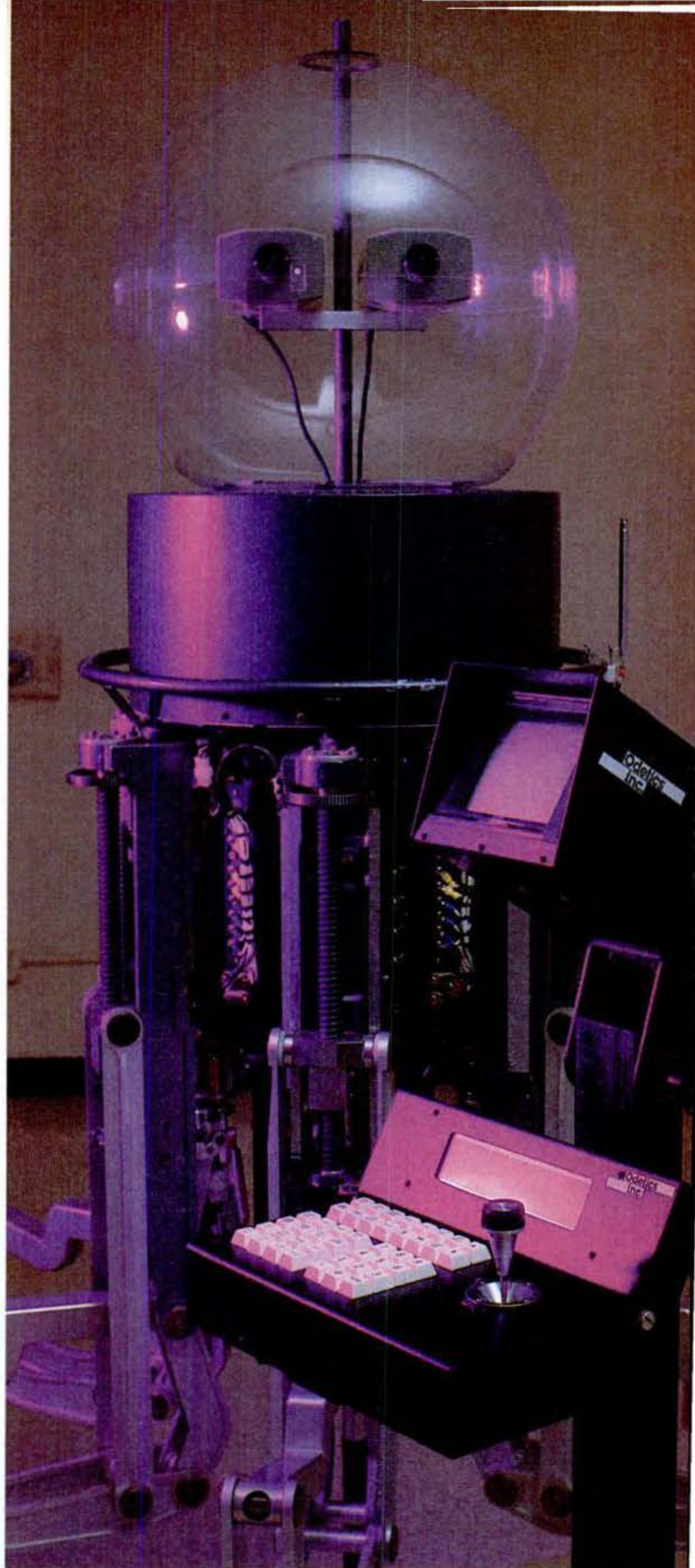
Versatile Odex I hefts a 275-lb. weight (above) and squats low to the floor (below right). A command radioed from a separate control board (right) triggers pre-programmed sequences stored in the master computer in the robot's "neck."
