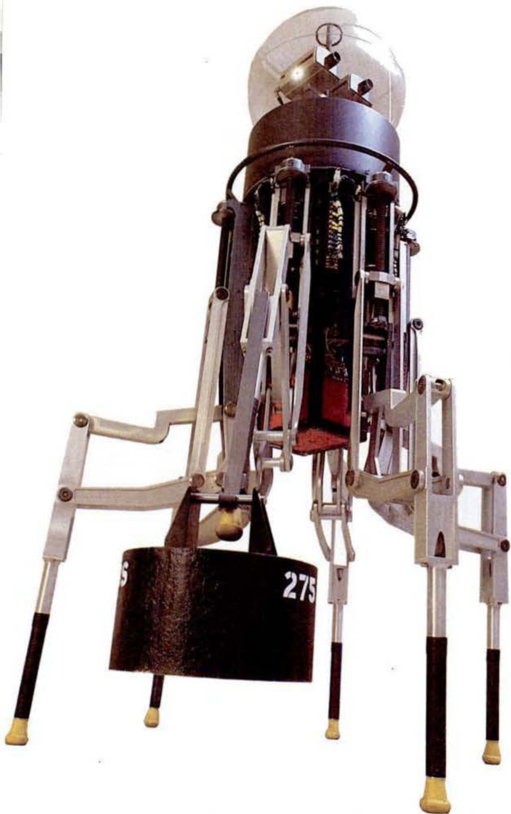
Versatile Odex I hefts a 275-lb. weight (above) and squats low to the floor (below right). A command radioed from a separate control board (right) triggers pre-programmed sequences stored in the master computer in the robot's "neck."
