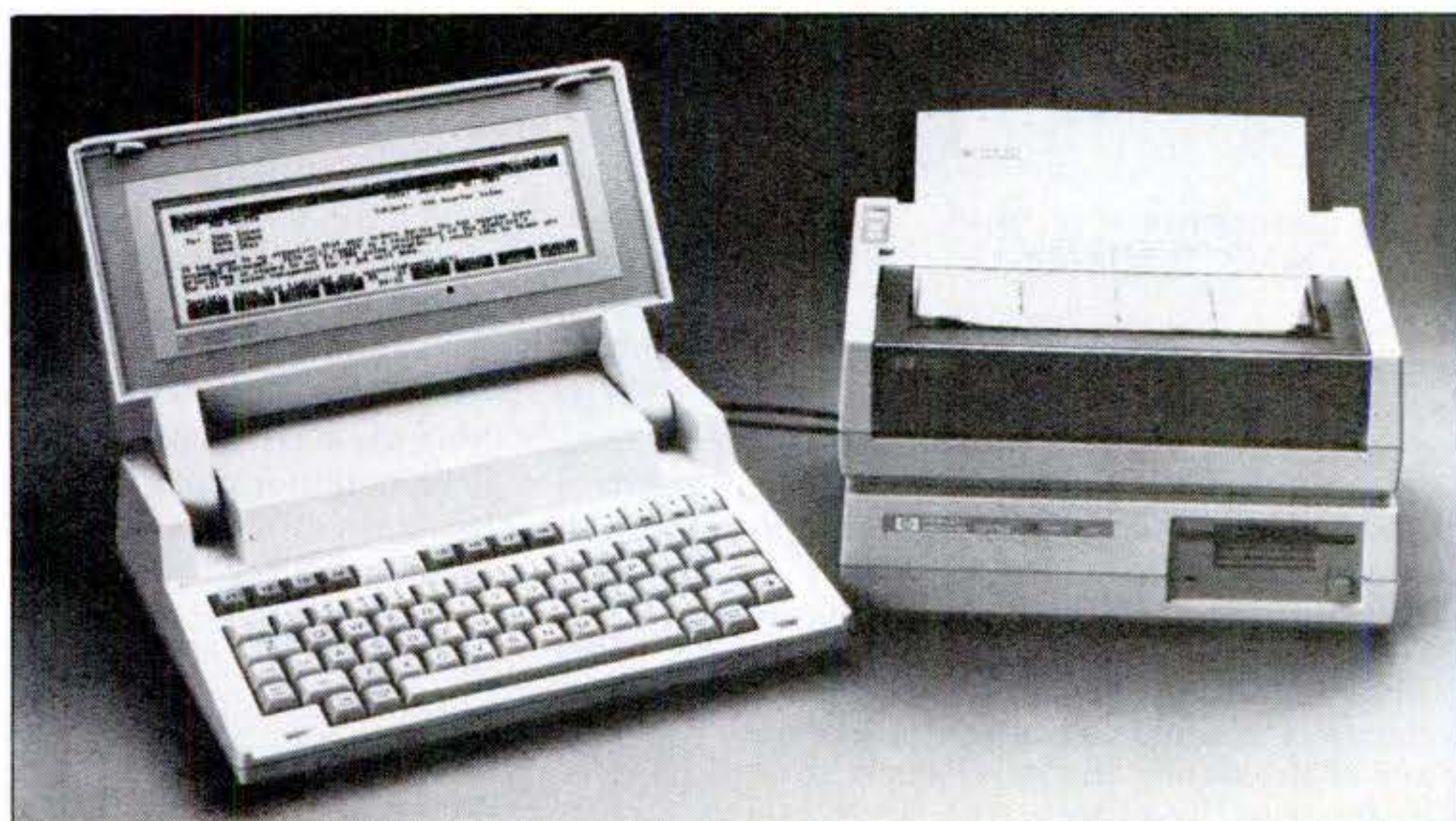
Liquid-crystal display of the Hewlett-Packard portable flips up to show 16
