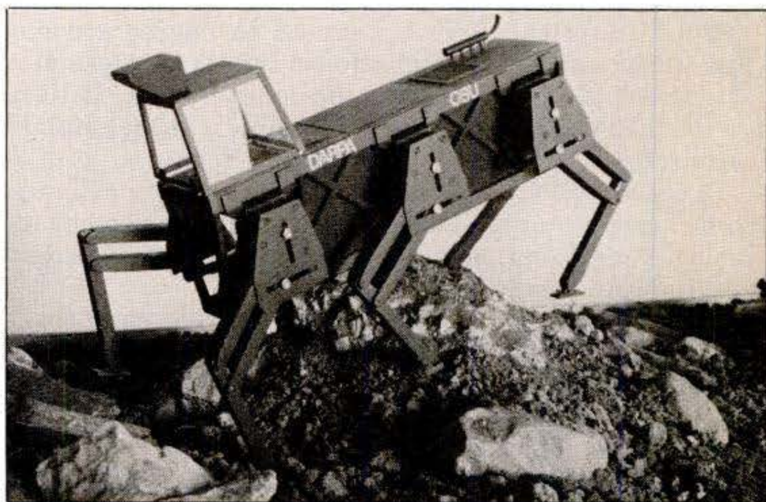
Hexapod (top), an early walking machine developed by OSU’s McGhee, was controlled via a cable link. OSU’s 2.5-ton Adaptive Suspension Vehicle (above) has six-ft. double-jointed legs with “ankle” sensors to handle rough terrain.
