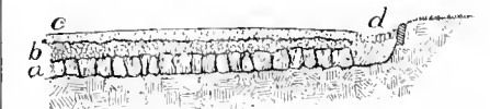
Fig. 35. Section of the Telford Garden Road, a large stones, b broken stones, c gravel, d gutter.
