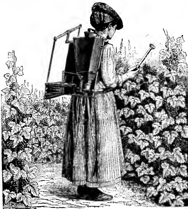
Knapsack Apparatus with Bellows, for Powders used in the Vineyards of France.
