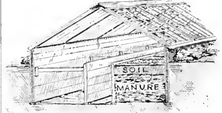
Cross-section of Manure Heated House.
