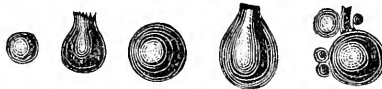
FIG. 5.—GLOBULES OF MAGNETIC OXIDE OF IRON OBTAINED BY BURNING FINE IRON FILINGS IN A HYDROGEN FLAME. (500 Diameters.)
