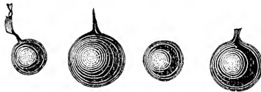
FIG. 6.—SPHERICAL GLOBULES OF MAGNETIC OXIDE OF IRON OBTAINED BY COLLECTING THE SPARKS STRUCK OFF BY A FLINT. (250 Diameters.)
