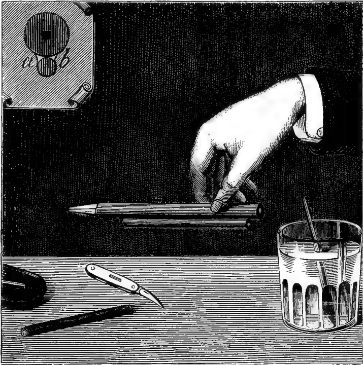
FIG. 1.—ADHERENCE OF ONE PENCIL TO ANOTHER BY THE TENSION OF CONCAVE SURFACES OF WATER.
