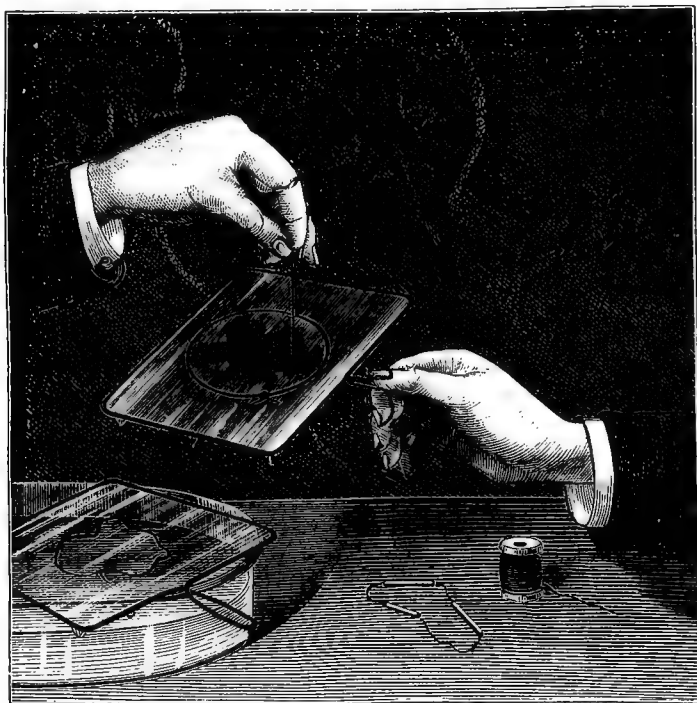
FIG. 5.—A CONTOUR OF SILKEN THREAD EXPANDING INTO A CIRCLE WHEN THE FILM ON WHICH IT HAS BEEN LAID IS BROKEN.
