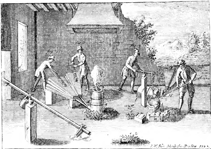
FIG. 8.—MELTING IRON FOR CASTING IN SMALL FURNACES.
