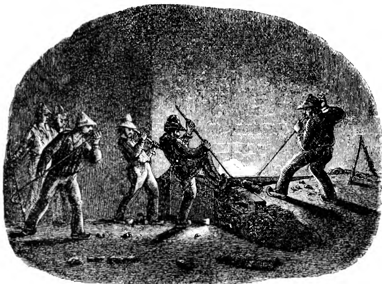
FIG. 11.—REMOVING A BALL FROM A CATALAN FORGE.
