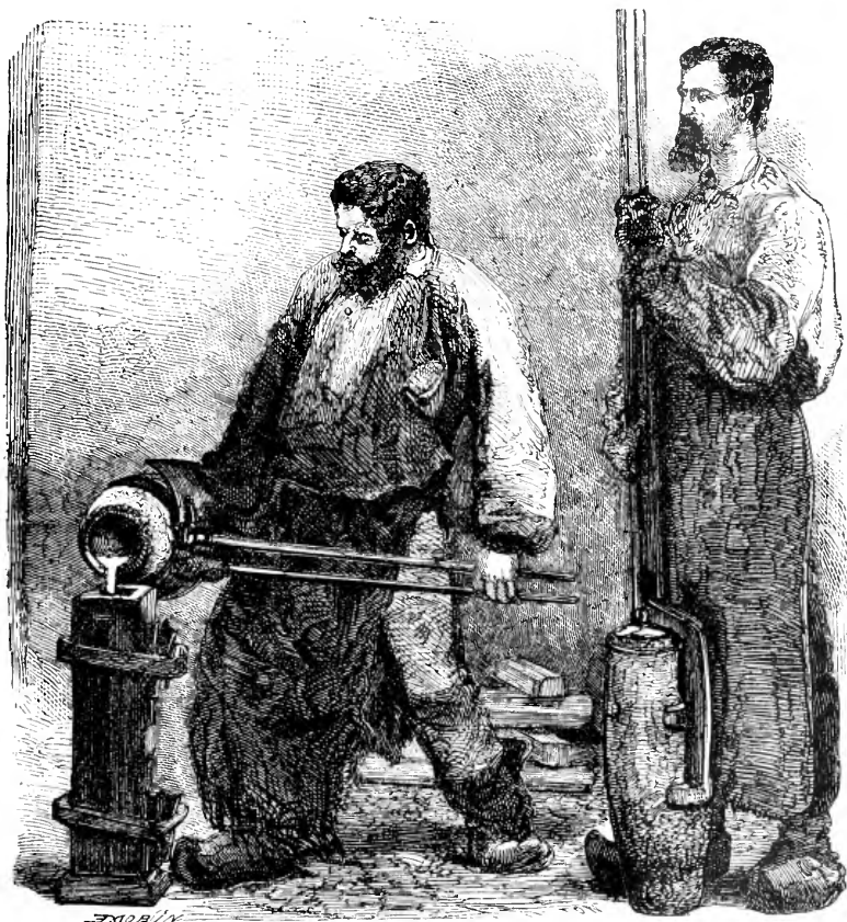
FIG. 53.—"TEEMING" AN INGOT OF STEEL.
