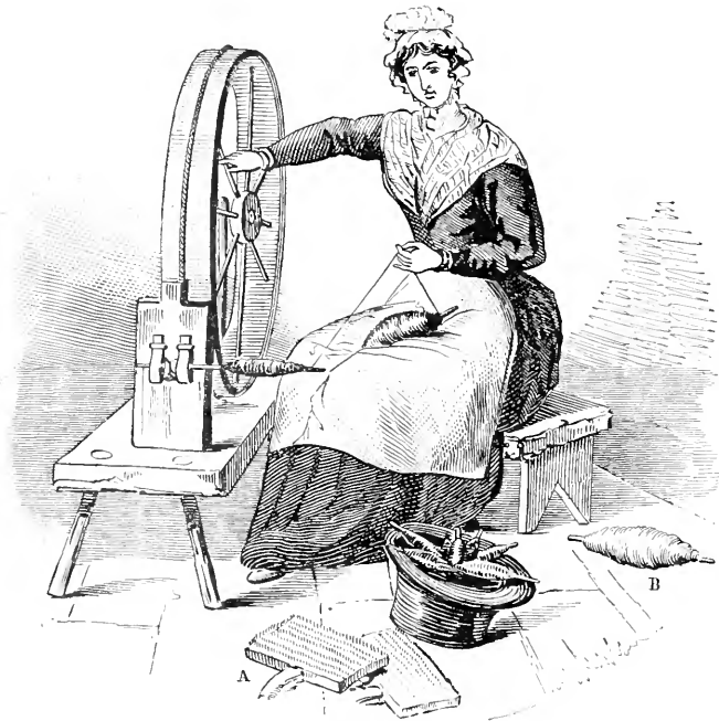
FIG. 10.—A WOOL SPINNING-WHEEL. A, hand-cards; B, bobbin of roving.
