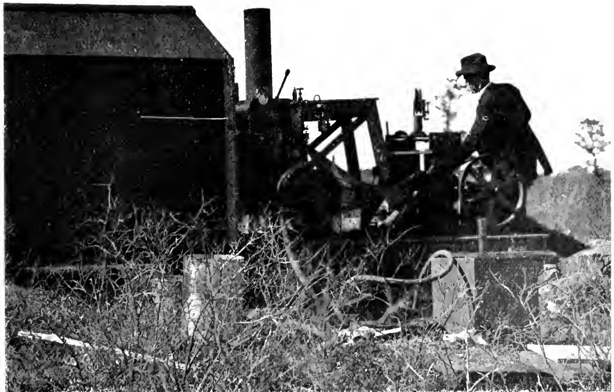
KITE REEL, OPERATED BY STEAM ENGINE.
