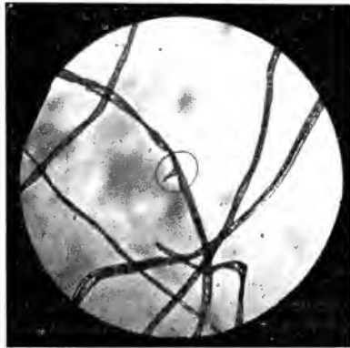
FIG. 12. COTTON FIBER INJURED IN THE PROCESS OF GINNING. \times 40 DIAMETERS.
