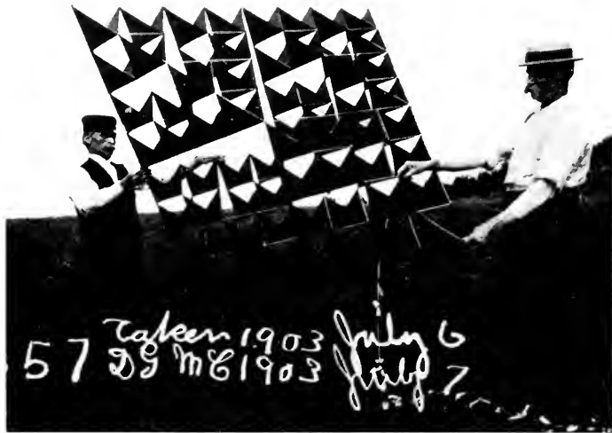
FIG. 6. SIXTY-FOUR CELLED KITE COMPOSED OF FOUR OF PRECEDING. 'RED FLIER.'
