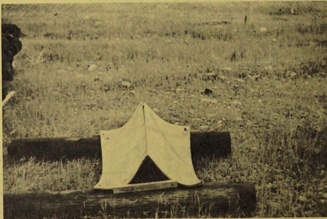
Figure 3 - After three years in the field this station is typical of wood and masonite construction.
