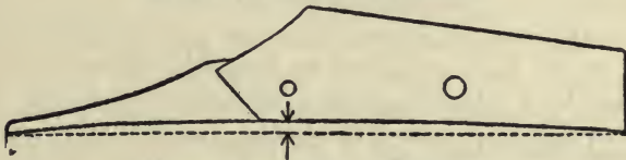
Suction of the plow—downward.
