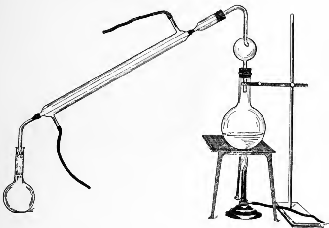
FIG. 28.—Apparatus for determining the Reichert-Meissl value of fats.
