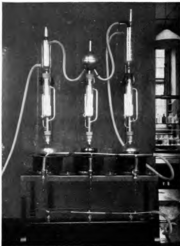
FIG. 6.—Battery of extraction apparatus, showing different types of condensers.
