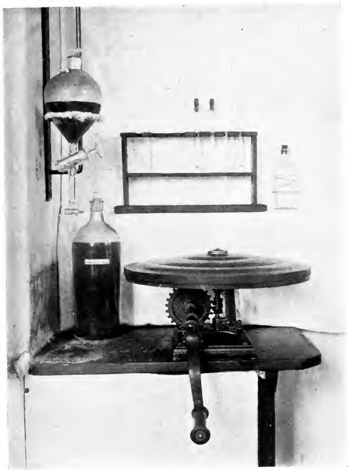
FIG. 26.—Apparatus used in the estimation of milk-fat by Gerber's process.
