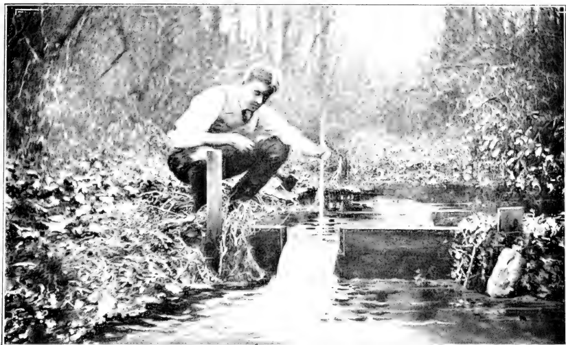
"IN MEASURING THE FLOW OF LARGE STREAMS A WEIR GAGE BOARD IS USED"
