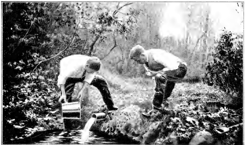
"AN EASY WAY OF MEASURING THE FLOW OF WATER IS TO DAM UP THE STREAM"
